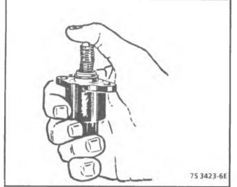
Figure 4-41 - Adjusting Valve Pintle - TBI 700
