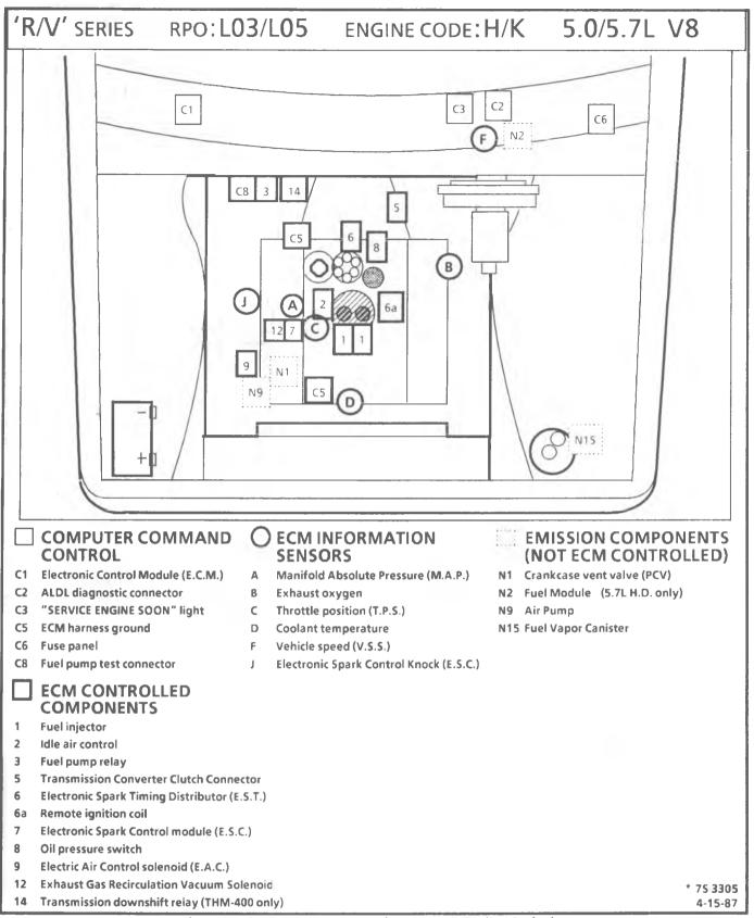
Figure 1-12 - Component Locations 5.0L/5.7L (RV Series)
