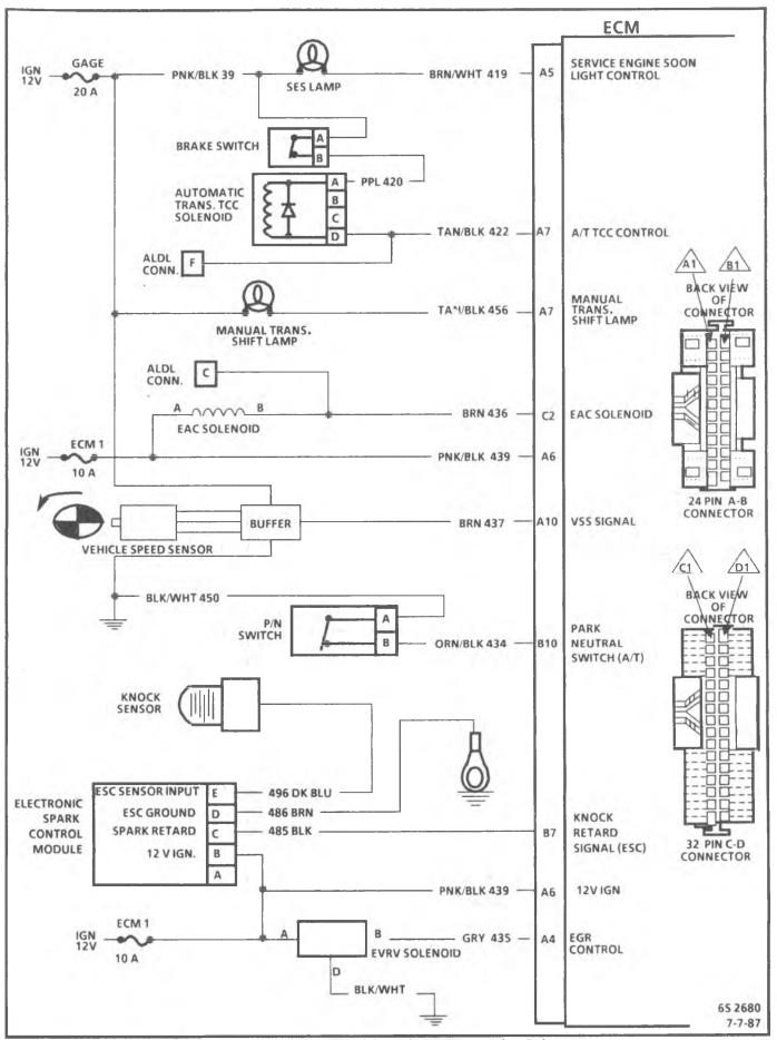
Figure 3-28 - ECM Wiring Diagram - 2.8L (3 of 3)
