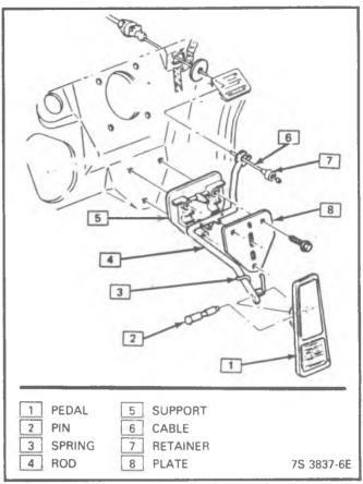
Figure 4-87 - Accelerator Pedal - M
