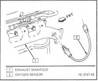
Figure 3-60 - Oxygen Sensor - 7.4L (CK)
