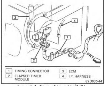
Figure 6-4 - Timing Connector (2.8L)
