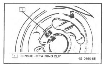
Figure 12-7 - Replacing THERMAC Sensor - S/T Series
