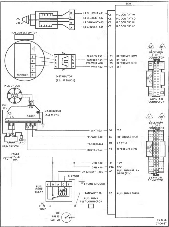
Figure 3-24 - ECM Wiring Diagram - 2.5L (2 of 3)
