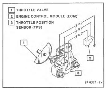
Figure 4-11 - Throttle Position Sensor (TBI 220)
