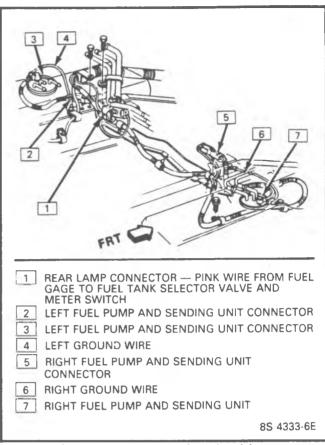
Figure 3 - 15 Two Fuel Tank Wiring
