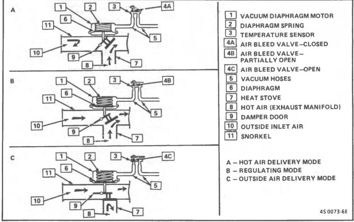
Figure 12-4 - THERMAC Operation - S/T Series
