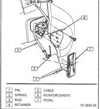
Figure 4-90 - Accelerator Pedal - G
