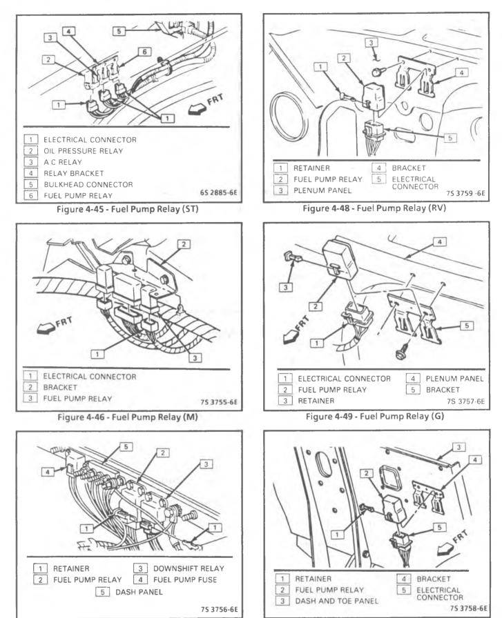
Figure 4-47 - Fuel Pump Relay (CK)
