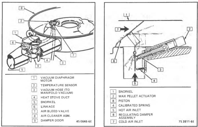
Figure 12-2 - THERMAC Air Cleaner - S/T Series
