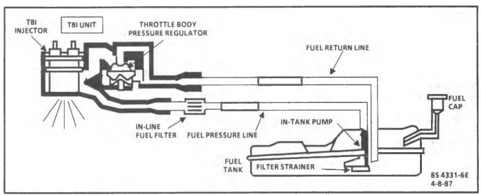
Figure 4-13 TBI Fuel Supply System (Typical)
