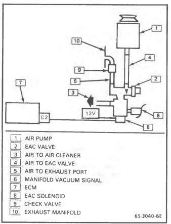
Figure 8-1 - AIR System - 2.8L
