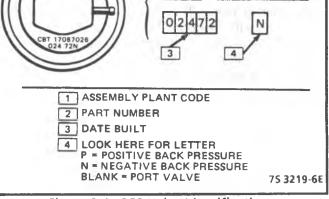
Figure 9-4 - EGR Valve Identification
