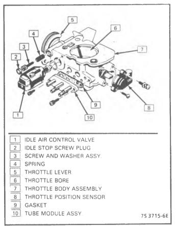
Figure 4-43 - Throttle Body Assembly
