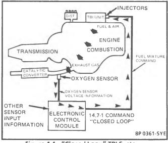
Figure 4-1 - "Closed Loop" TBI System
