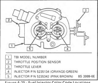
Figure 4-25 - Fuel Injector Color Code Locations TBI 220 (4.3L Engine)
