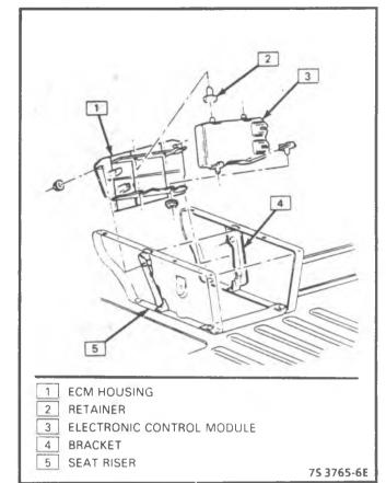
Figure 3-41 - Electronic Control Module (G)
