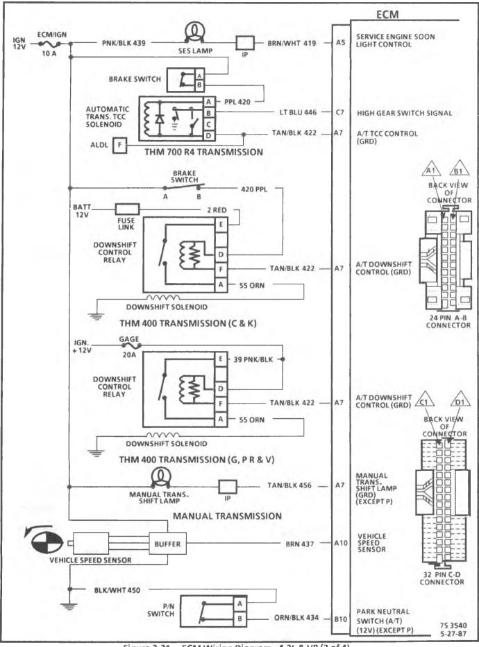
Figure 3-31 - ECM Wiring Diagram - 4.3L & V8 (3 of 4)
