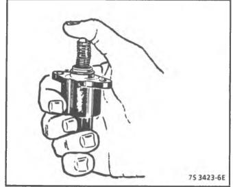
Figure 4-33 - Adjusting Valve Pintle - Flange Type
