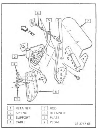
Figure 4-85 - Control Cable - 2.5L
