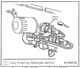
Figure 4-55 - Oil Pressure Switch (2.8L)
