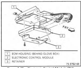
Figure 3-42 - Electronic Control Module (RV)
