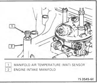
Figure 3-11 Manifold Air Temperature Sensor - L4
