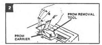
3. Inspect reference end of the PROM carrier and carefully set aside. Do not remove PROM from the carrier to confirm PROM correctness. Notch in PROM referenced to smaller notch in carrier and the 1.
