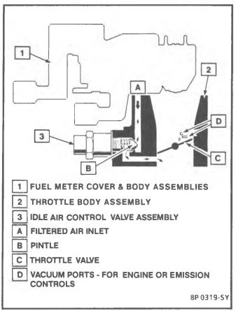
Figure 4-7 - Idle Air Control System (TBI 220 Unit)
