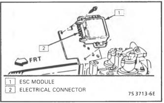
Figure 7-5 - ESC Module - CK RV MP Series
