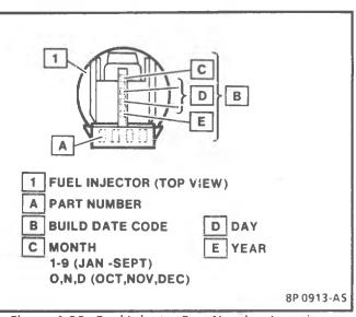
Figure 4-36 - Fuel Injector Part Number Location TBI 700
