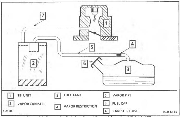
Figure 5-5 Evaporative Emissions Control System Schematic - 2.5L & 4.3L (ST)
