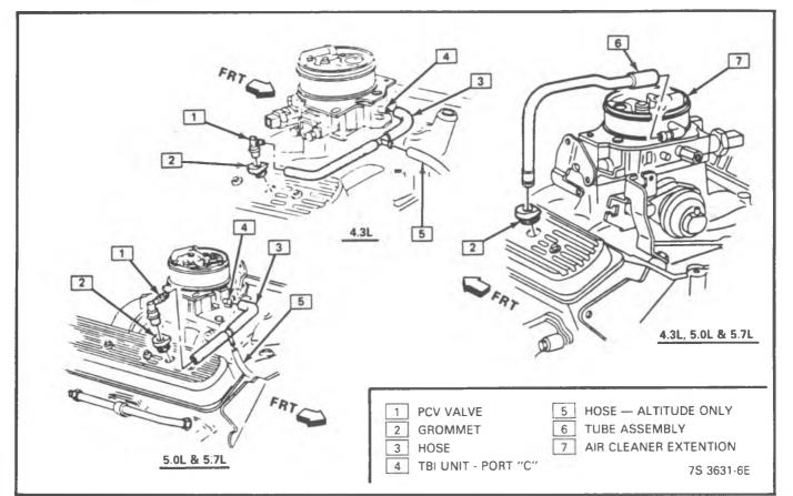
Figure 11-7 - PCV System (4.3L, 5.0L & 5.7L)
