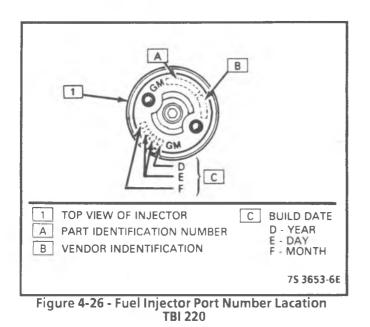
Be sure to replace the injector with one having an identical part number. Injectors from other models can also fit in TBI model 220, but are calibrated for different flow rates. (See Figure 4-26 for part number location).
