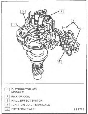
Figure 6-3 - Distributor (2.5L S/T Truck)
