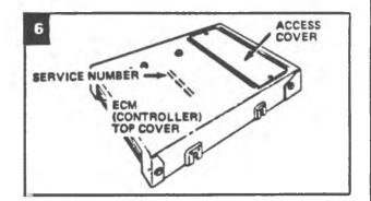
Install PROM and CALPAK (if used). If a service PROM or CALPAK is being installed, make sure they have the same part number as the removed PROM or CALPAK.
