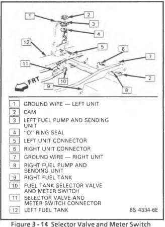
Figure 3 - 14 Selector Valve and Meter Switch Connector
