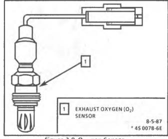
Figure 3-8 Oxygen Sensor
