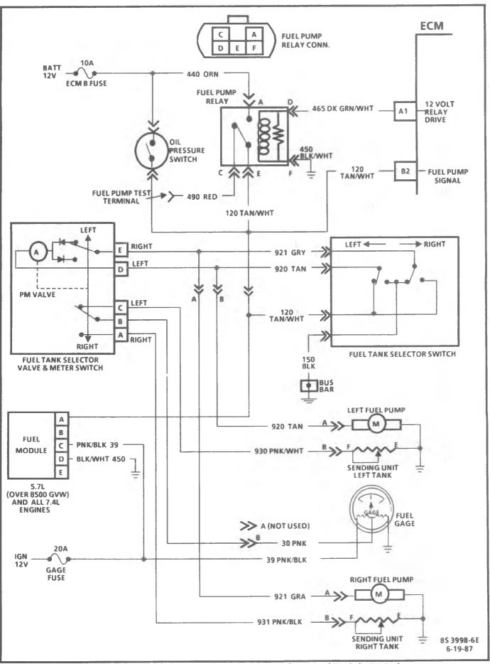
CHART A-5A, Fuel Pump Relay Circuit Diagnosis - (Two Fuel Tanks) - RV Series
