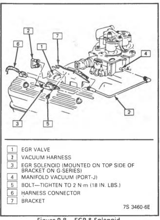
Figure 9-8 - EGR & Solenoid (5.0L & 5.7L under 8500 GVW)
