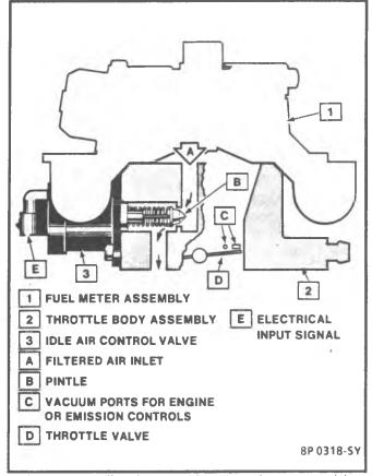
Figure 4-8 - Idle Air Control SYstem (TBI 700 Unit)
