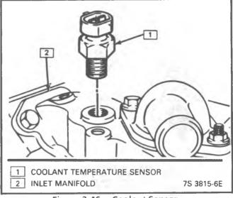
Figure 3-46 - Coolant Sensor
