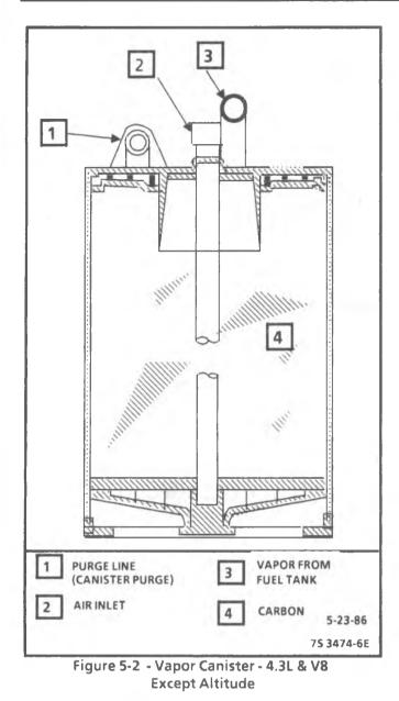
TBI unit. When the engine is below  $46^{\circ}$  C (115° F), the TVS is closed preventing purge of the canister. When engine temperature is above  $46^{\circ}$  C (115° F), the TVS opens, allowing purge of the canister.
