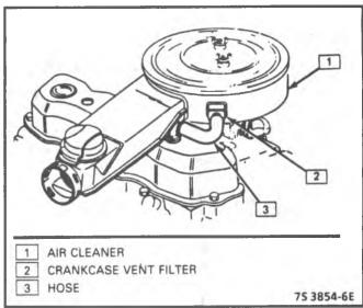
Figure 11-4 - Crankcase Vent Filter
