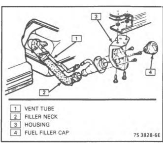
Figure 4-72 - Filler Neck - RV Chassis Cab
