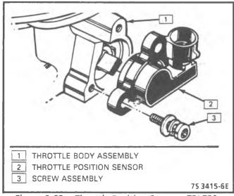
Figure 3-62 - Throttle Position Sensor - TBI 700
