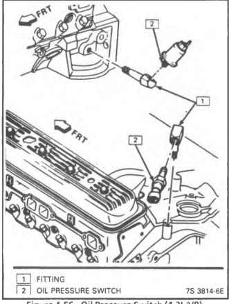
Figure 4-56 - Oil Pressure Switch (4.3L/V8)
