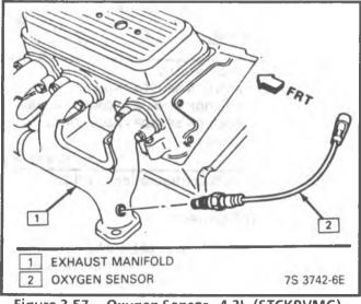
Figure 3-57 - Oxygen Sensor - 4.3L (STCKRVMG)
