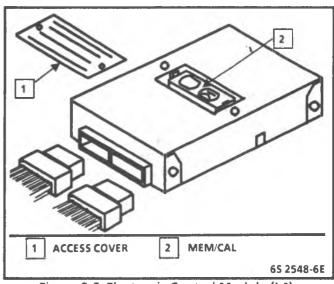
Figure 3-3 Electronic Control Module (L4)
