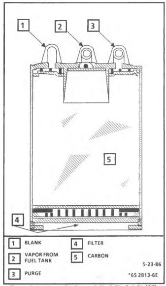
Figure 5-1 - Vapor Canister - 2.5L, 2.8L & 4.3L (ST)
