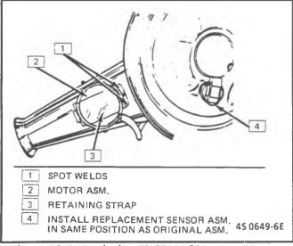
Figure 12-5 - Replacing THERMAC Vacuum Motor **S/T Series**
