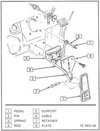
Figure 4-88 - Accelerator Pedal - RV
