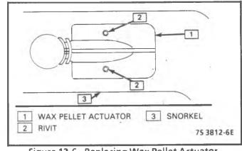
Figure 12-6 - Replacing Wax Pellet Actuator All except S/T Series
