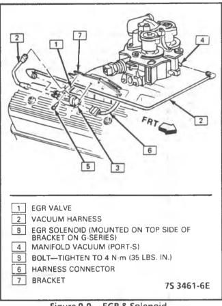
Figure 9-9 - EGR & Solenoid (4.3L (ST) & 5.7L over 8500 GVW)
