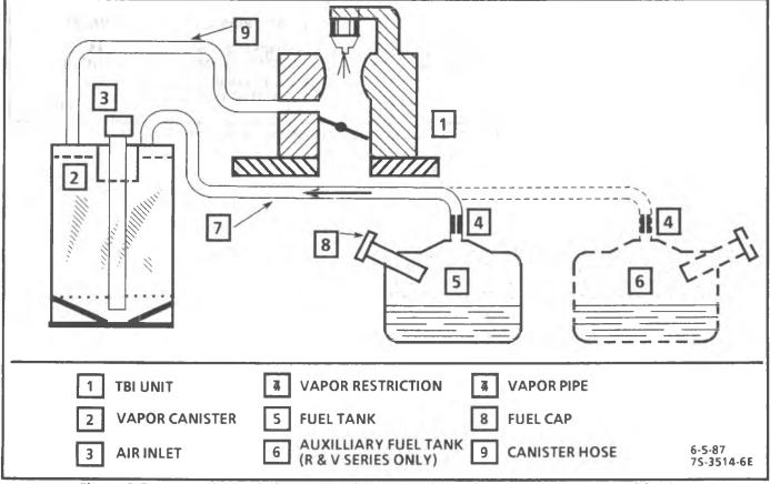
Figure 5-7 Evaporative Emissions Control System Schematic - 4.3L & V8 - Except Altitude
