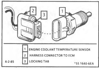
Figure 3-6 Coolant Temperature Sensor
