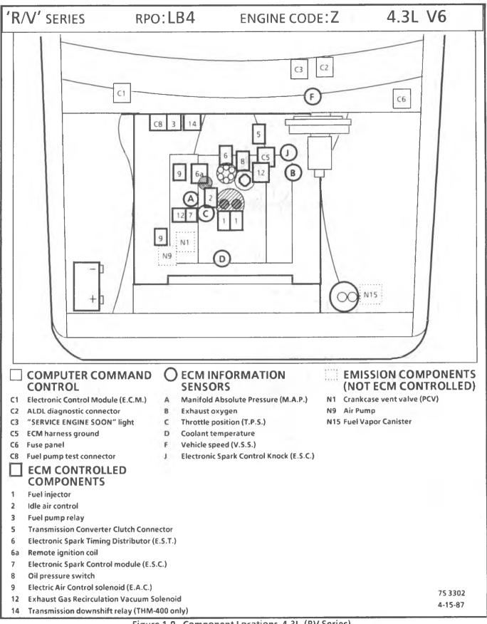
Figure 1-9 - Component Locations 4.3L (RV Series)
