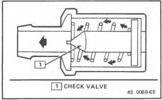
Figure 11-3 - PCV Valve Cross Section
