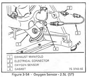
New, or service sensors will already have the compound applied to the threads. If a sensor is removed from an engine, and if for any reason it is to be reinstalled, the threads must have anti-seize
