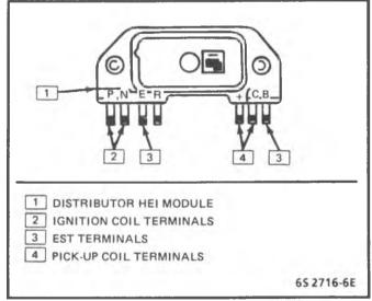
Figure 6-2 - Module (2.5L S/T Truck)
