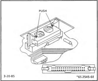
Figure 3-39 - Mem/Cal Unit Installation
