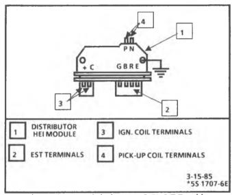
Figure 6-1 - Module (Except 2.5L S/T Truck)
