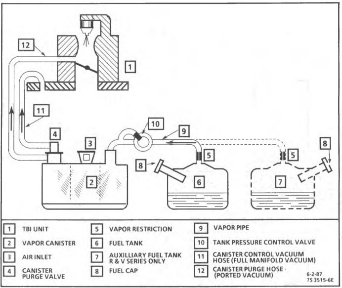
Figure 5-8 Evaporative Emissions Control System Schematic - 4.3L & V8 - Altitude
