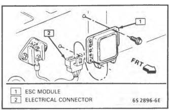
Figure 7-4 - ESC Module - ST Series
