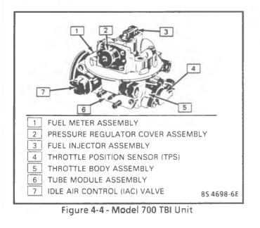
The fuel which is not used by the injectors passes through the pressure regulator before being returned to the fuel tank.
