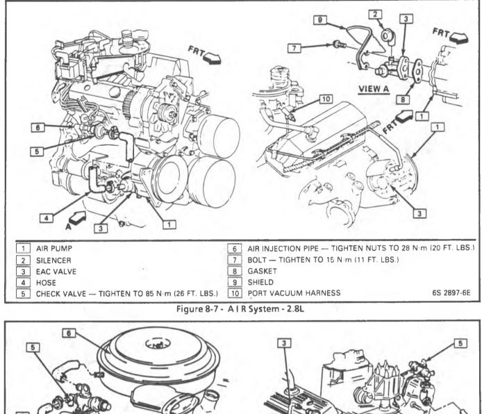
4 3 2 7 1 **AIR PUMP** 5 DIVERTER VALVE OR EAC VALVE 1 ADAPTER AND SEAL - TIGHTEN SCREWS TO 25 N·m (18 FT. LBS.) 2 6 AIR CLEANER AIR INJECTION PIPE - TIGHTEN NUTS TO 28 N·m (20 FT. LBS.) 3 7 BOLT - TIGHTEN TO 34 N·m (25 FT. LBS.) 8 NUT-TIGHTEN TO 34 N·m (25 FT. LBS.) 75 3309-6E 4 CHECK VALVE - TIGHTEN TO 25 N·m (18 FT. LBS.)
