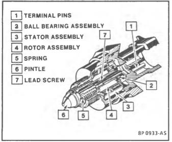
Figure 4-9 - Idle Air Control (IAC) Valve (TBI 220)
