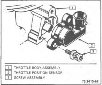
Figure 3-10 Throttle Position Sensor - L4
