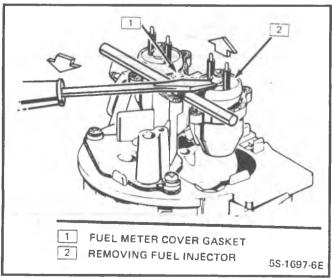
Figure 4-24 - Removing TBI 220 Fuel Injector
