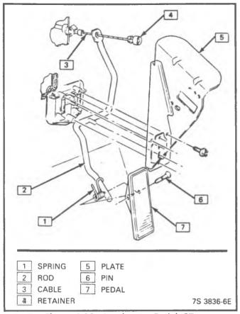
Figure 4-86 - Accelerator Pedal -ST
