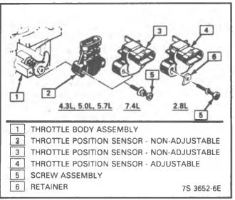
Figure 3-9 Throttle Position Sensor - V6/V8
