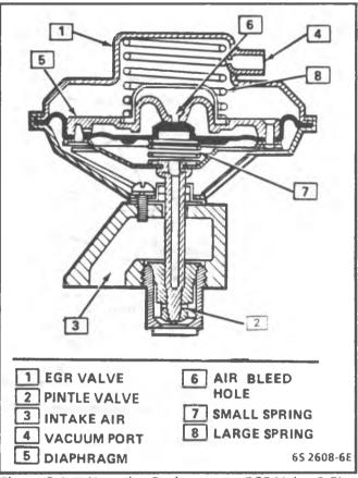
Figure 9-1 - Negative Backpressure EGR Valve 2.5L, 4.3L (except ST), 5.0L& 5.7L (under 8500 GVW)
