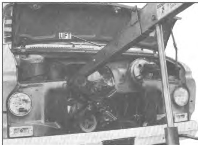
Fig. 4L—Lifting Device Installed to J-24680-2
