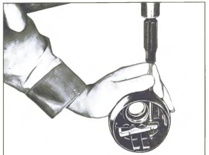
Fig. 94—Removing Release Lever Pivot Pin
