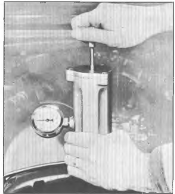
Fig. 20—Cooling System Pressure Check
