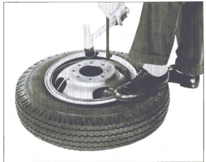
Fig. 13—Forcing Ring into Gutter
