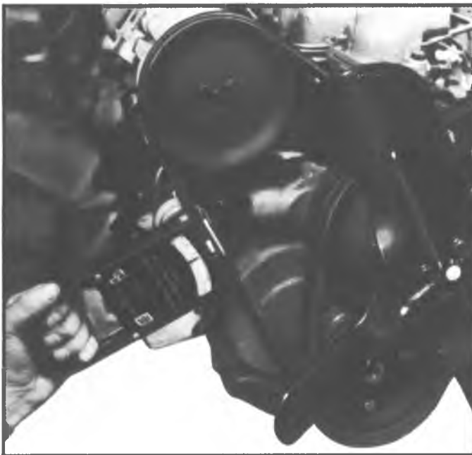
Fig. 13f—Checking A.I.R. Pump Belt Tension
