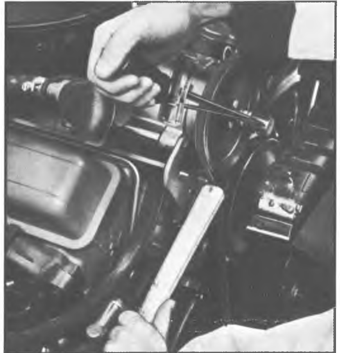
Fig. 14f—Tightening Pump Pulley Bolts
