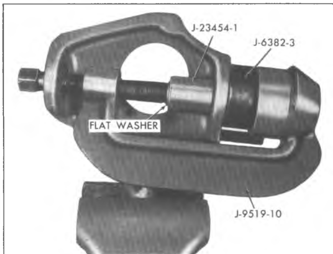
Fig. 64—Removing Upper Ball Joint
