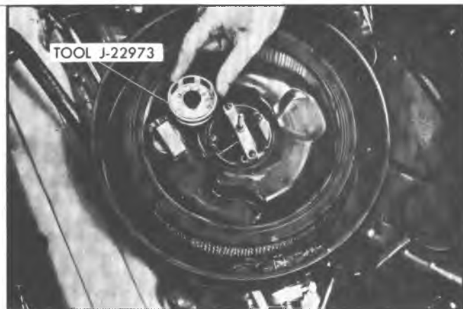
Fig. 12A--Temperature Gauge Installation
