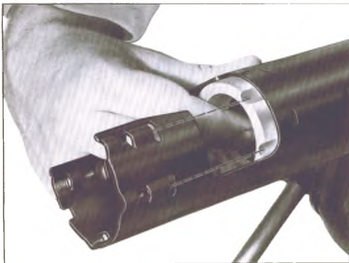
Fig. 71—Installing Gearshift Housing Lower Bearing
