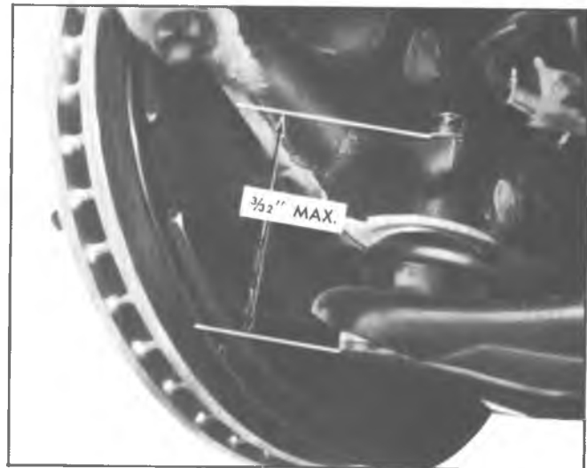
Fig. 35—Checking Lower Ball Joint
