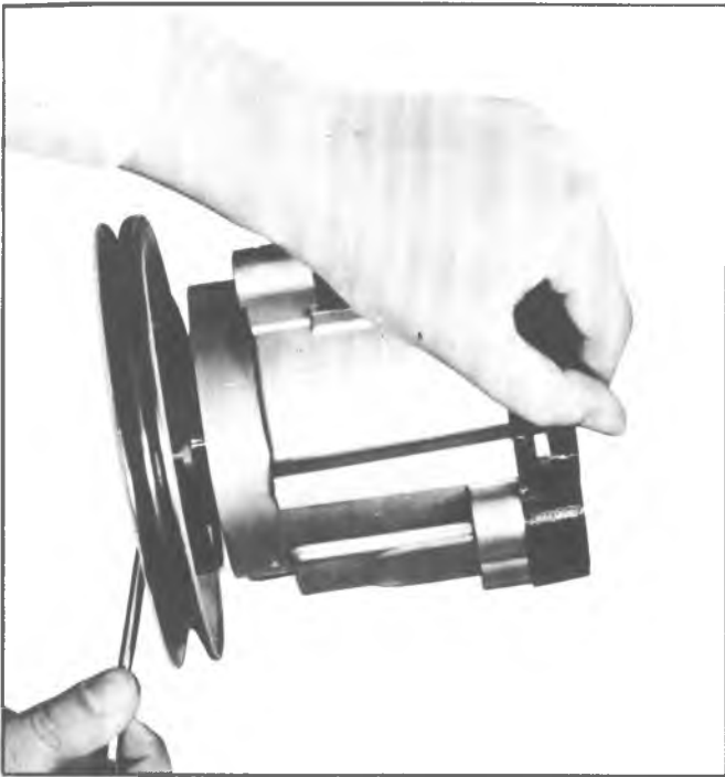
Fig. 16f—Installing Centrifugal Filter
