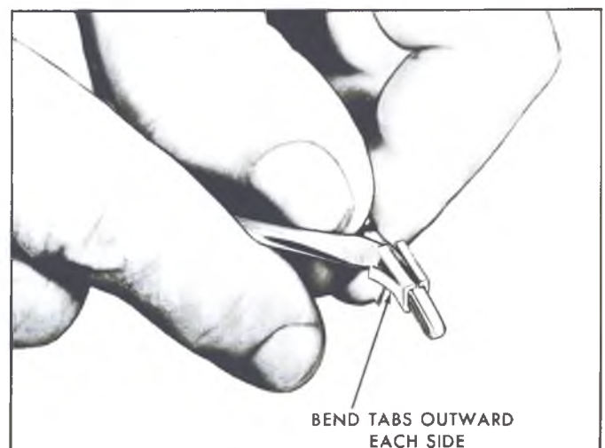
Fig. 86—Preparing Wire Retaining Tabs for Installation
