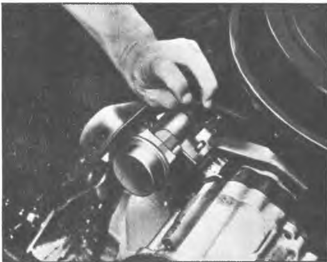
Fig. 22f—Checking for Vacuum Signal at Diverter Valve
