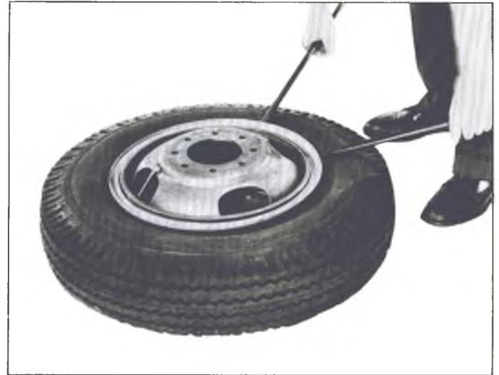
Fig. 5—Loosening First Bead
