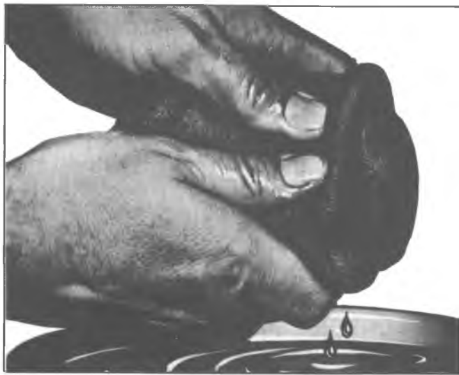
Fig. 8A—Cleaning the Polyurethane Band
