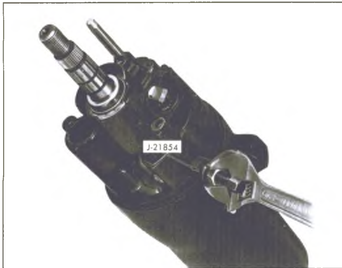
Fig. 75—Removing Bearing Housing Pivot Pins
