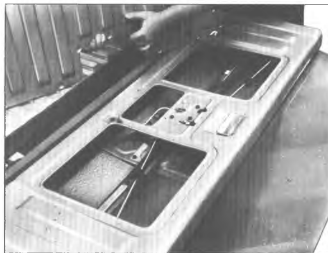
Fig. 58—Removing Access Cover (14)
