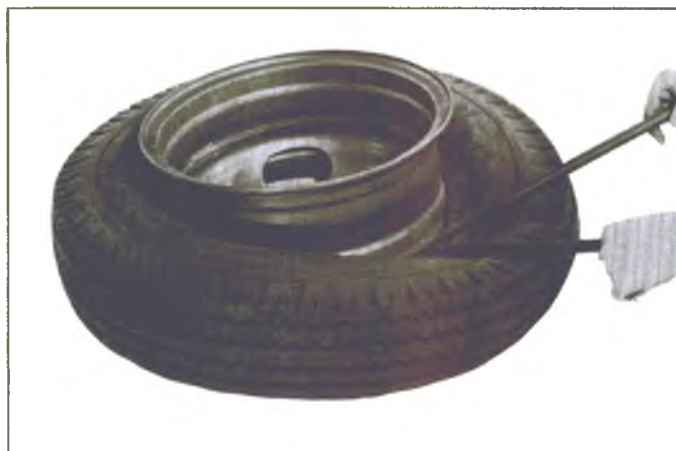
Fig. 9—Prying Second Bead From Rim
