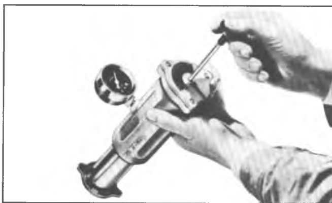
Fig. 10—Pressure Checking Radiator Cap
