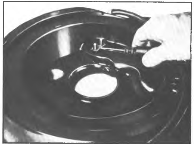
Fig. 15A--Removing Sensor Unit
