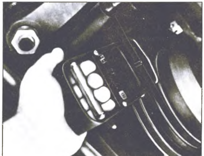
Fig. 40—Checking Belt Tension with J-23600
