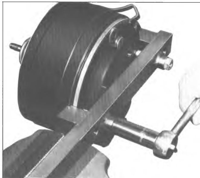
Fig. 24—Removing Shell Assembly
