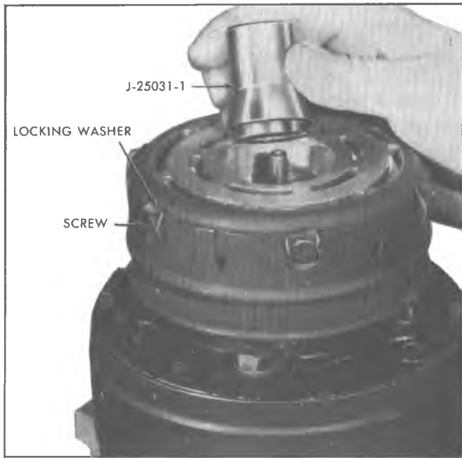
Fig. 11—Installing Rotor and Bearing Puller Guide
