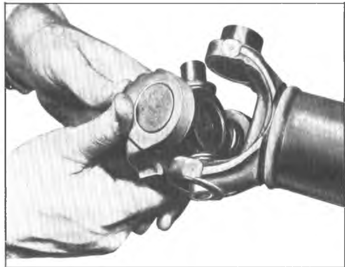
Fig. 4—Installing Trunnion into Yoke
