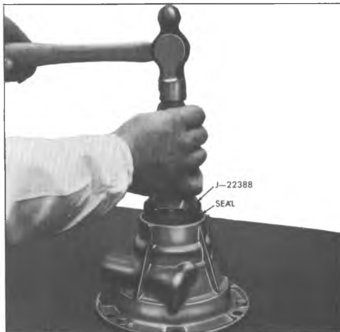
Fig. 7F—Installing Rear Output Housing Seal
