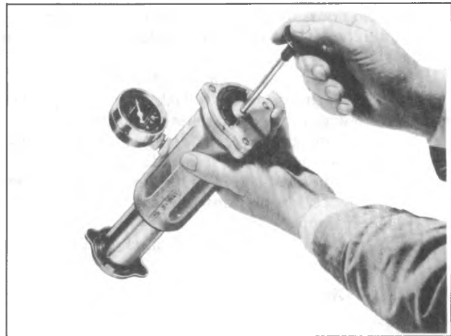
Fig. 6B-4--Pressure Checking Radiator Cap
