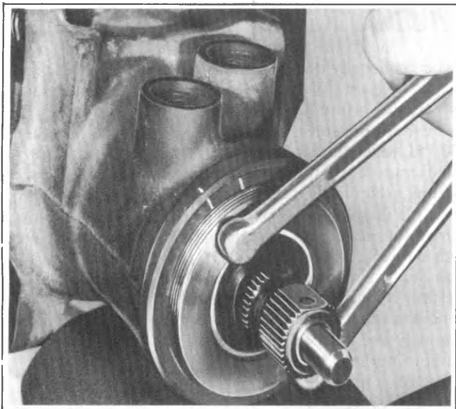
Fig. 3B-40--Align Hole With Second Mark
