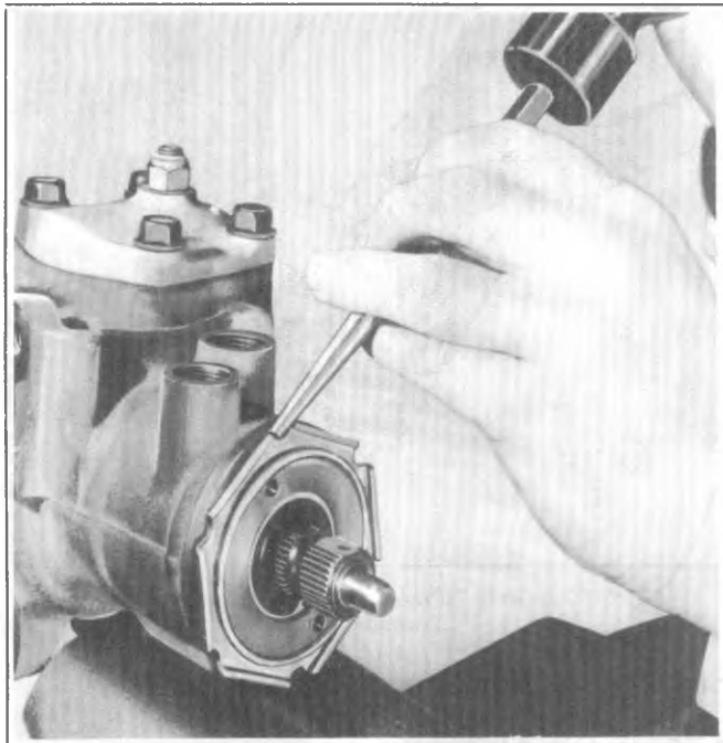
Fig. 3B-35--Loosening Lock Nut
