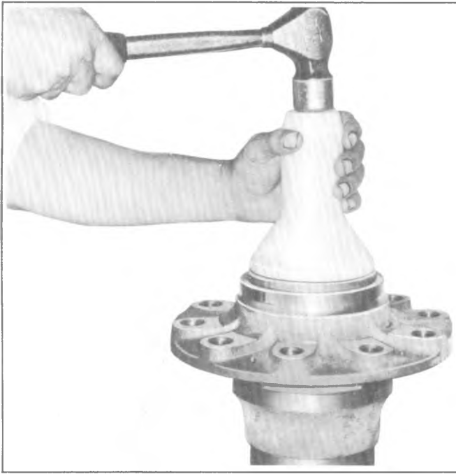
Fig. 4B-40--Installing Hub Oil Seal
