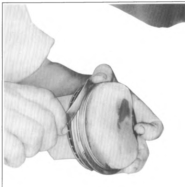
Fig. 6A1-44--Measuring Ring Groove Clearance
