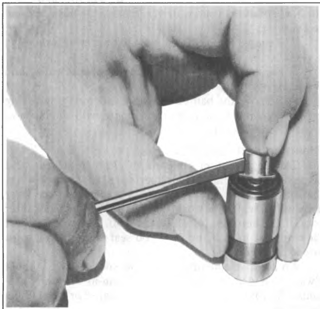
Fig. 6A1-13--Removing Ball Check Valve
