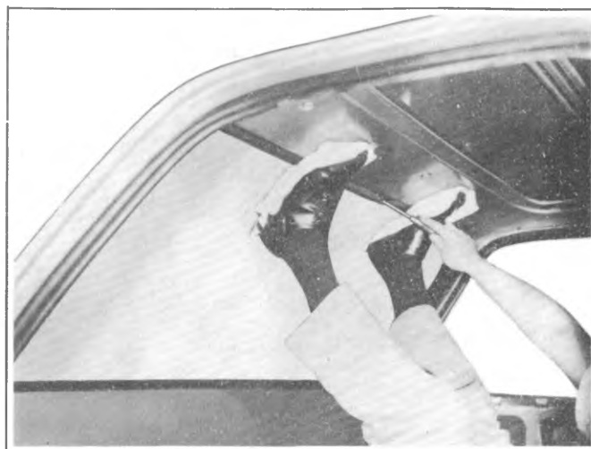
Fig. 2D-14--Applying Pressure to Windshield
