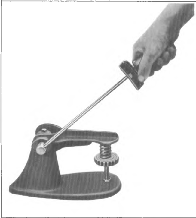
Fig. 6A2-25--Checking Valve Spring Tension
