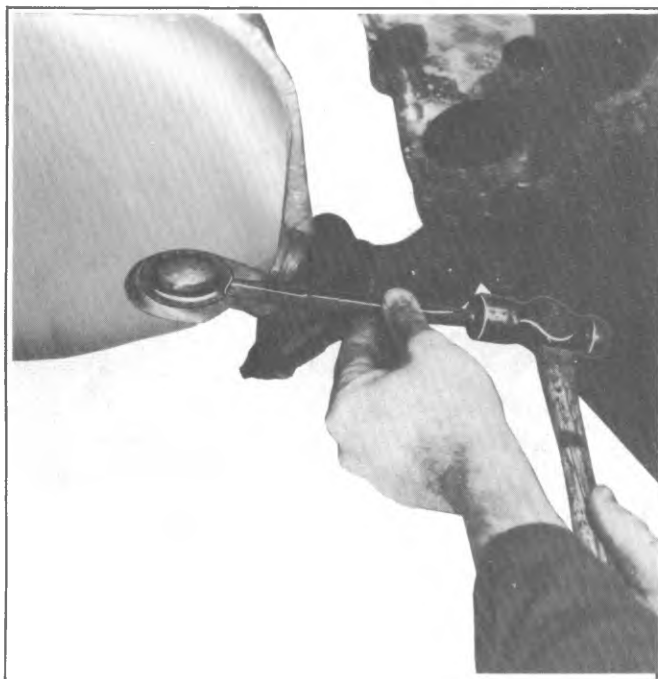
Fig. 6F-5--Removing Pressed Plug
