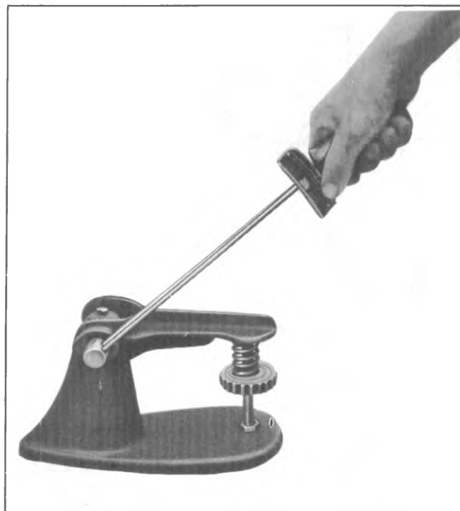
Fig. 6A1-16--Checking Valve Spring Tension
