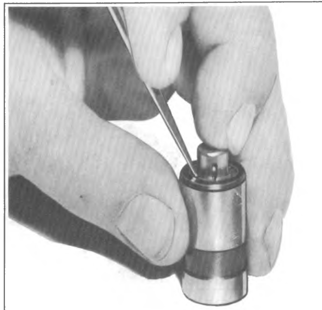
Fig. 6A1-14--Installing Ball Check Valve
