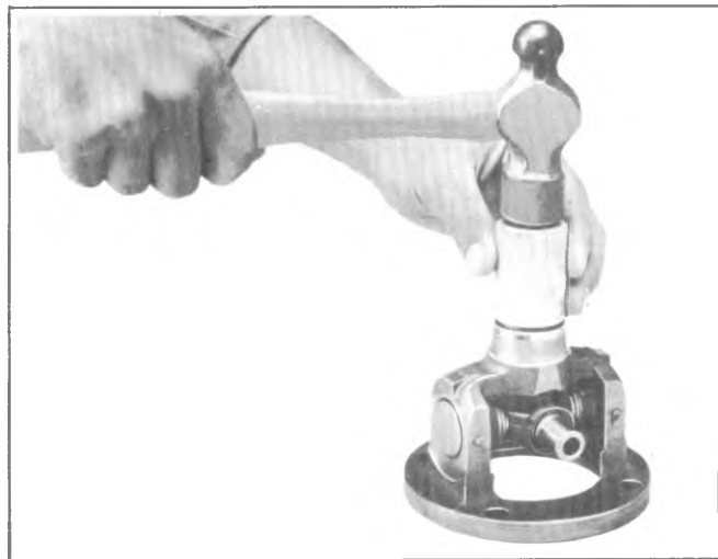
Fig. 4A-31--Installing Centering Ball Seal
