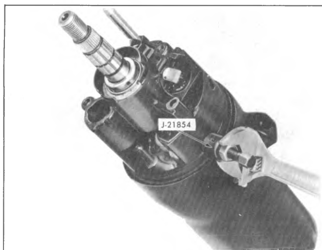
Fig. 3B-77--Removing Bearing Housing Pivot Pins
