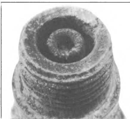
Insufficient Installation Torque
