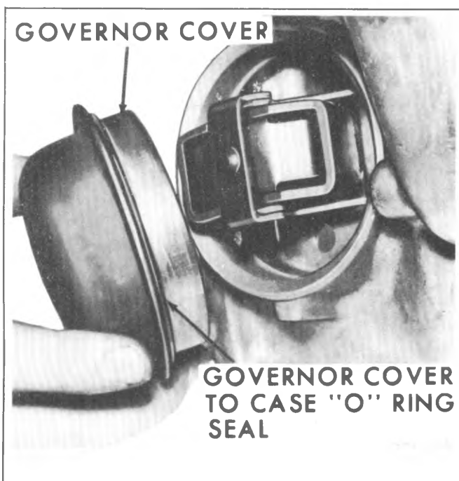
Fig. 7A-18--Governor Cover and O-Ring Seal
