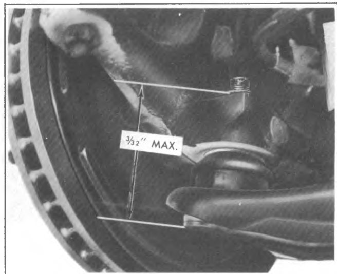
Fig. 3C-28--Checking Lower Ball Joint
