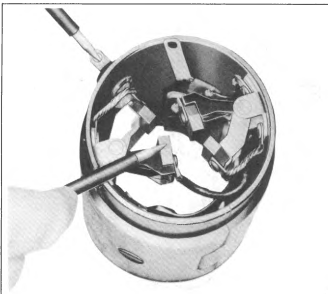
Fig. 6D-15s--Field Coil Open Circuit Test
