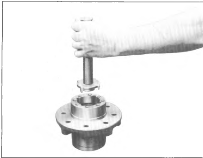
Fig. 4B-33--Removing Outer Bearing and Cup
