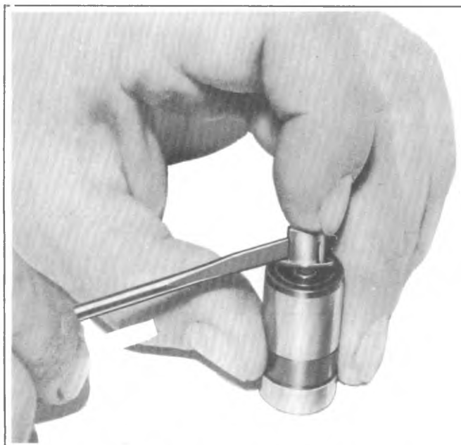
Fig. 6A2-18--Removing Ball Check Valve
