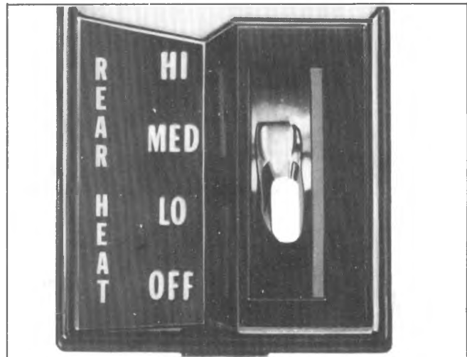
Fig. 1A-18--Auxiliary Heater Control
