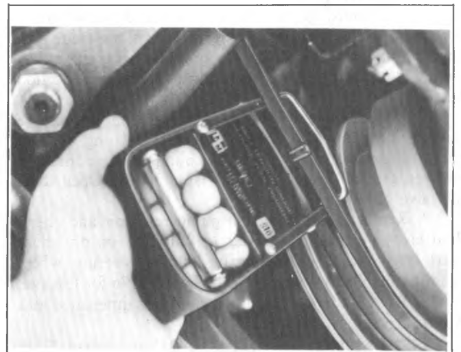
Fig. 3B-42--Checking Belt Tension with J-23600
