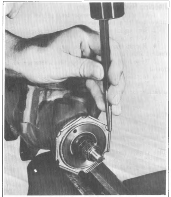
Fig. 3B-41--Tightening Lock Nut
