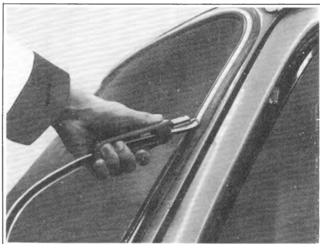
Fig. 2D-19--Installing Reveal Molding
