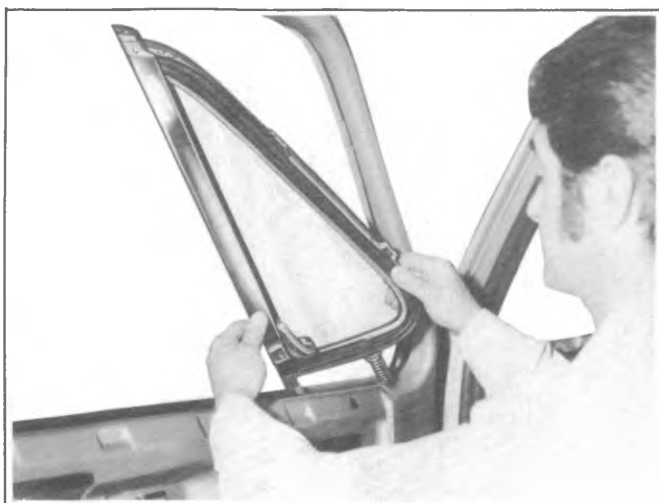
Fig. 2D-28--Removing Ventilator Assembly
