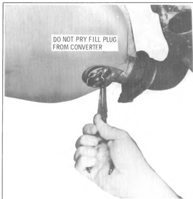
Fig. 6F-6--Removing Pressed Plug With Pliers
