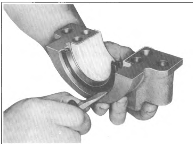
Fig. 6A2-60--Removing Oil Seal - Lower Half
