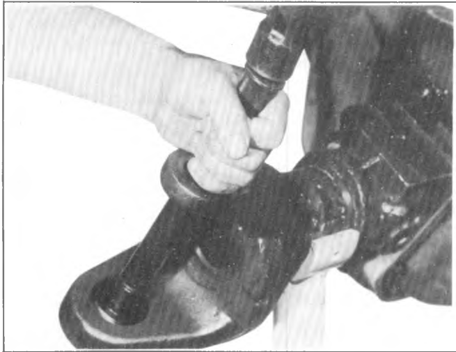
Fig. 3C-24K--Removing Cup, Cone and Seal
