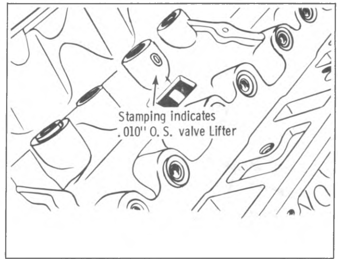
Fig. 6A3-34--O.S. Valve Lifter Identification
