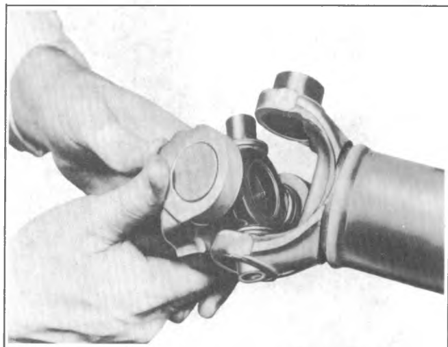
Fig. 4A-14--Installing Trunnion into Yoke
