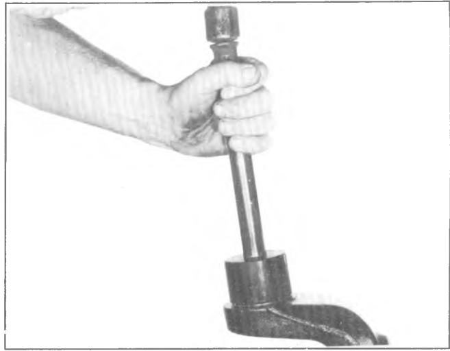
Fig. 3C-26K--Installing Oil Seal
