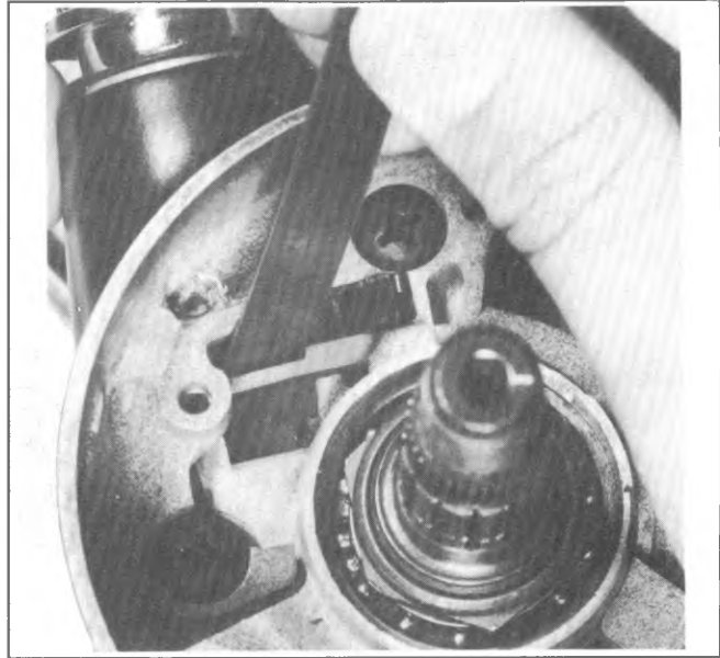
Fig. 3B-56--Lock Cylinder Removal
