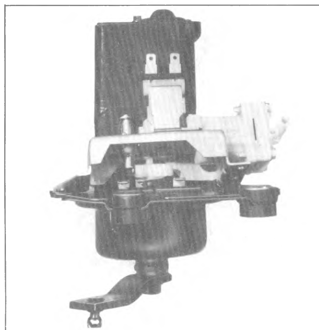
Fig. 8-31--Washer Pump Drive Cam and Actuator
