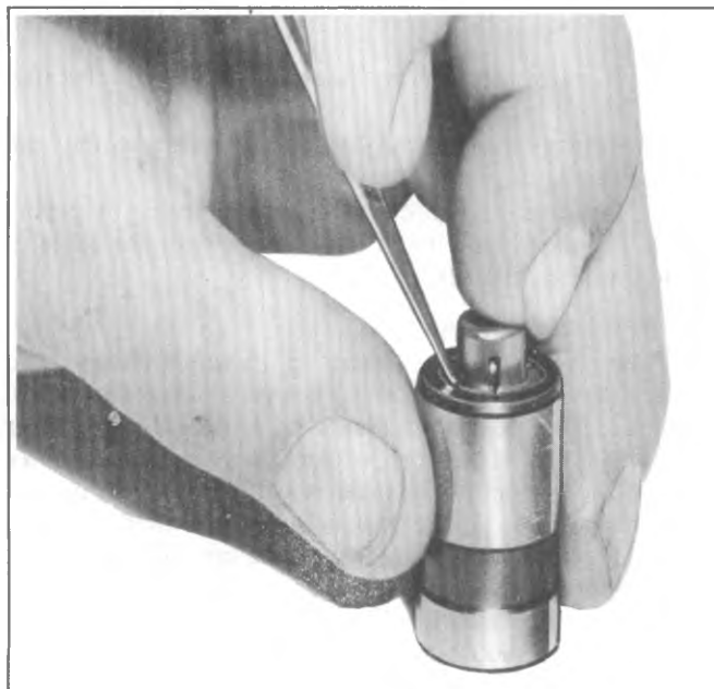
Fig. 6A2-19--Installing Ball Check Valve
