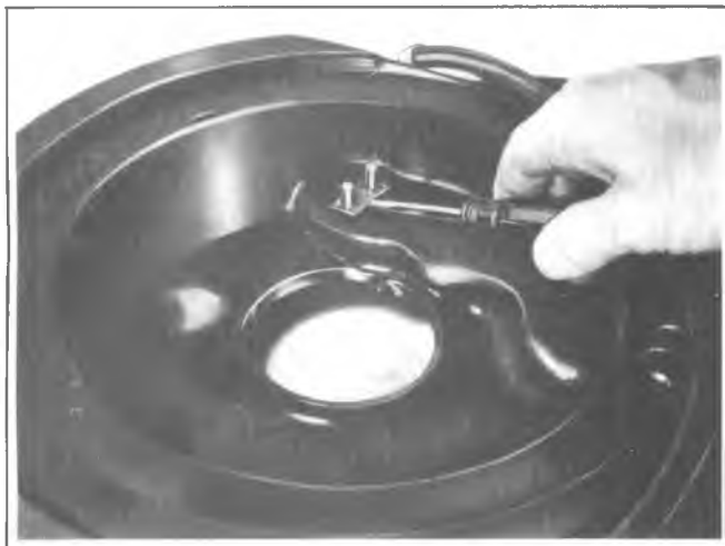
Fig. 6E-23-Removing Sensor Unit
