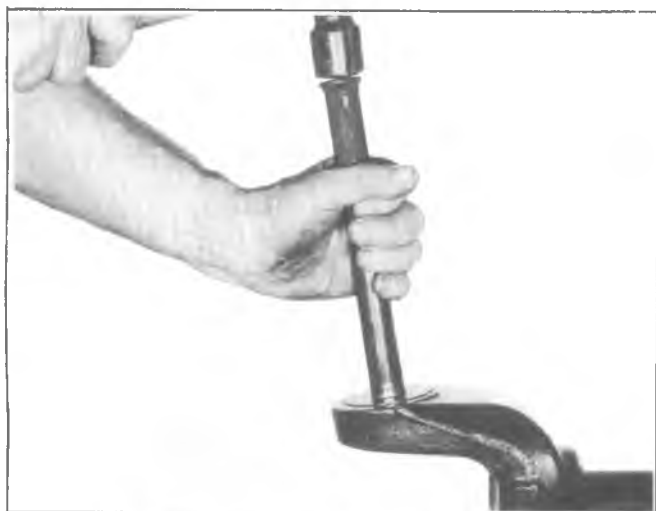
Fig. 3C-26K--Installing Grease Retainer
