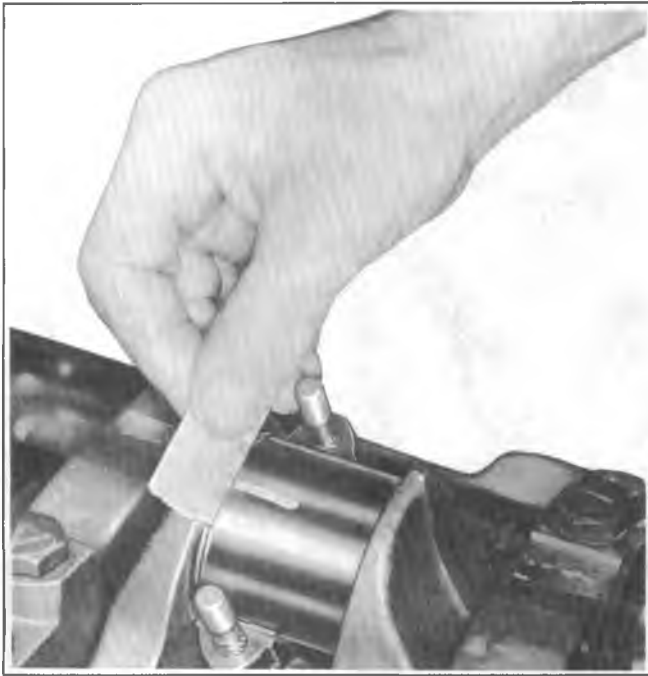
Fig. 6A5-42--Measuring Gaging Plastic
