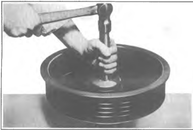
Fig. 4B-39--Installing Hub Inner Bearing Cup
