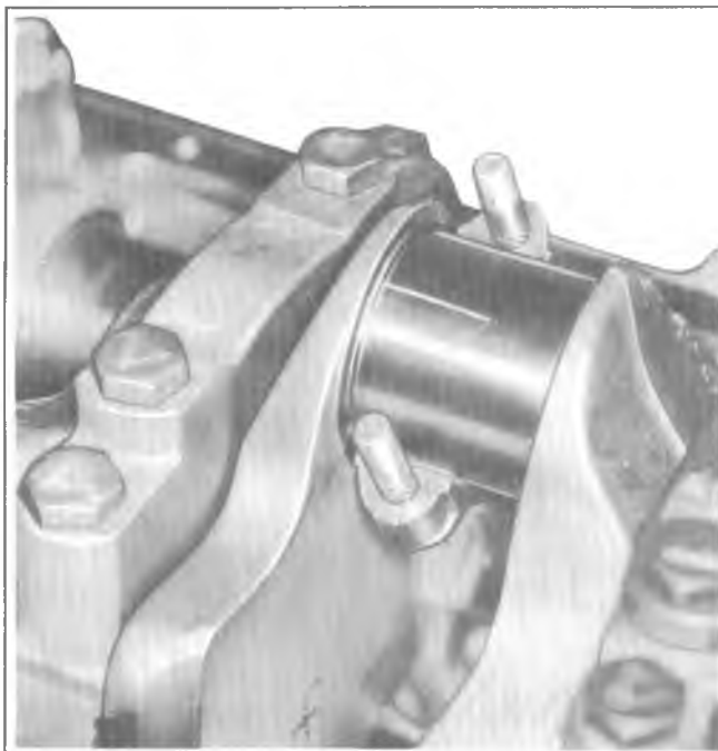
Fig. 6A1-27--Gaging Plastic on Crankpin
