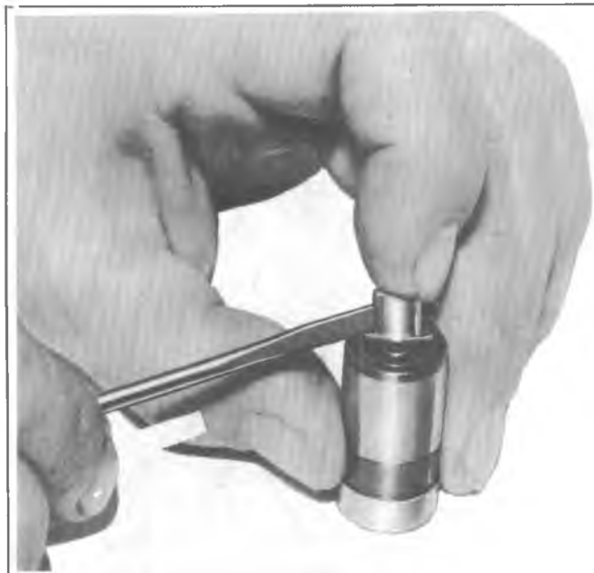
Fig. 6A4-15--Removing Ball Check Valve
