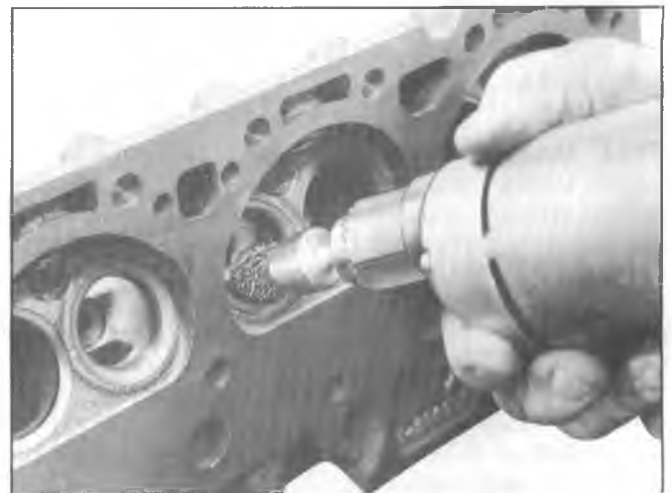
Fig. 6A4-19--Cleaning Combustion Chambers
