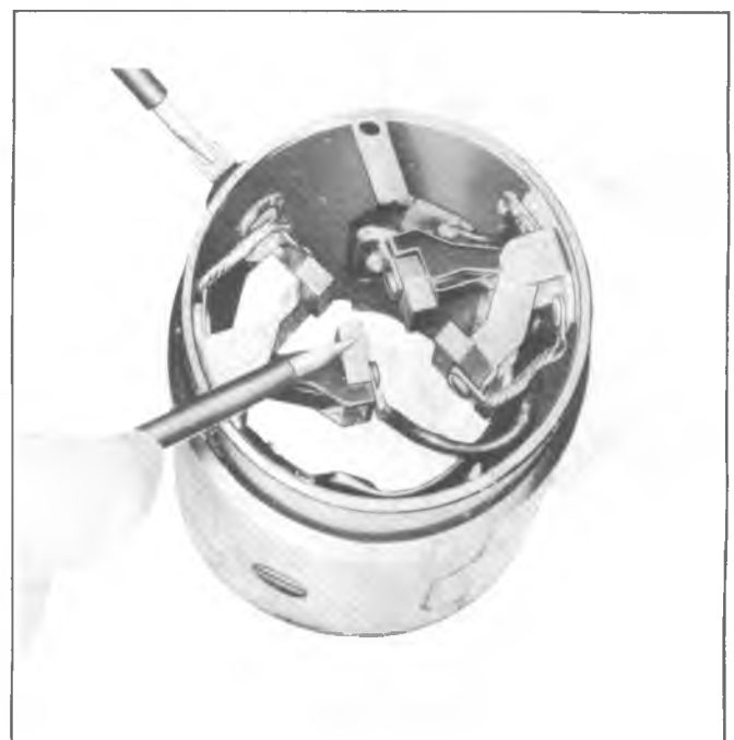
Fig. 6D-13E--Testing Field Coils for Open
