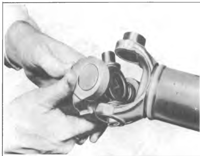
Fig. 4A-14--Installing Trunnion into Yoke
