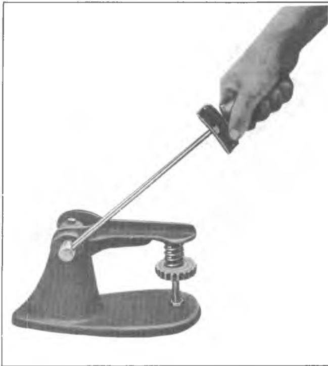
Fig. 6A1-16--Checking Valve Spring Tension
