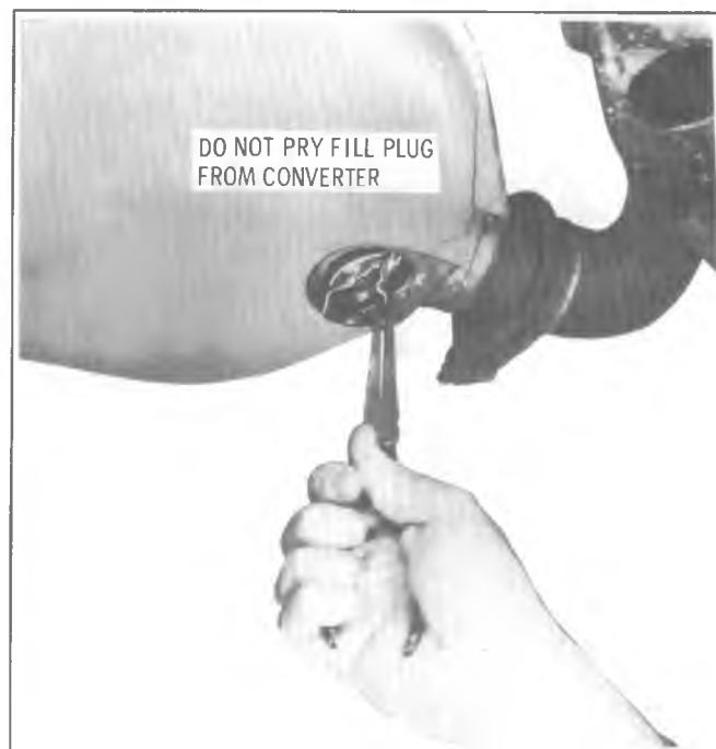
Fig. 6F-6--Removing Pressed Plug With Pliers
