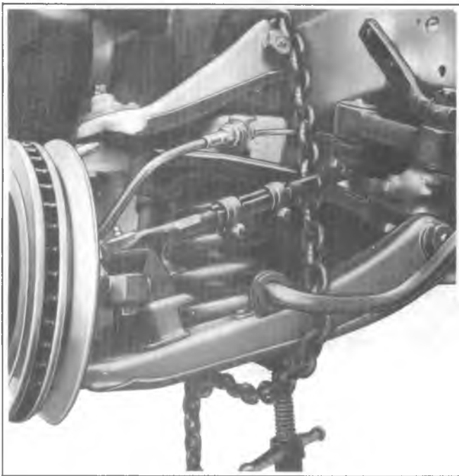
Fig. 3C-18--Removing Inner Pivot Shaft
