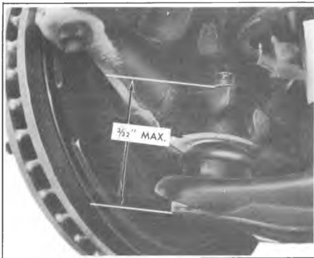
Fig. 3C-29—Checking Lower Ball Joint
