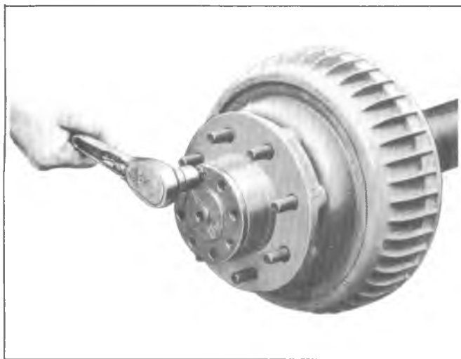
Fig. 4B-30—Removing Flange-to-Hub Bolts
