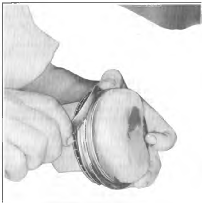
Fig. 6A1-43--Measuring Ring Groove Clearance
