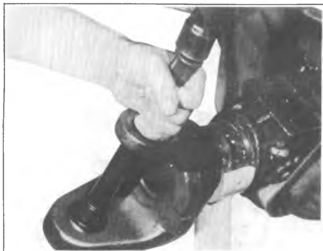
Fig. 3C-25K--Removing Cup, Cone and Seal
