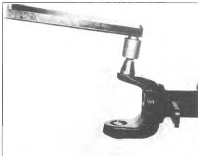
Fig. 3C-28K--Installing Upper King-Pin
