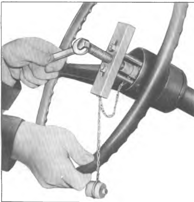
Fig. 3B4-59--Steering Wheel Removal-Typical
