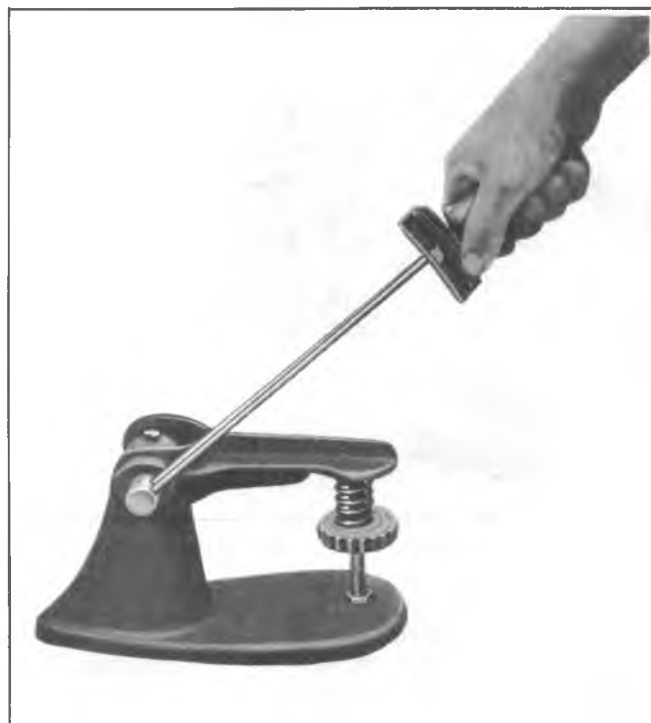
Fig. 6A5-22--Checking Valve Spring Tension
