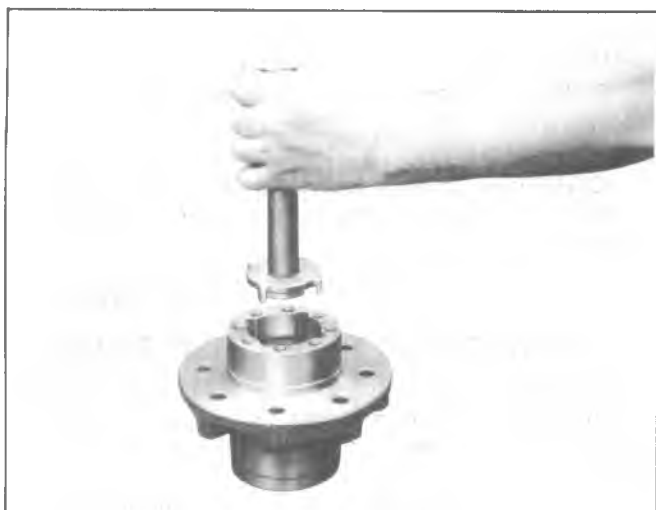
Fig. 4B-33--Removing Outer Bearing and Cup
