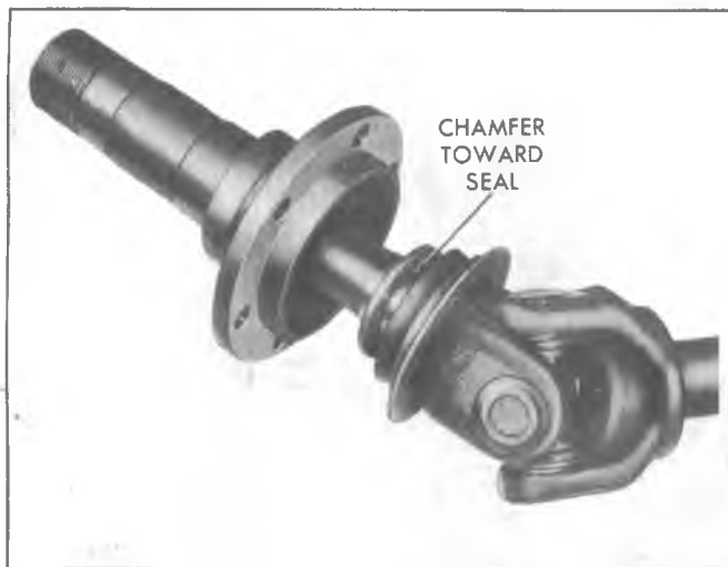
Fig. 3C-9K--Installing Spindle and Thrust Washer
