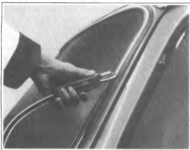
Fig. 2D-19--Installing Reveal Molding
