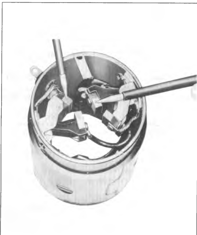
Fig. 6D-12E--Testing Field Coils for Ground
