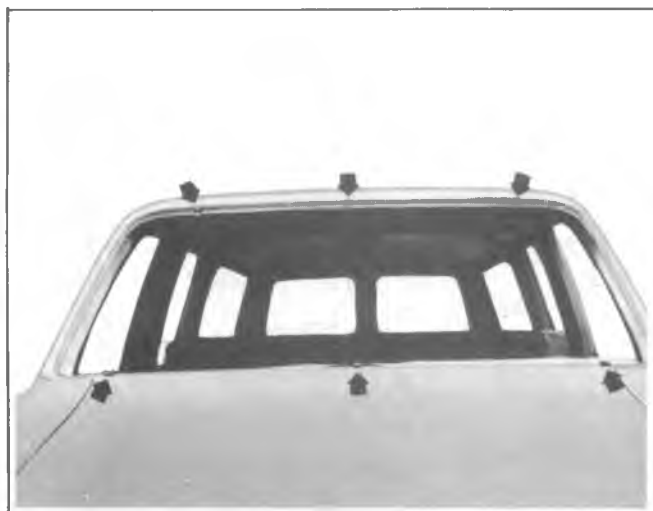
Fig. 2D-17--Checking Windshield Opening
