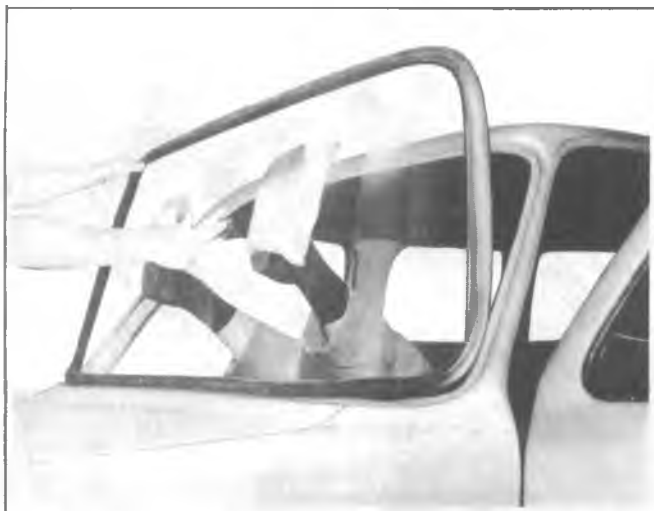
Fig. 2D-16--Removing Windshield from Opening
