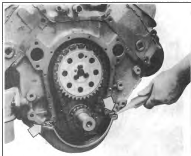
Fig. 6A5-33--Applying Front Cover Sealer
