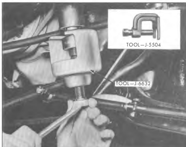
Fig. 3B2-9--Removing Pitman Arm-Typical
