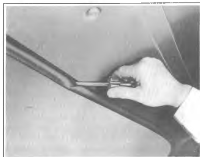
Fig. 2D-15--Assisting Weatherstrip over Flange
