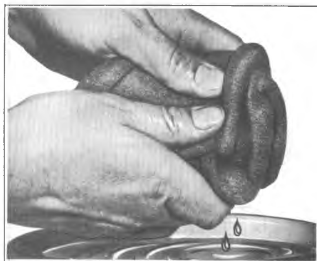
Fig. 6E-14-Cleaning Polywrap Band
