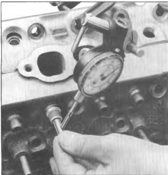
Fig. 6A4-20—Measuring Valve Stem Clearances
