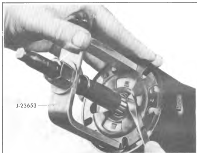
Fig. 3B4-26--Removing Lock Plate Retaining Ring
