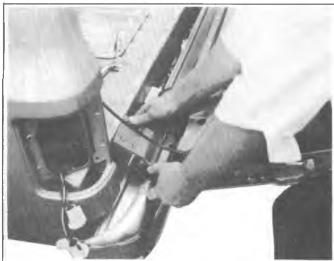
Fig. 2D-63--Pulling Hinge Away From Body (16)
