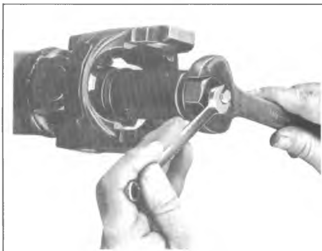
Fig. 4A-29--Removing Centering Ball
