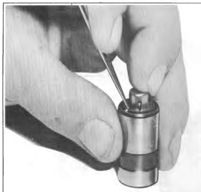
Fig. 6A5-16--Installing Ball Check Valve
