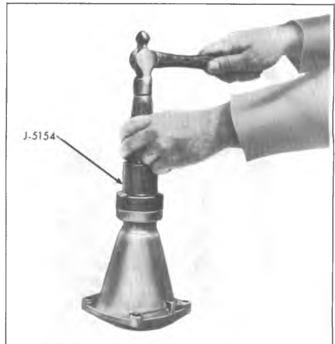
Fig. 7A-16—Installing Oil Seal into Extension Housing
