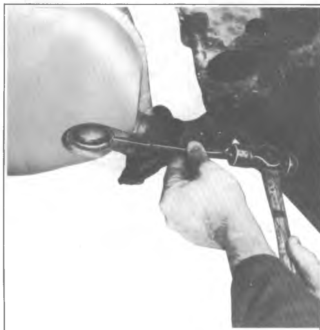
Fig. 6F-5--Removing Pressed Plug
