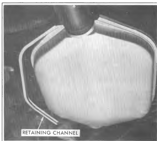
Fig. 6F-19--Installing Bottom Cover Retaining Channels
