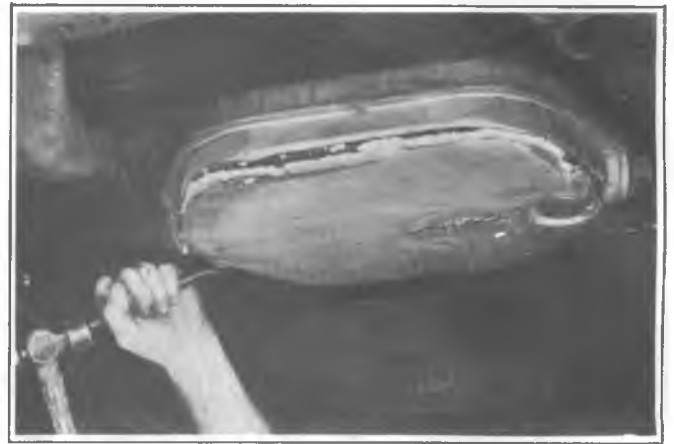
Fig. 6F-14--Removing Bottom Cover
