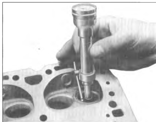
Fig. 6A4-29--Measuring Valve Seat Concentricity
