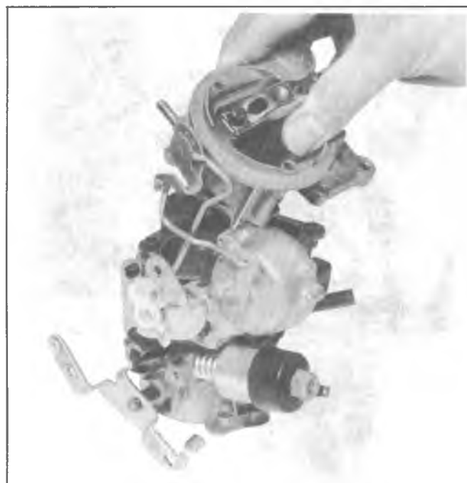
Fig. 6C1-15--Air Horn Removal
