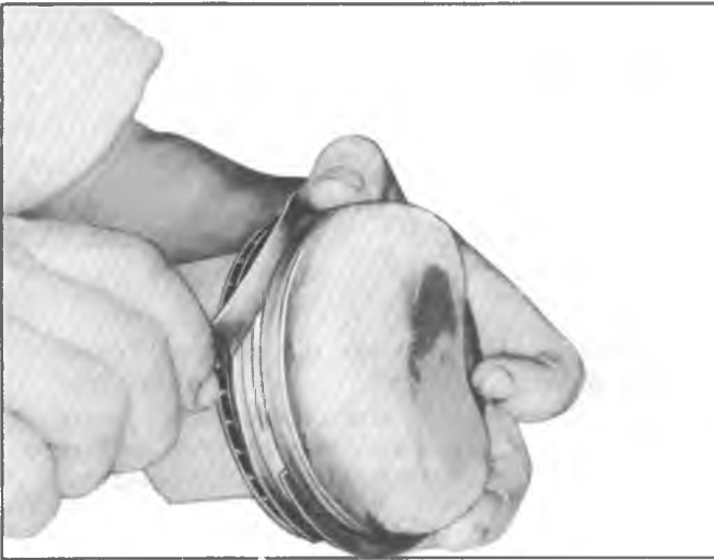
Fig. 6A4-57--Measuring Ring Groove Clearance
