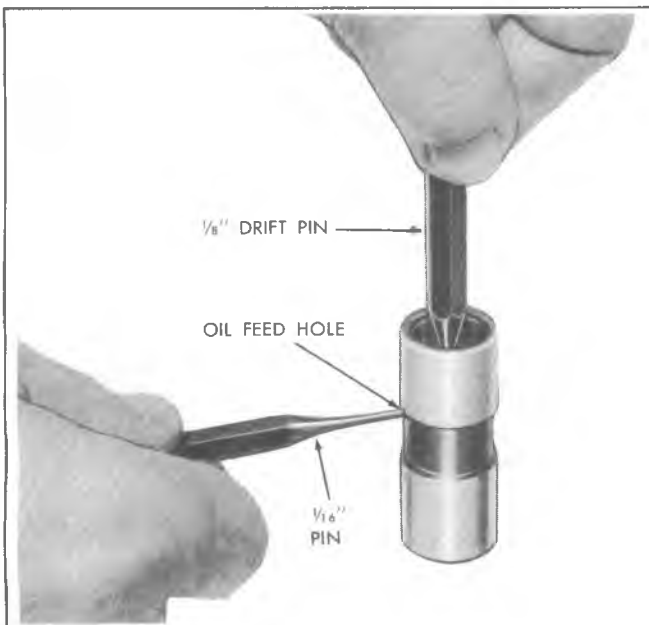
Fig. 6A1-15--Assembling Hydraulic Lifter
