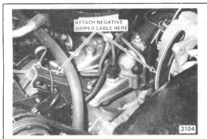
Fig. 6D-6B—Negative Jumper Cable Connection
