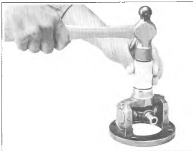
Fig. 4A-31--Installing Centering Ball Seal
