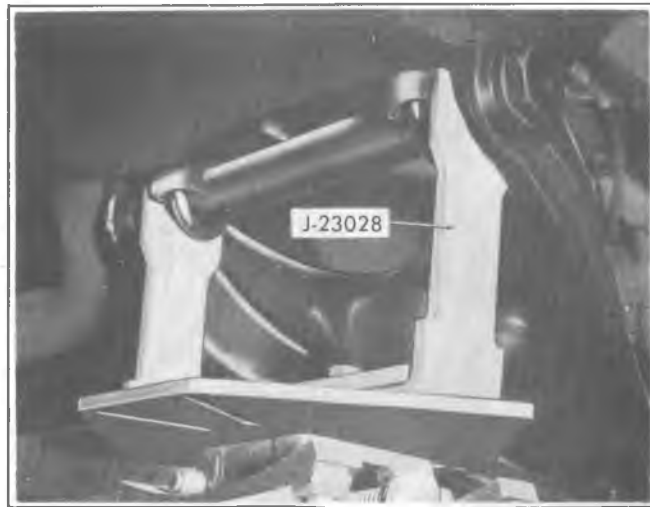
Fig. 3C-17--Removing Coil Spring with Tool J-23028
