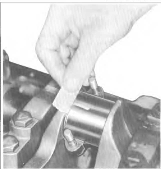
Fig. 6A1-28--Measuring Gaging Plastic
