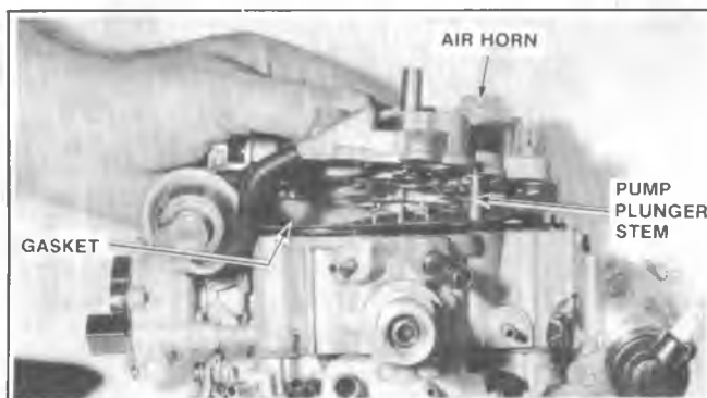
Fig. 6C3-20--Removing Air Horn
