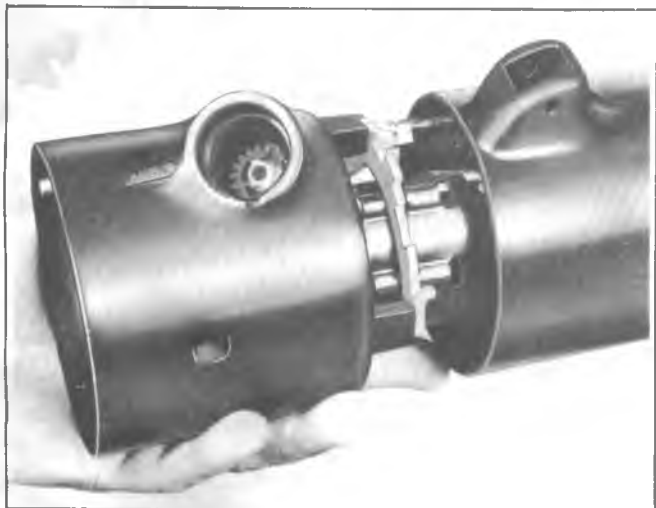
Fig. 3B4-42--Removing Turn Signal Housing
