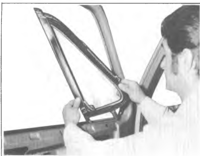
Fig. 2D-29--Removing Ventilator Assembly
