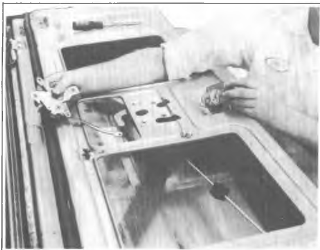
Fig. 2D-71--Removing Control Assembly and Inside Handle
