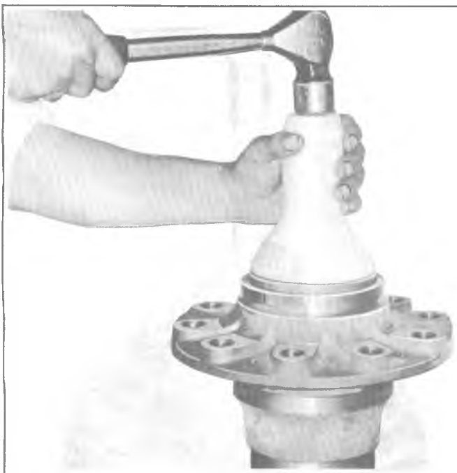
Fig. 4B-40--Installing Hub Oil Seal
