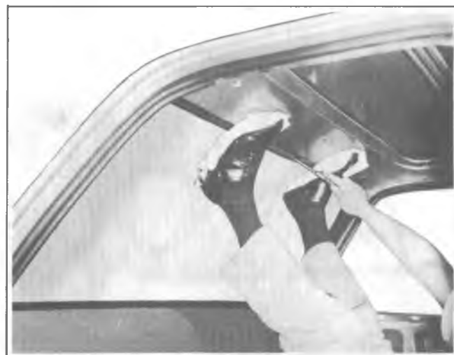
Fig. 2D-14--Applying Pressure to Windshield
