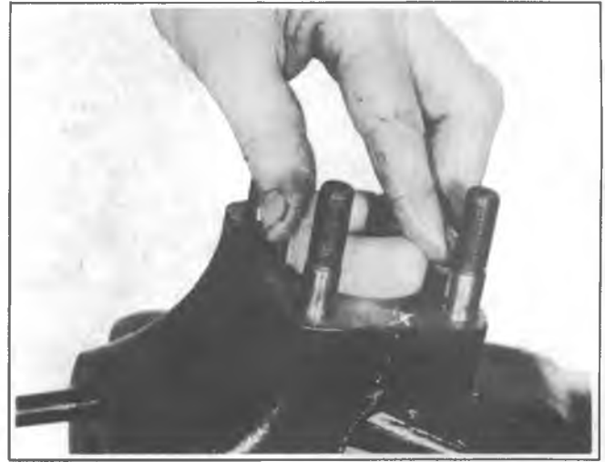
Fig. 3C-23K--Removing Tapered Bushing
