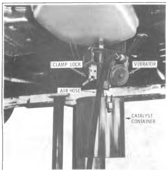
Fig. 6F-9--Installing Catalyst Container
