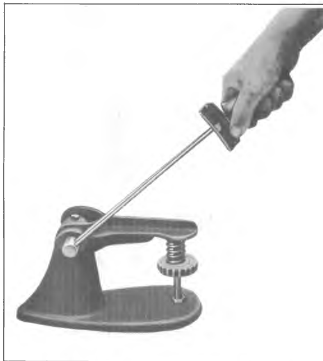
Fig. 6A4-21—Checking Valve Spring Tension
