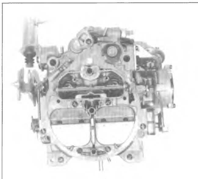
Fig. 6C4-24--Removing Air Horn Screws
