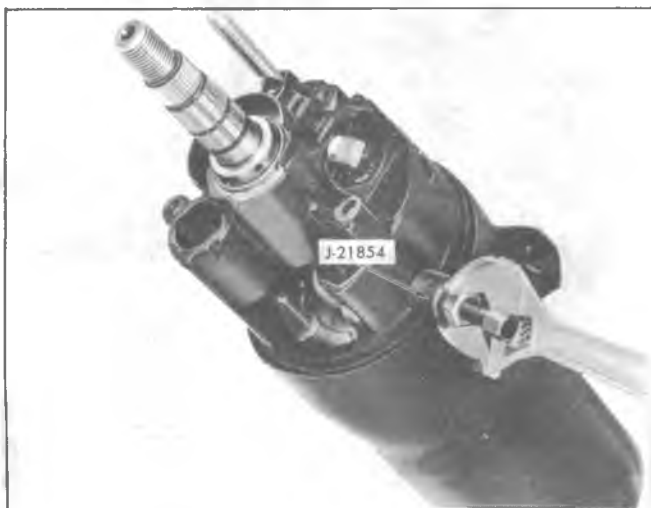
Fig. 3B4-51--Removing Bearing Housing Pivot Pins
