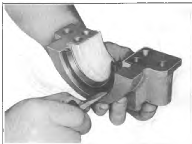
Fig. 6A4-47--Removing Oil Seal - Lower Half
