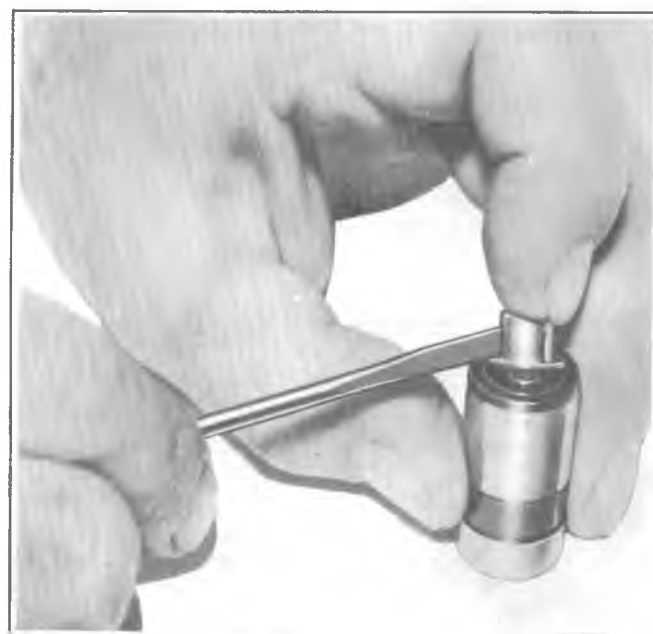
Fig. 6A1-13—Removing Ball Check Valve
