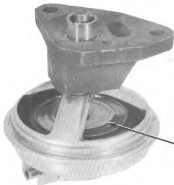
Fig. 6E-9—Ported EGR Identification
