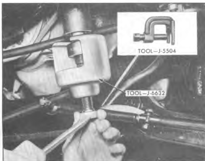
Fig. 3B3-13--Removing Pitman Arm
