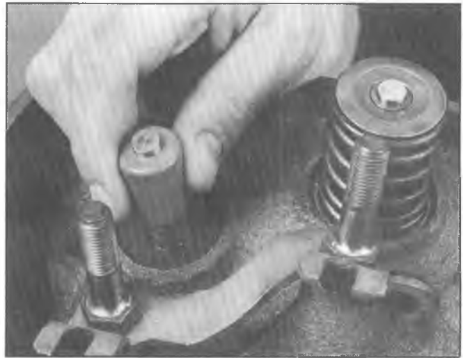
Fig. 6A5-13--Installing Valve Stem Oil Seal
