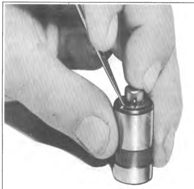
Fig. 6A4-16--Installing Ball Check Valve
