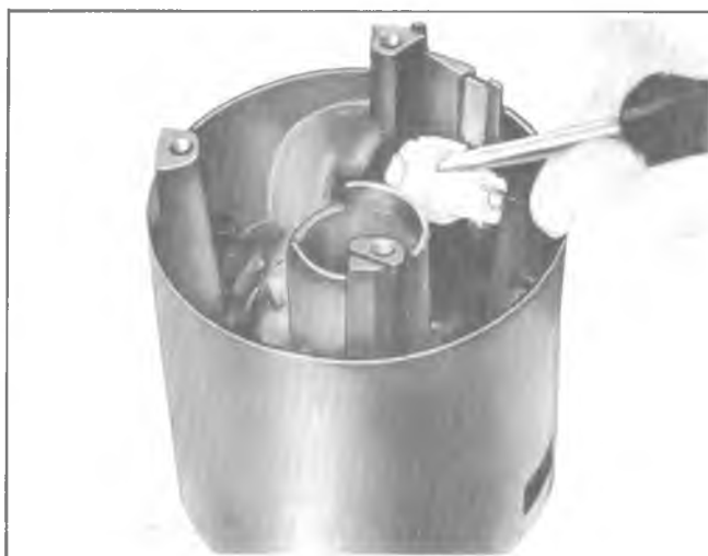
Fig. 3B4-44--Removing Ignition Switch Actuator Sector
