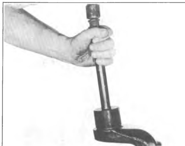
Fig. 3C-27K--Installing Oil Seal
