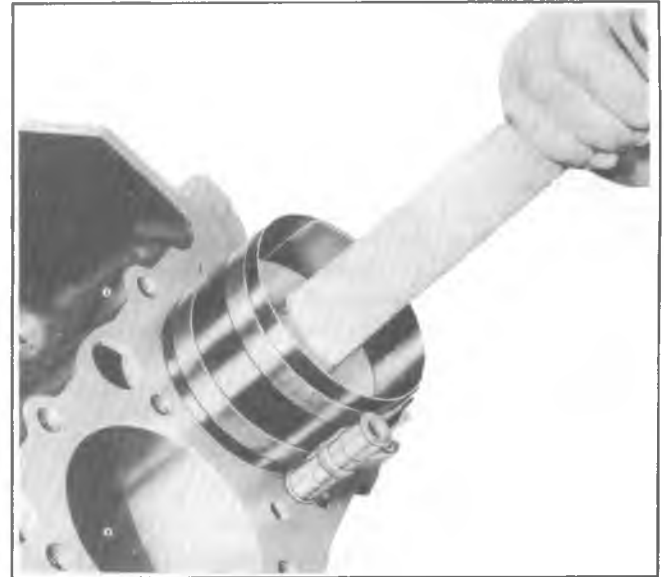
Fig. 6A4-58--Installing Connecting Rod &amp; Piston Assembly
