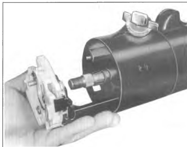
Fig. 3B4-28--Removing Directional Signal Switch Assembly
