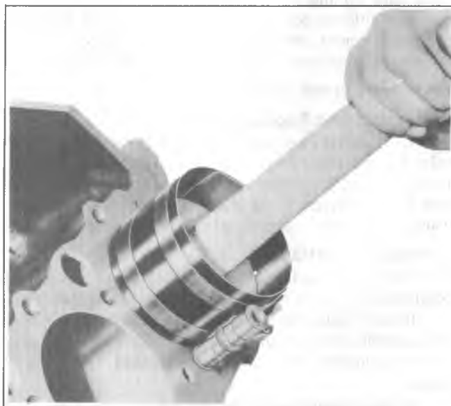
Fig. 6A1-45--Installing Connecting Rod and Piston Assembly
