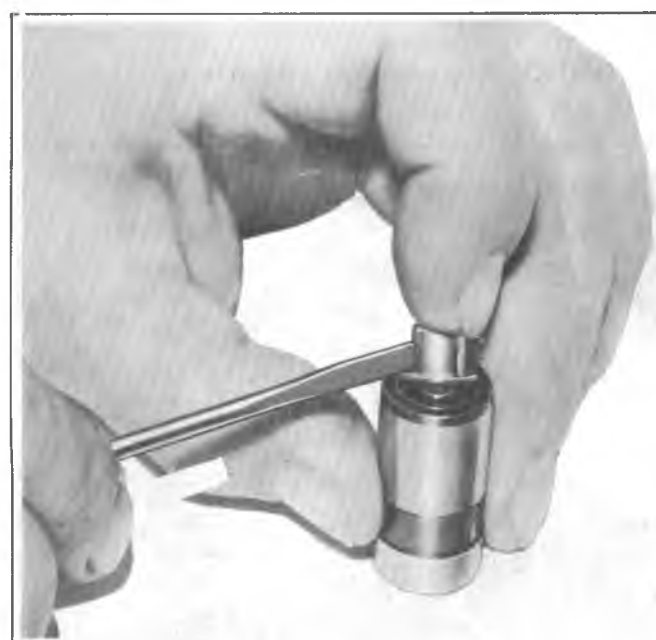
Fig. 6A5-15--Removing Ball Check Valve
