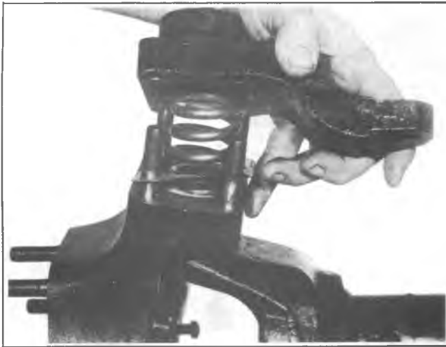
Fig. 3C-21K--Removing Cap, Spring and Gasket
