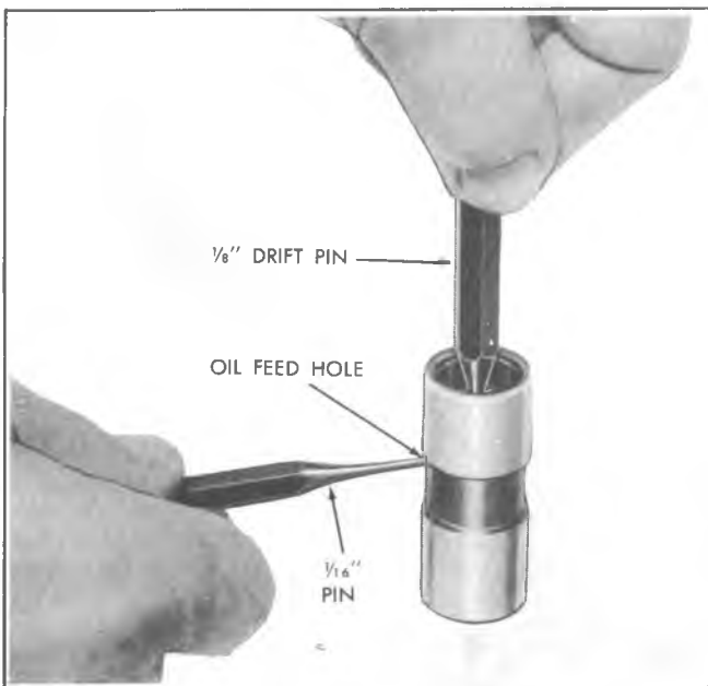
Fig. 6A4-17--Assembling Hydraulic Lifter
