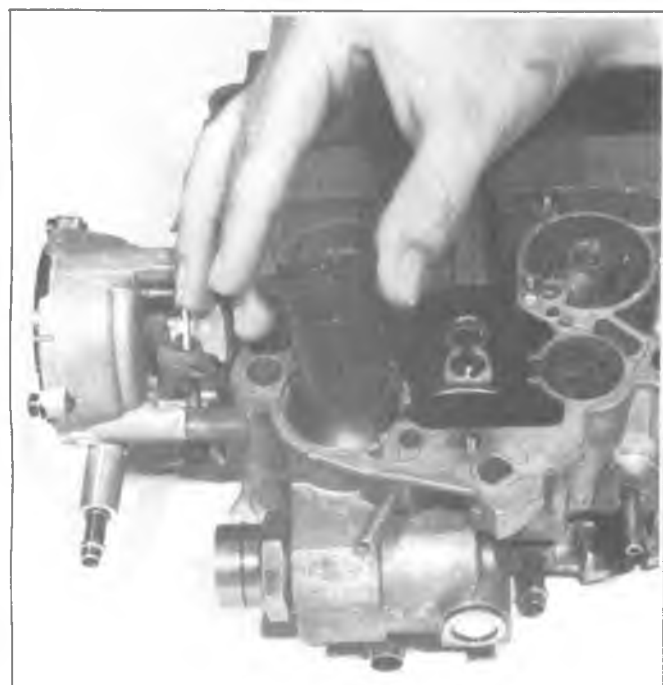
Fig. 6C4-31--Removing Aneroid Cavity Insert
