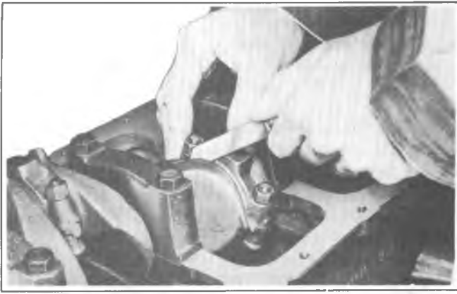
Fig 6A1-29--Measuring Connecting Rod Side Clearance
