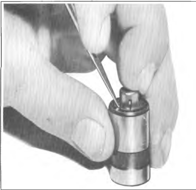
Fig. 6A1-14--Installing Ball Check Valve
