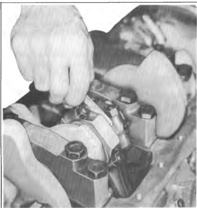
Fig. 6A4-42--Measuring Connecting Rod Side Clearance
