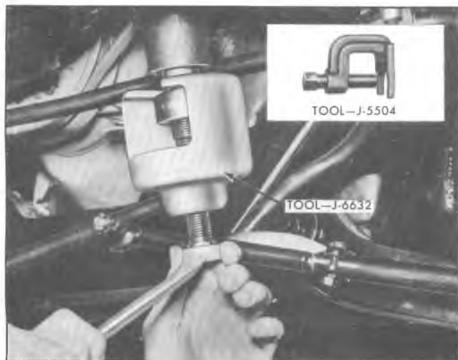
Fig. 3B2-4--Removing Pitman Arm
