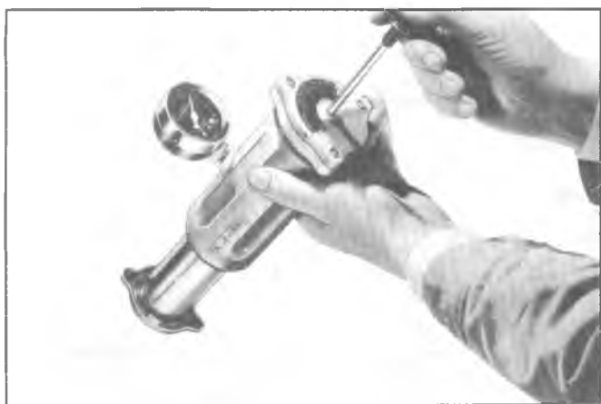
Fig. 6B-5--Pressure Checking Radiator Cap
