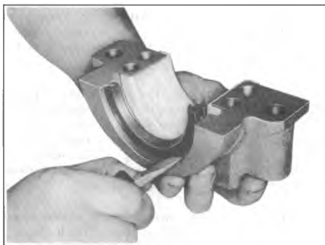
Fig. 6A5-48--Removing Oil Seal - Lower Half
