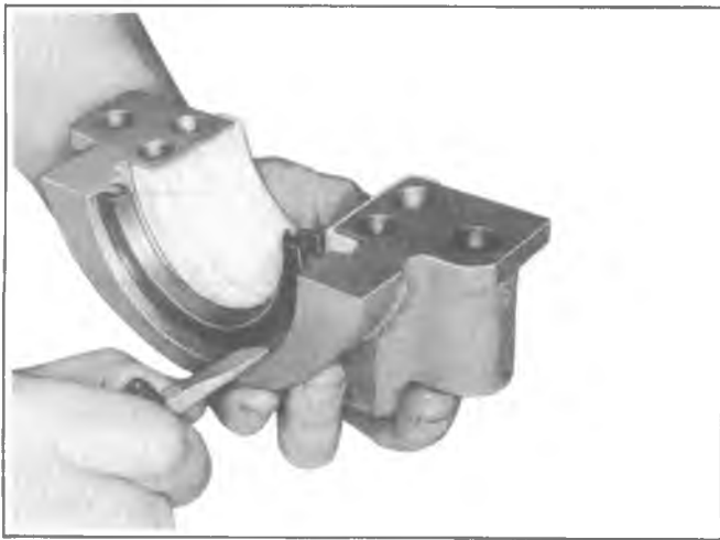
Fig. 6A1-35--Removing Oil Seal Lower Half - Typical
