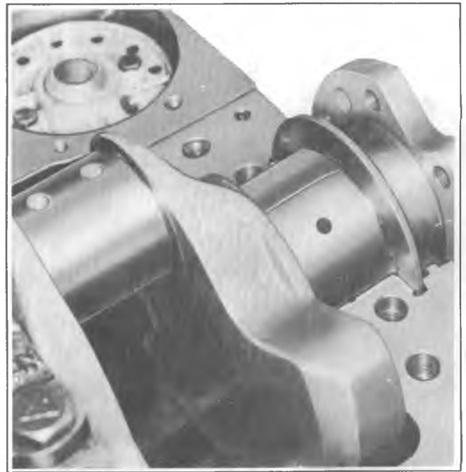
Fig. 6A1-30--Gaging Plastic on Journal – Typical
