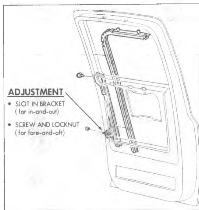
Fig. 2D-45--Glass Run Channel Adjustment
