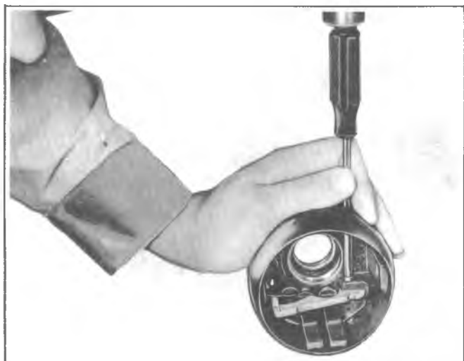
Fig. 3B4-80--Removing Release Lever Pivot Pin
