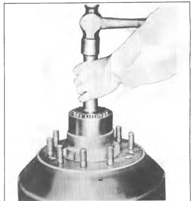
Fig. 4B-38--Removing Hub Outer Bearing
