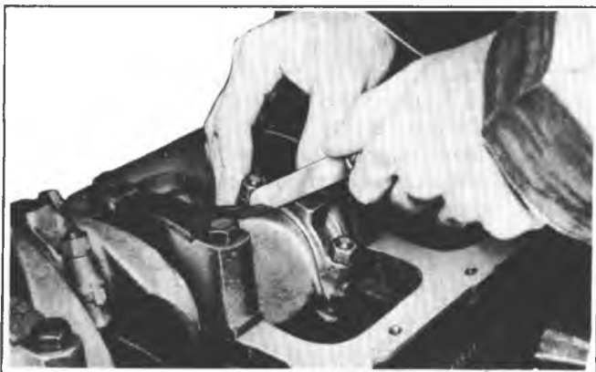
Fig. 6A1-29—Measuring Connecting Rod Side Clearance
