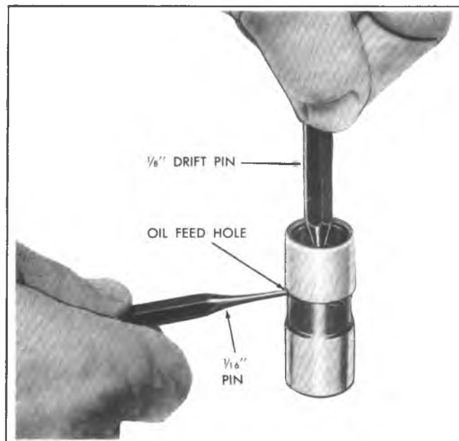
Fig. 6A1-15--Assembling Hydraulic Lifter
