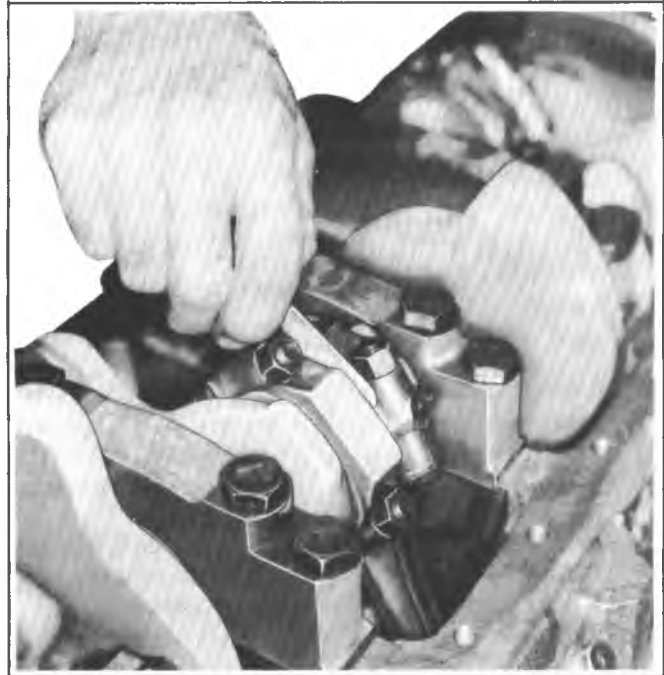
Fig. 6A5-43--Measuring Connecting Rod Side Clearance
