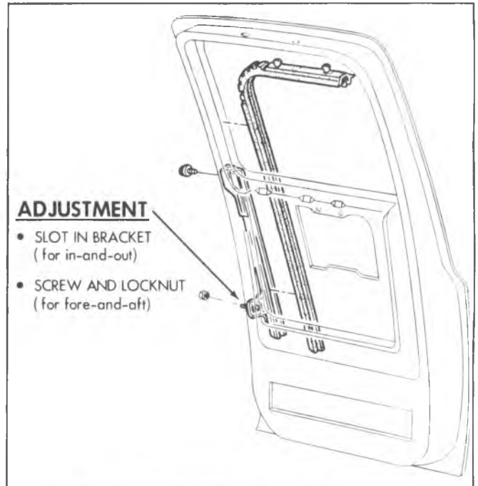
Fig. 2D-45--Glass Run Channel Adjustment
