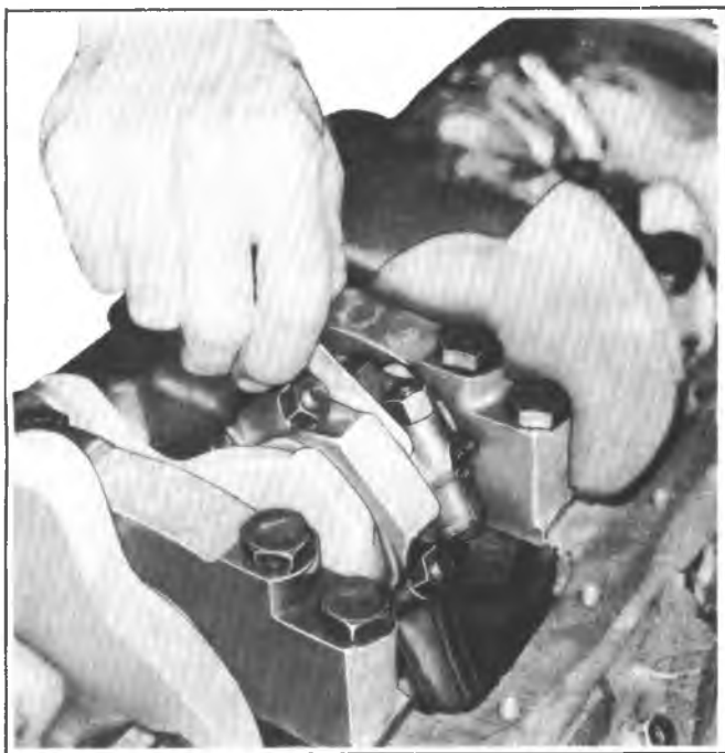
Fig. 6A4-42--Measuring Connecting Rod Side Clearance
