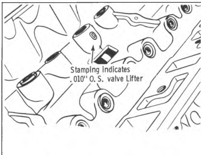
Fig. 6A6-38--O.S. Valve Lifter Identification
