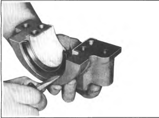
Fig. 6A1-35--Removing Oil Seal Lower Half - Typical
