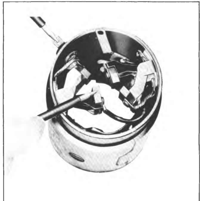
Fig. 6D-13E--Testing Field Coils for Open
