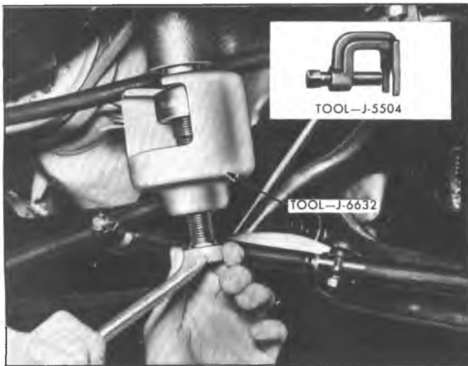
Fig. 3B2-9--Removing Pitman Arm-Typical
