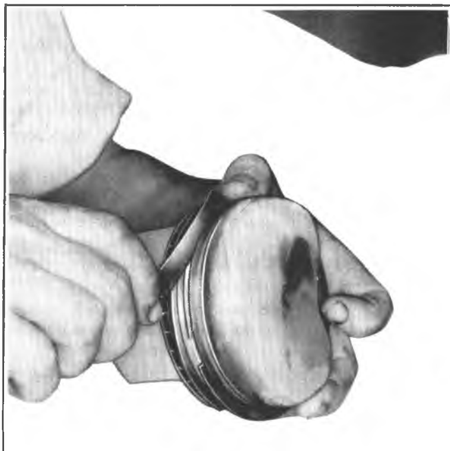
Fig. 6A1-43—Measuring Ring Groove Clearance
