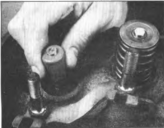
Fig. 6A5-13--Installing Valve Stem Oil Seal
