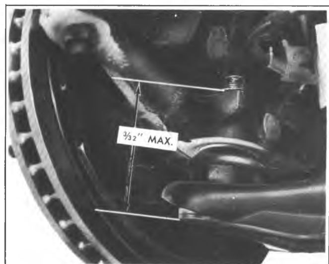
Fig. 3C-29--Checking Lower Ball Joint
