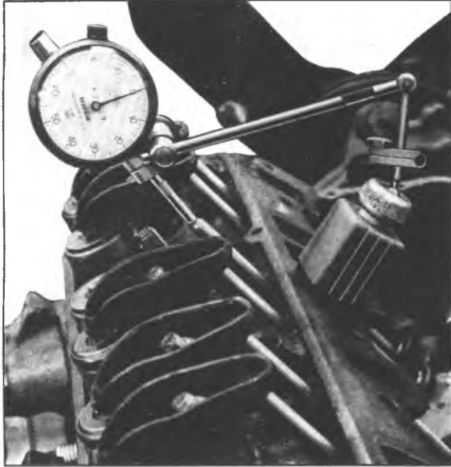
Fig. 6A4-33--Measuring Camshaft Lobe Lift
