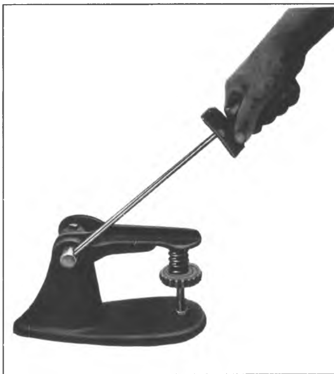
Fig. 6A1-16—Checking Valve Spring Tension
