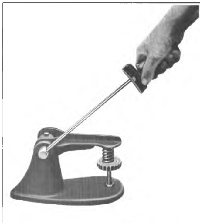
Fig. 6A5-22--Checking Valve Spring Tension
