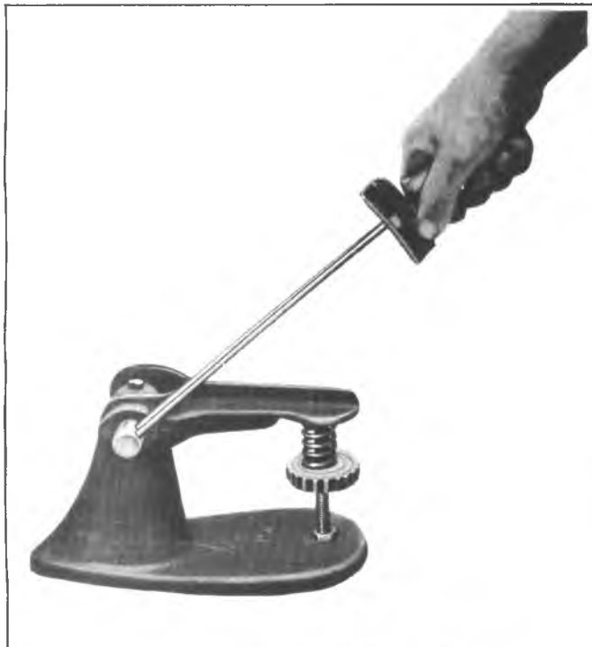
Fig. 6A4-21--Checking Valve Spring Tension
