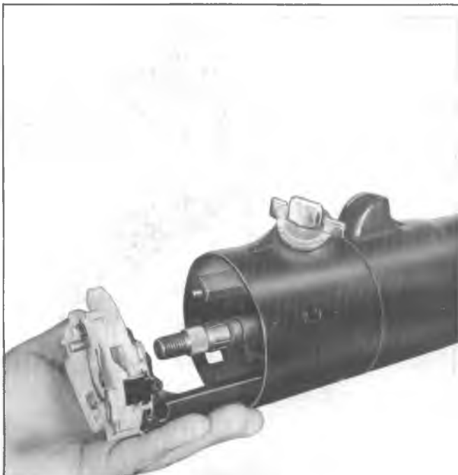
Fig. 3B4-25—Directional Signal Switch
