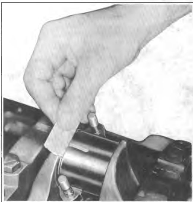
Fig. 6A5-42--Measuring Gaging Plastic
