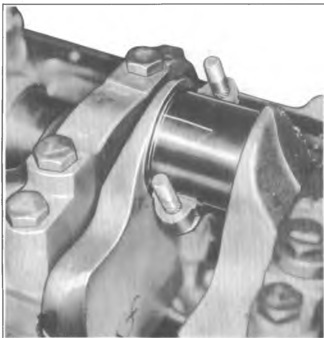
Fig. 6A4-40--Gaging Plastic On Crankpin
