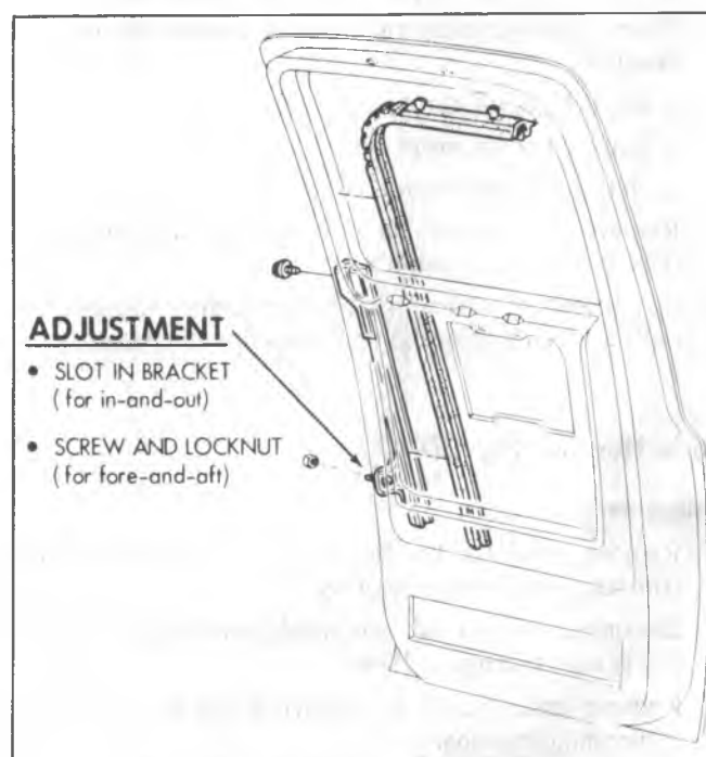
Fig. 2D-45--Glass Run Channel Adjustment
