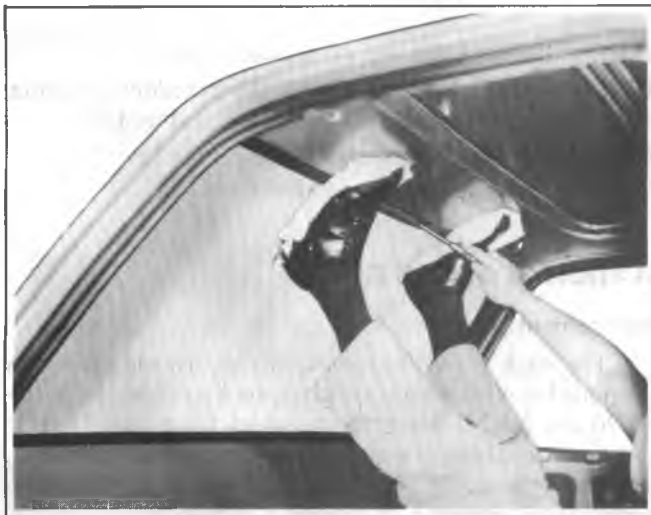
Fig. 2D-14--Applying Pressure to Windshield
