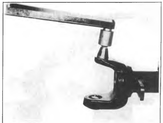
Fig. 3C-26K--Installing Upper King-Pin
