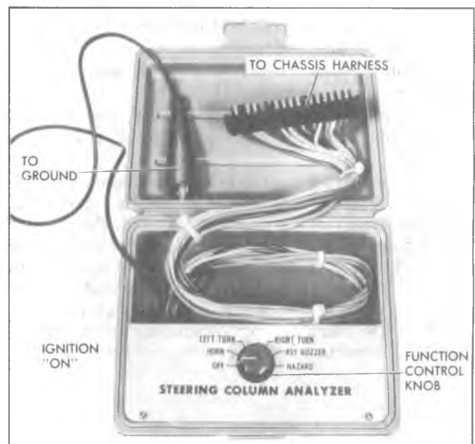
Fig. 3B4-2—Steering Column Electrical Analyzer J-23980
