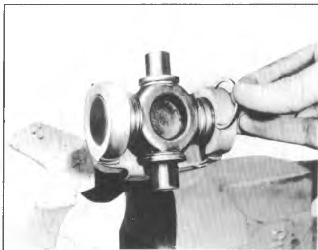
Fig. 4A-15--Installing Snap Ring to Retain Trunnion
