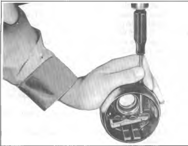
Fig. 3B4-80—Removing Release Lever Pivot Pin
