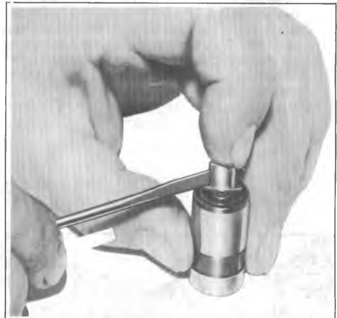
Fig. 6A5-15--Removing Ball Check Valve
