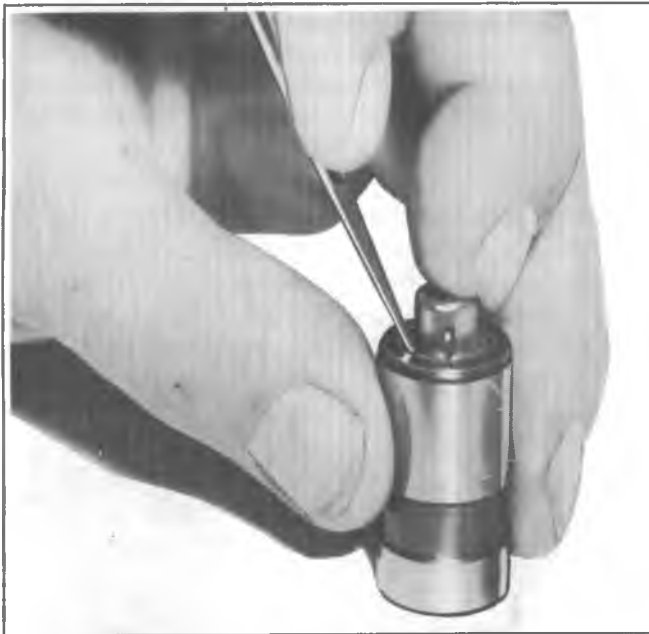
Fig. 6A5-16--Installing Ball Check Valve
