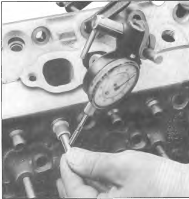
Fig. 6A4-20--Measuring Valve Stem Clearances
