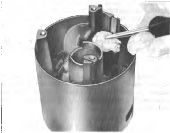
Fig. 3B4-44—Removing Ignition Switch Actuator Sector
