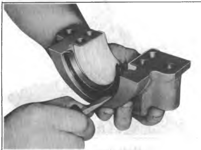
Fig. 6A4-47--Removing Oil Seal - Lower Half
