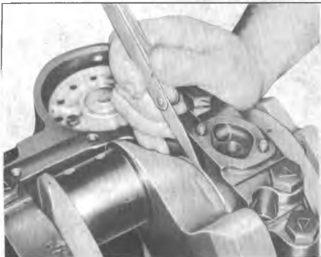
Fig. 6A4-45--Measuring Crankshaft End Play
