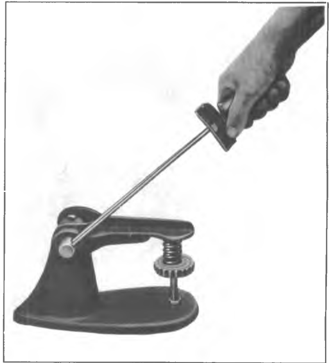
Fig. 6A1-16--Checking Valve Spring Tension
