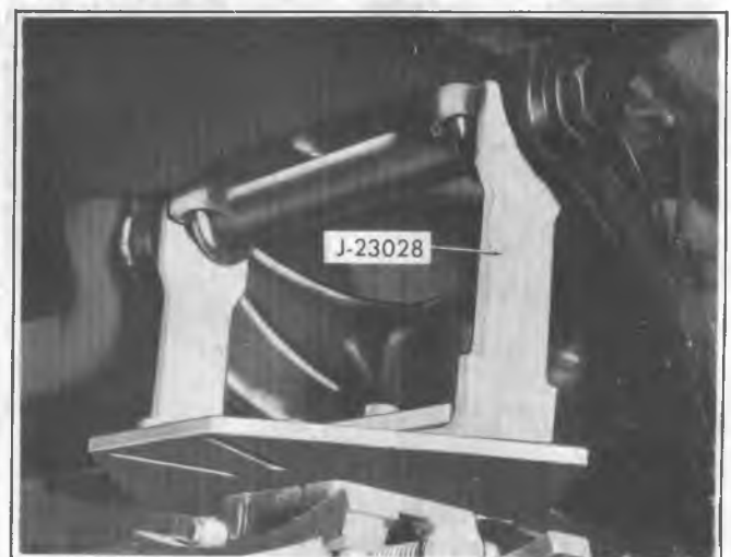
Fig. 3C-17--Removing Coil Spring with Tool J-23028
