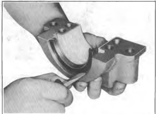
Fig. 6A5-48--Removing Oil Seal - Lower Half
