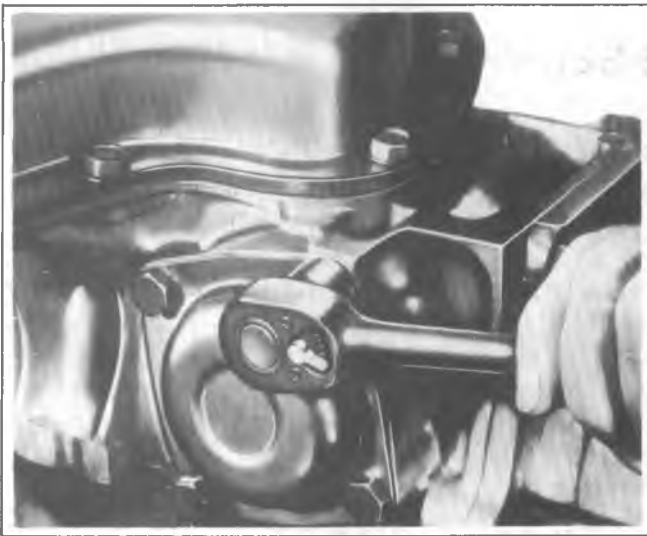
Fig. 7A-46--Removing Governor Attaching Screws
