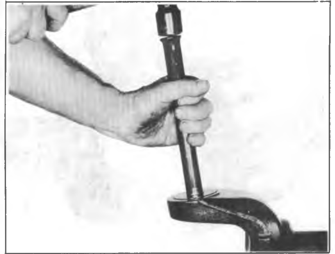
Fig. 3C-24K--Installing Grease Retainer
