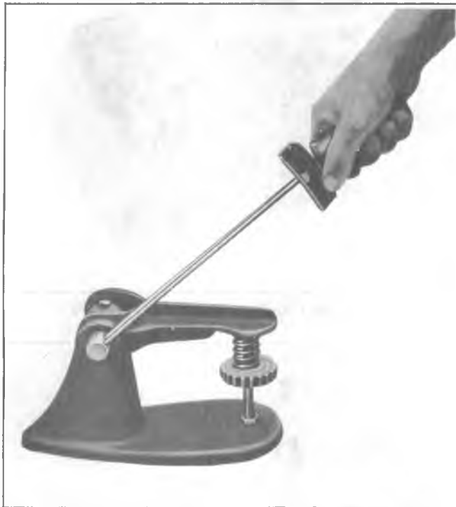
Fig. 6A4-21--Checking Valve Spring Tension
