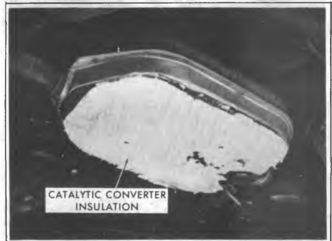
Fig. 6F-12 — Catalytic Converter Insulation
