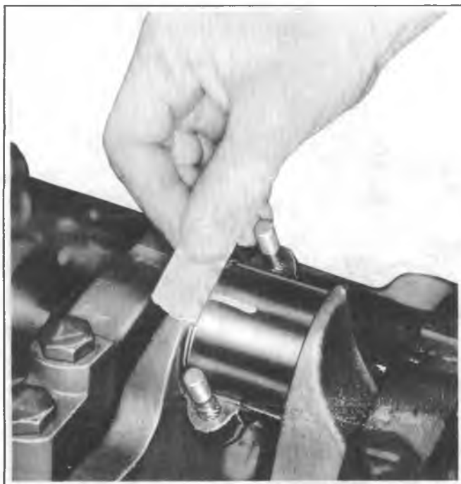
Fig. 6A1-28--Measuring Gaging Plastic
