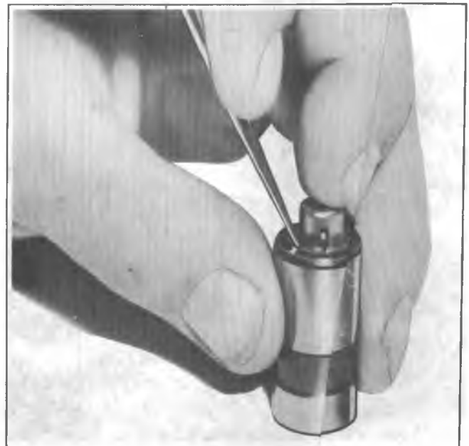
Fig. 6A4-16--Installing Ball Check Valve
