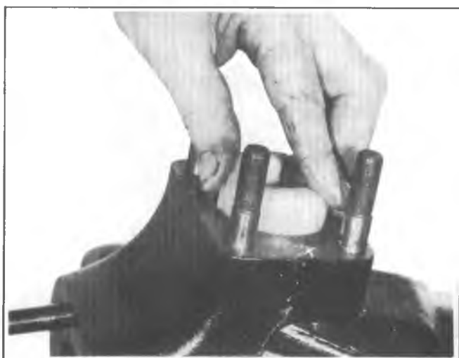
Fig. 3C-21K--Removing Tapered Bushing
