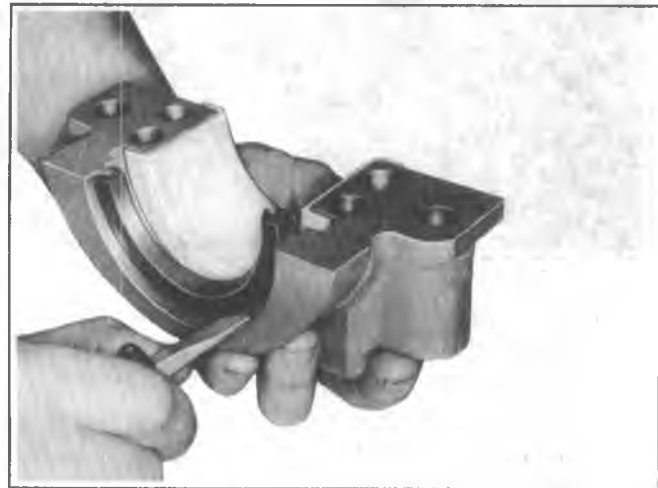
Fig. 6A1-35--Removing Oil Seal Lower Half - Typical
