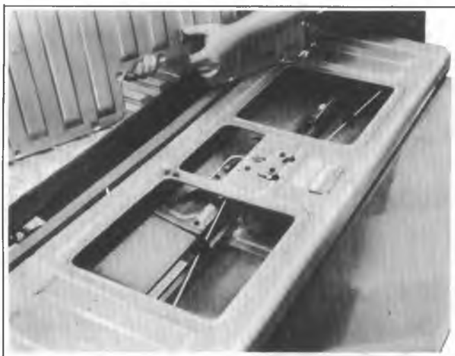
Fig. 2D-65--Removing Access Cover (Utility)
