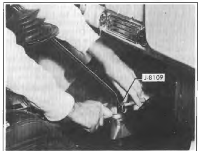
Fig. 7B-15--Removing Gearshift Lever
