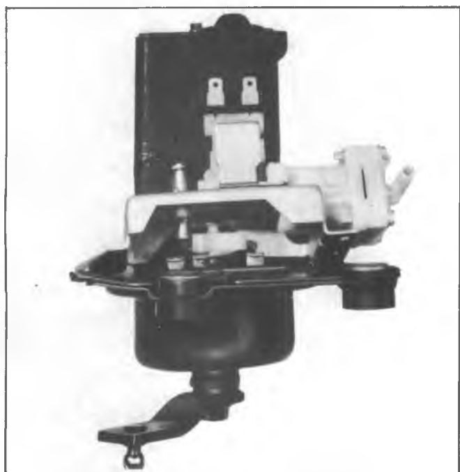
Fig. 8C-39--Washer Pump Drive Cam and Actuator
