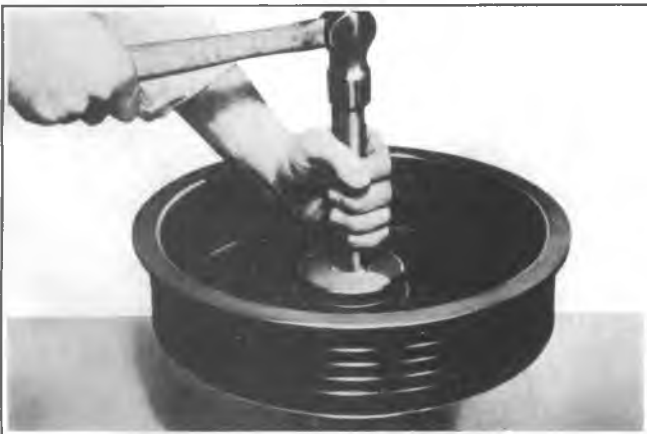
Fig. 4B-40--Installing Hub Inner Bearing Cup
