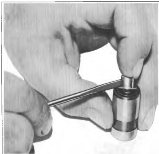
Fig. 6A1-13--Removing Ball Check Valve
