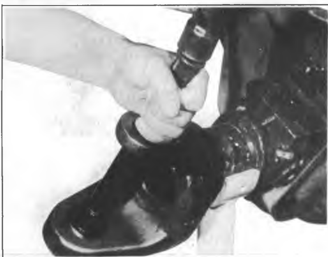
Fig. 3C-23K--Removing Cup, Cone and Seal
