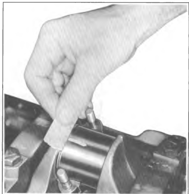
Fig. 6A4-41--Measuring Gaging Plastic
