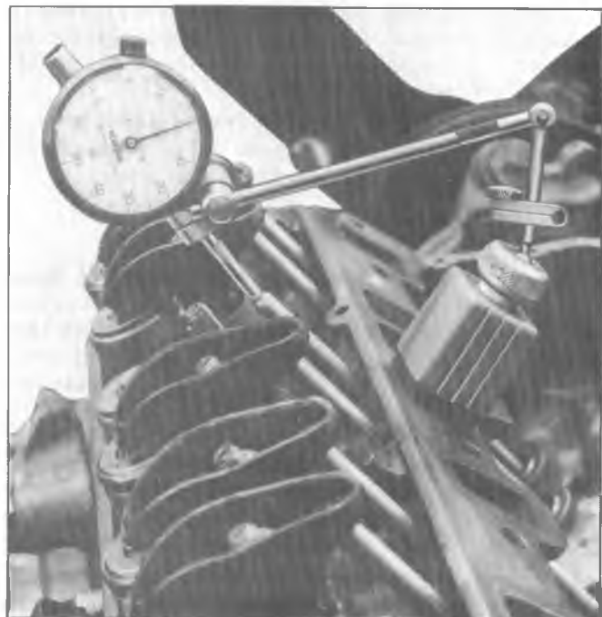
Fig. 6A4-33--Measuring Camshaft Lobe Lift
