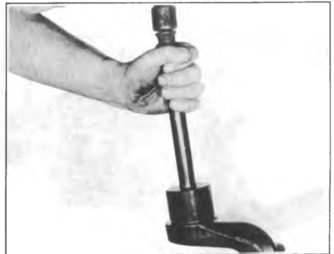
Fig. 3C-25K--Installing Oil Seal
