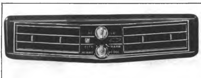
Fig. 1B-12--Motor Home Unit Control
