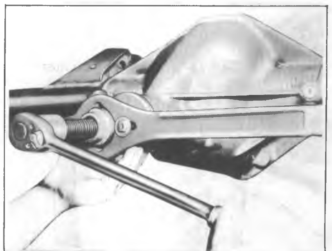
Fig. 4B-27--Drive Pinion Flange Removal
