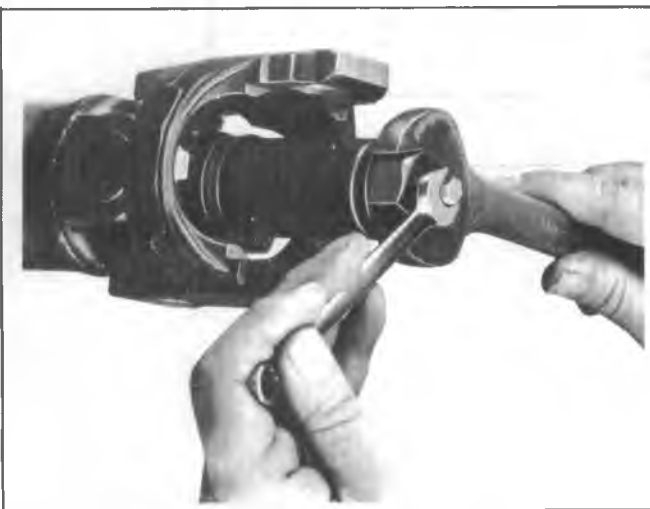
Fig. 4A-26--Removing Centering Ball
