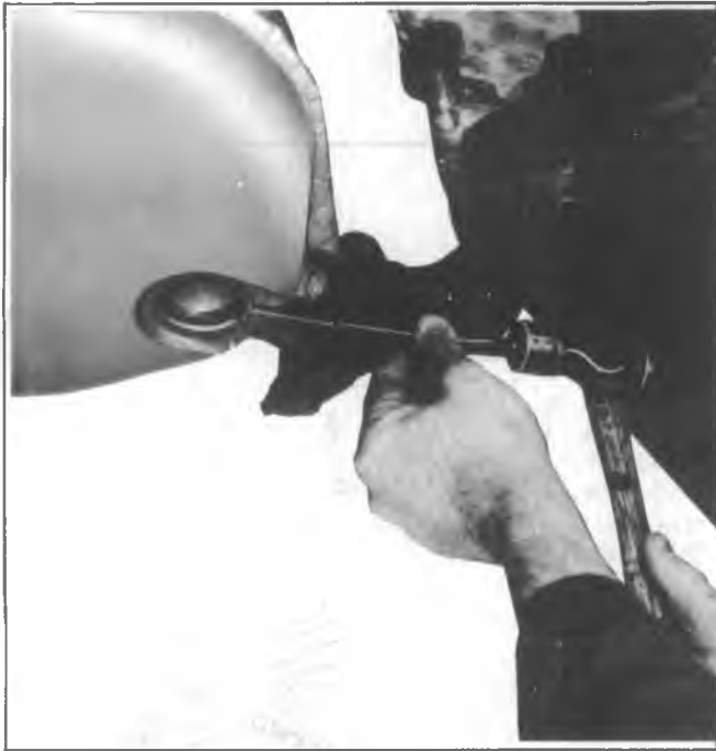
Fig. 6F-5 — Removing Pressed Plug
