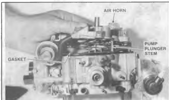
Fig. 6C3-9--Removing Air Horn bracket assembly. (Fig. 6C3-10). Do not place vacuum break assembly in carburetor cleaner.
