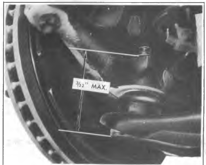
Fig. 3C-29--Checking Lower Ball Joint
