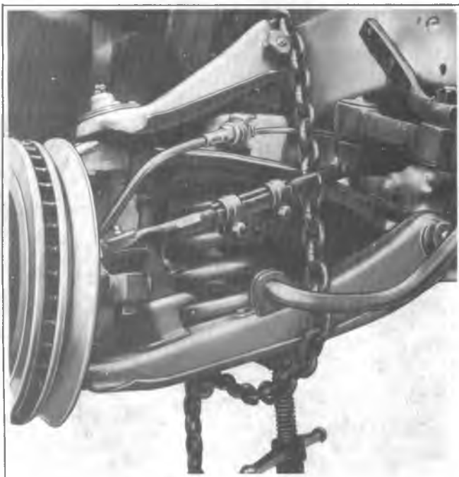
Fig. 3C-18--Removing Inner Pivot Shaft
