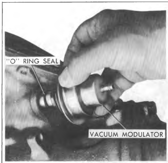
Fig. 7A-19—Removing Vacuum Modulator
