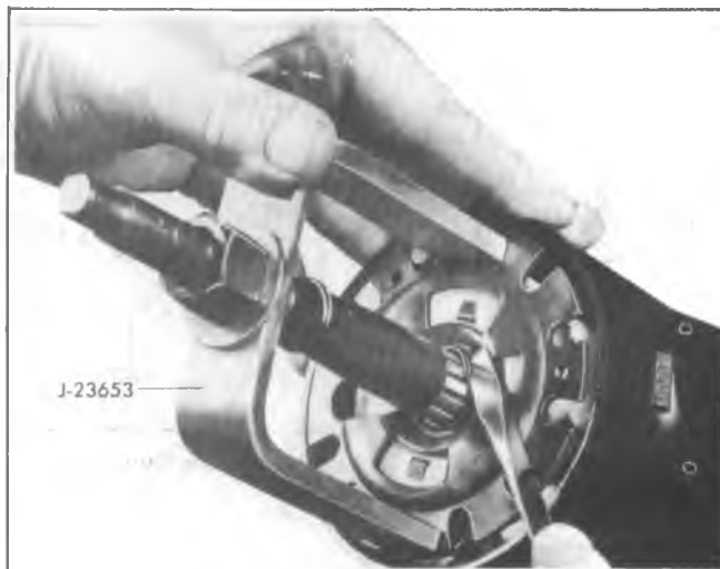
Fig. 3B4-26—Removing Lock Plate Retaining Ring
