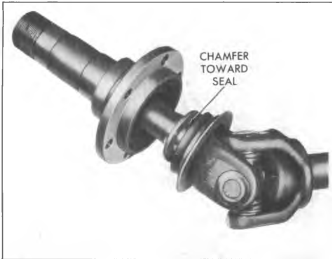
Fig. 3C-8K--Installing Spindle and Thrust Washer
