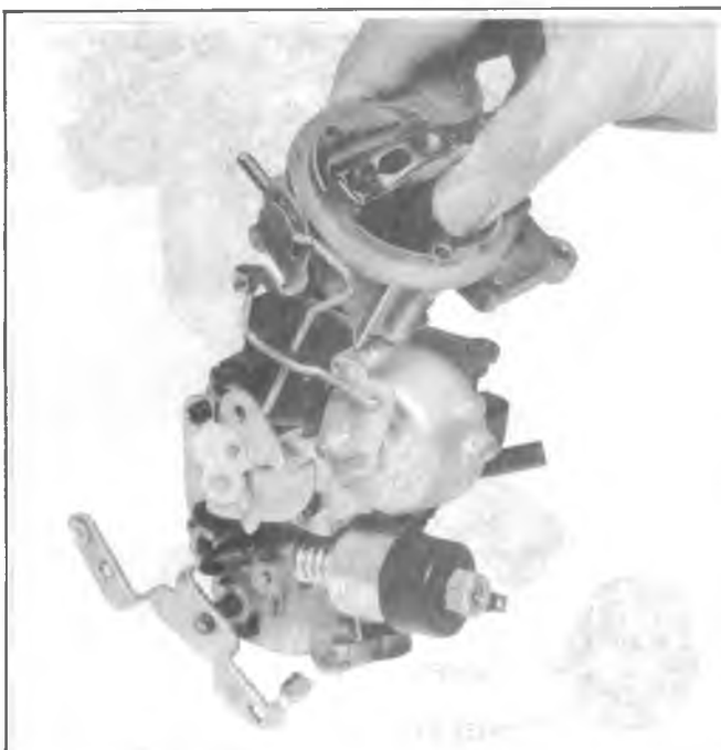
Fig. 6C1-15--Air Horn Removal
