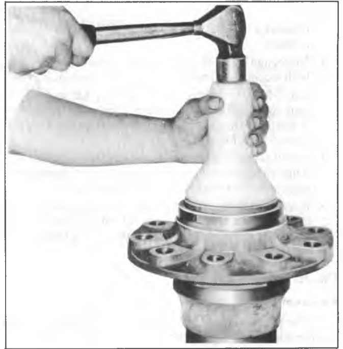
Fig. 4B-41--Installing Hub Oil Seal
