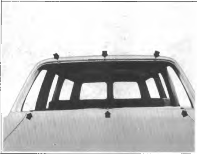
Fig. 2D-17--Checking Windshield Opening
