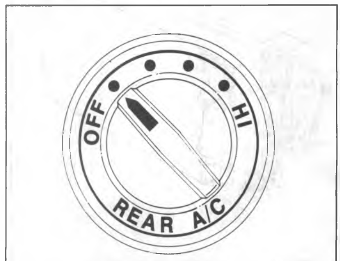
Fig. 1B-41--Blower Switch (C-K Overhead System)
