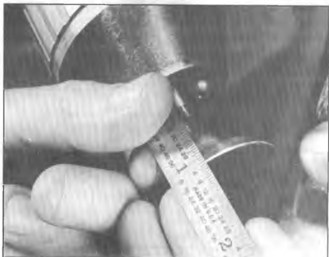
Fig. 6A5-29--Measuring Valve Head
