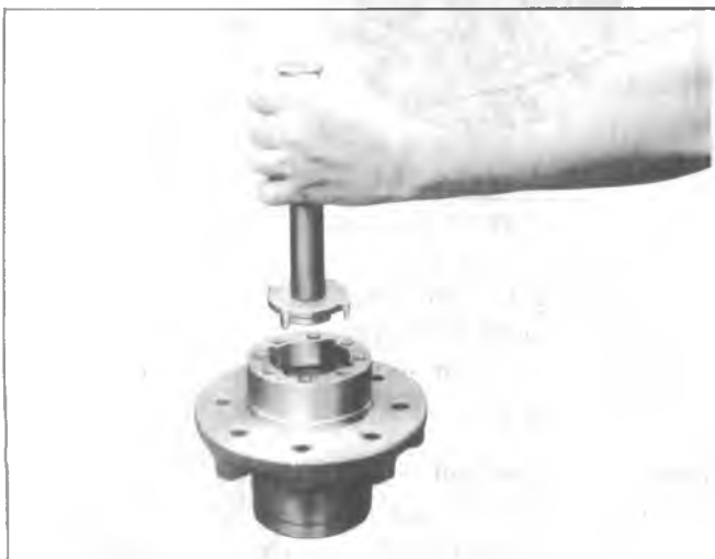
Fig. 4B-33--Removing Outer Bearing and Cup
