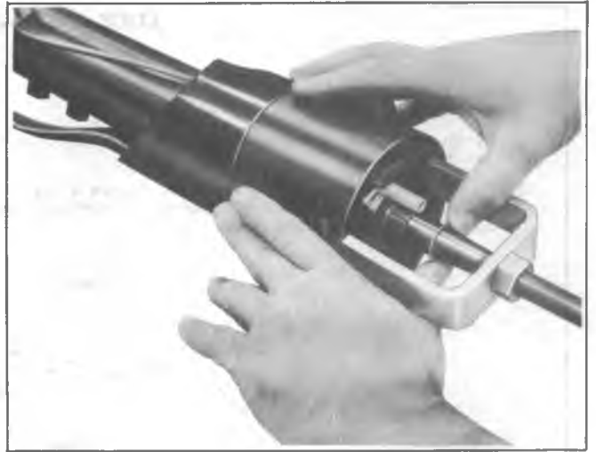
Fig. 3B4-30--Installing Snap Ring
