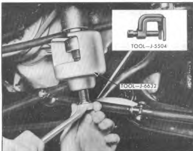
Fig. 3B2-4--Removing Pitman Arm
