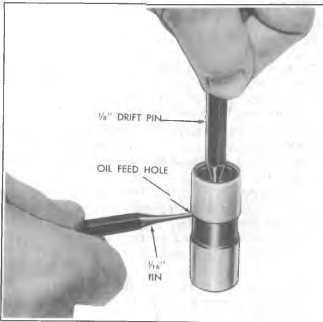
Fig. 6A4-17--Assembling Hydraulic Lifter
