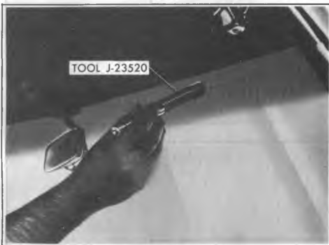
Fig. 9-4R--Testing Windshield Antenna (Typical)
