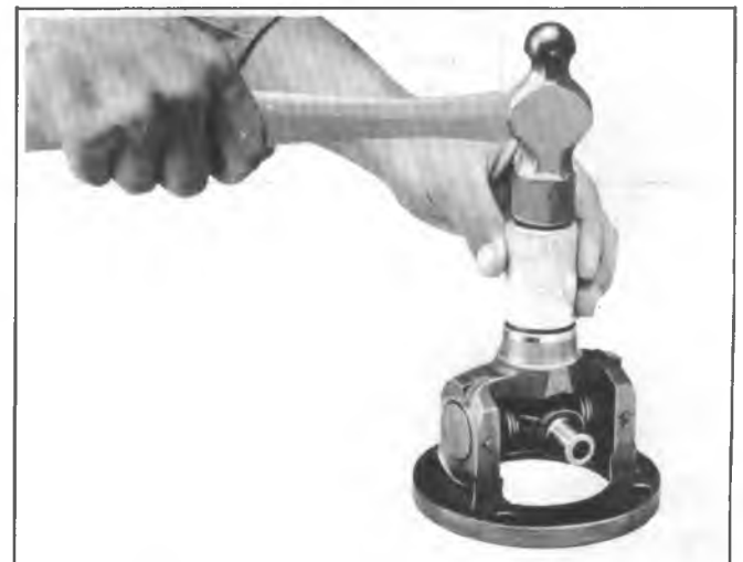
Fig. 4A-28--Installing Centering Ball Seal
