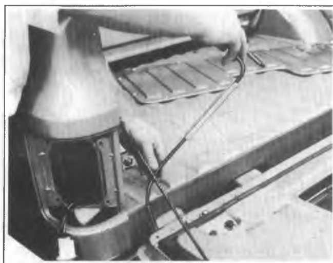
Fig. 2D-67--Removing Torque Rod (Utility)
