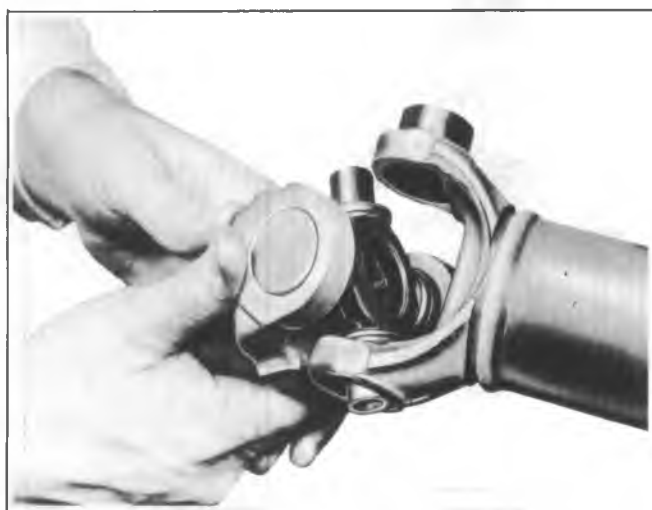
Fig. 4A-14--Installing Trunnion into Yoke
