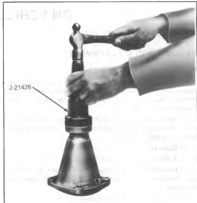
Fig. 7A-16--Installing Oil Seal into Extension Housing
