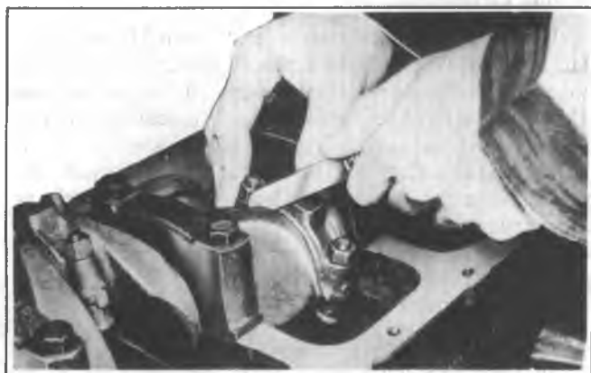
Fig. 6A1-29--Measuring Connecting Rod Side Clearance
