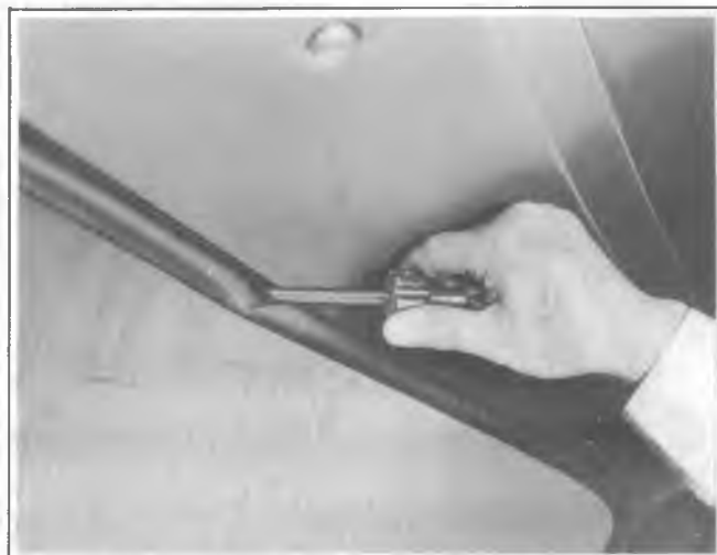
Fig. 2D-15--Assisting Weatherstrip over Flange
