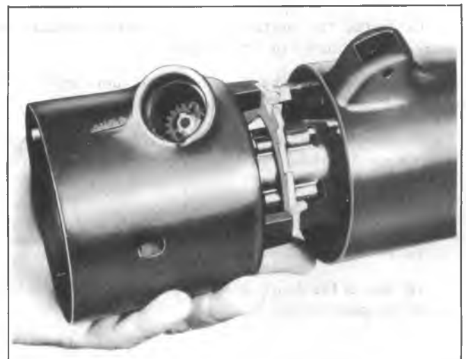
Fig. 3B4-42—Removing Turn Signal Housing
