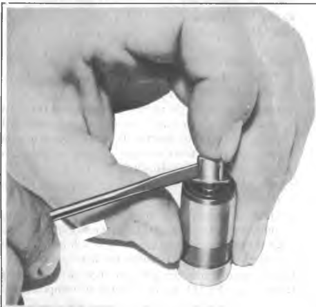
Fig. 6A4-15--Removing Ball Check Valve
