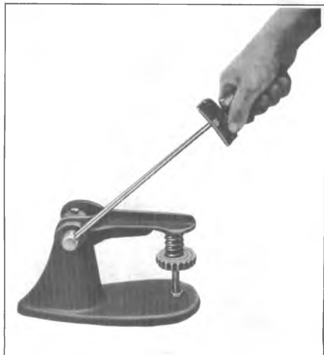
Fig. 6A5-22--Checking Valve Spring Tension
