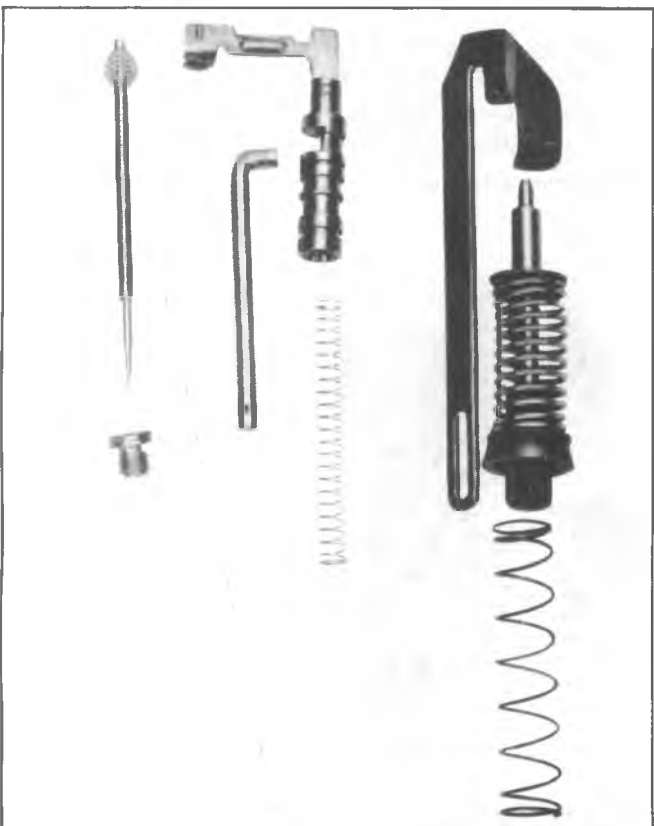
Fig. 6C1-19—Metering Rod and Accelerator Pump
