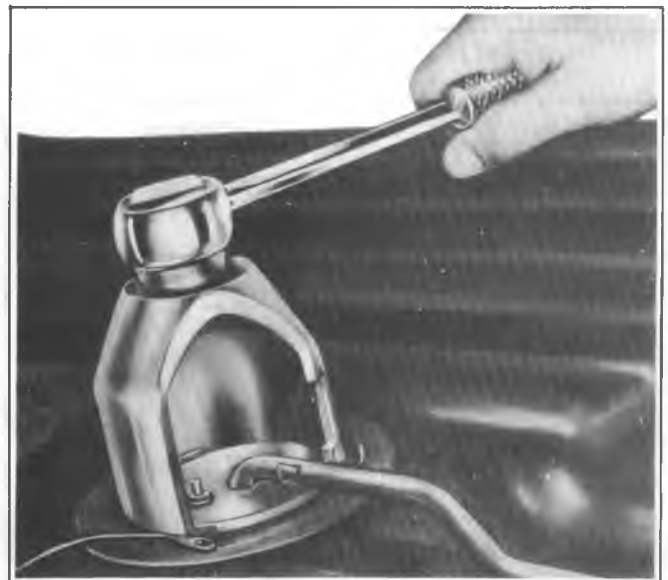
Fig. 6C5-10--Removing Meter Assembly
