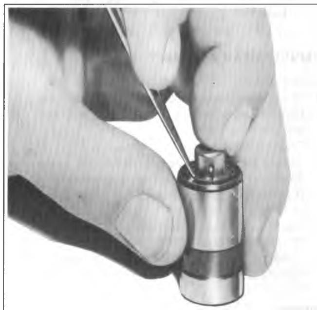
Fig. 6A1-14--Installing Ball Check Valve
