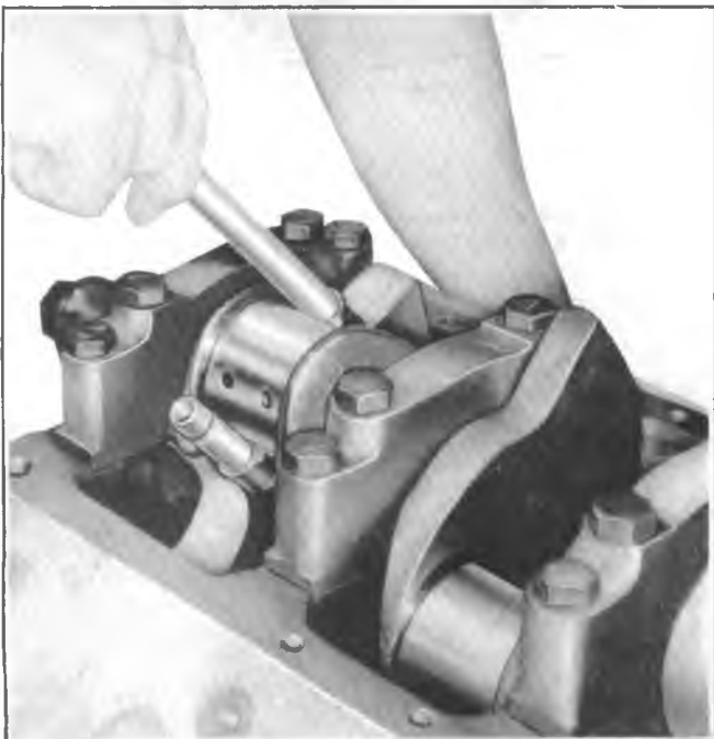
Fig. 6A4-51--Removing Connecting Rod & Piston Assembly
