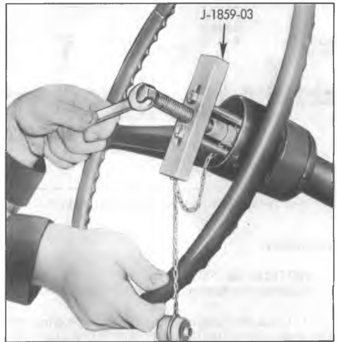
Fig. 3B4-59—Steering Wheel Removal-Typical
