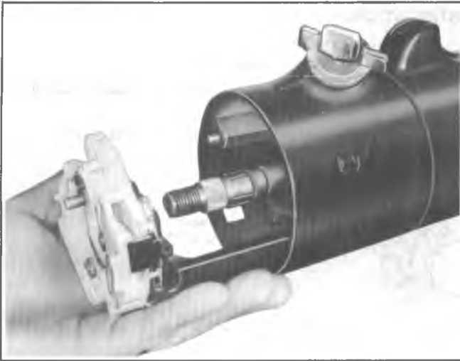
Fig. 3B4-28--Removing Directional Signal Switch Assembly
