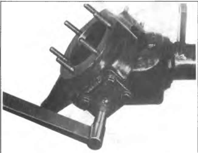
Fig. 3C-28K--Installing Lower Bearing Cap-and-King Pin
