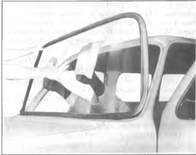
Fig. 2D-16--Removing Windshield from Opening
