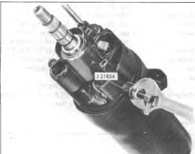
Fig. 3B4-51—Removing Bearing Housing Pivot Pins
