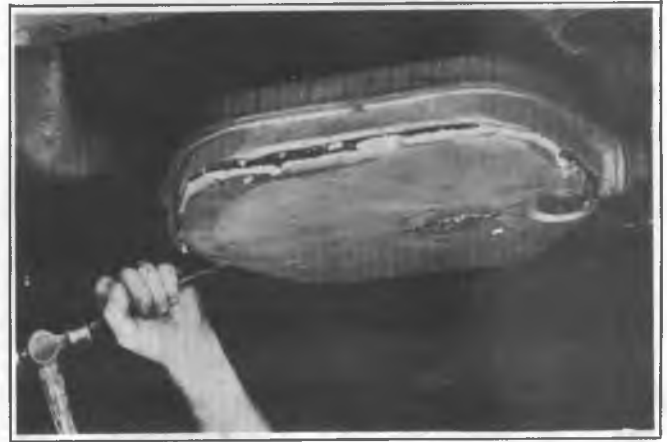
Fig. 6F-11 — Removing Bottom Cover
