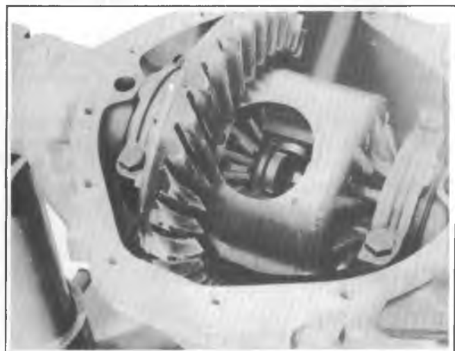
Fig. 4B-18--Push Axle Shaft Inward
