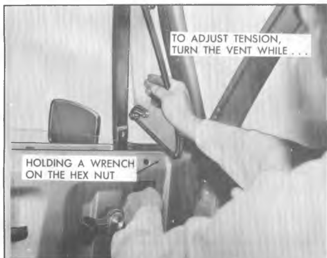
Fig. 2D-30--Adjusting Tension
