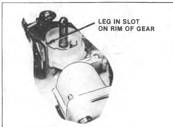
Fig. 8C-15--Armature Leg Position
