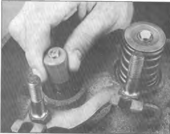
Fig. 6A5-13--Installing Valve Stem Oil Seal
