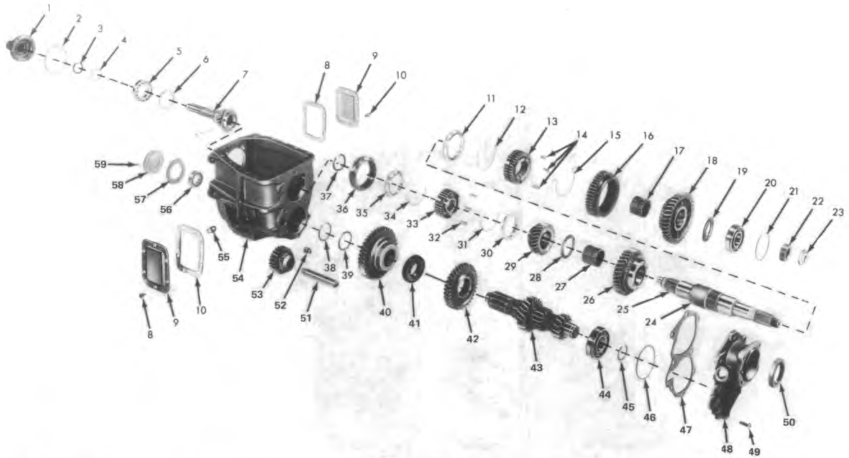
Fig. 7B-6-4-Speed 117mm, Exploded View
