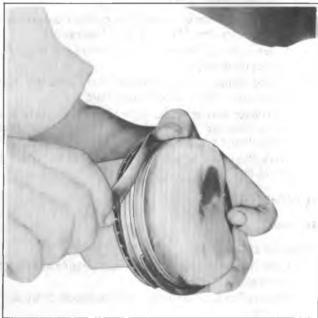
Fig. 6A1-43--Measuring Ring Groove Clearance
