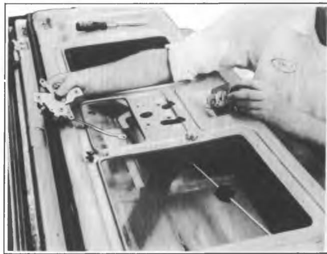
Fig. 2D-71--Removing Control Assembly and Inside Handle
