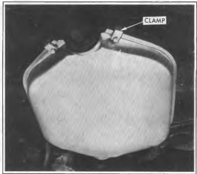
Fig. 6F-16 — Installing Bottom Cover Clamps
