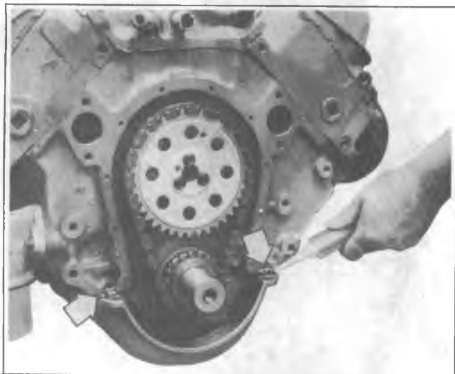
Fig. 6A5-33--Applying Front Cover Sealer
