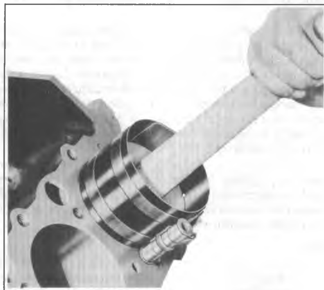
Fig. 6A1-45--Installing Connecting Rod and Piston Assembly
