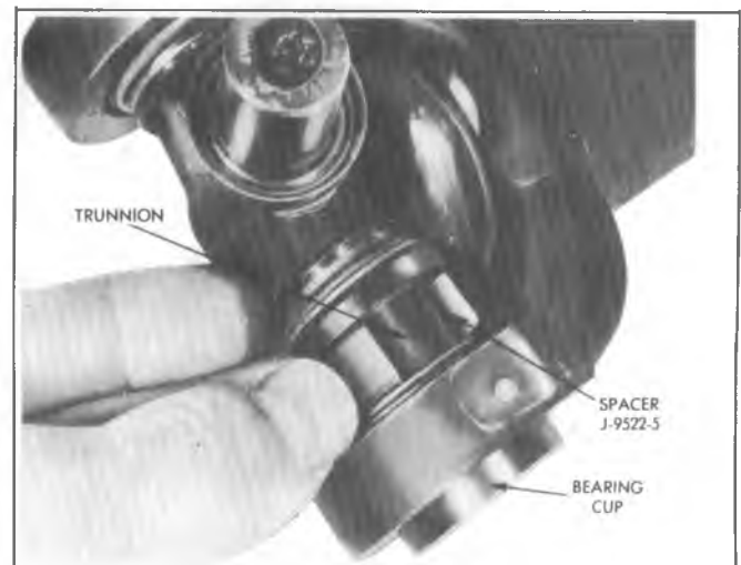
Fig. 4A-12--Using Spacer to Remove Bearing Cup
