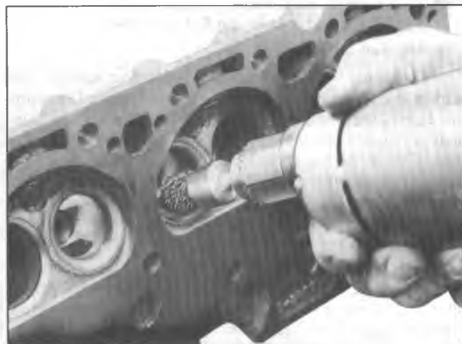
Fig. 6A4-19--Cleaning Combustion Chambers
