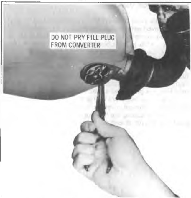
Fig. 6F-6 — Removing Pressed Plug With Pliers
