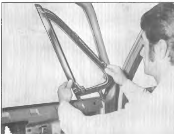
Fig. 2D-29--Removing Ventilator Assembly
