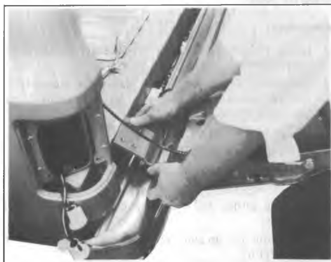
Fig. 2D-63--Pulling Hinge Away From Body (Utility)
