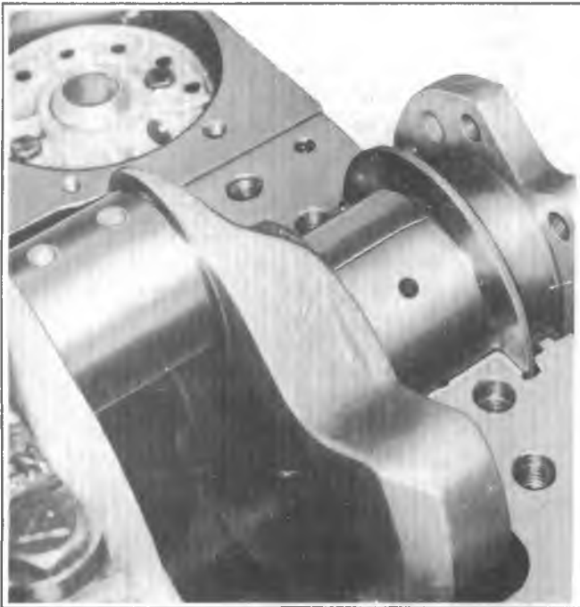
Fig. 6A1-30--Gaging Plastic on Journal - Typical
