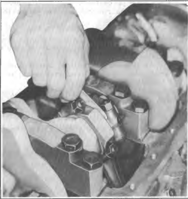
Fig. 6A4-42--Measuring Connecting Rod Side Clearance
