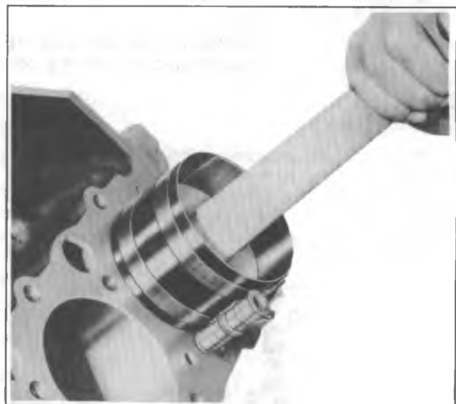
Fig. 6A4-58--Installing Connecting Rod Piston Assembly
