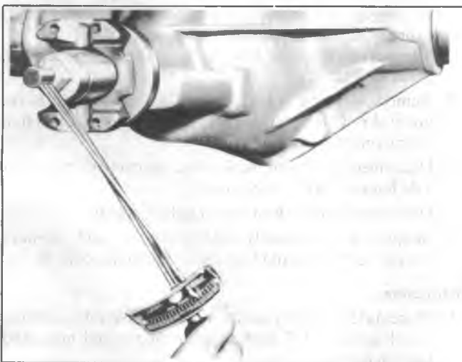
Fig. 4B-24--Measuring Pinion Rotating Torque
