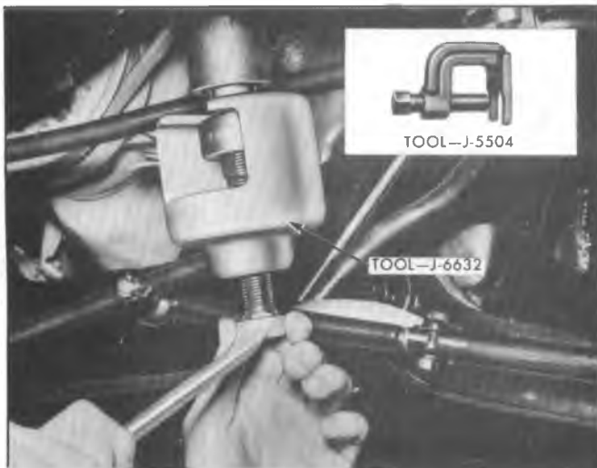
Fig. 3B2-9--Removing Pitman Arm-Typical
