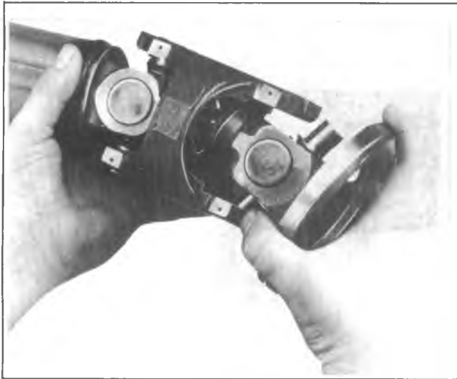
Fig. 4A-29--Reassembling Flange Yoke
