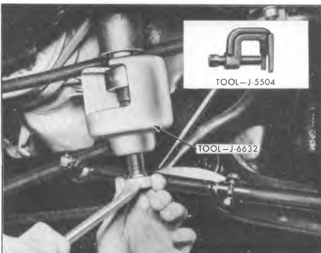
Fig. 3B3-13--Removing Pitman Arm
