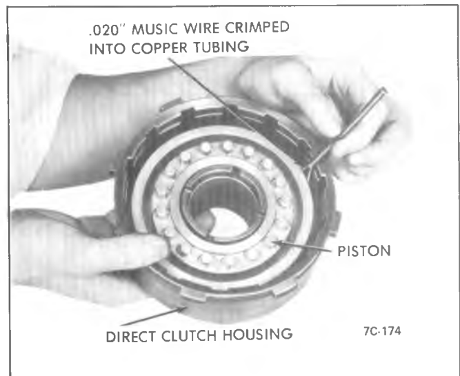
Figure 350C-86 Install Piston
