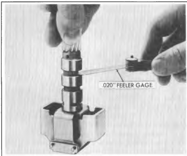
Figure400-50 Checking Valve Opening - Weights Extended
