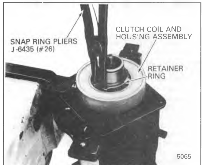
Fig. 1D-15 Removing A-6 Coil Housing Retainer Ring
