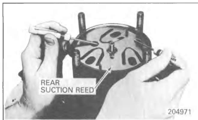
Fig. 1D-27 Removing A-6 Rear Suction Reed
