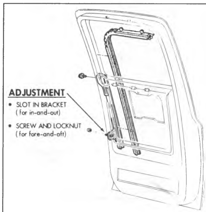
Fig. 2D-45--Glass Run Channel Adjustment
