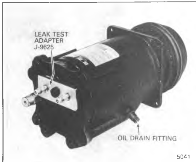
Fig. 1D-22 Leak Testing A-6 Compressor
