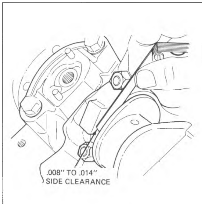
Fig. 45--Measuring Connecting Rod Side Clearance
