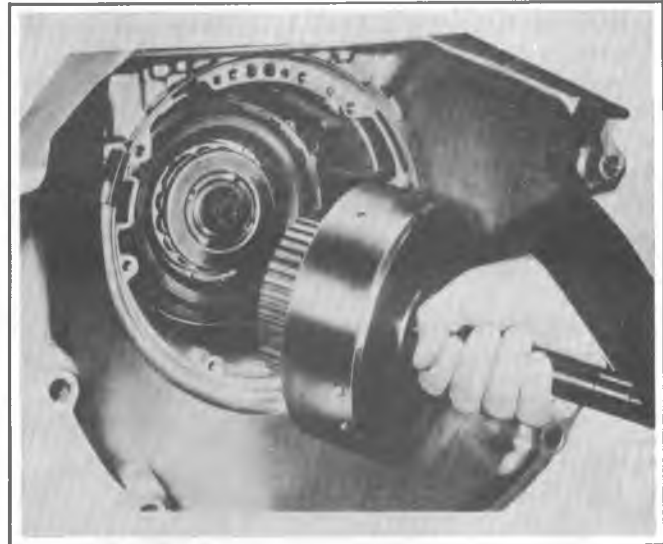
Figure 400-106 Installing Forward Clutch Assembly
