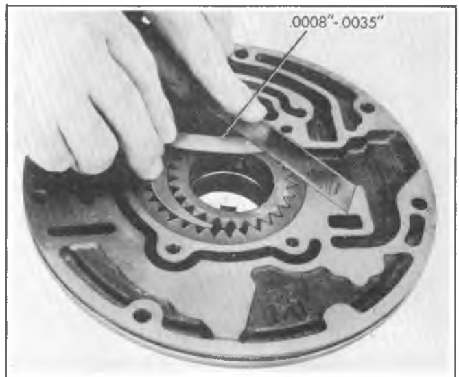
Figure 400-61 Pump Body Face to Gear Face Clearance
