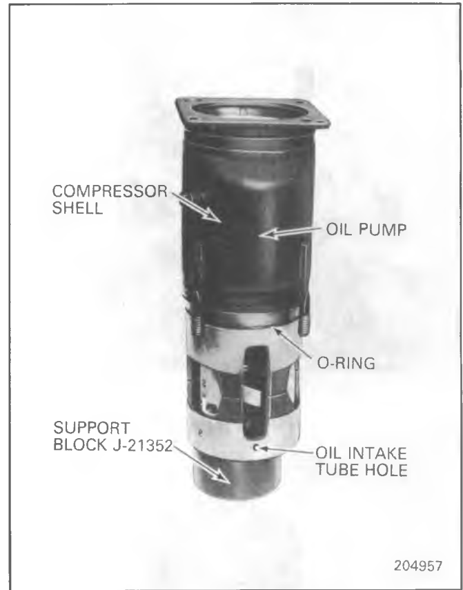
Fig. 1D-63 Installing A-6 Compressor Shell
