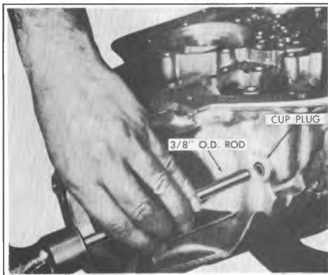
Figure 400-99 Installing Cup Plug
