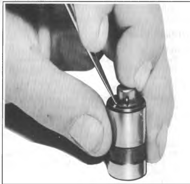
Fig. 6A1-14--Installing Ball Check Valve
