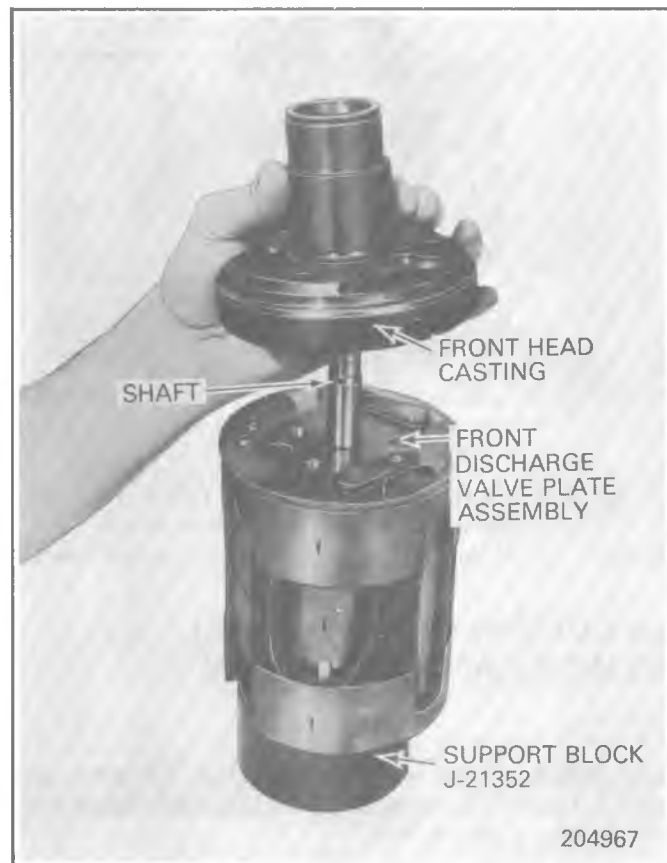
Fig. 1D-61 Installing A-6 Front Head Casting
