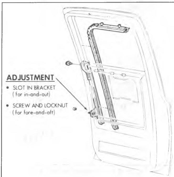
Fig. 2D-45--Glass Run Channel Adjustment
