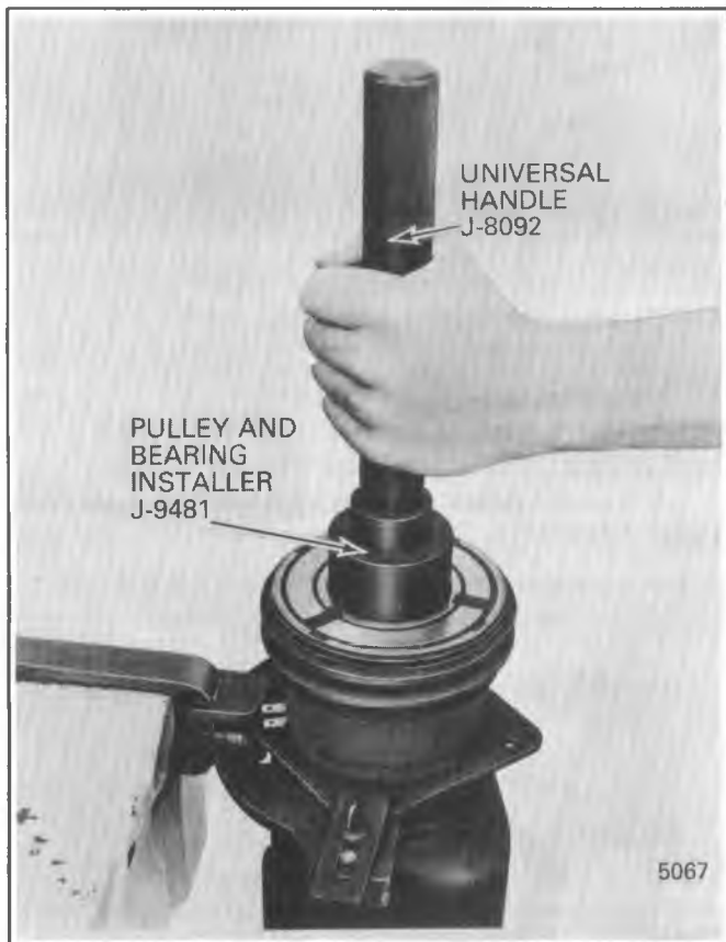
Fig. 1D-11 Installing A-6 Pulley and Bearing Asm.
