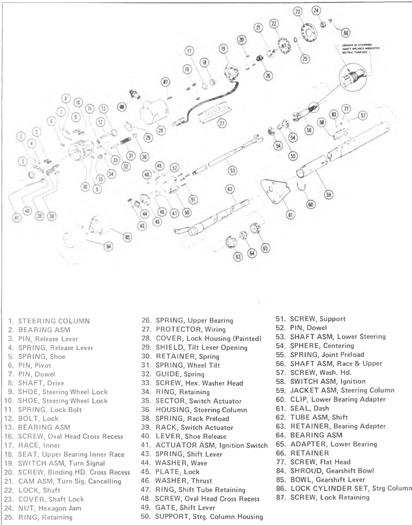
Fig. 3B4-49a--Tilt Column With Auto. Trans.
