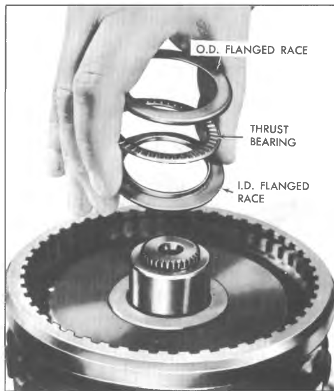
Fig. 7A-144C--Installing Rear Internal Gear to Output Shaft Bearing and Races
