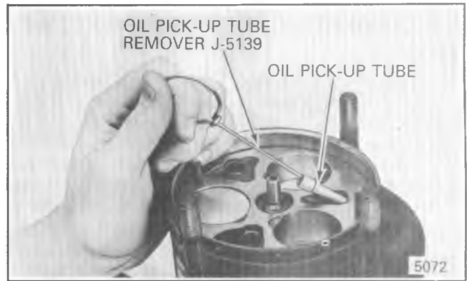
Fig. 1D-28 Removing A-6 Oil Pick-Up Tube
