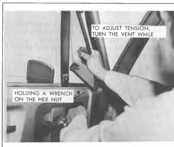
Fig. 2D-30--Adjusting Tension
