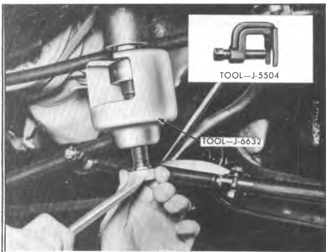
Fig. 3B3-13--Removing Pitman Arm
