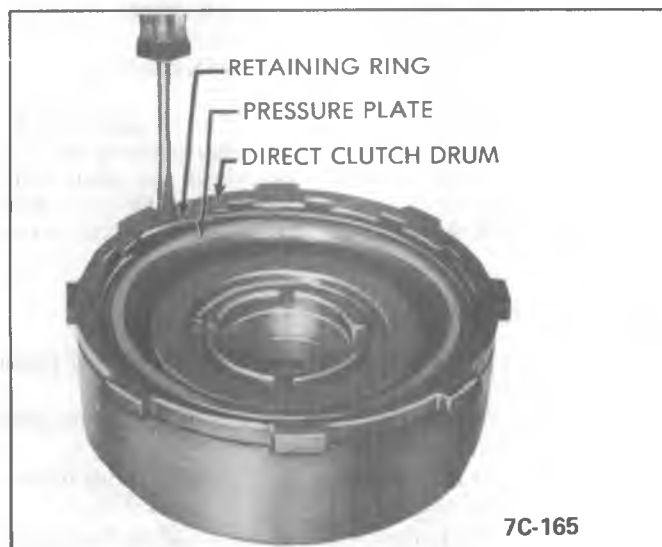
Figure 350C-80 Disassembly of Direct Clutch
