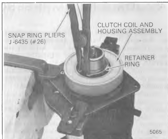
Fig. 1D-15 Removing A-6 Coil Housing Retainer Ring
