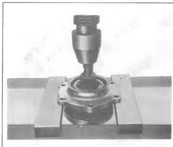
Fig. 4B2-16--Pressing Drive Pinion from Bearing Retainer
