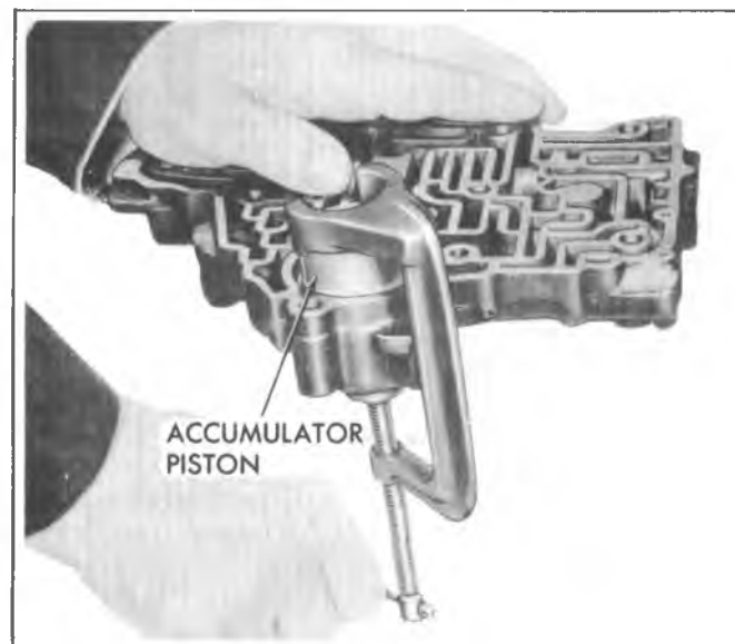
Fig. 7A-65C--Installing Compressor Tool to Front Accumulator Piston
