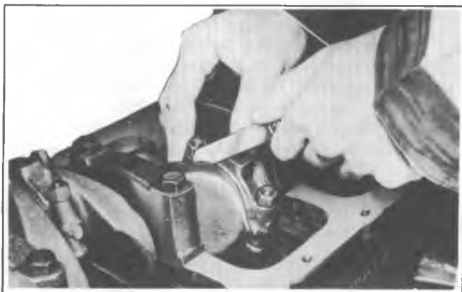
Fig. 6A1-29--Measuring Connecting Rod Side Clearance
