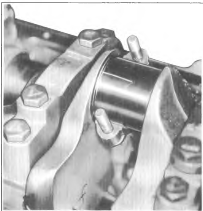
Fig. 6A4-40--Gaging Plastic On Crankpin
