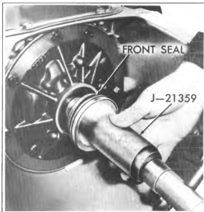
Fig. 7A-168C--Installing Pump Seal
