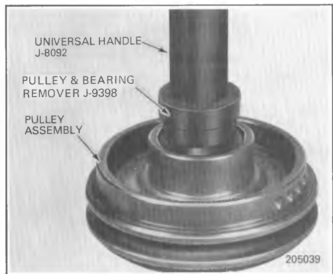
Fig. 1D-13 Removing Bearing From A-6 Pulley Asm.
