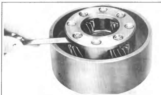
Fig. 7A-128C--Checking Pinions End Play
