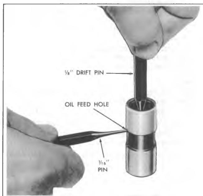
Fig. 6A1-15--Assembling Hydraulic Lifter
