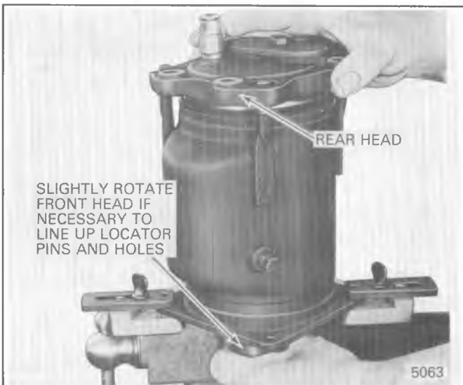
Fig. 1D-67 Installing A-6 Rear Head
