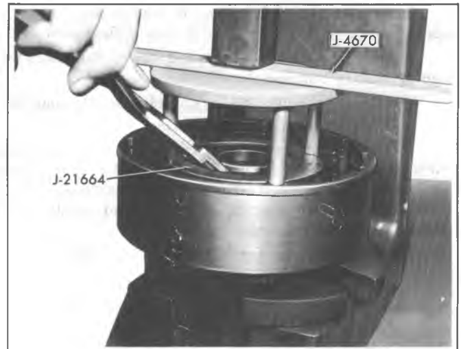
Fig. 7A-94C--Removing or Installing Direct Clutch Snap Ring
