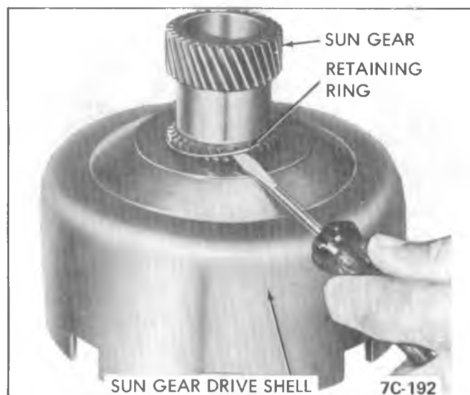
Figure 350C-102 Sun Gear Retaining Ring Removal
