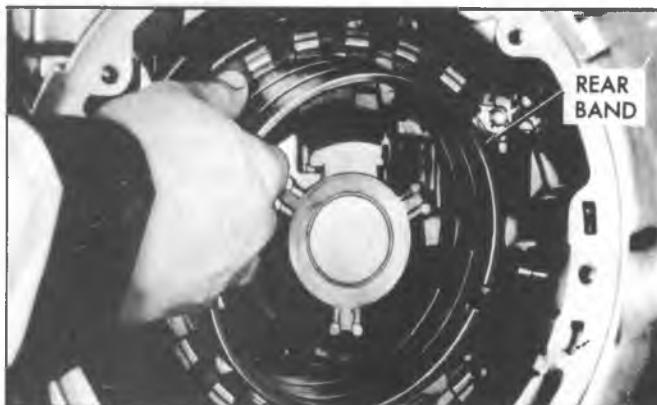
Fig. 7A-156C--Installing Rear Band
