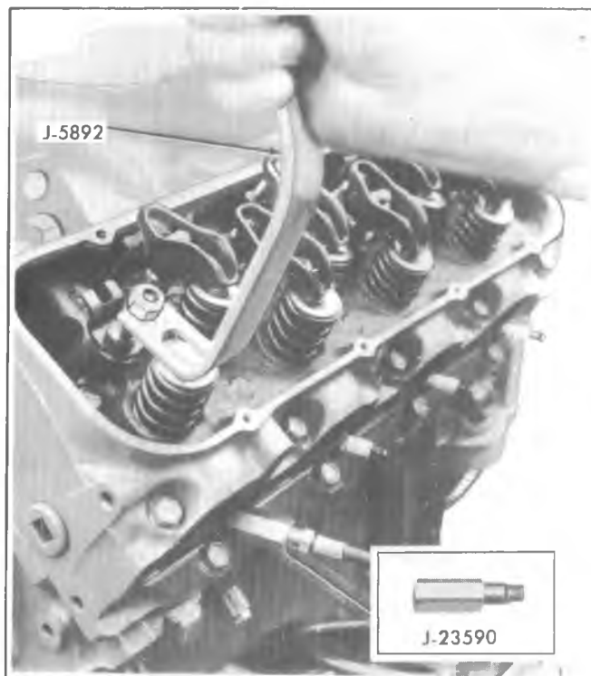
Fig. 6A5-12--Compressing Valve Spring
