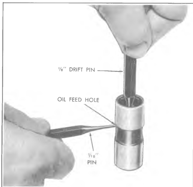
Fig. 6A4-17--Assembling Hydraulic Lifter
