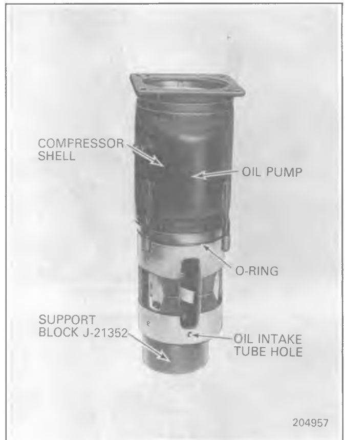
Fig. 1D-63 Installing A-6 Compressor Shell
