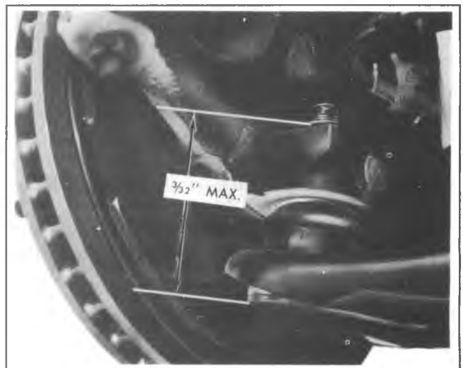
Fig. 3C-29--Checking Lower Ball Joint
