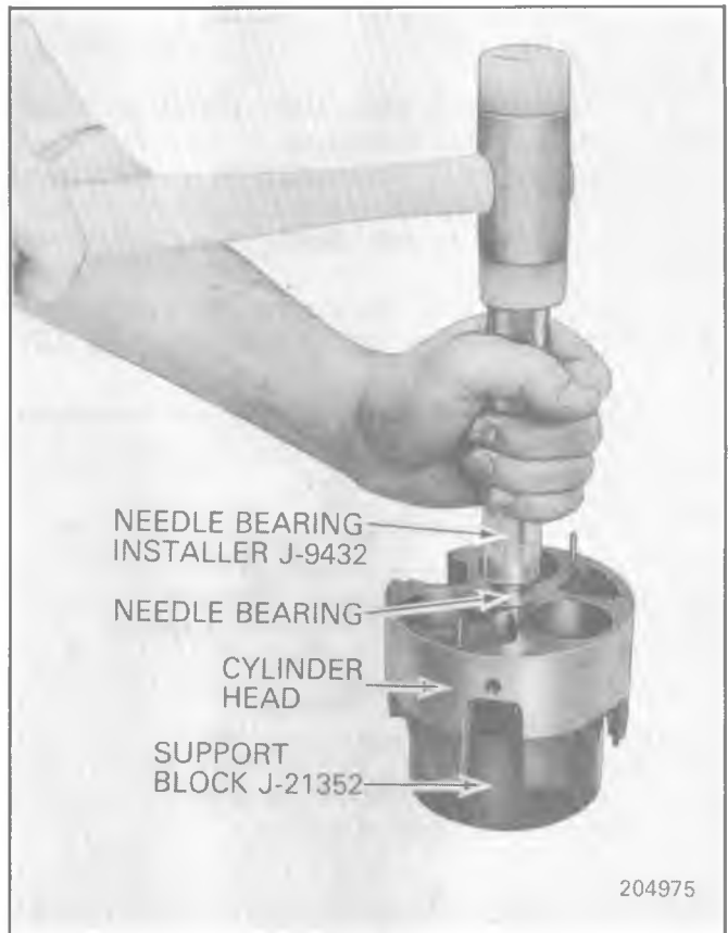
Fig. 1D-35 Installing A-6 Needle Bearing
