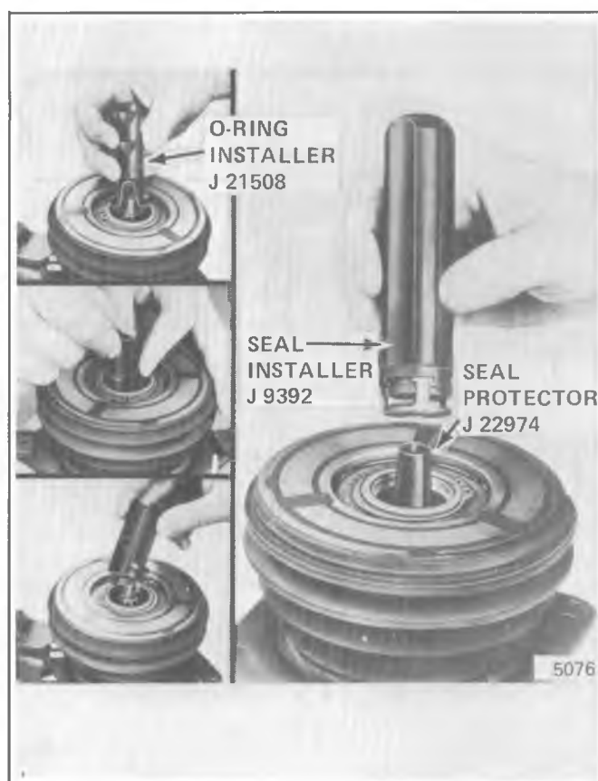
Fig. 1D-20 Replacing A-6 Seal and O-Ring
