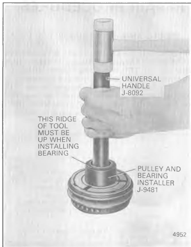
Fig. 1D-14 Installing Bearing on A-6 Pulley
