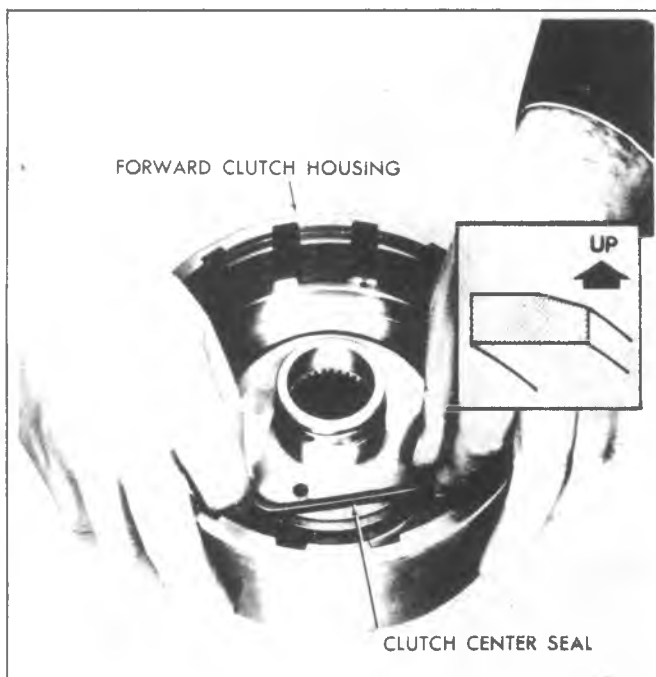
Fig. 7A-85C--Removing Forward Clutch Center Seal
