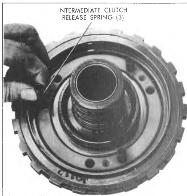
Fig. 7A-115C--Removing Clutch Release Springs
