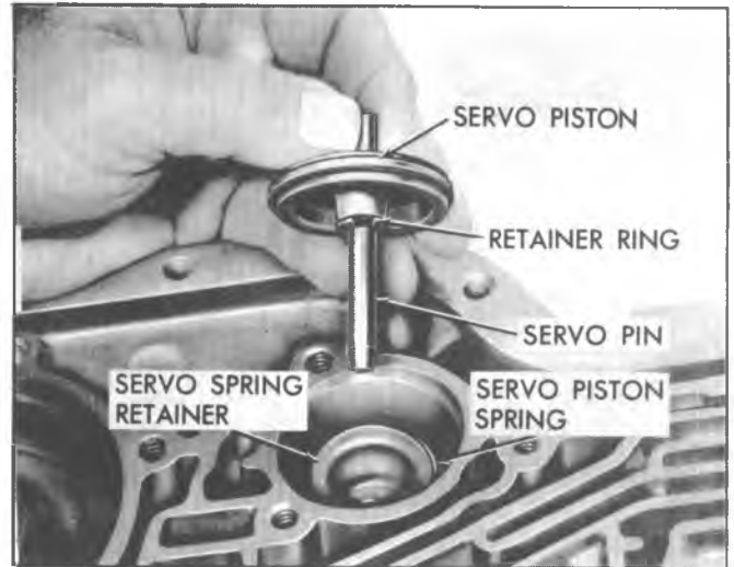
Fig. 7A-20C--Removing Front Servo Piston, Retainer Ring, and Pin
