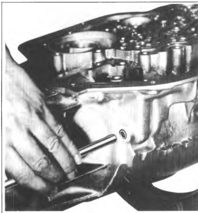
Fig. 7A-154C--Installing Parking Pawl Shaft Cup Plug
