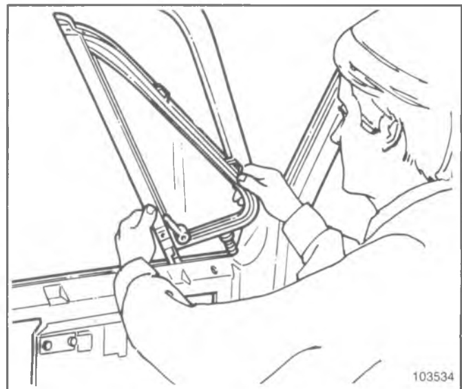
Fig. 10-29--Removing Ventilator Assembly
