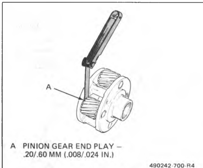
Figure 73 Pinion End Play Check
