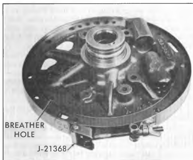
Figure 400-64 Aligning Pump Cover and Body
