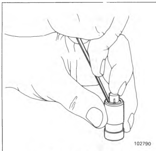
Fig. 6A5-16--Installing Ball Check Valve
