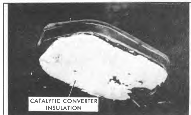
Fig. 6F-4--Catalytic Converter Insulation
