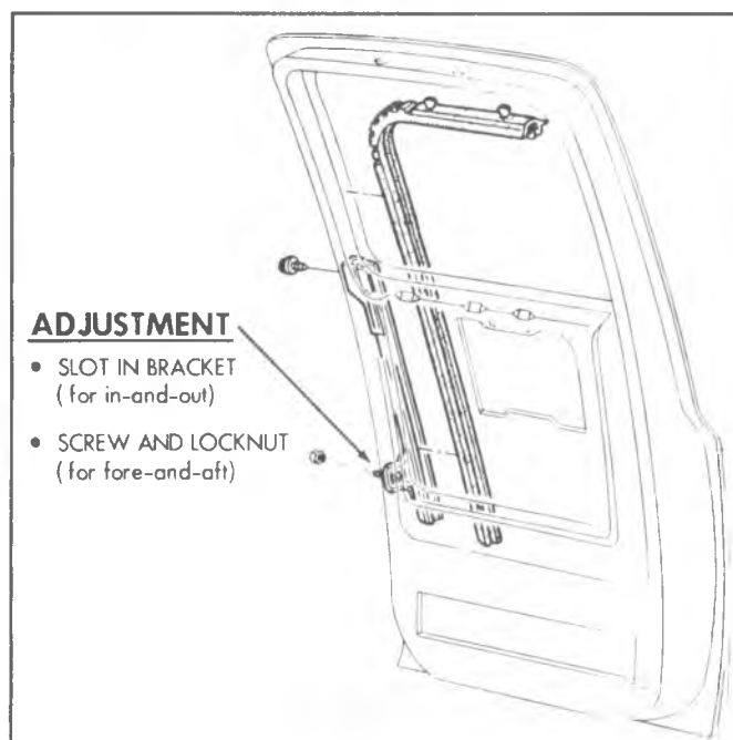
Fig. 10-45--Glass Run Channel Adjustment
