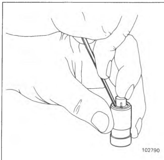
Fig. 6A1-14--Installing Ball Check Valve
