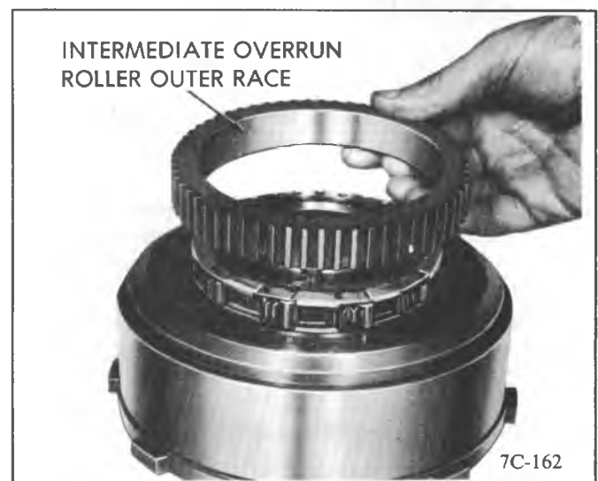
Figure 350C-54 Roller Clutch Outer Race
