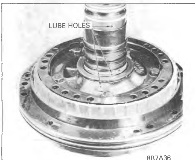
Figure 350C-52 Lube Hole Location
