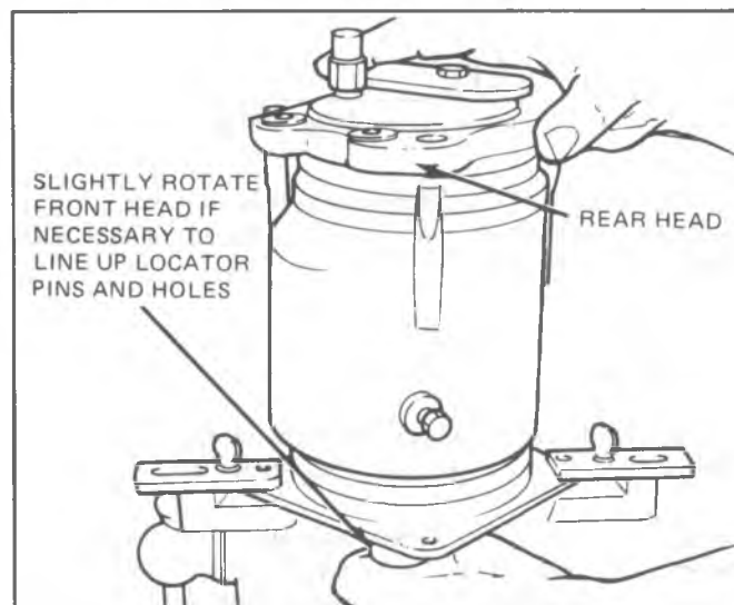
Fig. 1D-67 Installing A-6 Rear Head
