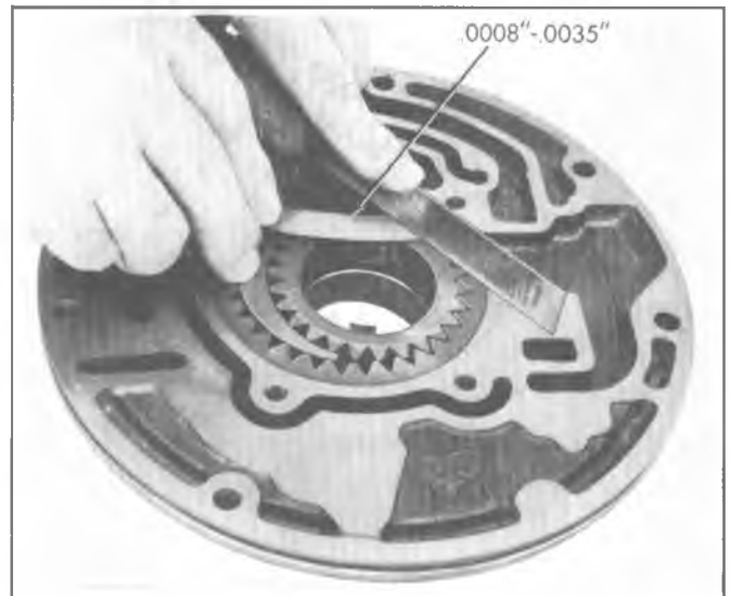
Figure 400-61 Pump Body Face to Gear Face Clearance
