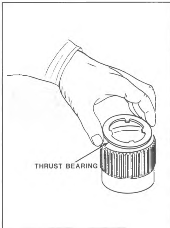
Fig. 3C-21K--Removing Thrust Bearing
