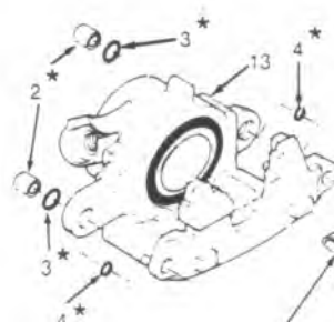
2. Sleeve 3. Bushing 4. Bushing 5. Outboard shoe & lining 6. Inboard shoe & lining 7. Wear sensor
