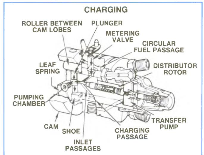
Figure 4-41, Pumping Chamber.
