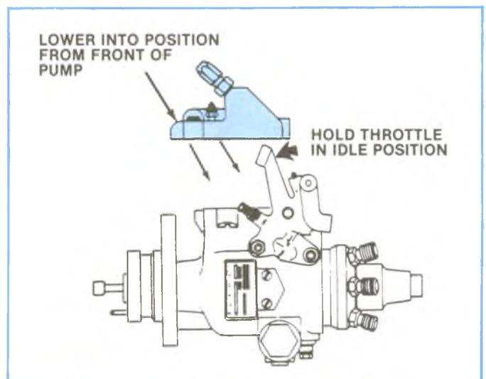
Figure 4-155, Installing Governor Cover.
