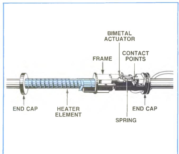
**Figure 4-15, Diesel Fuel Heater Components.**
