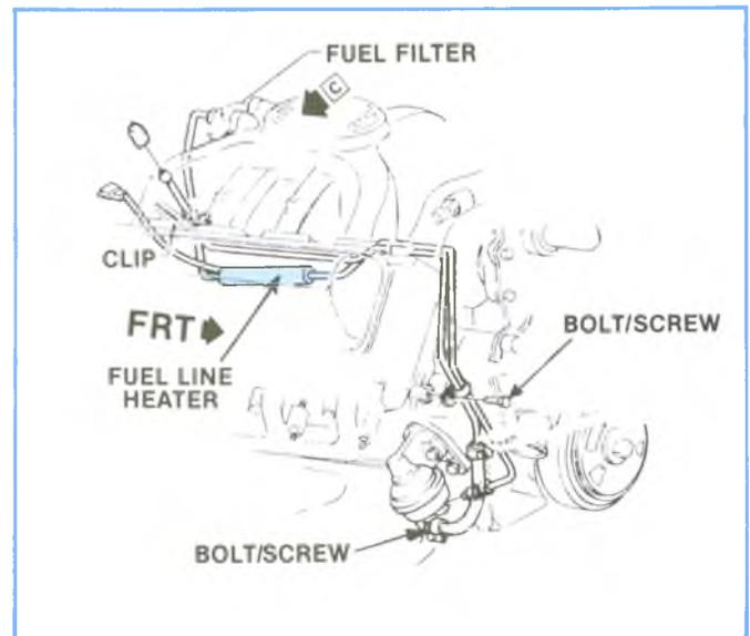
**Figure 4-14, Fuel Line Heater Installation.**
