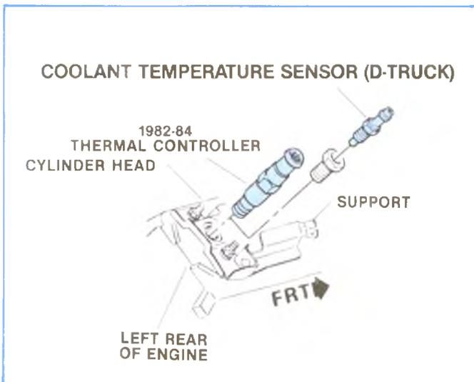
Figure 6-11, Thermal Controller.
