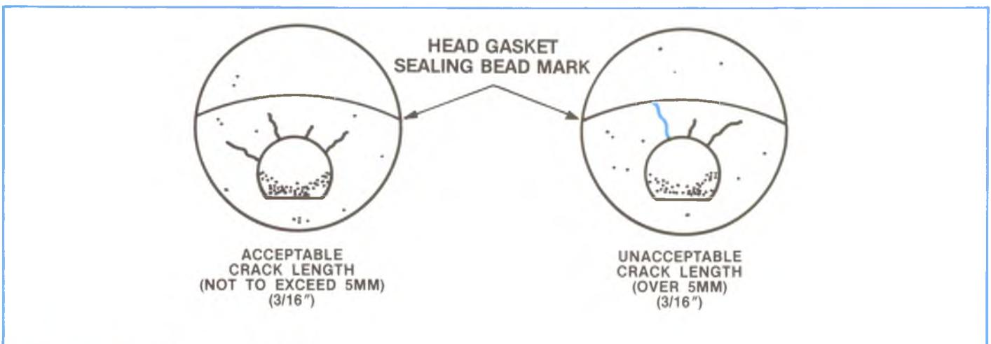
Figure 3-8, Pre-Chamber Cracks.
