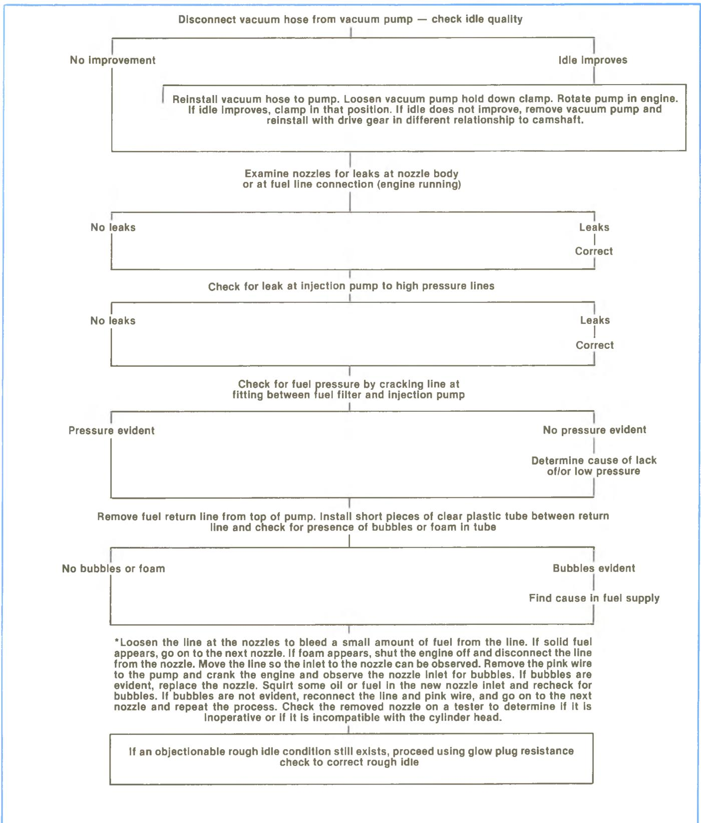
Figure 7-3, (Cont'd.) Diesel Engine Roughness Diagnosis Procedure.
