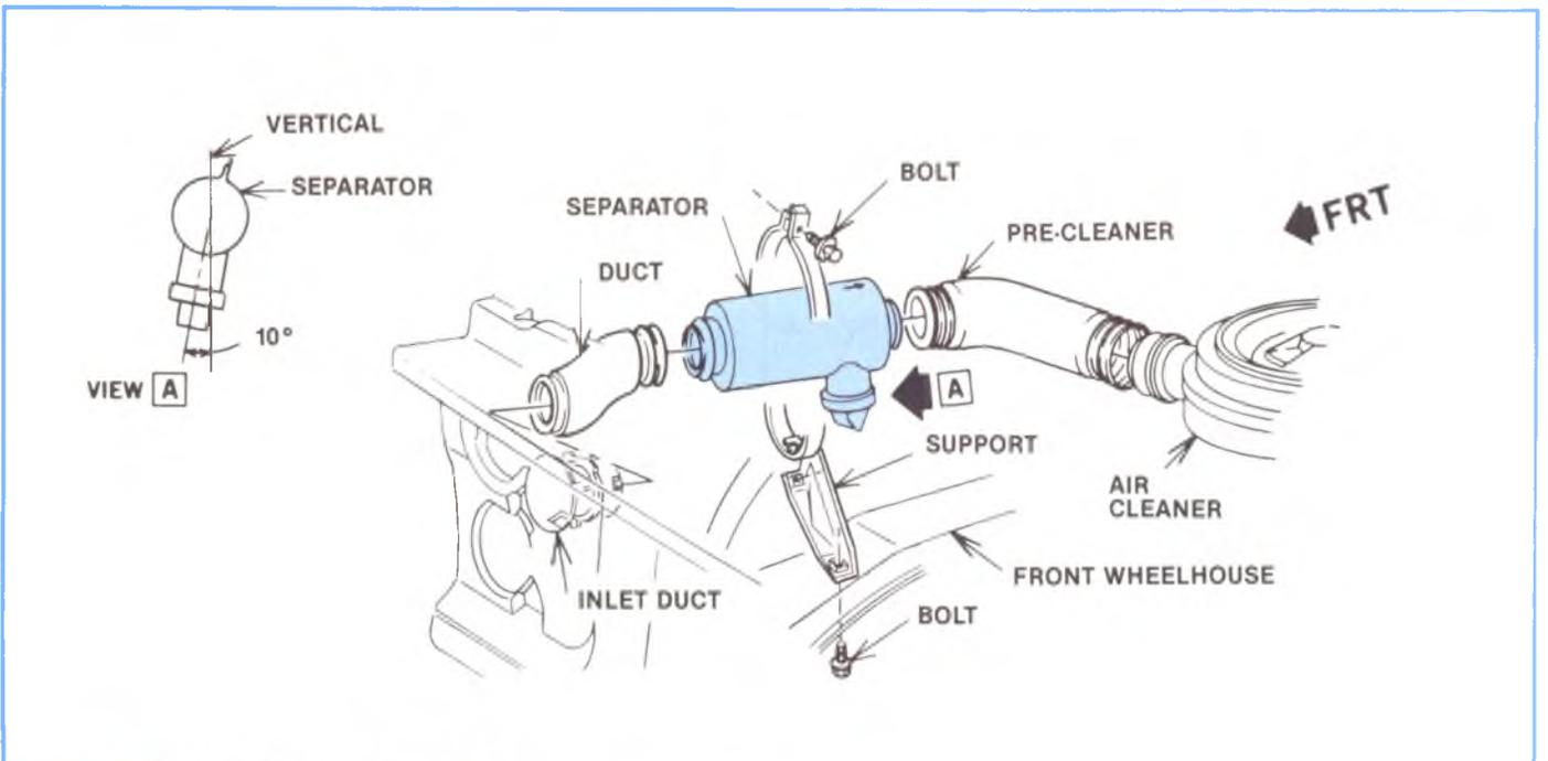
Figure 3-3. RPO K46 Air Pre-Cleaner Chamber.
