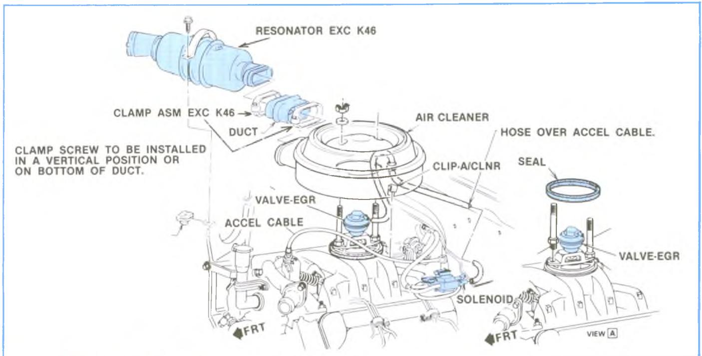
Figure 3-1, LH6 Air Intake System With EGR Valve
