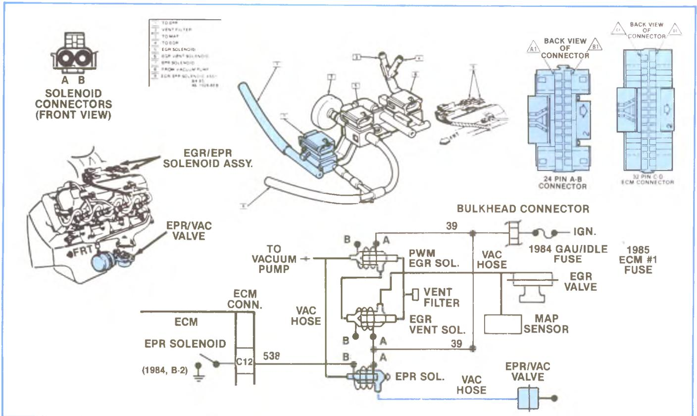
**Figure 5-49, EPR Solenoid Schematic (1984 & 1985).**
