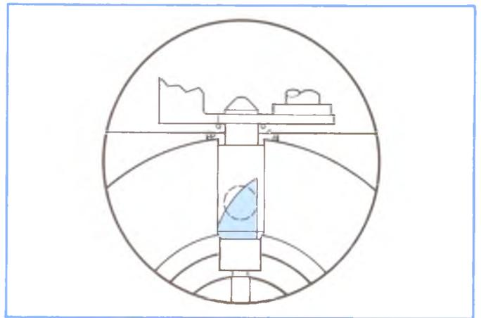
Figure 4-38, Metering Valve Full Load.
