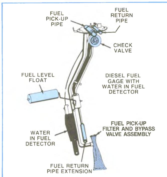
**Figure 4-4, Fuel Pickup/Sending Unit With Water-in-Fuel Warning.**
