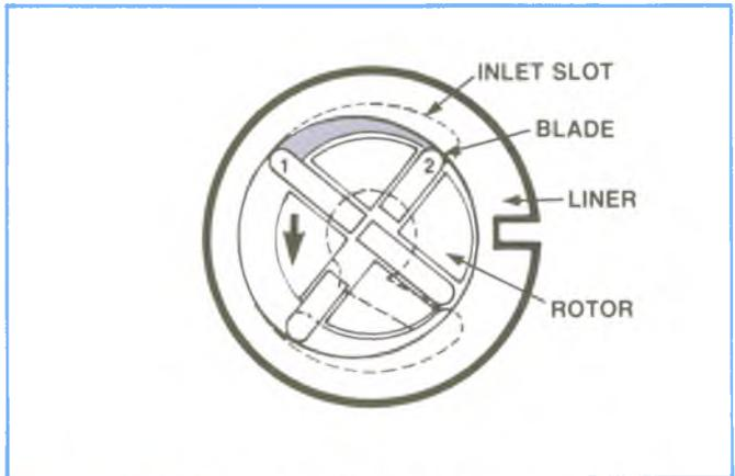
Figure 4-46, Transfer Pump Construction.
