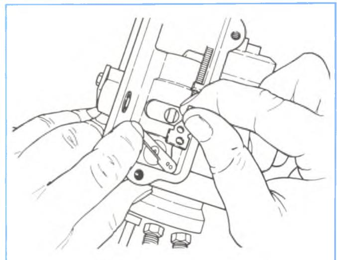
Figure 4-95, Disengaging Linkage Hook.
