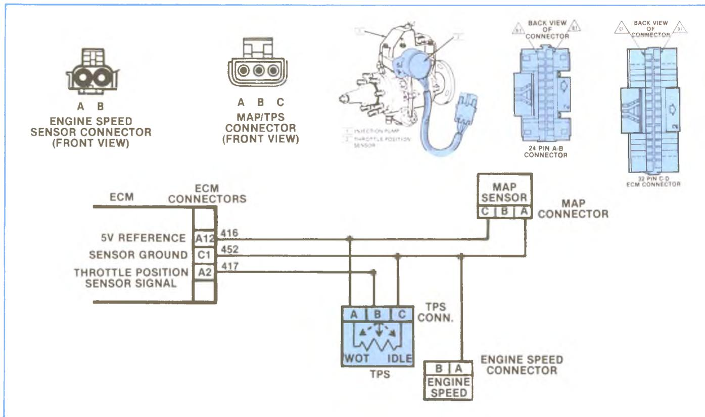
Figure 5-63, 1985 TPS Schematic.
