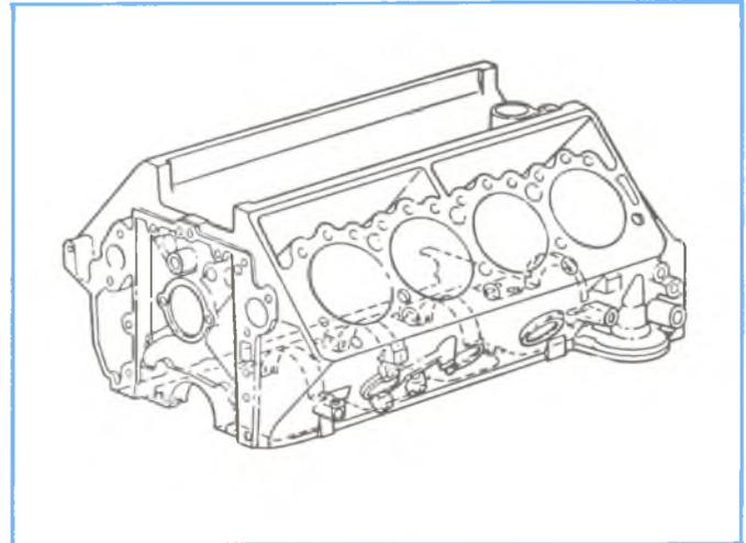
Figure 2-1, Cylinder Case.
