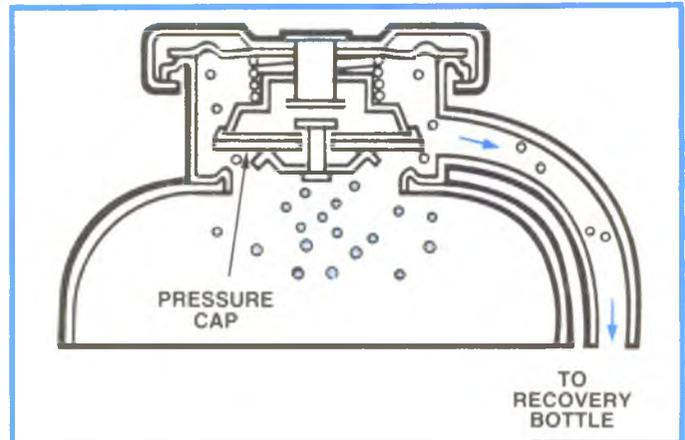
Figure 2-52, Radiator Cap With Pressure Valve Open.
