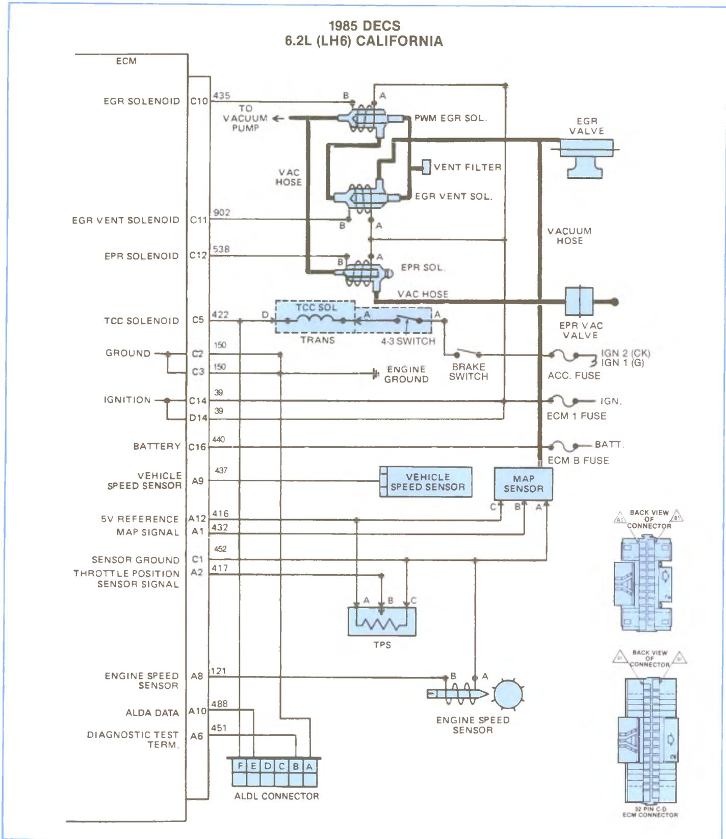
Figure 5-79, 1985 California (DECS) Diesel ECS Wiring Schematic.
