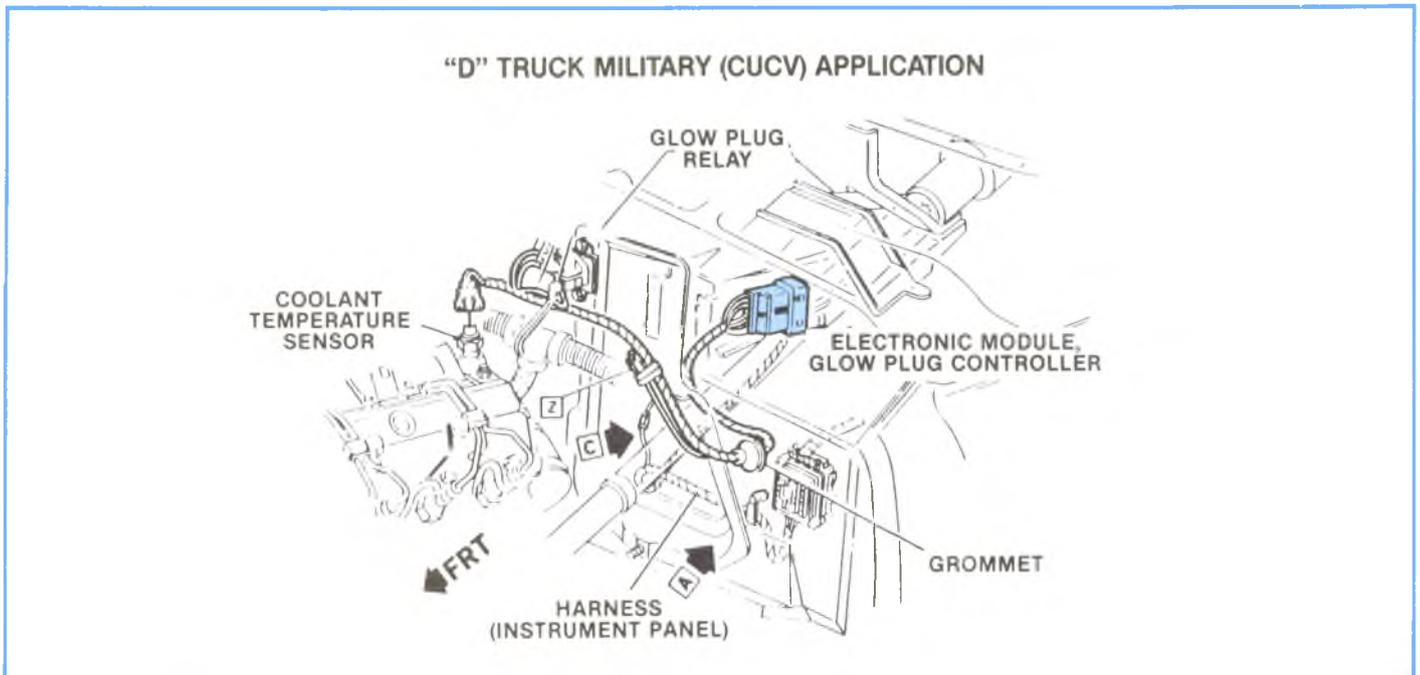
Figure 6-13, Electronic Module Glow Plug Controller (D-Truck).
