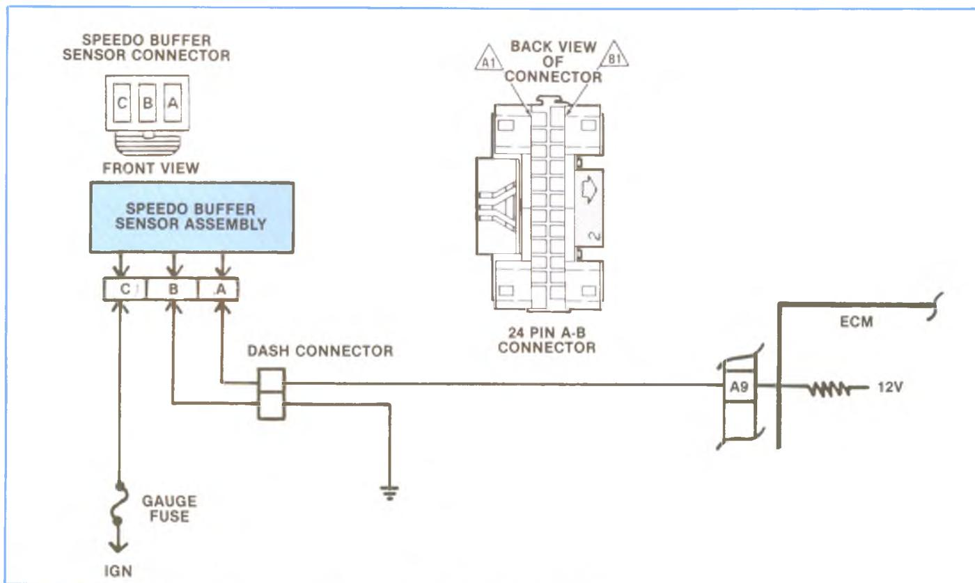
Figure 5-70, VSS Wiring Diagram — Code 24 (1985 only).
