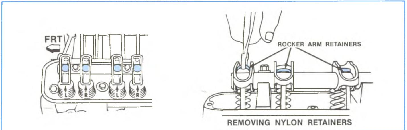
Figure 2-5, 1985 and Later Rocker Arm Assembly.
