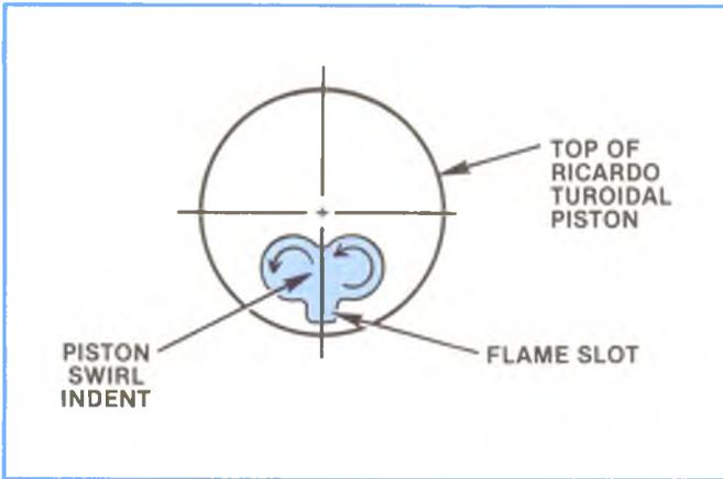
This piston has a half-clover shaped indentation on the piston face, which at T.D.C. outlets to the pre-chamber, Figure 2-19. As the piston rises during the compression stroke, the air swirl begins in these two indentations. When the piston reaches the pre-chamber opening, the air swirl is increased in the spherical pre-chamber. This is a Ricardo Turoidal Piston design and is used with the Ricardo COMET V Pre-Chamber for more complete mixing of the air and fuel.
