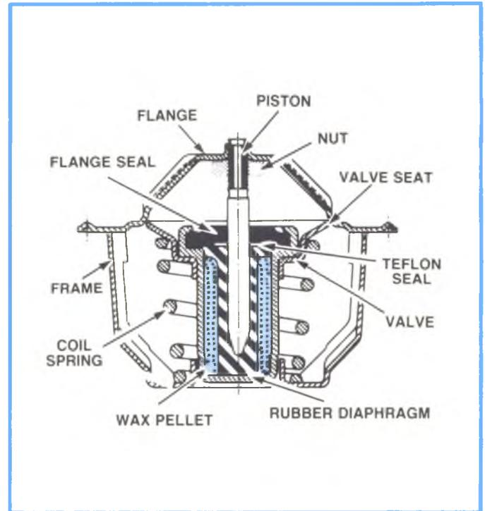
Figure 2-56, Thermostat Construction.
