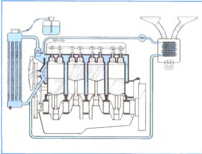
**Figure 2-43, Cooling System.**
