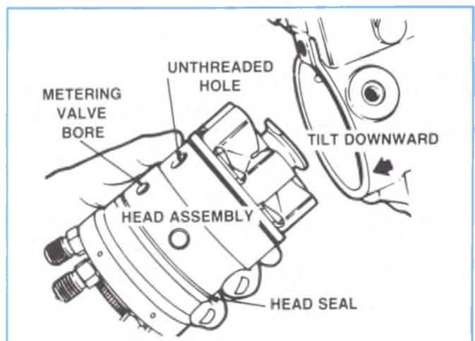
**Figure 4-130, Cam Positioning.**
