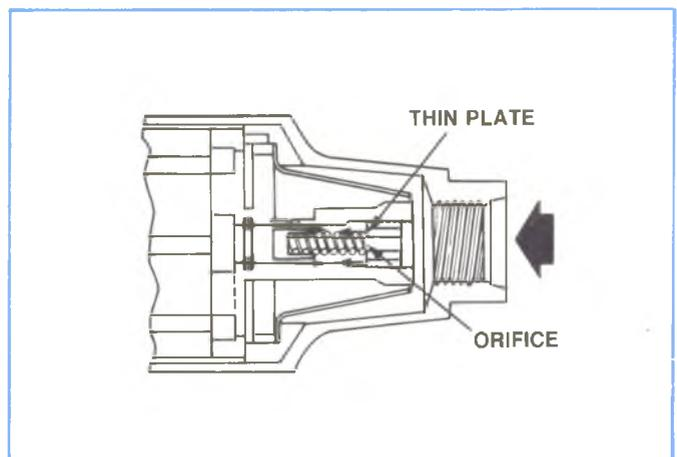
Figure 4-54, Orifice Control.
