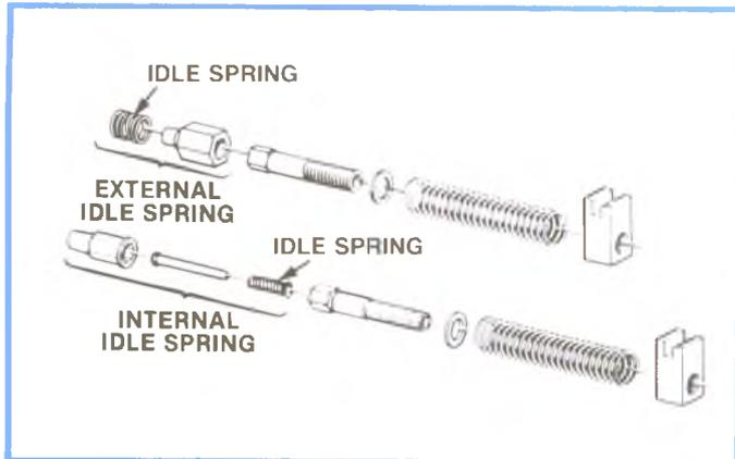
Figure 4-74, Internal Idle Spring Design.
