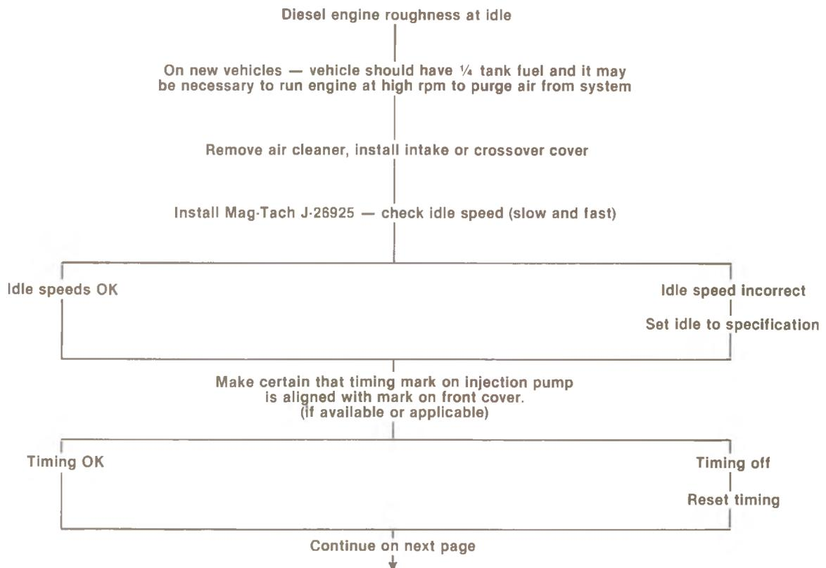
Figure 7-3, Diesel Engine Idle Roughness Diagnosis Procedure.
