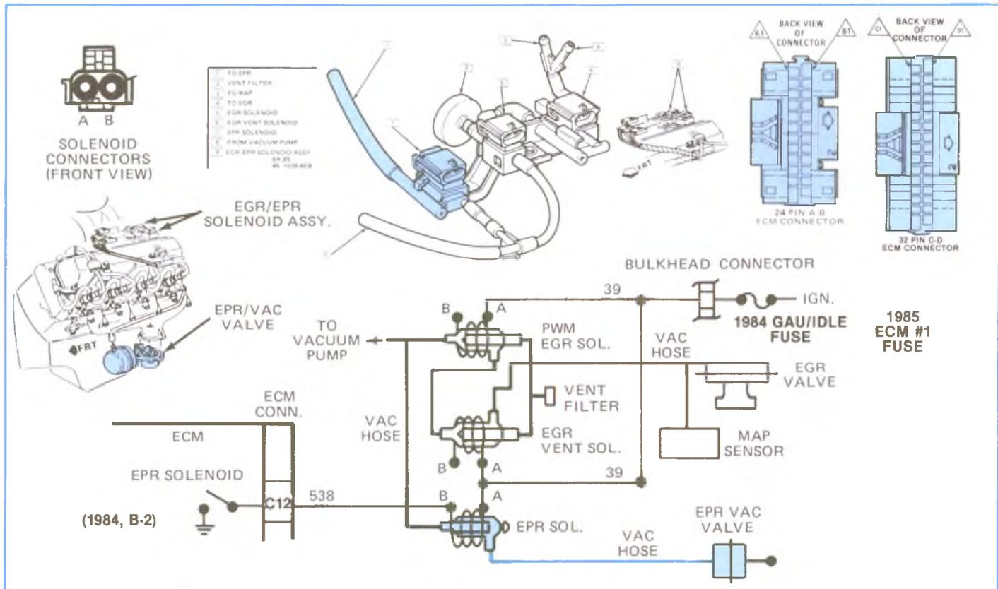
**Figure 5-51, EPR Solenoid Schematic (1984 & 1985).**
