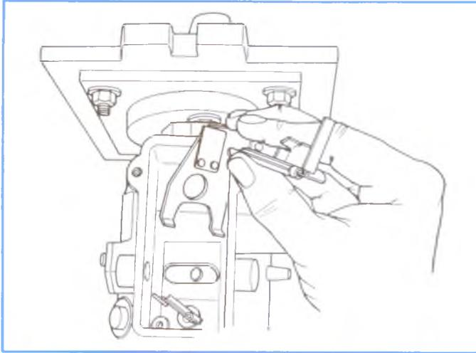
**Figure 4-96, Removing Governor Arm and Linkage (Late Model).**
