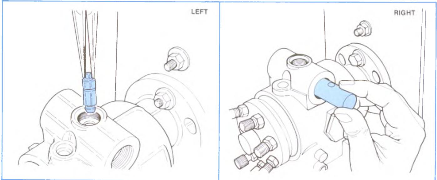
**Figure 4-107, Removing Cam Advance Pin and Advance Piston.**
