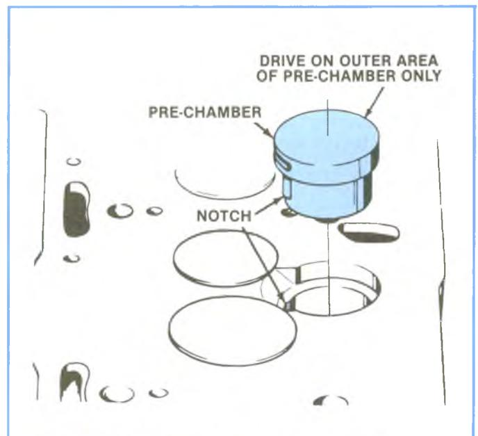
Figure 3-7, Pre-Chamber Installation in Cylinder Head.
