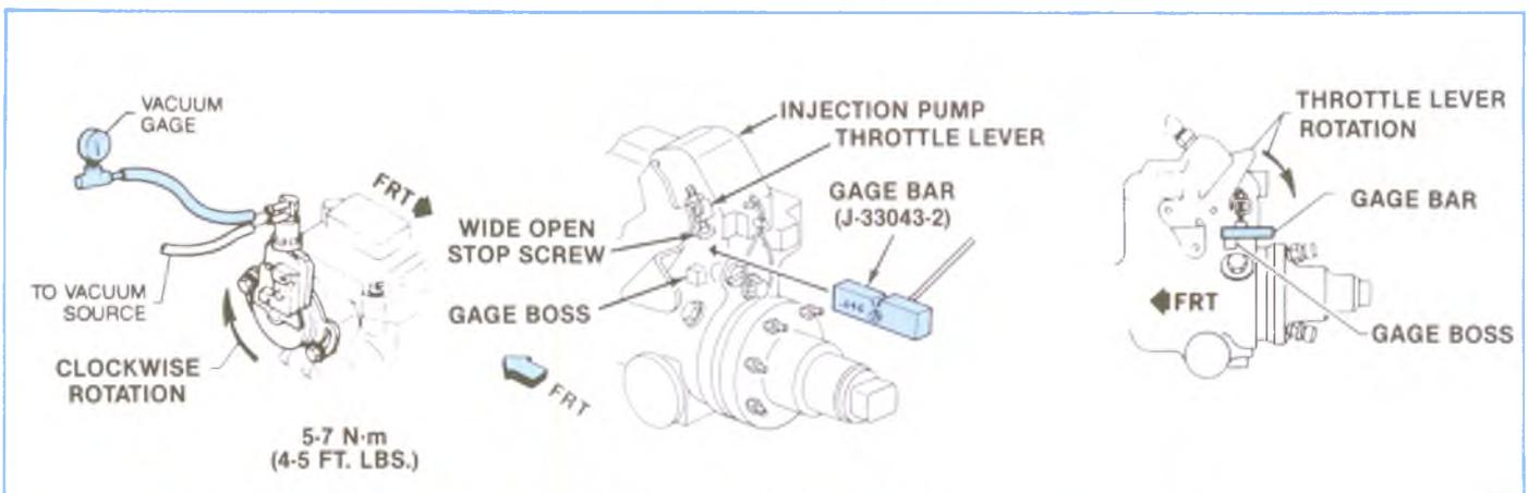
Figure 5-19, VRV Adjustment LL4-Model With THM 400 (M40) Transmission.
