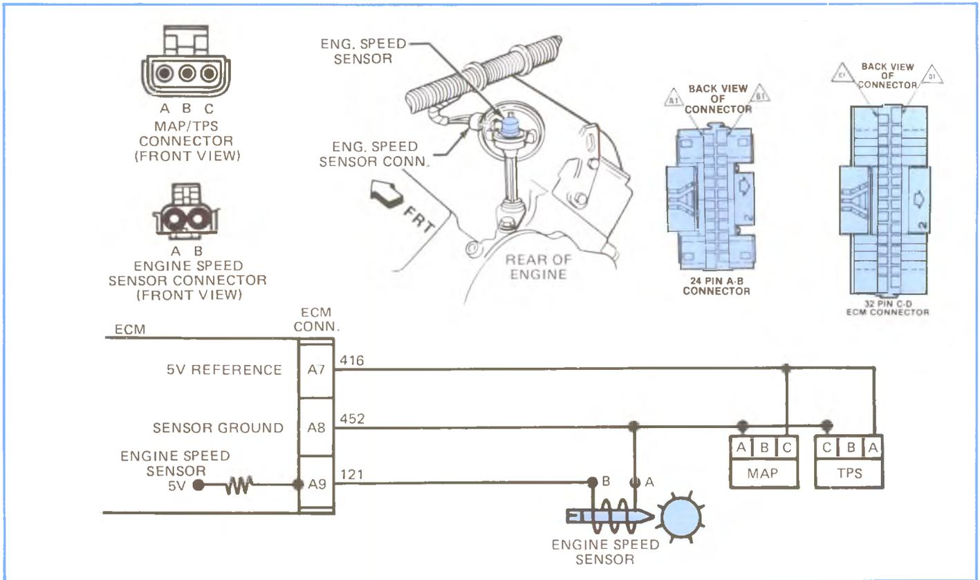
**Figure 5-41, 1984 Engine Speed Sensor Check Schematic.**
