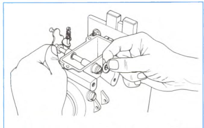
Figure 4-94, Removing Throttle Assembly.
