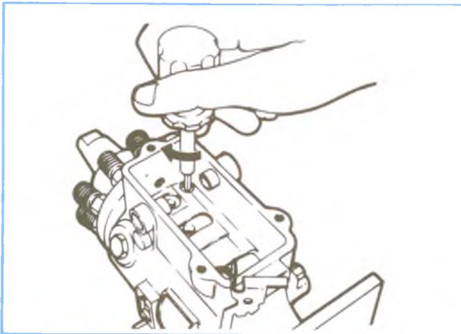
Figure 4-136, Installing Vent Wire Assembly.
