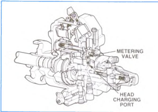
Figure 4-36, Metering Valve.
