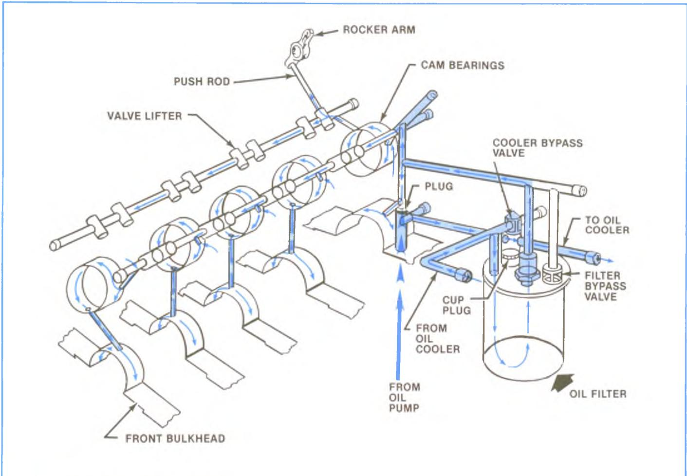
Figure 2-33, Lubrication System.
