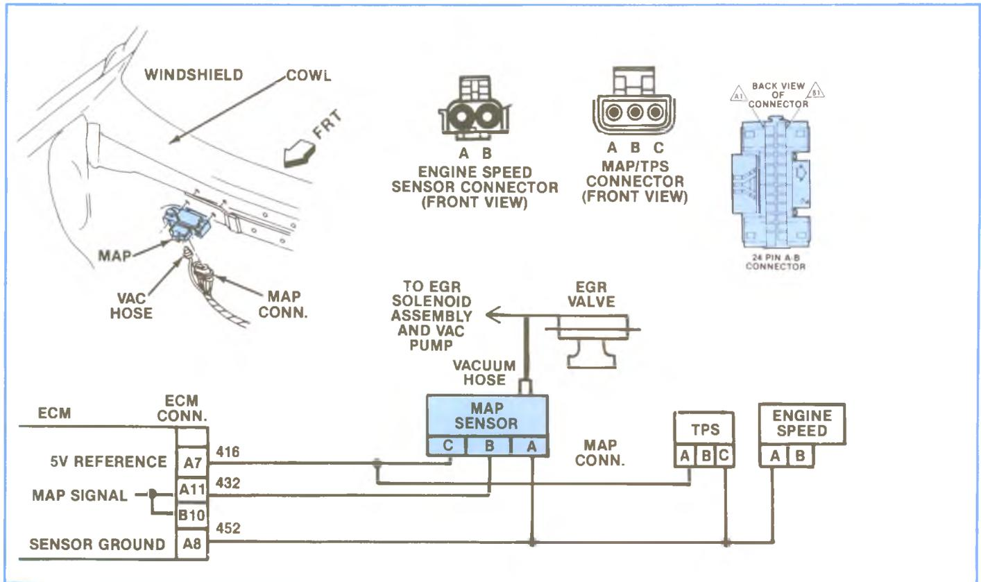
Figure 5-54, 1984 (Only) MAP Sensor Check Schematic.
