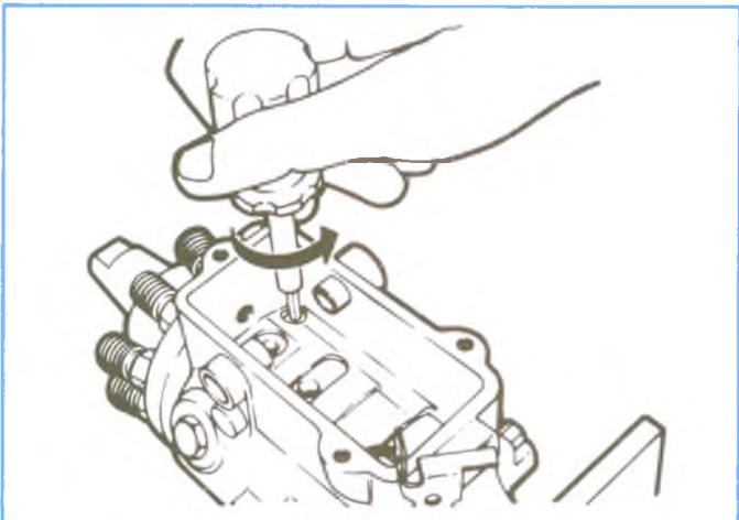
**Figure 4-98, Removing Vent Wire Assembly.**
