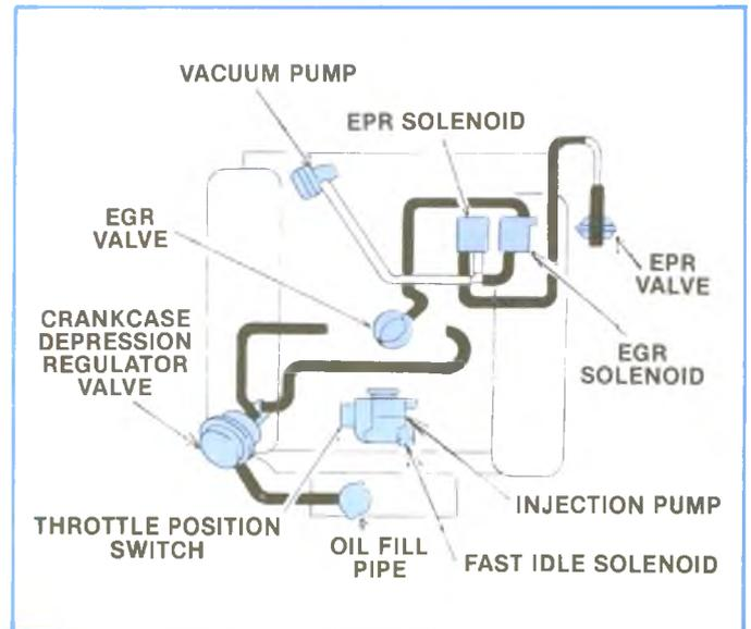
Figure 5-2, Emission Systems — Federal CK (LH6 Engine).
