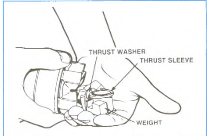
Figure 4-109, Governor Disassembly.
