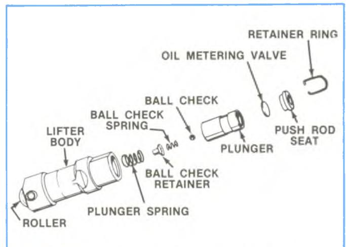
Figure 2-8, Valve Lifter Disassembled.
