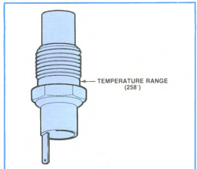
Figure 2-54, Temperature Switch.
