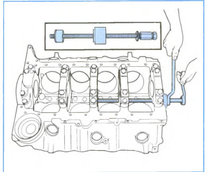
**Figure 2-28, Removing or Replacing Camshaft Bearings**
