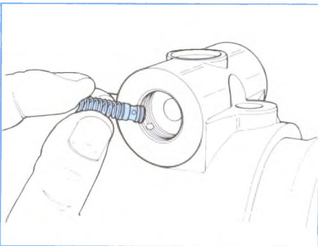
**Figure 4-146, Installing Servo Valve.**
