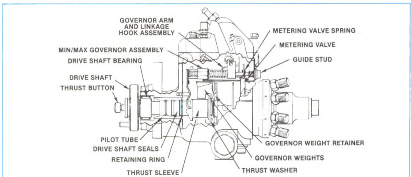
Figure 4-134, Installing Shaft in Pump.
