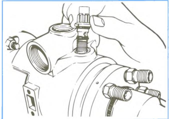
Figure 4-142, Installing Head Locating Screw.
