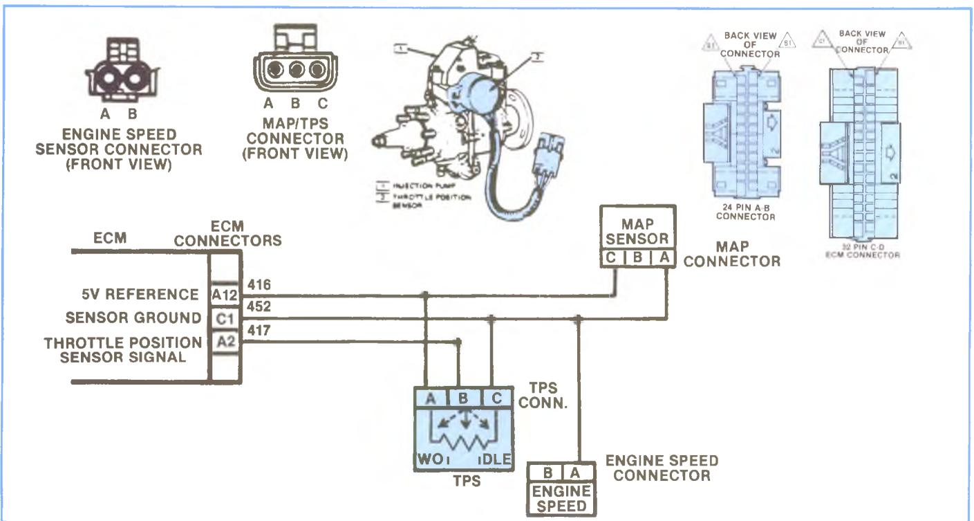
Figure 5-62, 1985 TPS Schematic.
