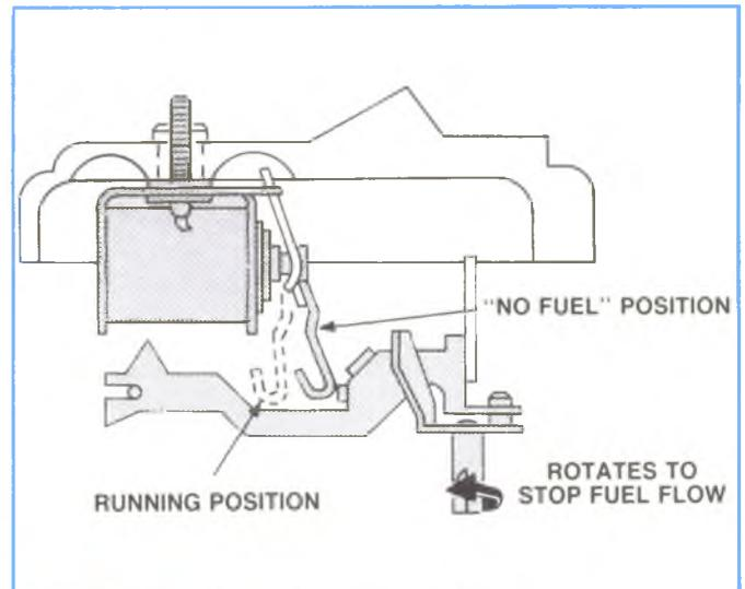
Figure 4-57, Shutoff Solenoid.
