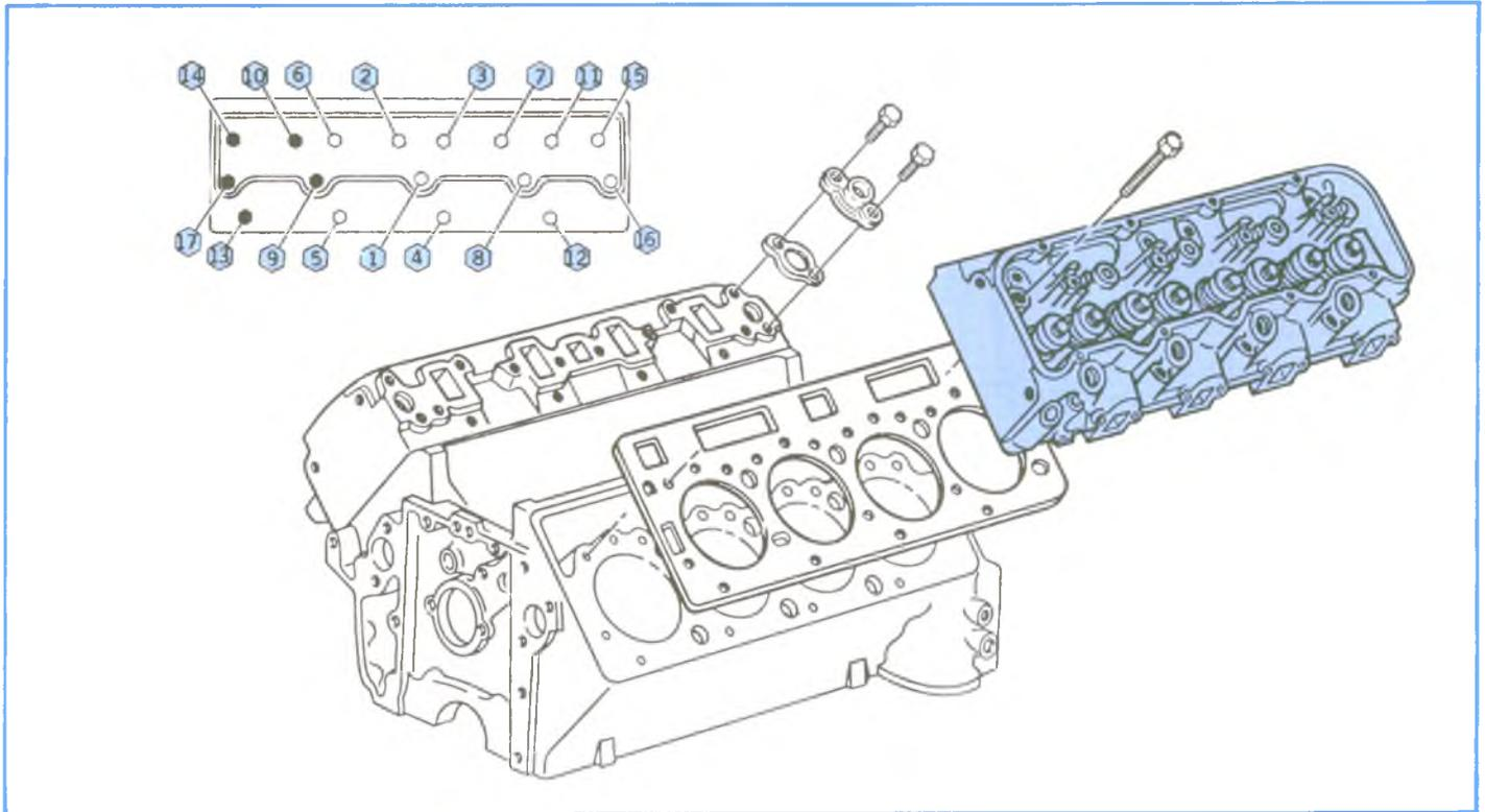
Figure 2-12, Cylinder Head.
