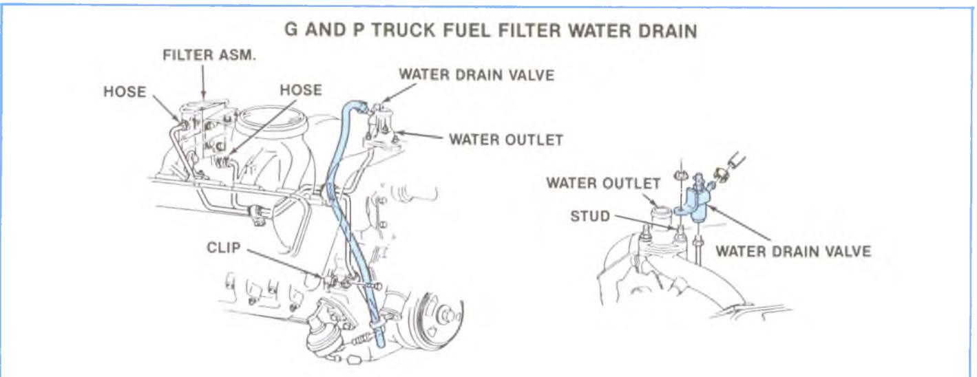
Figure 4-25, G-P Truck Remote Fuel Filter Water Drain.
