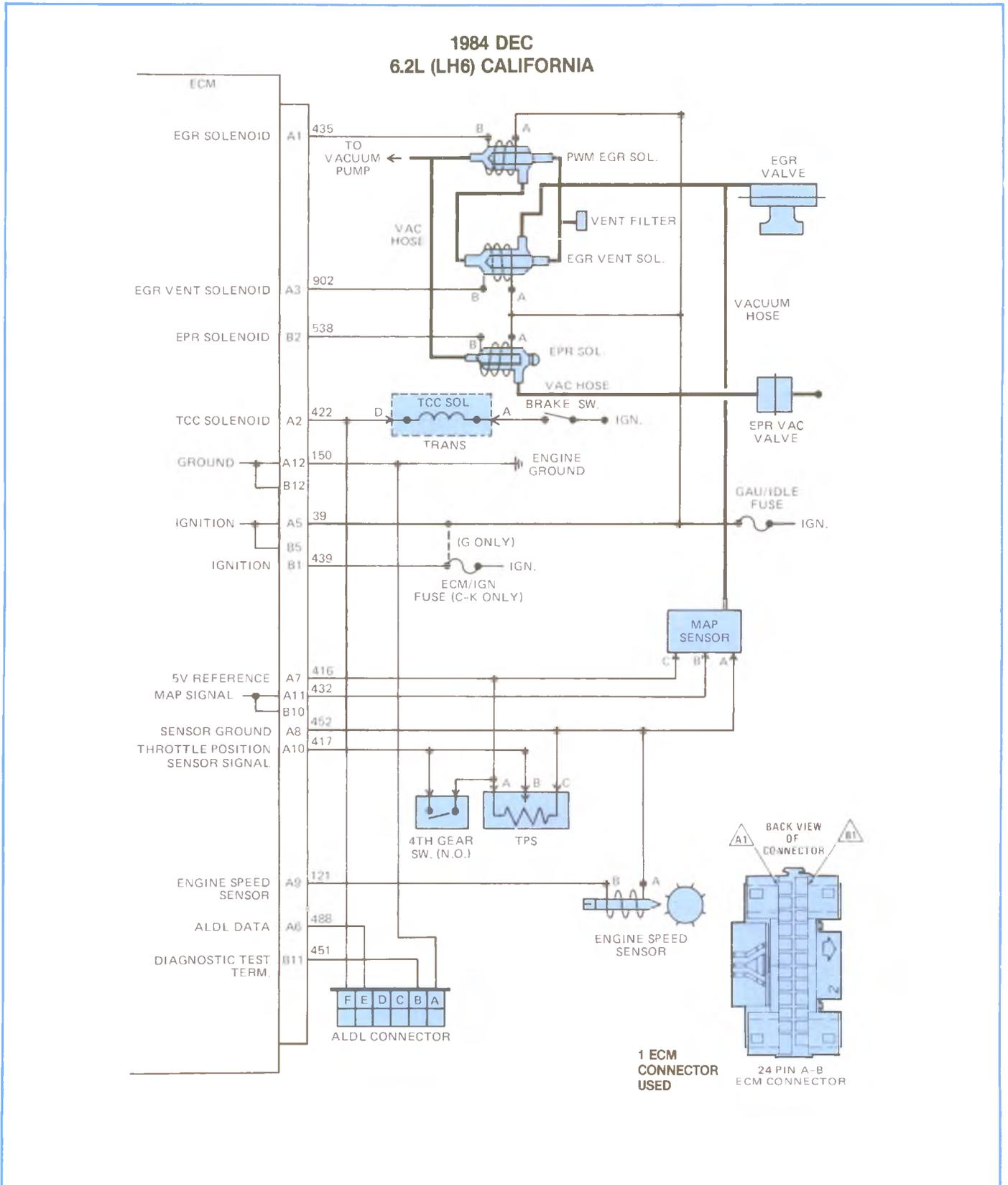
Figure 5-76, 1984 Calif. (DECS) Diesel Electronic Control System Wiring Schematic.
