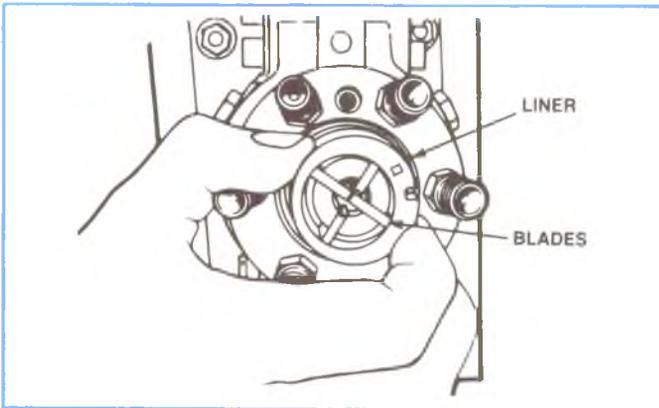
**Figure 4-102, Removing Transfer Pump Blades and Liner.**
