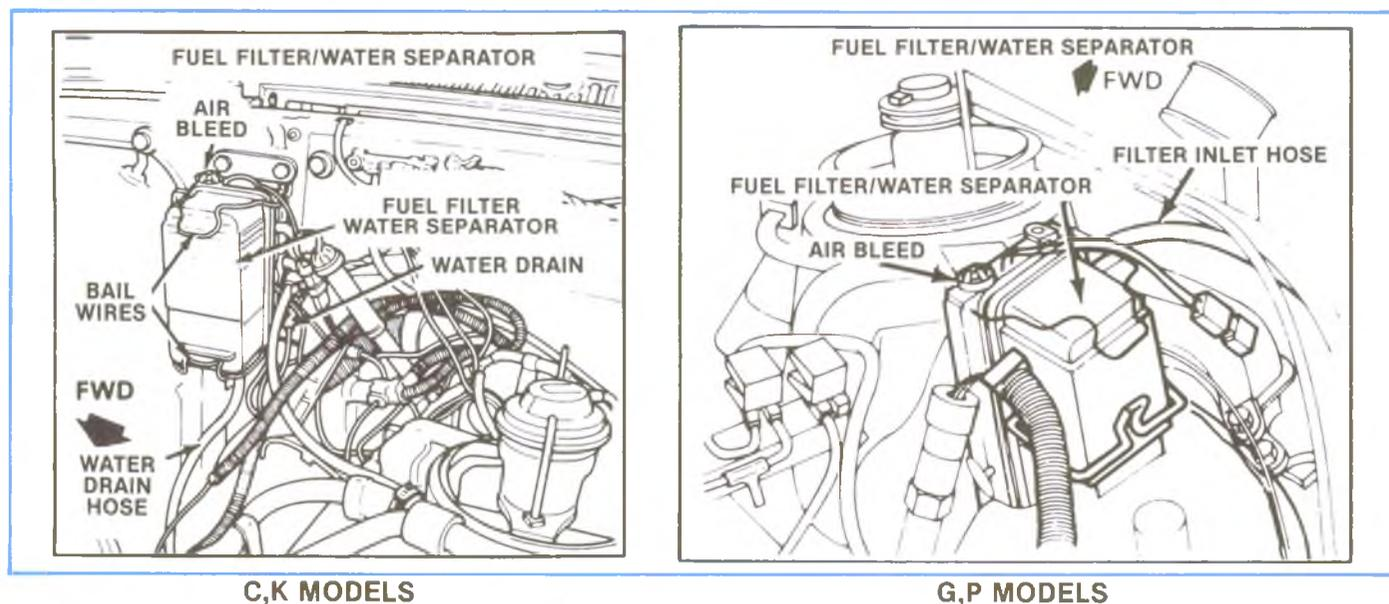
**Figure 4-27, Electrical Connections, Fuel Filter/Water Separator.**
