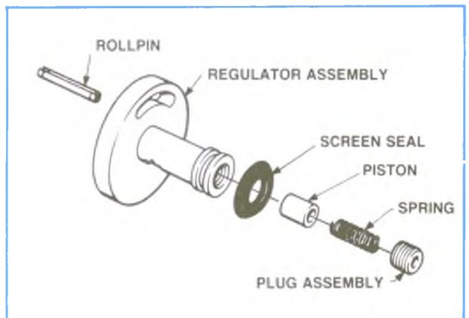
Figure 4-101, Regulator Components.
