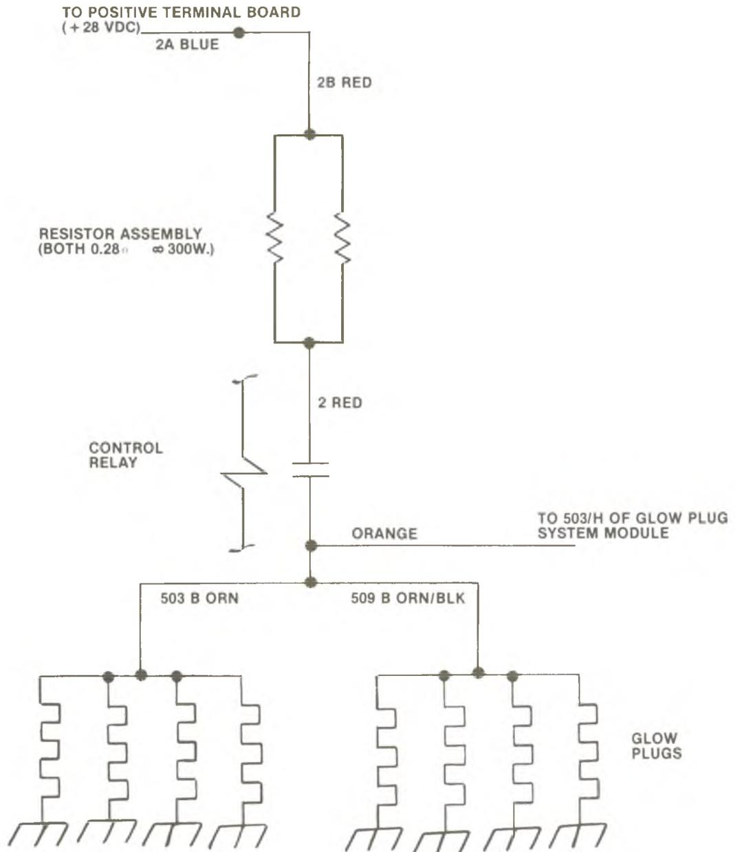
Figure 6-28, Glow Plug Power System, D-Truck.
