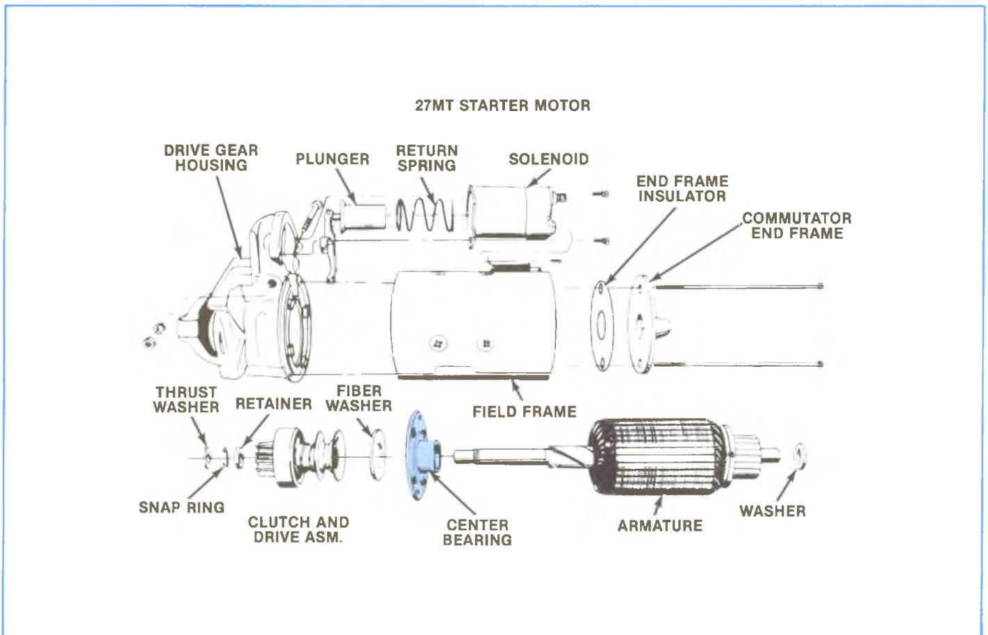
Figure 6-1, 6.2L - 27MT Starting Motor Exploded View.
