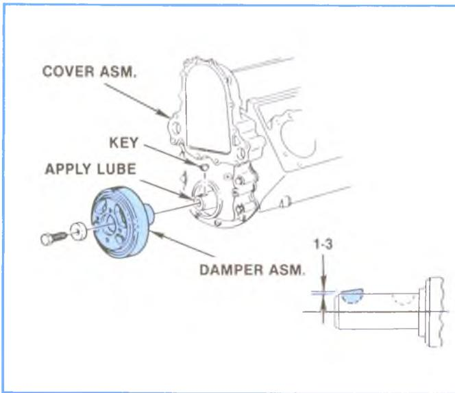
**Figure 2-26, Torsional Damper.**
