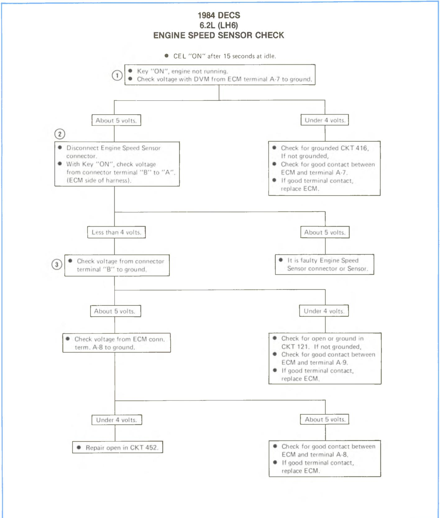
Figure 5-42, 1984 Engine Speed Sensor Chart.
