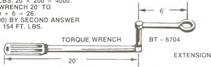
154 FT. LBS. WILL BE THE READING ON THE TORQUE WRENCH WHEN THE DESIRED TORQUE OF 200 FT. LBS. IS ACHIEVED AT THE NUT.
