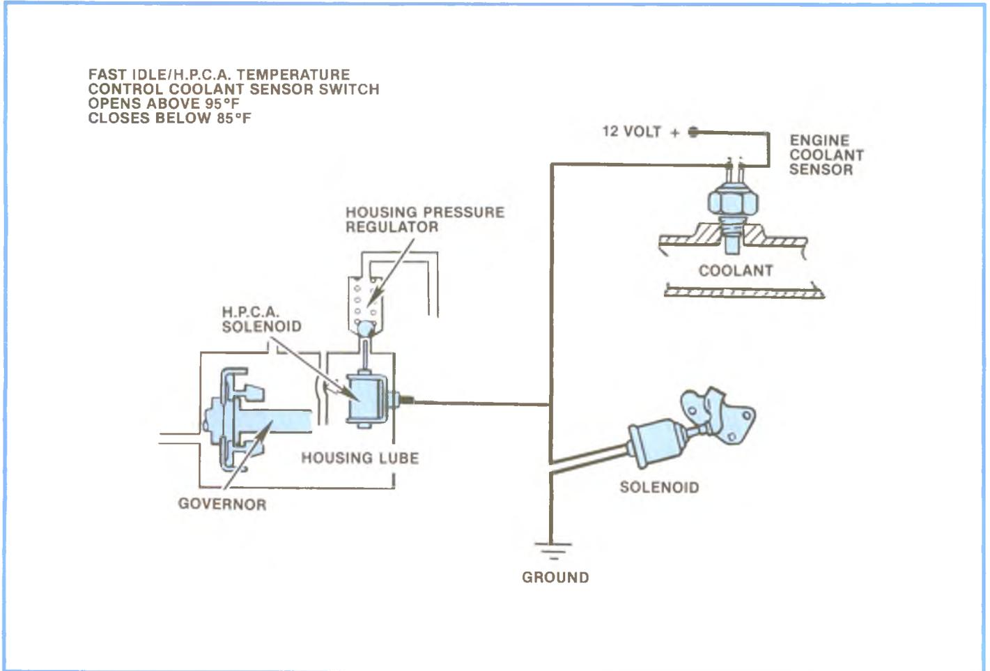
**Figure 4-67, H.P.C.A. Solenoid Installation.**
