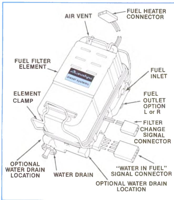
Figure 4-18, Model 80 Fuel Filter and Base Assembly.
