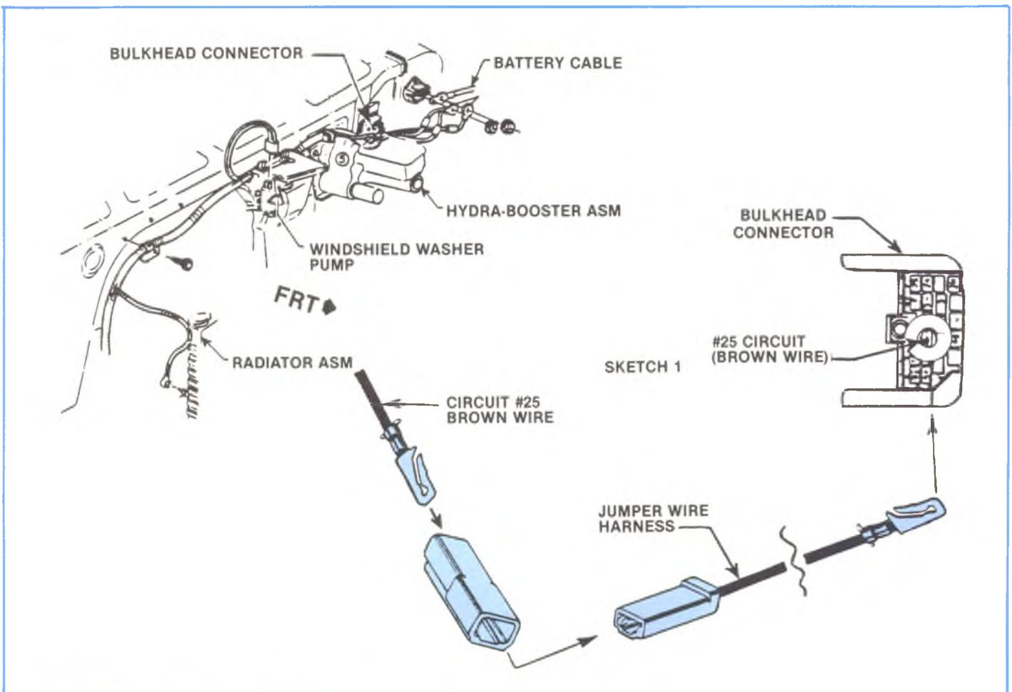
Figure 6-34, Jumper Wire Harness Installation.
