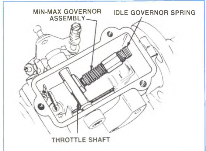
Figure 4-93, Removing Governor Spring.
