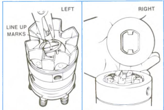
Figure 4-110, Removing Weight Retainer.
