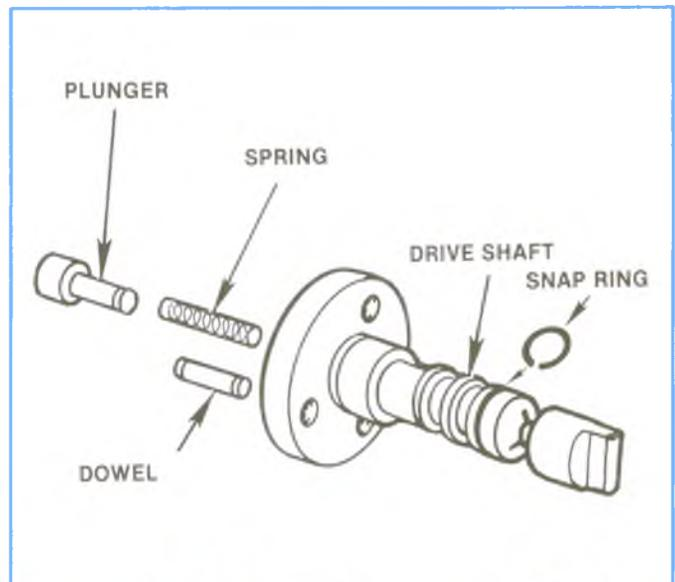
Figure 4-111, Drive Shaft With Retaining Clip.
