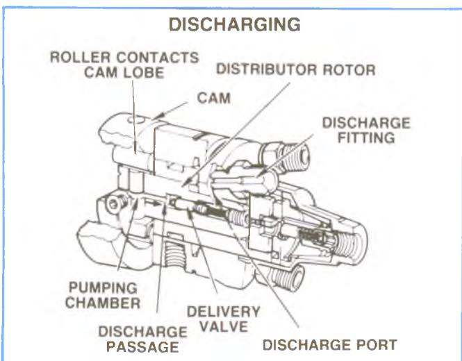
The magnitude of this pressure drop is controlled by the delivery valve which retains a definite residual pressure in the discharge circuit. This pressure is low enough to assure prompt nozzle closing yet high enough to prevent cavitation of the fuel between injections. (Figure 4-45).
