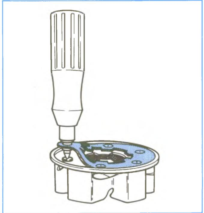
Figure 4-117, Installing Ring With Tool BT 8209-A.
