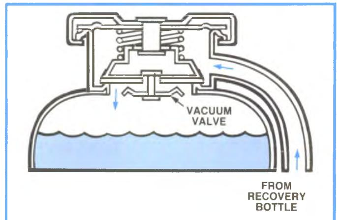
Figure 2-53, Radiator Cap With Vacuum Valve Open.
