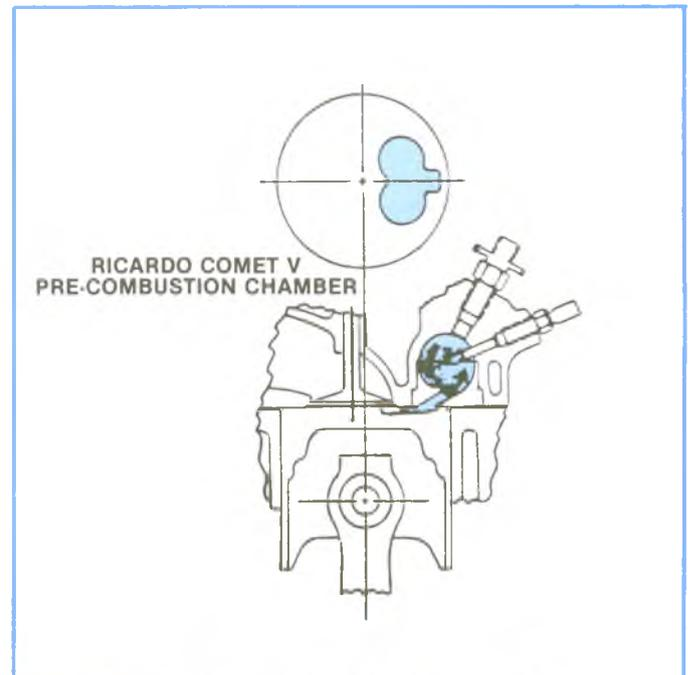
Figure 3-6, Pre-Combustion Chamber.
