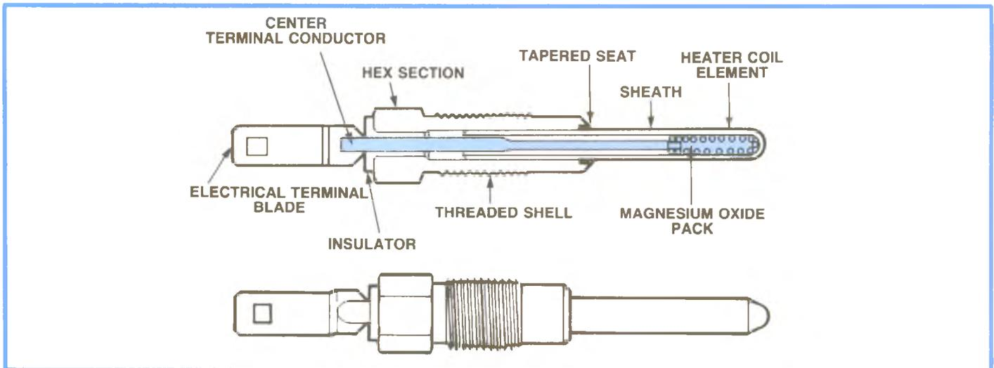
**Figure 6-8, Typical AC Diesel Engine Glow Plug.**
