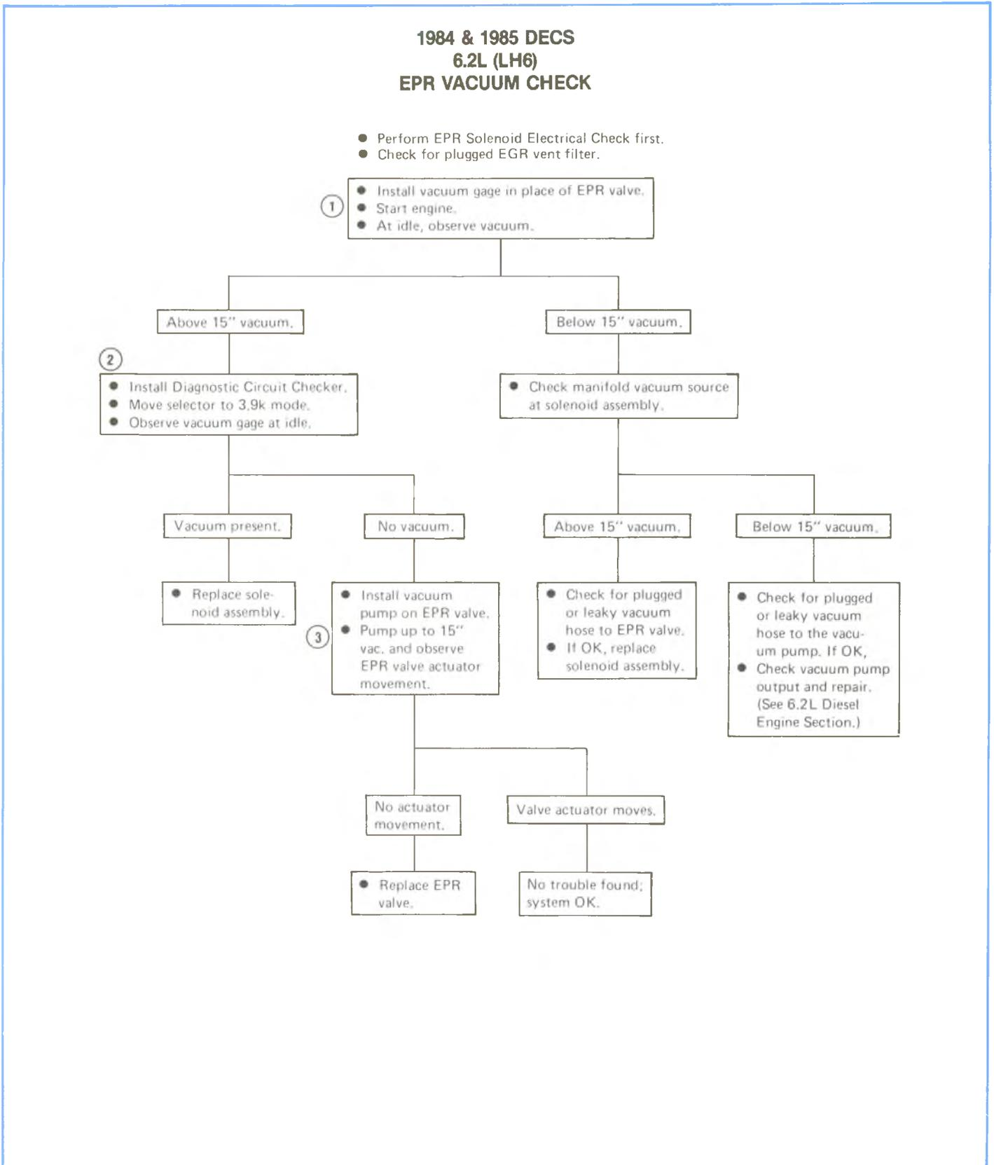
Figure 5-52, EPR Vacuum Check (1984 & 1985).
