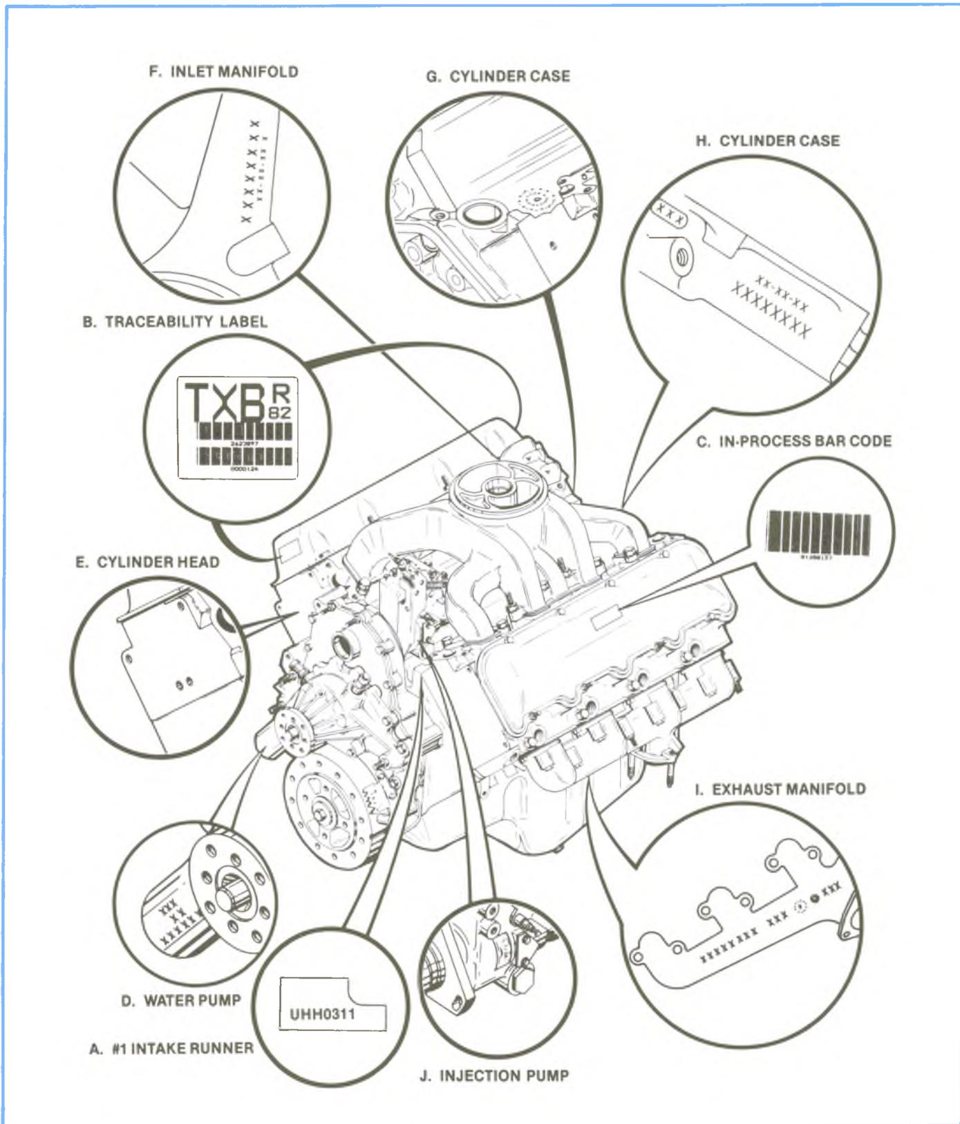
Figure 1-2, Engine Identification.
