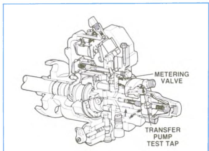
Figure 4-35, Fuel Flow To Transfer Pump and Metering Valve.
