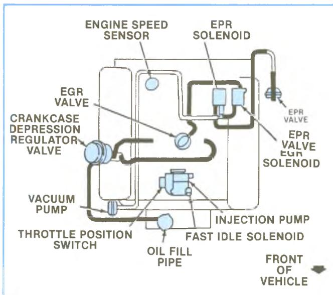
Figure 5-3, Emission Systems — Federal G (LH6 Engine).
