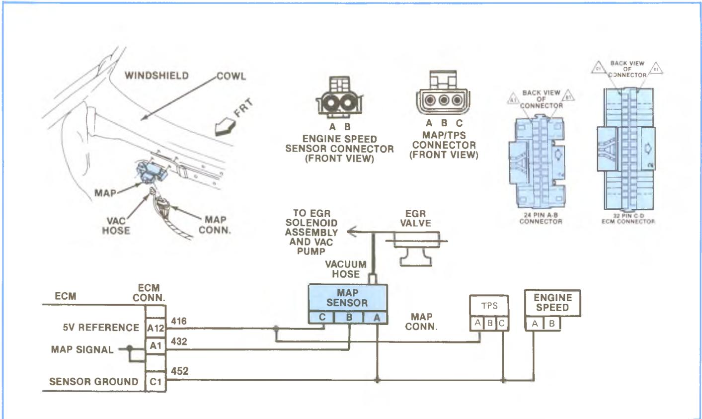
**Figure 5-53, 1985 MAP Sensor Schematic.**
