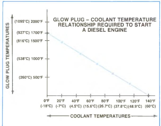
Figure 6-6, Glow Plug Temperature Required for Engine Start.
