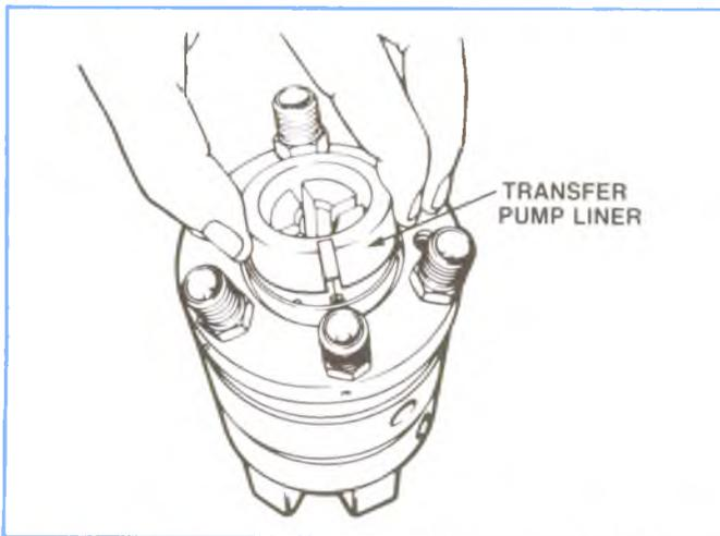
Figure 4-120, Installing Transfer Pump Liner.
