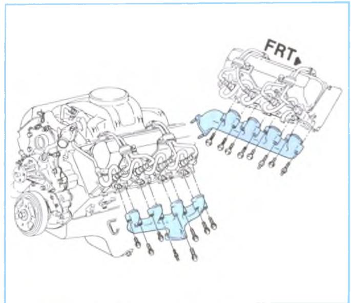
Figure 2-32, Exhaust Manifolds.
