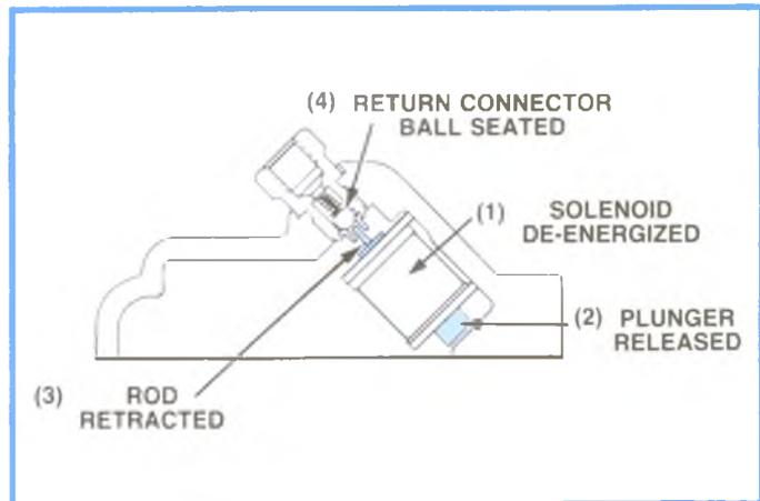
Figure 4-69, Solenoid De-Energized.
