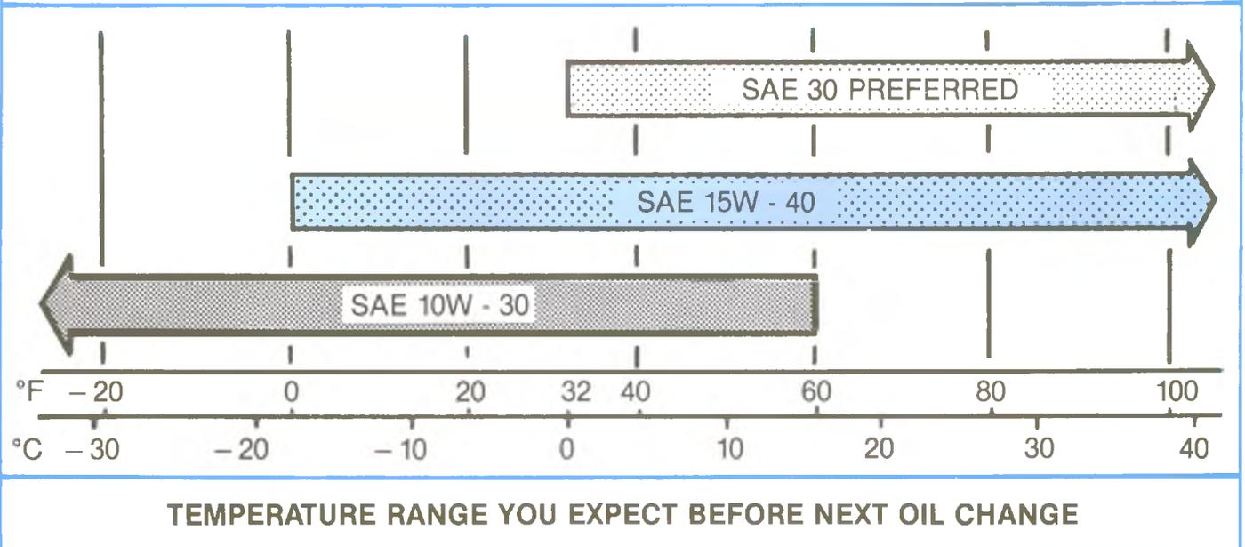
Figure 1-7, Ambient Temperature Range For Engine Oil.
