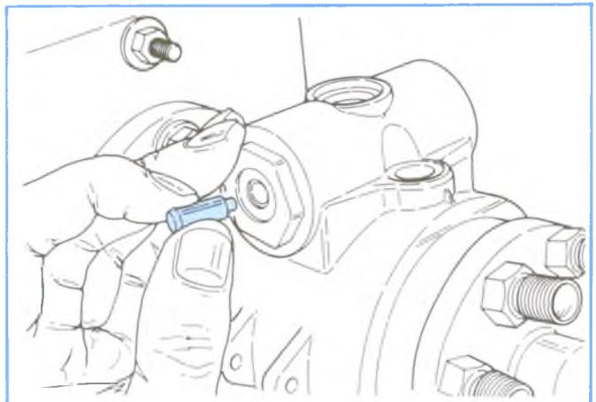
**Figure 4-150, Installing Servo Advance Plunger.**
