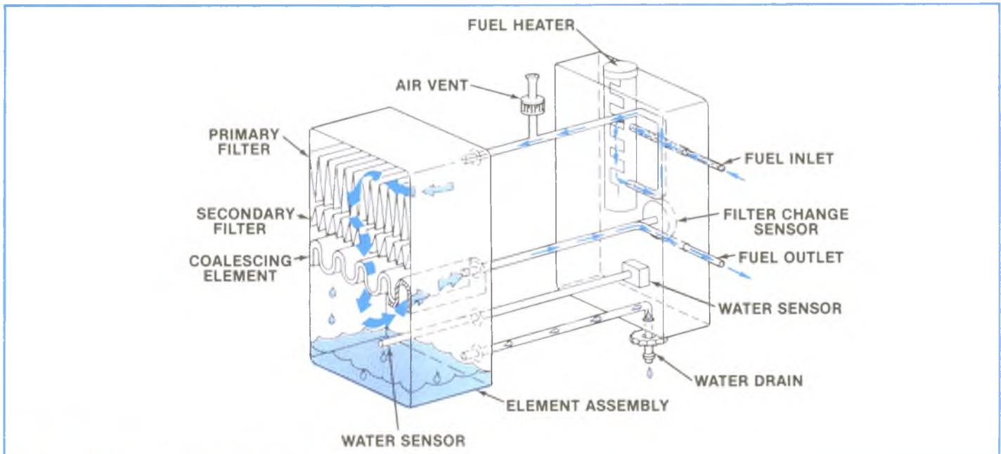
Figure 4-22, Filter and Base Flow Schematic.
