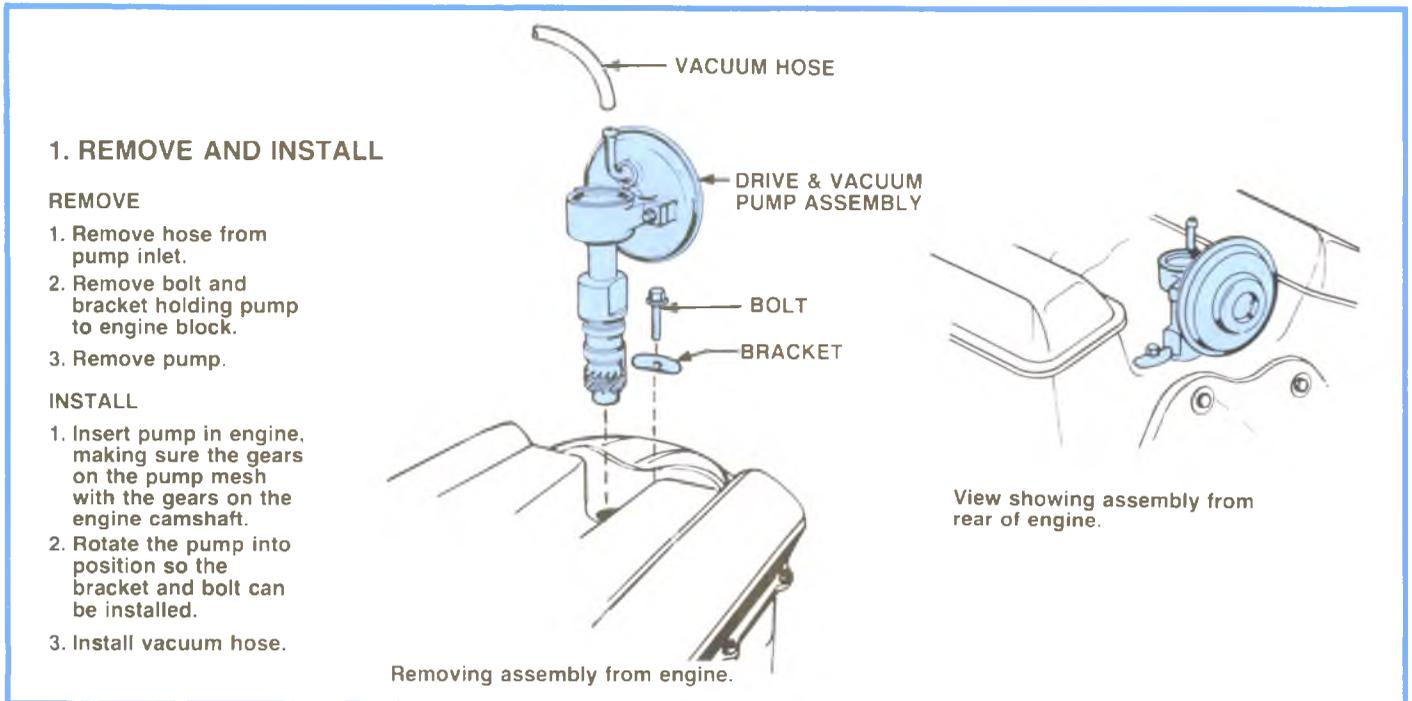
**Figure 2-39, Repair Procedures.**
