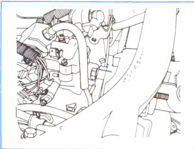
Figure 4-164, Aligned Timing Marks.
