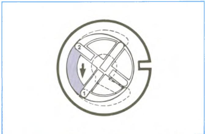
Figure 4-47, Transfer Pump In Mid Position.
