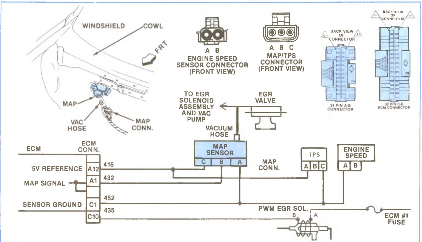
Figure 5-56, 1985 MAP Sensor Schematic (Code 31).
