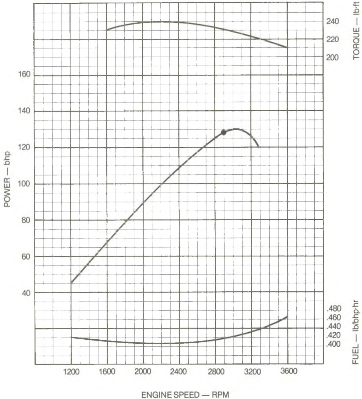
Figure 1-3, Engine Performance Curve, 6.2L — Light Duty (LH6).
