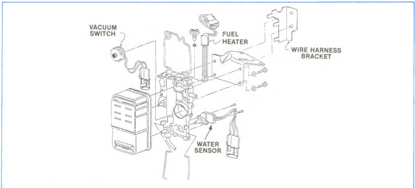
**Figure 4-28, 1985 Model 80 Filter, Exploded View.**
