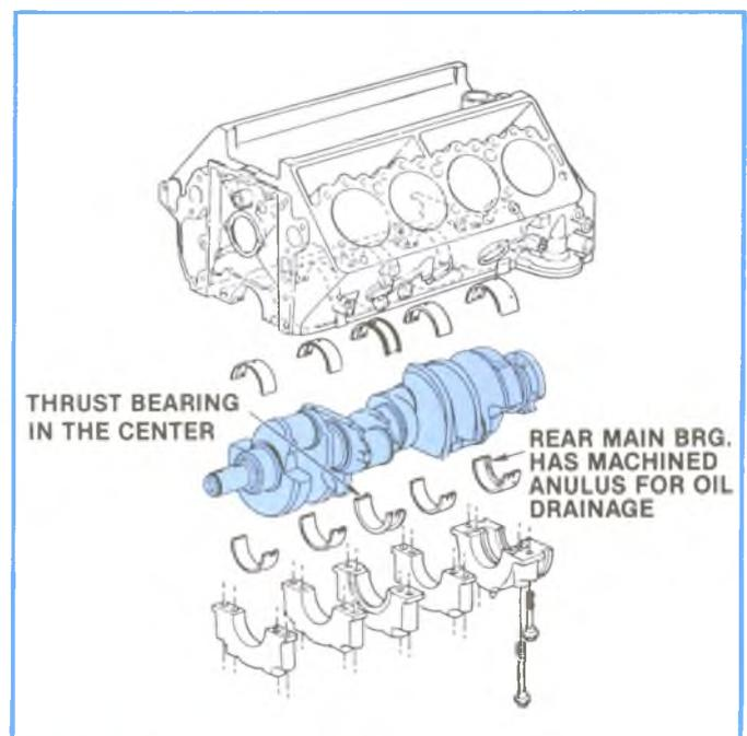
Figure 2-20, Crankshaft.
