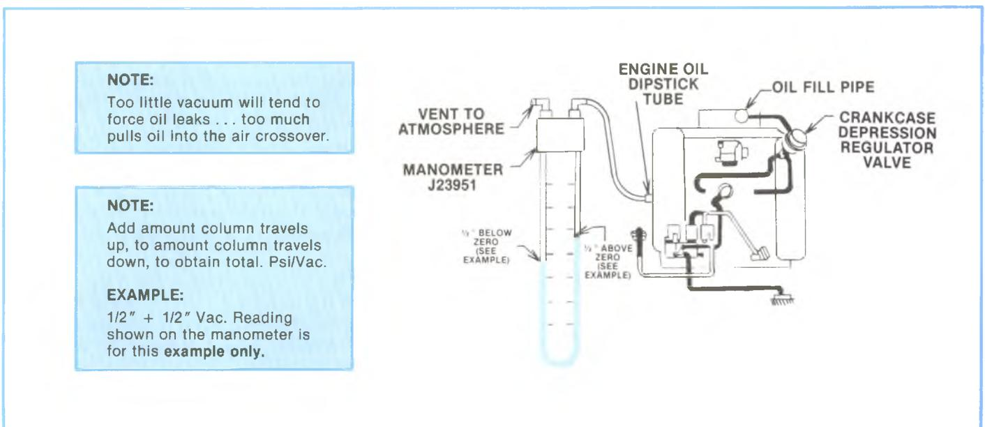
Figure 5-8, CDR Valve Test with Manometer.
