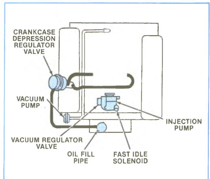
Figure 5-4, Emission System — LL4 Engine.
