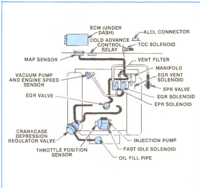
**Figure 5-44, Emission Systems — California CK (LH6 Engine).**
