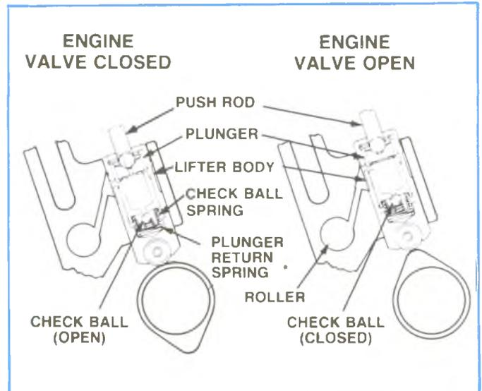
Figure 2-7, Roller Valve Lifter Operation.
