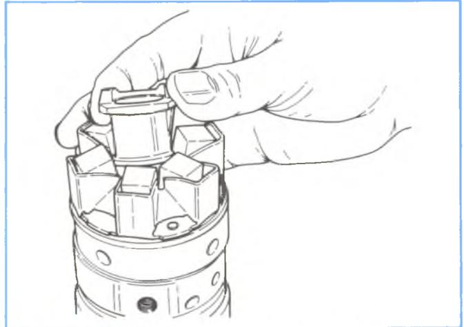
**Figure 4-128, Installing Thrust Sleeve and Checking Weights.**
