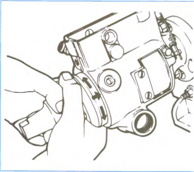
Figure 4-131, Installing Head.
