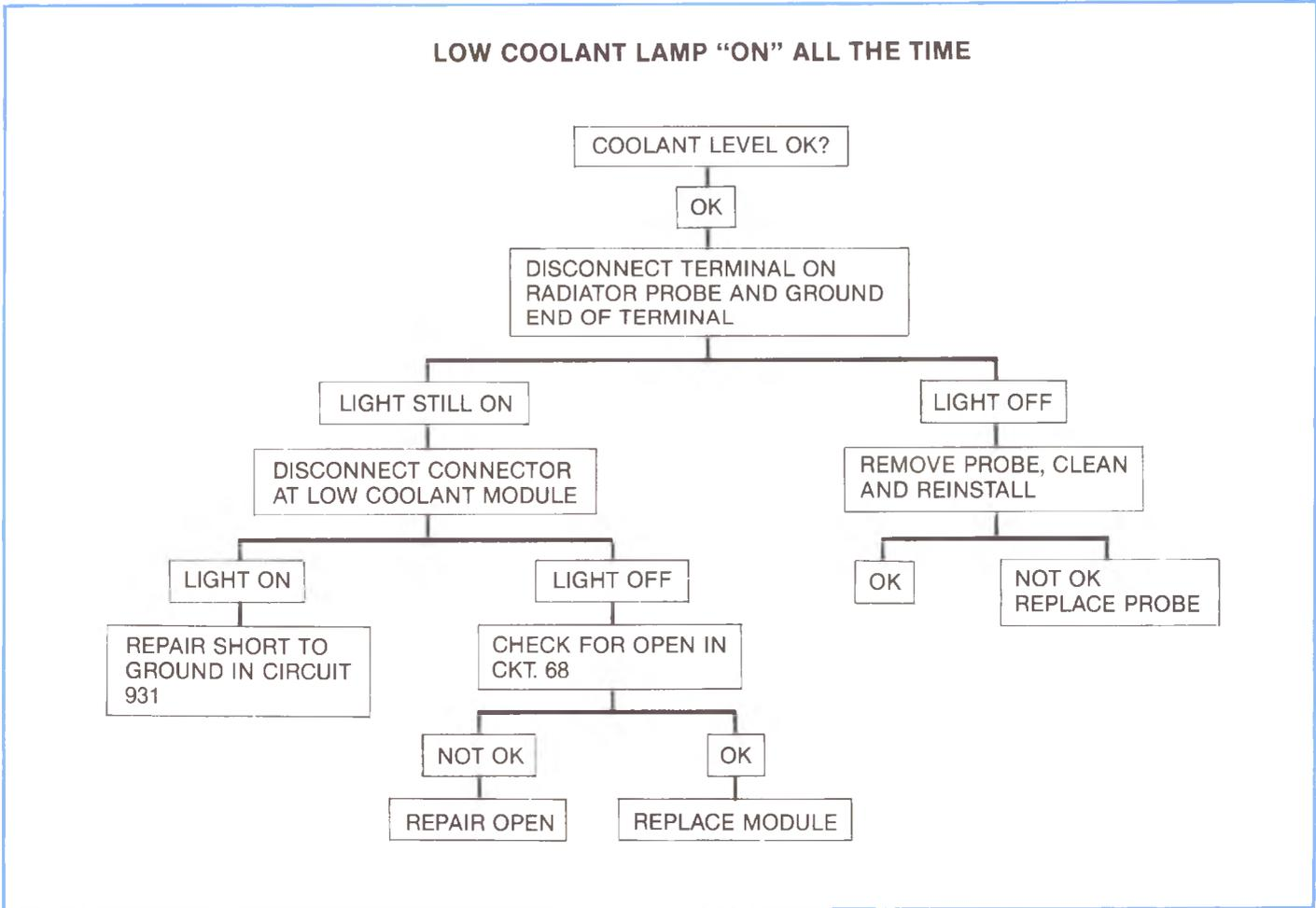
Figure 2-62, Low Coolant Lamp Remains "On".
