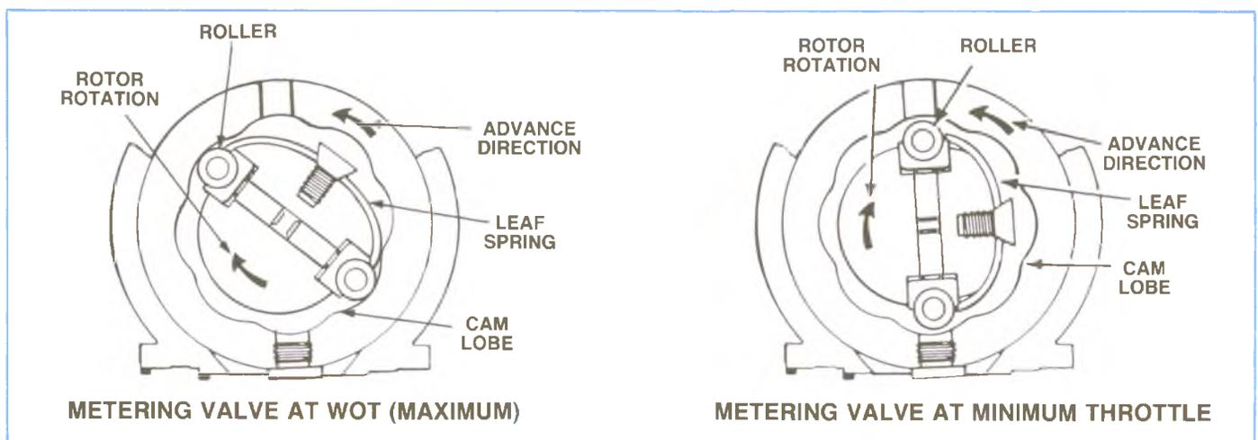
Figure 4-60, Cam Positioning.
