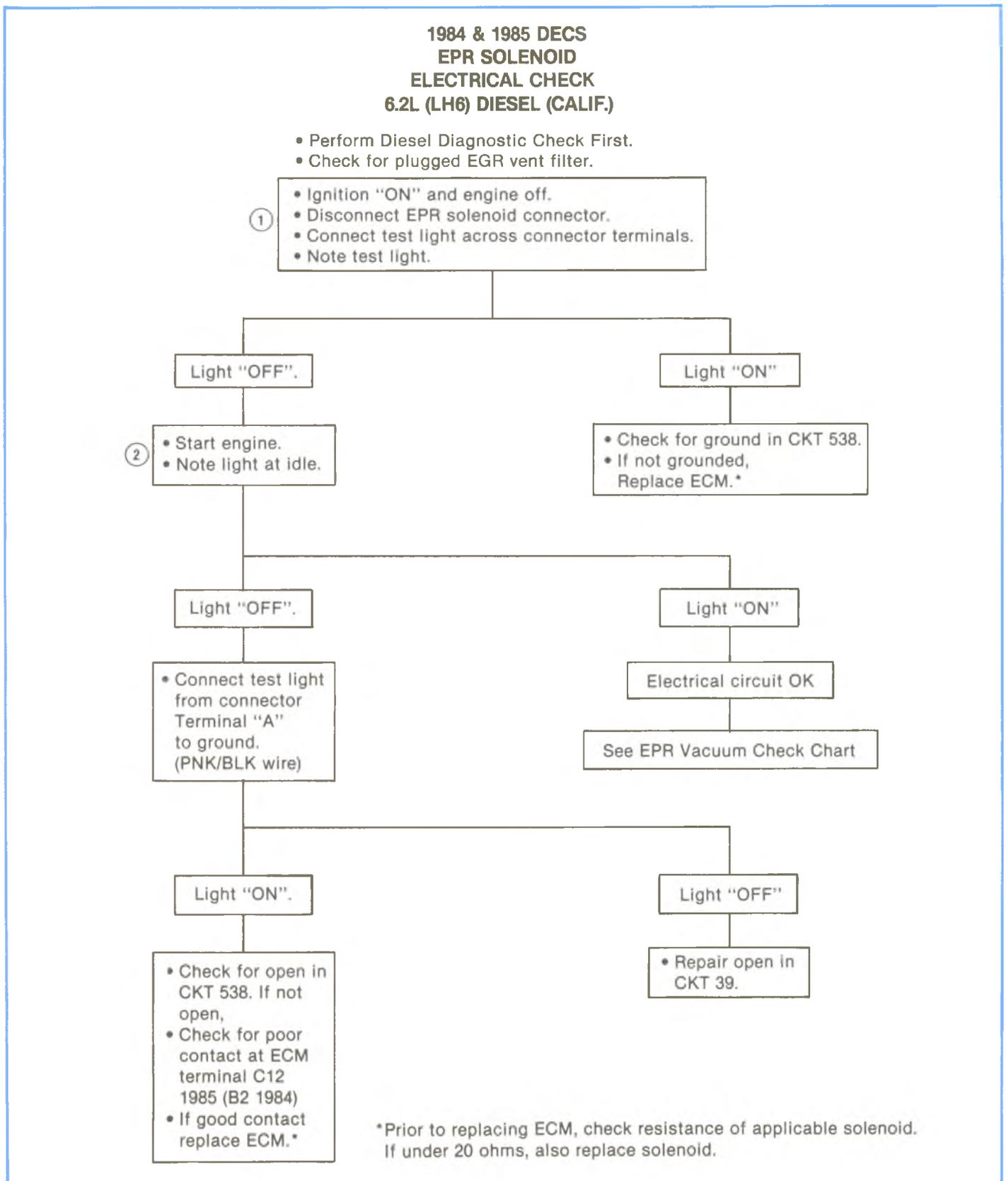
Figure 5-50, EPR Solenoid Electrical Check (1984 & 1985).
