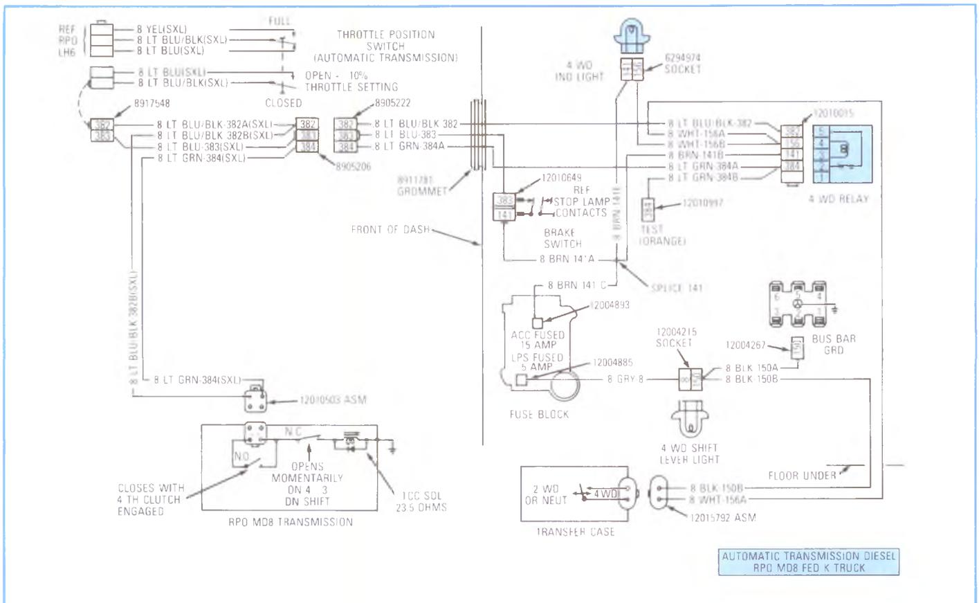
**Figure 5-14, Wiring Diagram T.C.C. MD-8 K Truck.**
