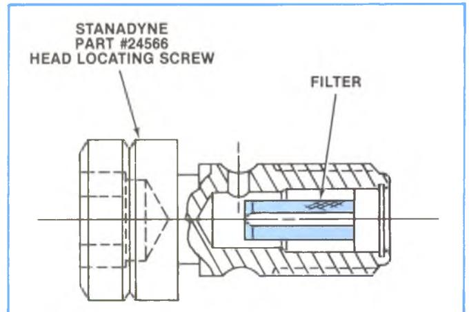
Figure 4-66, Head Locating Screw With Filter.
