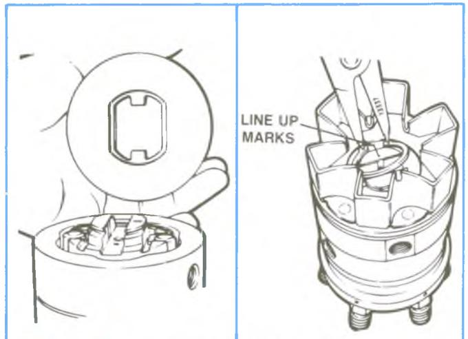
Figure 4-118, Installing Weight Retainer.
