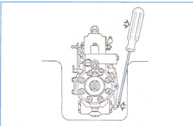
Figure 4-167, Depressing Rocker Lever.
