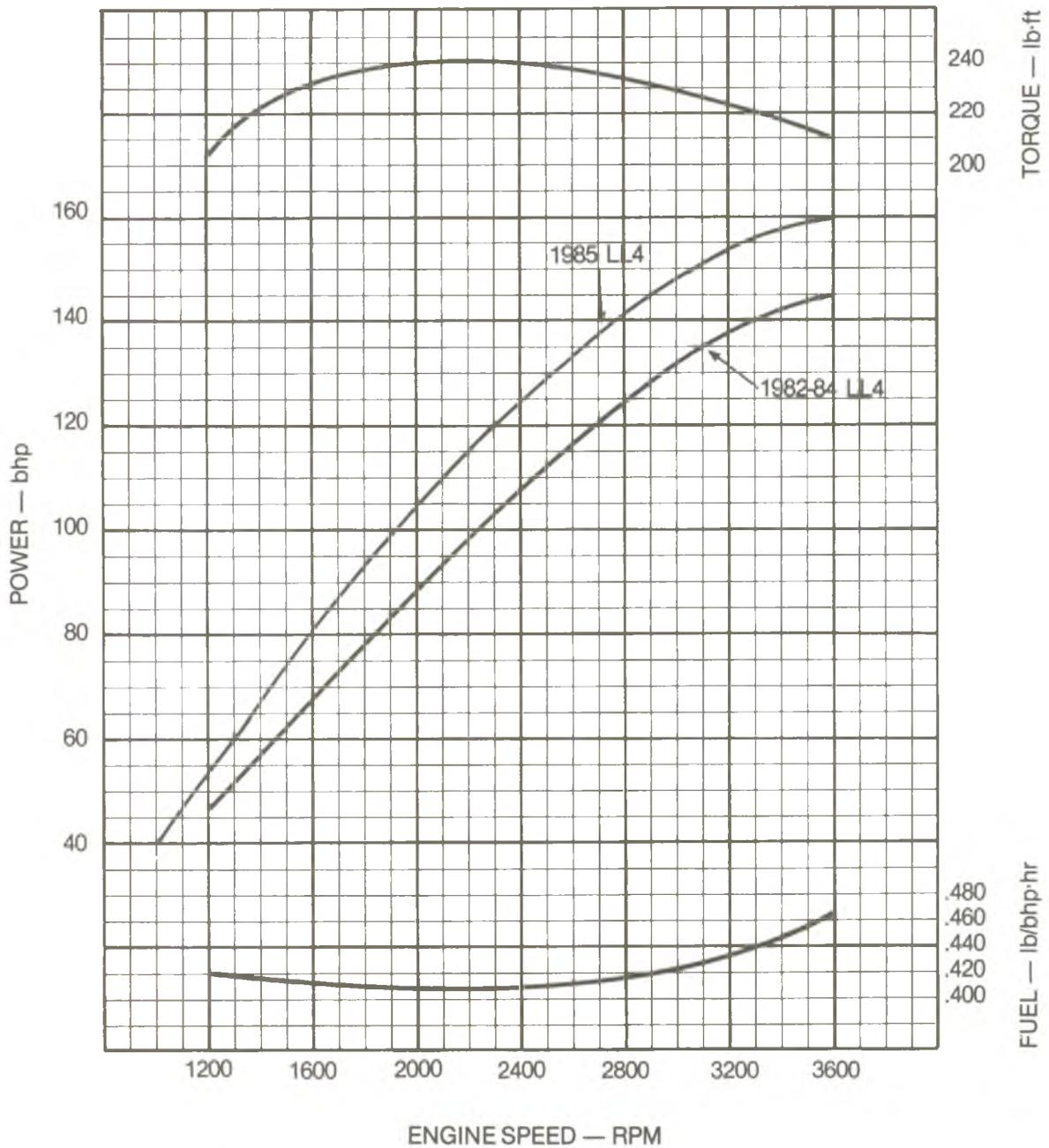
Figure 1-4, Engine Performance Curve, 6.2L — Heavy Duty (LL4)
