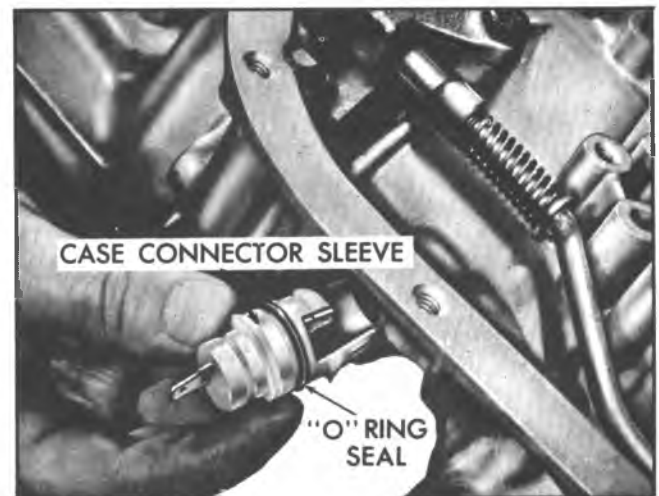
Fig. 15T--Removing Electrical Connector and "O" Ring Seal
