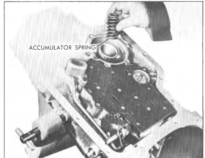
Fig. 147T-Installing Rear Accumulator Spring
