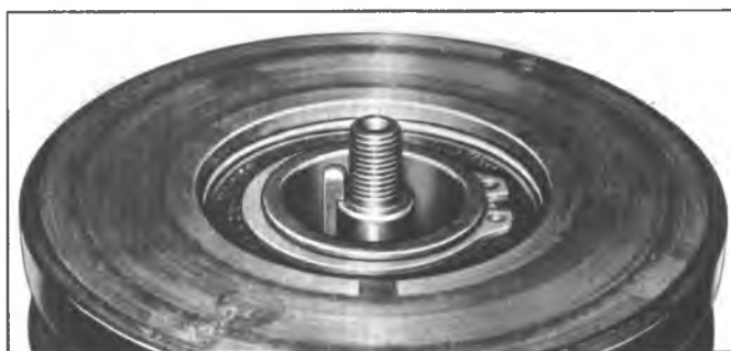
Fig. 4--Drive Plate Key Installed in Keyway
