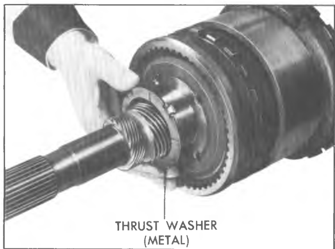
Fig. 126T--Installing Case to Output Shaft Thrust Washer
