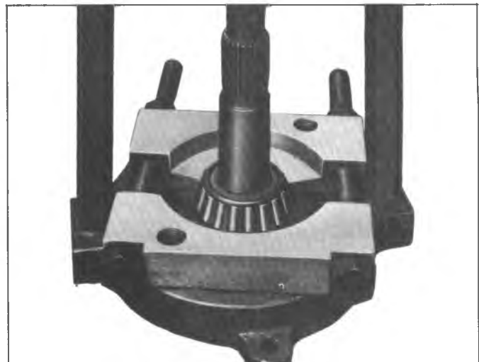
Fig. 18F—Removing Inner Pinion Bearing Cone and Roller
