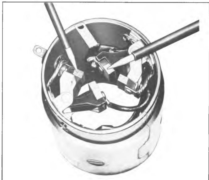
Fig. 7S--Field Coil Ground Test
