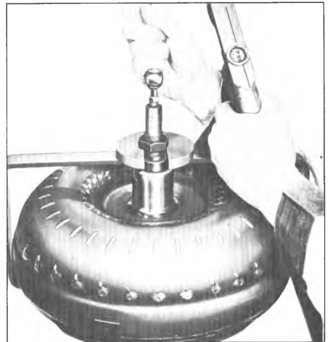
Fig. 114T--Air Checking Converter
