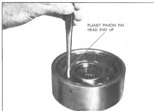
Fig. 109T-Installing Planet Pinion Pin
