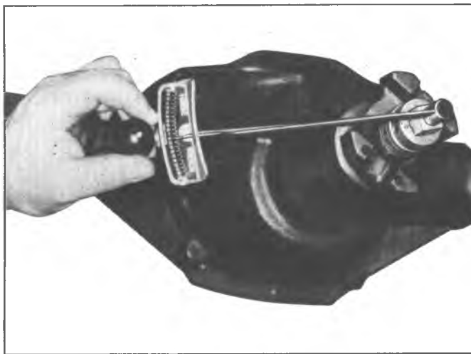
Fig. 24A—Measuring Rotating Torque
