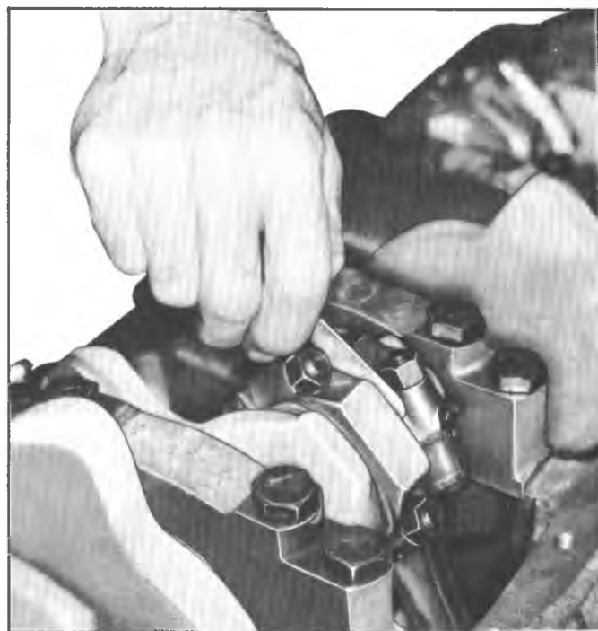
Fig. 46—Measuring Connecting Rod Side Clearance (V8)
