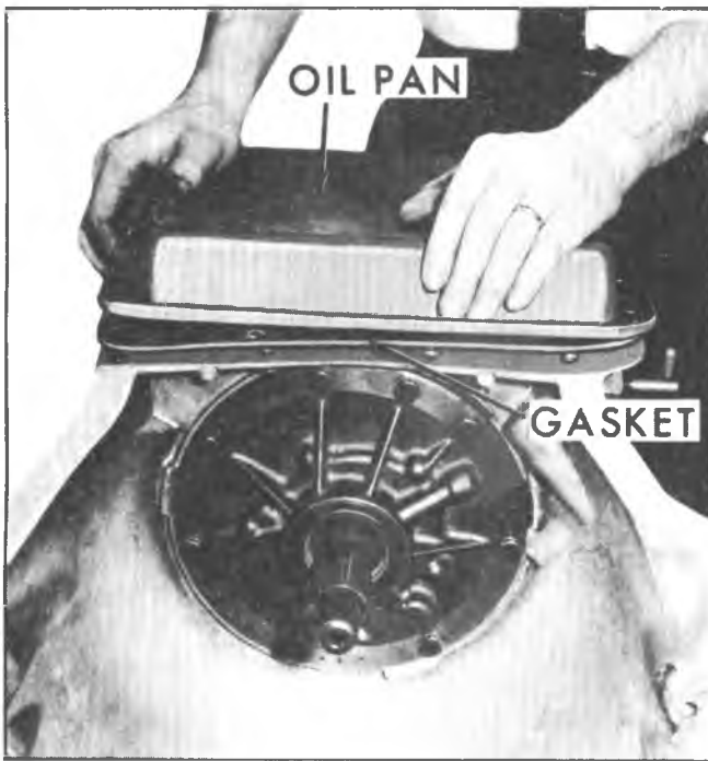
Fig. 9M--Removing Transmission Oil Pan
