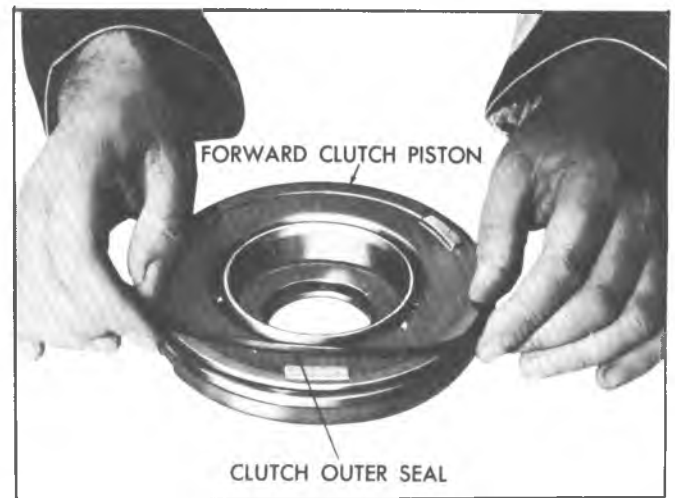
Fig. 71T--Removing Forward Clutch Piston Outer Seal
