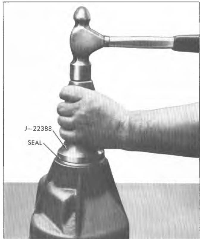
Fig. 18F—Installing Rear Output Housing Seal
