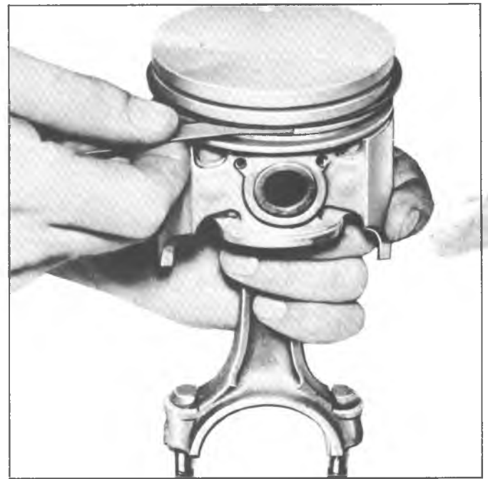
Fig. 58—Measuring Ring Groove Clearance
