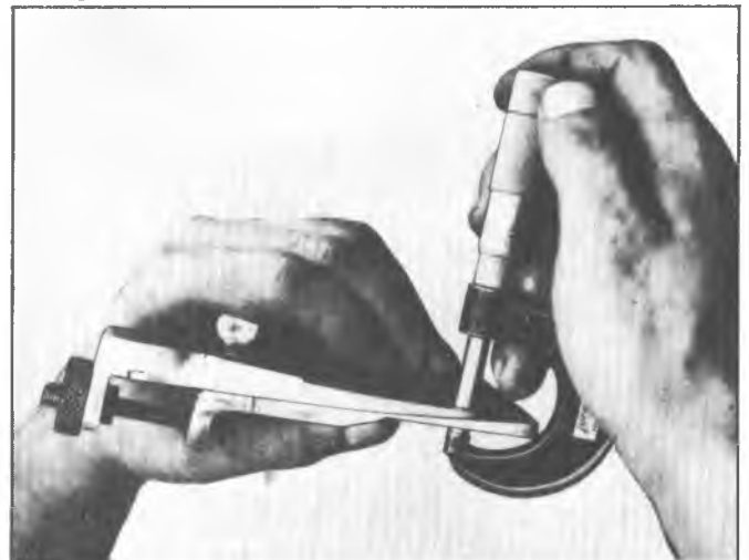
Fig. 10C—Measuring Gauge Plate Thickness
