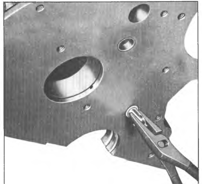
Fig. 64—Measuring Camshaft End Play
