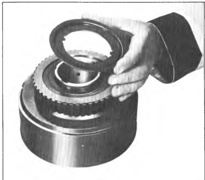
Fig. 94T--Installing Intermediate Clutch Retainer
