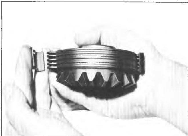
Fig. 10D—Assembling Clutch Pack
