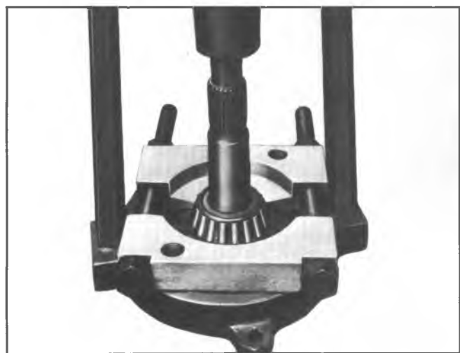
Fig. 15A—Removing Drive Pinion Rear Bearing.
