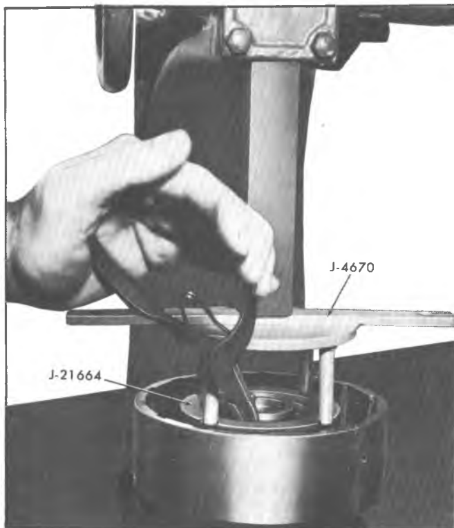
Fig. 70T--Removing Forward Clutch Spring Retaining Snap Ring
