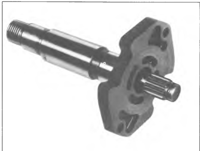
Fig. 22--Installing Thrust Plate
