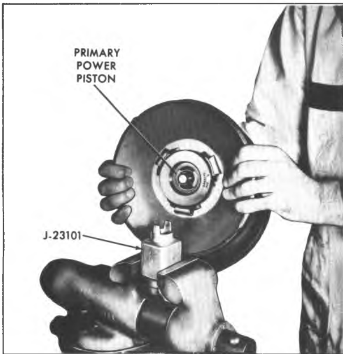
Fig. 8B--Positioning Primary Power Piston in Tool J-23101 (Small Dia. End Up)
