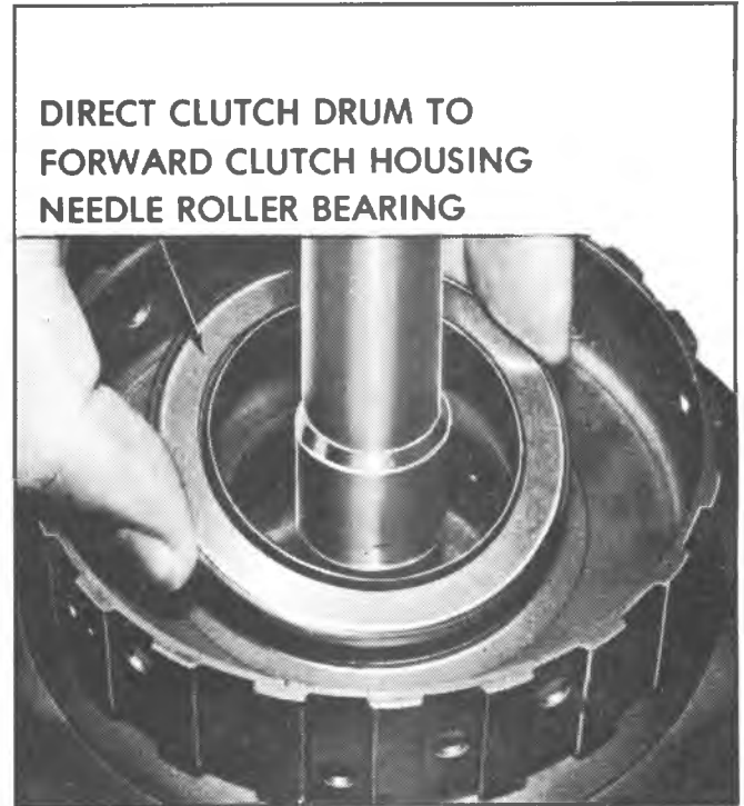
Fig. 69M--Direct Clutch Drum to Forward Clutch Housing Needle Roller Bearing
