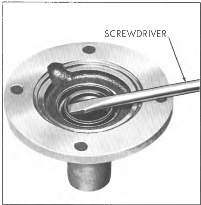
Fig. 14X-Removing Bearing Retainer Oil Seal
