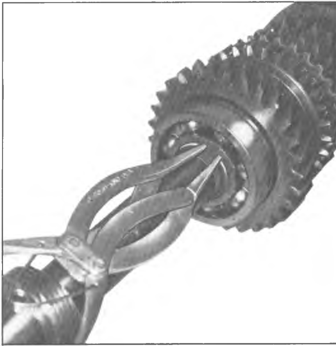
Fig. 8X--Rear Bearing to Mainshaft Snap Ring
