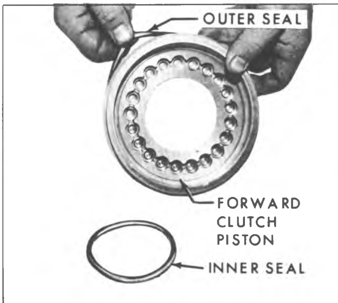
Fig. 81M--Removing Forward Clutch Piston Inner and Outer Seals
