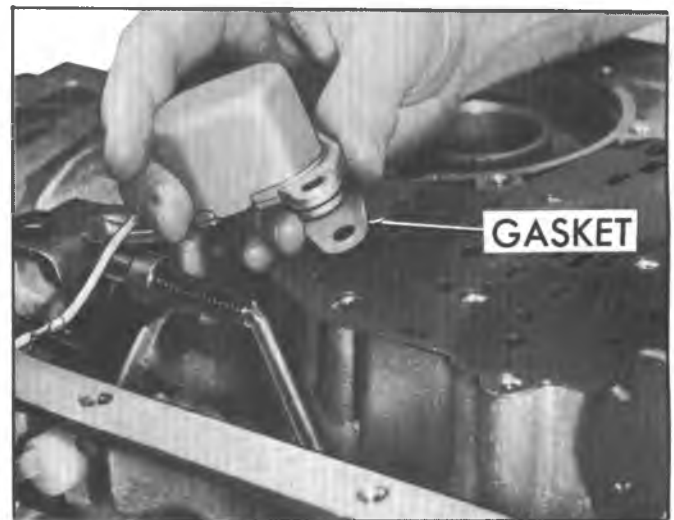
Fig. 14T--Removing Detent Solenoid and Gasket
