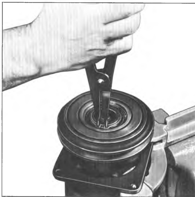
Fig. 6--Removing Pulley and Bearing Assembly Retainer Ring
