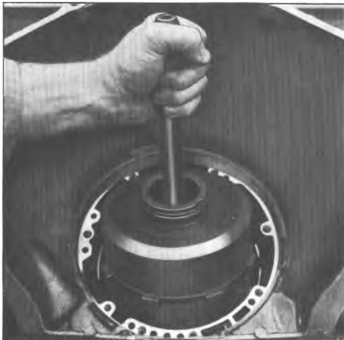
Fig. 31N--Removing Direct and Forward Clutch Assemblies
