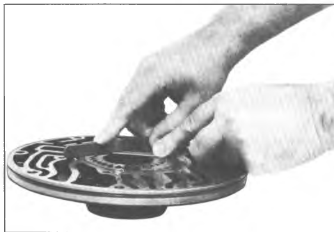
Fig. 60M--Checking Pump Body to Gear Face Clearance
