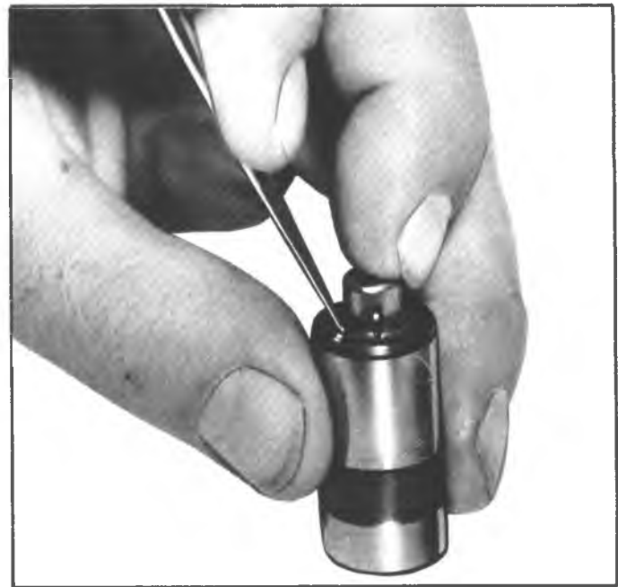
Fig. 32—Installing Ball Check Valve
