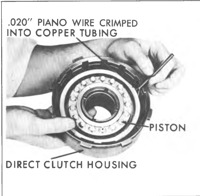
Fig. 68N--Installing Direct Clutch Piston
