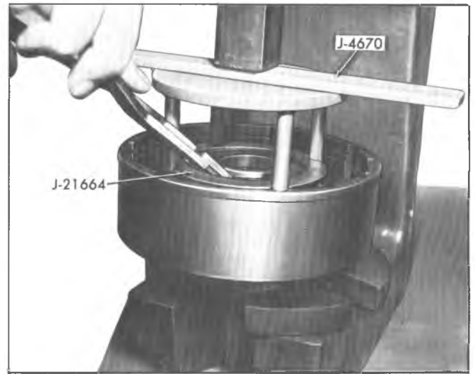
Fig. 81T--Removing or Installing Direct Clutch Snap Ring
