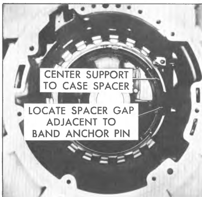
Fig. 37T-A-Removing Center Support to Case Spacer
