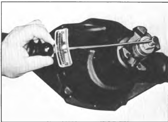
Fig. 28B—Measuring Rotating Torque
