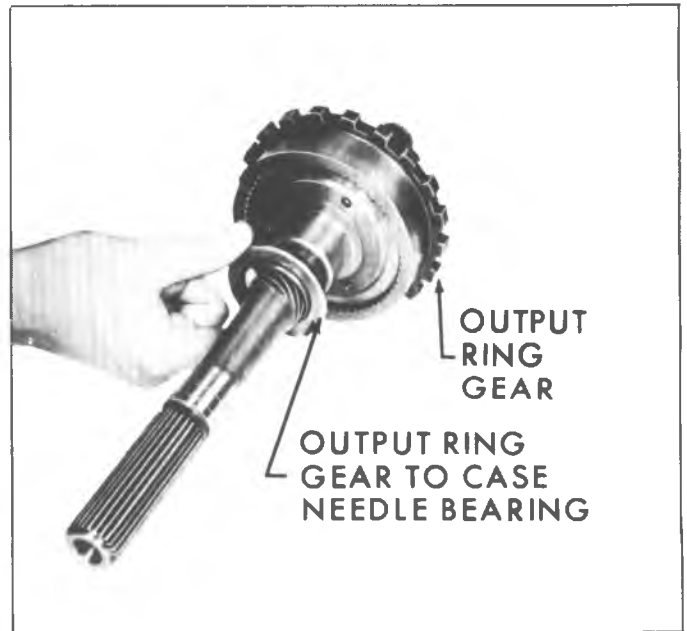
Fig. 44M--Removing Output Ring Gear to Case Needle Bearing Assembly
