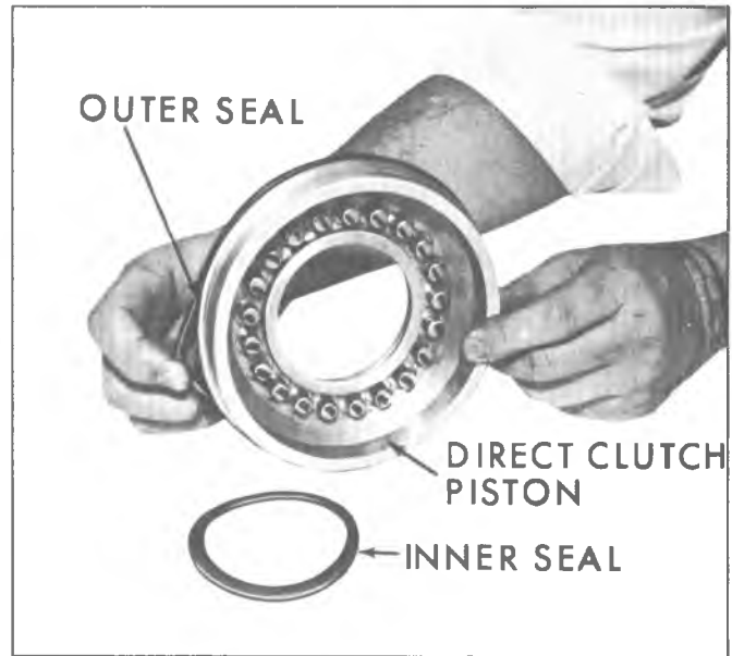
Fig. 66N--Removing Direct Clutch Outer and Inner Seals
