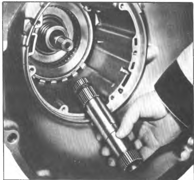
Fig. 31T--Removing Sun Gear Shaft
