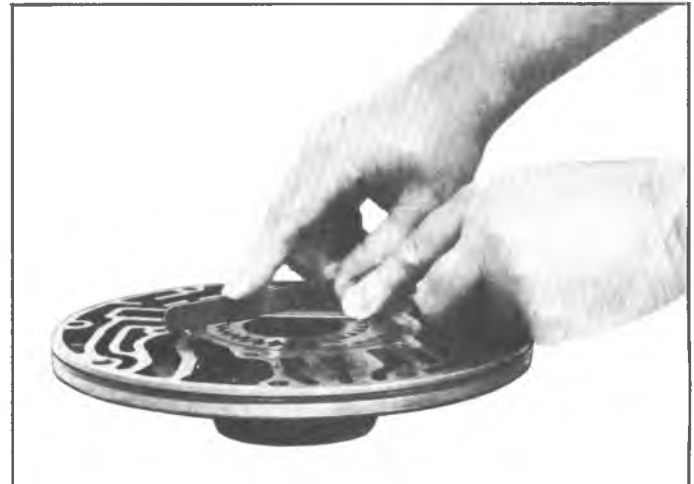
Fig. 56N--Checking Pump Body to Gear Face Clearance
