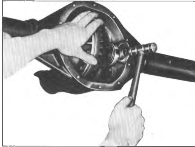
Fig. 9B—Installing Differential Shim
