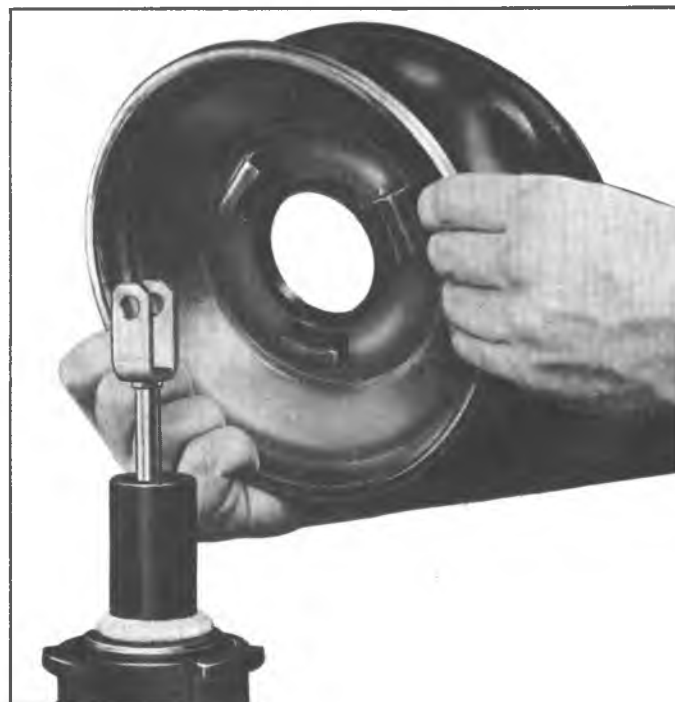
Fig. 11A--Installing Power Piston to Support Plate
