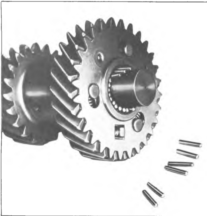
Fig. 19X--Loading Countergear Bearings
