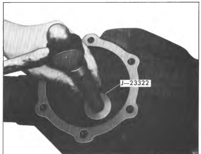
Fig. 14E—Installing Straddle Bearing
