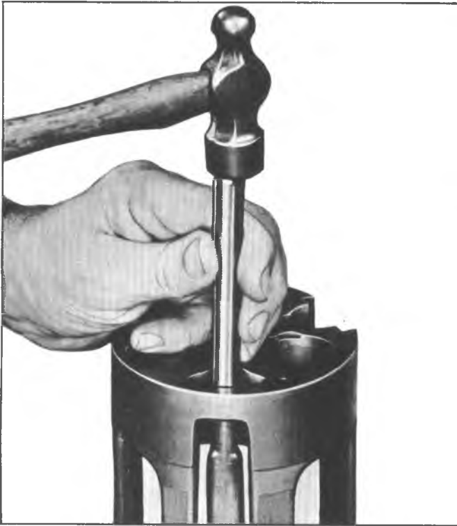
Fig. 18--Unseating Discharge Crossover Tube
