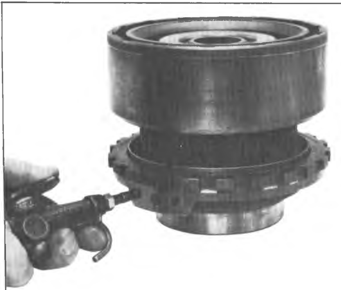
Fig. 96T--Air Checking Direct Clutch Assembly
