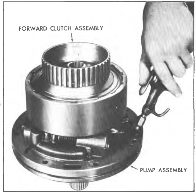
Fig. 77T--Air Checking Forward Clutch Assembly
