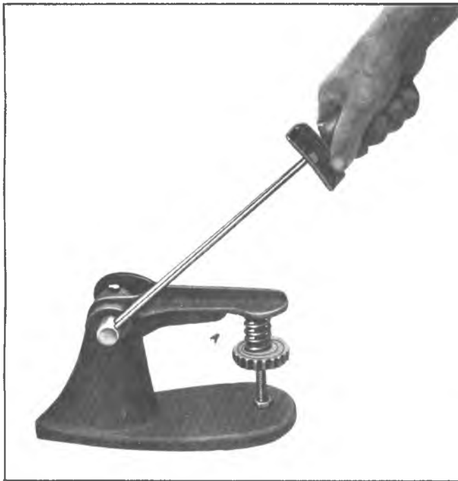
Fig. 17—Checking Valve Spring Tension
