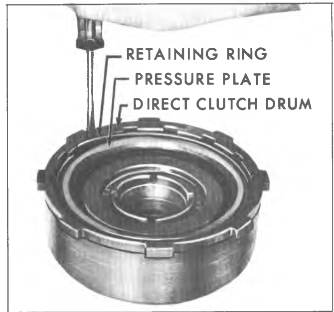
Fig. 70M--Removing Direct Clutch Pressure Plate
