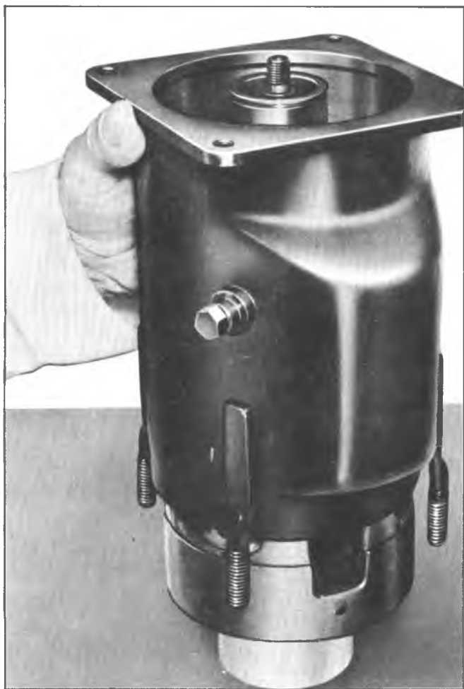
Fig. 27--Installing Shell Over Internal Mechanism
