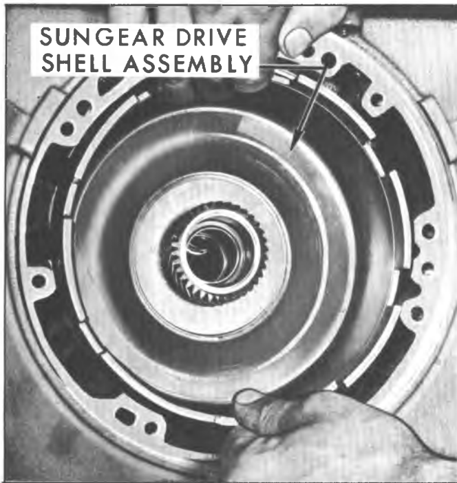
Fig. 38M--Removing Sun Gear Drive Shell
