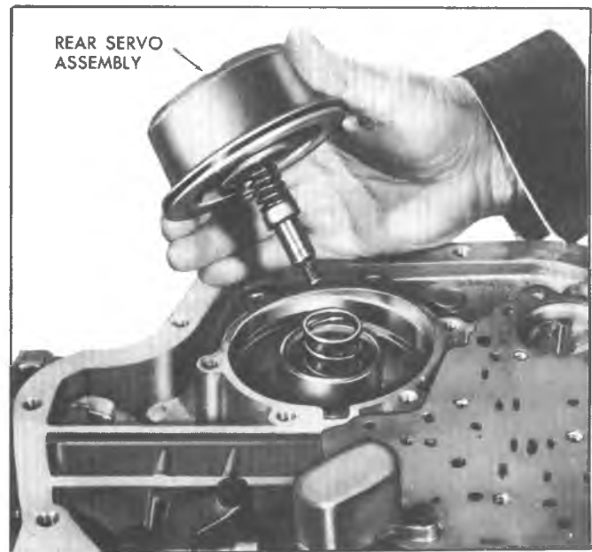
Fig. 12T--Removing Rear Servo Assembly
