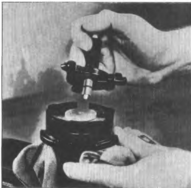
Fig. 12A-Installing Reaction Retainer on Power Piston
