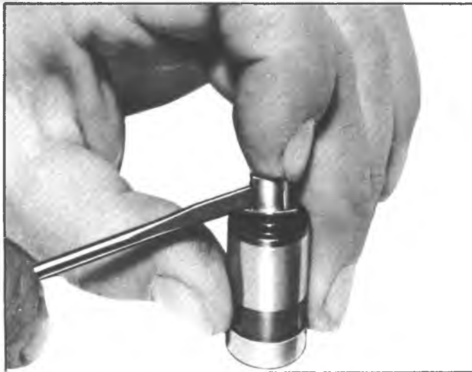
Fig. 31—Removing Ball Check Valve
