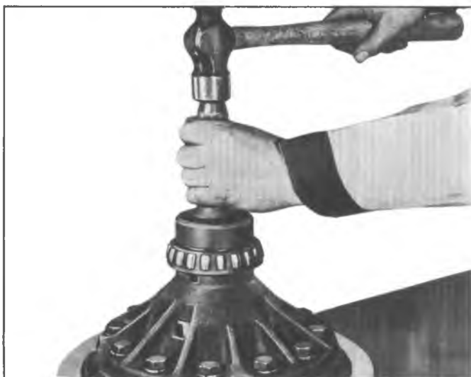
Fig. 8G—Differential Bearing Installation
