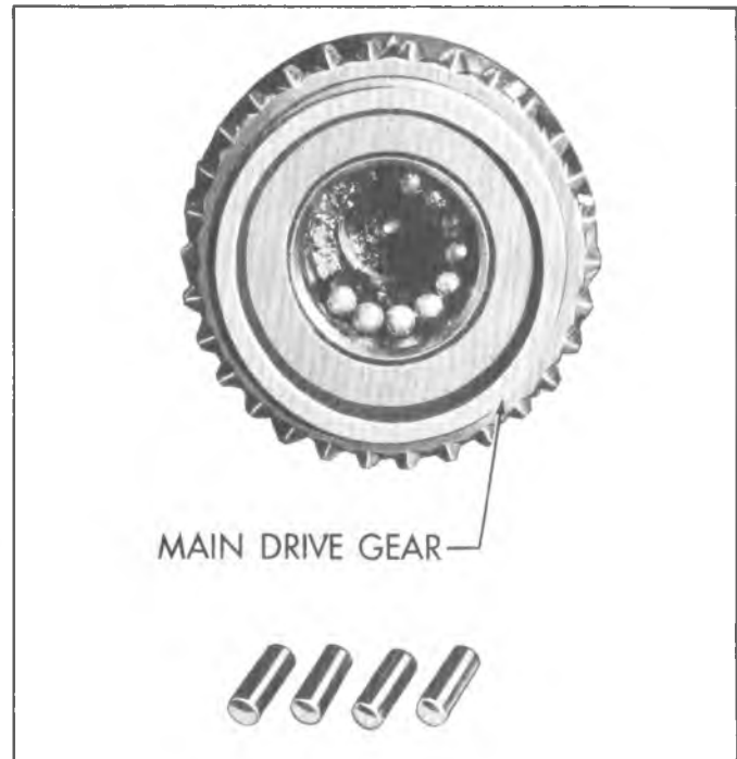
Fig. 20X--Loading Mainshaft Pilot Bearings
