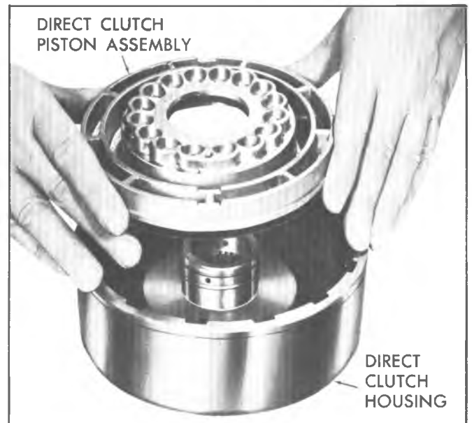
Fig. 82T--Removing Direct Clutch Piston Assembly
