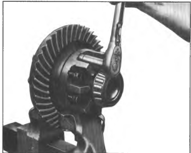
Fig. 3F—Separating Case Halves
