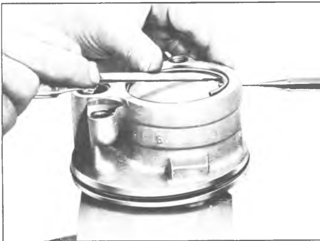
Fig. 18--Removing End Plate Ring
