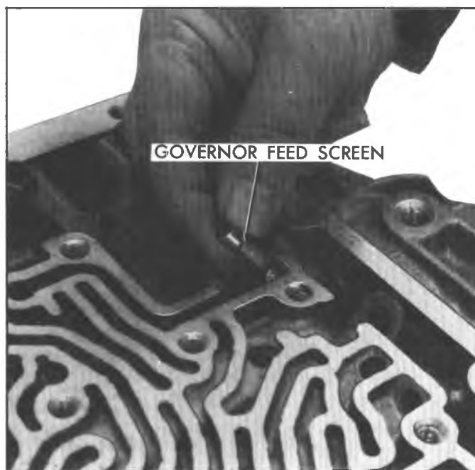
Fig. 17N--Removing Governor Feed Screen
