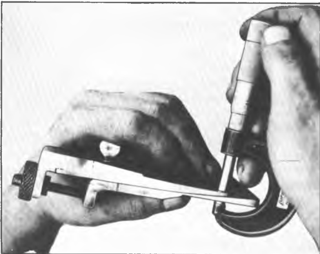
Fig. 8A—Measuring Gauge Thickness
