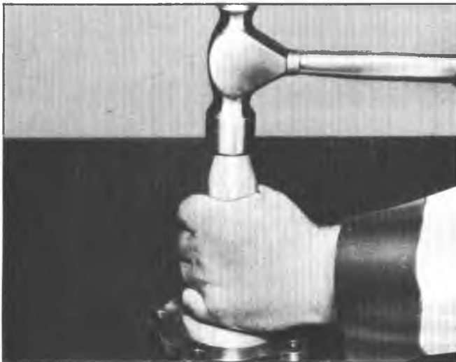
Fig. 4G—Pinion Oil Seal Installation
