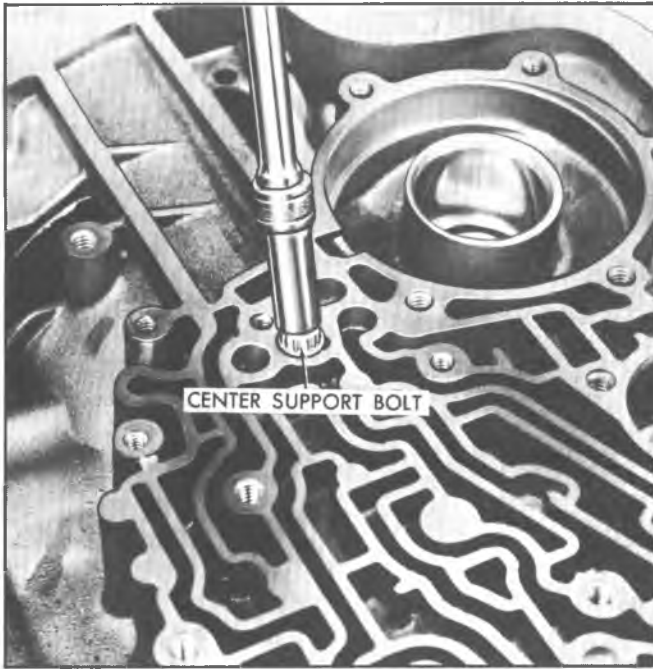
Fig. 33T--Removing Center Support Bolt
