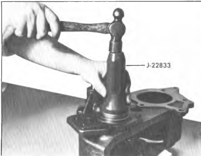
Fig. 15D--Installing Front Output Shaft Seal
