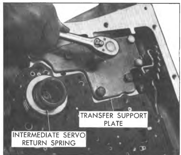
Fig. 13N--Removing Transfer Support Plate and Intermediate Servo Return Spring
