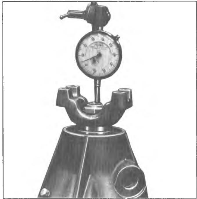
Fig. 23F—Checking Rear Output Shaft End Play
