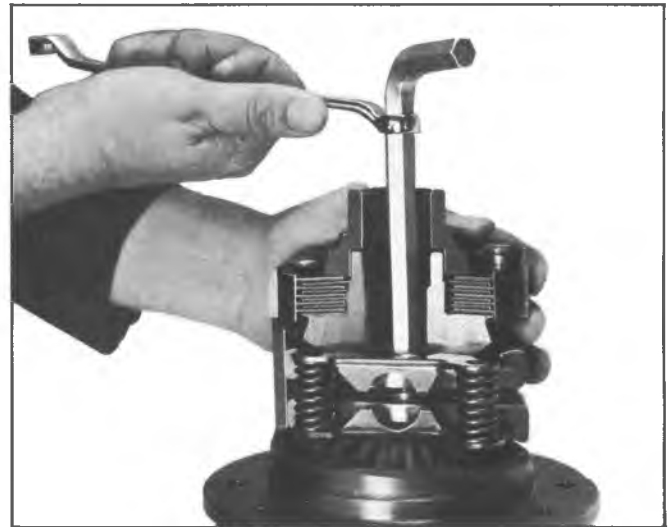
Fig. 5D—Removing Preload Spring Pack (Corvette)
