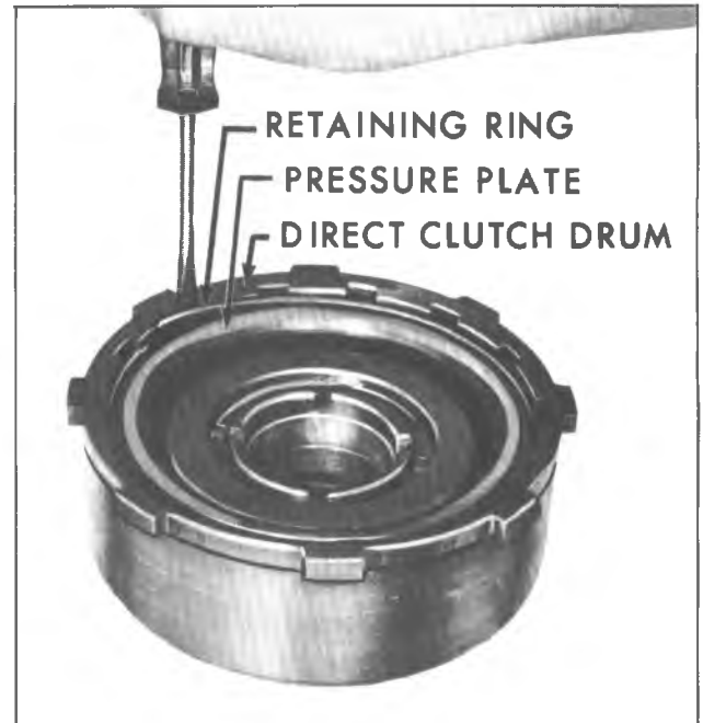
Fig. 63N--Removing Direct Clutch Pressure Plate
