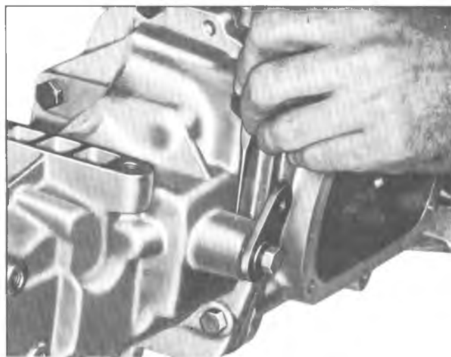
Fig. 4B--Removing Reverse Shifter Shaft Lock Pin
