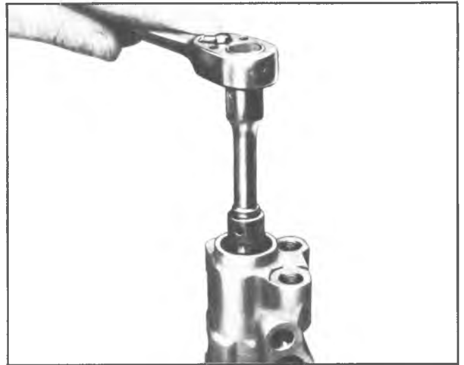
Fig. 64--Removing Adjusting Nut
