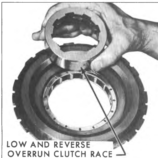
Fig. 84N--Removing Overrun Clutch Inner Race
