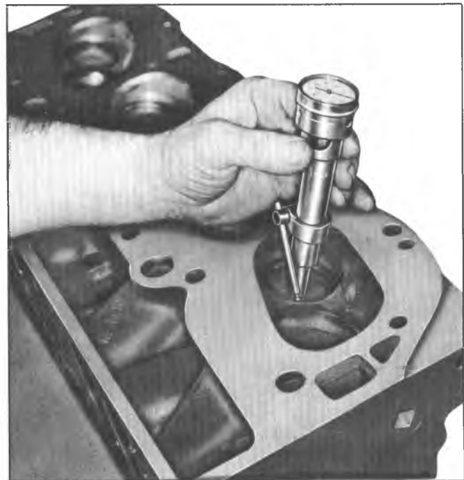
Fig. 24—Measuring Valve Seat Concentricity
