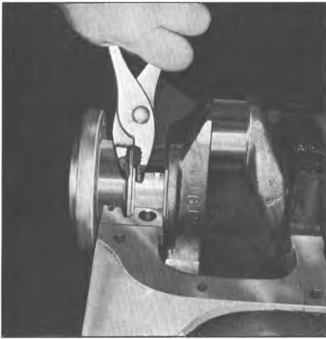
Fig. 42—Replacing Upper Main Bearing (In-Line)
