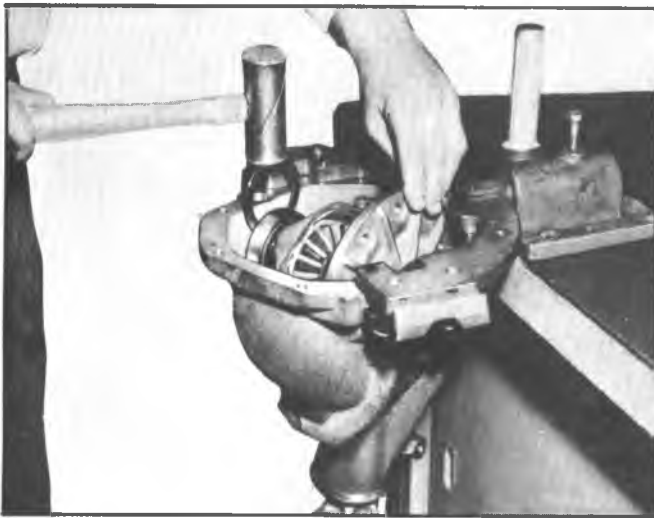
Fig. 11C—Installing Differential Shim
