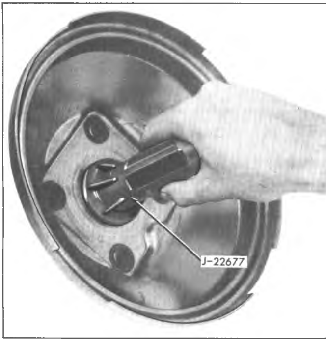
Fig. 4C--Installing Rear Housing Seal
