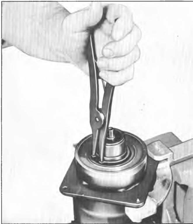
Fig. 8--Removing Coil Housing Retainer Ring
