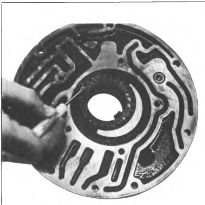
Fig. 63M--Installing Pump Drive and Driven Gears
