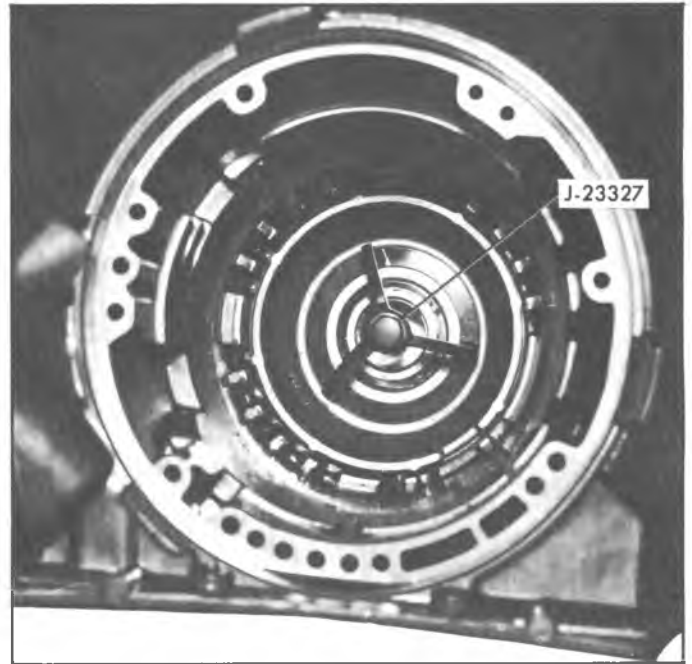
Fig. 44N--Compressing Low and Reverse Clutch Piston Spring Retainer
