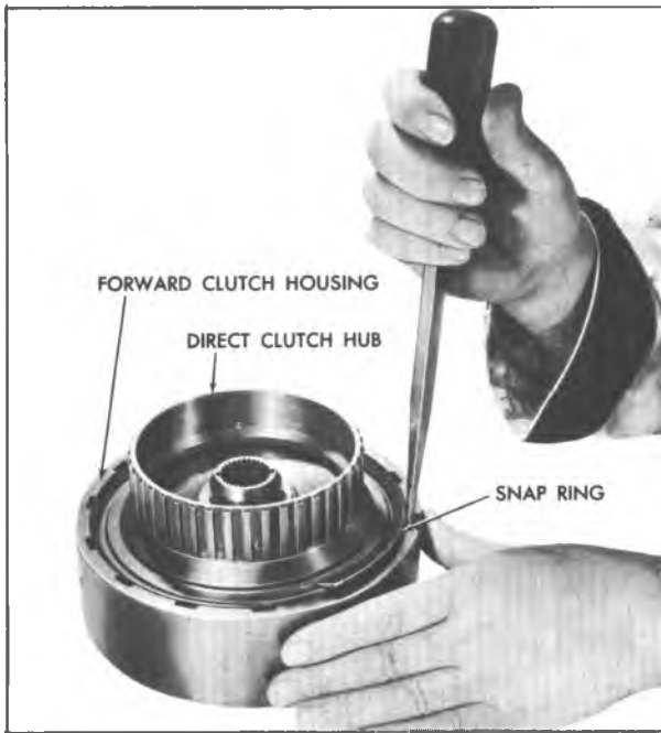
Fig. 76T--Installing Forward Clutch Housing to Direct Clutch Hub Snap Ring
