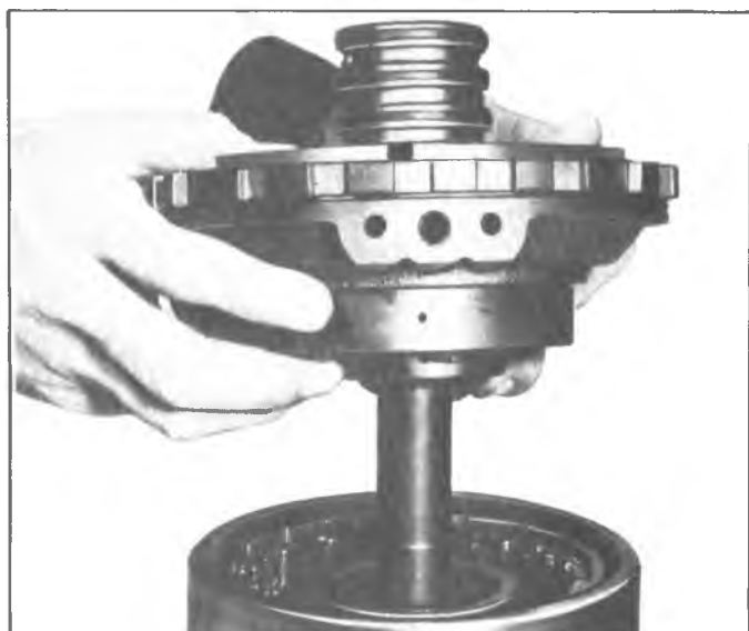
Fig. 125T--Installing Center Support to Reaction Carrier
