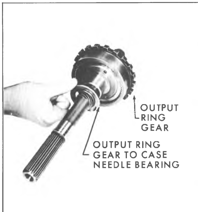
Fig. 43N--Removing Output Ring Gear to Case Needle Bearing Assembly
