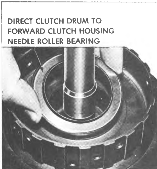
Fig. 71N--Direct Clutch Drum to Forward Clutch Housing Needle Roller Bearing
