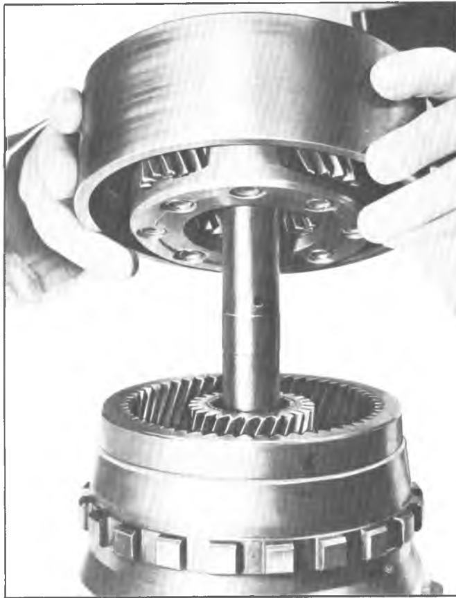
Fig. 121T--Installing Reaction Carrier
