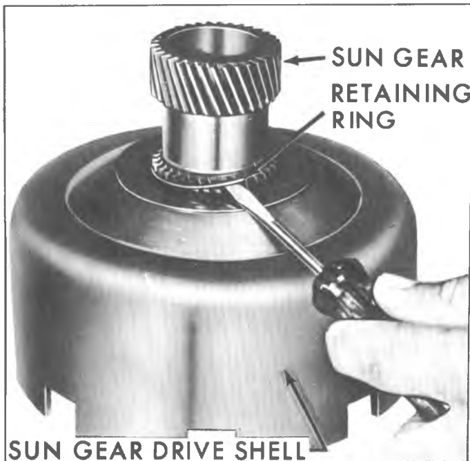
Fig. 80N--Removing Sun Gear Drive Shell Rear Retaining Ring
