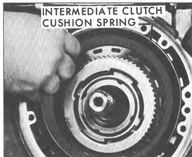
Fig. 28M--Removing Intermediate Clutch Cushion Spring
