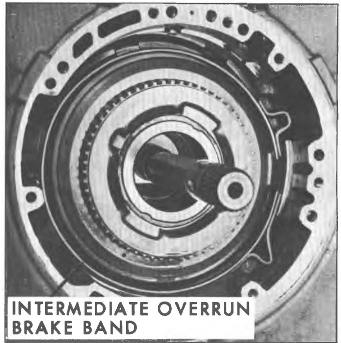
Fig. 31M--Removing Intermediate Overrun Brake Band
