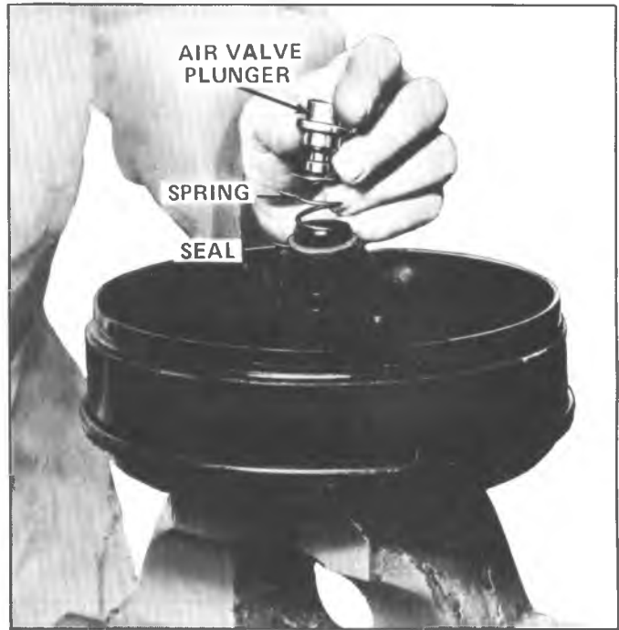
Fig. 9D--Installing Air Valve Assembly
