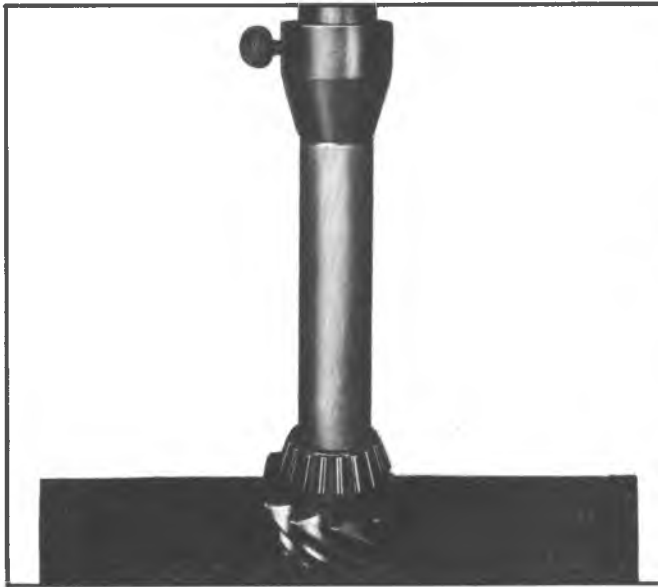
Fig. 24B—Installing Rear Bearing—Truck
