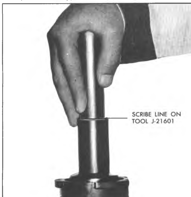
Fig. 10A--Installing Air Valve and Retainer
