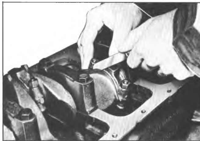
Fig. 45—Measuring Connecting Rod Side Clearance (In-Line)
