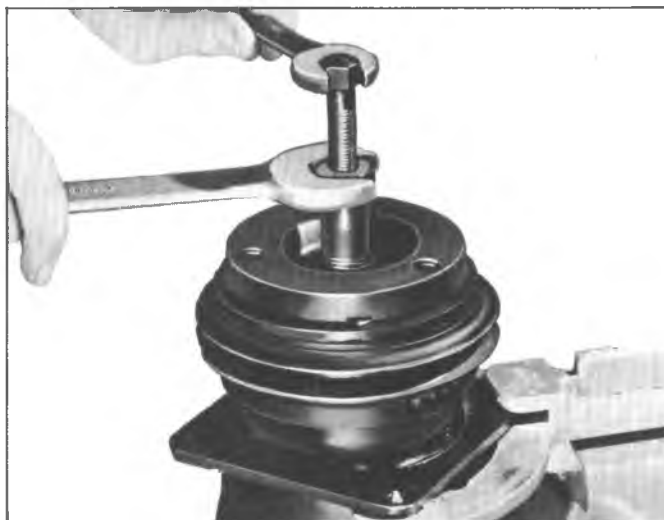
Fig. 3--Removing Hub and Drive Plate Assembly
