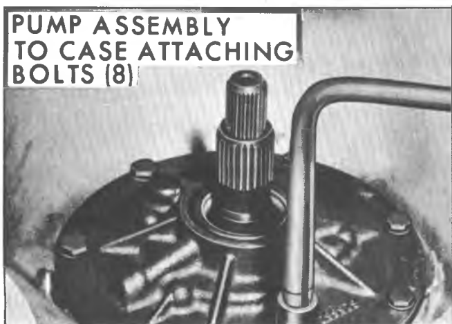
Fig. 26M--Removing Pump Attaching Bolts
