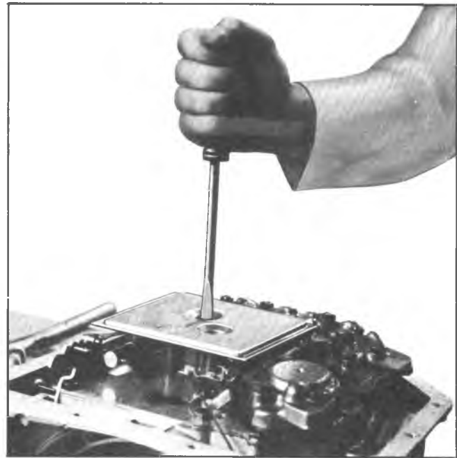
Fig. 10M--Removing Oil Pump Suction Screen (Strainer) from Valve Body
