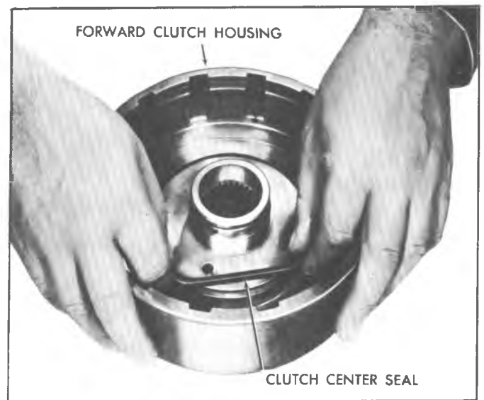
Fig. 72T--Removing Forward Clutch Center Seal
