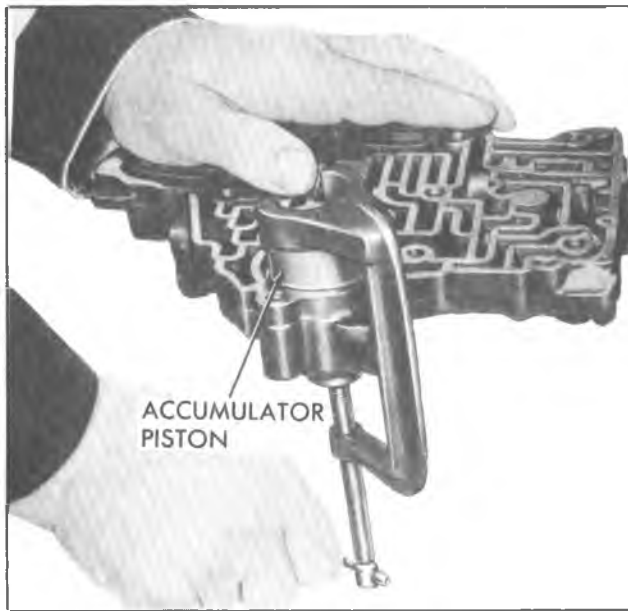
Fig. 53T—Installing Compressor Tool to Front Accumulator Piston
