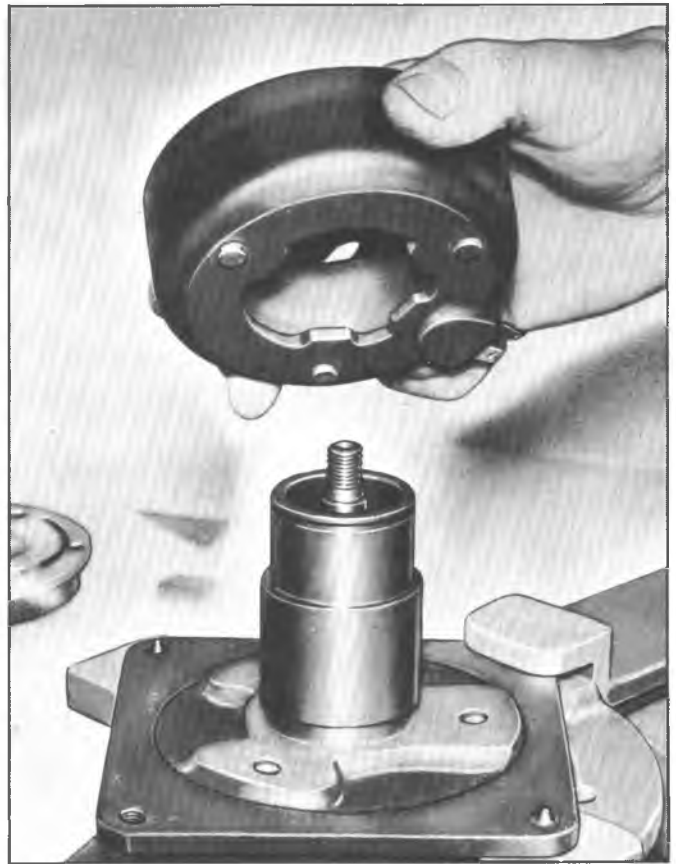
Fig. 9--Installing Coil Housing
