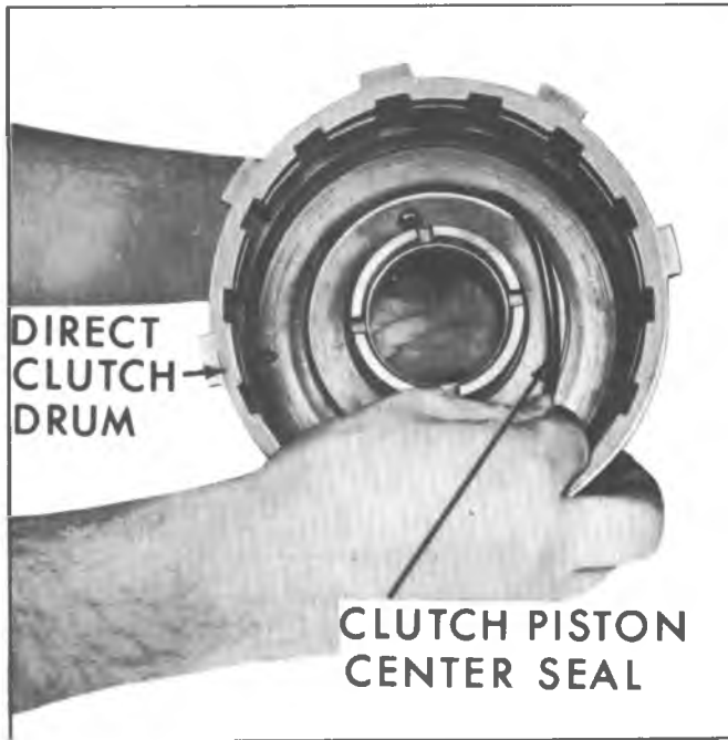
Fig. 74M--Removing Direct Clutch Piston Center Seal
