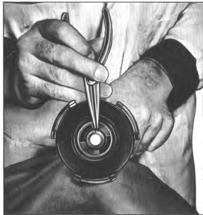
Fig. 10B--Removing Retaining Ring From Air Valve
