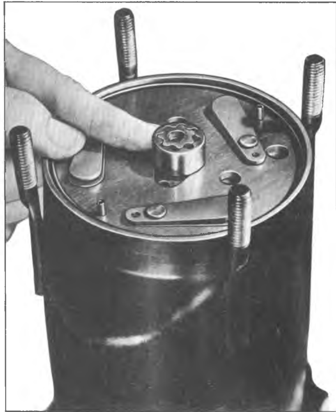
Fig. 15-Proper Oil Pump Gear Positioning
