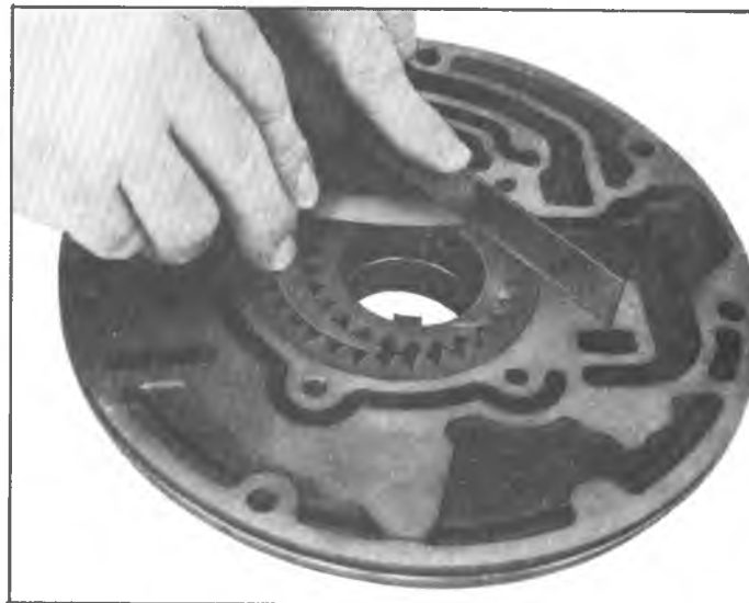
Fig. 65T--Checking Pump Body Face to Gear Face Clearance
