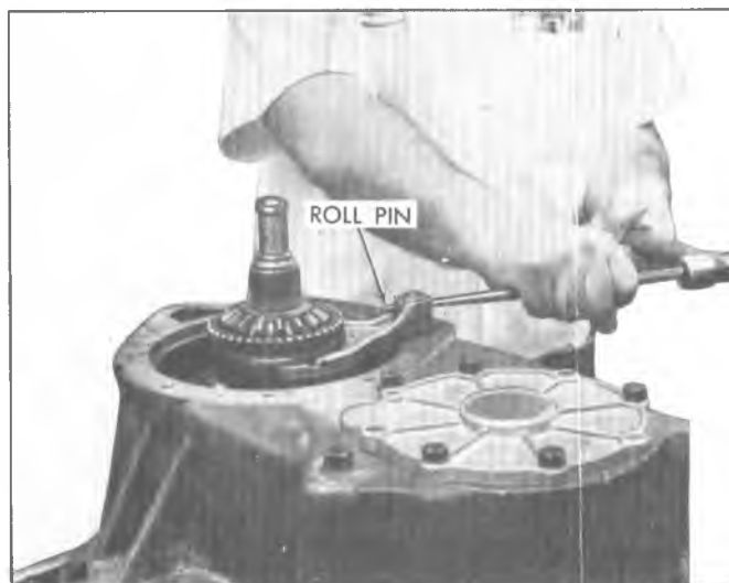
Fig. 7F—Removing Shift Fork Retaining Pin
