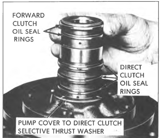
Fig. 58M--Pump Hub Oil Seal Rings
