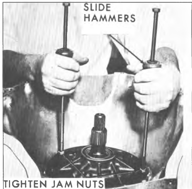
Fig. 27M--Removing Pump from Case
