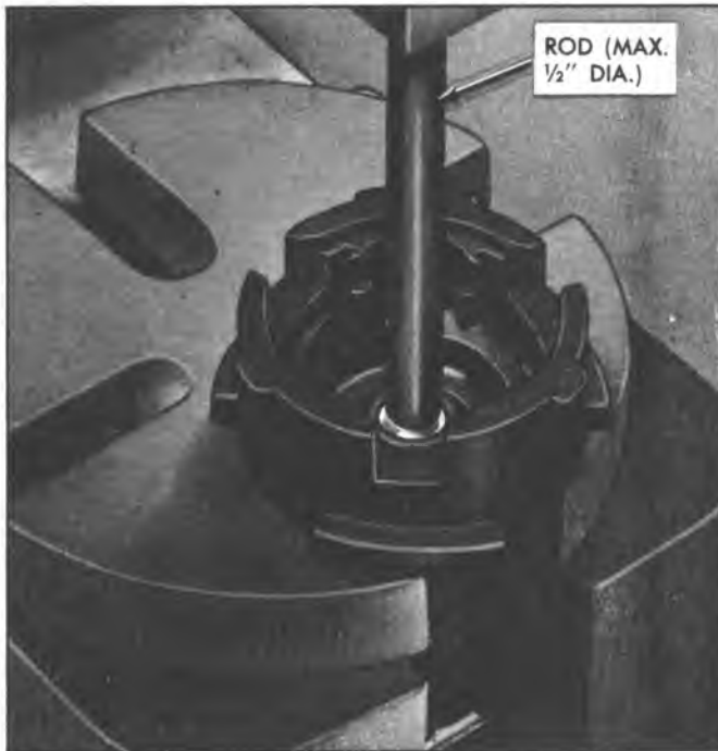
Fig. 9A--Removing Air Valve Assembly from Power Piston
