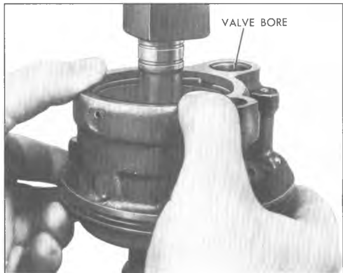
Fig. 29--Installing End Plate Retaining Ring
