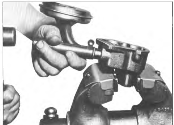
Fig. 38—Installing Screen ("Mark IV V8")
