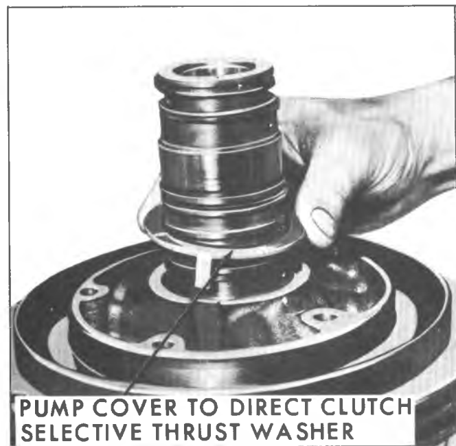
Fig. 104M--Pump Cover to Direct Clutch Selective Thrust Washer
