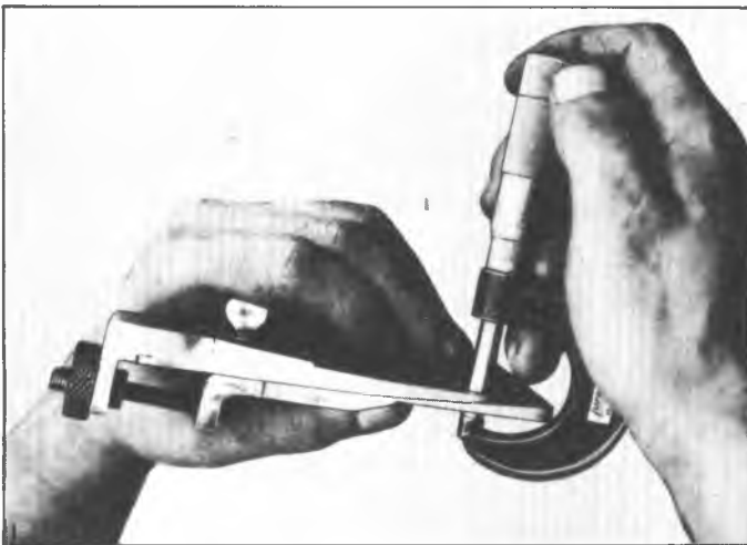
Fig. 8B—Measuring Gauge Plate Thickness
