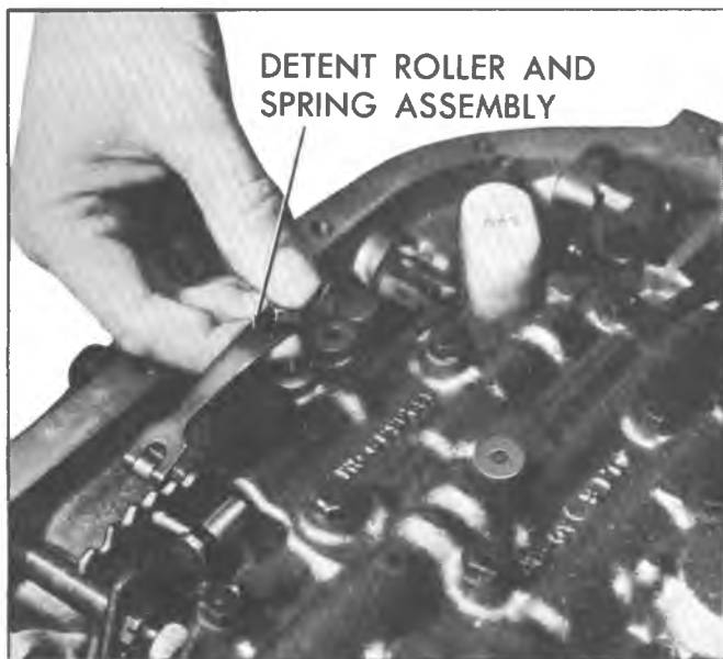
Fig. 9T--Removing Detent Roller and Spring Assembly
