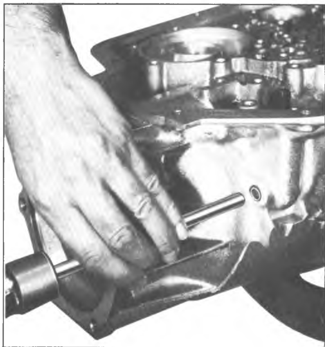
Fig. 127T--Installing Parking Pawl Shaft Cup Plug
