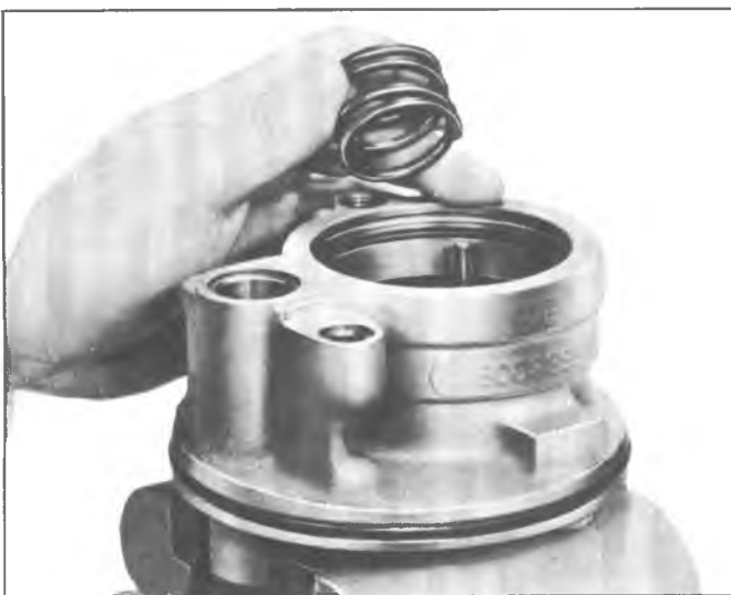
Fig. 28--Installing Pressure Plate Spring
