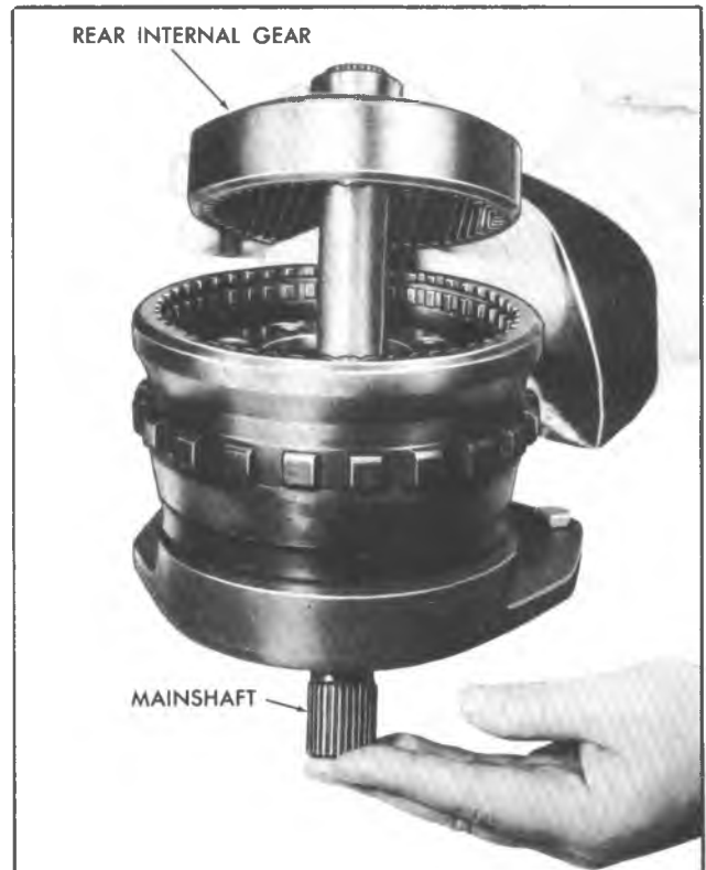
Fig. 44T--Removing Rear Internal Gear and Mainshaft
