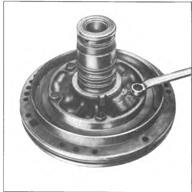
Fig. 53N--Removing Pump Cover to Pump Body Bolts
