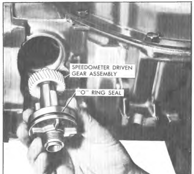
Fig. 155T--Installing Speedometer Driven Gear and Sleeve
