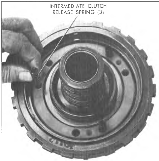
Fig. 98TB—Removing Clutch Release Springs
