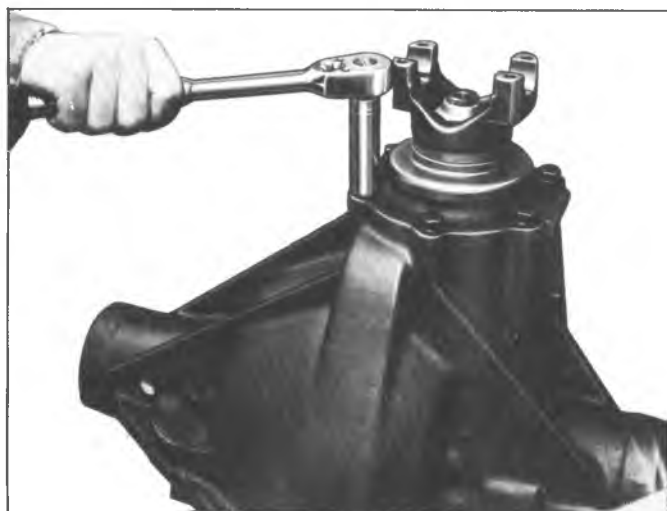
Fig. 7E—Removing Retainer Bolts
