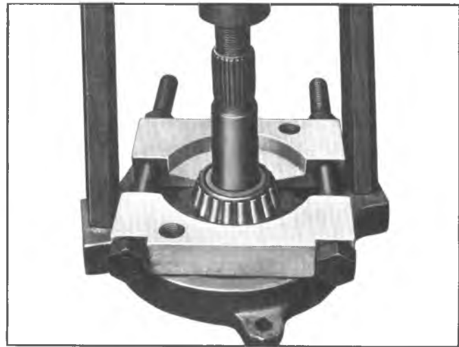
Fig. 6—Removing Inner Pinion Bearing Cone and Roller
