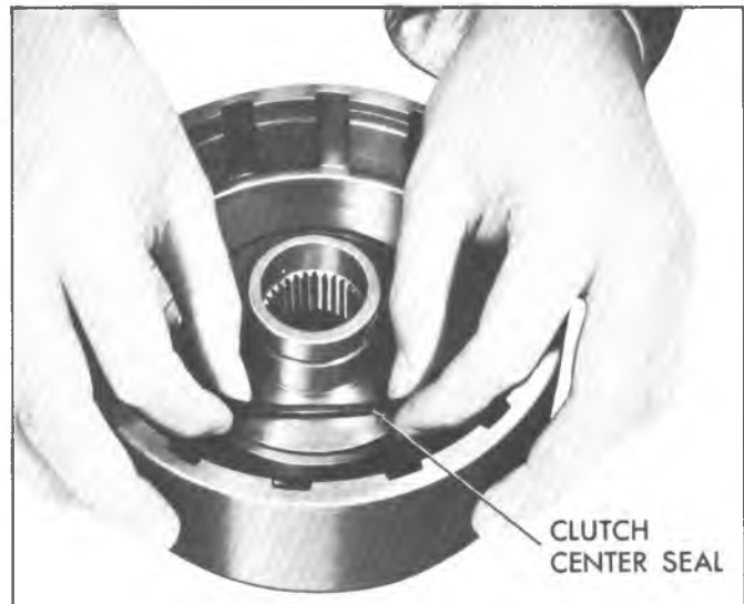
Fig. 86T--Installing Direct Clutch Center Seal
