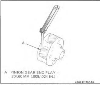
Figure 75 Pinion End Play Check
