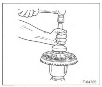
Figure 160-Installing the Differential Bearings
