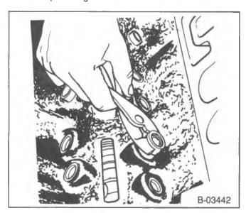
Figure 10—Removing the Hydraulic Lifter
