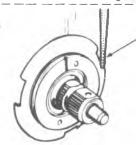
Using punch in notch tighten lock nut securely. Hold adjuster plug to maintain alignment of the marks.
