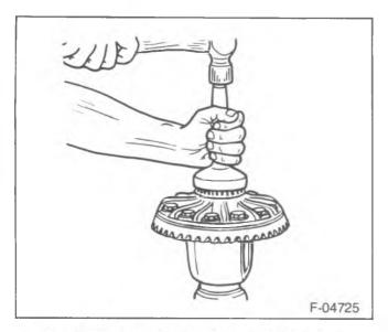
Figure 62—Installing the Differential Bearings
