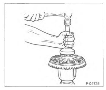
Figure 119—Installing the Differential Bearings
