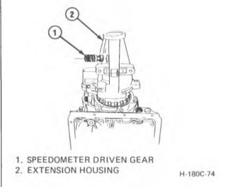
Figure 57 Extension Housing and Speedometer Driven Gear
