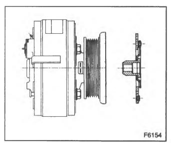
Figure 2—R-4 Compressor, Poly-Groove Pulley Type with a 6 Pole Clutch and Driver Shown
