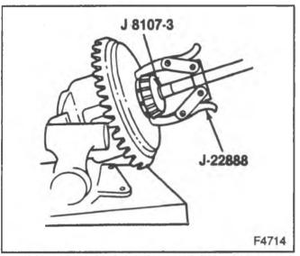
Figure 4—Removing Differential Side Bearings
