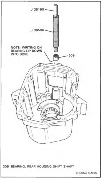
Figure 53 Shift Shaft Bearing Installation
