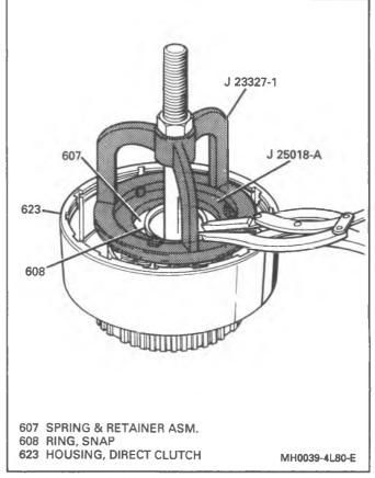
Figure 42 Removing Piston Release Spring Retainer
