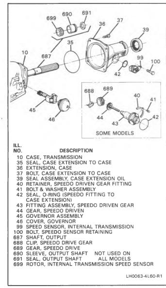
Figure 134 Case Extension and Associated Parts
