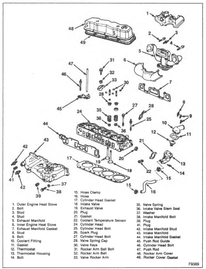
Figure 2---Cylinder Head, Manifolds, and Components
