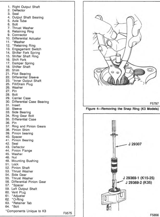
Figure 3—Front Axle Components (K1, 2,3 Models)
