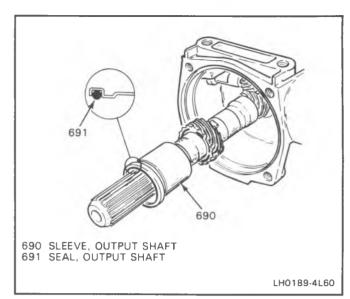
Figure 131 Output Shaft Sleeve and Seal
