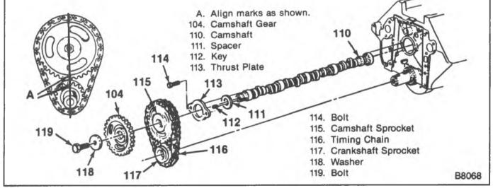
Figure 14—Camshaft and Components
