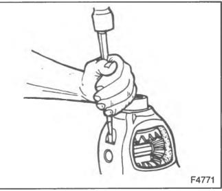
Figure 18—Installing the Lock Pin
