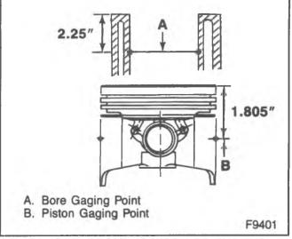
Figure 21-Measuring the Piston Diameter
