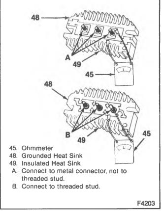
Figure 12—Rectifier Bridge Check
