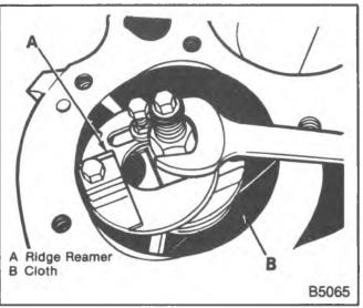
Figure 14—Removing the Cylinder Ridge
