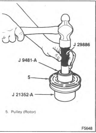
Figure 13---Installing the Pulley Rotor Bearing
