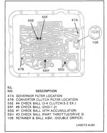
Figure 16 Case Checkballs and Filters
