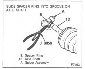
Figure 41—Installing Spider Assembly
