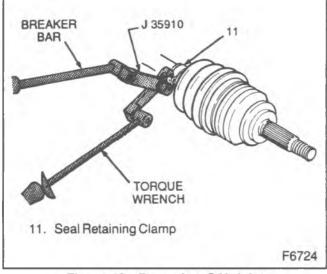
Figure 43—Removing C/V Joint
