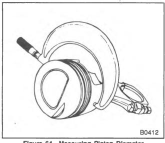
Figure 64—Measuring Piston Diameter
