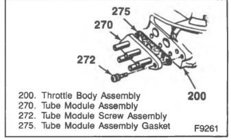
Figure 10-Tube Module Assembly-TBI 700
