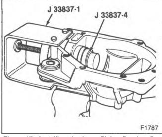
Figure 17-Installing the Inner Pinion Bearing Cup
