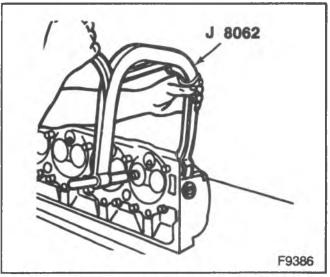
Figure 24—Compressing the Valve Springs
