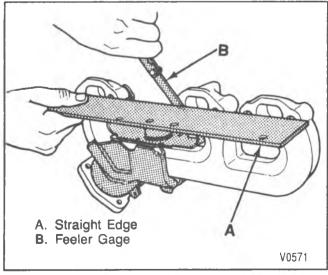
Figure 16—Checking Alignment of Manifold Flanges
