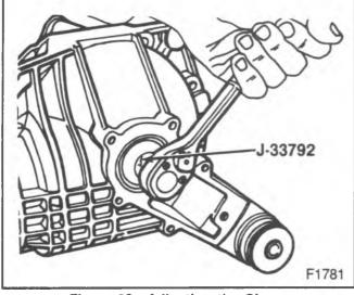
Figure 23—Adjusting the Sleeve
