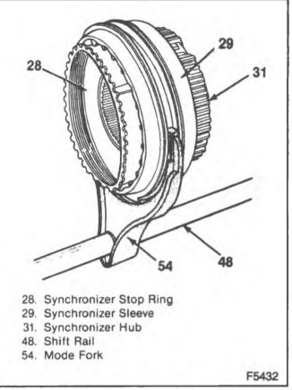
Figure 14-Synchronizer Hub Assembly and Mode Fork
