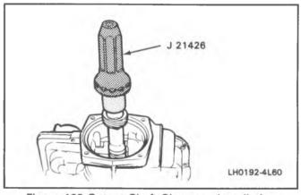
Figure 132 Output Shaft Sleeve — Installation
