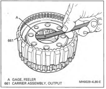
Figure 32 Measuring Pinion End Play
