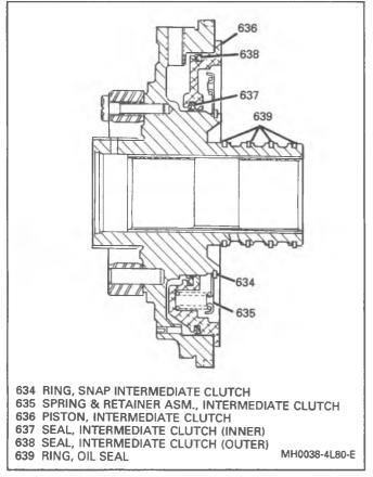
Figure 41 Center Support and Reaction Carrier Assembly
