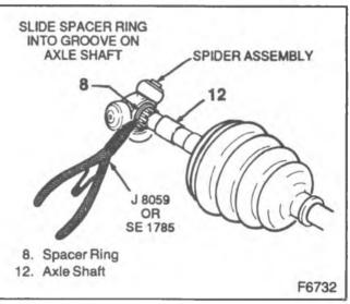
Figure 51—Installing Spider Assembly
