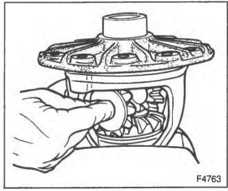
Figure 10-Removing the Pinion Gears
