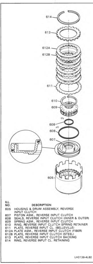
Figure 81 Reverse Input Clutch Assembly
