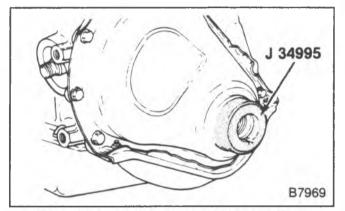
Figure 44—Installing the Timing Gear Cover
