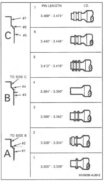
Figure 91 Servo Pin Selection
