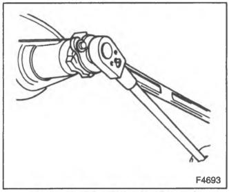
Figure 12-Drive Pinion Nut Removal
