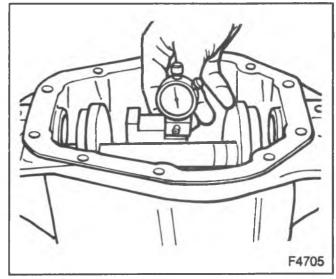
Figure 25—Scooter Gage on the Height Block
