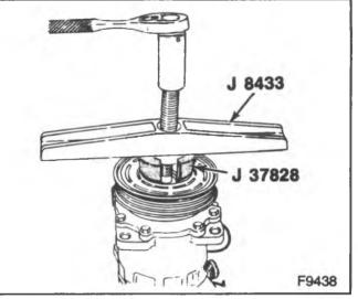
Figure 8—Removing the Rotor Pulley (Cont.)
