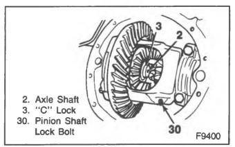
Figure 28—"C" Lock and Axle Shaft Seated in the Side Gear
