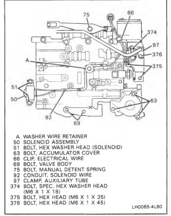
Figure 9 Valve Body Bolt Locations
