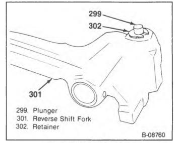
Figure 33 Plunger Retainer
