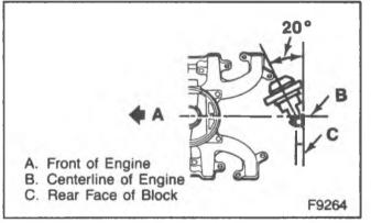
Figure 61—Vacuum Pump Installed
