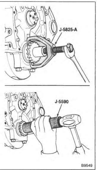
Figure 20—Replacing and installing the Camshaft Sprocket
