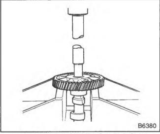
Figure 26-Removing the Camshaft Gear
