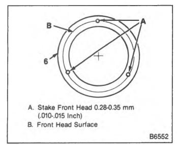
Figure 19—Clutch Coil Staking Locations
