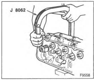
Figure 40—Compressing the Valve Springs
