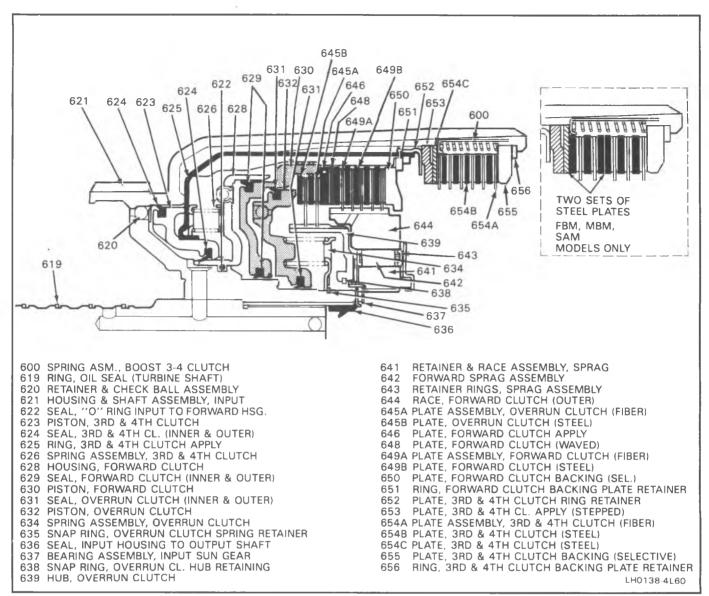
Figure 80 Input Clutch Assembly
