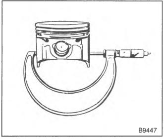
Figure 12—Measuring the Piston Skirt
