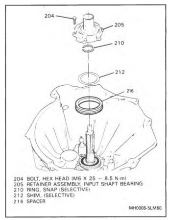
Figure 6 Removing Input Shaft Bearing Retainer Assembly
