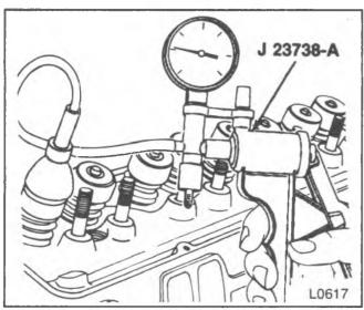
Figure 44—Checking the Valve Seal (5.0L and 5.7L Engines)
