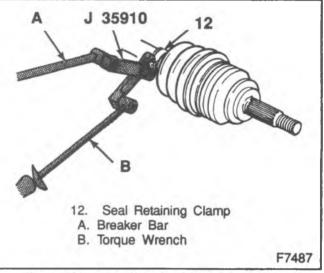
Figure 41-Installing Seal Retaining Clamp
