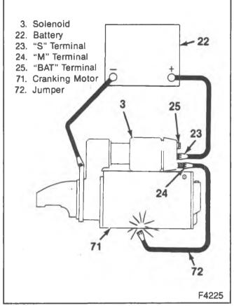
Figure 19—Pinion Clearance Circuit
