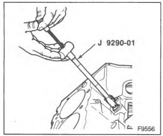
Figure 11-Removing the Hydraulic Lifters (Typical)
