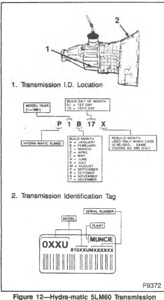
Figure 12—Hydra-matic 5LM60 Transmission I.D.Location
