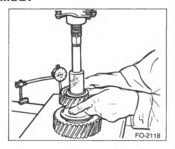
Figure 10—Idler Gear End Play Check
