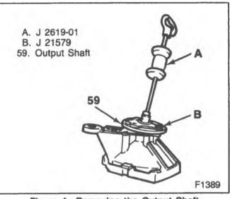
Figure 4-Removing the Output Shaft
