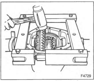
Figure 39-installing the Differential Case
