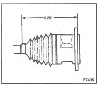
Figure 49-Tri-pot Seal Installation Measurement
