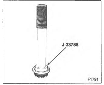
Figure 23-Installing the Sleeve Bearing
