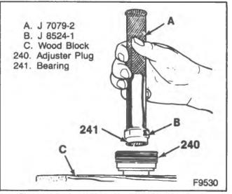
Figure 15—Installing the Needle Bearing in Adjuster Plug
