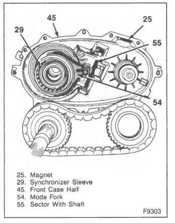
Figure 6—Mode Fork and Shaft Assembly
