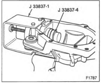
Figure 18-installing the Inner Pinion Bearing Cup
