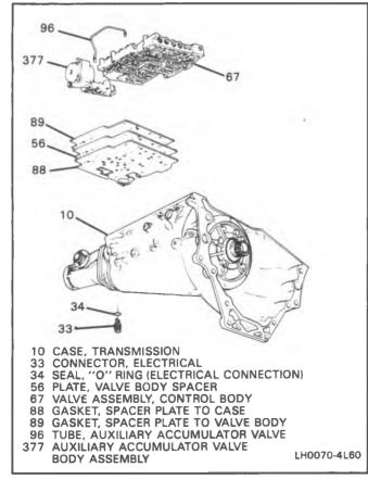
Figure 14 Control Valve, Auxiliary Valve Body, Spacer Plate and Gaskets
