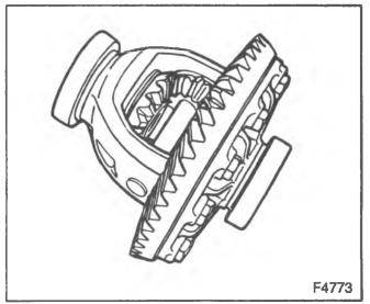
Figure 21—Differential with Master Bearings
