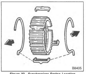
Figure 23—Synchronizer Spring Location
