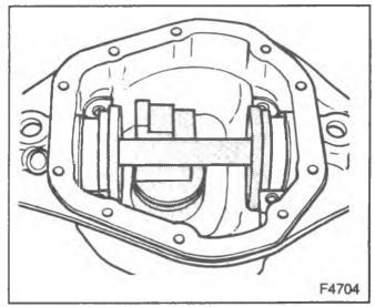
Figure 65—Pinion Height Block
