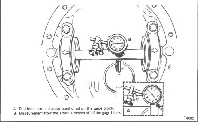
Figure 15-Checking Pinion Depth
