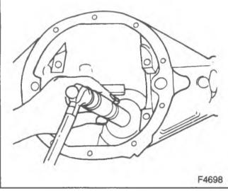
Figure 11-Installing the Rear Pinion Bearing Cup
