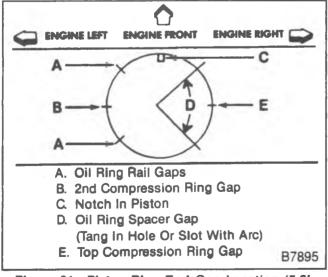
Figure 61—Piston Ring End Gap Location (5.0L and 5.7L Engines)
