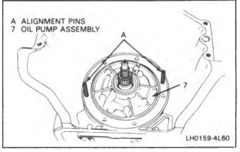
Figure 101 Oil Pump and Case
