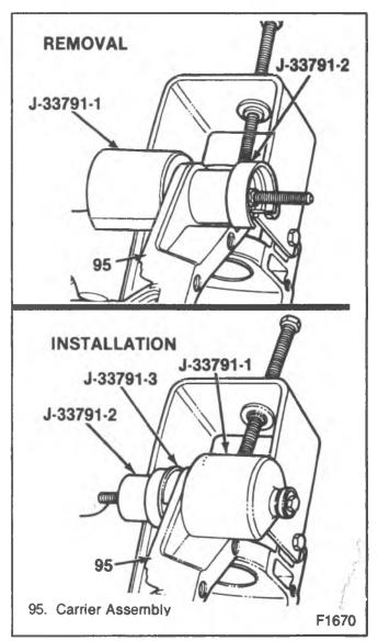
Figure 15-Replacing the Case Bushings
