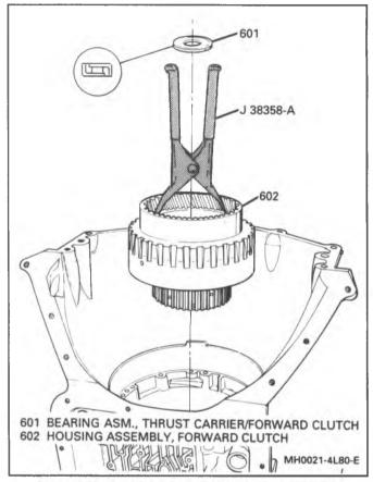
Figure 62 Installing Forward Clutch Assembly
