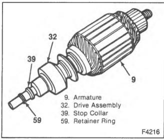
Figure 8—Retaining Ring on Armature
