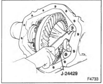
Figure 22—Adjusting the Nut
