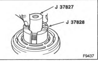
Figure 7—Removing the Rotor Pulley
