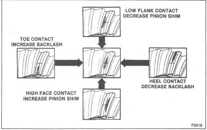
Figure 30---Gear Tooth Pattern
