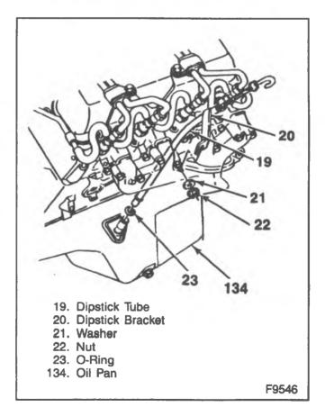
Figure 8-Dipstick Tube Assembly
