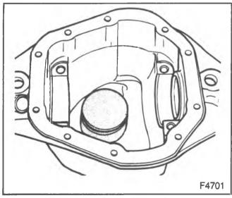
Figure 23—Master Pinion Block
