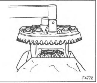
Figure 60—Installing the Ring Gear Bolts
