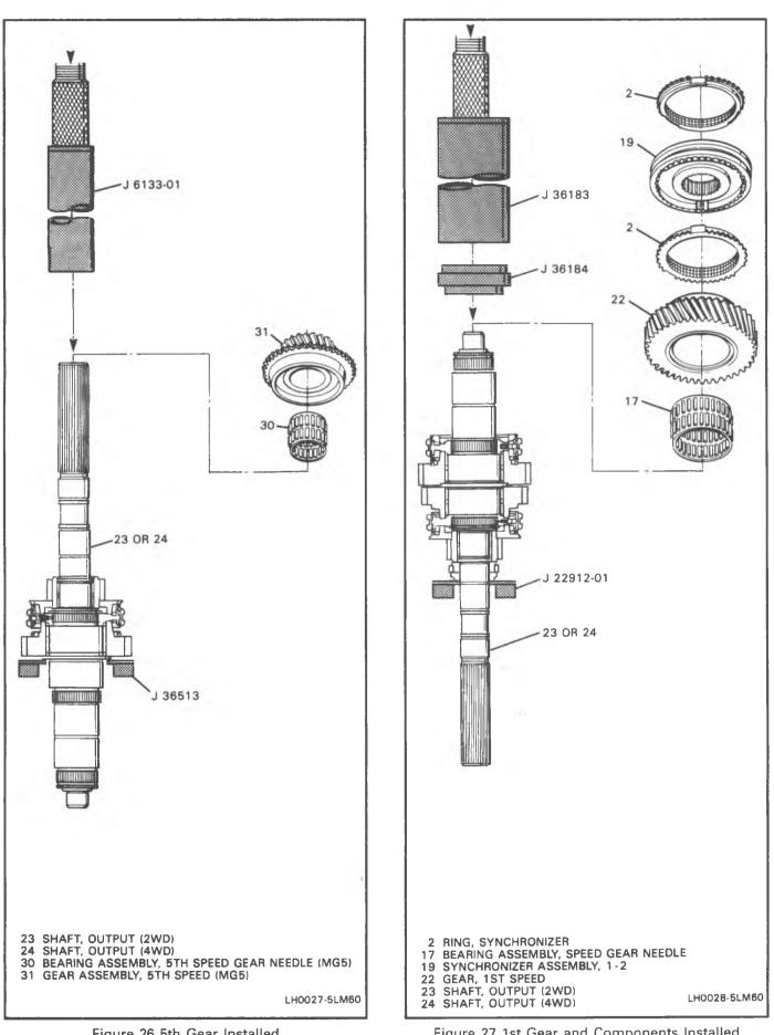
Figure 26 5th Gear Installed
