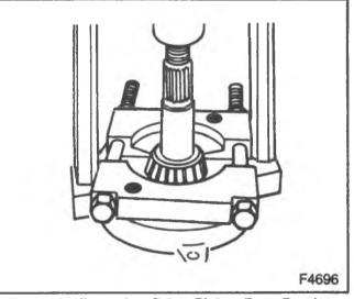
Figure 8—Removing Drive Pinion Rear Bearing
