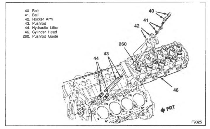
Figure 12-Cylinder Head Components (7.4L Engines)
