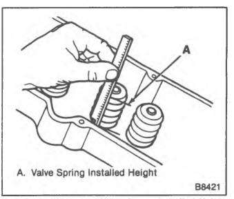
Figure 29-Measuring Valve Spring Installed Height
