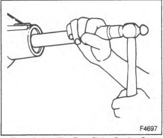
Figure 9-Installing Front Pinion Bearing Cup
