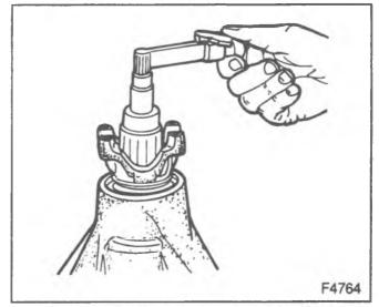
Figure 52—Checking the Pinion Preload
