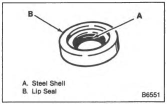
Figure 20—Compressor Shaft Seal
