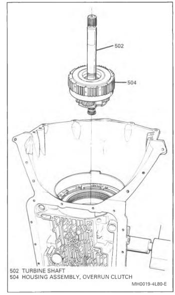
Figure 19 Removing Overdrive Clutch Assembly
