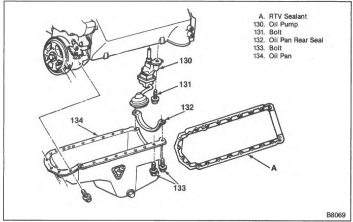
Figure 15-Oil Pan and Oil Pump
