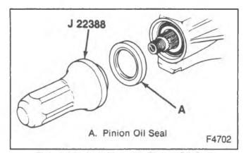
Figure 15-Installing the Pinion Oil Seal
