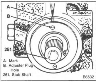
Figure 17—Marking the Housing
