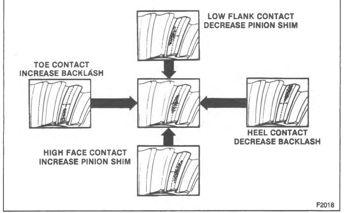
Figure 30-Gear Tooth Contact Pattern
