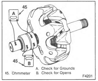
Figure 10—Checking Rotor Field Windings
