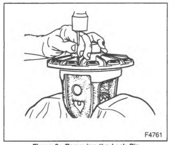
Figure 8—Removing the Lock Pin
