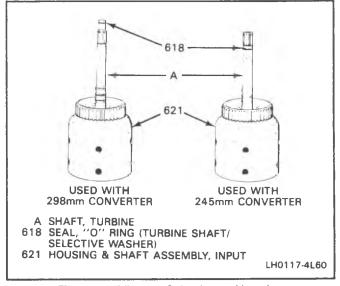
Figure 59 Views of the Input Housing
