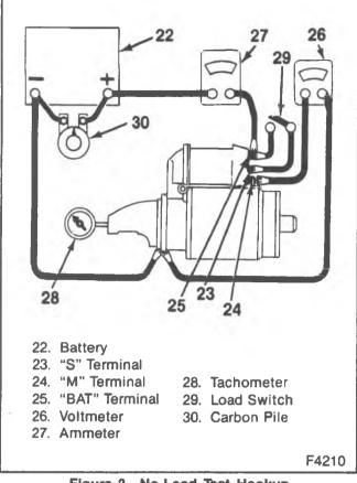
Figure 3-No-Load Test Hookup
