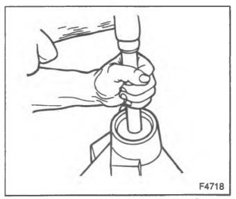
Figure 30-Installing the Pinion Front Cup
