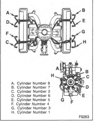
Figure 57—Injection Line Routing
