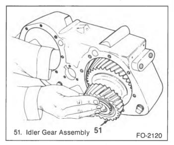
Figure 11—Installing the Idler Gear Assembly
