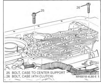
Figure 18 4th Clutch Bolt and Center Support Bolt Location
