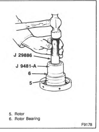
Figure 13-Installing the Clutch Rotor Bearing
