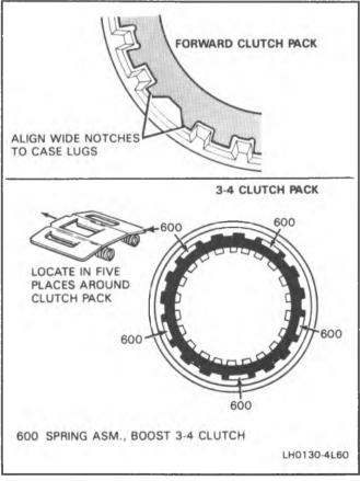
Figure 72 Forward and 3-4 Clutch Plates — Installed
