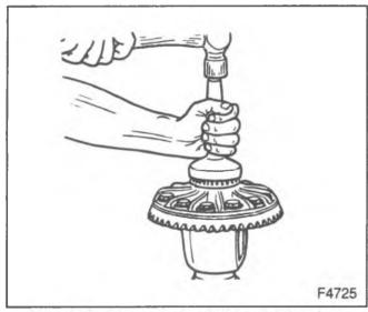
Figure 78—Installing the Differential Bearings
