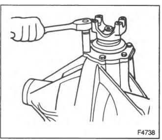
Figure 4—Removing the Pinion Cage
