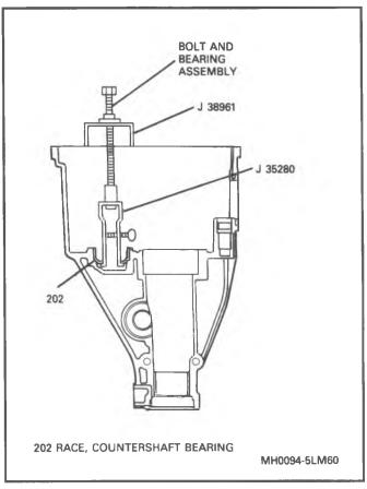
Figure 51 Removing Countershaft Bearing Race
