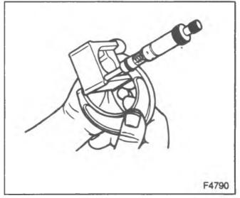
Figure 7—Measuring the Thrust Block
