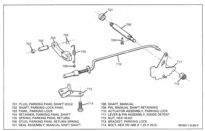
Figure 112 Parking Lock and Actuator Assembly
