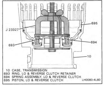
Figure 24 Lo and Reverse Snap Ring Removal
