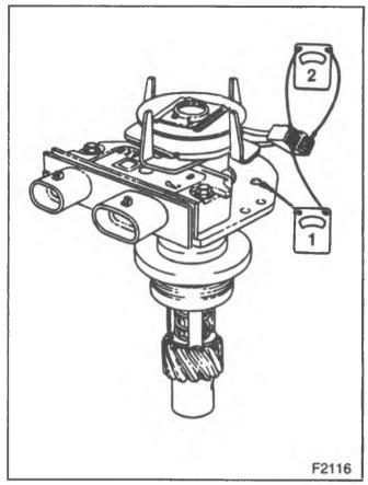
Figure 10—Testing the Pickup Coil
