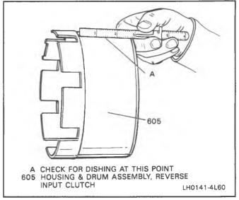
Figure 83 Check Reverse Input Housing For Dishing
