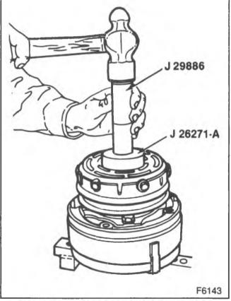
Figure 15—Installing the Rotor and Bearing (V-Groove Type)
