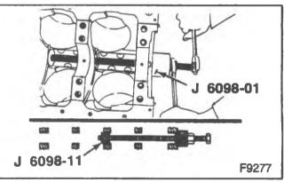
Figure 20-Replacing the Inner Camshaft Bearings
