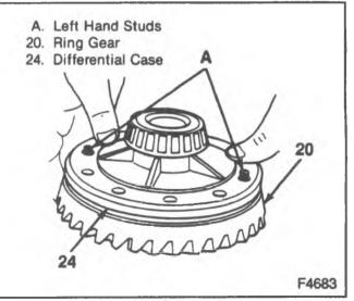
Figure 16-Ring Gear Studs
