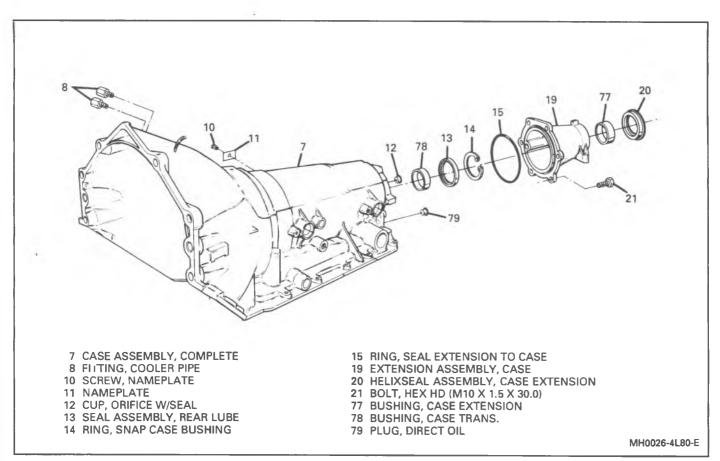
Figure 27 Transmission Case and Extension Assembly
