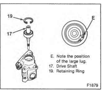
Figure 28—Removing and Installing Retaining Ring
