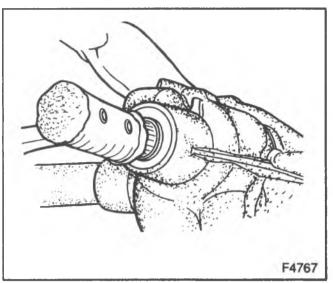
Figure 14—Removing the Pinion
