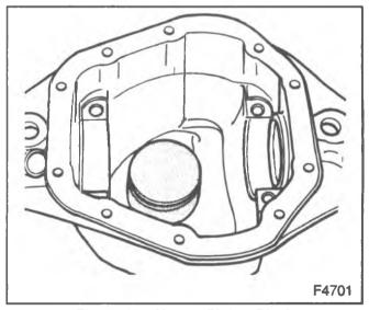
Figure 22—Master Pinion Block
