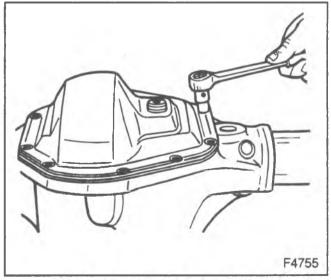
Figure 82—Installing the Axle Cover
