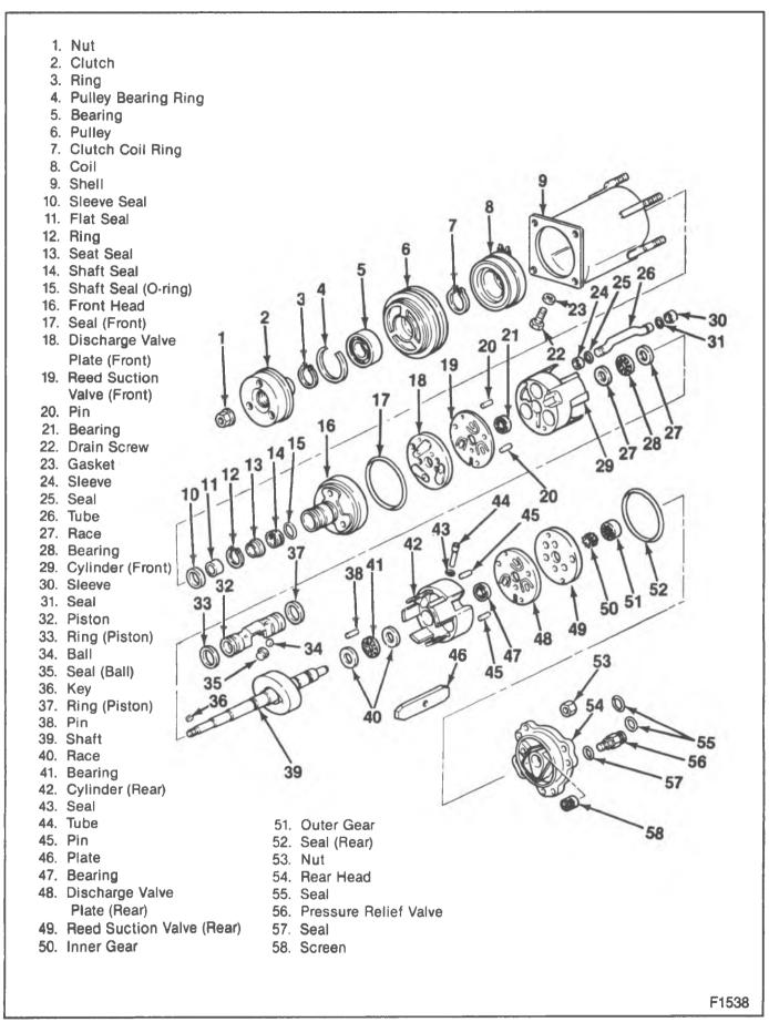
Figure 1-Compressor Component View
