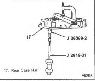
Figure 9—Front Output Shaft Rear Bearing Removal
