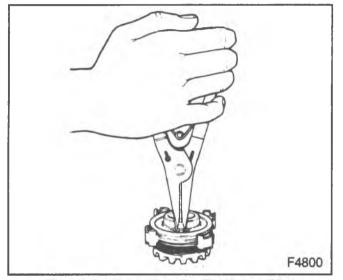
Figure 3—Removing the Retaining Ring
