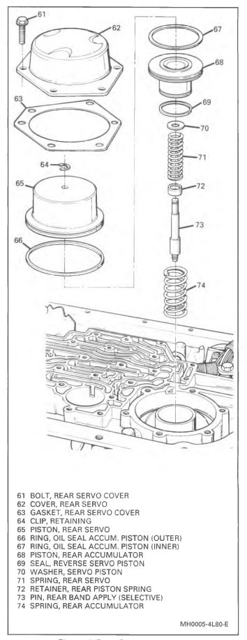
Figure 5 Rear Servo Assembly
