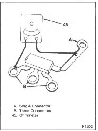
Figure 11—Diode Trio Check
