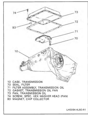
Figure 119 Case, Pan and Filter Assembly
