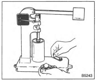
Figure 29—Testing the Hydraulic Lifter—Flat Type Only
