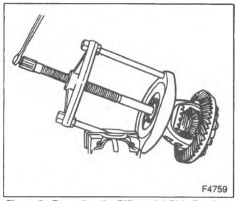
Figure 6-Removing the Differential Side Bearings
