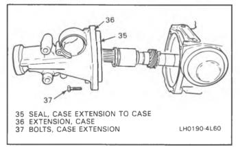
Figure 133 Case Extension and Seal
