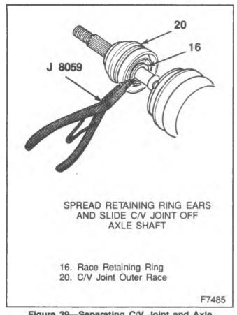
Figure 39-Separating C/V Joint and Axle
