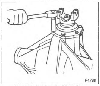
Figure 15—Installing the Pinion Cage
