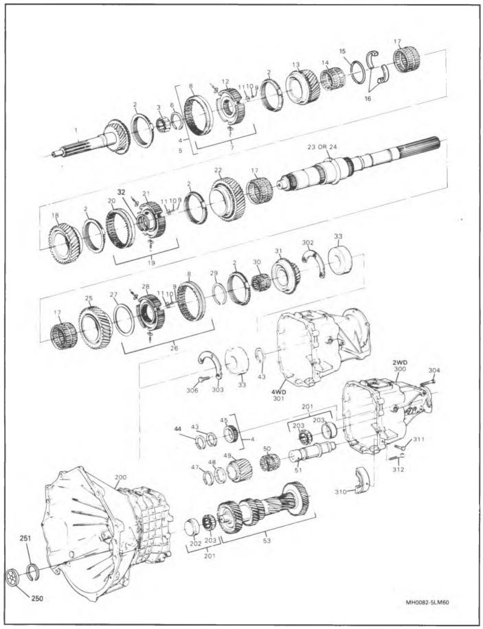
Figure 79 Transmission Gear Components
