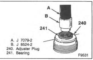
Figure 8—Removing the Needle Bearing from **Adjuster Plug**
