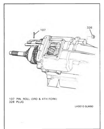
Figure 10 Removing 3-4 Rail Plug and Roll Pin
