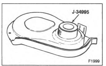
Figure 29-Installing the Front Crankshaft Seal
