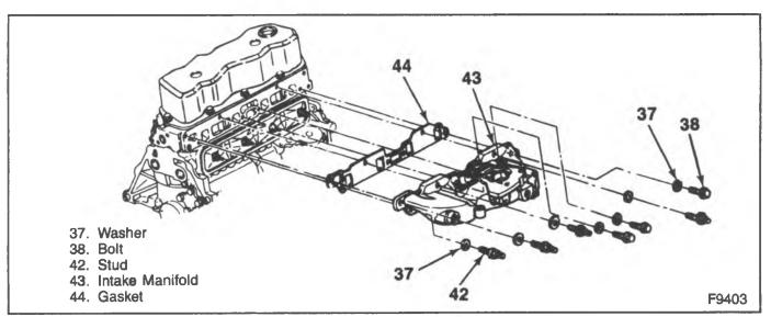
Figure 5-Intake Manifold Components
