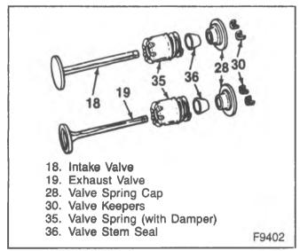
Figure 32—Valves and Components
