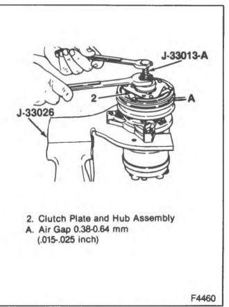
Figure 8-Installing the Clutch Plate and **Hub Assembly**
