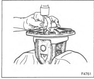
Figure 49—Removing the Lock Pin
