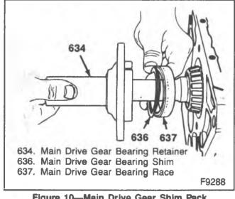
Figure 10—Main Drive Gear Shim Pack
