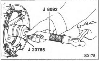
Figure 26-Installing the Axle Bearing
