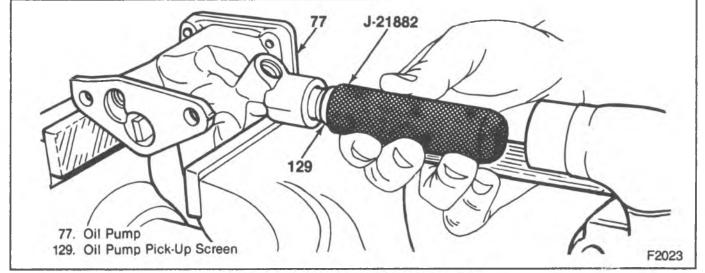
Figure 31-Installing the Oil Suction Pipe
