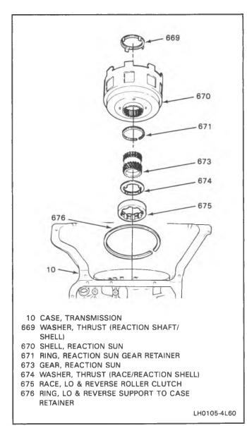
Figure 48 Reaction Sun Gear and Shell Installation
