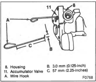
Figure 4-Removing the Accumulator Valve
