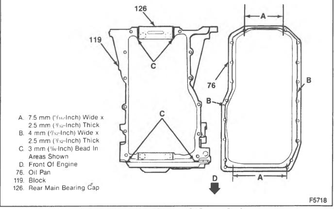
Figure 49—Applying RTV to the Oil Pan and Block
