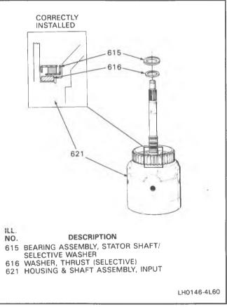
Figure 105 Selective Washer and Thrust Bearing Properly Installed
