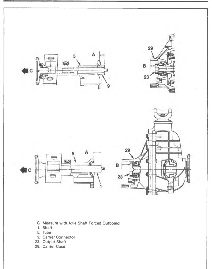
Figure 36—Measuring to Calculate Shim Size
