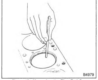
Figure 16—Measuring the Ring End Gap
