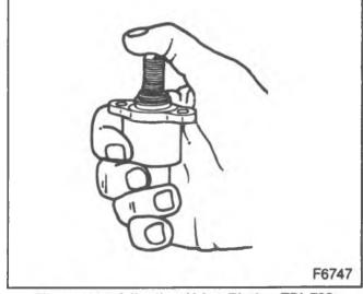
Figure 11-Adjusting Valve Pintle-TBI 700
