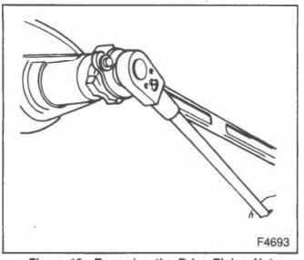
Figure 12—Removing the Drive Pinion Nut
