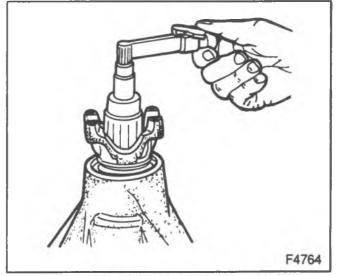
Figure 35—Checking Pinion Preload
