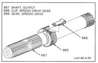
Figure 129 Speedometer Gear
