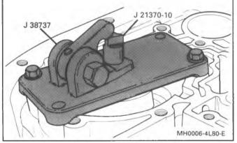
Figure 89 Installing Servo Pin Gage
