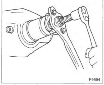
Figure 13-Removing the Pinion Flange
