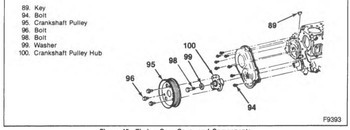
Figure 45—Timing Gear Cover and Components
