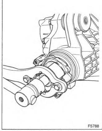
Figure 10-Removing the Pinion Nut
