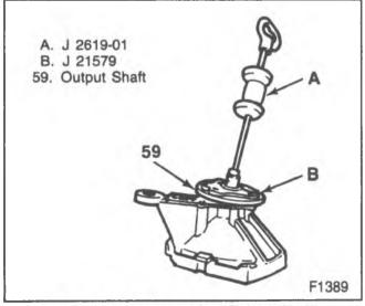
Figure 5—Removing the Output Shaft
