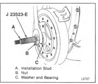
Figure 34—Installing the Torsional Damper
