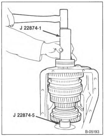
Figure 39 Installing the Mainshaft Rear Bearing
