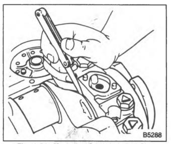
Figure 54-Measuring Crankshaft End Play
