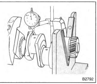
Figure 36—Checking Crankshaft Runout
