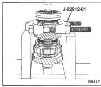
Figure 19—Removing the 3rd and 4th Synchronizer
