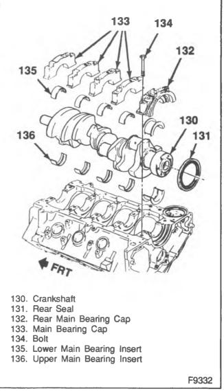
Figure 27—Crankshaft and Components (7.4L Engines)
