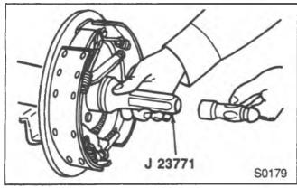
Figure 27-Installing the Axle Seal
