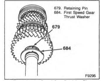
Figure 21-1st Speed Gear Retaining Ring
