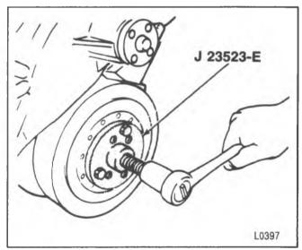
Figure 5-Removing the Torsional Damper
