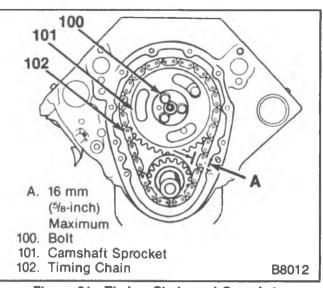
Figure 21—Timing Chain and Sprockets
