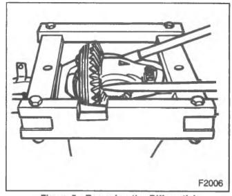
Figure 5-Removing the Differential
