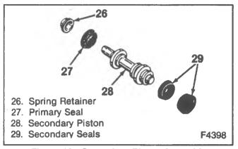
Figure 16—Secondary Piston Assembly
