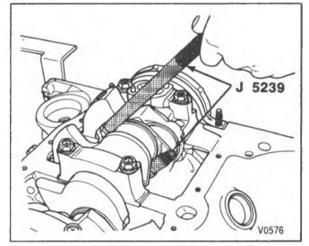
Figure 37—Guiding the Connecting Rod
