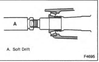
Figure 7—Removing the Drive Pinion
