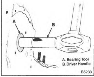
Figure 28—Removing or Installing Camshaft Bearings
