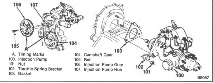
Figure 47—injection Pump
