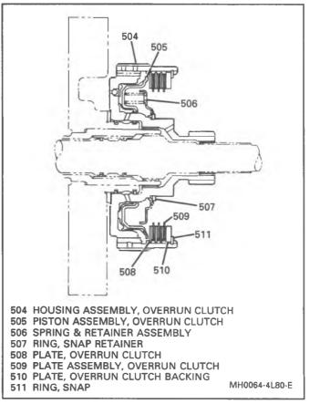
Figure 71 Overrun Clutch Assembly
