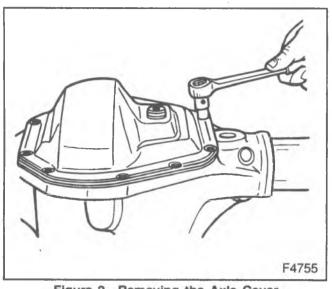
Figure 2-Removing the Axle Cover
