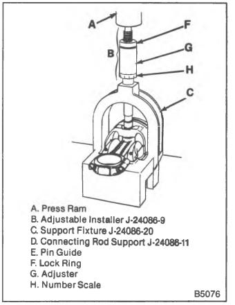
Figure 13—Installing the Piston Pin
