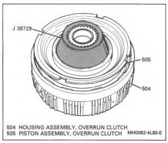
Figure 69 Installing Overrun Clutch Piston
