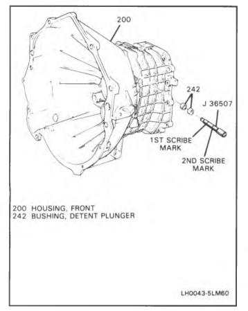
Figure 42 Detent Plunger Bushing Installation
