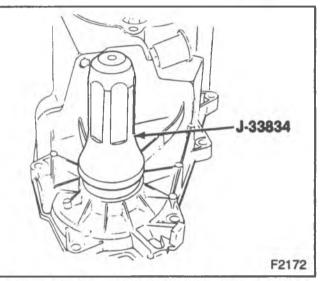
Figure 12-Front Output Shaft Seal Installation
