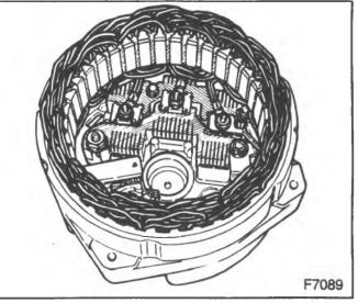
Figure 13-Stator in the Slip Ring End Frame
