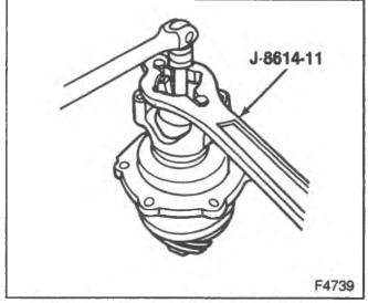
Figure 5-Removing the Drive Pinion Nut
