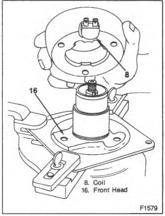
Figure 12—Installing the Coll Housing
