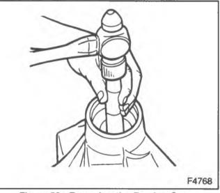
Figure 56—Removing the Bearing Cups
