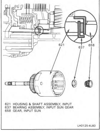
Figure 67 Input Sun Gear Thrust Bearing
