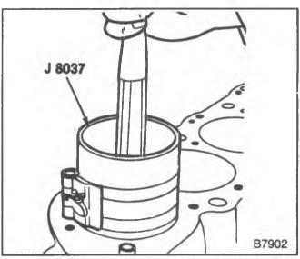
Figure 38—Installing the Piston and Connecting Rod
