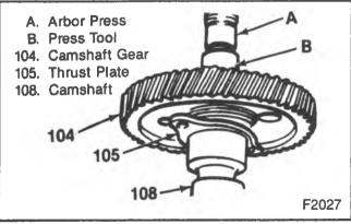
Figure 27-Installing the Camshaft Gear
