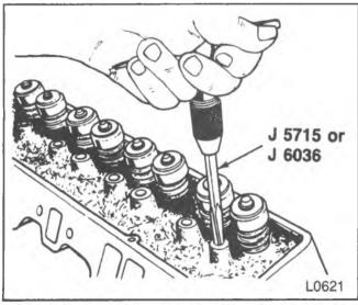
Figure 42—Reaming the Rocker Arm Stud Bore (5.0L and 5.7L Engines)
