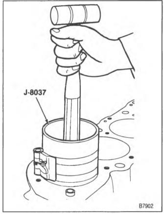
Figure 36—Installing the Piston
