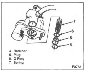
Figure 3—Removing the Plug and Spring
