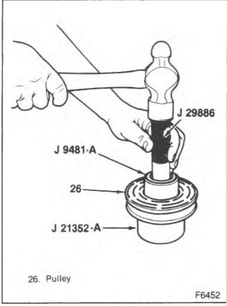
Figure 12-Installing the Pulley Rotor Bearing
