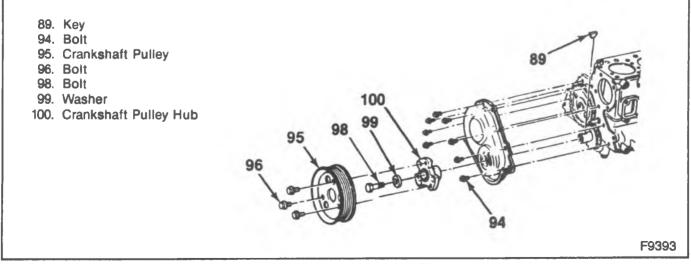
Figure 12—Timing Gear Cover and Components
