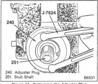
Figure 16-Bottoming the Adjuster Plug
