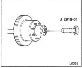
Figure 3 - Removing/Installing the Axle Shaft.
