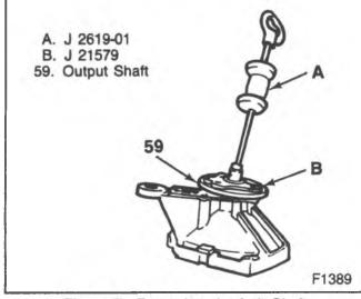
Figure 7-Removing the Left Shaft
