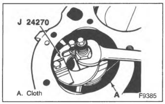
Figure 14—Removing the Cylinder Ridge
