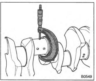
Figure 49-Measuring the Crankshaft Journals
