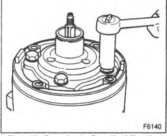
Figure 26—Removing the Front Head Mounting Screws
