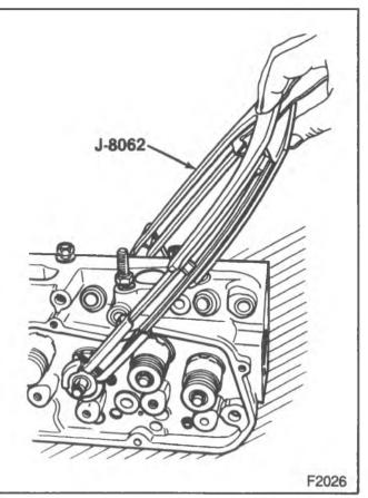
Figure 33-Compressing the valve Springs
