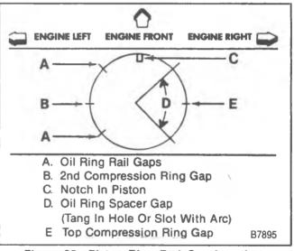
Figure 35—Piston Ring End Gap Locations
