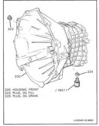
Figure 39 Removing Drain/Fill Plugs
