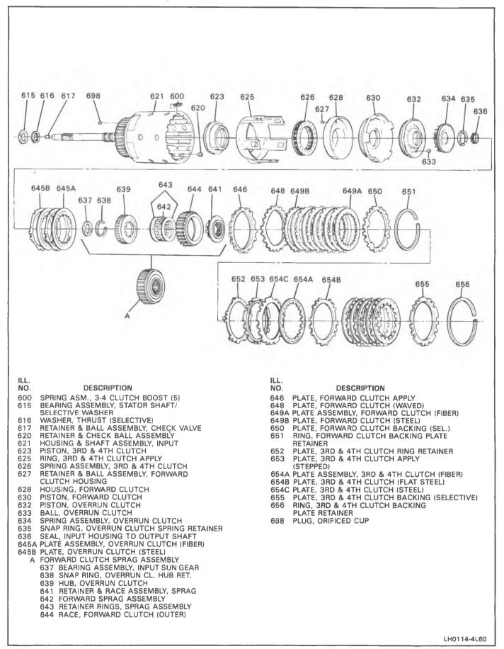
Figure 56 Input Clutch Assembly
