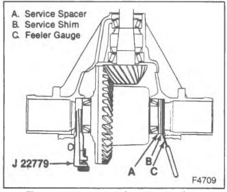
Figure 22—Measuring Side Bearing Shim Requirements
