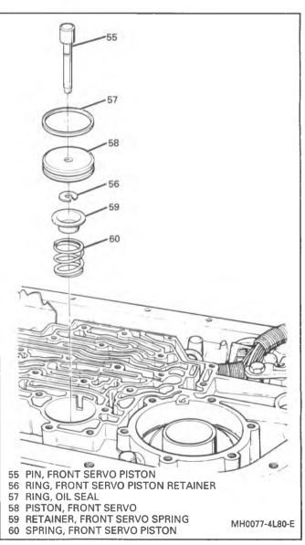
Figure 88 Front Servo Assembly
