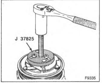
Figure 4-Removing the Clutch Plate
