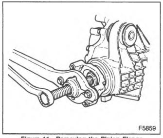
Figure 11—Removing the Pinion Flange
