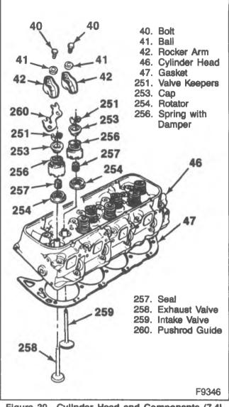
Figure 39—Cylinder Head and Components (7.4L Engines)
