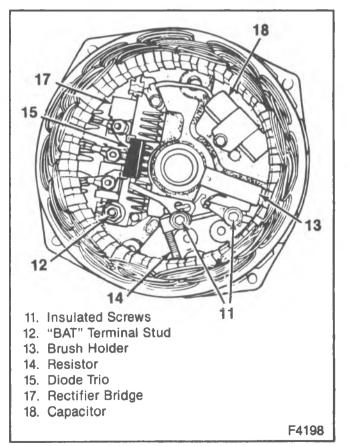
Figure 7-Slip Ring End Frame: 17-SI 100
