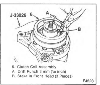
Figure 19—Staking the Clutch Coil Assembly to the Coil Head
