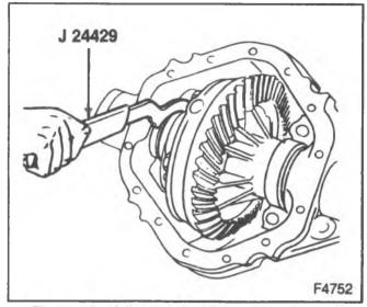
Figure 18-Adjusting the Differential Preload
