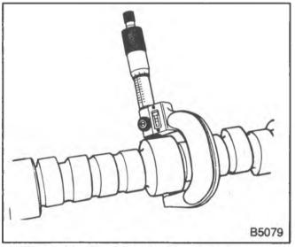
Figure 24—Checking the Camshaft Journals
