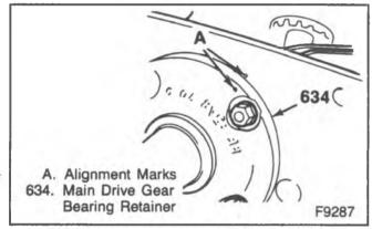
Figure 9—Bearing Cap Alignment Marks
