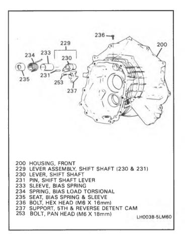
Figure 37 Removing Bias Spring Components
