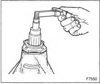
Figure 21—Measuring Pinion Bearing Preload
