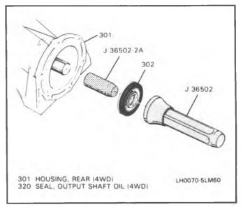
Figure 67 4WD Oil Seal Installation
