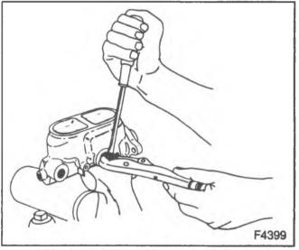
Figure 17-Removing the Tube Seats
