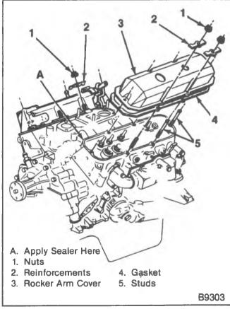
Figure 43—Rocker Arm Cover Installation
