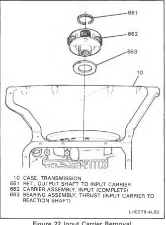
Figure 22 Input Carrier Removal
