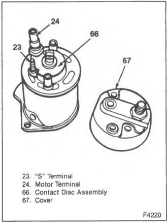
Figure 12-Solenoid Disassembled
