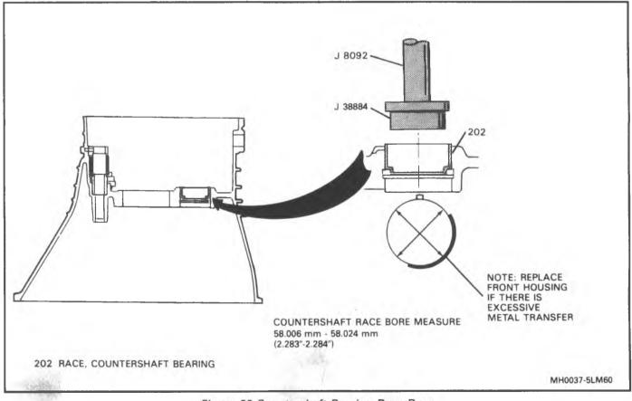
Figure 36 Countershaft Bearing Race Bore
