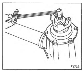
Figure 12—Checking Pinion Preload
