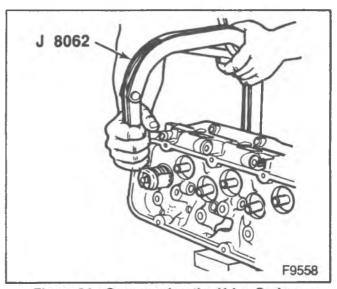
Figure 24-Compressing the Valve Springs
