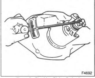
Figure 5-Checking Pinion Preload
