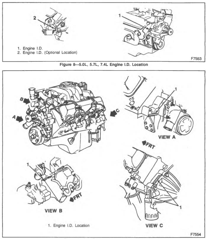
Figure 9-6.2L Diesel Engine I.D. Location
