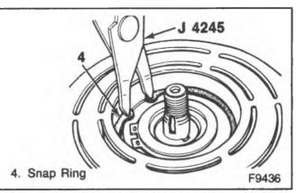
Figure 6-Removing the Internal Snap Ring
