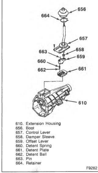
Figure 3—Shift Lever Components
