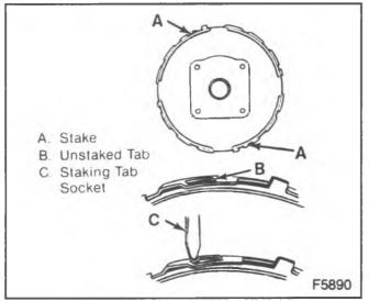
Figure 23-Staking the Tabs
