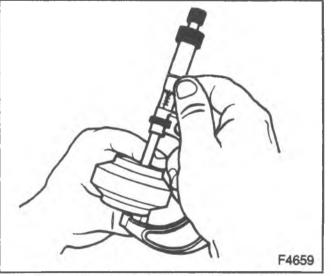
Figure 17—Measuring the Reaction Block
