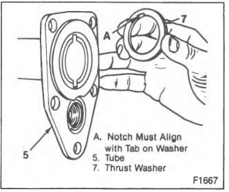
Figure 34-Installing the Thrust Washer
