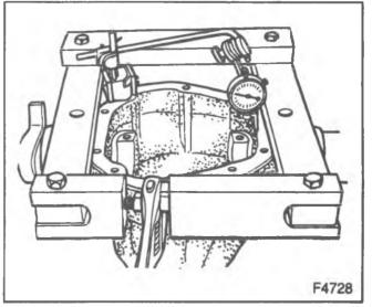
Figure 38—Mounting the Carrier Spreader
