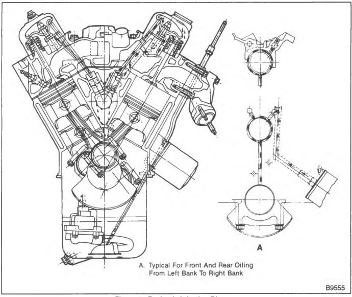
Figure 4---Engine Lubrication Diagram
