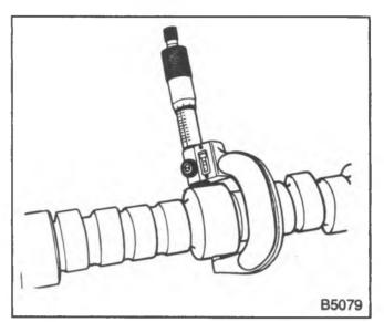
Figure 31—Checking the Camshaft Journals
