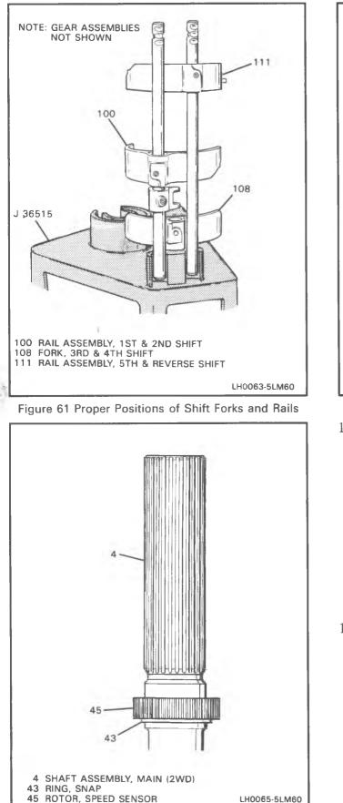
Figure 62 2WD Speed Sensor Rotor Installation
