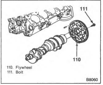
Figure 25—Flywheel (5.0L and 5.7L Engines)
