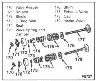
Figure 23—Valves and Components
