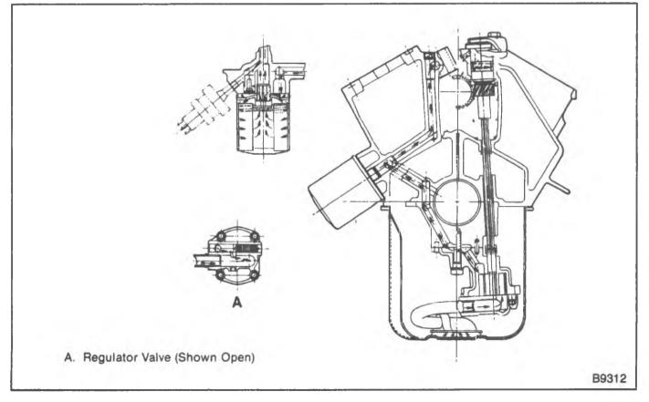
Figure 2—Engine Lubrication Diagram
