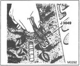
Figure 10—Removing the Hydraulic Lifters with J 3049
