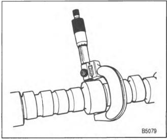
Figure 17-Checking the Camshaft Journals
