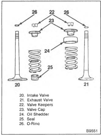
Figure 23—Valves and Components
