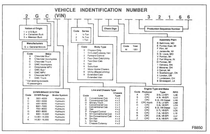
Figure 3—Vehicle Identification Number
