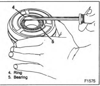
Figure 8—Removing the Pulley and Bearing Retainer Ring
