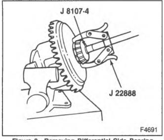
Figure 3—Removing Differential Side Bearing
