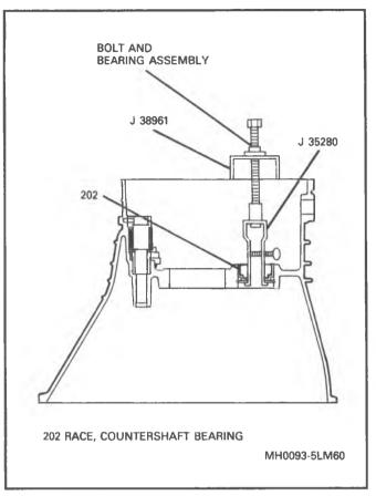
Figure 35 Removing Countershaft Bearing Race
