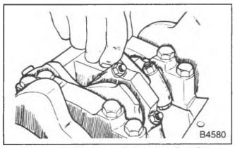
Figure 67—Measuring Connecting Rod Side Clearance
