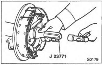
Figure 27-Installing the Axle Seal
