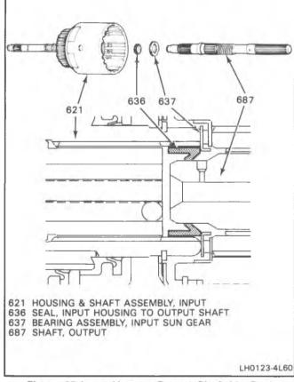
Figure 65 Input Hsg. to Output Shaft Lip Seal
