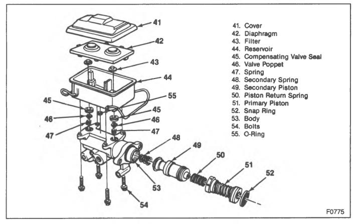
Figure 19—Bendix Master Cylinder Components
