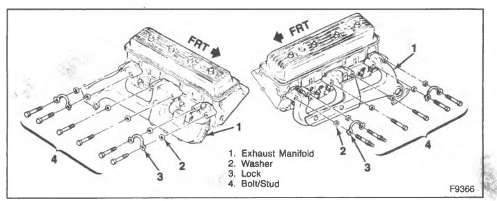
Figure 83—Exhaust Manifold (5.0L and 5.7L Engines)
