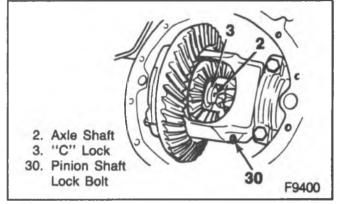
Figure 28—"C" Lock and Axle Shaft seated in the Side Gear
