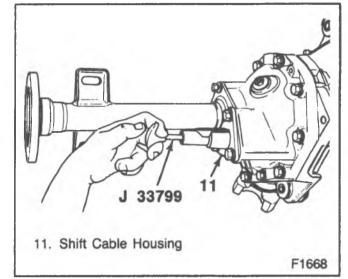
Figure 35—Checking the Shift Mechanism
