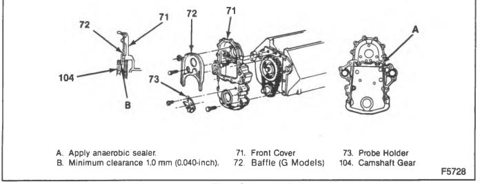
Figure 43—Front Cover Installation
