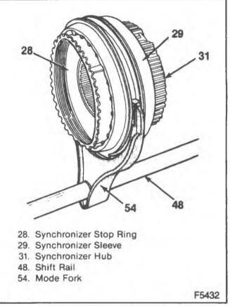
Figure 16—Synchronizer Hub Assembly and Mode Fork
