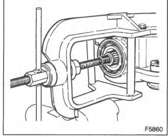
Figure 12—Removing the Pinion
