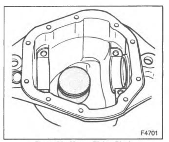
Figure 63—Master Pinion Block
