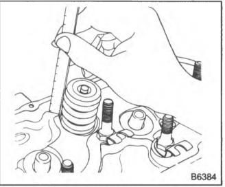
Figure 34-Measuring Valve Spring Installed height
