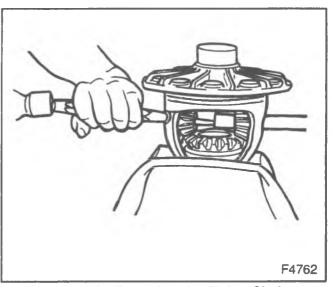
Figure 50—Removing the Pinion Shaft
