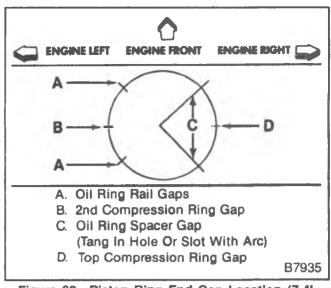
Figure 62—Piston Ring End Gap Location (7.4L Engines)
