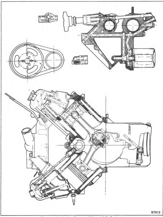
Figure 1—Lubrication Diagram (5.0L and 5.7L Engines)
