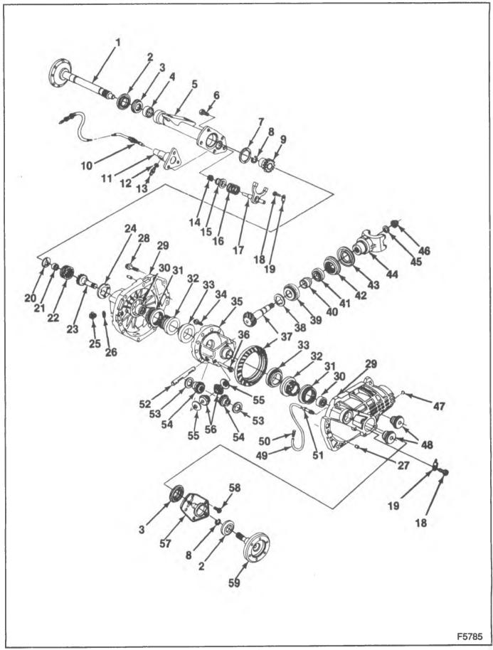
Figure 1—Axle Components
