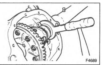
Figure 25—Installing the Differential Bearing Preload Shim
