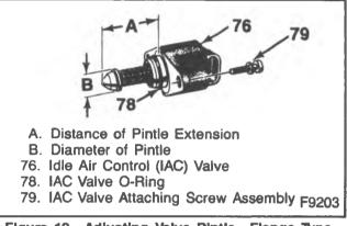
Figure 12—Adjusting Valve Pintle—Flange Type
