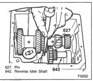
Figure 14—Removing the Reverse Idler Shaft Pin
