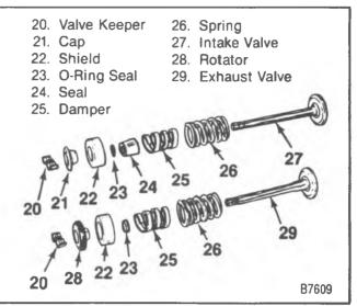
Figure 21-Valve and Components
