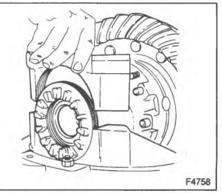
Figure 23-Installing the Bearing Cup
