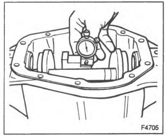
Figure 26—Scooter Gage on the Height Block
