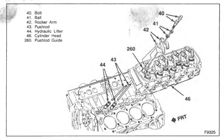
Figure 72—Cylinder Head and Components (7.4L Engines)
