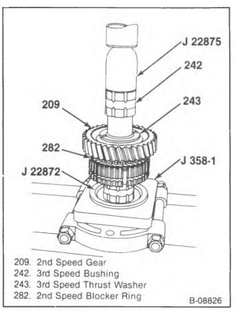
Figure 20 Installing the 3rd Speed Gear Bushing
