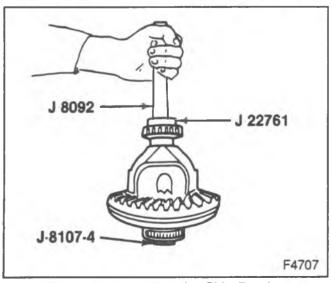
Figure 20-Installing the Side Bearing
