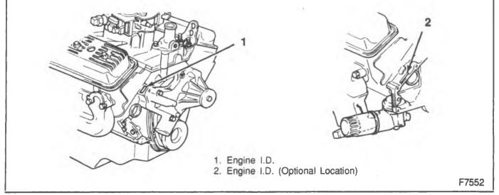
Figure 7-4.3L Engine I.D. Location
