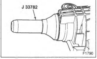
Figure 20—Installing the Pinion Seal
