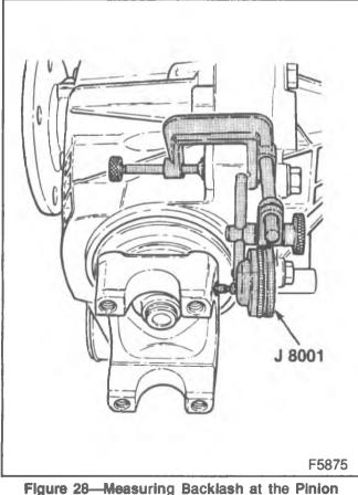
Figure 28—Measuring Backlash at the Pinion Flange
