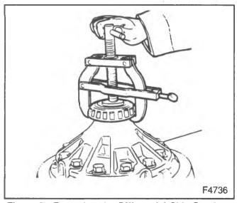
Figure 2—Removing the Differential Side Bearings
