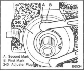
Figure 19—Aligning the Adjuster Hole with the Second Mark
