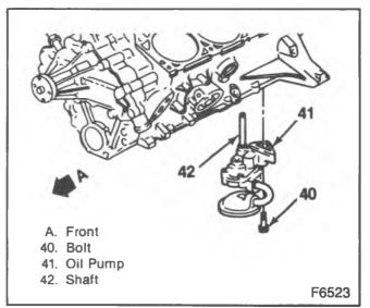
Figure 12—Oil Pump Removal
