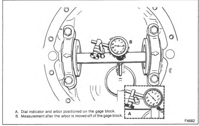
Figure 14—Checking Pinion Depth
