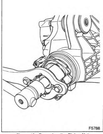
Figure 10-Removing the Pinion Nut
