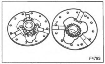
Figure 10-Differential Case Halves
