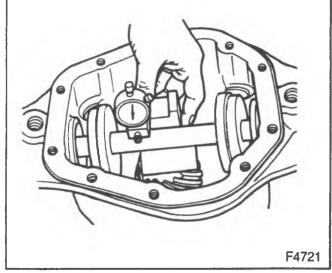
Figure 73---Checking the Pinion Depth Setting
