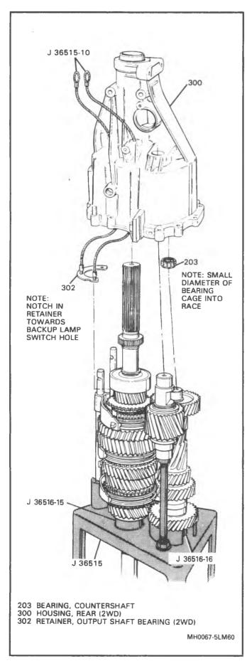
Figure 64 2WD Rear Housing Installation
