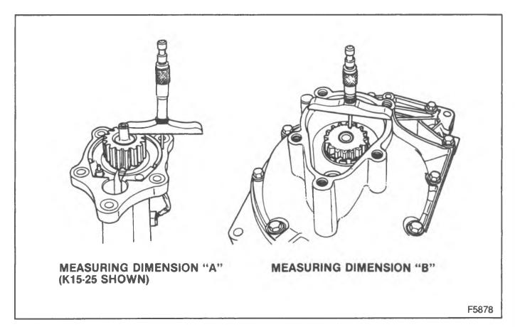
Figure 37—Measuring to Calculate Shim Size
