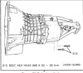
Figure 78 Bolts Installation
