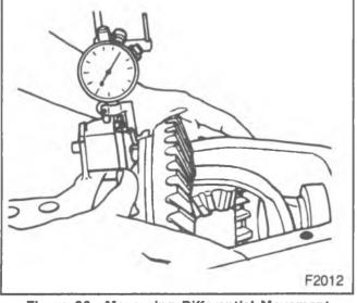
Figure 36-Measuring Differential Movement
