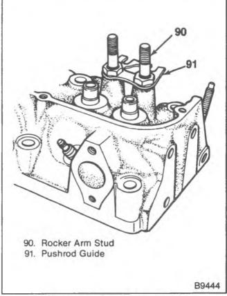
Figure 25—Rocker Arm Studs
