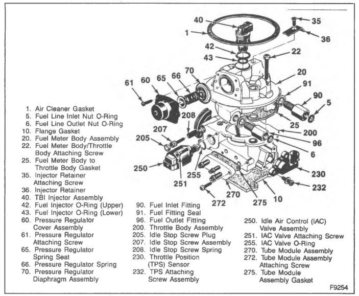
Figure 2—Model 700 TBI Parts Identification
