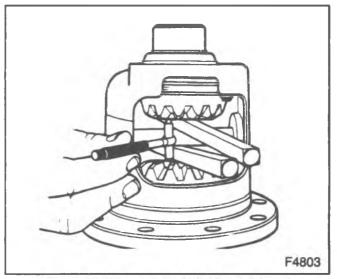
Figure 6—Measuring Side Gear Spread
