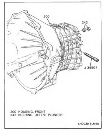
Figure 38 Removing Detent Plunger Bushings
