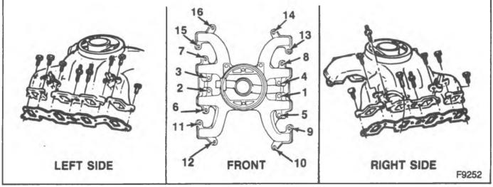
Figure 58-Intake Manifold Installation
