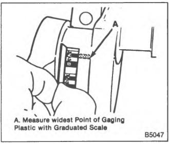
Figure 38—Measuring the Gaging Plastic
