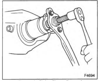
Figure 13—Pinion Flange Removal
