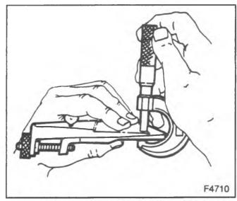
Figure 20—Measuring the Gage Plate Thickness
