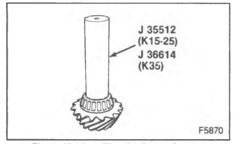
Figure 22-Installing the Pinion Bearing
