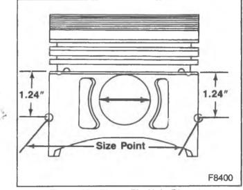
Figure 63-Piston Pin Hole Diameter
