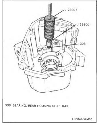
Figure 48 Removing Shift Rail Bushing
