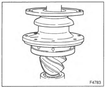
Figure 16-Installing the Pinion Flange
