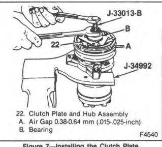
Figure 7—Installing the Clutch Plate and Hub Assembly
