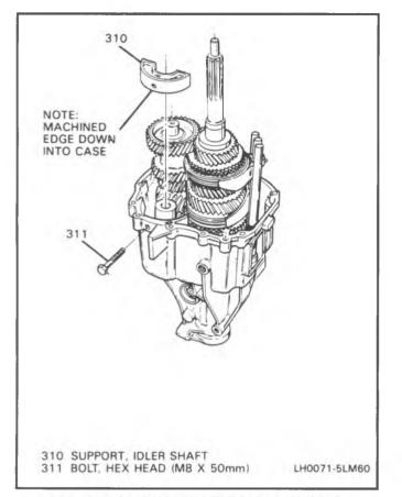
Figure 68 Reverse Idler Support Installation
