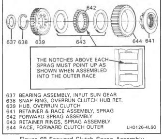
Figure 68 Forward Clutch Sprag Assembly
