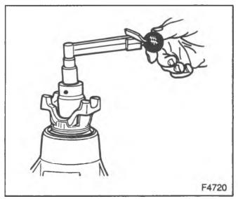
Figure 72—Checking the Pinion Preload
