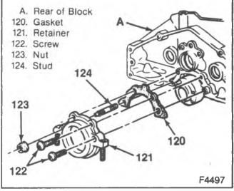
Figure 26—Rear Crankshaft Oil Seal Retainer (5.0L and 5.7L Engines)
