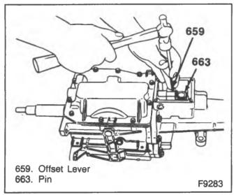
Figure 4—Removing the Offset Lever Pin
