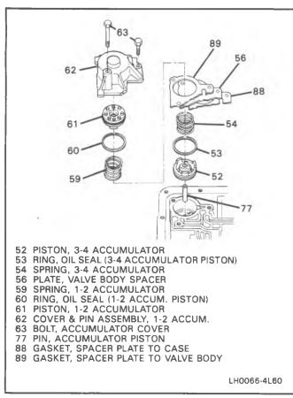
Figure 10 Accumulator Assembly
