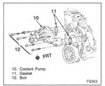
Figure 85-Coolant Pump (5.0L and 5.7L Engines)
