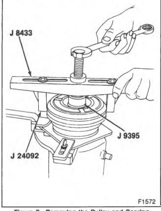
Figure 7—Removing the Pulley and Bearing
