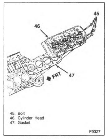
Figure 11—Cylinder Head (7.4L Engines)
