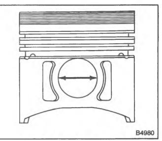
Figure 9—Piston Pin Hole Diameter
