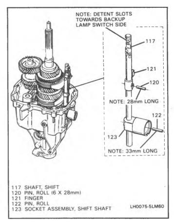
Figure 72 Shift Shaft Installation
