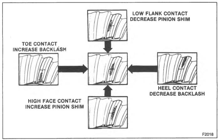
Figure 28-Gear Tooth Contact Pattern
