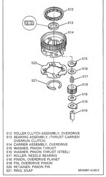
Figure 74 Overdrive Carrier Assembly
