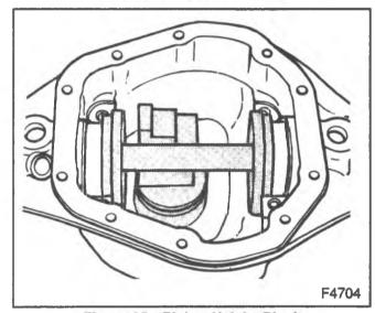
Figure 25—Pinion Height Block
