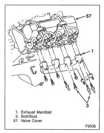
Figure 7-Exhaust Manifold Left Side
