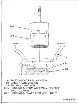
Figure 90 Installing Input Clutch
