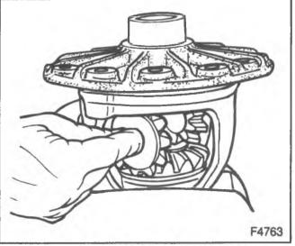
Figure 58—Installing the Pinion Gears
