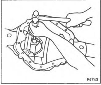
Figure 9-Removing the Pilot Bearing
