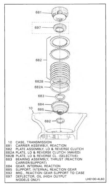
Figure 44 Reaction Internal Gear and Carrier Assembly Installation
