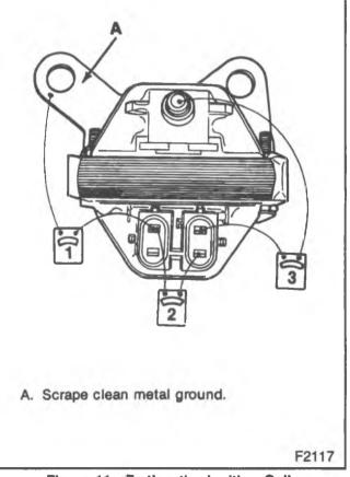
Figure 11—Testing the Ignition Coll
