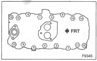
Figure 80—Intake Manifold Tightening Sequence (7.4L Engines)
