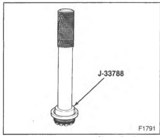
Figure 22—installing the Sleeve Bearing
