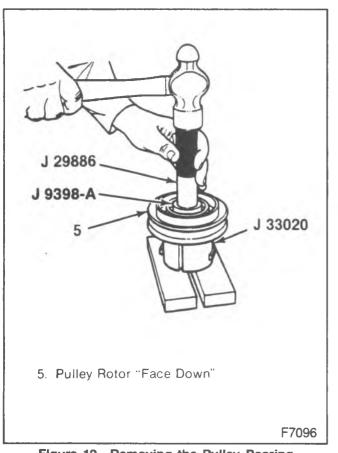
Figure 12—Removing the Pulley Bearing
