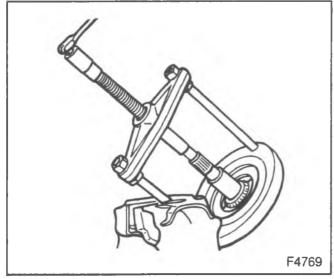
Figure 16—Removing the Pinion Inner Bearing
