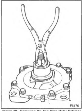
Figure 10-Removing the Felt Ring Metal Retainer
