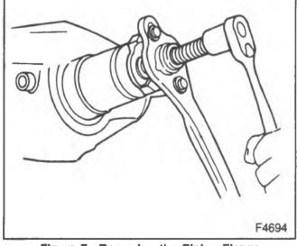
Figure 7—Removing the Pinion Flange
