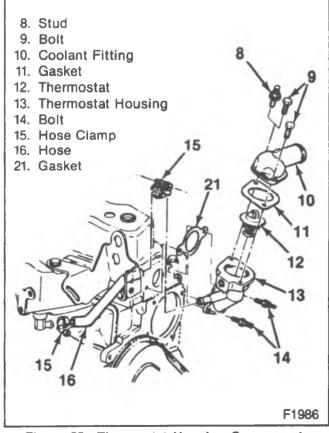
Figure 55—Thermostat Housing Components
