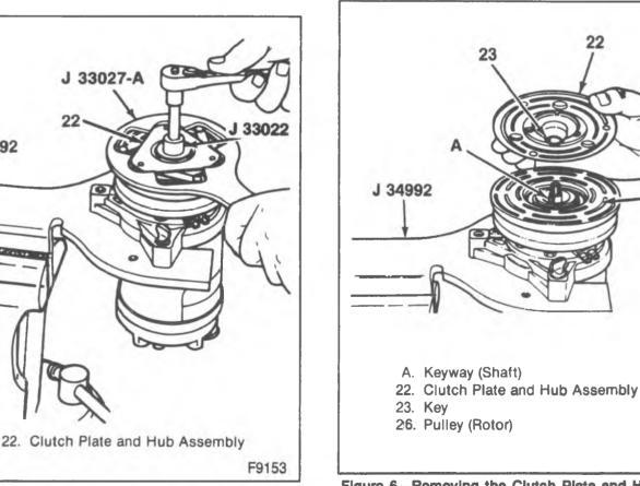
Figure 4-Removing the Shaft Nut
