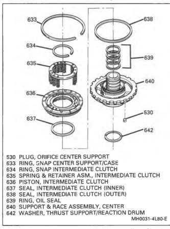
Figure 34 Center Support and Intermediate Clutch Piston
