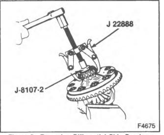
Figure 8—Removing Differential Side Bearings
