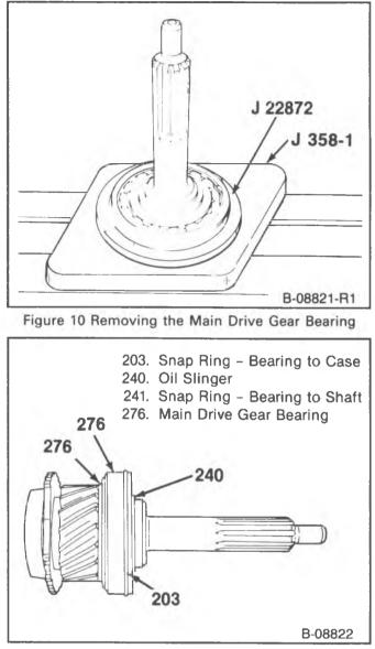
Figure 11 Main Drive Gear Assembly
