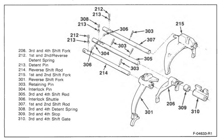
Figure 36 C/K Shift Rod and Fork Positions
