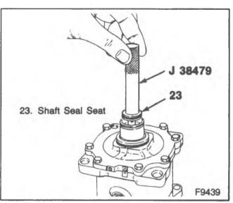
Figure 11-Removing the Shaft Seal Seat
