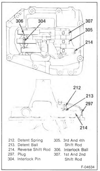
Figure 37 R/V/P Interlock Shuttles and Pin
