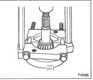
Figure 11---Removing the Pinion Bearing
