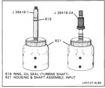
Figure 79 Turbine Shaft Oil Seal Rings
