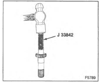
Figure 33-Installing the Differential Pilot Bearing
