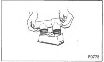
Figure 13-Installing The Reservoir
