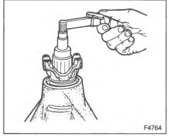
Figure 24—Measuring Pinion Bearing Preload
