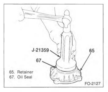
Figure 18—Installing the Rear Bearing Retainer Seal
