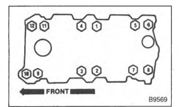
Figure 78—Intake Manifold Bolt Tightening Sequence (5.0L and 5.7L Engines)
