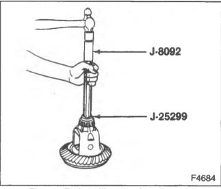
Figure 17-Installing the Side Bearing
