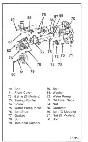
Figure 11—Front Cover and Components
