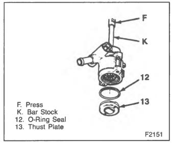
Figure 33—Removing the Thrust Plate
