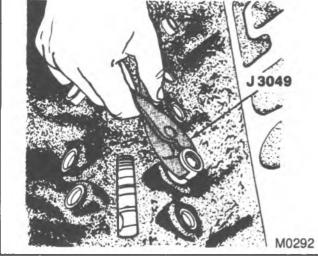
Figure 14-Removing the Hydraulic Lifter
