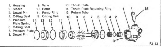
Figure 34—Pump Housing Components
