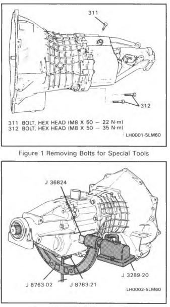
Figure 2 Holding Fixture Installed
