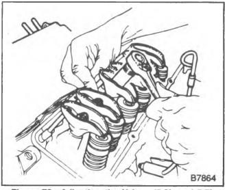
Figure 76—Adjusting the Valves (5.0L and 5.7L Engines)
