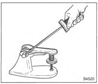
Figure 33-Measuring Valve Spring Tension
