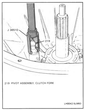
Figure 41 Clutch Fork Pivot Assembly Installation
