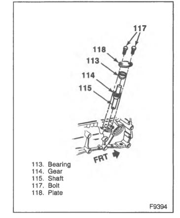
Figure 50—Oil Pump Drive Shaft
