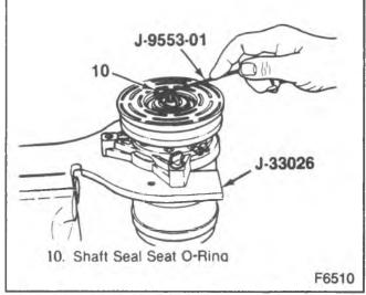
Figure 24-Removing the Shaft Seal Seat O-Ring
