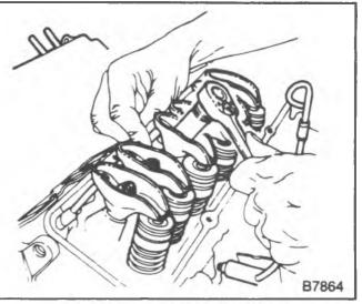
Figure 41-Adjusting the Valves
