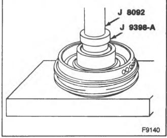
Figure 9—Removing the Bearing from the Pulley
