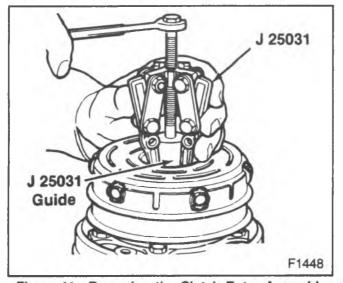
Figure 11-Removing the Clutch Rotor Assembly
