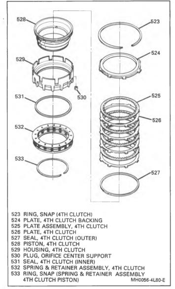
Figure 63 Fourth Clutch Assembly
