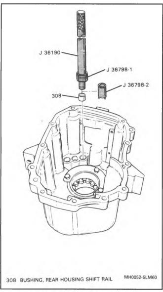
Figure 52 Shift Rail Bushings Installation
