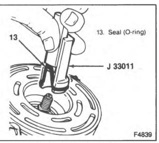
Figure 24-Installing the Seal
