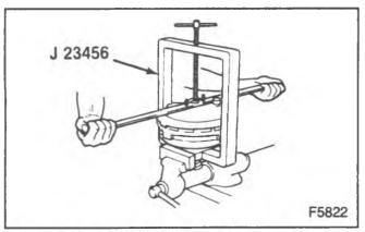
Figure 21-Unlocking and Locking the Booster
