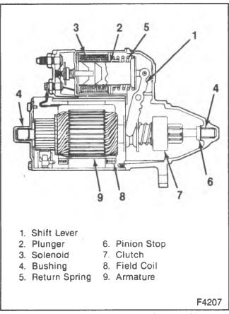
Figure 1-SD-200 and SD-260 Starting Motor
