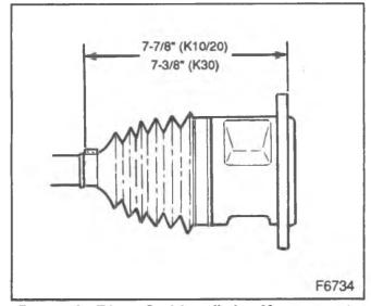
Figure 53—Tri-pot Seal Installation Measurements
