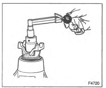
Figure 31-Checking the Pinion Preload
