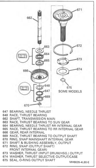
Figure 38 Assembling Output Shaft and Rear Internal Gear
