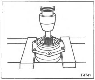
Figure 7—Pressing the Drive Pinion from the Cage
