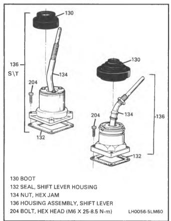
Figure 56 Shift Housing Assembly Components
