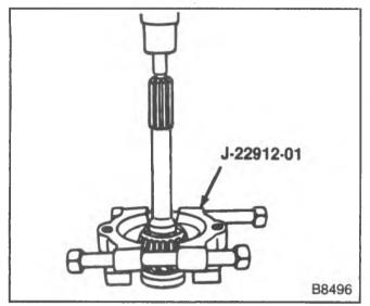
Figure 17-Removing the Main Drive Gear Bearing
