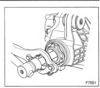
Figure 9—Removing the Pinion Nut
