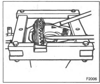
Figure 5-Removing the Differential
