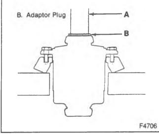
Figure 20-Installing the Ring Gear to the Case
