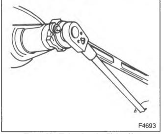
Figure 35—Tightening the Pinion Nut
