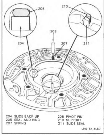
Figure 96 Slide Back Up and Slide Seal
