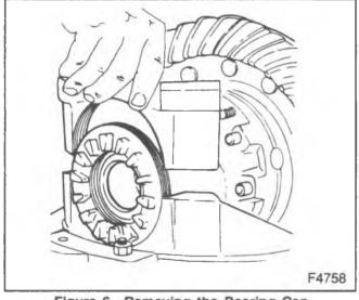
Figure 6—Removing the Bearing Cap
