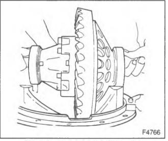
Figure 7—Removing the Differential
