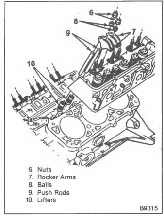
Figure 9—Valve Train Components
