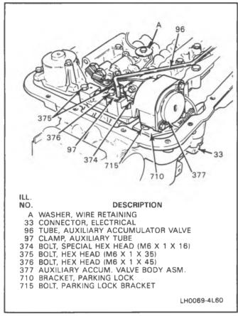
Figure 13 Removing Auxiliary Valve Body Assembly
