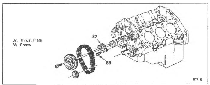
Figure 31—Camshaft and Components
