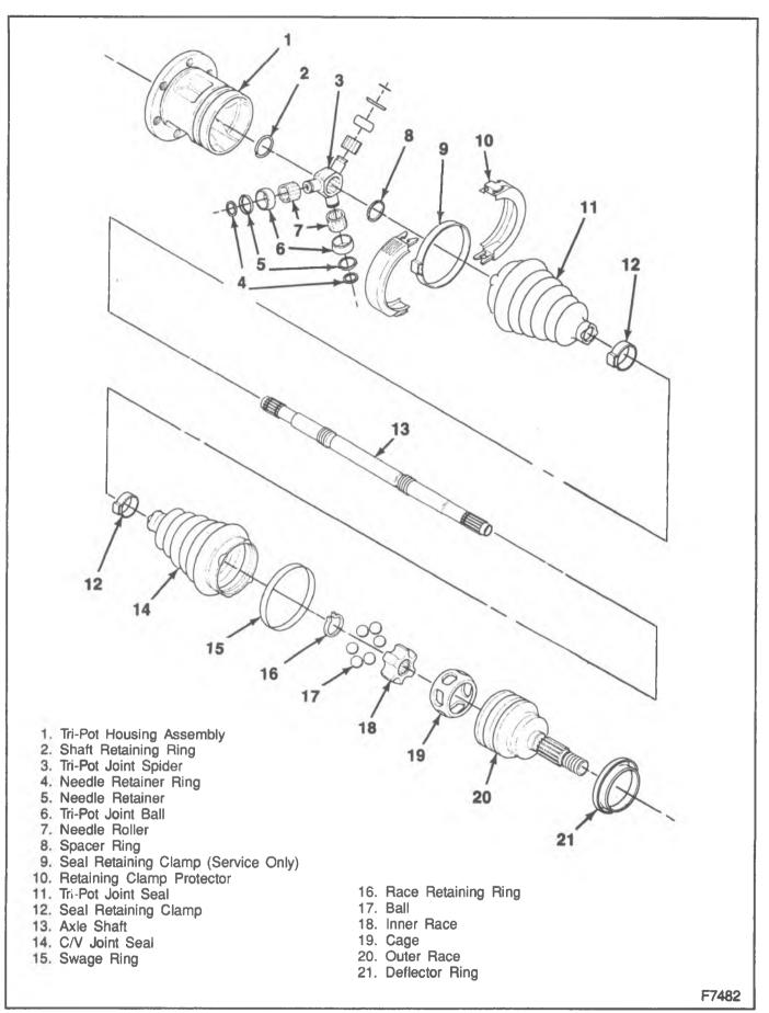
Figure 36—Front Drive Axle
