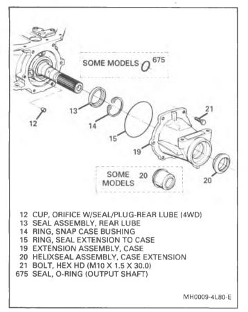
Figure 9 Removing Case Extension Assembly
