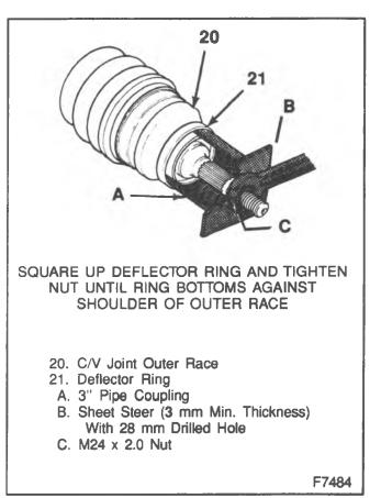
Figure 32-Installing Outer Deflector Ring
