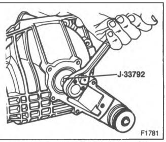
Figure 8—Removing the Side Bearing Cup
