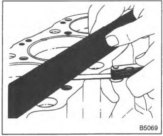
Figure 28-Checking the Block Gasket Surface
