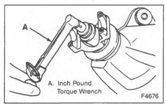
Figure 9—Checking Pinion Preload
