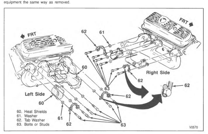
Figure 45—Exhaust Manifold Installation
