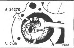
Figure 10—Removing the Cylinder Ridge
