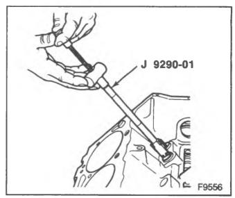
Figure 15—Removing the Hydraulic Lifter
