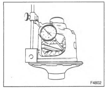
Figure 5-Checking Cam Gear Backlash
