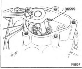
Figure 27—Turning the Adjuster Sleeve
