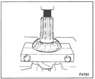
Figure 14-Removing the Pinion Inner Bearing
