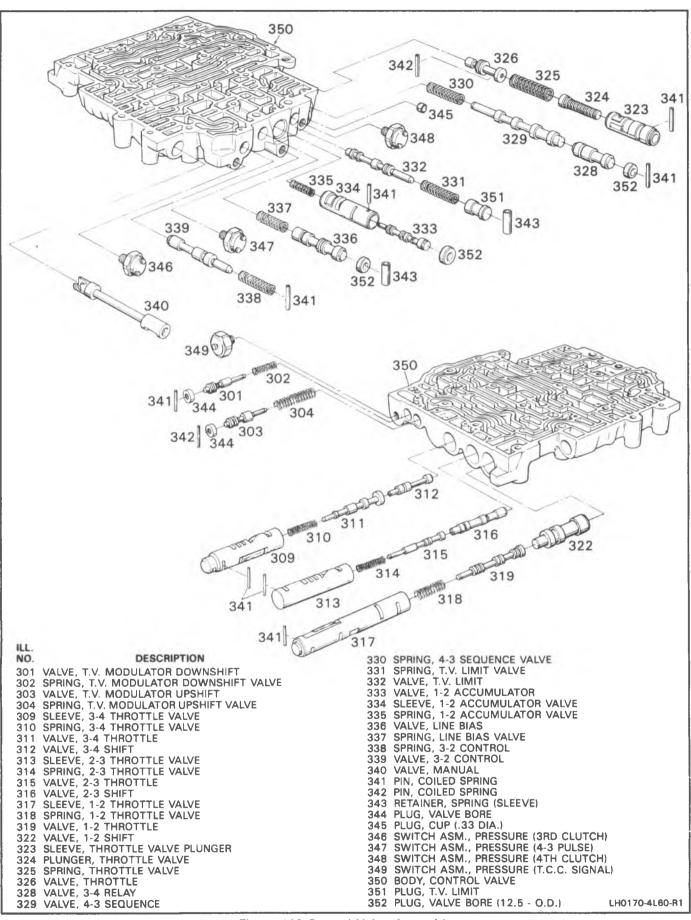
Figure 112 Control Valve Assembly
