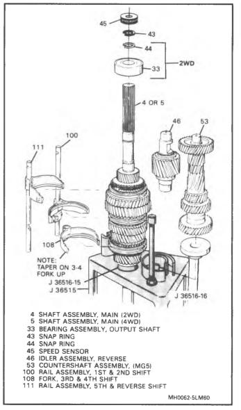
Figure 60 Countershaft and Reverse Idler Assembly Installation
