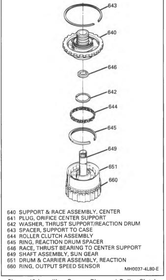
Figure 40 Installing Spacer Ring and Roller Clutch Assembly
