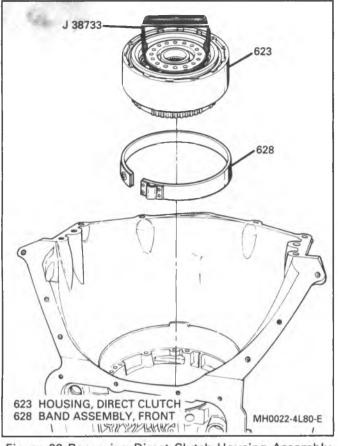
Figure 22 Removing Direct Clutch Housing Assembly
