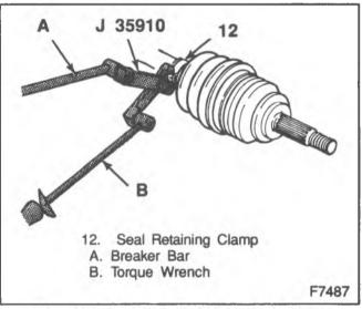
Figure 35-Installing Seal Retaining Clamp
