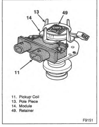
Figure 4—Distributor with Sealed Module Connector
