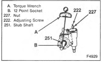
Figure 22—Aligning the Over-Center Preload
