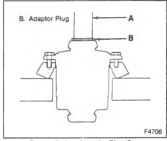
Figure 17-Installing the Ring Gear
