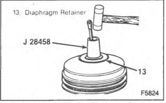
Figure 22—Installing the Diaphragm Retainer
