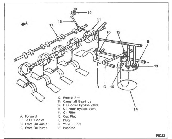
Figure 1—Lubrication Diagram
