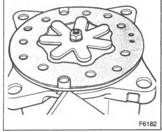
Figure 15—Loosening the Valve Plate
