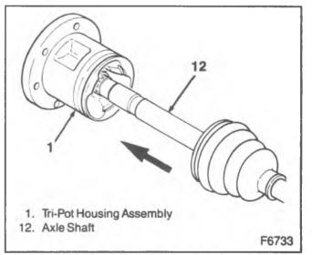
Figure 52—Installing Tri-pot to Housing
