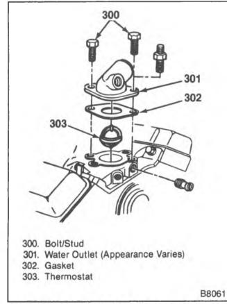
Figure 47—Thermostat and Components (5.0L and 5.7L Engines)
