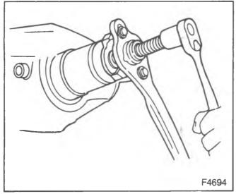
Figure 7—Removing the Pinion Flange
