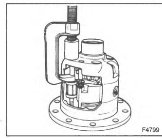
Figure 2-Removing the Governor Bushings
