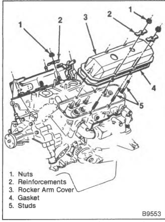
Figure 8-Rocker Arm Cover Removal
