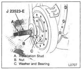
Figure 60---Installing the Torsional Damper
