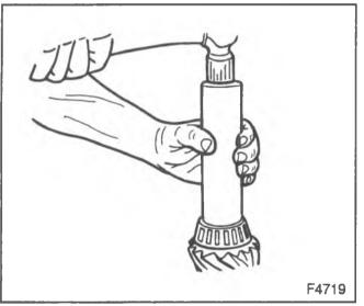
Figure 31-Installing the Inner Bearing
