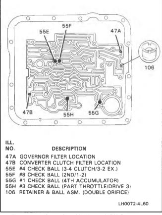
Figure 111 Case Checkballs and Oil Screens — Location
