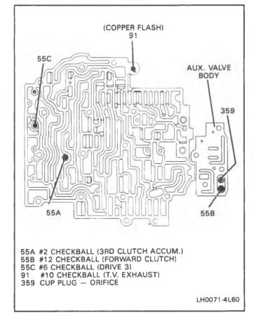
Figure 15 Valve Body Checkballs
