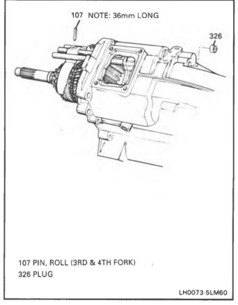
Figure 70 3-4 Fork Roll Pin and Plug Installation
