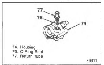
Figure 48---Threaded Return Removal and installation-Model N
