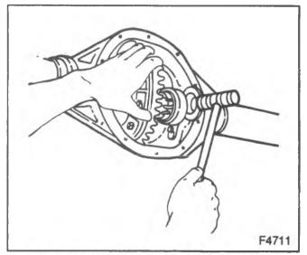
Figure 22-Installing the Final Preload Shim
