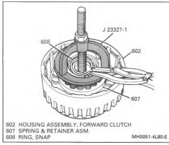
Figure 56 Removing Forward Clutch Piston Release Springs
