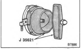
Figure 56—Installing the Rear Crankshaft Oil Seal (5.0L and 5.7L Engines)
