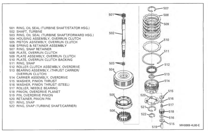
Figure 76 Overdrive/Overrun Clutch Assembly
