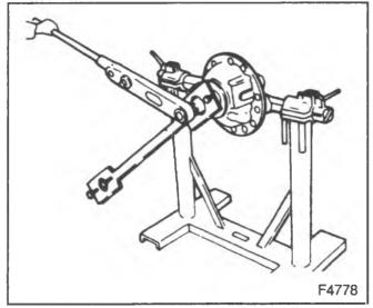
Figure 11—Removing the Pinion Nut
