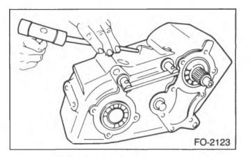
Figure 14—Installing the Shift Fork Roll Pin
