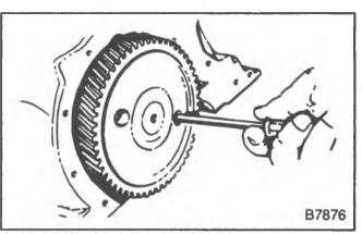
Figure 18—Removing the Camshaft Thrust Plate Bolts
