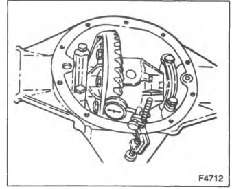
Figure 23-Checking Ring Gear Backlash
