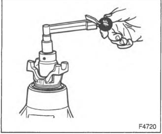
Figure 32-Checking the Pinion Preload
