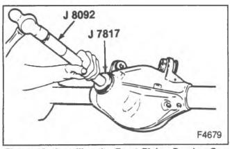
Figure 12-Installing the Front Pinion Bearing Cup
