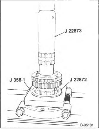
Figure 19 Installing the 1st Speed Gear Bushing
