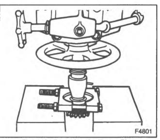
Figure 4—Removing the Thrust Ring
