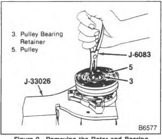
Figure 9—Removing the Rotor and Bearing Retaining Ring
