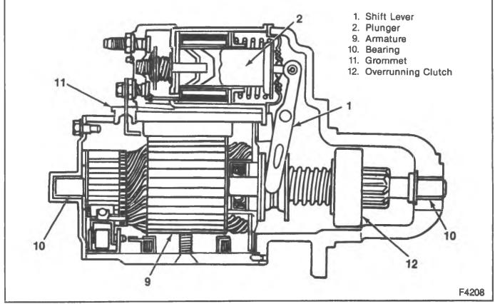
Figure 2---SD-300 Starting Motor
