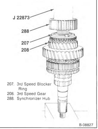
Figure 21 Installing the 3rd and 4th Speed Synchronizer Hub
