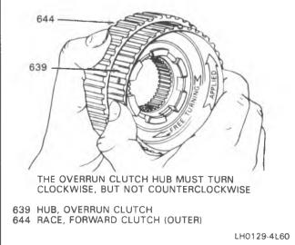
Figure 71 Sprag Operation Check
