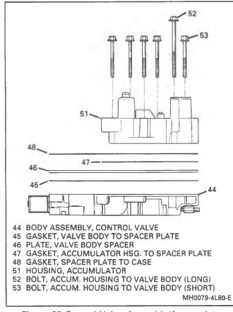
Figure 93 Control Valve Assembly/Accumulator Housing
