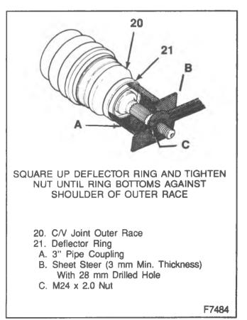
Figure 38-Installing Outer Deflector Ring
