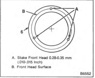
Figure 20-Staking Locations on the Front Head
