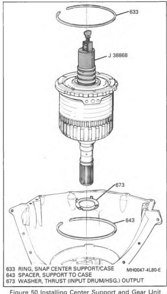
Figure 50 Installing Center Support and Gear Unit Assembly
