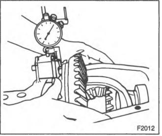
Figure 62-Determining Differential Shim Pack
