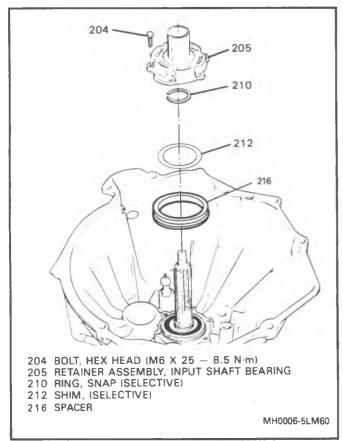
Figure 76 Install Input Shaft Bearing Retainer Assembly
