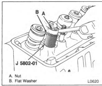
Figure 41—Removing the Rocker Arm Stud (5.0L and 5.7L Engines)
