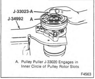
Figure 9—Installing the Pulley Rotor and Bearing Puller Guide
