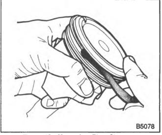
Figure 18—Measuring Ring Clearance
