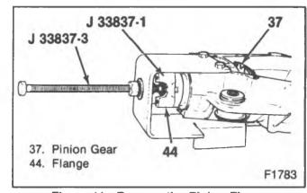
Figure 11-Remove the Pinion Flange
