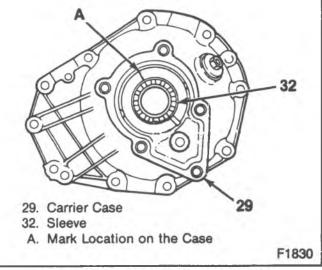
Figure 26-Marking Sleeve Location
