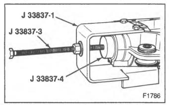
Figure 16-Installing the Outer Pinion Bearing Cup
