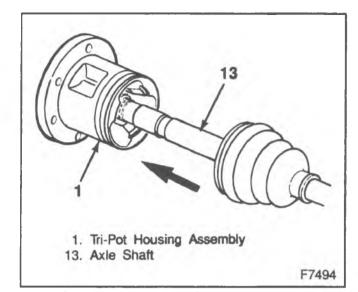
Figure 42-Installing Tri-pot to Housing
