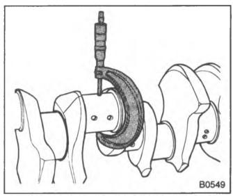
Figure 30-Measuring the Crankshaft Journals
