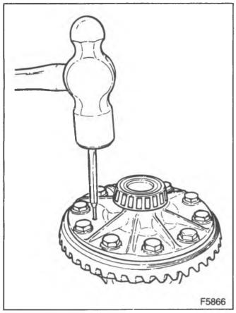
Figure 17-Removing the Pin (K1, 2 Models)
