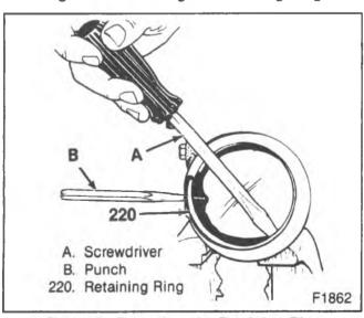
Figure 3—Removing the Retaining Ring
