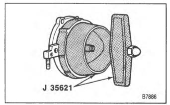
Figure 30—Installing the Rear Crankshaft Oil Seal
