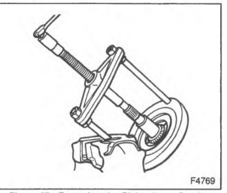
Figure 57—Removing the Pinion Inner Bearing
