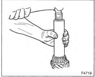
Figure 30-Installing the Inner Bearing
