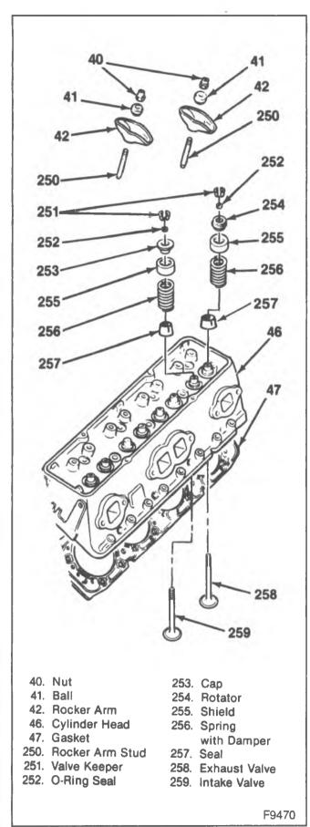
Figure 38—Cylinder Head and Components (5.0L and 5.7L Engines)
