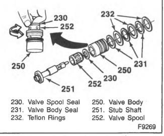
Figure 12—Removing or Installing Valve Spool Assembly
