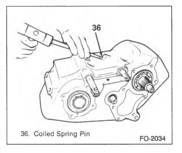
Figure 6—Removing the Shift Fork Roll Pin
