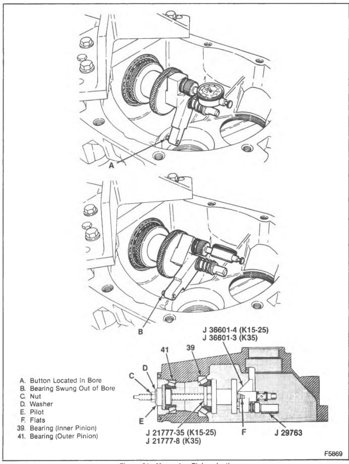
Figure 21—Measuring Pinion depth
