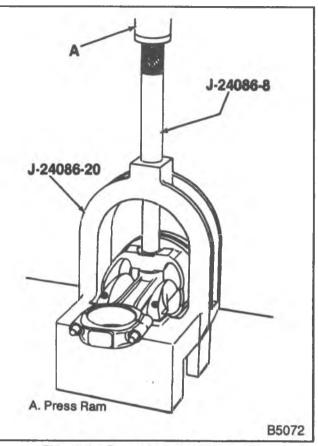
Figure 6-Removing the Piston Pin
