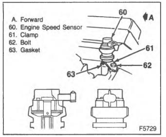
Figure 59—Oil Pump Drive Installed
