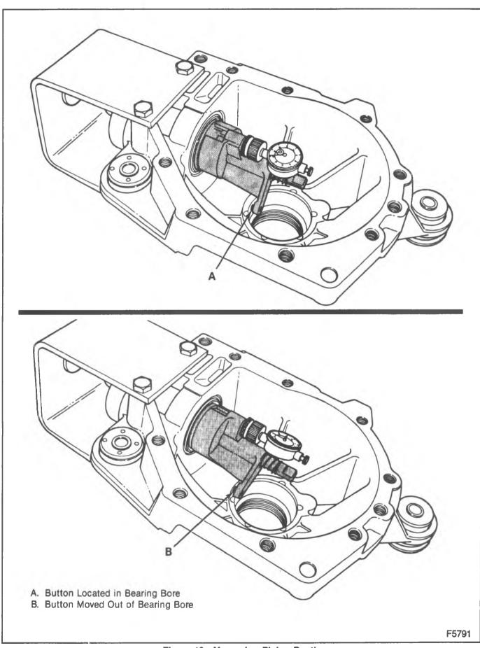
Figure 19-Measuring Pinion Depth
