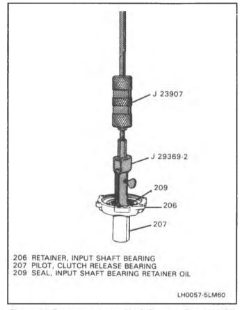
Figure 57 Removing Input Shaft Bearing Retainer Oil Seal
