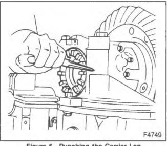
Figure 5—Punching the Carrier Leg
