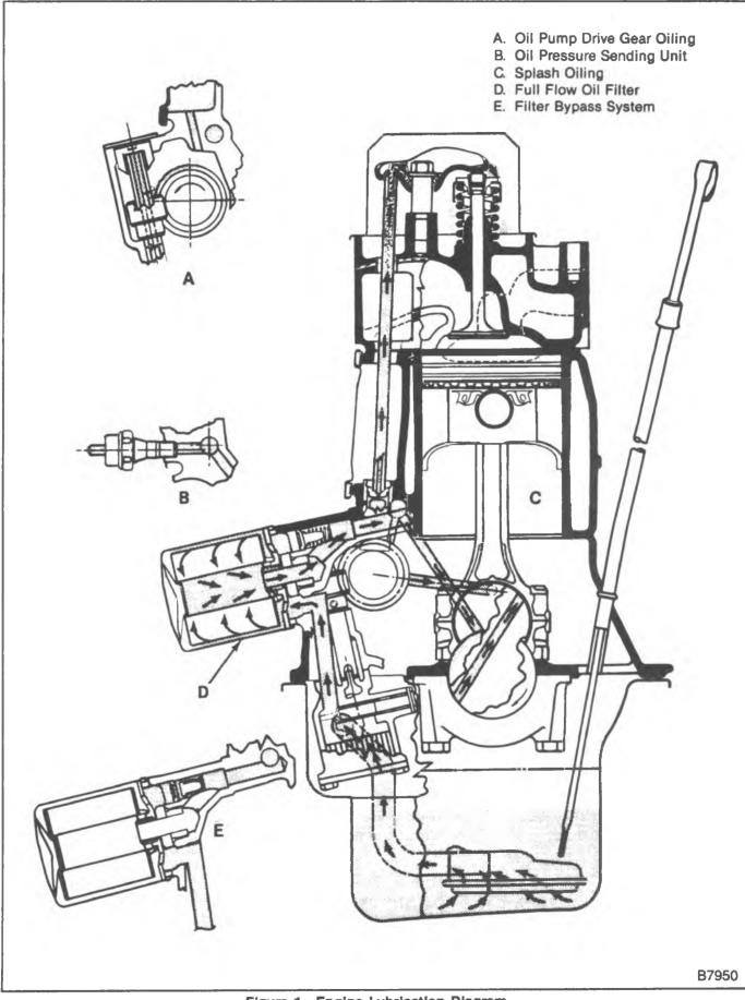
Figure 1—Engine Lubrication Diagram
