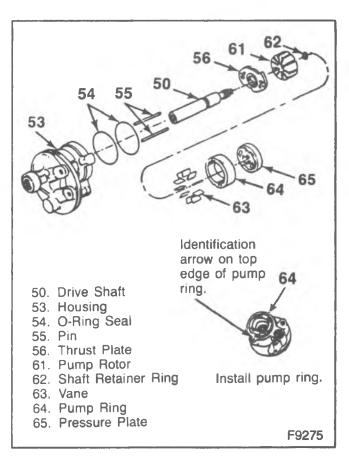
Figure 46—Rotating Group Removal and Installation
