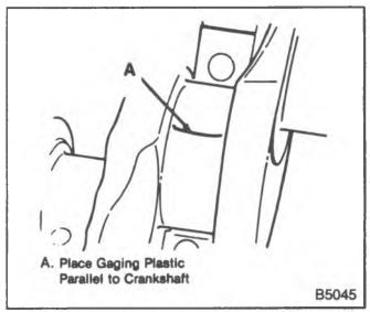
Figure 37—Placing the Gaging Plastic on the Bearing Journal
