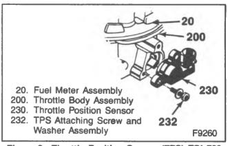
Figure 8-Throttle Position Sensor (TPS) TBI 700
