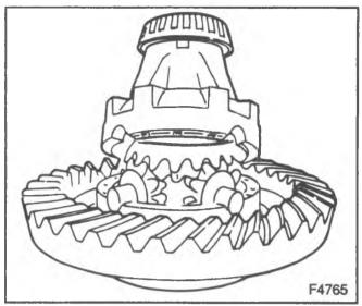
Figure 21-Installing the Case Halves
