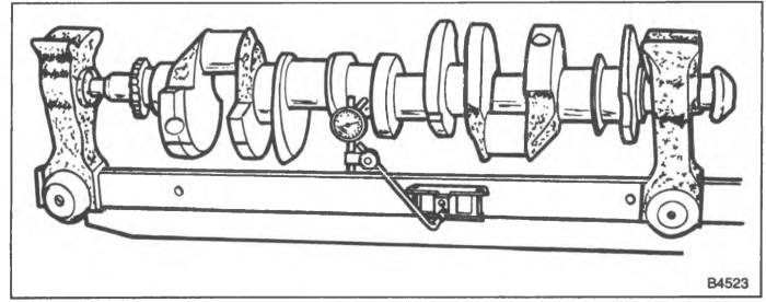
Figure 31—Checking the Crankshaft Run-Out
