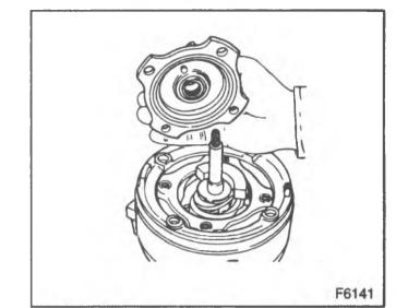
Figure 27—Removing the Front Head Assembly
