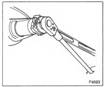
Figure 34-Tightening the Pinion Nut
