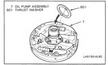
Figure 92 Oil Pump Thrust Washer Location
