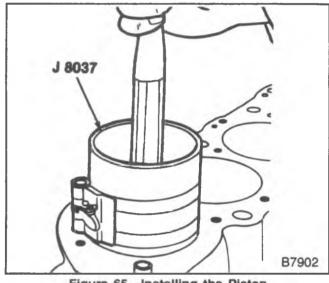
Figure 65—Installing the Piston
