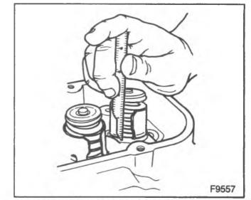
Figure 46—Measuring Valve Spring Installed Height (7.4L Engine)
