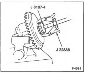
Figure 4-Removing Differential Side Bearing
