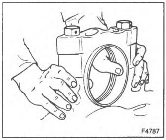
Figure 18—Removing the Pinion Nut
