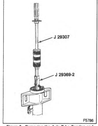
Figure 3—Removing the Axle Tube Bearing and Seal
