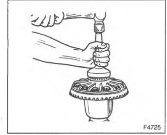
Figure 38-Installing the Differential Bearings
