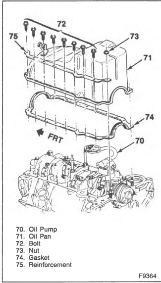
Figure 17-Oil Pan (5.0L and 5.7L Engines)
