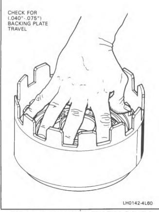
Figure 84 Reverse Input Backing Plate Selection
