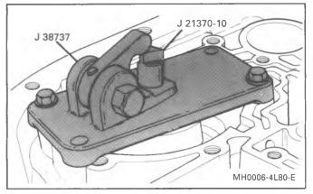
Figure 6 Installing Servo Pin Gage
