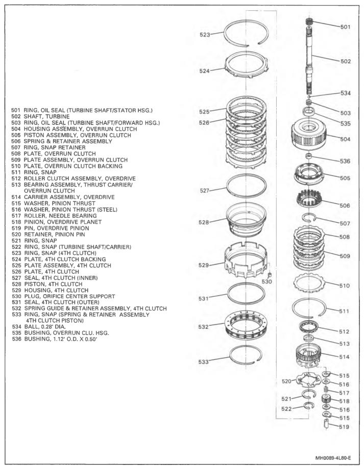
Figure 109 Overrun, Overdrive and 4th Clutch Assembly
