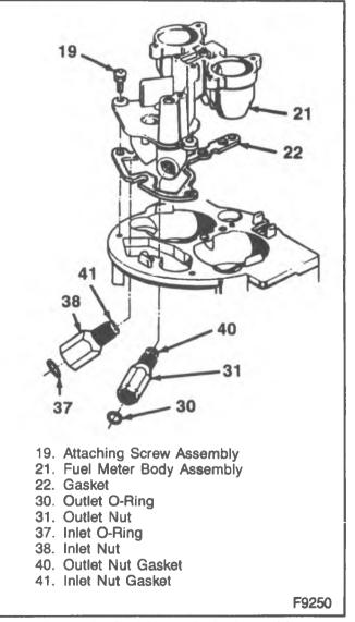
Figure 9—Fuel Meter Body Assembly
