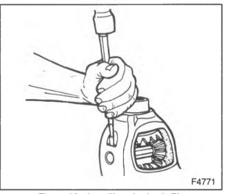
Figure 59-Installing the Lock Pin
