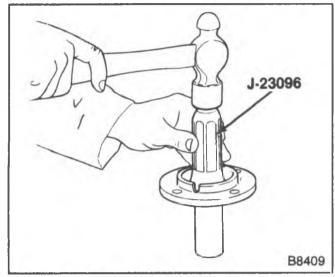
Figure 29-Installing the Bearing Retainer Oil Seal
