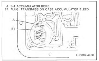
Figure 31 Third Accumulator Bore
