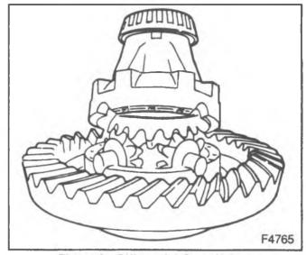
Figure 8-Differential Case Halves
