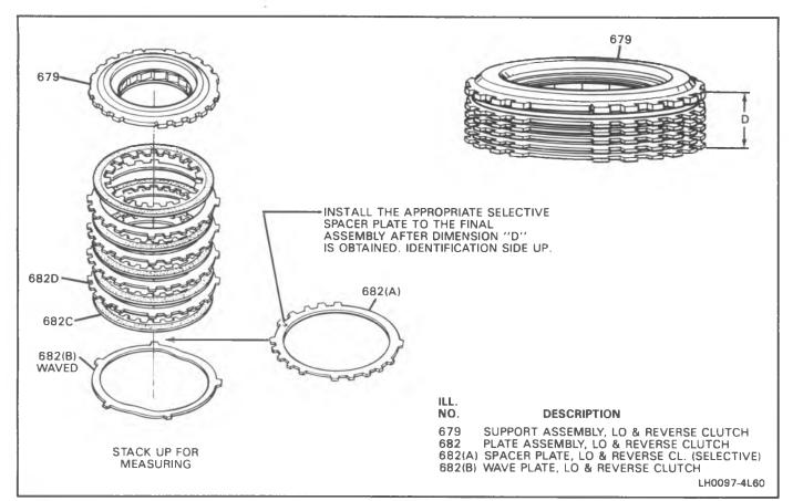
Figure 40 Measuring For Spacer Plate Selection
