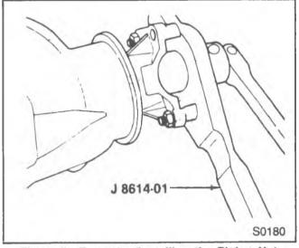
Figure 5-Removing/Installing the Pinion Nut.
