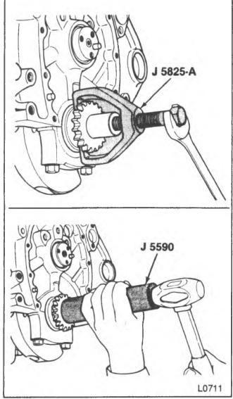
Figure 32—Crankshaft Sprocket Replacement (5.0L and 5.7L Engines)
