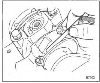
Figure 38—Measuring Connecting Rod Side Clearance
