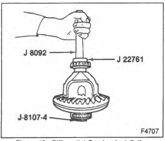
Figure 18—Differential Bearing Installation
