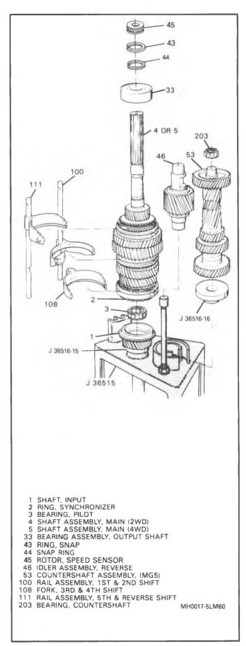
Figure 16 Removing Gears and Shift Rails
