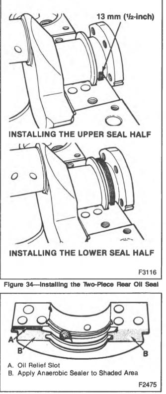
Figure 35—Applying Sealant to the Main Bearing Cap
