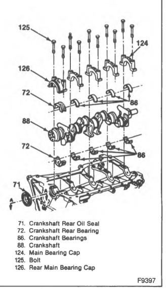
Figure 37-Crankshaft and Bearing Components
