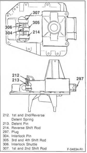
Figure 38 C/K Interlock Shuttles and Pin
