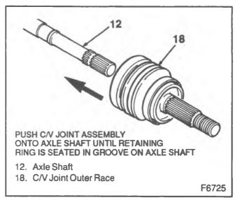
Figure 44—installing C/V Joint
