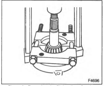
Figure 9—Removing the Pinion Rear Bearing
