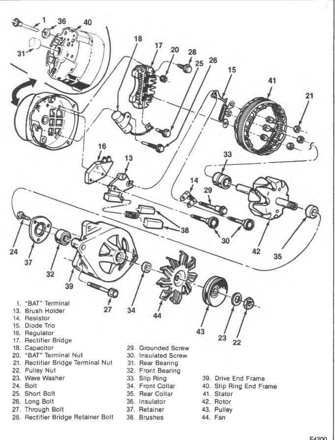
Figure 9-17-SI Series 100 Components
