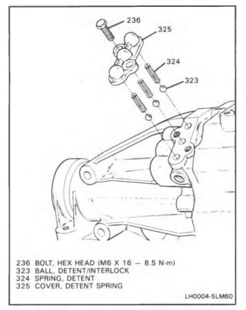
Figure 4 Removing Shift Rail Detent System
