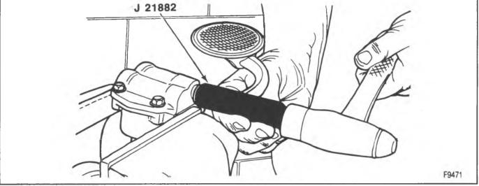
Figure 20-Installing the Oil Pump Screen
