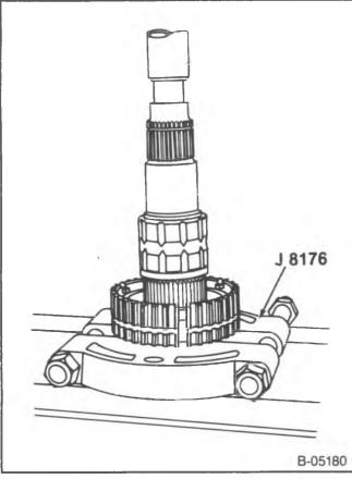
Figure 18 Installing the 1st and 2nd Synchronizer
