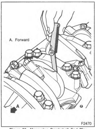
Figure 36—Measuring Crankshaft End Play
