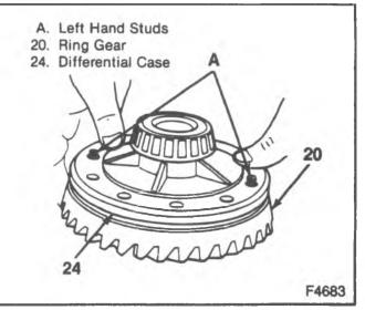
Figure 18—Aligning the Ring Gear Studs
