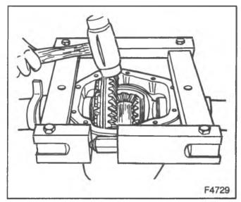
Figure 40-Installing the Differential Case
