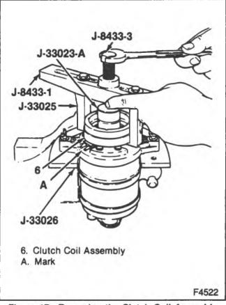
Figure 17—Removing the Clutch Coll Assembly
