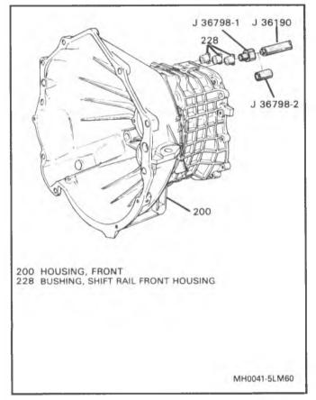
Figure 40 Shift Rail Bushings Installation
