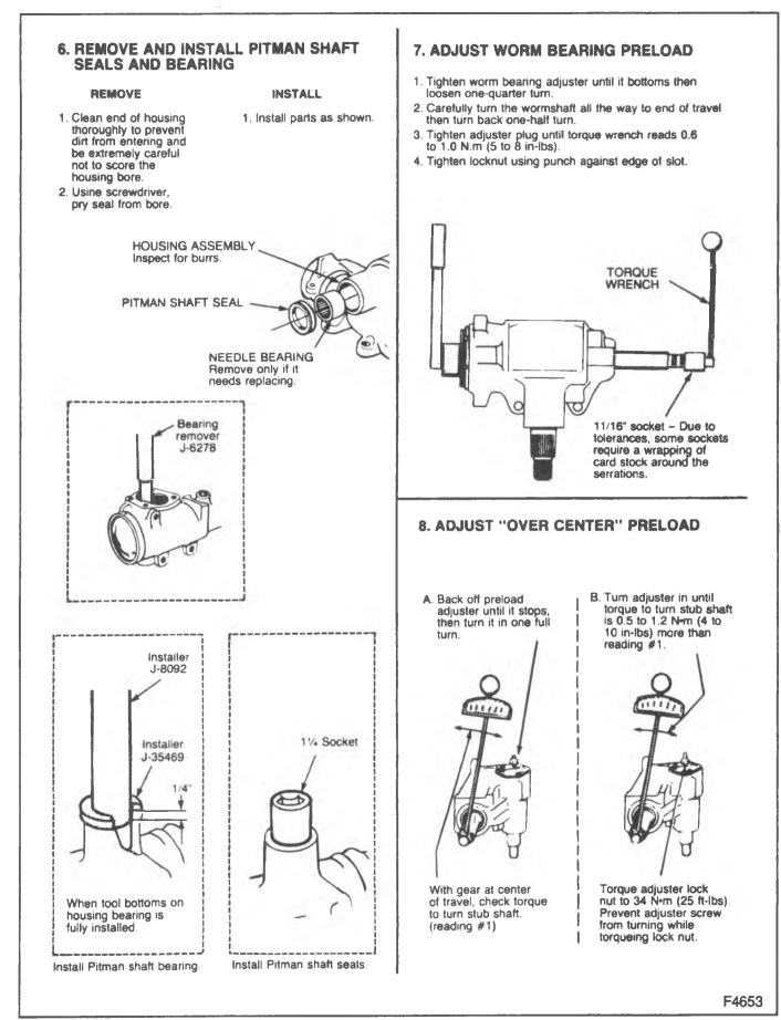
Figure 4-Model 535-Chart C-Adjustment
