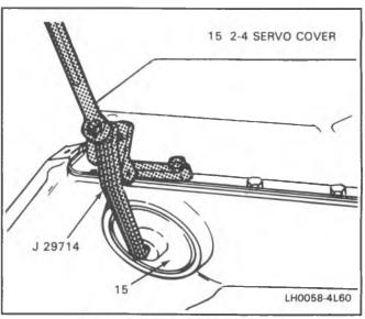
Figure 2 Servo Cover Removal
