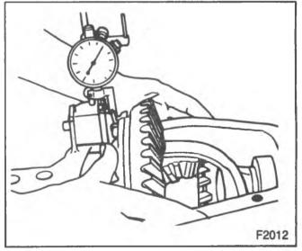
Figure 37-Measuring Differential Movement
