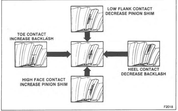
Figure 27—Gear Tooth Pattern
