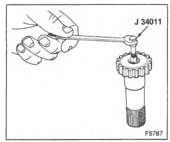
Figure 6-Removing the Pilot Bearing
