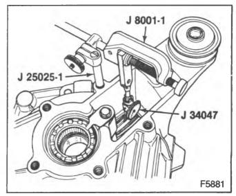
Figure 26-Measuring Backlash at the Ring Gear
