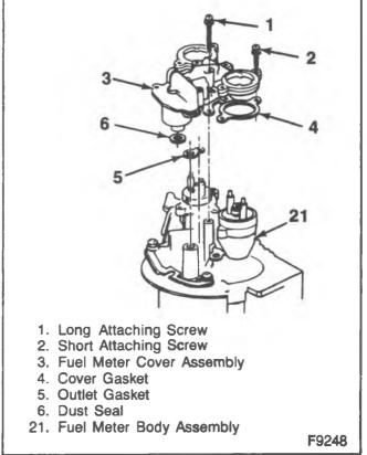
Figure 6—Replacing Model 220 Fuel Meter Cover
