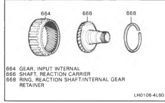
Figure 49 Input Internal Gear and Reaction Shaft
