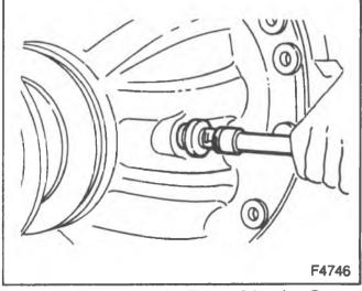
Figure 4-Loosening the Thrust Adjusting Screw
