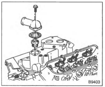
Figure 27-Thermostat and Coolant Outlet
