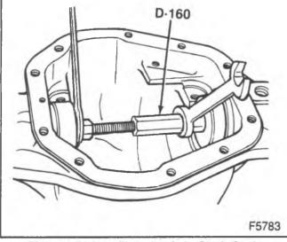
Figure 17-Installing the Axle Shaft Seals
