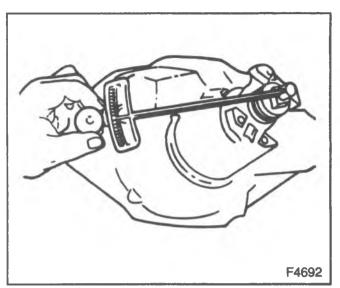
Figure 15-Checking Pinion Bearing Preload
