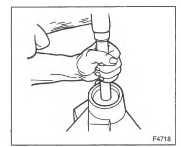
Figure 70—Installing the Pinion Front Cup
