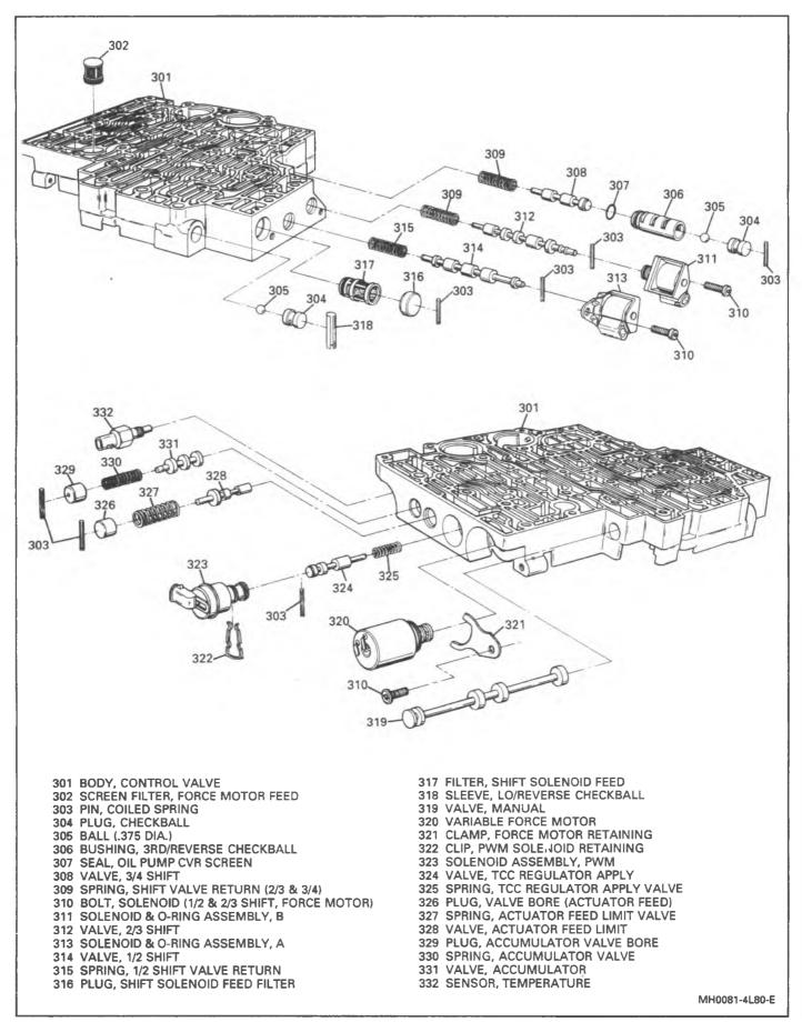
Figure 95 Control Valve Assembly
