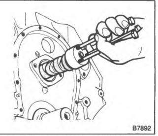
Figure 32—Replacing the Camshaft (Typical)
