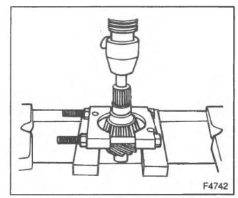
Figure 8—Removing the Pinion Inner Bearing
