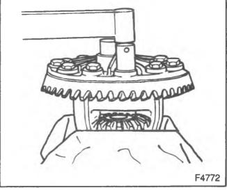
Figure 19—Installing the Ring Gear Bolts
