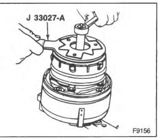
Figure 5---Replacing the Shaft Nut
