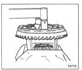
Figure 61-Differential with the Master Bearings
