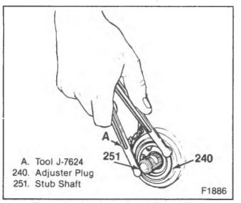
Figure 6—Removing the Adjuster Plug
