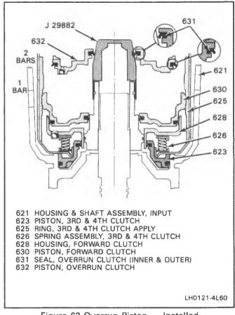
Figure 63 Overrun Piston — Installed
