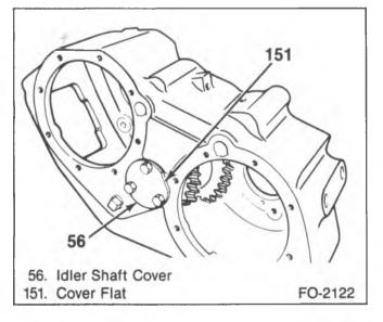
Figure 13-Idler Shaft Cover Alignment
