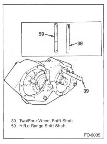
Figure 7—Removing the Shift Rail
