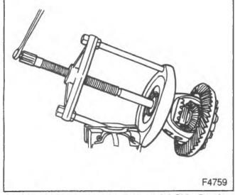
Figure 14—Removing the Differential Side Bearing
