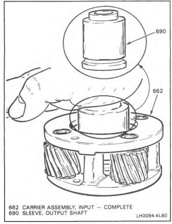
Figure 38 Captive Thrust Bearing Check
