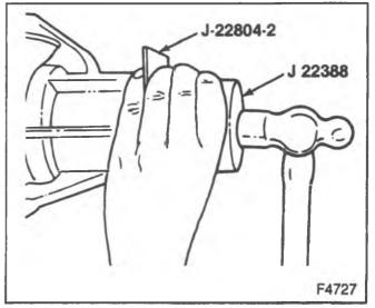
Figure 16-Installing the Pinion Oil Seai
