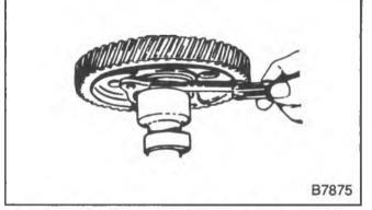
Figure 25—Measuring Camshaft Thrust Plate Clearance (Camshaft End Play)
