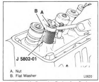
Figure 23—Removing Rocker Arm Stud
