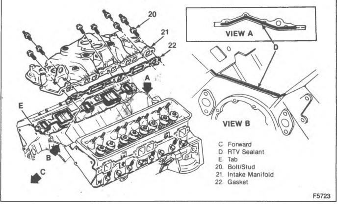
Figure 77-Intake Manifold (5.0L and 5.7L Engines)
