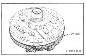
Figure 98 Oil Pump Alignment Band
