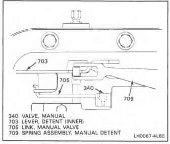
Figure 11 Manual Valve Link
