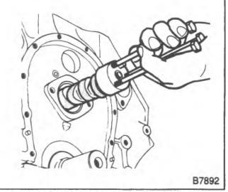
Figure 13-Replacing the Camshaft (Typical)
