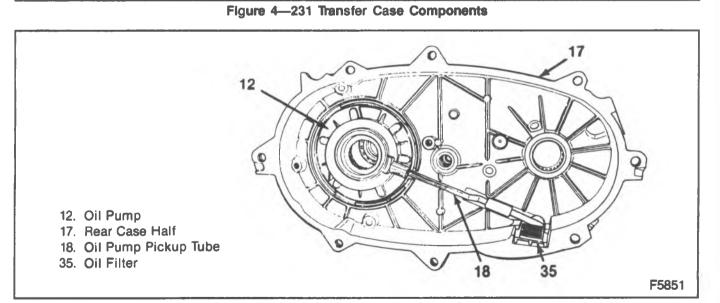
Figure 5-Oil Pump, Pickup Tube and Screen
