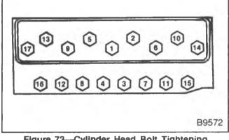
Figure 73—Cylinder Head Bolt Tightening Sequence (5.0L and 5.7L Engines)
