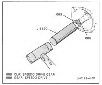
Figure 130 Speedometer Gear — Installation
