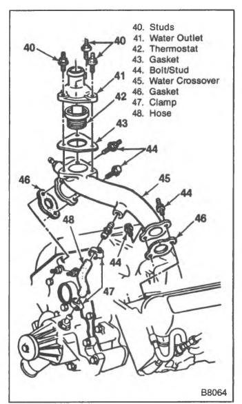
Figure 54—Thermostat and Coolant Crossover
