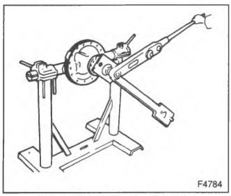
Figure 17-Installing the Pinion Nut
