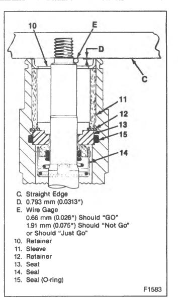
Figure 16—Shaft and Seal Position and Correct Position Gaging Guide
