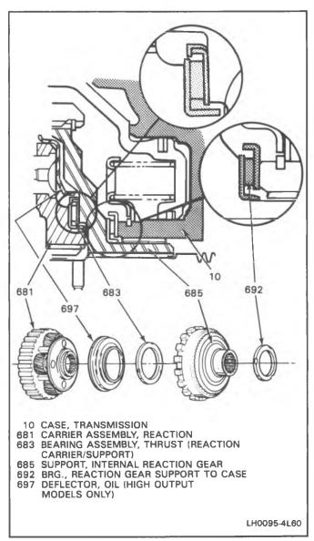
Figure 39 Reaction Internal Gear and Carrier Bearing Locations
