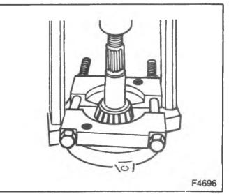
Figure 9---Removing the Pinion Rear Bearing
