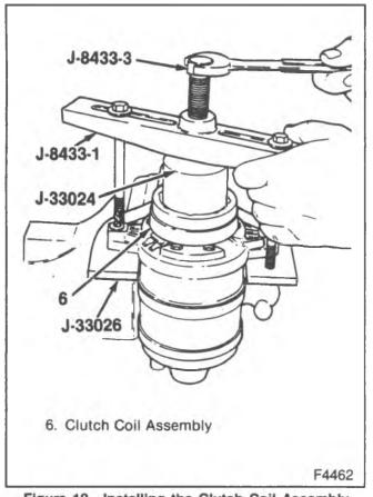
Figure 18—Installing the Clutch Coil Assembly
