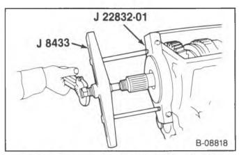
Figure 7 Removing the Mainshaft Rear Bearing
