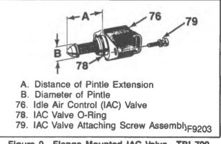
Figure 9—Flange Mounted IAC Valve—TBI 700
