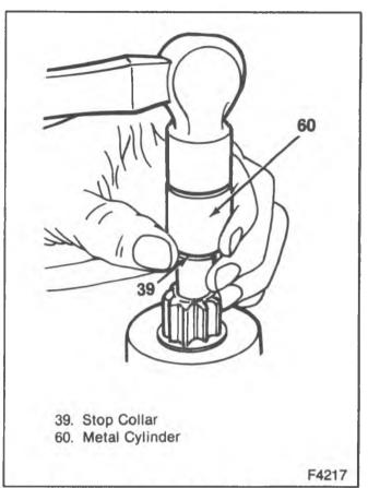
Figure 9—Driving the Stop Collar Off the Retaining Ring
