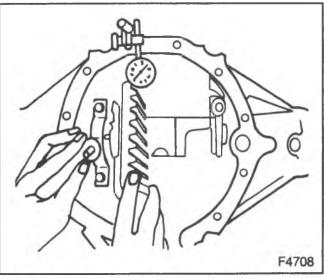
Figure 19-Installing Side Bearing Gaging Tools
