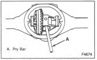
Figure 7-Removing the Differential Case
