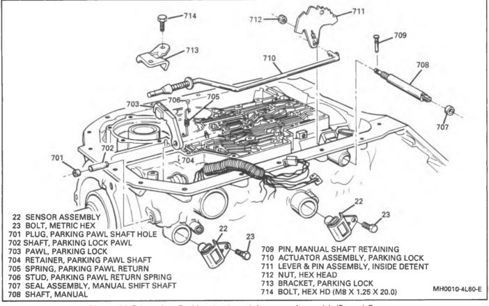
Figure 29 Removing Parking Lock and Actuator Assembly/Speed Sensors
