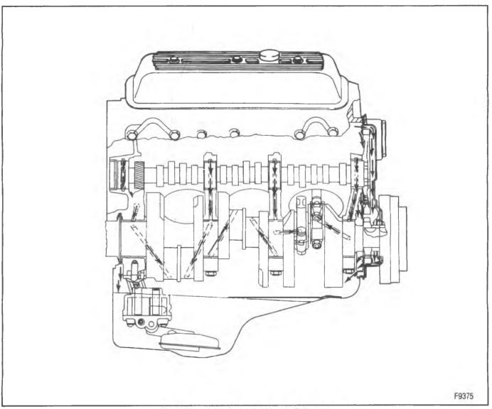
Figure 1—Engine Lubrication Diagram
