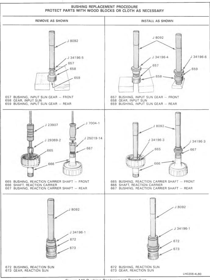
Figure 146 Bushing Replacement Procedure
