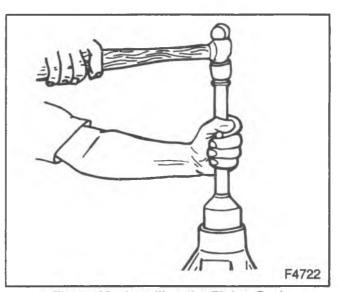
Figure 33—Installing the Pinion Seal
