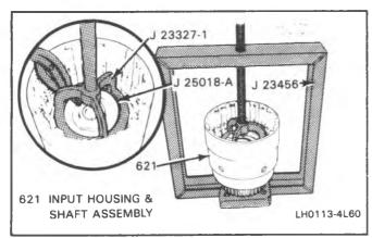
Figure 55 Overrun Clutch Retainer Ring - Removal
