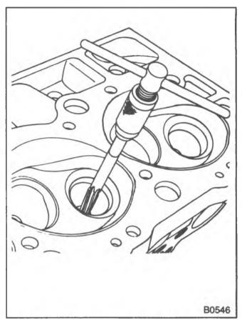
Figure 36-Reaming the Valve Guides (Typical)
