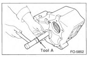
Figure 8—Removing the Idler Shaft
