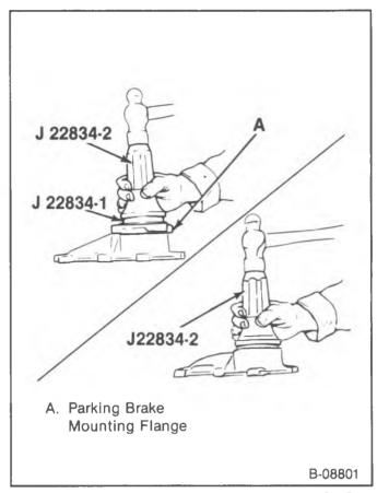
Figure 29 Installing the Rear Bearing Retainer Oil Seal
