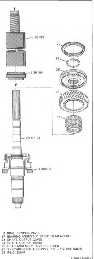
Figure 25 Reverse Gear Components Installed
