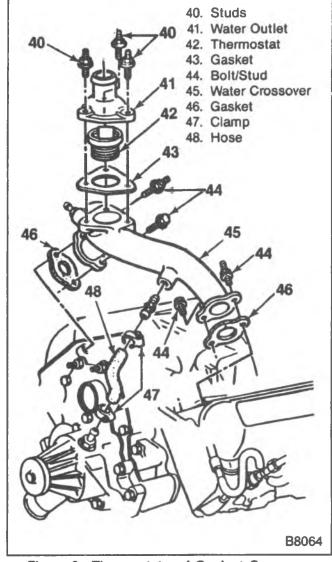
Figure 9—Thermostat and Coolant Crossover
