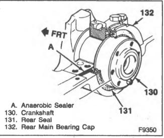
Figure 53—Applying Sealant to the Block (7.4L Engines)
