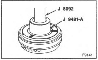
Figure 10-Installing the Pulley Bearing
