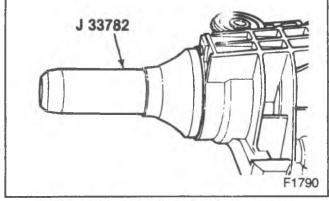
Figure 21-Installing the Pinion Seal
