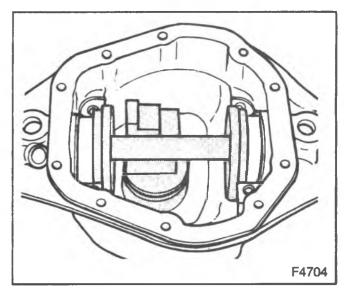
Figure 24—Pinion Height Block
