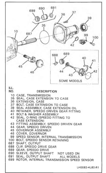
Figure 7 Extension and Associated Parts
