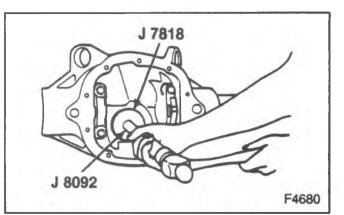
Figure 13-Installing the Rear Pinion Bearing Cup
