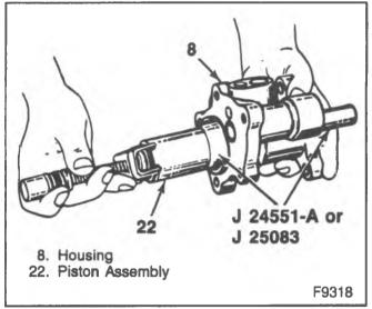
Figure 7-Installing the Piston Assembly
