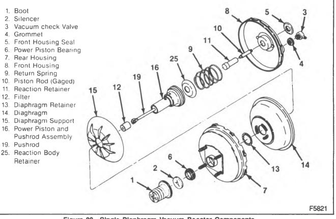
Figure 20-Single Diaphragm Vacuum Booster Components
