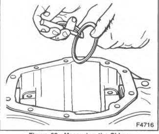
Figure 68—Measuring the Shims
