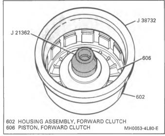
Figure 58 Installing Forward Clutch Piston
