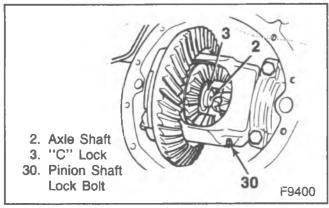
Figure 2—Pinion Shaft Lock Bolt
