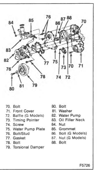
Figure 42—Front Cover and Components
