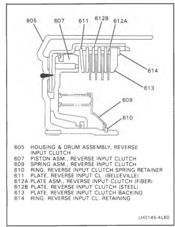
Figure 87 Reverse Input Clutch
