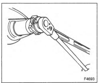
Figure 5—Pinion Flange Nut Removal
