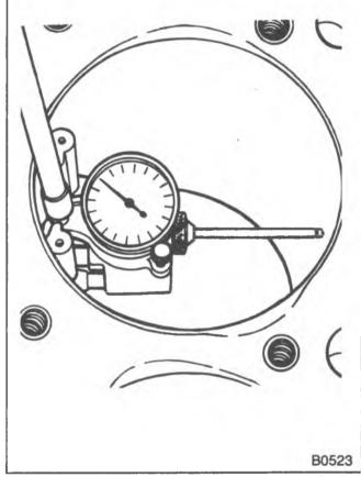
Figure 1—Checking the Cylinder Bore
