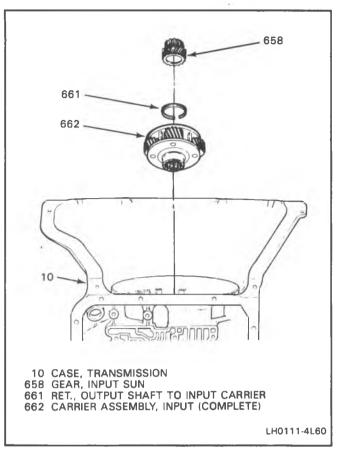
Figure 53 Input Carrier and Sun Gear — Installation
