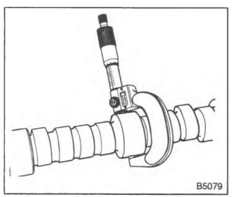
Figure 19—Inspecting the Camshaft Journals
