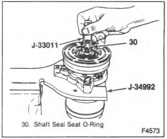
Figure 24-Installing the Shaft Seal Seat O-Ring
