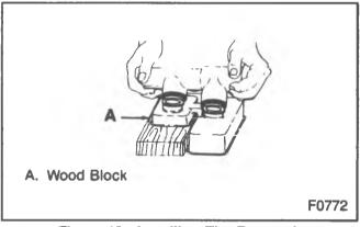
Figure 12---Installing The Reservoir
