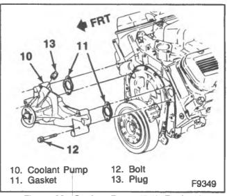
Figure 86-Coolant Pump (7.4L Engines)
