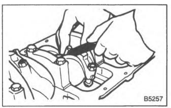
Figure 48—Measuring Connecting Rod Side Clearance
