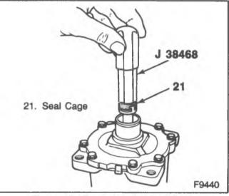
Figure 12-Removing the Seal Cage
