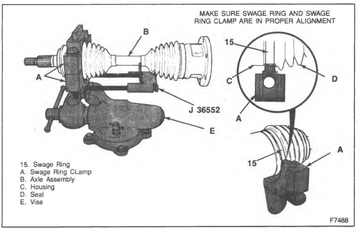
Figure 42-Installing Swage Ring
