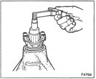
Figure 76—Checking Pinion Preload
