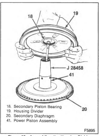
Figure 29—Assembling the Housing Divider
