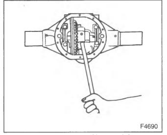
Figure 3—Prying the Differential Case
