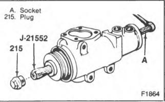
Figure 4-Removing the Plug and Piston Rack
