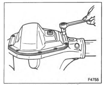
Figure 41-Installing the Axle Cover
