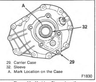
Figure 25—Marking Sleeve Location
