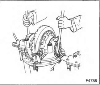
Figure 24—Adjusting Side Bearing Preload
