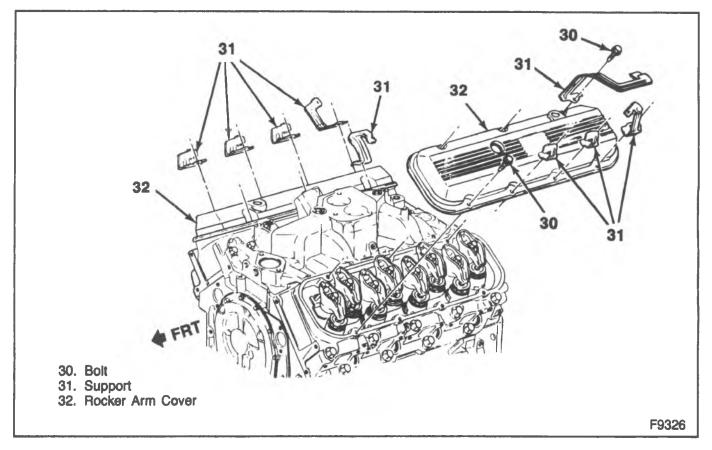
Figure 10—Rocker Arm Cover (7.4L Engines)
