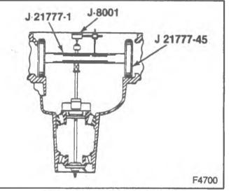
Figure 13—Pinion Depth Tools
