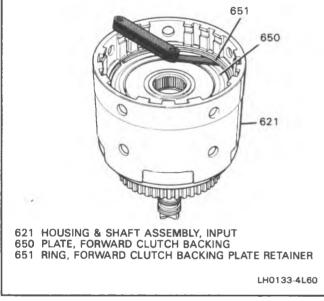
Figure 75 Forward Clutch Backing Plate Travel
