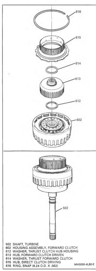
Figure 61 Checking Forward Clutch Piston Travel
