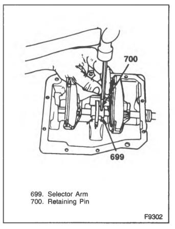
Figure 32-Removing the Shift Shaft Retaining Pin
