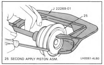
Figure 5 Second Servo Piston Retaining Ring Removal
