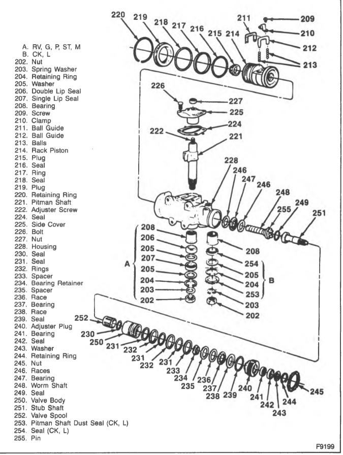
Figure 1—Integral Steering Gear Components
