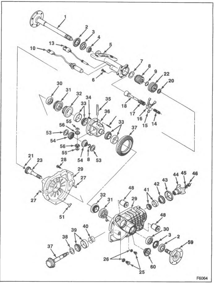
Figure 1—Front Axie Components (K1, 2 Models)
