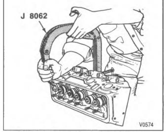
Figure 22—Compressing the Valve Springs
