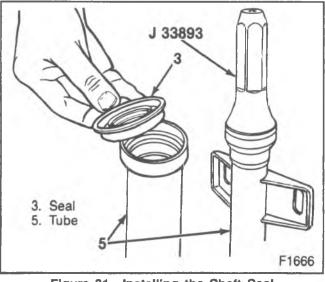
Figure 31-Installing the Shaft Seal
