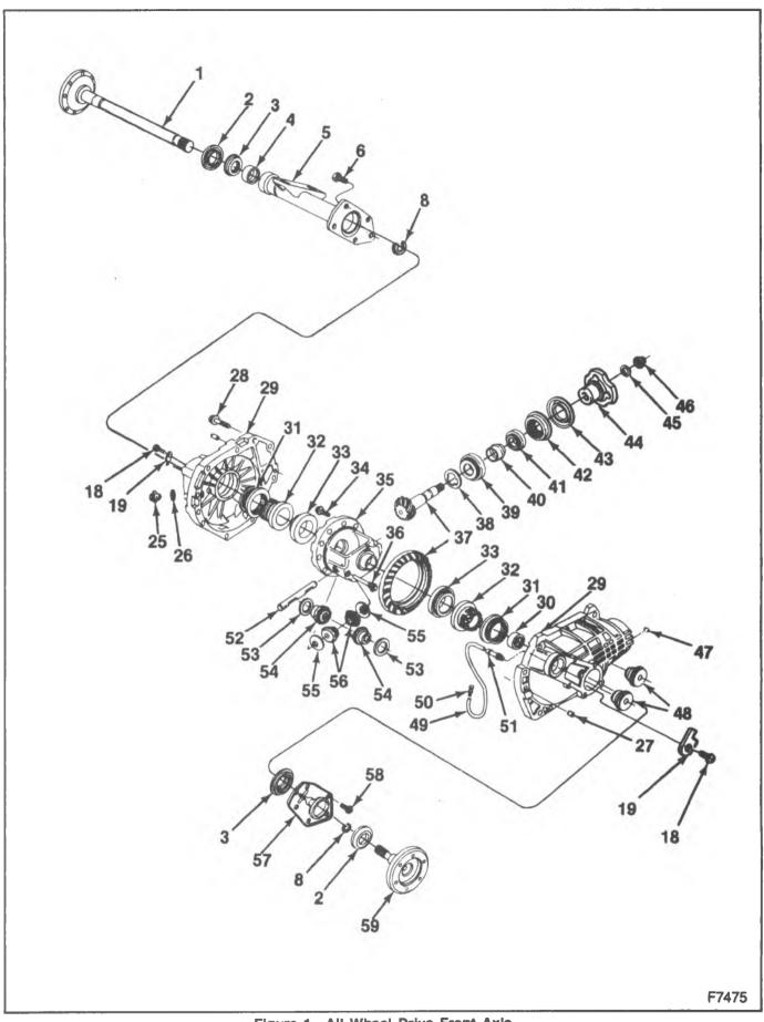
Figure 1-All Wheel Drive Front Axle
