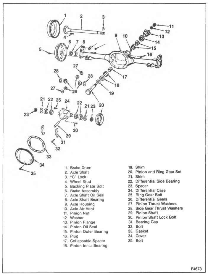
Figure 2-Rear Axle Components
