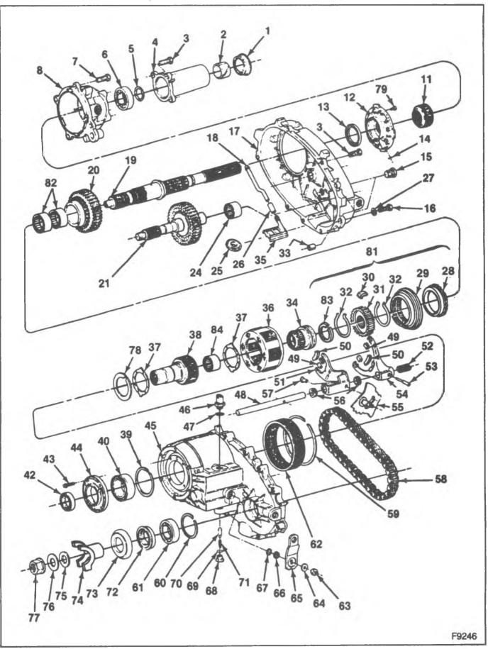
Figure 3-231 Transfer Case Components
