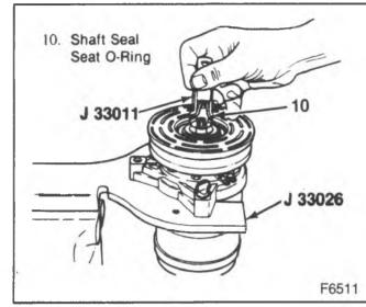
Figure 25-Installing the Seal Seat O-Ring
