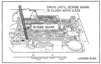
Figure 33 Third Accumulator Retainer and Ball Asm.— Installation
