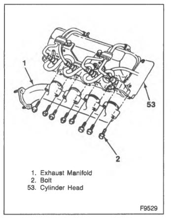
Figure 6—Exhaust Manifold Right Side
