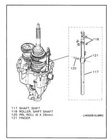
Figure 8 Removing Shift Shaft Rollers and Finger
