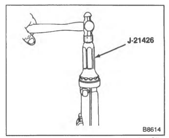
Figure 27—Installing the Extension Housing Oil Seal
