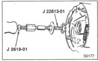
Figure 4—Removing the Axle Bearing
