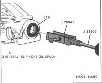
Figure 50 Removing 2WD Slip Yoke Oil Seal
