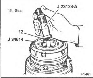
Figure 22—Removing the Shaft Seal with J 23128-A
