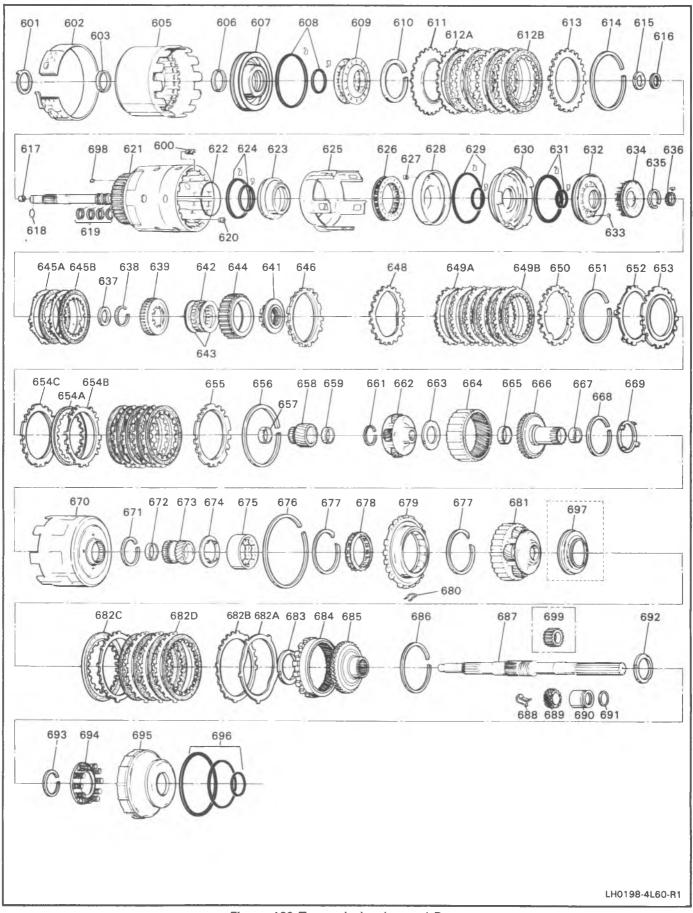
Figure 139 Transmission Internal Parts
