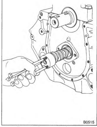
Figure 22-Removing the Camshaft
