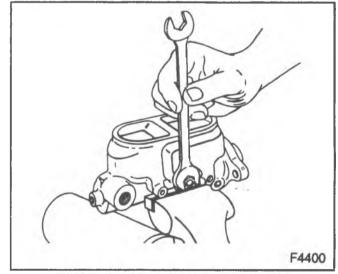
Figure 18-Installing the Tube Seats
