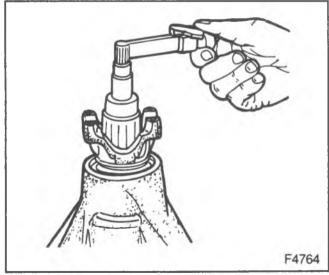
Figure 36—Checking Pinion Preload
