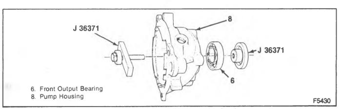
Figure 13—Installing the Pump Housing Bearing
