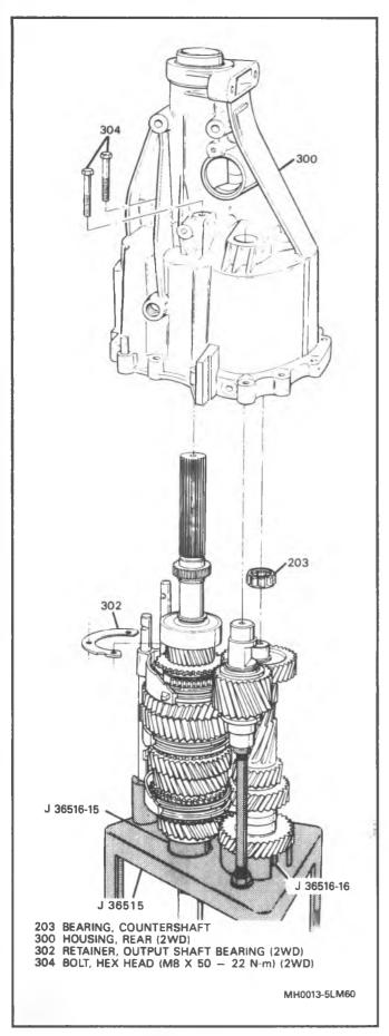
Figure 13 Removing 2WD Rear Housing
