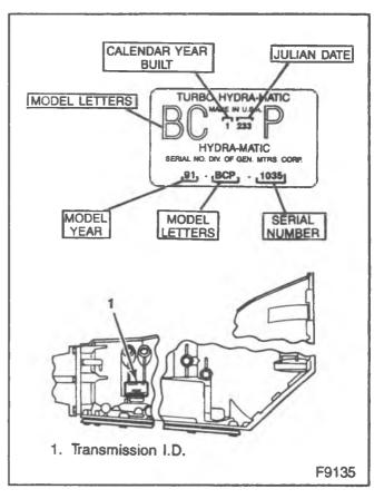
Figure 13—Hydra-Matic 4L80E Transmission i.D.Location
