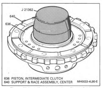
Figure 36 Installing Intermediate Piston Seals
