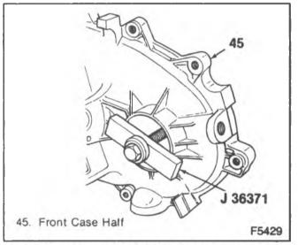
Figure 12-Installing the Front Output Bearing with J 36371
