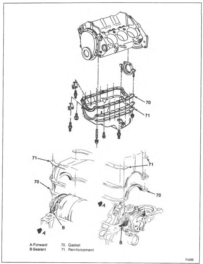
Figure 39-Oil Pan Installation
