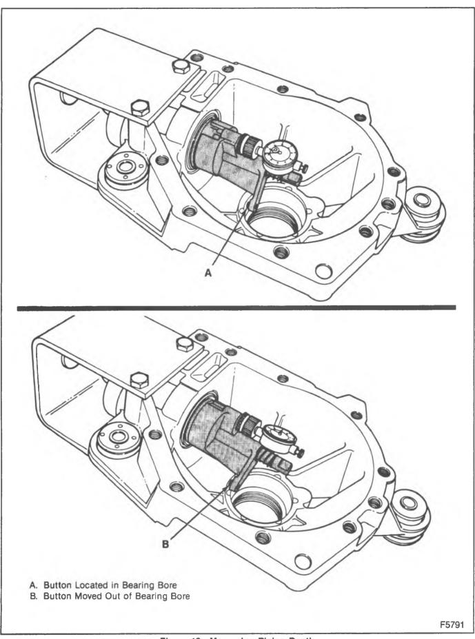
Figure 18—Measuring Pinion Depth
