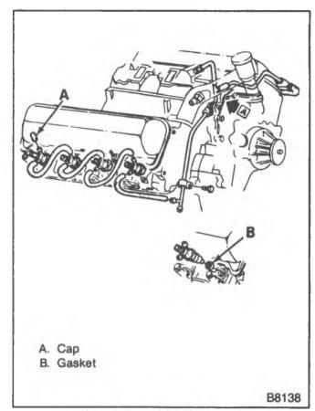
Figure 55—Injection Nozzles
