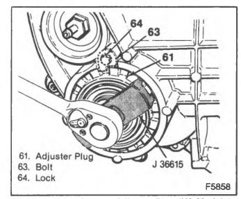
Figure 9—Turning the Adjuster Plug (K3 Models)
