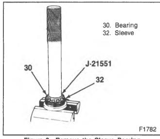
Figure 9-Remove the Sleeve Bearing
