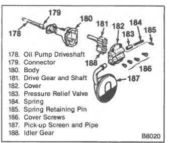
Figure 35—Oil Pump Components (5.0L and 5.7L Engines)
