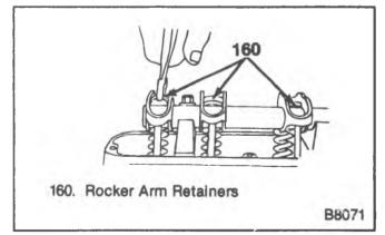
Figure 22-Removing the Rocker Arm Retainers
