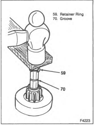
Figure 17-Forcing the Retainer Ring on the Shaft
