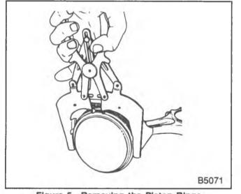
Figure 5—Removing the Piston Rings
