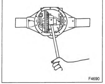
Figure 3-Removing the Differential Case
