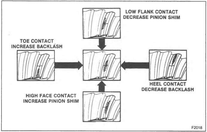
Figure 21—Gear Tooth Pattern
