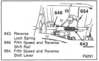
Figure 13----5th Speed and Reverse Shift Shaft
