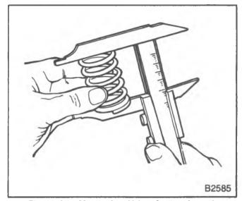
Figure 34—Measuring Valve Spring Length
