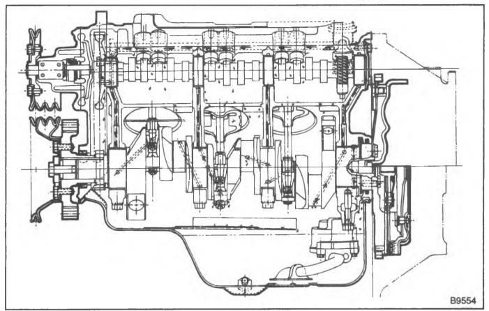
Figure 1—Engine Lubrication Diagram
