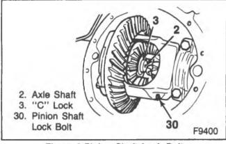
Figure 2-Pinion Shaft Lock Bolt
