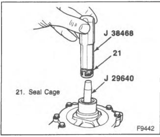
Figure 13—Installing the Seal Cage
