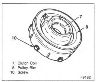
Figure 20—Assembling Clutch Coil, Pulley Rim, Rotor and Bearing Assembly
