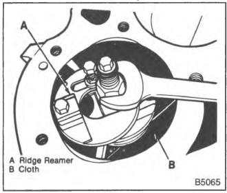
Figure 23—Removing the Cylinder Ridge
