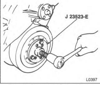
Figure 12—Removing the Torsional Damper
