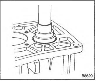
Figure 33----Installing the Countergear Front Bearing
