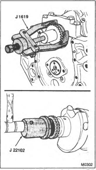
Figure 33—Crankshaft Sprocket Replacement (7.4L. Engines)
