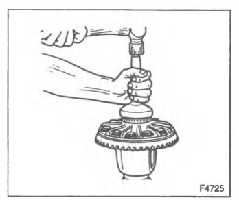
Figure 37—Installing the Differential Bearings
