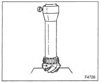
Figure 15-Installing the Pinion Inner Bearing
