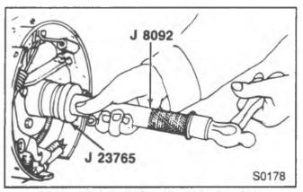
Figure 26—Installing the Axle Bearing
