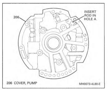
Figure 80 TCC Enable Valve Spring Rod Location
