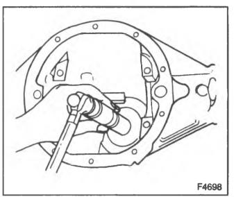
Figure 10-installing Rear Pinion Bearing Cup
