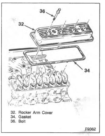
Figure 81—Rocker Arm Cover Installation (5.0L and 5.7L Engines)
