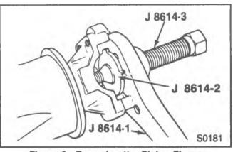
Figure 6-Removing the Pinion Flange
