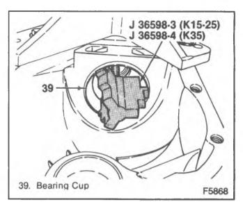
Figure 20—Installing the Inner Pinion Bearing Cup
