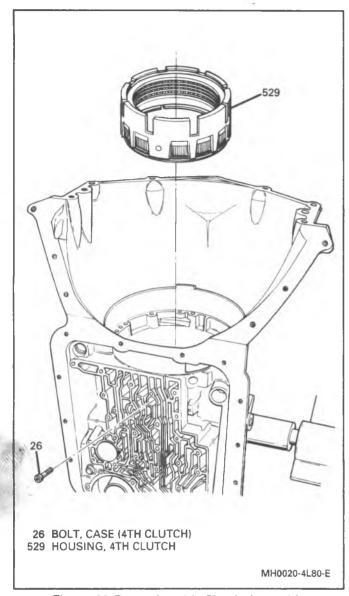
Figure 20 Removing 4th Clutch Assembly
