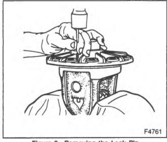
Figure 8-Removing the Lock Pin
