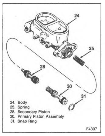
Figure 15—Cast Iron Master Cylinder Components
