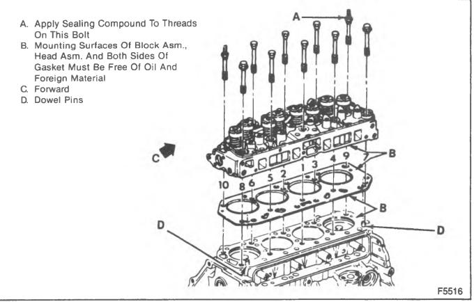
Figure 51—Cylinder Head Installation
