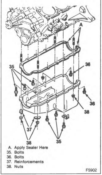
Figure 38—OII Pan Installation
