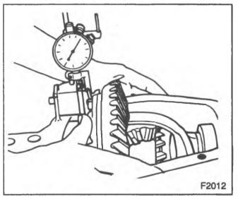
Figure 77—Measuring Differential Movement
