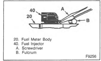
Figure 4—Removing TBI 700 Fuel Injector
