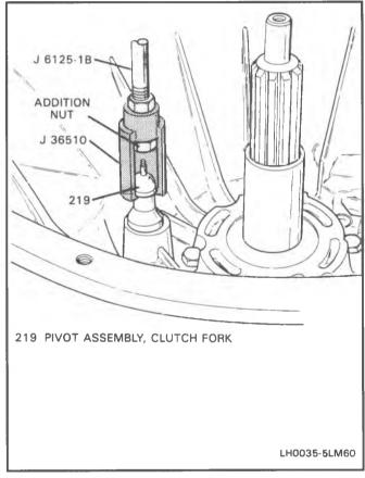
Figure 34 Removing Clutch Fork Pivot Assembly
