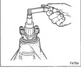
Figure 22—Measuring Pinion Bearing Preload
