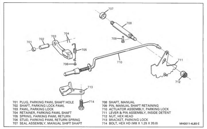
Figure 28 Parking Lock and Actuator Assembly
