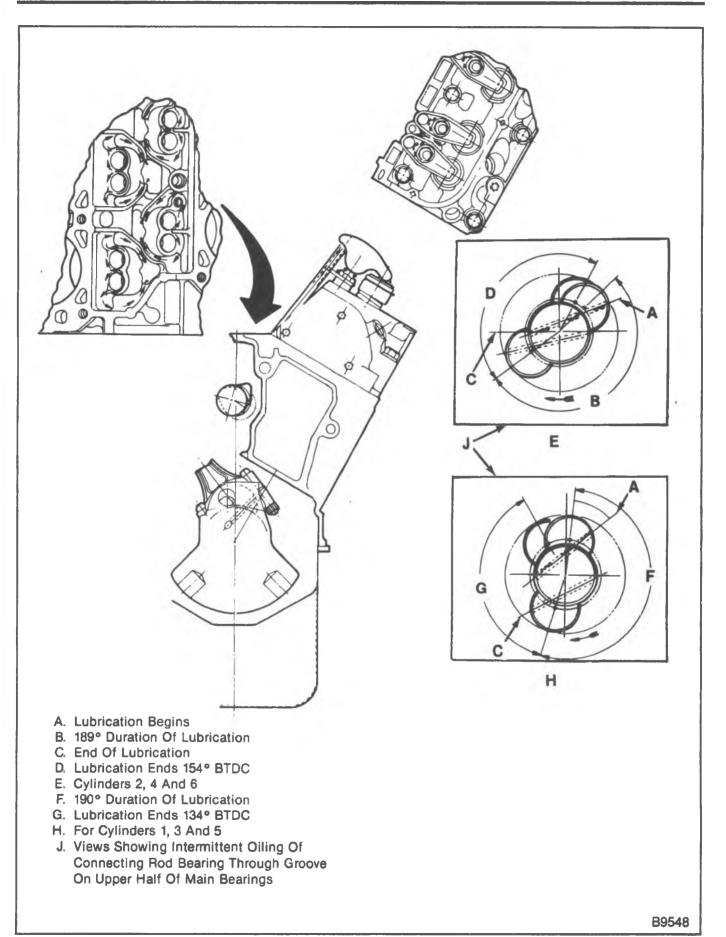
Figure 3—Engine Lubrication Diagram
