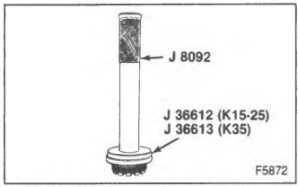
Figure 26-Installing the Adjuster Sleeve Bearing
