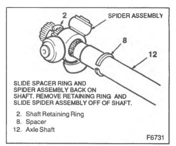
Figure 50—Removing Spider Assembly
