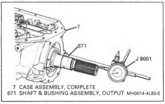
Figure 14 Checking Rear Unit End Play
