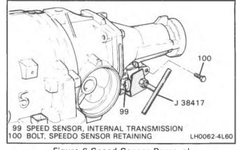
Figure 6 Speed Sensor Removal
