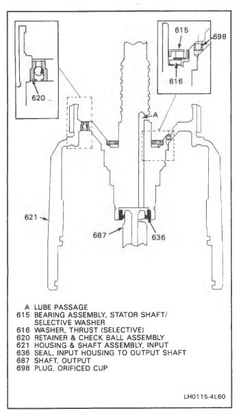
Figure 57 Input Housing Check Valve Ball
