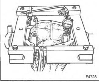
Figure 79—Mounting the Carrier Spreader
