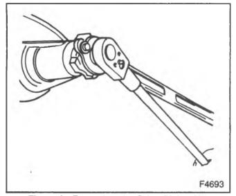
Figure 6-Removing the Drive Pinion Nut
