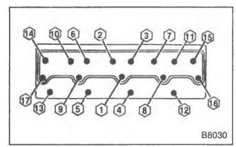
Figure 51-Head Bolt Tightening Sequence
