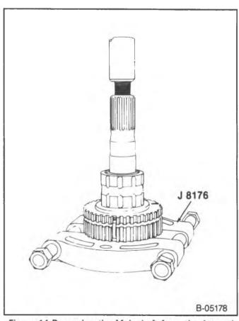
Figure 14 Removing the Mainshaft from the 1st and 2nd Speed Synchronizer Hub
