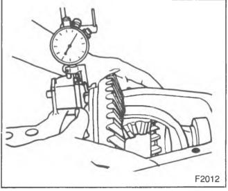
Figure 21-Determining Differential Shim Pack
