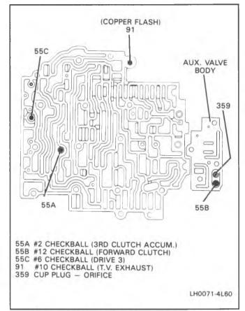
Figure 113 Valve Body Checkball Locations
