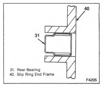
Figure 15-Slip Ring End Frame Bearing
