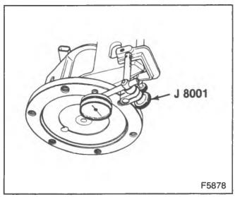
Figure 38—Measuring Axle Shaft End Play
