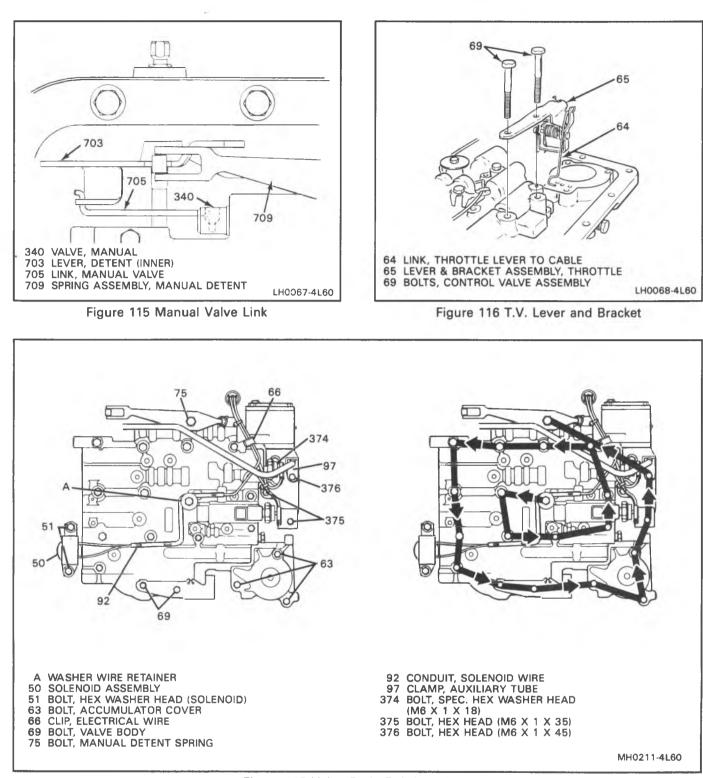
Figure 117 Valve Body Bolt Locations
