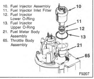
Figure 7—Model 220 Fuel Injection Parts
