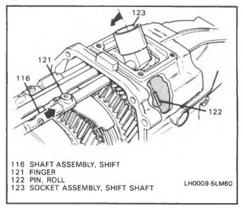
Figure 9 Removing Shift Socket Assembly Roll Pin
