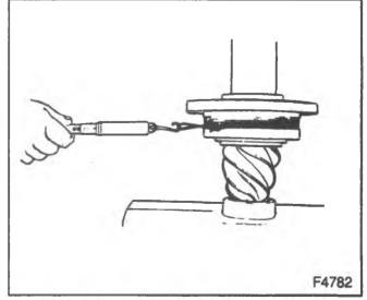
Figure 15-Measuring the Preload Torque
