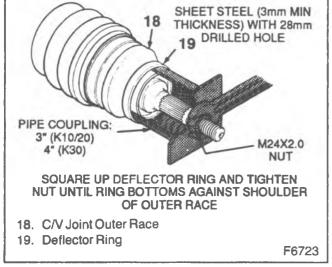
Figure 42-Installing Outer Deflector Ring
