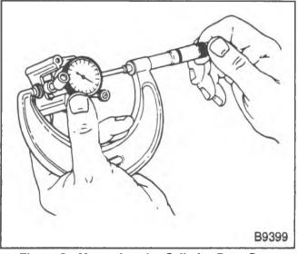
Figure 3—Measuring the Cylinder Bore Gage
