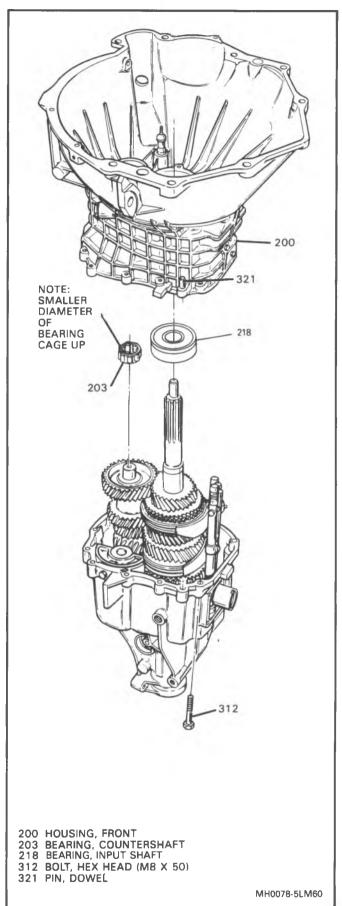
Figure 75 Front Housing Installation
