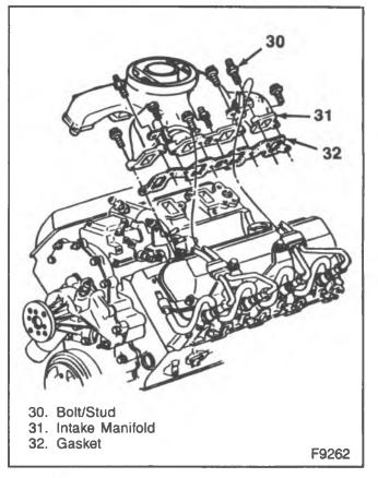
Figure 3-Single Plane Intake Manifold
