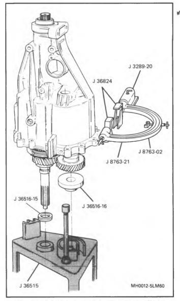
Figure 12 Removing and Installing Special Tools
