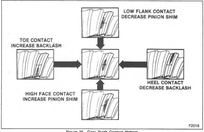
Figure 25—Gear Tooth Contact Pattern
