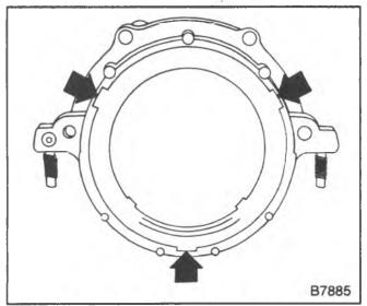
Figure 51—Seal Removal Notches (5.0 and 5.7L Engines)
