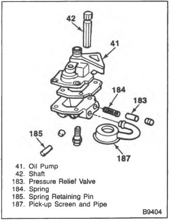
Figure 21—Oil Pump Components
