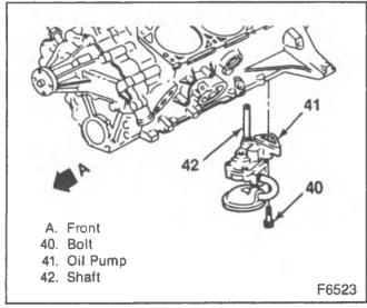
Figure 37—Oil Pump Installation
