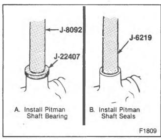
Figure 21—Installing the Pitman Shaft Bearing and Seals
