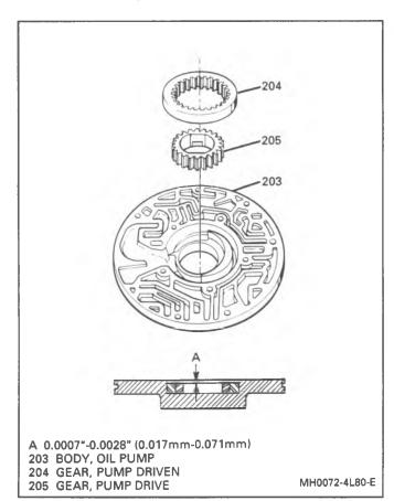
Figure 79 Measuring Pump Body Face To Gear Face Clearance
