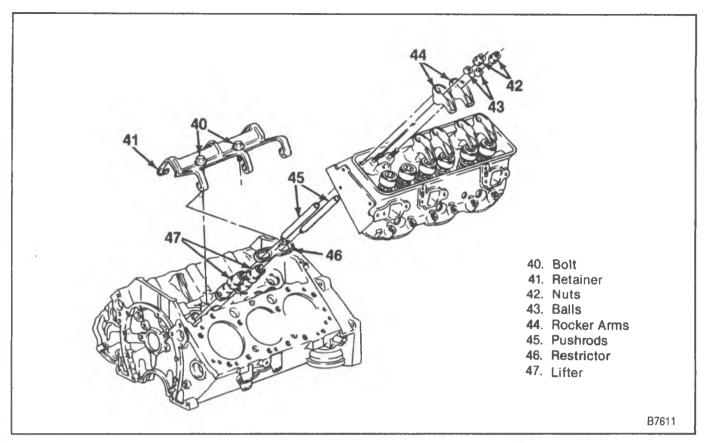
Figure 4—Valve Train Components
