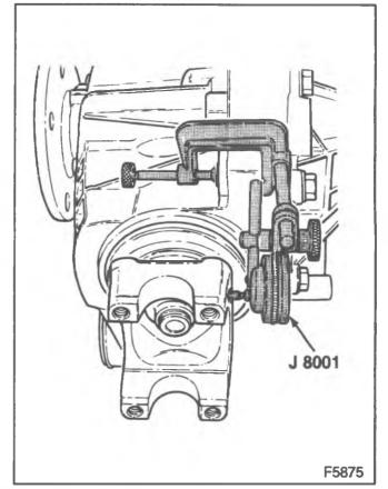
Figure 31—Measuring Backlash at the Pinion Flange
