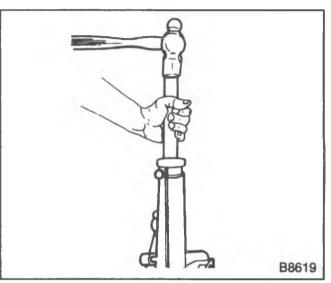
Figure 26—Installing the Extension Housing Bushing
