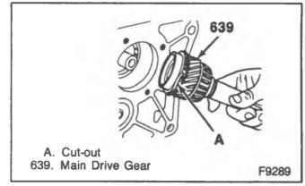
Figure 11-Main Drive Cut Out
