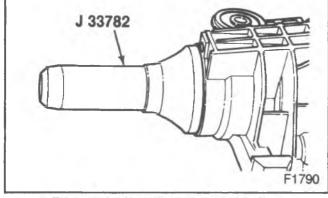
Figure 23-Installing the Pinion Seal
