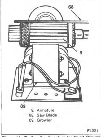
Figure 14—Testing the Armature for Short Circuits
