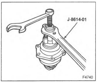
Figure 6—Removing the Pinion Flange
