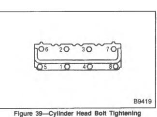
Figure 39—Cylinder Head Bolt Tightening Sequence
