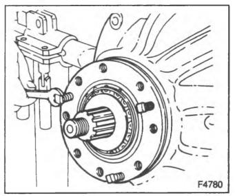
Figure 13----Removing the Pinion Cage
