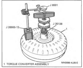
Figure 103 Converter End Play Check
