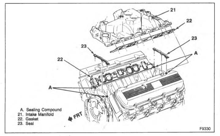
Figure 79-Intake Manifold (7.4L Engines)
