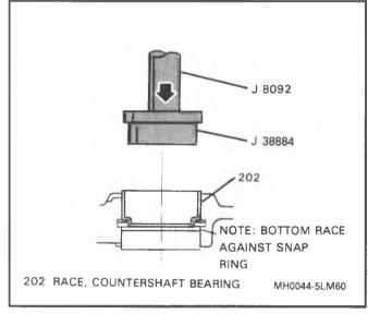
Figure 43 Countershaft Bearing Race Installation
