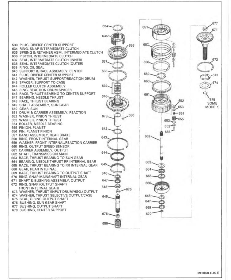
Figure 31 Center Support and Gear Unit Assembly
