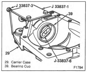
Figure 13—Removing the Inner Pinion Bearing Cup
