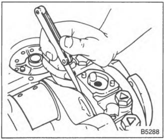
Figure 30-Measuring Crankshaft End Play (Typical)
