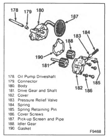
Figure 36—Oil Pump Components (7.4L Engines)
