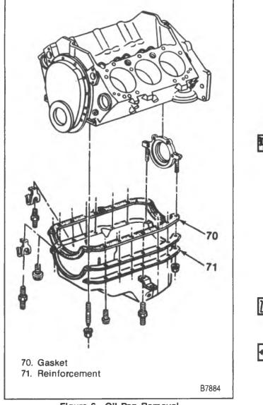
Figure 6-Oil Pan Removal
