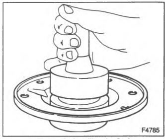
Figure 19-Installing the Seal
