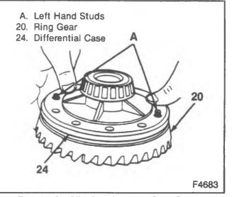
Figure 19-Aligning the Ring Gear Studs
