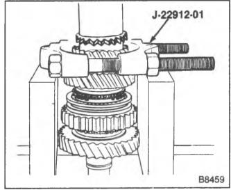
Figure 20-Removing the 5th Speed Driven Gear
