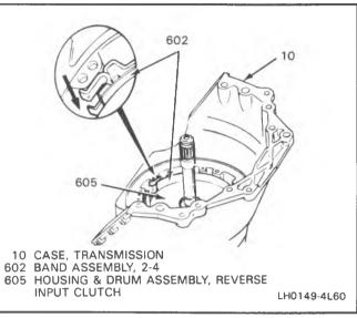
Figure 91 2-4 Band Assembly — Installed
