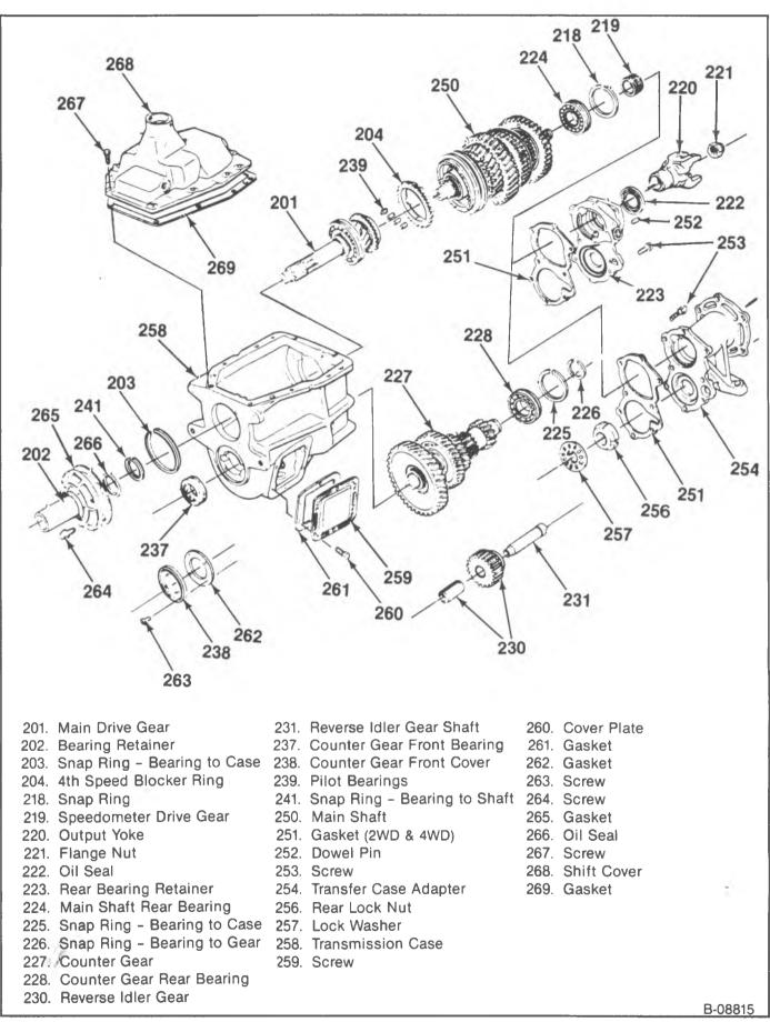
Figure 3 Transmission Components
