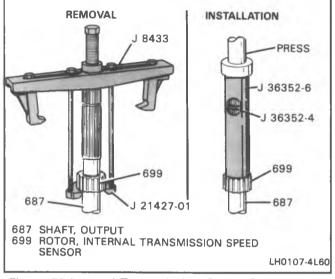
Figure 50 Internal Transmission Speed Sensor Rotor
