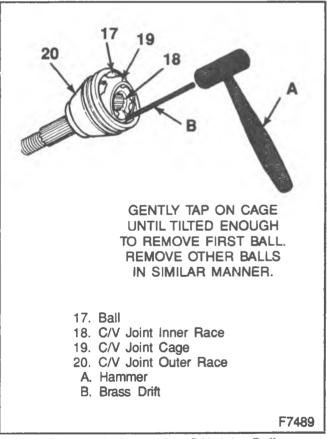
Figure 43—Removing C/V Joint Ball
