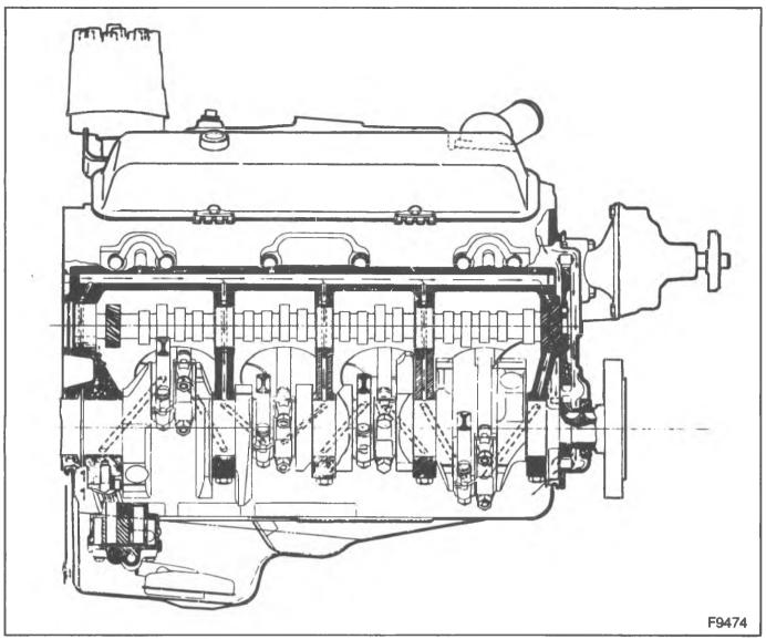
Figure 2—Lubrication Diagram (5.0L and 5.7L Engines)
