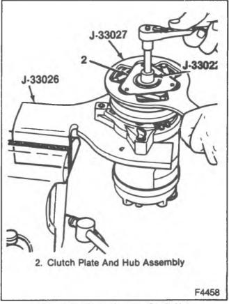
Figure 5—Removing the Shaft Nut
