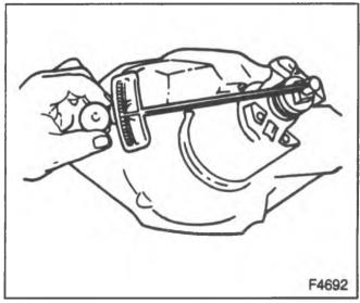
Figure 5—Checking Pinion Preload
