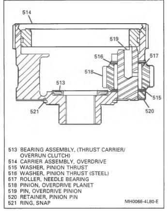
Figure 73 Overdrive Carrier Assembly
