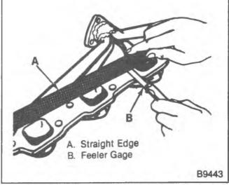
Figure 18—Inspecting Manifold Flange Alignment
