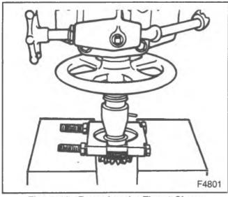
Figure 11—Removing the Thrust Sleeve
