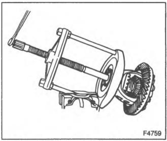
Figure 6-Removing the Differential Side Bearings
