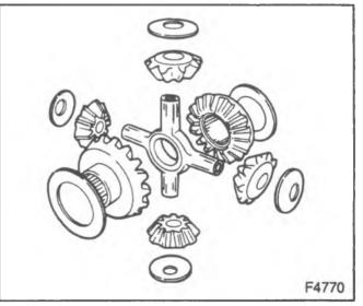
Figure 9----Differential Components
