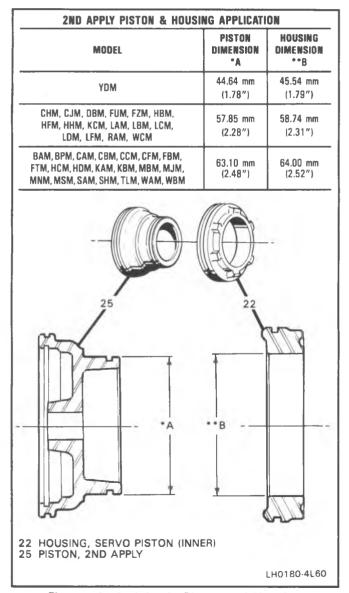
Figure 121 2nd Apply Piston and Housing Measurement
