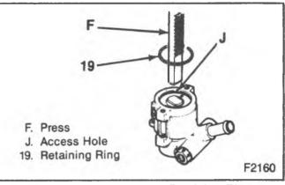
Figure 42-Installing the Retaining Ring.
