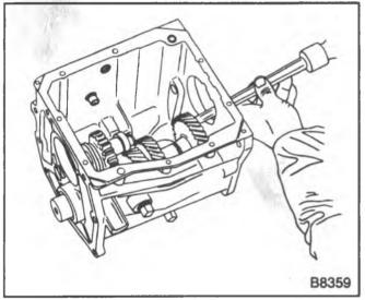
Figure 15—Removing the Countergear Rear Bearing
