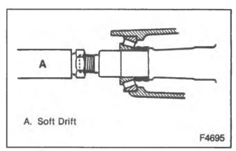
Figure 8—Removing the Drive Pinion
