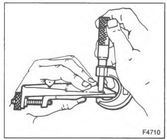
Figure 23—Measuring the Gage Plate Thickness
