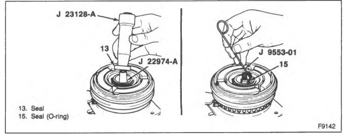
Figure 14-Removing/Installing the Shaft Seal Seat and O-Ring
