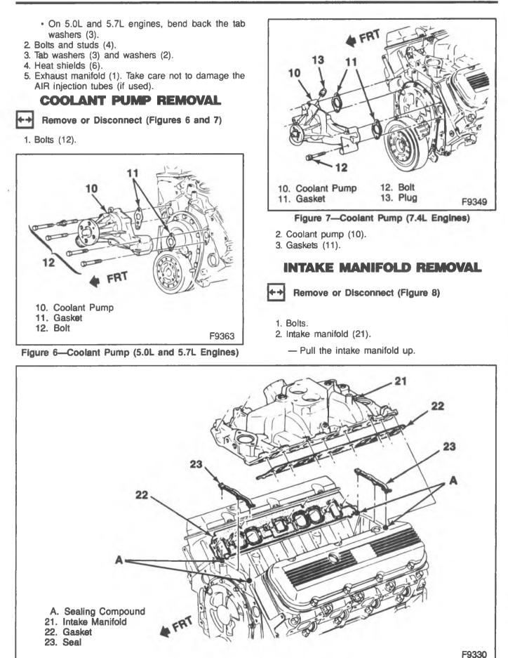
Figure 8-Intake Manifold (7.4L Engines)
