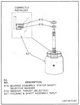
Figure 88 Thrust Bearing and Selective Washer Location
