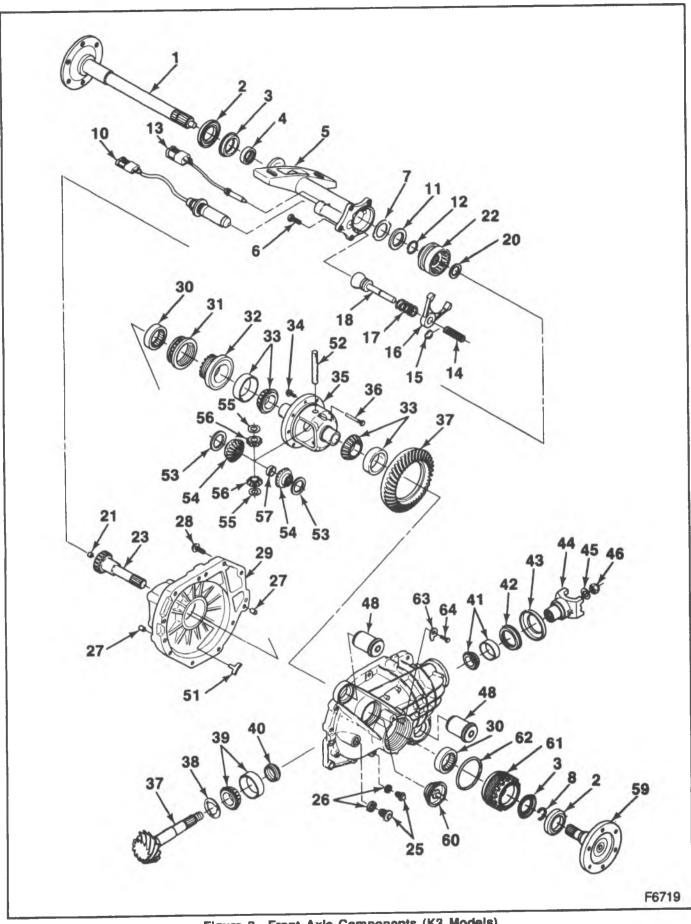
Figure 2---Front Axle Components (K3 Models)
