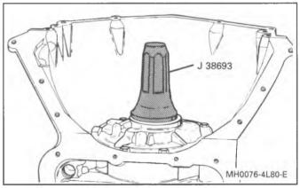
Figure 83 Installing Pump Seal
