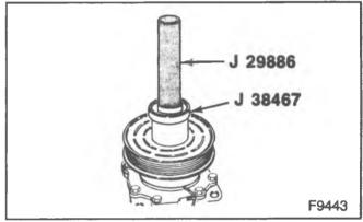
Figure 14-Installing the Rotor Pulley
