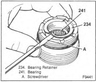
Figure 7-Removing the Bearing Retainer from **Adjuster Plug**
