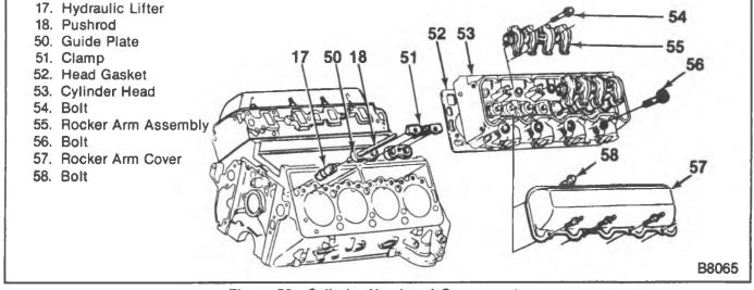
Figure 50—Cylinder Head and Components
