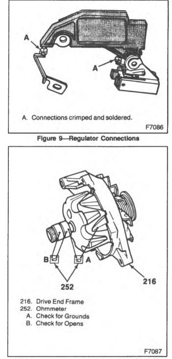
Figure 10—Checking the Rotor Field Windings
