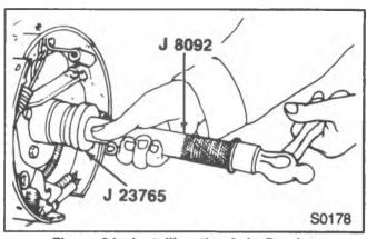
Figure 24-Installing the Axle Bearing
