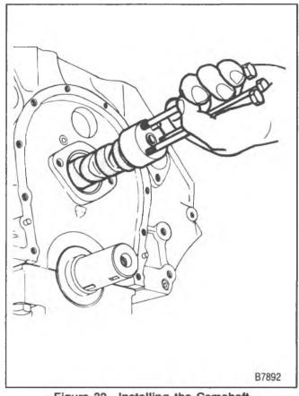
Figure 32-Installing the Camshaft
