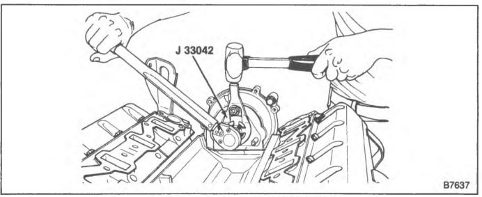
Figure 45—Marking TDC on the Front Cover
