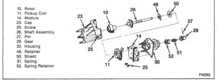
Figure 5-Distributor Components (Separate Coil and Sealed Connector)
