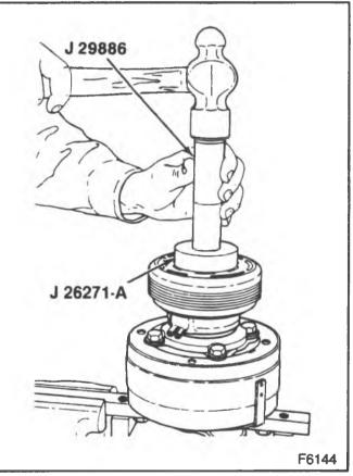
Figure 19—Installing the Rotor and Bearing (Poly-Groove Type)
