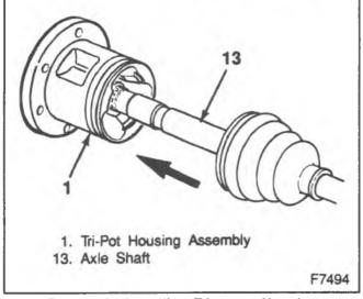
Figure 48-installing Tri-pot to Housing
