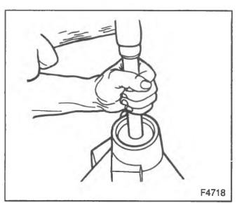
Figure 29-Installing the Pinion Front Cup
