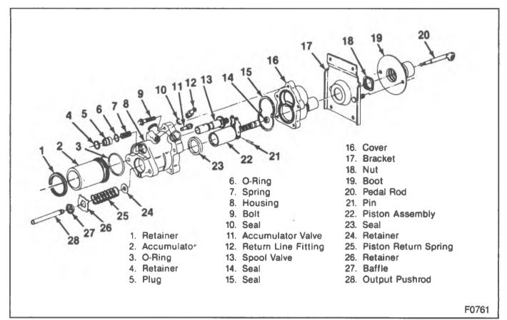
Figure 1-Hydro-Boost Components
