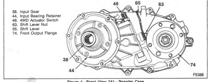
Figure 1—Front View 241—Transfer Case
