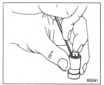
Figure 27—Installing the Check Ball Retainer (Typical)
