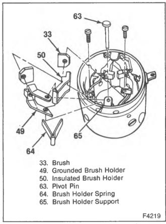
Figure 11-Replacing Brushes on the SD-300
