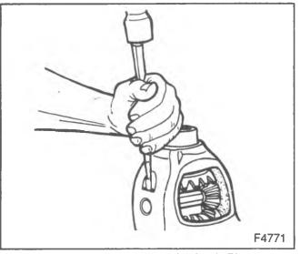
Figure 19---Installing the Lock Pin
