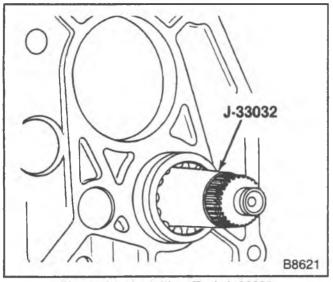
Figure 34-Installing Tool J 33032
