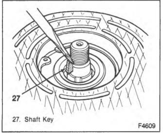
Figure 5---Removing the Shaft Key
