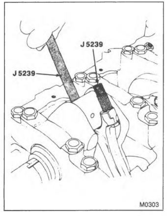
Figure 15—Replacing the Piston and Connecting Rod (Typical)
