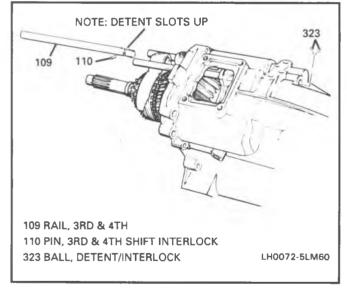
Figure 69 Interlock Balls and 3-4 Shift Rail Installation
