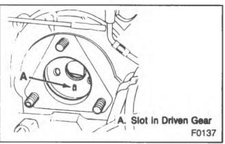
Figure 44—Slot in Injection Pump Gear
