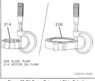
Figure 93 Oil Pump Rotor and Slide Selection
