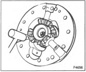
Figure 14-Installing the Pinion Yoke
