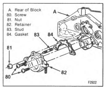
Figure 29—Rear Crankshaft Oil Seal Retainer Installation
