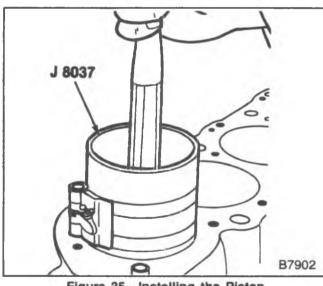
Figure 35-Installing the Piston
