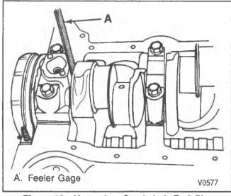
Figure 28—Measuring Crankshaft End Play
