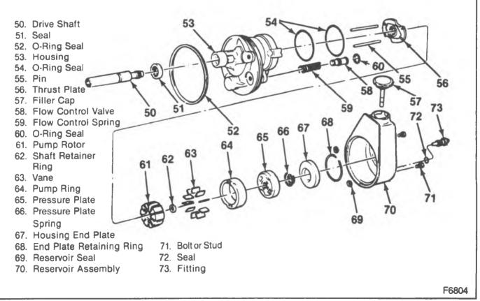
Figure 43—Power Steering Pump—Model P
