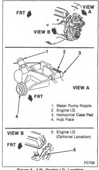
Figure 6-2.8L Engine I.D. Location
