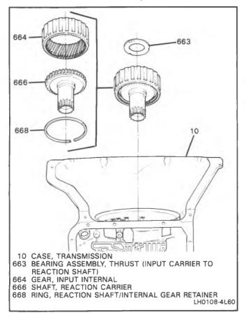
Figure 51 Input Internal Gear Installation
