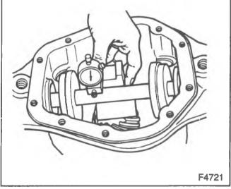
Figure 33—Checking the Pinion Depth Setting
