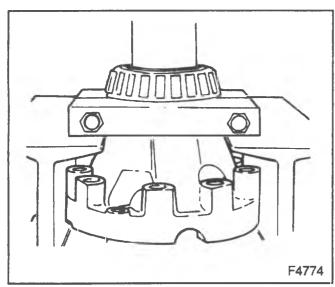
Figure 10-Removing the Differential Side Bearing
