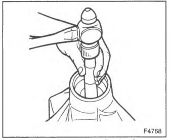
Figure 15—Removing the Bearing Cups
