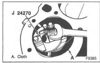
Figure 16—Removing the Cylinder Ridge
