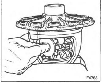
Figure 18-Installing the Pinion Gears
