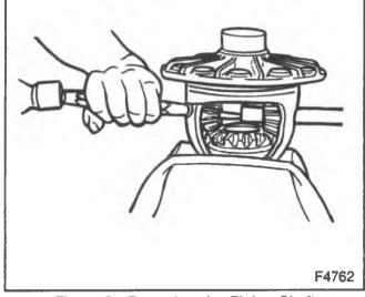
Figure 9—Removing the Pinion Shaft
