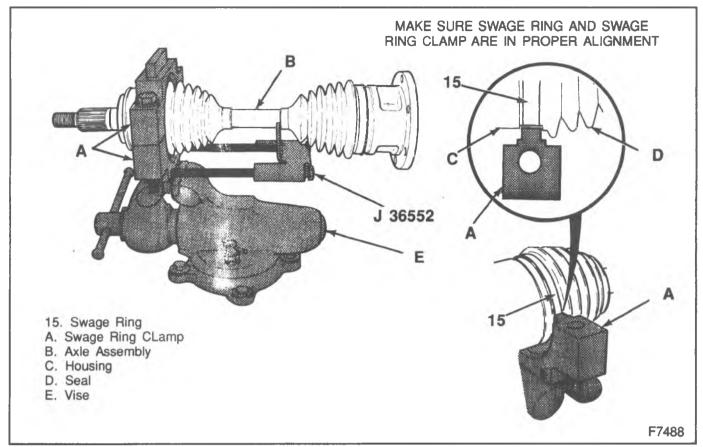
Figure 36—Installing Swage Ring
