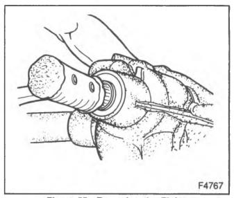
Figure 55—Removing the Pinion
