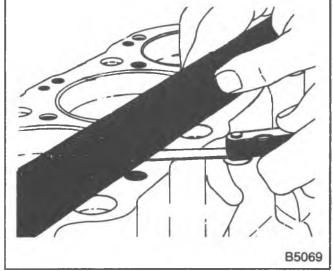
Figure 20-Checking the Block Gasket Surface
