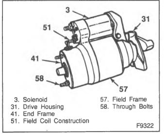
Figure 6—Light Duty Starting Motor
