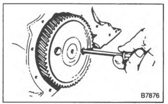
Figure 42—Installing the Camshaft Thrust Plate Bolts
