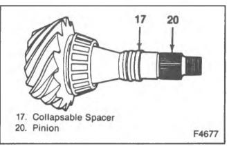
Figure 10—Pinion Collapsible Spacer
