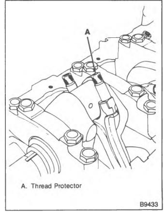
Figure 15—Connecting Rod Thread Protectors
