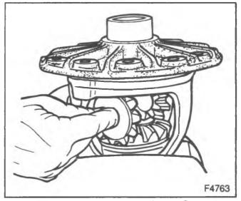
Figure 10-Removing the Pinion Gears
