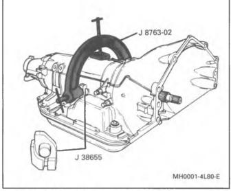
Figure 1 Transmission Holding Fixture, Base and Adapter
