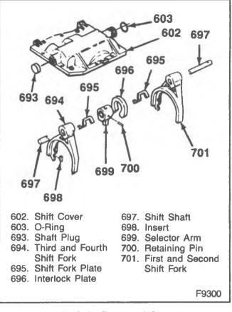
Figure 30—Shift Cover and Components
