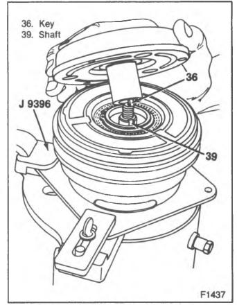
Figure 4—Aligning the Drive Plate Key
