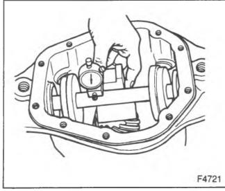
Figure 32—Checking the Pinion Depth Setting
