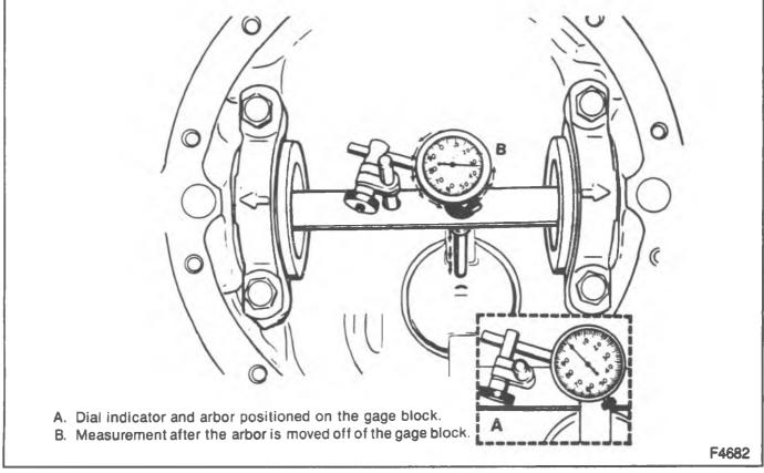
Figure 14—Checking Pinion Depth
