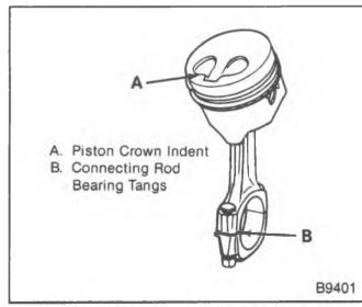
Figure 14—Aligning the Piston and Connecting Rod
