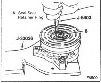
Figure 22—Removing or installing the Shaft Lip Seal Retaining Ring
