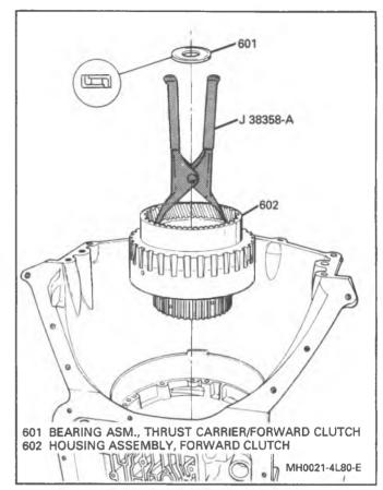
Figure 21 Removing Forward Clutch Assembly
