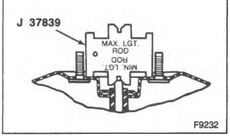
Figure 24—Gaging the Piston Rod
