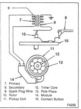
Figure 3—Basic Wiring Schematic
