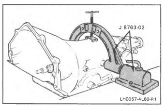
Figure 1 Holding Fixture
