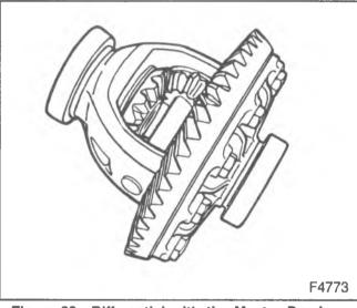
Figure 20-Differential with the Master Bearings
