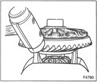
Figure 48-Removing the Ring Gear
