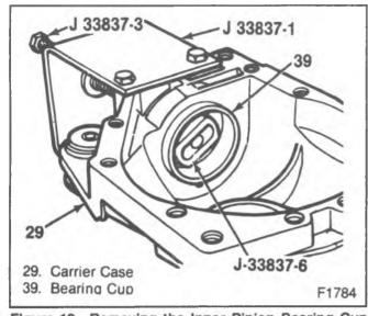
Figure 12—Removing the Inner Pinion Bearing Cup
