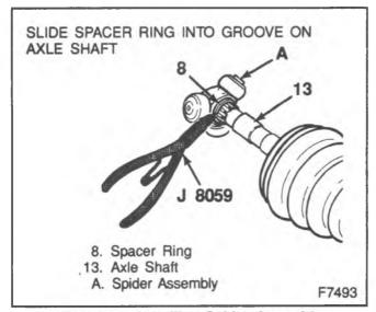
Figure 47-Installing Spider Assembly
