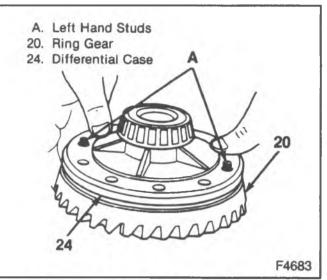
Figure 16-Aligning the Ring Gear Studs
