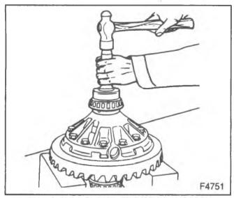
Figure 17-Installing Differential Bearings
