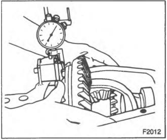
Figure 22-Determining Differential Shim Pack
