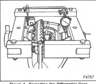
Figure 4—Spreading the Differential Case
