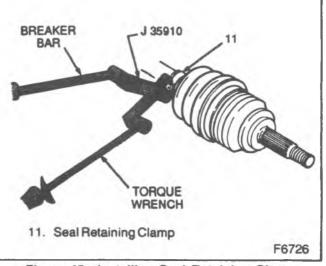
Figure 45—Installing Seal Retaining Clamp
