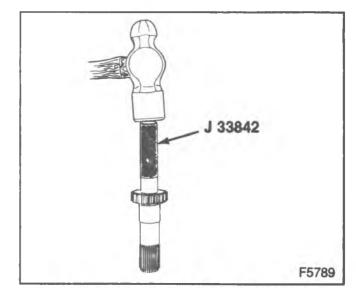
Figure 34—Installing the Pilot Bearing
