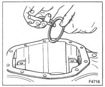
Figure 28—Measuring the Shims
