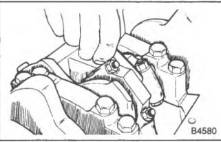
Figure 36—Méasuring the Connecting Rod Side Clearance (Typical)
