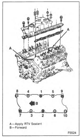
Figure 42-Intake Manifold Installation
