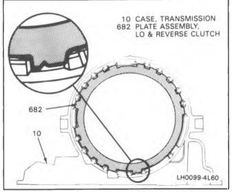
Figure 43 Lo and Reverse Clutch Plates Properly Installed
