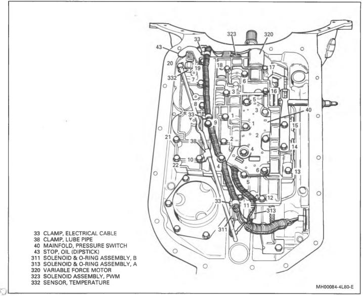
Figure 99 Control Valve Assembly, Bolt Tighten Sequence/Clips and Retainer
