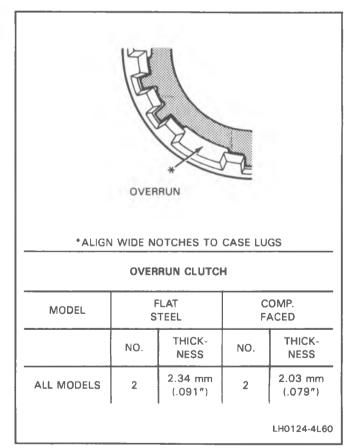
Figure 66 Overrun Clutch Plate Chart
