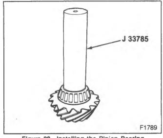
Figure 20-Installing the Pinion Bearing
