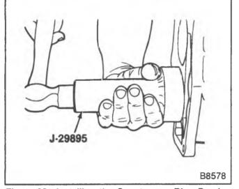
Figure 35-installing the Countergear Ring Bearing
