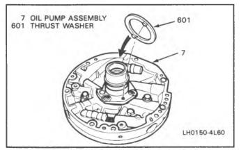
Figure 100 Oil Pump Thrust Washer
