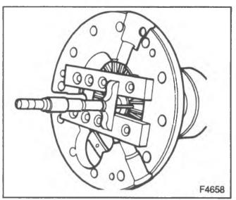
Figure 16-Side Gear Spread
