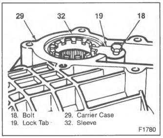
Figure 6—Removing the Lock Tabs
