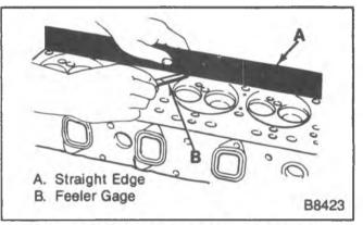
Figure 27—Checking the Cylinder Head for Warpage
