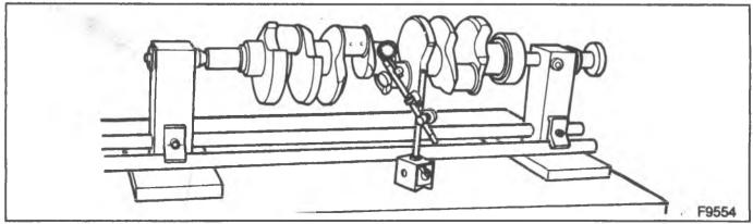
Figure 50—Checking the Crankshaft Run-Out
