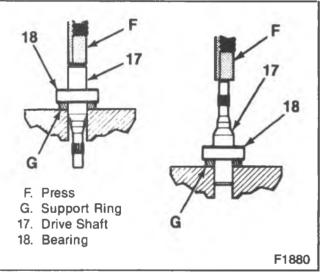
Figure 29—Removing and Installing Driveshaft Bearing
