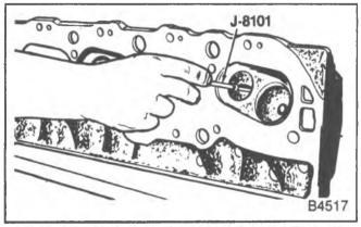
Figure 31-Cleaning the Valve Guides (Typical)
