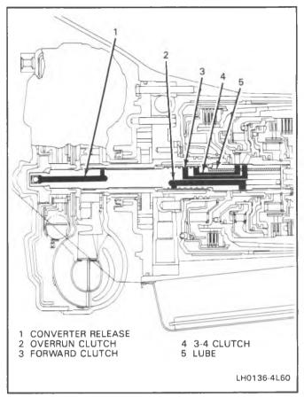
Figure 78 Turbine Shaft Fluid Passages
