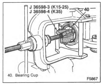
Figure 19-Installing the Outer Pinion Bearing Cup
