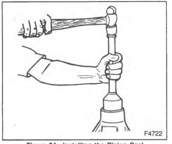
Figure 34—Installing the Pinion Seal
