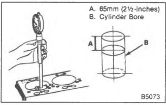
Figure 11—Measuring Cylinder Bore Diameter
