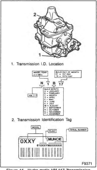
Figure 11—Hydra-matic HM-117 Transmission I.D.Location
