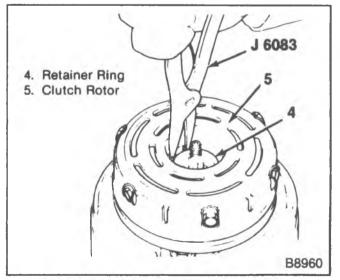
Figure 9-Removing the Retaining Ring
