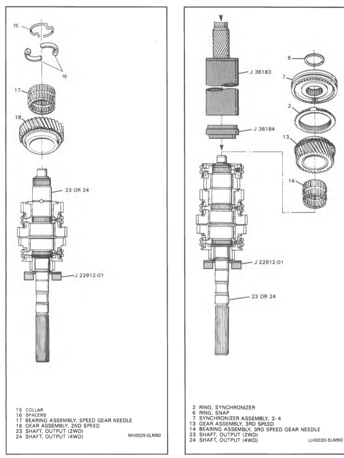
Figure 28 2nd Gear and Components Installed
