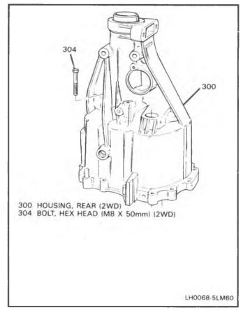
Figure 65 2WD Rear Bearing Retainer Bolts Installation
