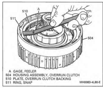
Figure 70 Measuring Overrun Clutch Piston Travel
