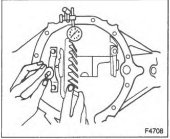
Figure 21—Installing Side Bearing Gaging Tool
