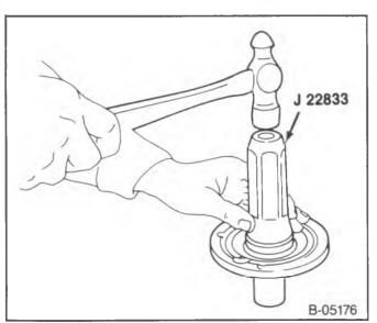
Figure 30 Installing the Drive Gear Bearing Retainer Oil Seal
