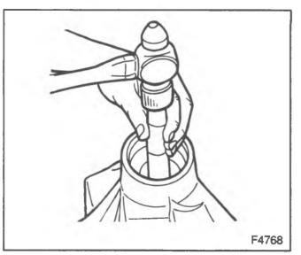
Figure 15—Removing the Bearing Cups
