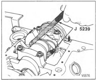
Figure 11—Removing the Connecting Rod and Piston
