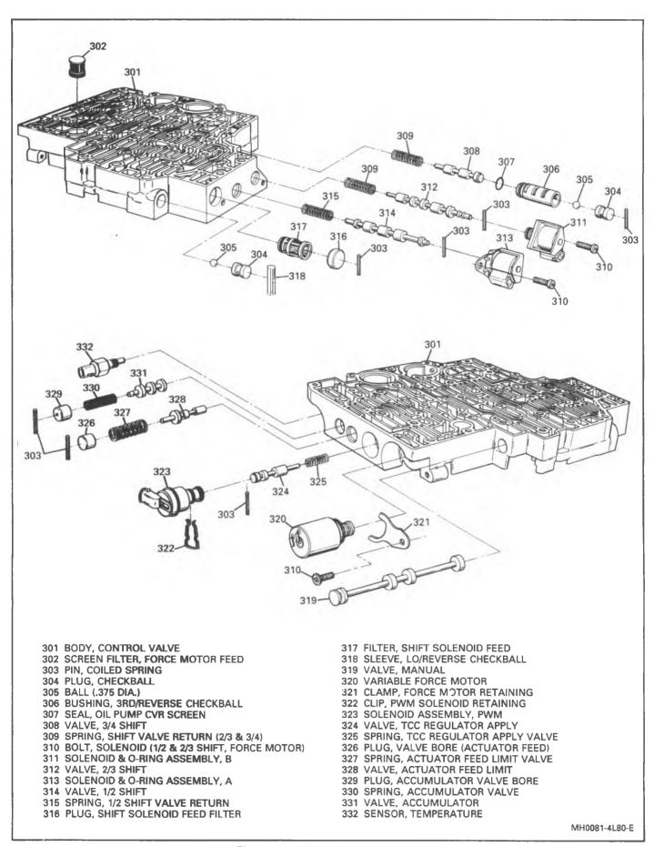
Figure 107 Valve Body Assembly
