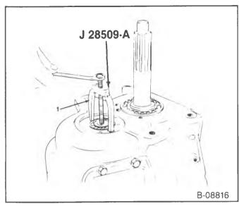
Figure 4 Removing the Countergear Front Bearing
