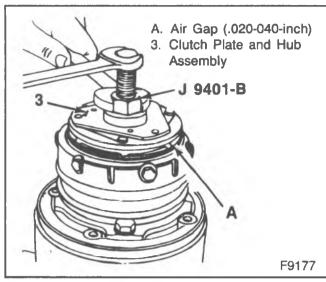
Figure 8---Installing the Clutch Plate and Hub
