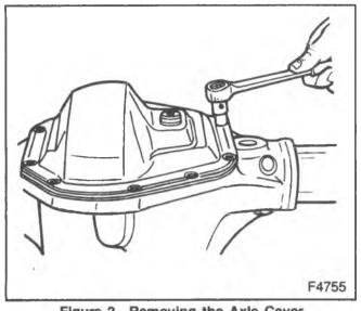
Figure 2-Removing the Axle Cover
