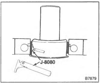
Figure 17—Removing the Upper Main Bearing Insert
