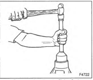
Figure 74—Installing the Pinion Seai
