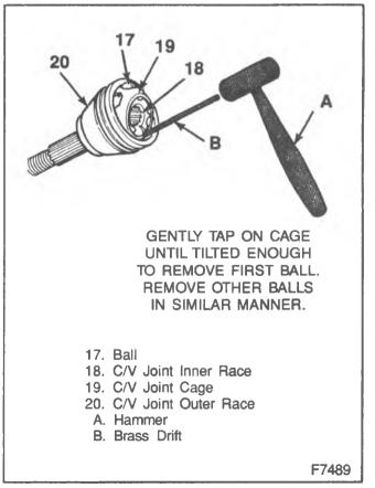
Figure 37—Removing C/V Joint Ball
