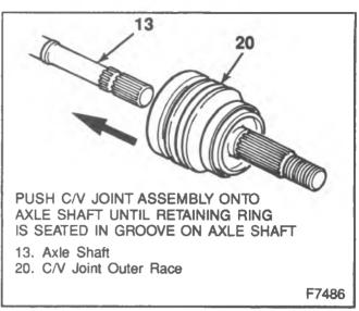
Figure 40-Installing C/V Joint to Axle
