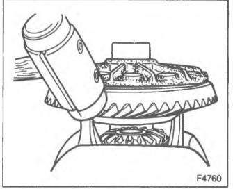
Figure 7-Removing the Ring Gear
