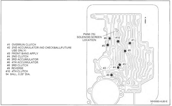
Figure 97 Checkball Location
