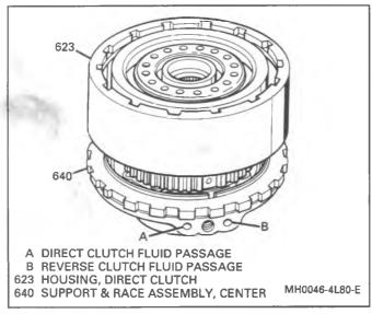
Figure 49 Air Checking Direct Clutch
