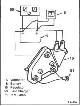
Figure 14—Testing the Voltage Regulator
