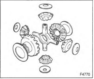
Figure 20-Differential Components
