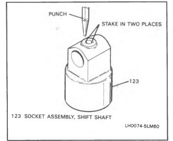
Figure 71 Staking Shift Shaft Socket Assembly
