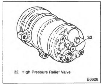
Figure 26-HR-6 HE Compressor Rear Head Detail
