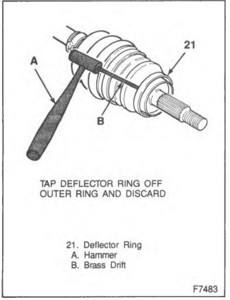
Figure 37—Removing Outer Deflector Ring
