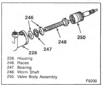
Figure 9—Bearing, Worm and Valve Assembly
