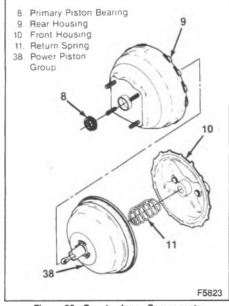
Figure 26—Booster Inner Components
