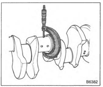
Figure 35—Measuring the Crankshaft Journals
