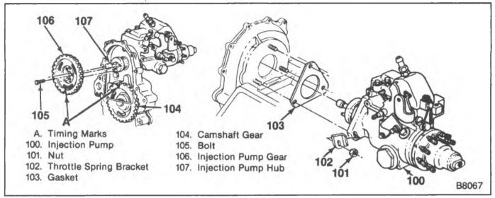
Figure 13—Injection Pump
