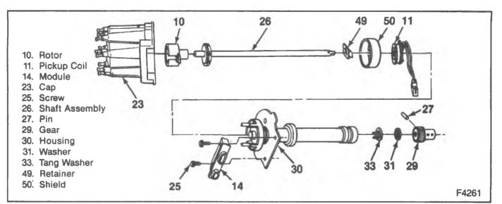
Figure 6—Distributor Components (Separate Coil and Sealed Connector) for an 8-Cylinder Engine
