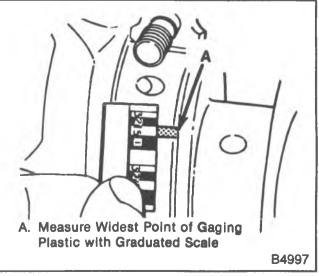
Figure 40—Measuring the Gaging Plastic
