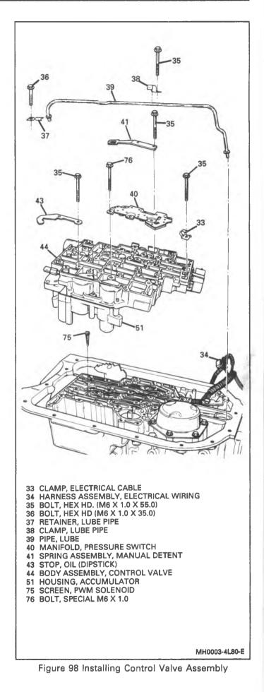
4L80-E-50 HYDRA-MATIC AUTOMATIC TRANSMISSION UNIT REPAIR
