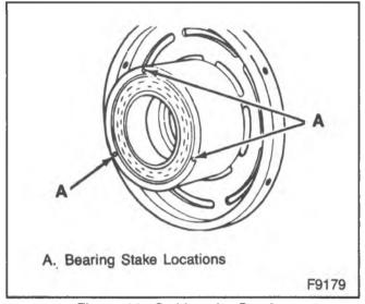
Figure 14---Staking the Bearing
