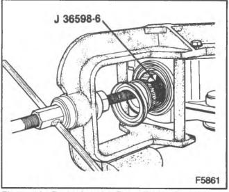
Figure 14—Removing the Outer Pinion Bearing and Seal
