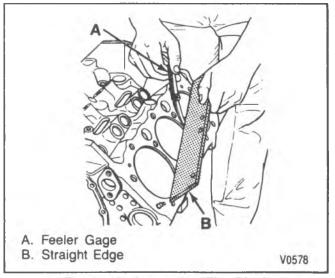
Figure 15—Inspecting The Block
