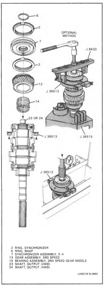
Figure 17 Removing 3-4 Gear Components
