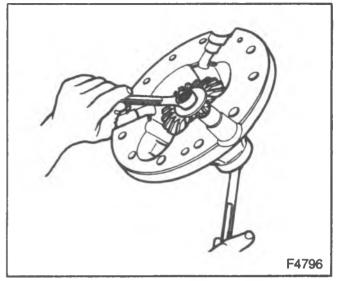
Figure 13—Clamping the Cam Unit in Place
