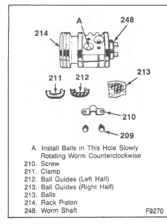
Figure 13-Installing the Balls into the Rack Piston
