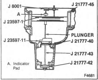
Figure 14-Pinion Depth Tools
