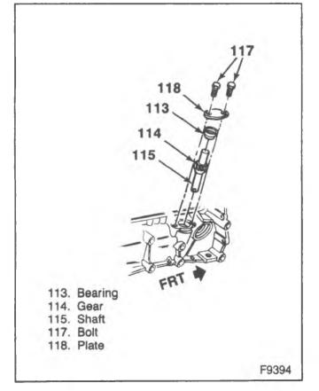
Figure 13-Oil Pump Drive Shaft
