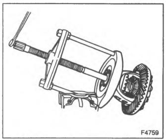
Figure 47-Removing the Differential Side Bearings
