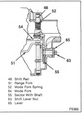
Figure 7-Shift Rail Assembly
