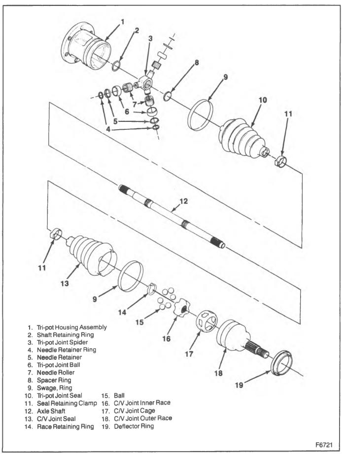
Figure 40—Front Drive Axle Components
