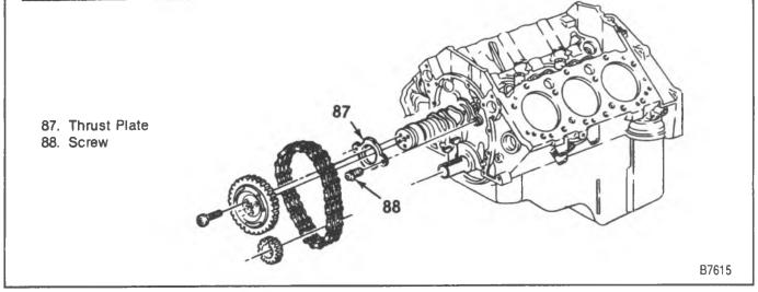
Figure 7—Camshaft and Components
