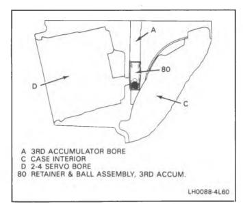
Figure 32 Leak Check — 3rd Accumulator
