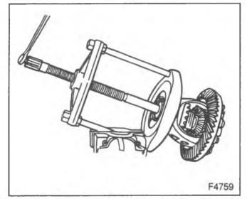
Figure 13-Removing the Differential Side Bearings
