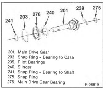
Figure 8 Main Drive Gear Components
