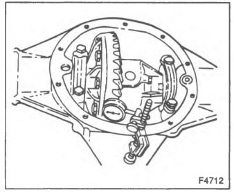
Figure 25—Checking Ring Gear Backlash
