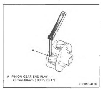
Figure 37 Pinion End Play Check
