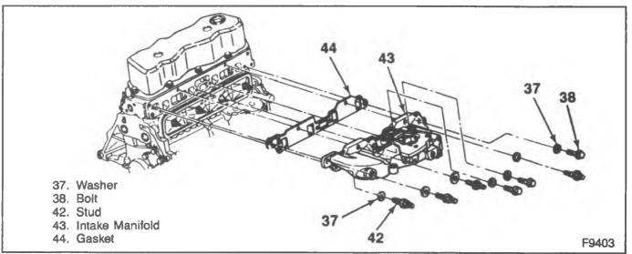
Figure 56-Intake Manifold Installation
