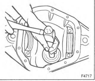
Figure 28-Installing the Pinion Inner Cup
