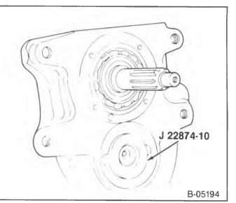
Figure 40 Tool J-22874-10 Installed
