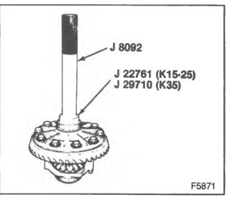
Figure 25—Installing the Differential Side Bearing
