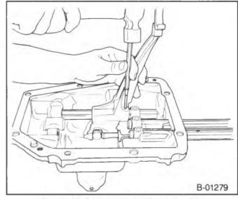
Figure 32 Removing the Retaining Pin
