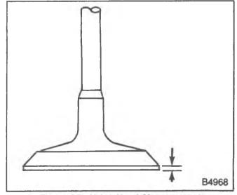
Figure 35—Valve Head Measurement
