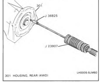
Figure 5 Removing 4WD Oil Seal
