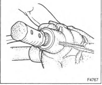
Figure 14—Removing the Pinion
