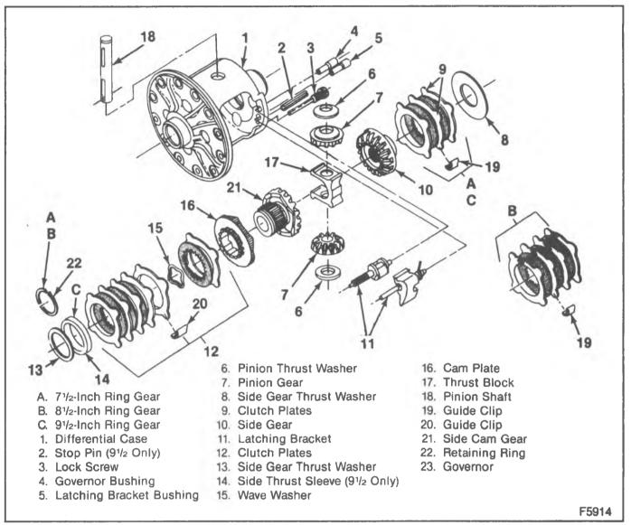
Figure 1—Differential Components
