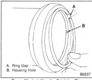
Figure 23—Installing the Retaining Ring
