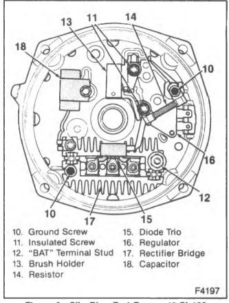
Figure 6—Slip Ring End Frame: 12-Sl 100
