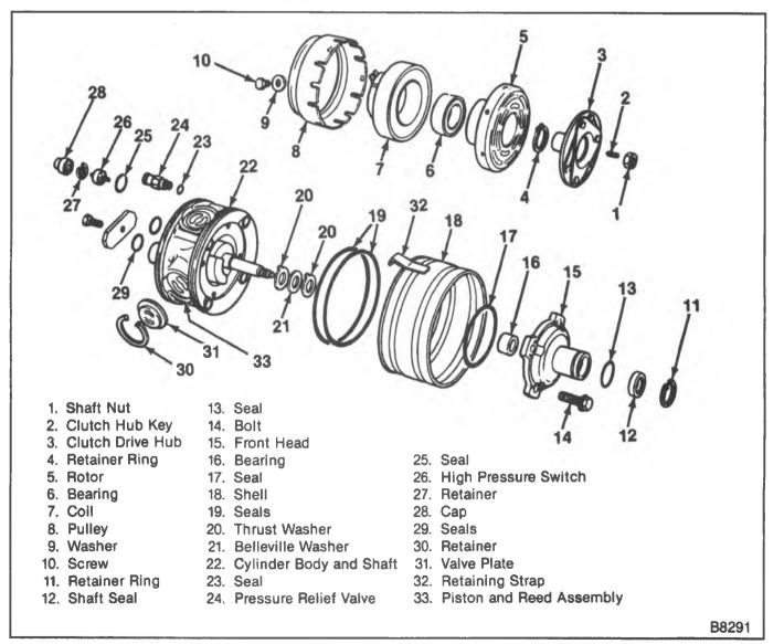
Figure 3—Compressor Component View
