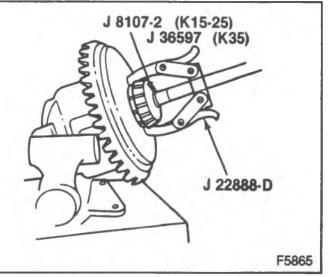
Figure 16-Removing the Side Bearings
