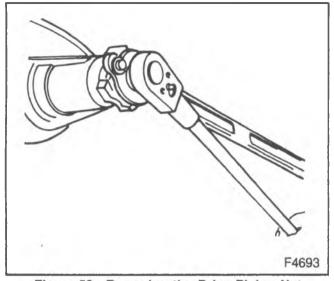
Figure 53—Removing the Drive Pinion Nut
