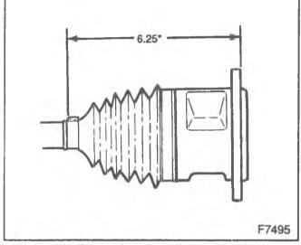
Figure 43—Tri-pot Seal Installation Measurement
