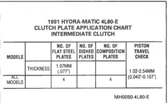
Figure 55 Intermediate Clutch Plate Chart
