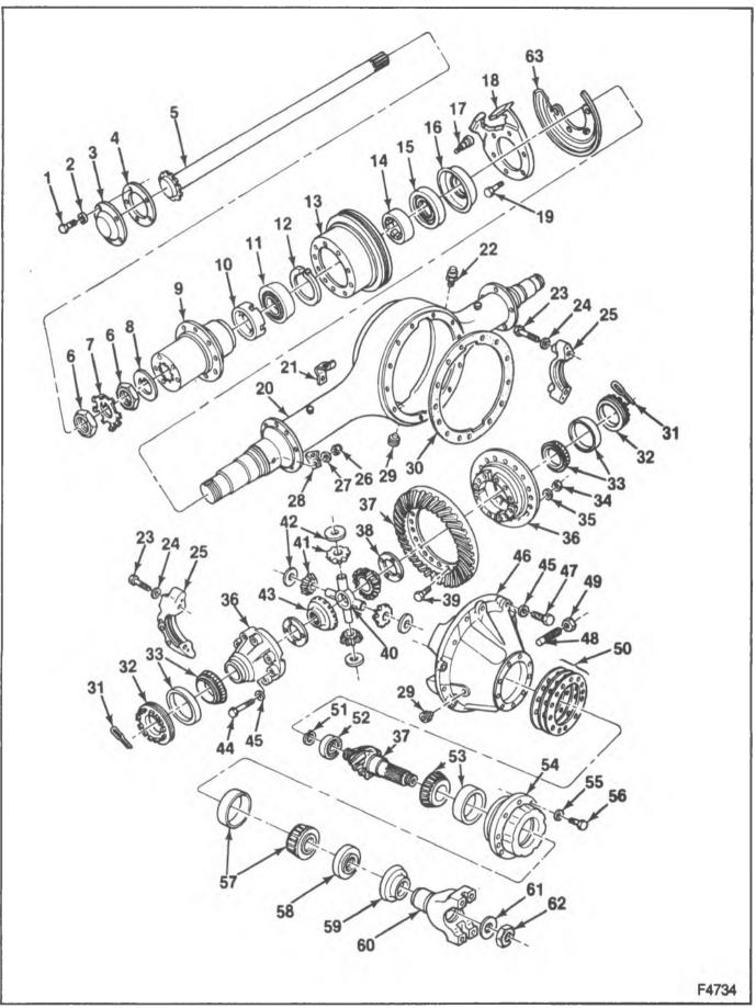
Figure 1—Rear Axle Components
