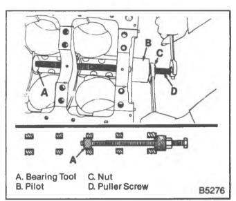
Figure 19—Removing or installing the inner Camshaft Bearings
