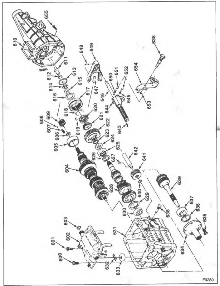
Figure 1-77 mm Transmission and Components
