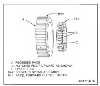
Figure 69 Sprag Assembly Procedure
