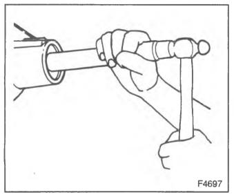
Figure 10-Installing the Front Pinion Bearing Cup
