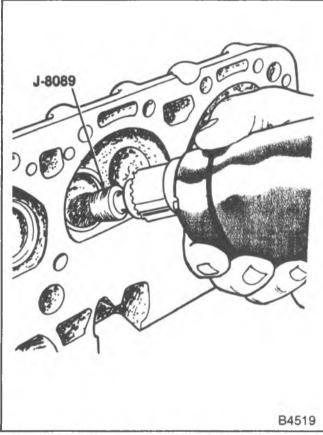
Figure 30—Cleaning the Combustion Chambers (Typical)
