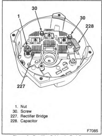
Figure 8-Rectifier Bridge in End Frame
