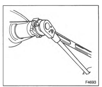
Figure 75-Tightening the Pinion Nut
