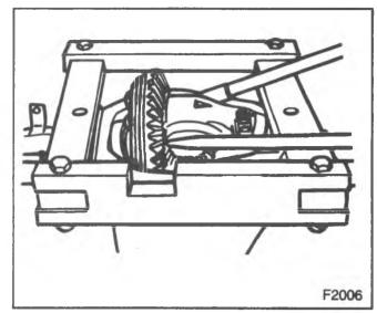
Figure 46—Removing the Differential
