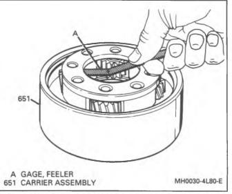
Figure 33 Measuring Reaction Carrier Pinion End Play
