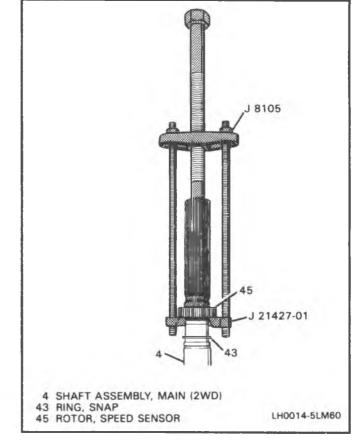
Figure 14 Removing 2WD Speed Sensor Rotor
