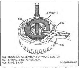
Figure 59 Installing Forward Clutch Piston Release Springs
