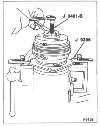
Figure 5-Installing the Drive Plate
