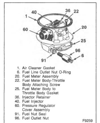
Figure 7—Fuel Meter Assembly—TBI 700
