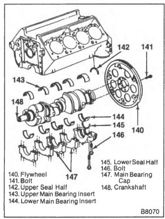
Figure 33—Crankshaft and Components
