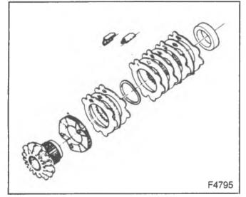
Figure 12—Cam Unit Components
