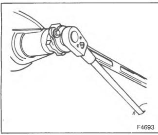
Figure 6—Removing the Drive Pinion Nut
