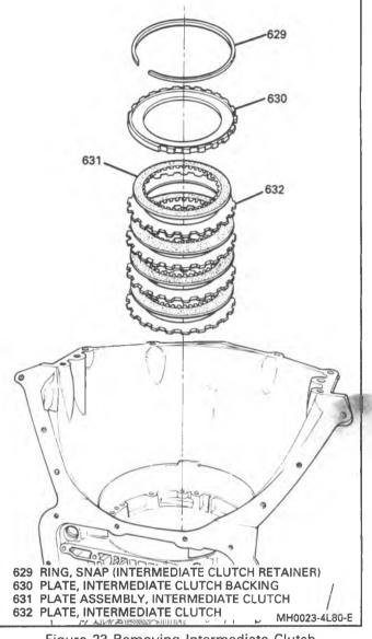
Figure 23 Removing Intermediate Clutch
