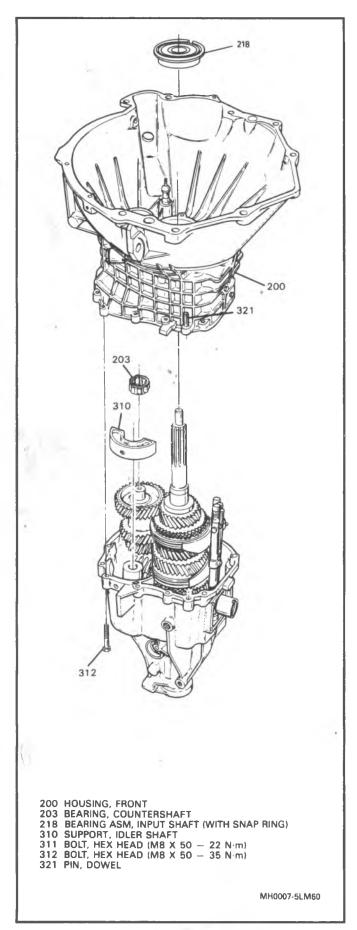
Figure 7 Removing Front Housing
