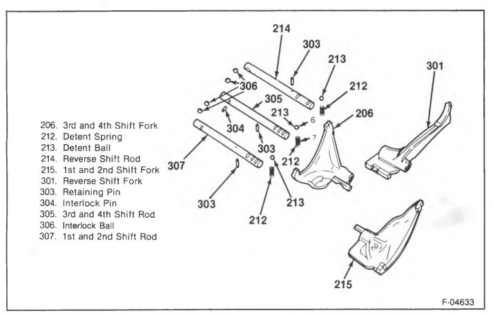
Figure 35 R/V/P Shift Rod and Fork Positions
