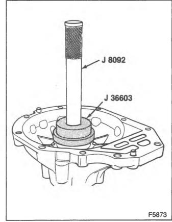
Figure 29---Installing the Side Bearing Cups
