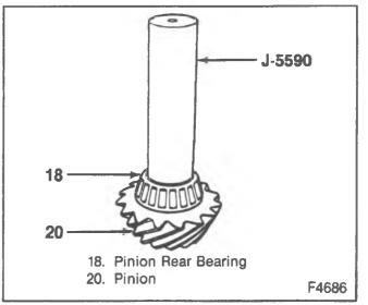
Figure 22-installing the Pinion Inner Bearing
