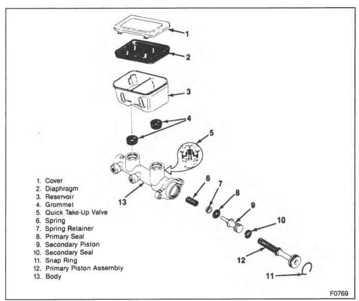
Figure 9—Composite Master Cylinder Components
