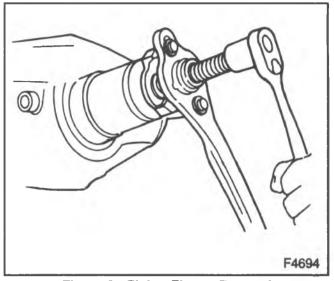
Figure 6—Pinion Flange Removal
