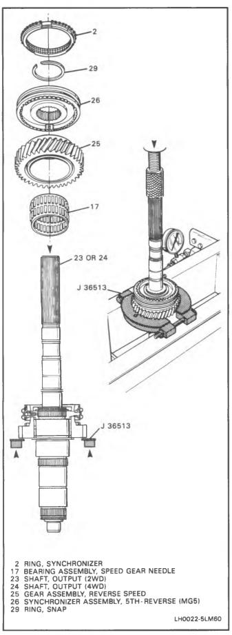
Figure 21 Removing Reverse Gear Components
