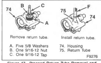
Figure 47—Pressed Return Tube Removal and Installation—Model N
