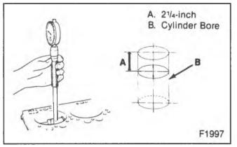
Figure 22—Measuring Cylinder Bore Diameter
