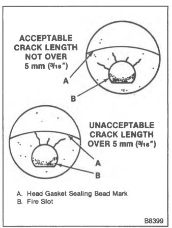
Figure 26-Prechamber Inspection
