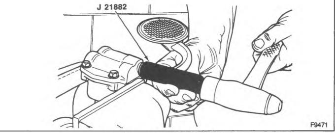
Figure 22-Installing the Oil Pump Screen
