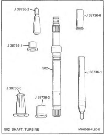
Figure 75 Turbine Shaft Seal Installation
