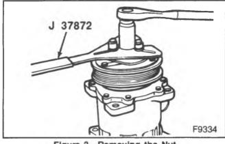
Figure 3—Removing the Nut
