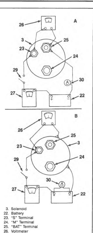
Figure 16-Solenoid Test Connections
