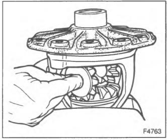
Figure 51-Removing the Pinion Gears
