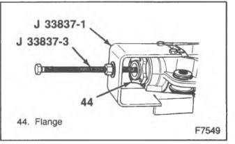
Figure 10-Removing the Pinion Flange
