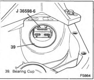
Figure 15-Removing the Inner Bearing Cap
