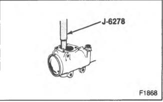
Figure 5-Removing the Pitman Shaft Bearing
