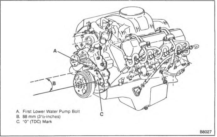
Figure 52—Aligning the Timing Mark
