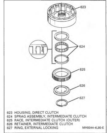
Figure 47 Installing Sprag Assembly
