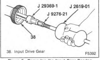
Figure 8-Removing the Input Gear Bearing
