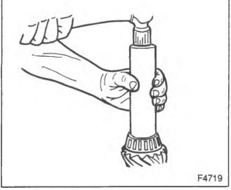
Figure 71—Installing the Inner Bearing
