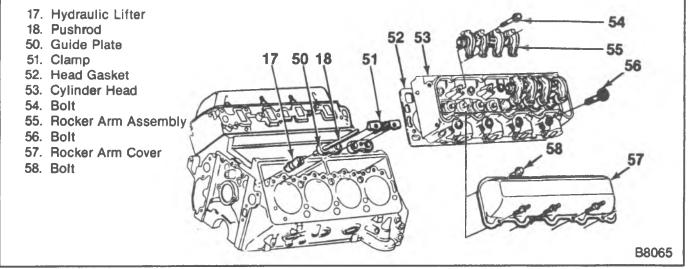
Figure 10—Cylinder Head and Components
