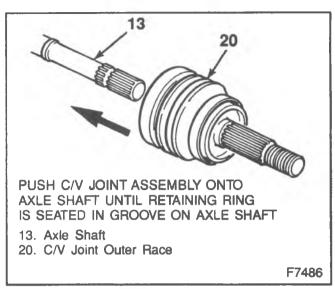
Figure 34-Installing C/V Joint to Axle
