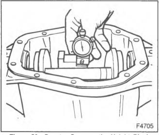
Figure 66—Scooter Gage on the Height Block
