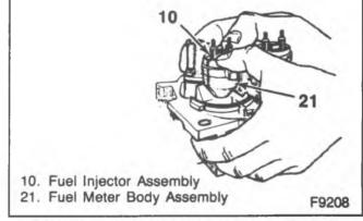
Figure 10-Installing Fuel Injector-TBI 220
