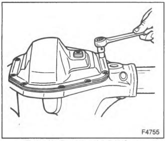
Figure 43-Removing the Axle Cover
