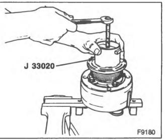
Figure 16—Clutch Rotor and Bearing Removal
