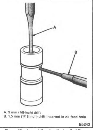
Figure 28—Assembling the Hydraulic Lifter (Typical)
