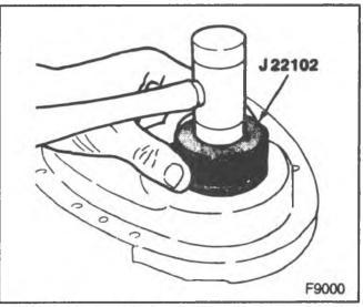
Figure 34-Installing the Front Crankshaft Seal
