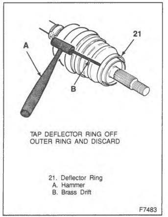
Figure 31—Removing Outer Deflector Ring
