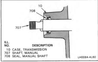
Figure 28 Manual Shaft Seal
