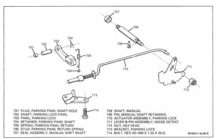
Figure 11 Parking Lock and Actuator Assembly
