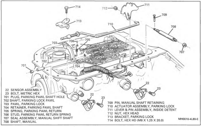
Figure 10 Removing Parking Lock and Actuator Assembly/Speed Sensors
