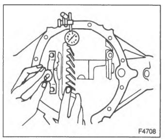
Figure 18—Installing Side Bearing Gaging Tool
