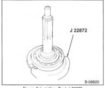
Figure 9 Installing Tool J-22872
