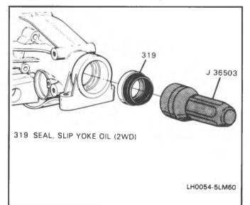
Figure 54 2WD Slip Yoke Oil Seal Installation
