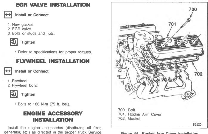
Figure 44—Rocker Arm Cover Installation
