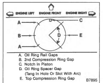
Figure 34—Piston Ring End Gap Locations
