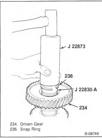
Figure 28 Installing the Driven Gear Snap Ring
