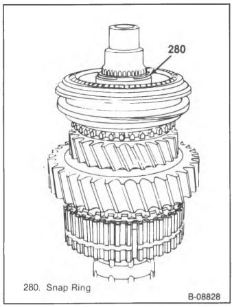
Figure 22 3rd and 4th Synchronizer Hub Snap Ring
