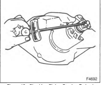
Figure 18—Checking Pinion Bearing Preload
