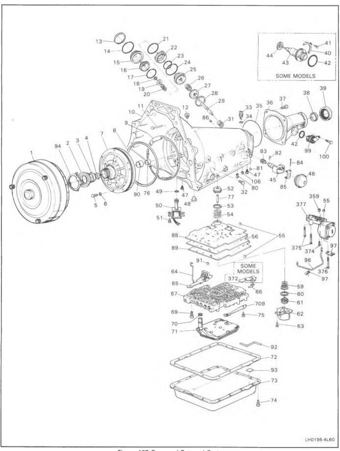
Figure 137 Case and External Parts
