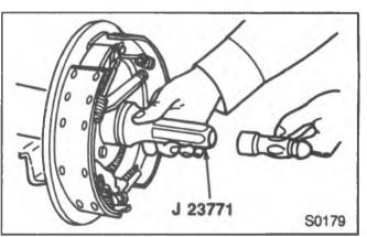
Figure 25-installing the Axle Seal
