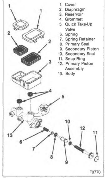
Figure 10—Composite Master Cylinder Components
