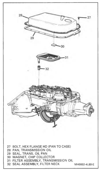
Figure 100 Pan and Filter
