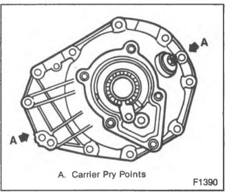
Figure 6—Separating the Carrier Case Halves
