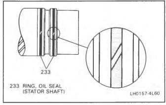
Figure 99 Oil Pump Hub Seal Rings
