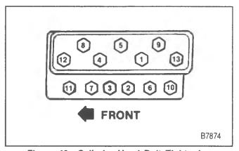
Figure 40—Cylinder Head Bolt Tightening Sequence
