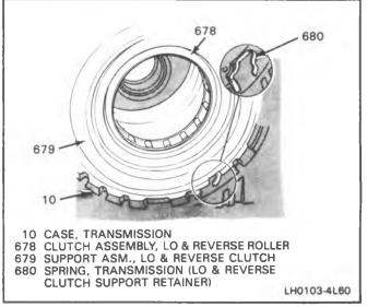
Figure 47 Support Spring — Installed
