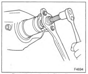
Figure 17-Installing the Pinion Flange
