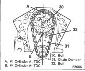
Figure 33—Camshaft Timing Marks
