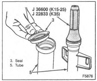
Figure 35-Installing the Axle Tube Seal
