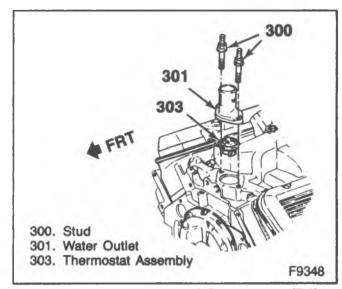
Figure 48—Thermostat and Components (7.4L Engines)
