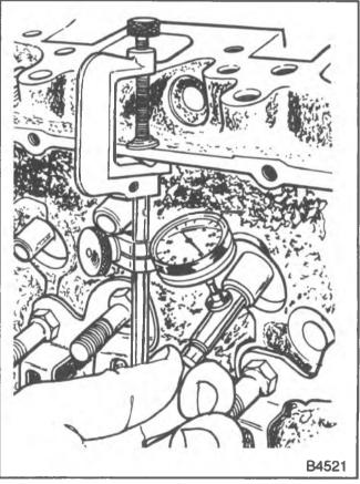
Figure 32—Measuring Stem to Bore Clearance (Typical)
