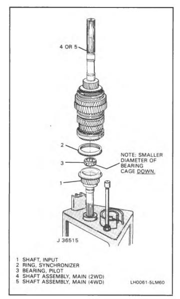
Figure 59 Mainshaft Components Installation
