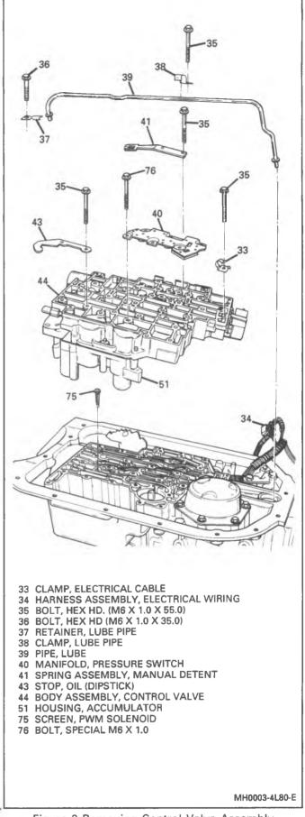
Figure 3 Removing Control Valve Assembly
