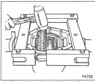
Figure 80-Installing the Differential Case
