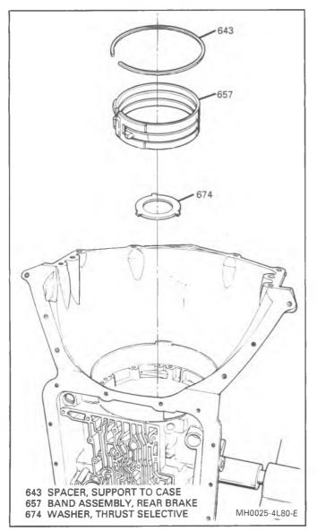
Figure 26 Removing Rear Band and Selective Thrust Washer
