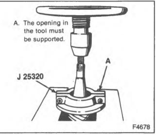
Figure 11-Removing the Pinion Rear Bearing
