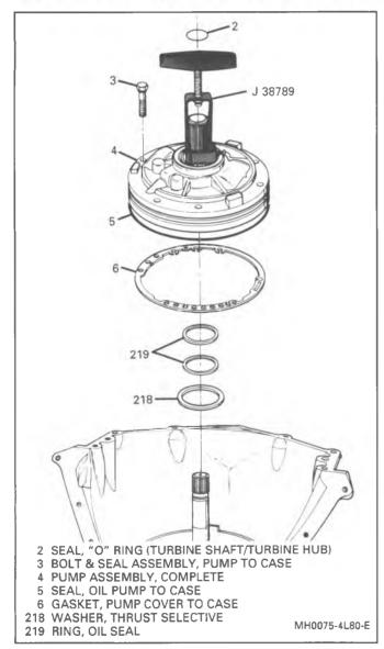
Figure 82 Gasket and Pump Assembly
