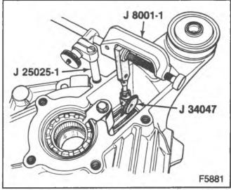
Figure 27-Measuring Backlash at the Ring Gear
