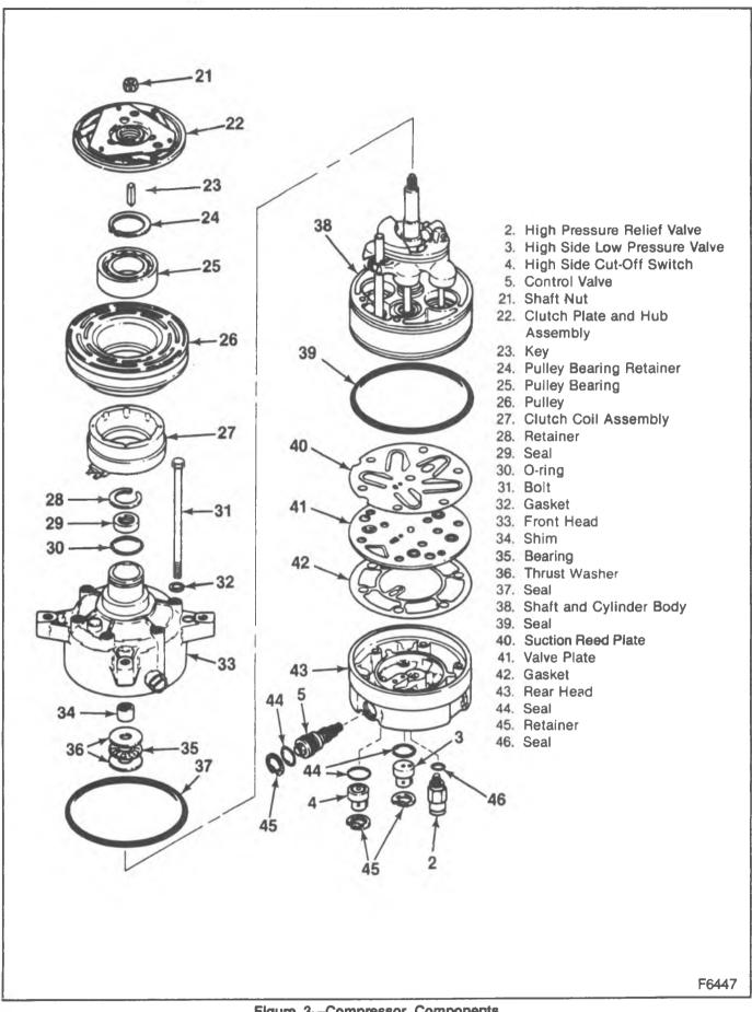
Figure 3---Compressor Components
