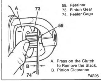
Figure 20—Measuring Pinion Clearance
