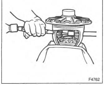
Figure 9—Removing the Pinion Shaft
