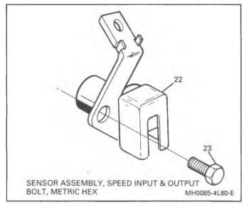
Figure 102 Speed Sensor Assembly
