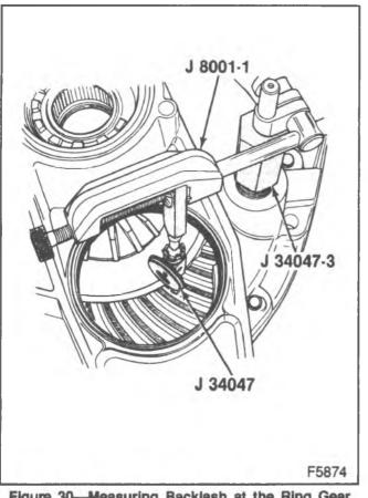
Figure 30-Measuring Backlash at the Ring Gear
