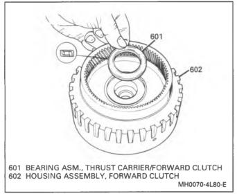
Figure 77 Installing Bearing Assembly
