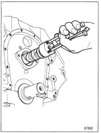
Figure 8—Removing the Camshaft
