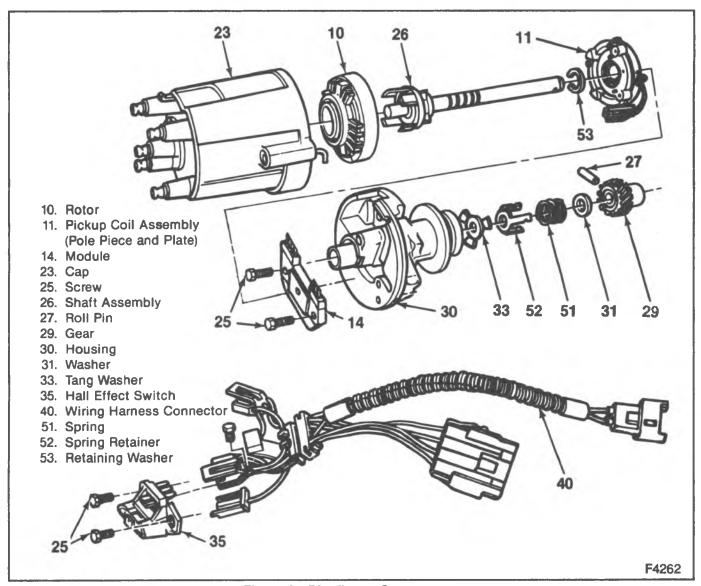
Figure 8—Distributor Components
