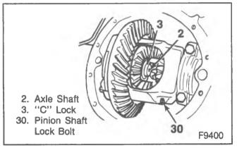
Figure 3—Pinion Shaft Lock Bolt
