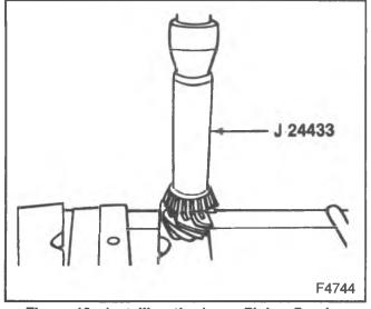
Figure 10-Installing the Inner Pinion Bearing
