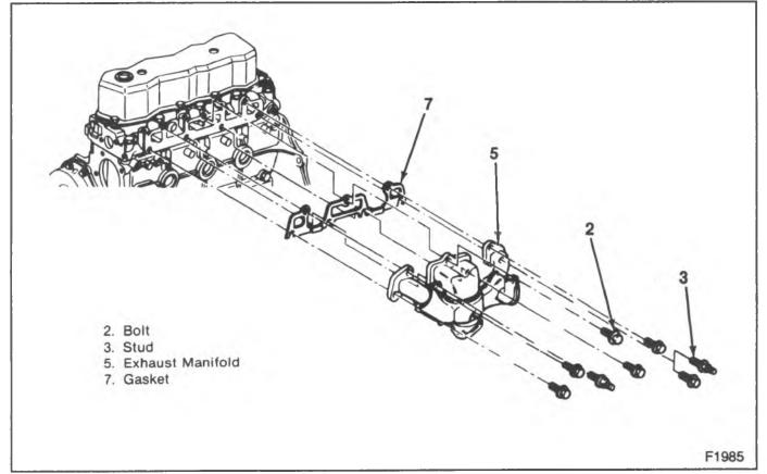
Figure 6—Exhaust Manifold Components
