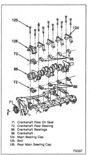
Figure 16-Crankshaft and Bearing Components
