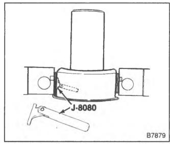
Figure 40-Installing the Upper Main Bearing Insert
