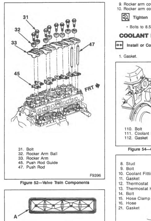
A. Apply A Continuous (5 mm 3/16-Inch) Diameter Bead Of RTV As Shown B7963
