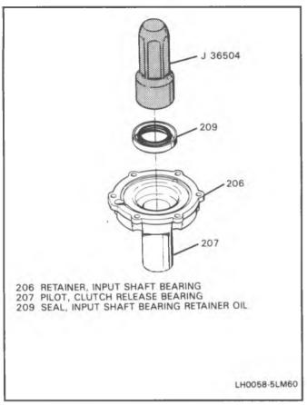
Figure 58 Input Shaft Bearing Retainer Oil Seal Installation
