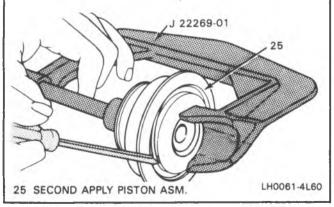
Figure 123 2nd Servo Piston — Assembly
