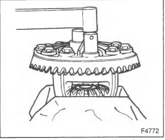
Figure 20-Installing the Ring Gear Bolts
