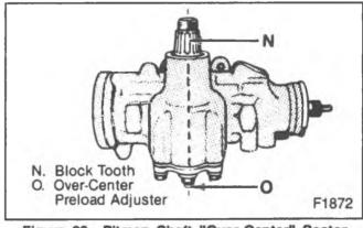
Figure 20—Pitman Shaft "Over-Center" Sector Adjustment
