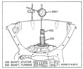
Figure 12 Front Unit End Play Check
