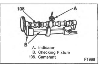
Figure 23----Measuring Camshaft Journal Runout
