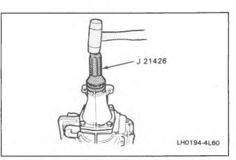
Figure 135 Case Extension Oil Seal Assembly
