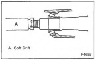
Figure 8—Removing the Drive Pinion
