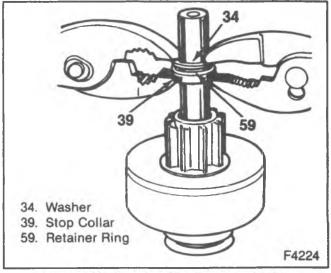
Figure 18—Forcing the Collar over the Retainer Ring
