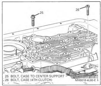
Figure 25 4th Clutch Bolt and Center Support Bolt Location
