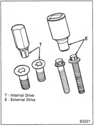
Figure 22—Six Lobed Socket Head Fasteners
