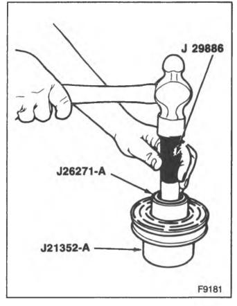
Figure 18—Bearing Installation
