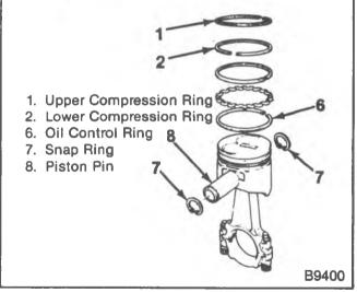
Figure 7---Piston and Components---6.2L Engine
