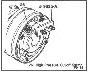
Figure 25-Compressor Leak Testing
