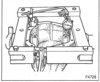
Figure 39—Mounting the Carrier Spreader
