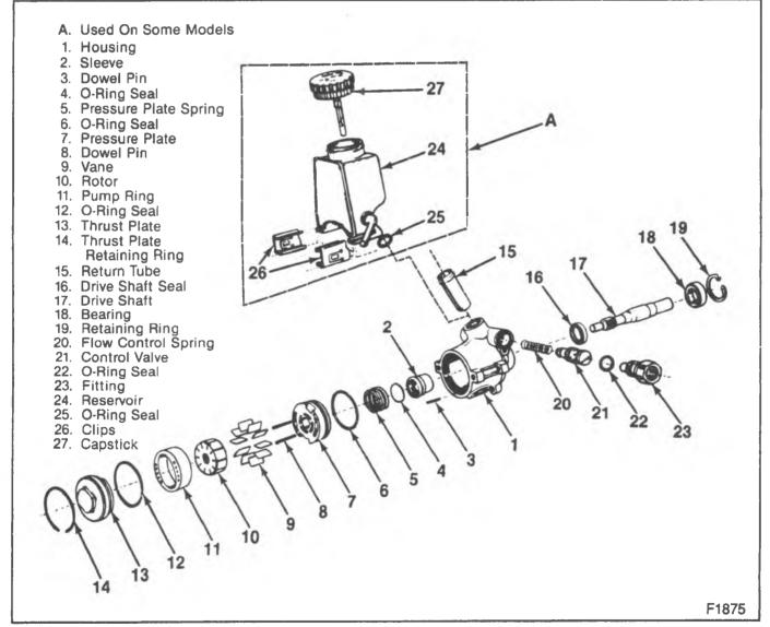
Figure 24—Power Steering (TC SERIES) Pump Components
