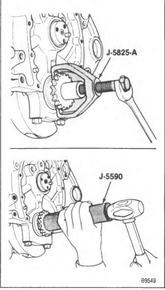
Figure 18—Replacing the Crankshaft Sprocket
