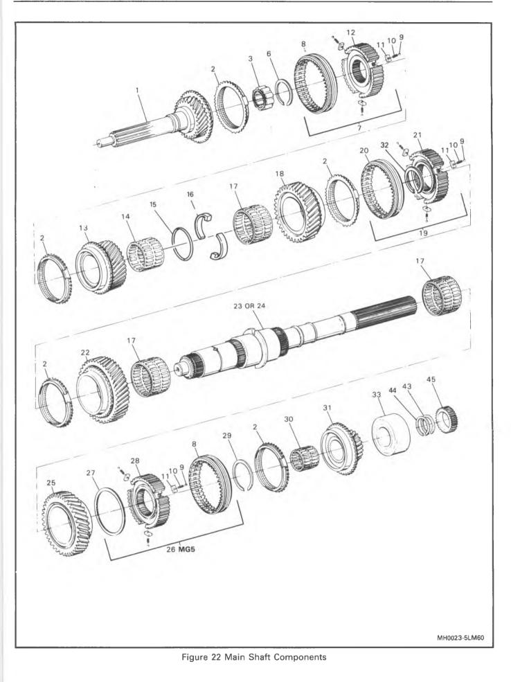
1 SHAFT, INPUT 2 RING, SYNCHRONIZER **3 BEARING, PILOT** 6 RING, SNAP (SELECTIVE) 7 SYNCHRONIZER ASSEMBLY, 3-4 8 SLEEVE, SYNCHRONIZER 9 BALL, SYNCHRONIZER DETENT 10 SPRING, SYNCHRONIZER DETENT 11 KEY, SYNCHRONIZER 12 HUB, 3-4 SYNCHRONIZER 13 GEAR ASSEMBLY, 3RD SPEED **14 RETAINER RING** 15 THRUST WASHER 16 SPACERS 17 BEARING ASSEMBLY, SPEED GEAR NEEDLE 18 GEAR ASSEMBLY, 2ND SPEED 19 SYNCHRONIZER ASSEMBLY, 1-2 19 SYNCHRONIZER ASSEMBLY, 1
