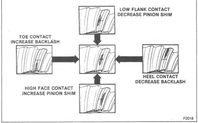
Figure 30-Gear Tooth Pattern
