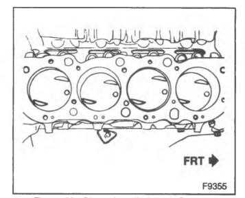
Figure 66—Piston Installed (7.4L Engines)
