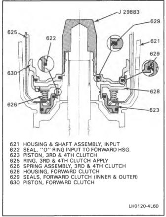
Figure 62 Forward Clutch and 3-4 Apply Ring --Installed
