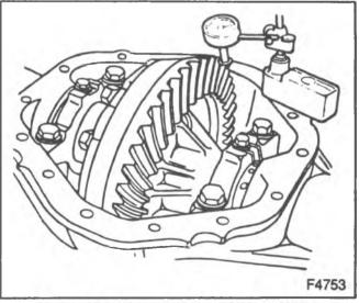
Figure 19-Measuring Gear Set Backlash
