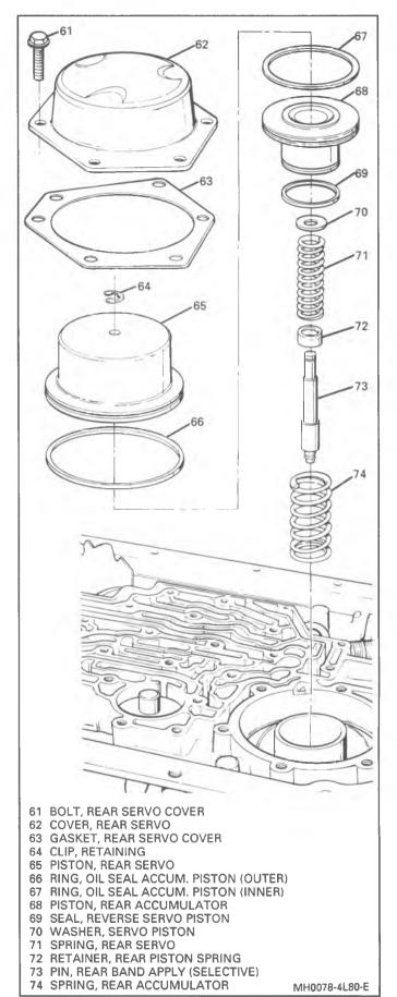
Figure 92 Installing Rear Servo
