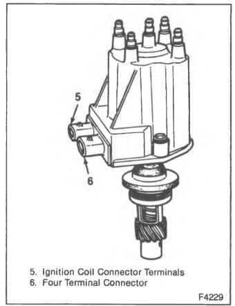
Figure 2—Distributor with Separate Coll and Sealed Connectors
