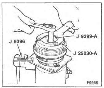
Figure 2-Removing the Shaft Nut
