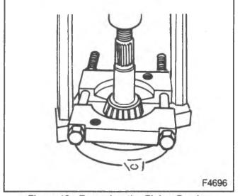
Figure 13—Removing the Pinion Bearing
