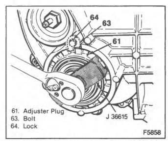
Figure 28—Turning the Adjuster Plug (K3 Models)
