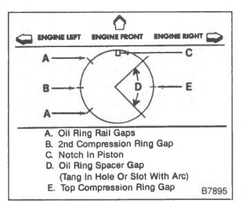
Figure 46—Piston Ring Gap Location
