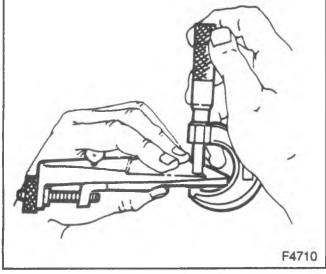
Figure 21-Measuring the Gage Plate Thickness
