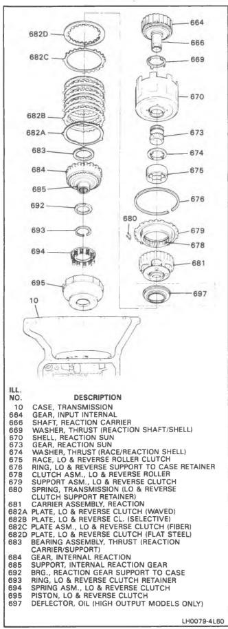
Figure 23 Reaction Gear Set Removal
