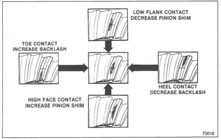
Figure 33—Gear Tooth Contact Pattern
