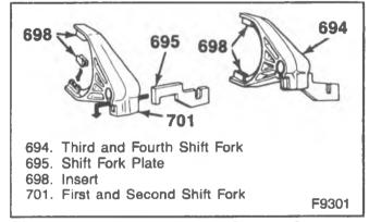
Figure 31-Shift Forks and Selector Plates
