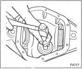
Figure 69-Installing the Pinion Inner Cup
