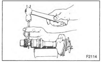
Figure 7—Removing the Roll Pin
