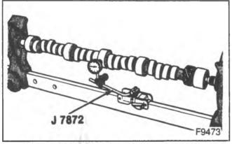
Figure 30—Measuring Camshaft Run-Out
