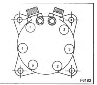
Figure 16-Torque Sequence
