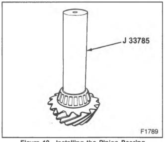
Figure 19—Installing the Pinion Bearing
