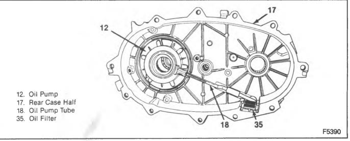
Figure 7-Oil Pump Assembly
