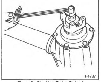
Figure 3—Checking Pinion Preload
