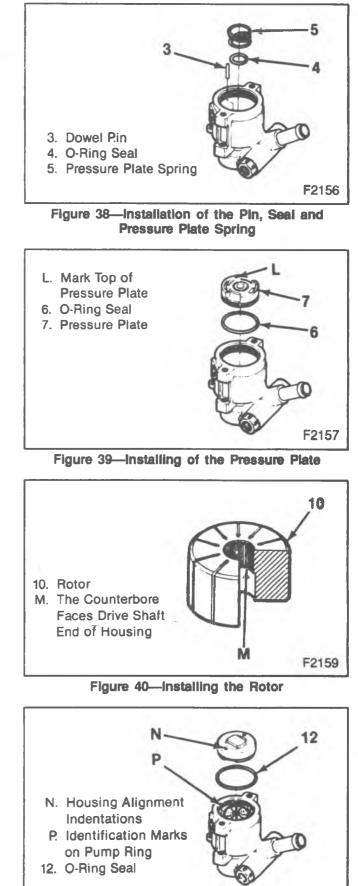
Figure 41-Aligning and Installing the Pump Ring
