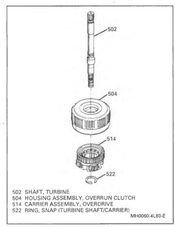
Figure 67 Overdrive Unit Assembly
