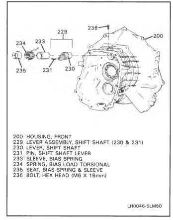
Figure 45 Bias Spring Component Installation
