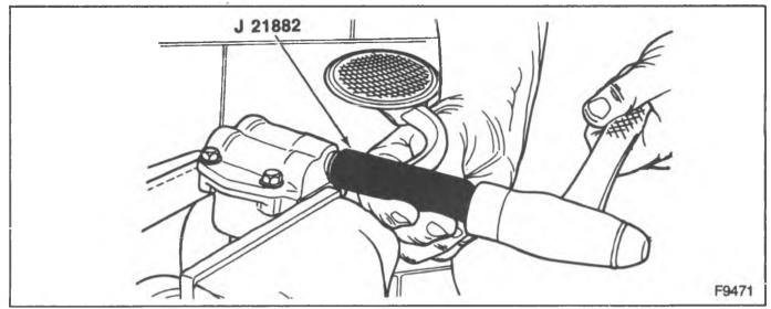
Figure 37-Installing the Oil Pump Pickup Tube and Screen (5.0L and 5.7L Engines)
