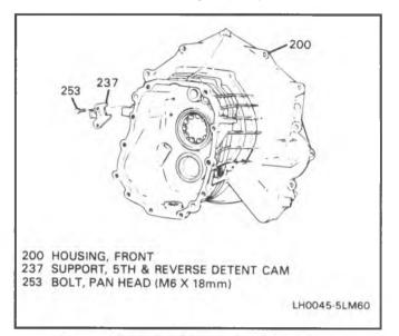
Figure 44 Detent Component Installation
