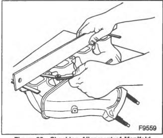
Figure 29—Checking Alignment of Manifold Flanges
