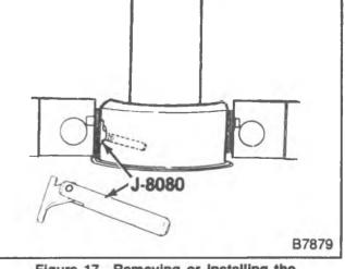
Figure 17—Removing or Installing the Main Bearing Insert
