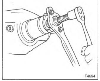
Figure 16—Installing the Pinion Flange
