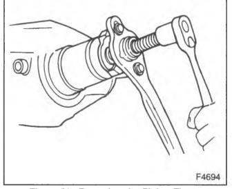
Figure 54—Removing the Pinion Flange
