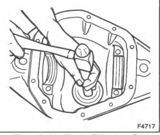
Figure 29—Installing the Pinion Inner Cup
