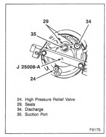
Figure 4---Compressor in Holding Fixture
