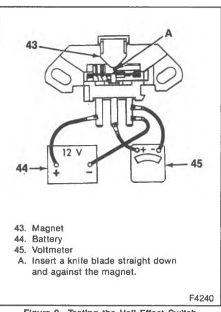
Figure 9----Testing the Hall Effect Switch
