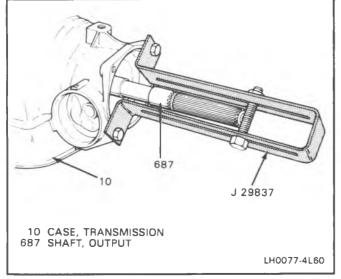
Figure 52 Output Shaft — Installation
