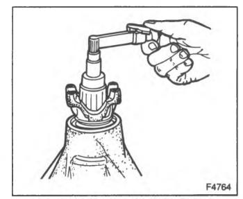
Figure 11-Checking the Pinion Preload
