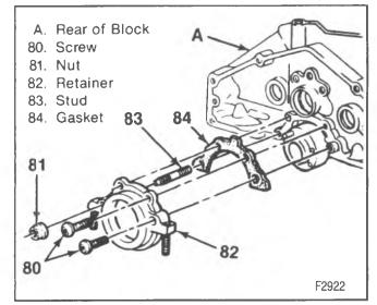
Figure 13-Rear Crankshaft Oil Seal Retainer
