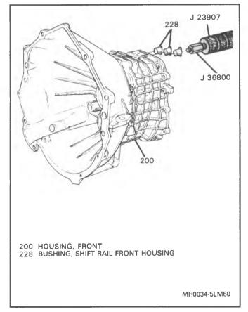
Figure 33 Removing Shift Rail Bushings
