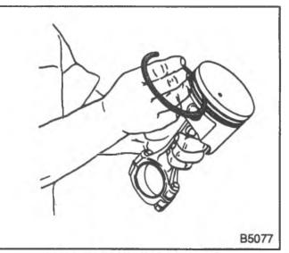
Figure 17-Checking Ring Fit
