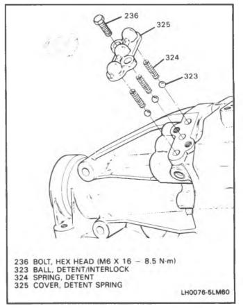
Figure 73 Detent Components Installation
