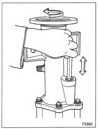
Figure 39—Checking the Shift Mechanism
