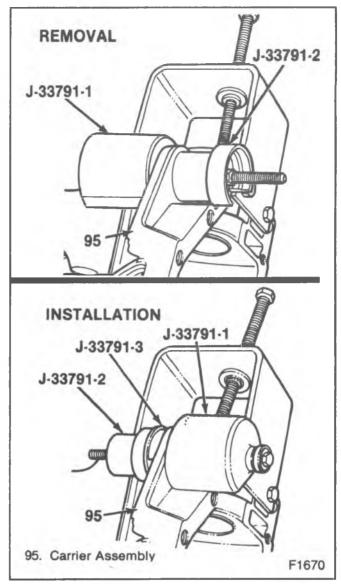
Figure 14—Replacing the Case Bushings
