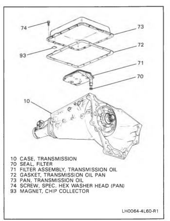
Figure 8 Pan, Filter & Seal Remove
