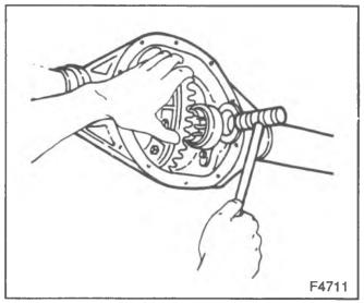
Figure 24—Installing the Final Preload Shim
