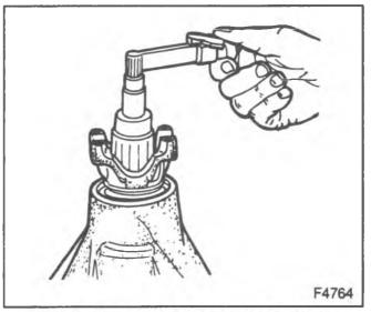
Figure 11-Checking the Pinion Preload
