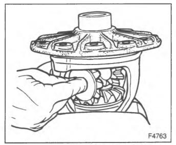
Figure 17-Installing the Pinion Gears
