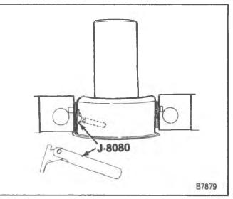
Figure 14—Removing the Main Bearing Insert
