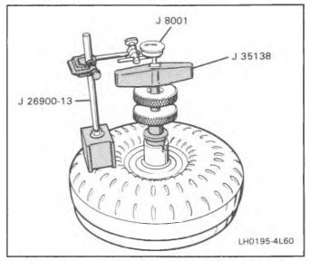
Figure 136 Checking Torque Converter End Play
