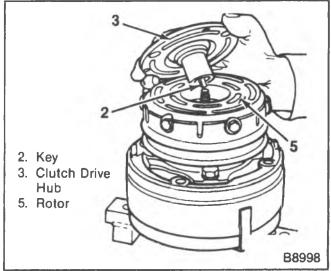
Figure 7-Installing the Shaft Key
