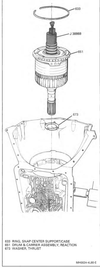
Figure 24 Removing Center Support and Gear Unit Assembly
