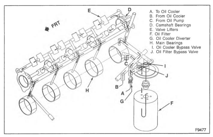
Figure 3—Lubrication Diagram (7.4L Engines)
