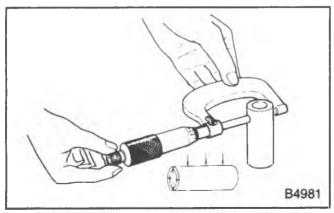
Figure 8—Measuring Piston Pin Diameter
