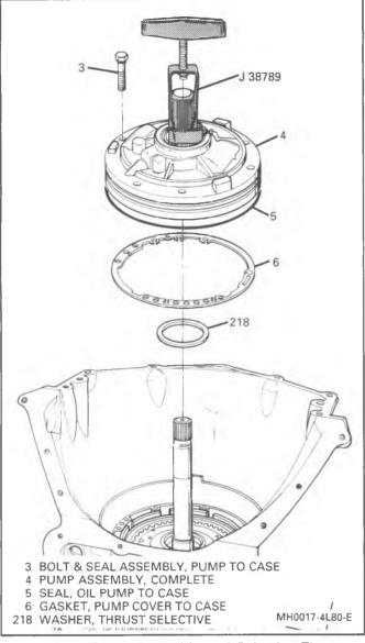
Figure 17 Pump Assembly and Selective Thrust Washer
