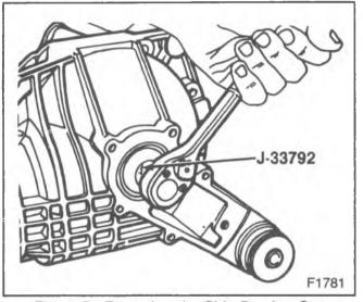
Figure 7-Removing the Side Bearing Cup
