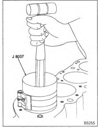
Figure 47-Installing the Piston
