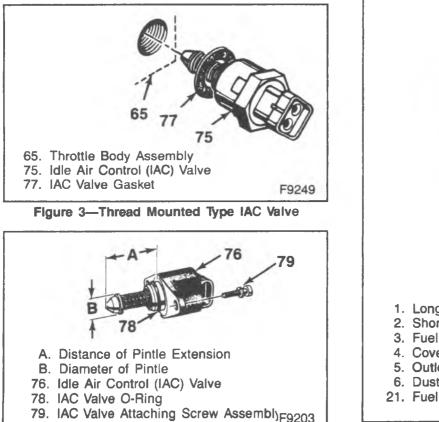
Figure 4—Flange Mounted Type IAC Valve
