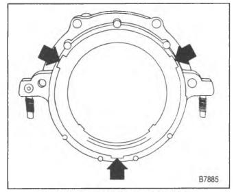
Figure 12-Seal Removal Notches
