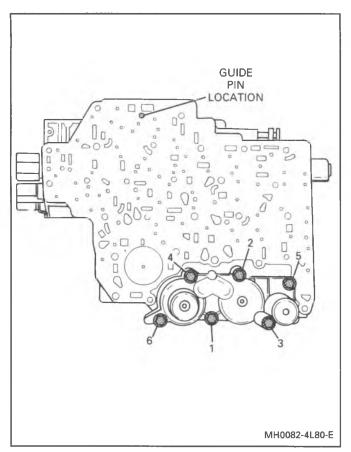
Figure 96 Torque Sequence & Guide Pin Location
