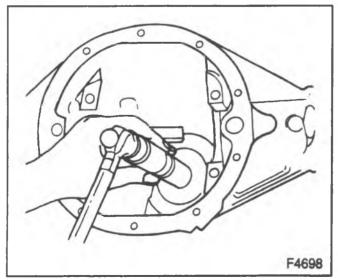
Figure 11---Installing the Rear Pinion Bearing Cup
