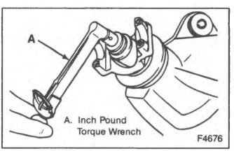
Figure 23—Checking Pinion Preload
