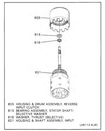
Figure 89 Reverse Input and Input Clutches
