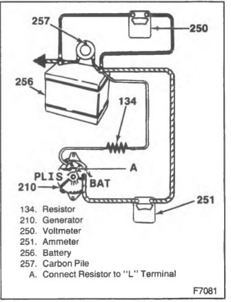
Figure 3—Connections for Generator Output Test
