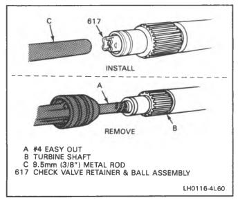
Figure 58 Retainer and Ball Assembly — Replacement
