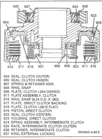
Figure 48 Direct and Intermediate Sprag Clutch Assembly
