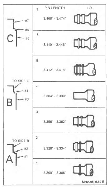
Figure 8 Band Apply Pin Selection Chart
