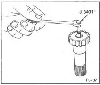
Figure 4—Removing the Output Shaft Pilot Bearing
