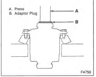
Figure 16-Installing the Ring Gear to Case
