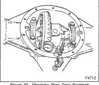
Figure 23—Checking Ring Gear Backlash
