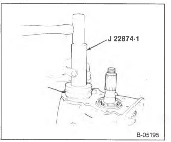
Figure 41 Installing the Countergear Rear Bearing
