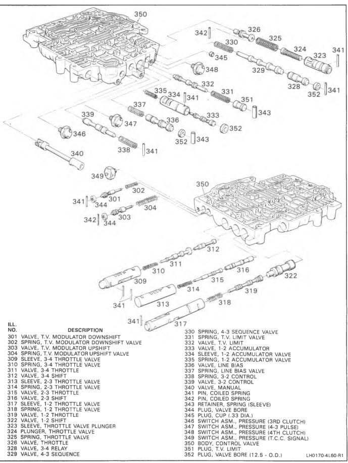
Figure 141 Control Valve Assembly
