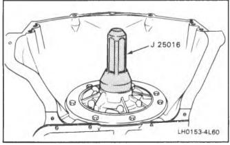
Figure 95 Oil Pump Seal
