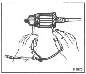
Figure 15—Testing the Armature for Grounds
