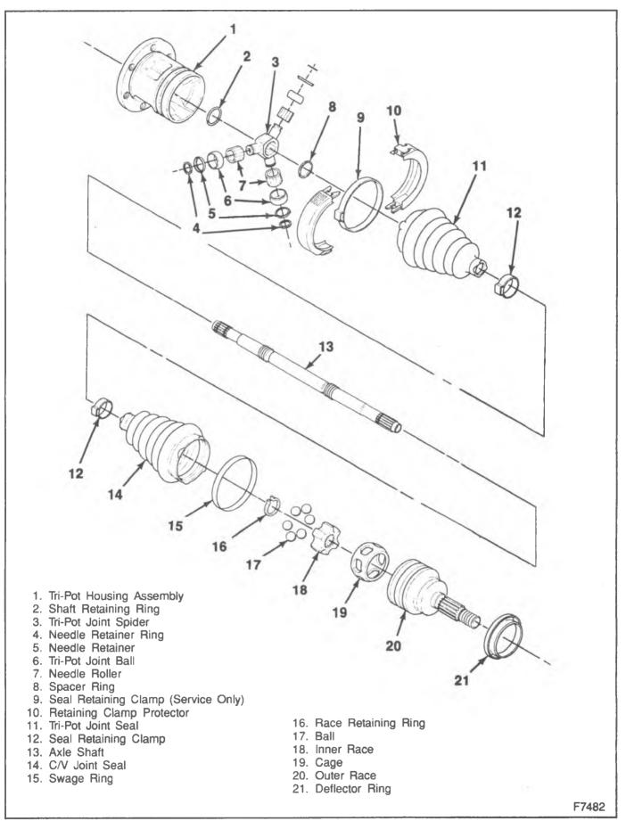
Figure 30—Front Drive Axle
