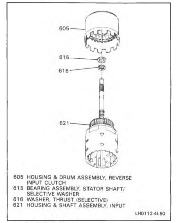
Figure 54 Reverse Input and Input Clutches
