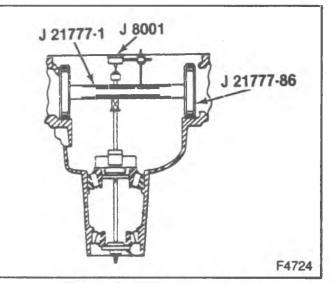
Figure 13—Pinion Depth Tools
