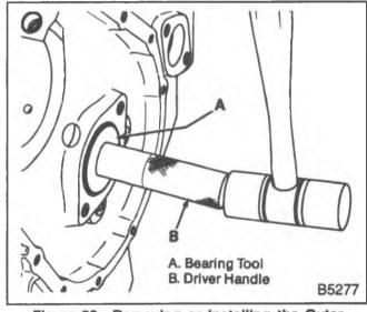
Figure 20—Removing or Installing the Outer Camshaft Bearings
