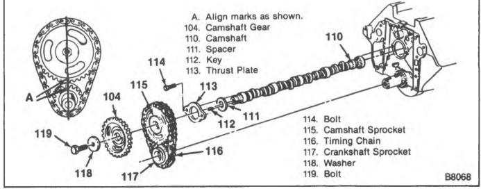
Figure 41—Camshaft and Components
