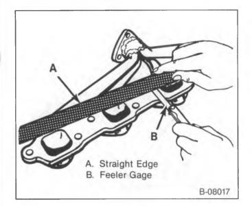
Figure 28—Checking Alignment of Manifold Flanges (Typical)
