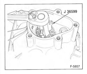
Figure 28—Turning the Adjuster Sleeve
