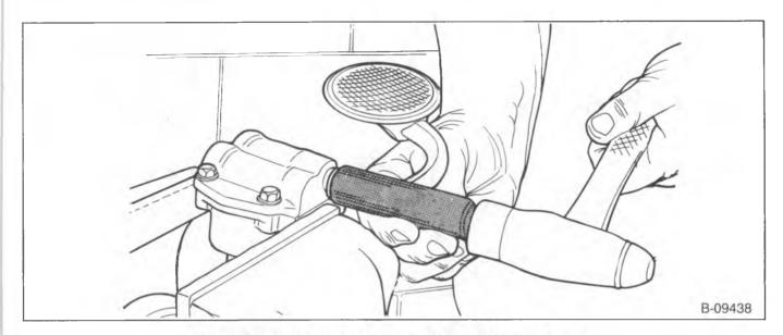
Figure 36—Installing the Oil Pump Pickup Tube and Screen
