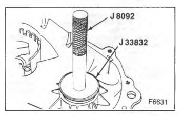
Figure 24—Installing the Front Output Bearing
