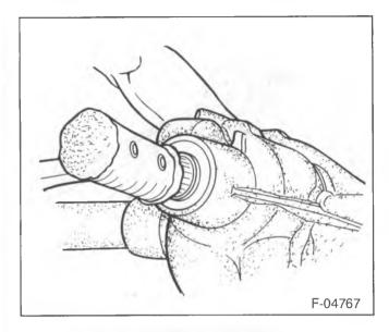
Figure 55—Removing the Pinion
