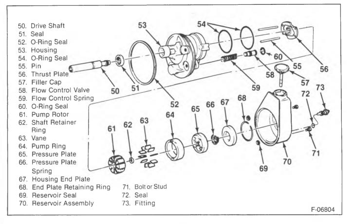
Figure 46—Power Steering Pump—Model P
