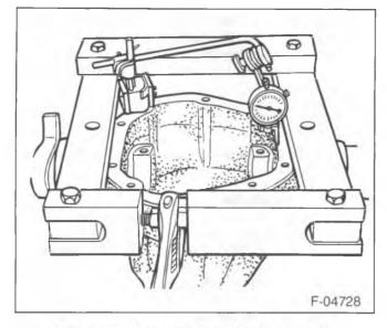
Figure 79—Mounting the Carrier Spreader
