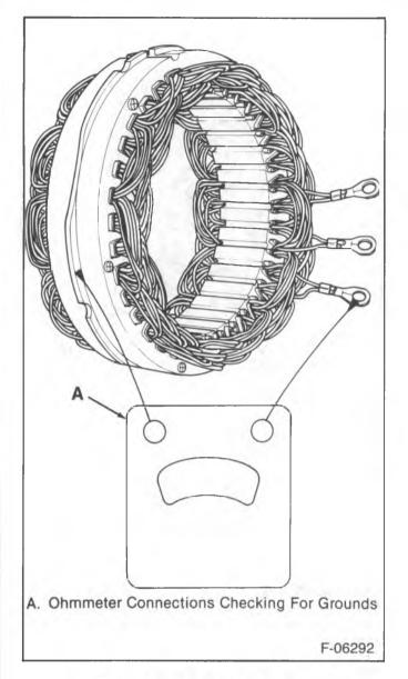
Figure 11—Checking the Stator
