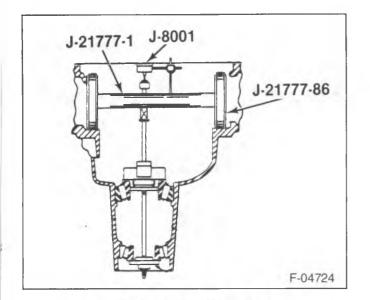
Figure 12—Pinion Depth Tools
