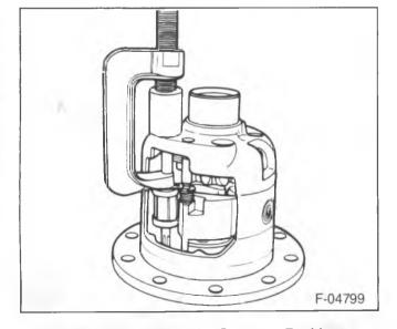
Figure 2—Removing the Governor Bushings
