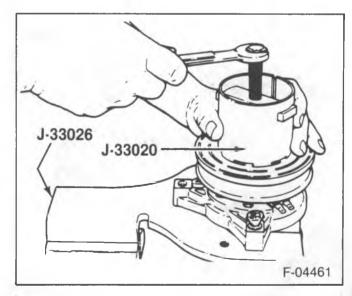
Figure 11 — Installing J-33020 in the Pulley Rotor Slots
