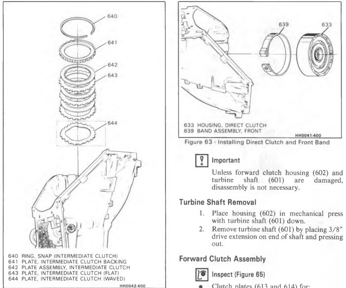
Figure 61 Intermediate Clutch Plates
