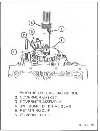
Figure 11 Speedometer Drive Gear and Governor
