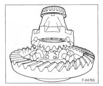
Figure 8—Differential Case Halves
