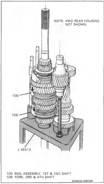
Figure 17 Locking Up Transmission
