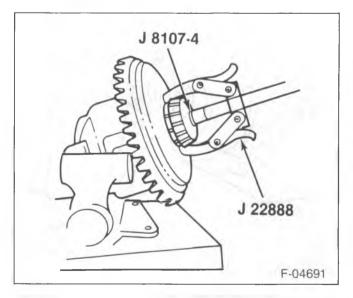
Figure 3-Removing Differential Side Bearing
