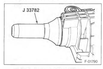
Figure 21-Installing the Pinion Seal
