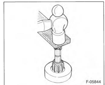
Figure 14—Forcing the Stop Ring on the Shaft
