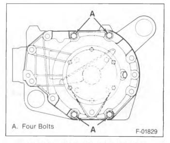
Figure 25—Carrier Case Bolts Installed
