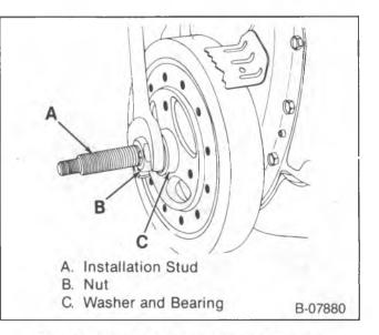
Figure 61—Installing the Torsional Damper
