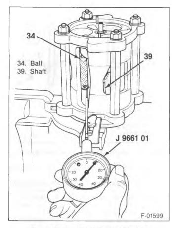
Figure 32—Gaging the Rear Piston Ball
