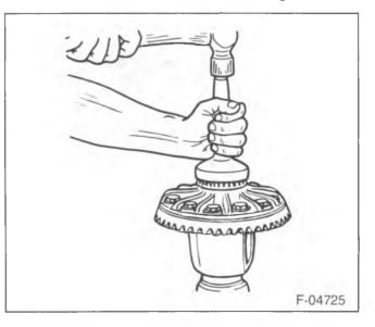
Figure 78—Installing the Differential Bearings
