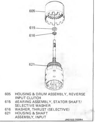
Figure 55 Reverse Input and Input Clutches
