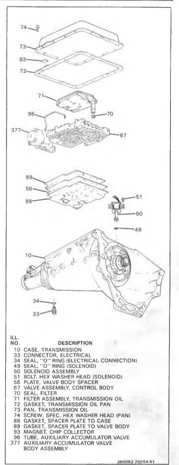
Figure 10 Case and Attaching Parts
