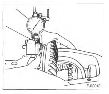
Figure 21—Determining Differential Shim Pack
