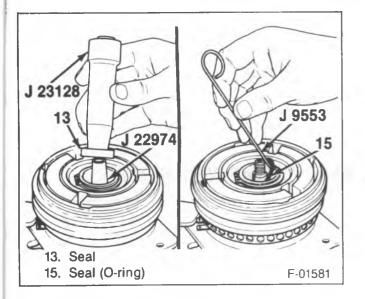
Figure 14—Removing/Installing the Shaft Seal Seat and Seal
