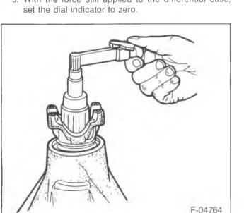
Figure 76—Checking Pinion Preload
