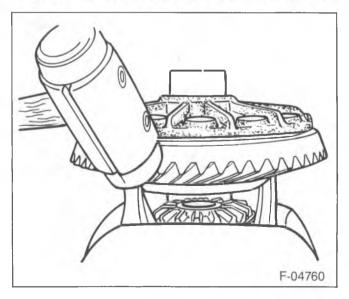
Figure 7—Removing the Ring Gear
