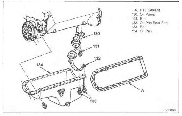
Figure 43—Oil Pan and Oil Pump
