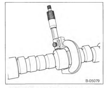
Figure 30—Checking the Camshaft Journals
