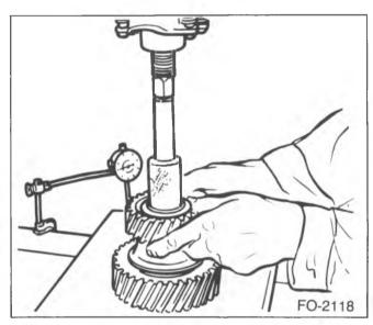
Figure 10—Idler Gear End Play Check
