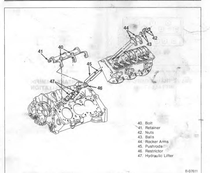
Figure 39—Valve Train Components
