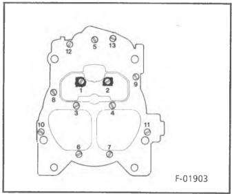
Figure 16 – Air Horn Screw Location and Tightening Sequence
