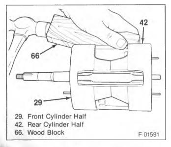
Figure 24—Separating the Cylinder Halves
