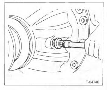
Figure 4 — Loosening the Thrust Adjusting Screw
