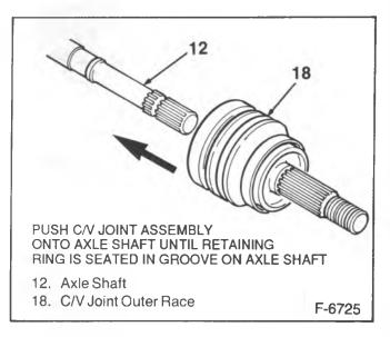
Figure 45—Installing C/V Joint
