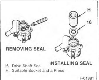
Figure 34—Remove and Install Driveshaft Seal
