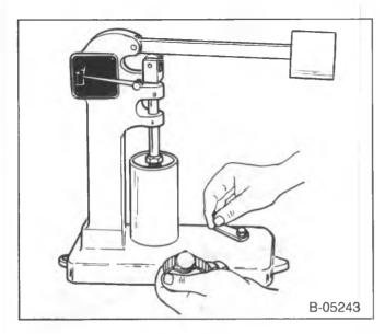
Figure 29—Testing the Hydraulic Lifter — Flat Type Only
