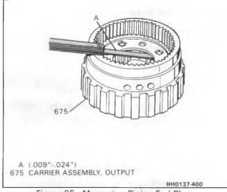
Figure 35 - Measuring Pinion End Play
