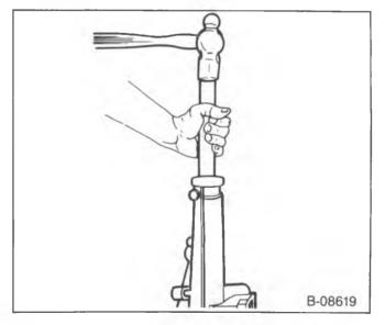
Figure 26—Installing the Extension **Housing Bushing**
