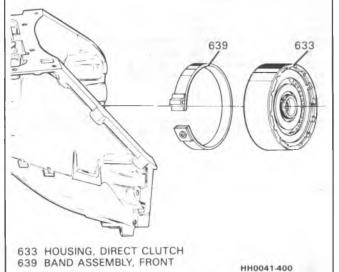
Figure 23 - Removing Direct Clutch Housing
