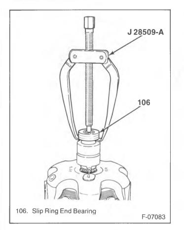
Figure 6—Removing the Slip Ring End Bearing
