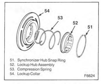
Figure 22—Synchronizer Hub Assembly
