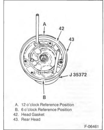
Figure 27—Installing the Rear Head Gasket
