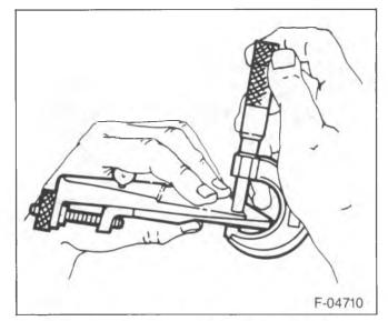
Figure 22—Measuring the Gage Plate Thickness
