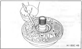
Figure 41 Marking Location of Oil Pump Gear
