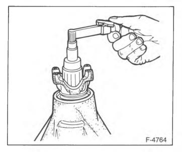
Figure 25—Measuring Pinion Preload
