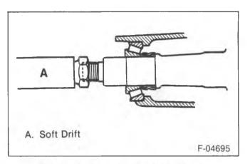
Figure 7—Removing the Drive Pinion
