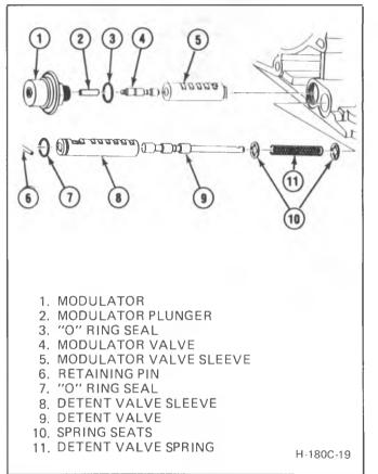
Figure 58 Installing Detent Valve and Modulator Valve
