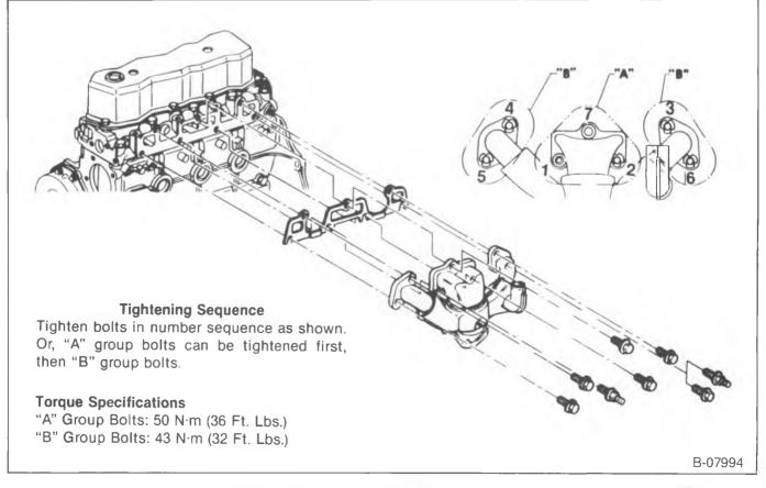
Figure 60—Exhaust Manifold Installation
