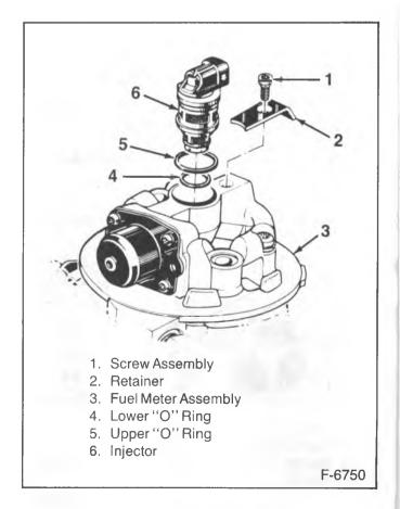
Figure 3-Model 700 Fuel Injection Parts
