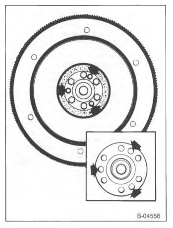
Figure 18—Flywheel Installed
