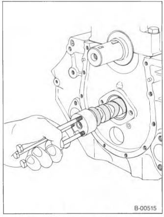
Figure 19-Removing the Camshaft
