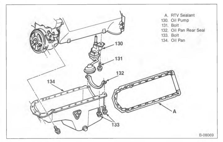
Figure 12-Oil Pan and Oil Pump
