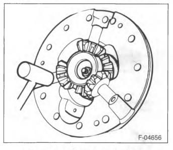
Figure 14—Installing the Pinion Yoke
