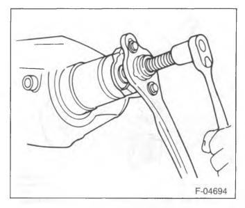
Figure 54—Removing the Pinion Flange
