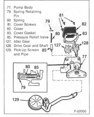
Figure 32—Oil Pump Components
