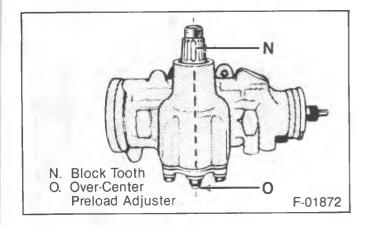
Figure 19—Pitman Shaft ''Over-Center'' Sector Adjustment
