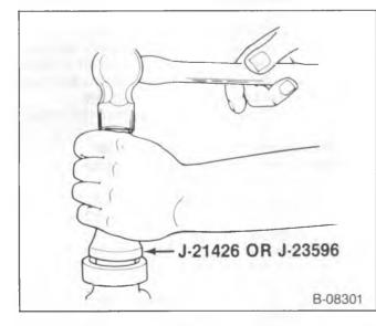
Figure 13—Installing the Rear Extension Bushing and Seal
