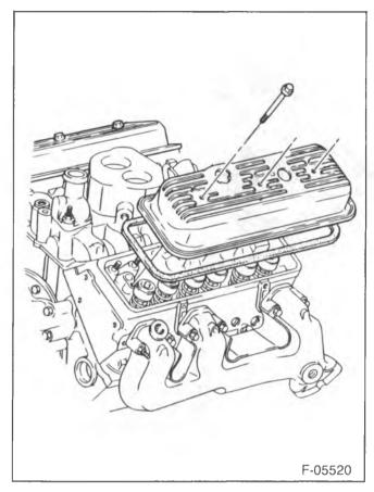
Figure 3—Rocker Arm Cover Installation
