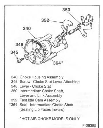
Figure 32 - Choke Housing Assembly
