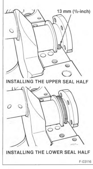
Figure 31—Installing the Two-Piece Rear Oil Seal
