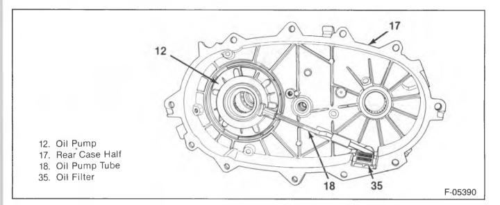
Figure 7—Pump Housing Installation
