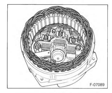
Figure 13—Stator in the Slip Ring End Frame
