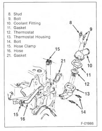
Figure 58—Thermostat Housing Components
