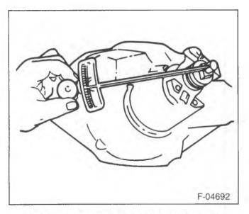
Figure 4—Checking Pinion Bearing Preload
