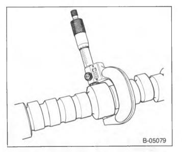
Figure 27—Checking the Camshaft Journals
