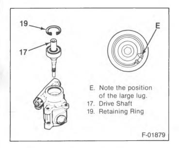
Figure 32—Remove and Install Retaining Ring
