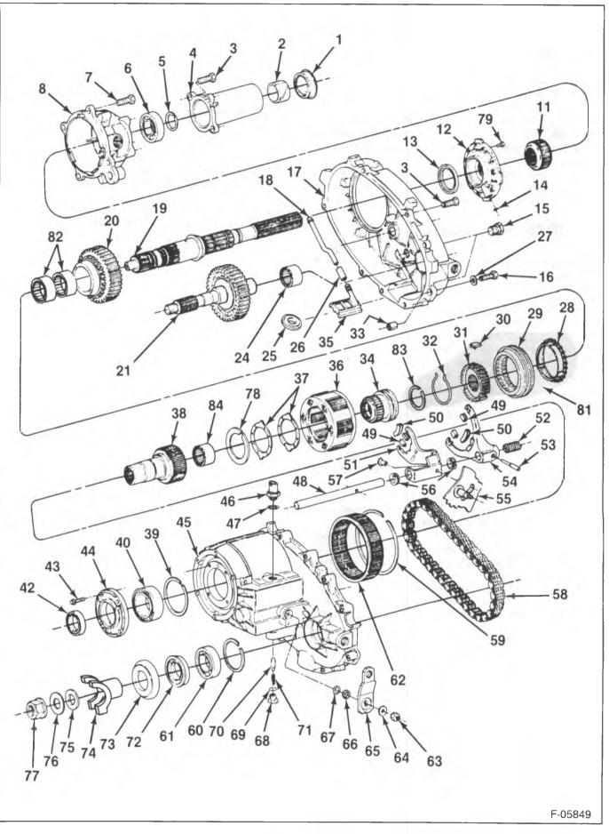
Figure 3—New Process 231 Transfer Case Components
