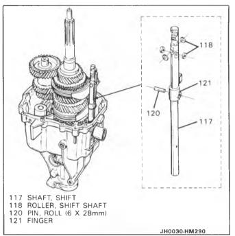
Figure 10 Removing Shift Shaft Rollers and Finger
