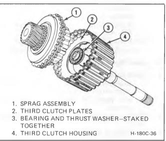
Figure 22 Sprag Assembly and Third Clutch Assembly
