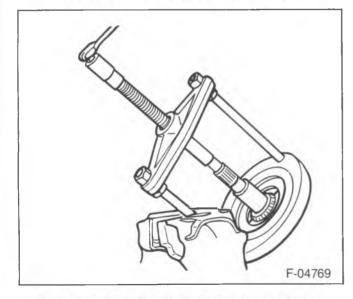
Figure 16—Removing the Pinion Inner Bearing
