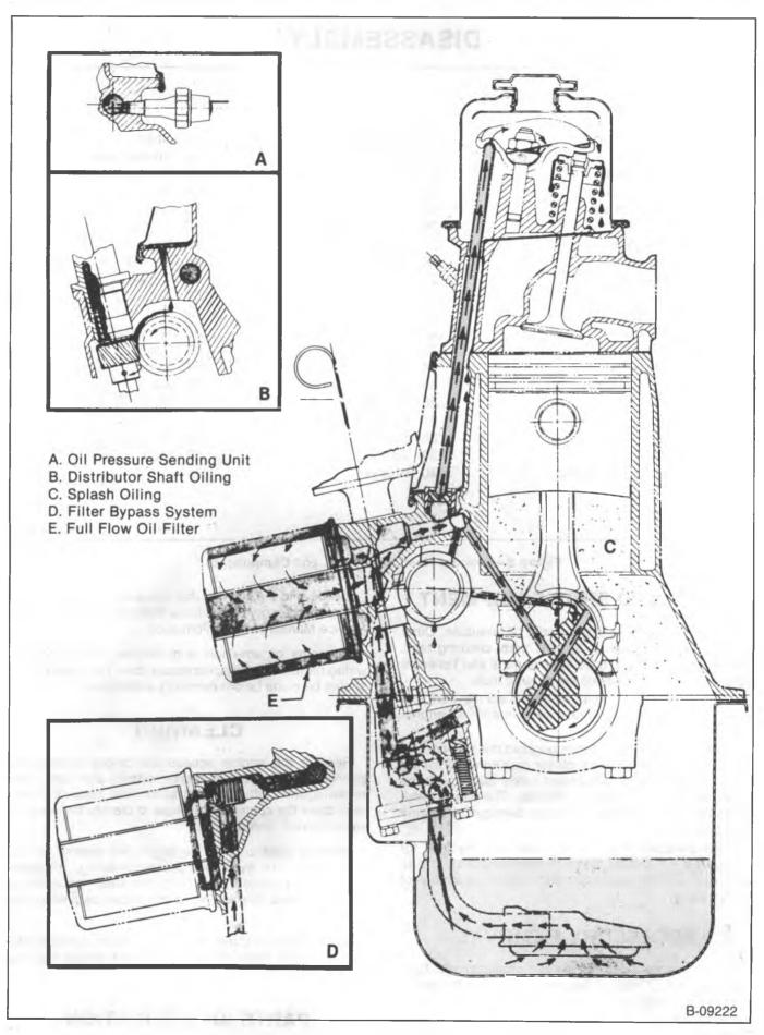
Figure 2—Lubrication Diagram (Front View)
