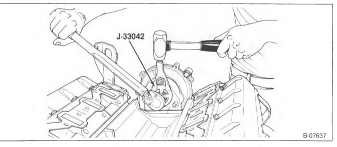
Figure 42—Marking TDC on the Front Cover
