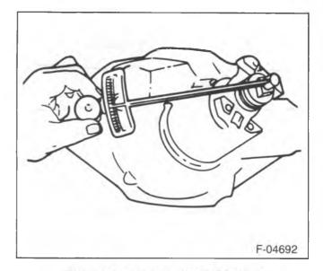
Figure 4—Checking Pinion Preload
