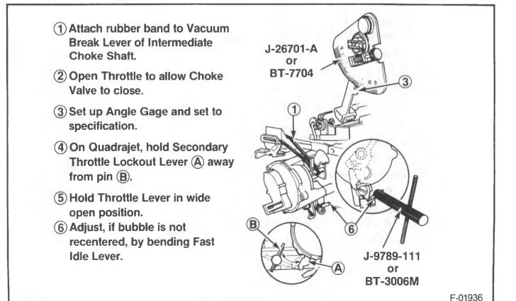
Figure 49 - Unloader Adjustment
