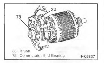
Figure 4—Armature Assembly
