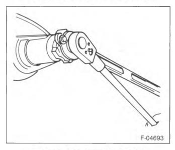
Figure 12-Drive Pinion Nut Removal
