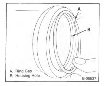
Figure 22—Installing the Retaining Ring
