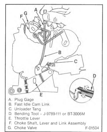
Figure 43 – Unloader Adjustment
