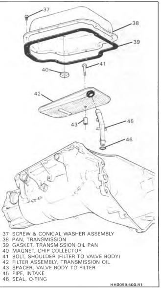
Figure 5 - Removing Pan & Filter Assembly
