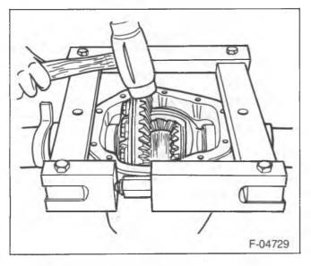
Figure 40—Installing the Differential Case
