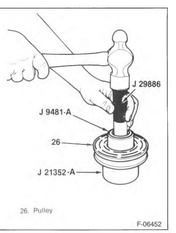
Figure 12—Installing the Pulley Rotor Bearing
