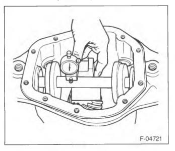
Figure 33—Checking the Pinion Depth Setting
