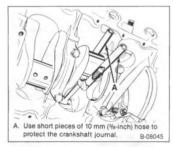
Figure 36—Installing the Connecting Rod and Piston
