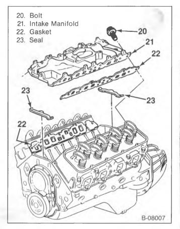
Figure 76—Intake Manifold (7.4L Engines)
