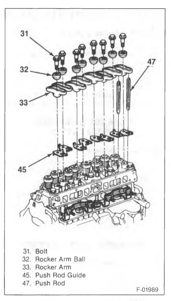
Figure 54—Valve Train Components
