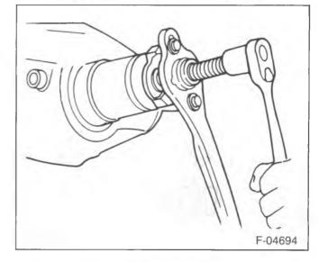
Figure 13—Pinion Flange Removal
