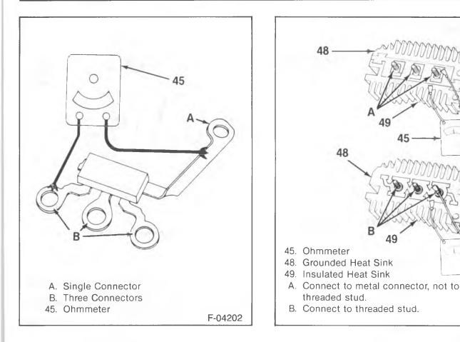
Figure 11—Diode Trio Check
