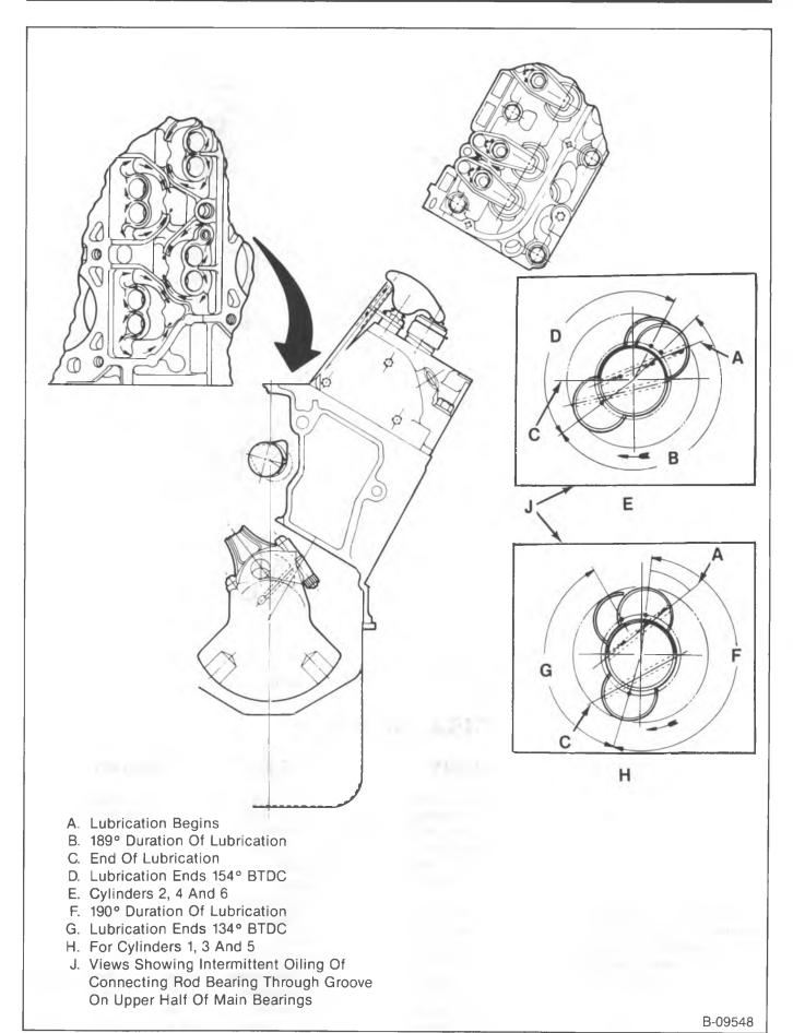
Figure 3—Engine Lubrication Diagram
