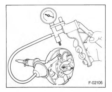
Figure 16—Checking the Vacuum Advance Unit
