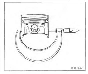
Figure 12-Measuring the Piston Skirt
