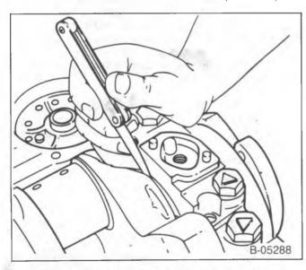
Figure 55—Measuring Crankshaft End Play
