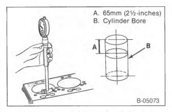
Figure 11-Measuring Cylinder Bore Diameter
