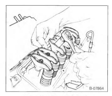
Figure 41—Adjusting the Valves
