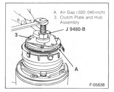
Figure 35—Installing the Clutch Plate and Hub Assembly
