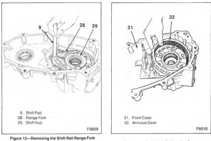
gure 12—Removing the Shift Rail Range Fol and the Shift Hub
