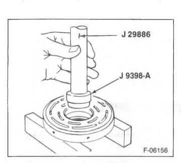
Figure 11—Removing the Clutch Rotor Bearing
