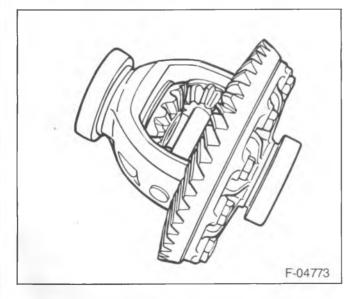
Figure 61—Differential with the Master Bearings
