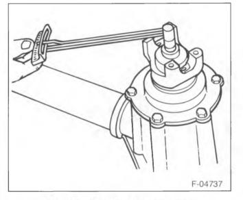
Figure 3—Checking Pinion Preload
