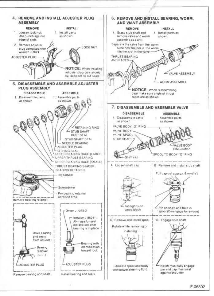
Figure 25—Removing and Installing the Adjuster Plug Assembly
