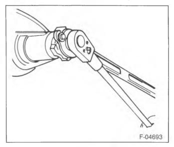
Figure 35—Tightening the Pinion Nut
