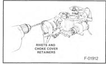
Figure 23 – Removing Choke Cover Rivets
