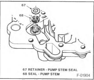
Figure 17 - Pump Stem Seal
