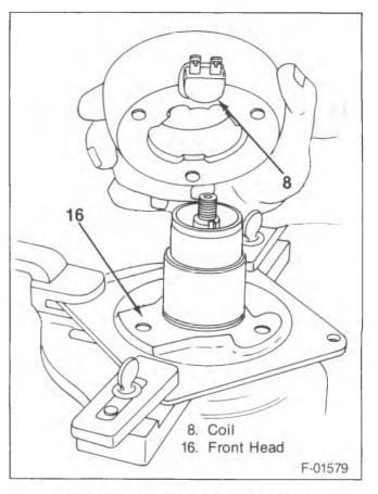
Figure 12—Installing the Coil Housing
