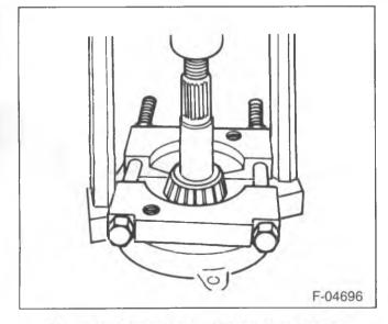
Figure 8—Removing the Pinion Rear Bearing
