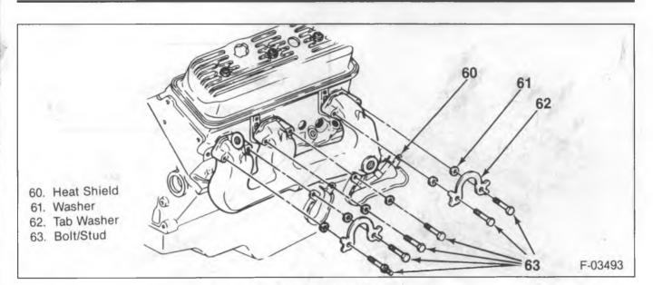
Figure 43—Exhaust Manifold Components
