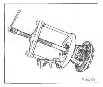
Figure 47—Removing the Differential Side Bearings
