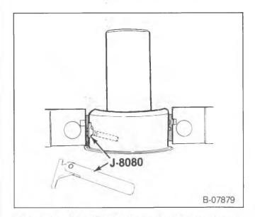
Figure 42—Installing the Upper Main Bearing Insert
