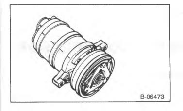
Figure 1 — HR-6 Compressor, V-Groove Pulley
