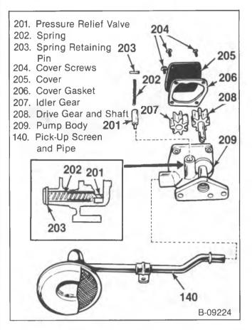
Figure 32—Oil Pump Components
