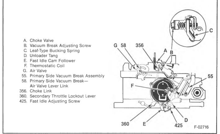
Figure 7 – Choke System - Electric - With Primary Side Vacuum Break Only
