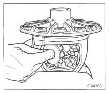
Figure 18—Installing the Pinion Gears
