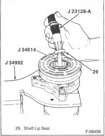
Figure 22—Removing or Installing the Shaft Seal
