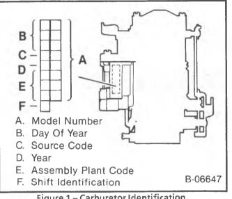
Figure 1 – Carburetor Identification
