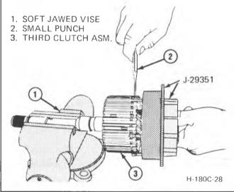
Figure 21 Removing Third Clutch Retaining Ring
