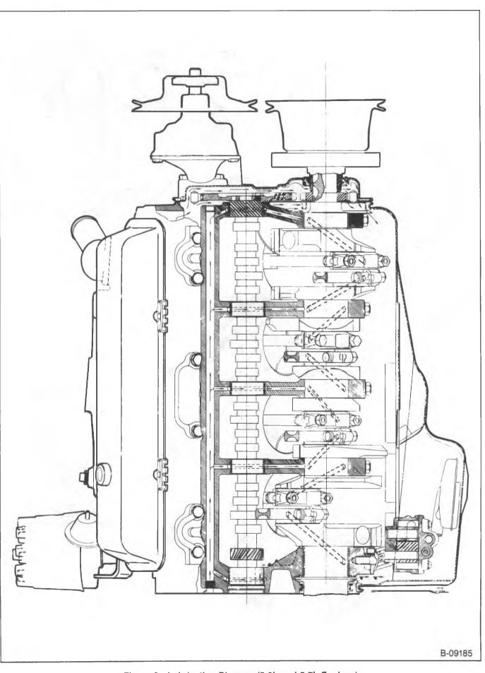
Figure 2—Lubrication Diagram (5.0L and 5.7L Engines)
