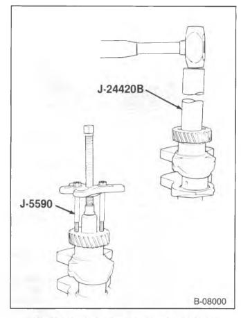
Figure 44-Replacing the Crankshaft Gear
