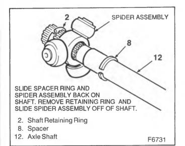
Figure 51—Removing Spider Assembly
