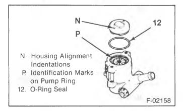
Figure 44—Aligning and Installing the Pump Ring
