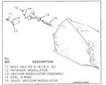
Figure 4 - Removing Vacuum Modulator Assembly
