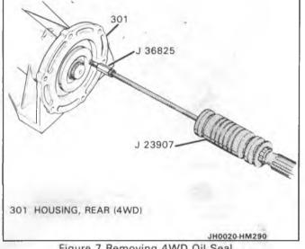
Figure 7 Removing 4WD Oil Seal
