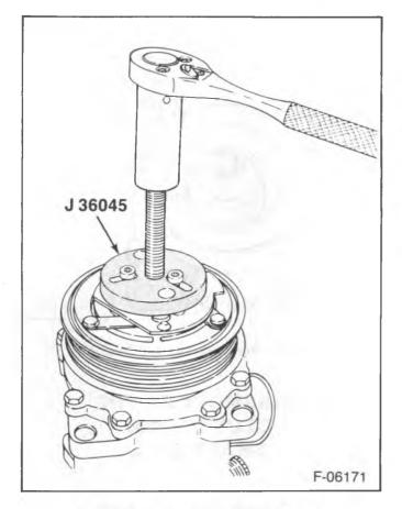
Figure 4—Removing the Clutch Plate
