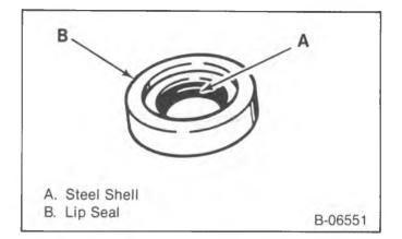
Figure 21 — Compressor Shaft Seal
