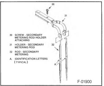
Figure 13 – Secondary Metering Rods and Holder
