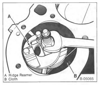
Figure 9—Removing the Cylinder Ridge
