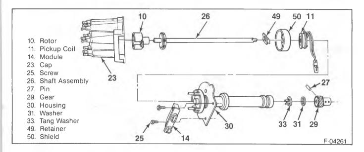
Figure 24—Distributor Components (Separate Coil and Sealed Connector) for an 8-Cylinder Engine
