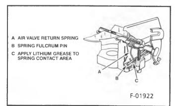
Figure 36 - Lubricating Air Valve Spring Pin
