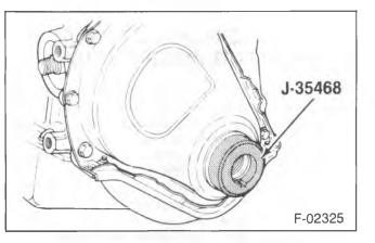
Figure 52—Front Cover Centering Tool
