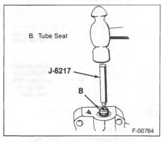
Figure 6-Installing the Tube Seat
