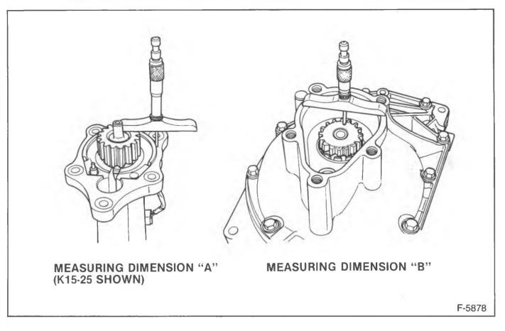
Figure 38—Measuring to Calculate Shim Size
