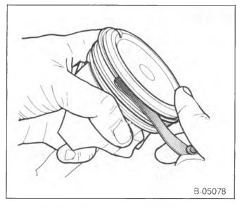
Figure 18—Measuring Ring Clearance
