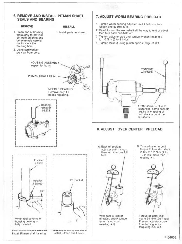
Figure 8—Model 535 — Chart C — Adjustment
