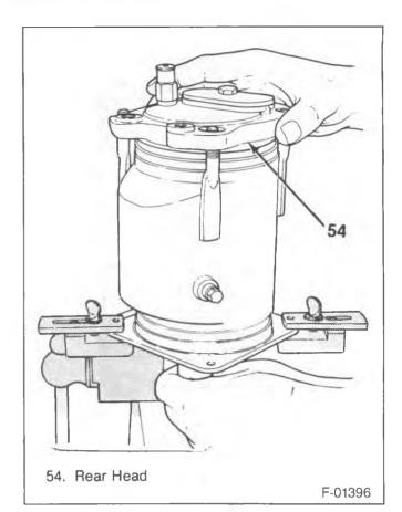
Figure 51—Installing the Rear Head
