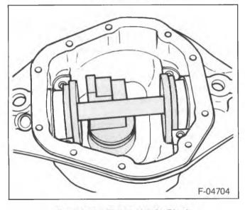
Figure 25—Pinion Height Block
