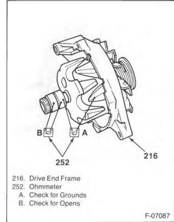
Figure 10—Checking the Rotor Field Windings
