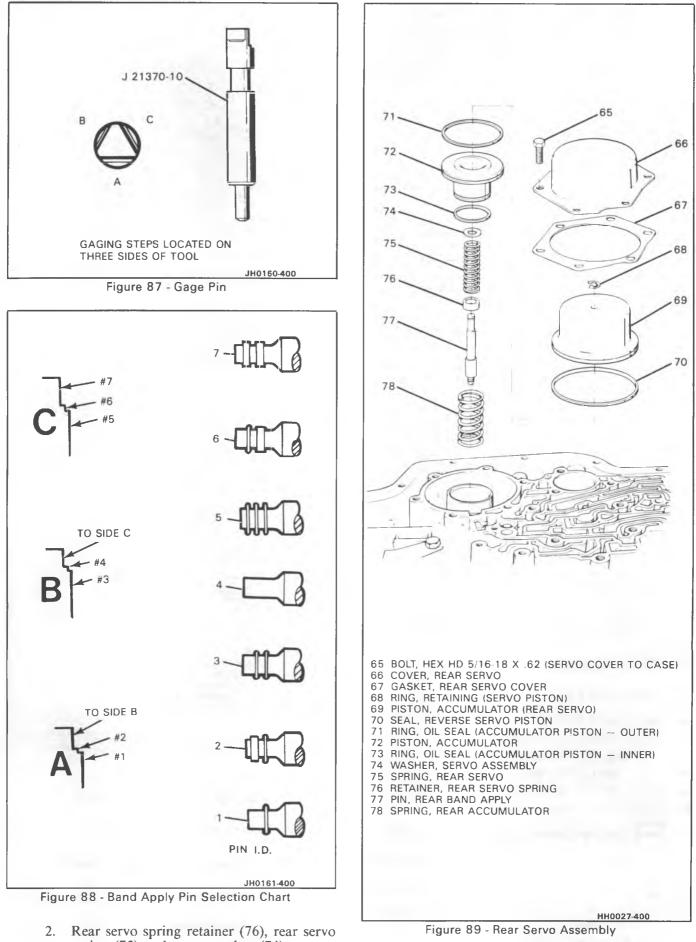
spring (75) and servo washer (74) on rear band apply pin (77).
