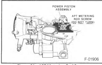
Figure 21 – APT Metering Rod Screw
