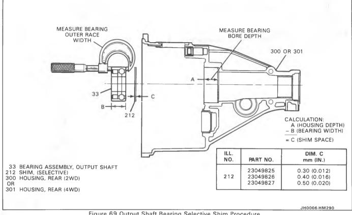
Figure 69 Output Shaft Bearing Selective Shim Procedure
