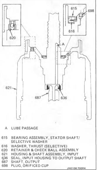
Figure 60 Input Housing Check Valve Ball
