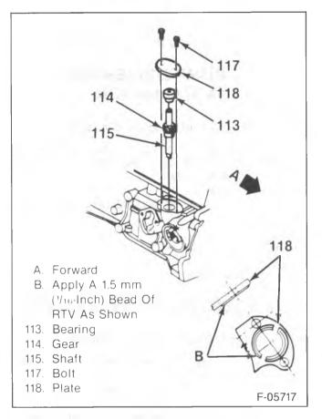
Figure 52—Oil Pump Drive Shaft
