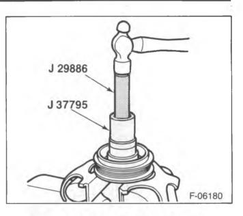
Figure 14—Installing the Rotor Bearing
