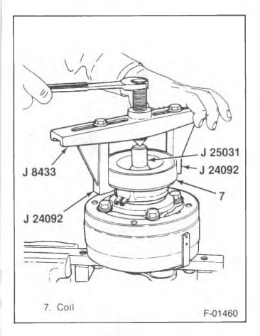
Figure 14---Removing the Poly-Groove Clutch Coil
