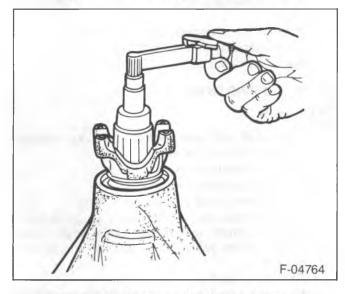
Figure 52—Checking the Pinion Preload
