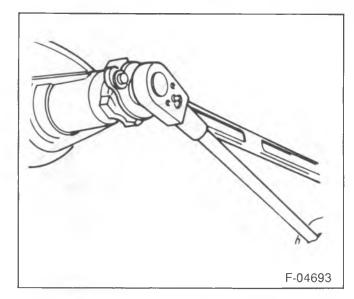
Figure 53—Removing the Drive Pinion Nut
