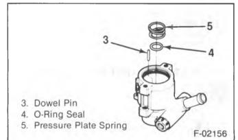
Figure 41—Installation of the Pin, Seal and Pressure Plate Spring
