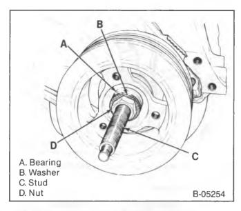
Figure 53—Installing the Torsional Damper
