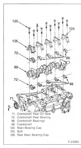
Figure 39—Crankshaft and Bearing Components
