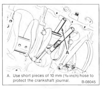
Figure 14—Removing the Piston and Connecting Rod
