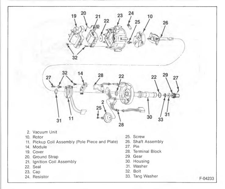
Figure 7—Distributor Components
