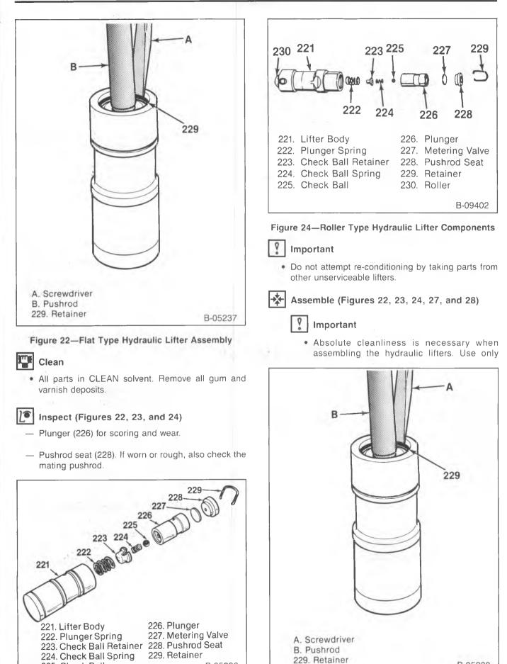
Figure 23—Flat Type Hydraulic Lifter Components
