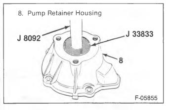
Figure 11—Pump Retainer Housing Bearing Installation
