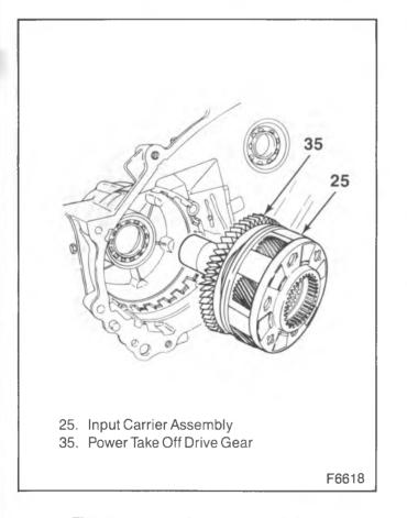
Figure 16—Input Carrier and PTO Gear
