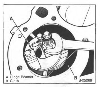
Figure 16—Removing the Cylinder Ridge
