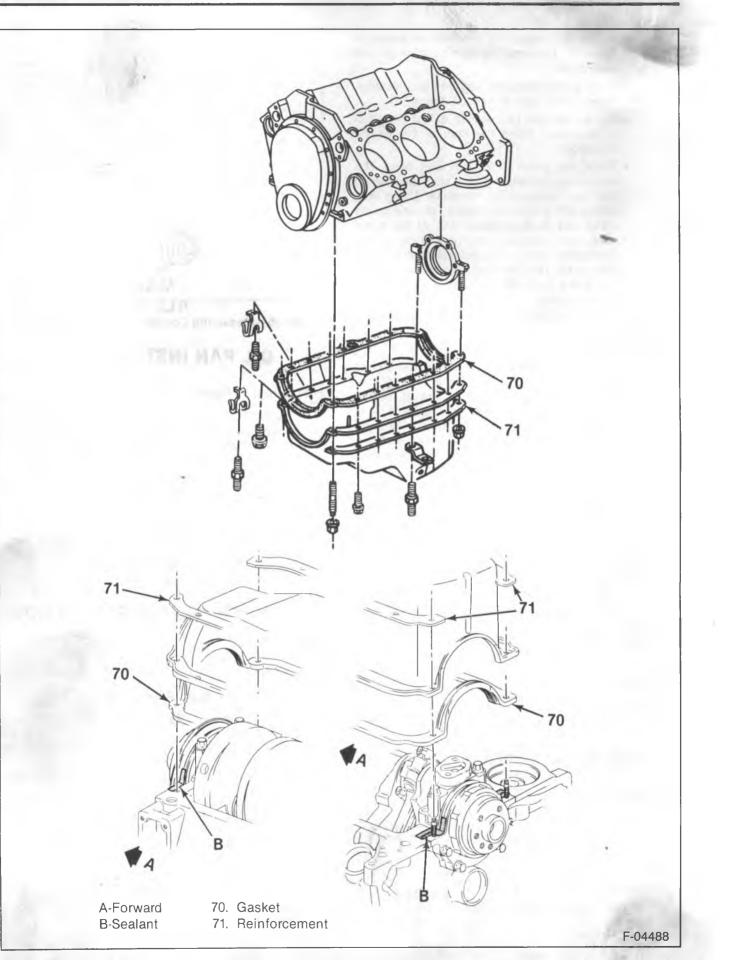
Figure 37—Oil Pan Installation
