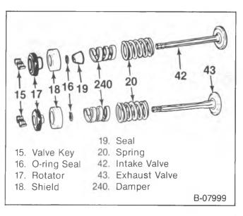
Figure 34—Valves and Components
