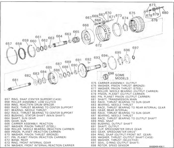
Figure 34 - Gear Unit Assembly
