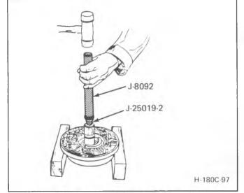
Figure 75 Installing Oil Pump Bushing - Front
