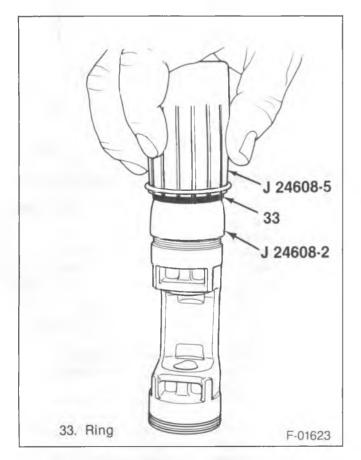
Figure 37—Installing the Piston Ring
