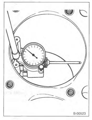
Figure 1—Checking the Cylinder Bore
