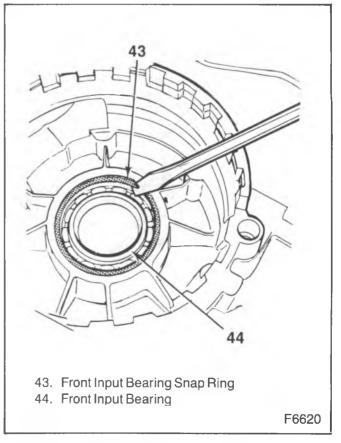
Figure 18—Front Input Bearing Snap Ring Removal
