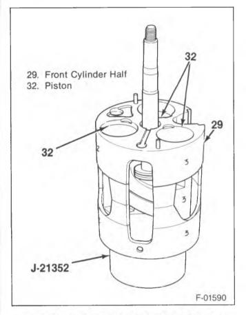
Figure 23-Numbering the Pistons and Cylinders
