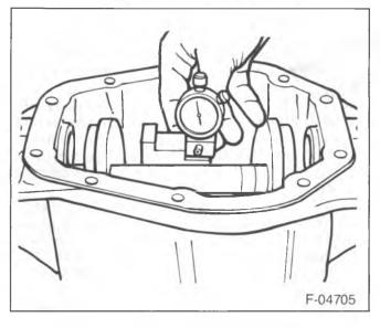
Figure 66—Scooter Gage on the Height Block
