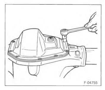
Figure 41—Installing the Axle Cover
