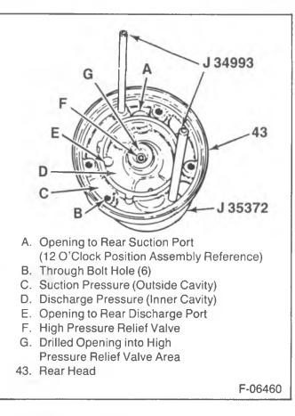
Figure 26—Positioning the J 34993 Guide Pins
