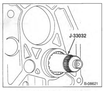
Figure 34—Installing Tool J 33032
