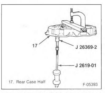
Figure 9—Front Output Shaft Rear Bearing Removal
