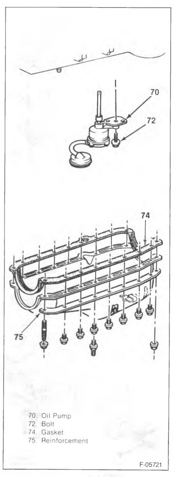
Figure 15—Oil Pan (5.0L and 5.7L Engines)
