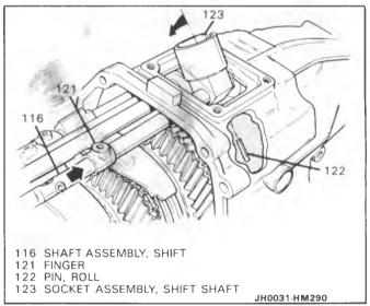
Figure 11 Removing Shift Socket Assembly Roll Pin
