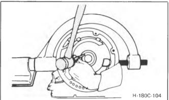
Figure 83 Removing Reaction Sun Gear Drum Bushing Sleeve
