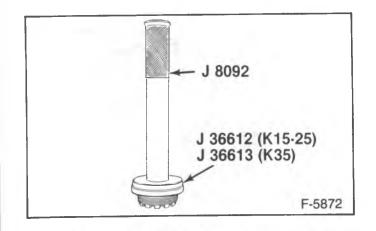
Figure 27—Installing the Adjuster Sleeve Bearing
