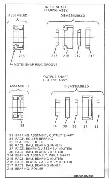
Figure 26 Main Bearing Components
