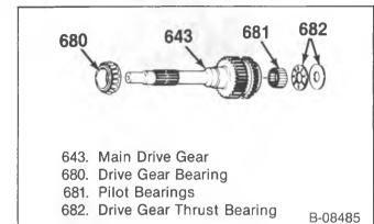
Figure 16—Main Drive Gear Bearings
