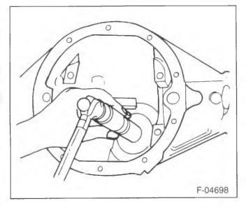
Figure 10-Installing Rear Pinion Bearing Cup
