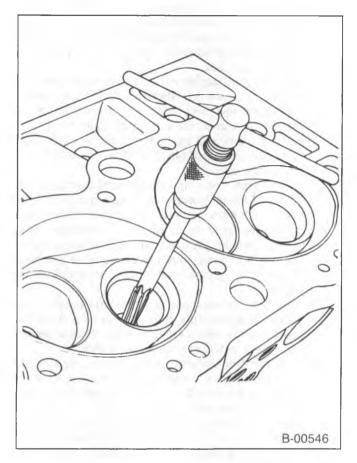
Figure 36—Reaming the Valve Guides (Typical)
