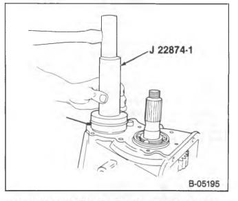
Figure 37—Installing the Countergear Rear Bearing
