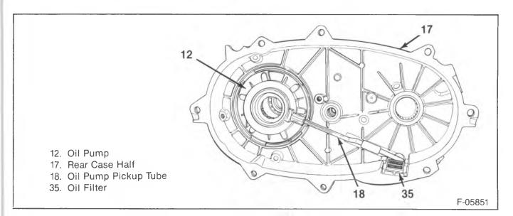
Figure 5—Oil Pump, Pickup Tube and Screen
