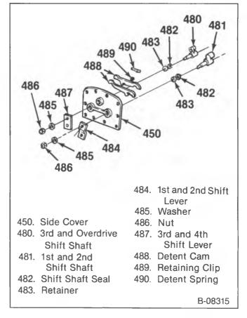
Figure 15—Side Cover and Components
