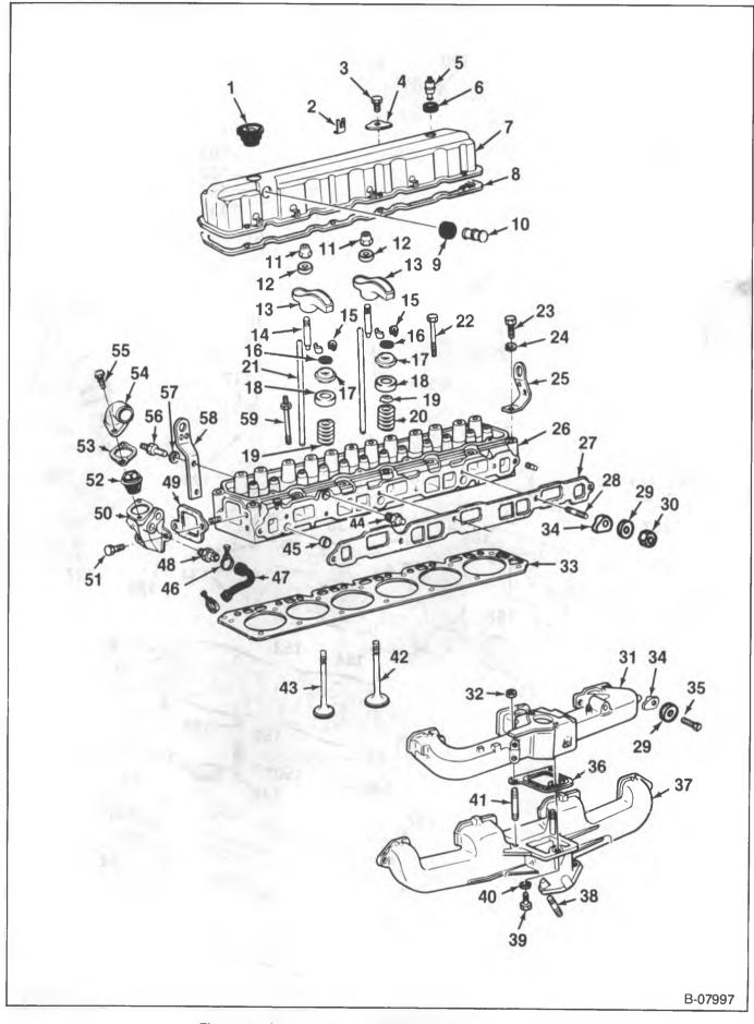
Figure 4—Cylinder Head, Manifolds, and Components
