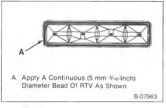
Figure 56—Applying RTV to the Pushrod Cover
