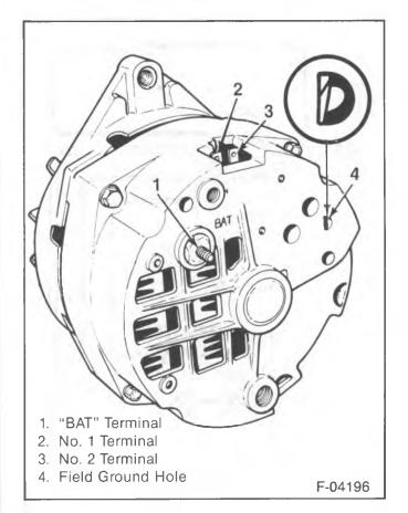
Figure 5—Field Ground Tab
