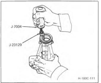
Figure 10 Removing Extension Housing Oil Seal
