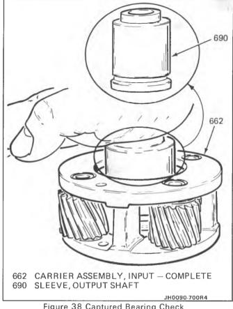
Figure 38 Captured Bearing Check
