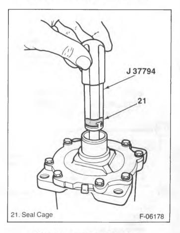
Figure 12—Removing the Seal Cage
