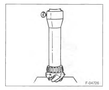
Figure 14—Installing the Pinion Inner Bearing
