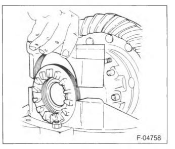
Figure 24—Installing the Bearing Cup
