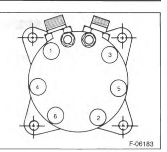
Figure 17—Torque Sequence
