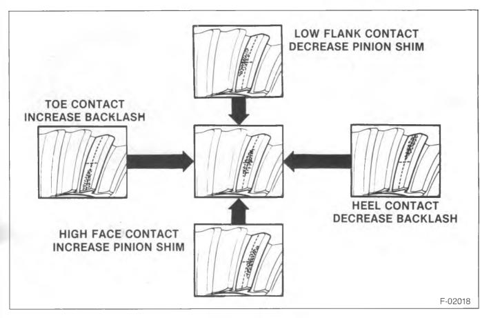
Figure 26—Gear Tooth Contact Pattern
