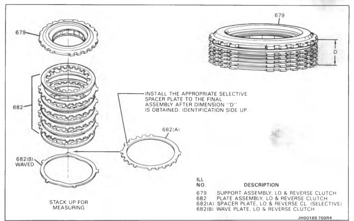
Figure 41 Measuring For Spacer Plate Selection
