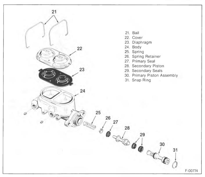
Figure 14—Cast Iron Master Cylinder Components
