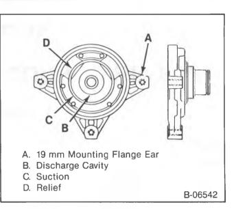
Figure 2 — HR-6 Front Head Assembly
