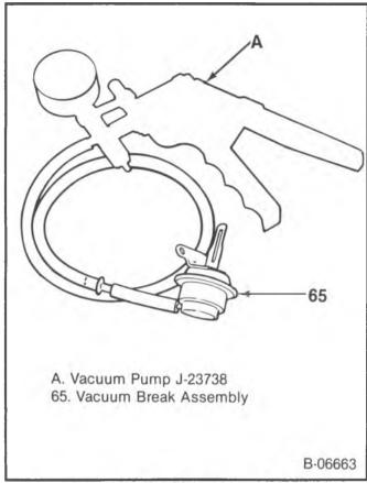
Figure 30 – Checking Vacuum Break
