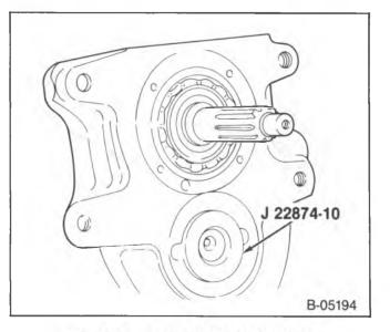
Figure 36-Tool J-22874-10 Installed
