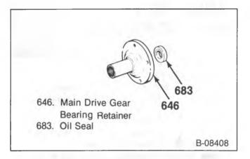
Figure 28—Main Drive Gear Bearing Retainer Oil Seal
