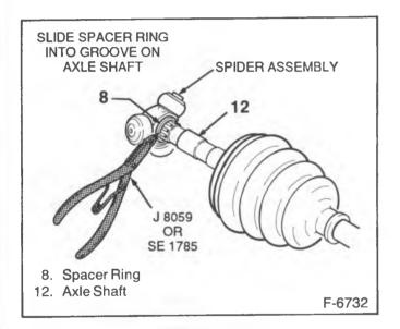
Figure 52—Installing Spider Assembly
