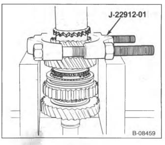
Figure 20—Removing the 5th Speed Driven Gear
