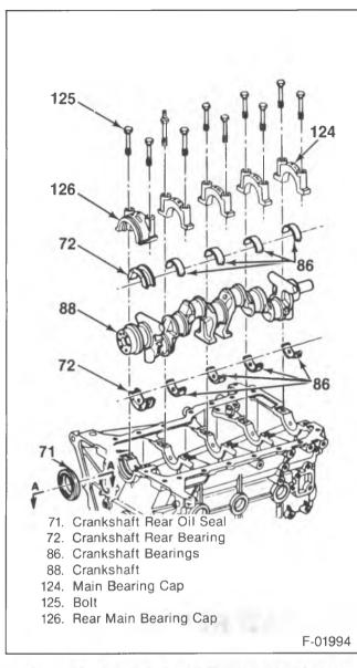
Figure 18—Crankshaft and Bearing Components
