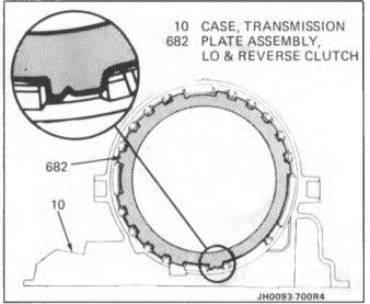
Figure 44 Lo and Reverse Clutch Plates Properly Installed
