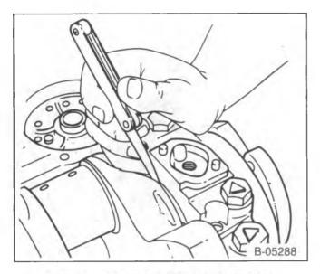
Figure 30—Measuring Crankshaft End Play
