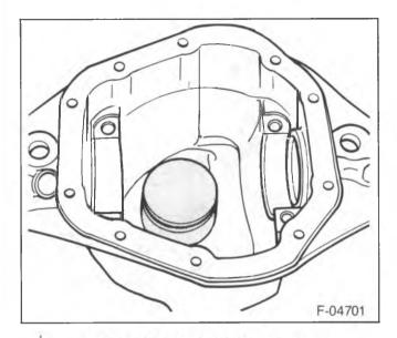
Figure 23—Master Pinion Block
