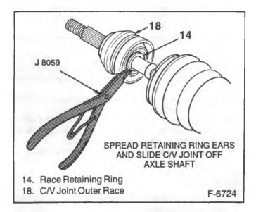
Figure 44—Removing C/V Joint
