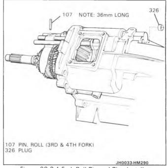
Figure 83 3-4 Fork Roll Pin and Plug Install
