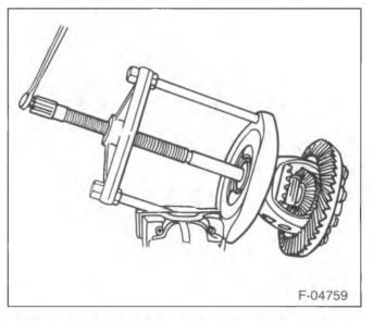
Figure 6—Removing the Differential Side Bearings
