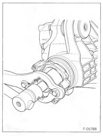
Figure 10—Removing the Pinion Nut
