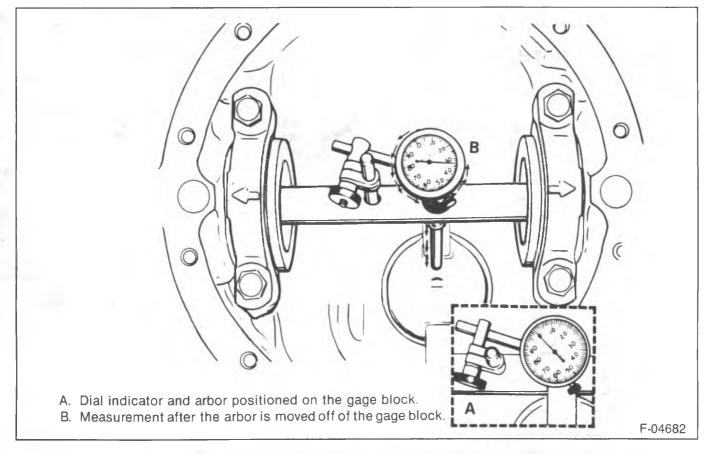
Figure 13—Checking Pinion Depth
