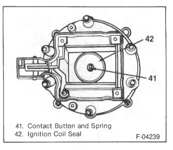
Figure 15—Cap and Seal
