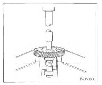
Figure 29—Removing the Camshaft Gear
