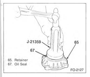
Figure 18—Installing the Rear Bearing Retainer Seal
