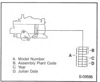
Figure 1 – Carburetor Identification
