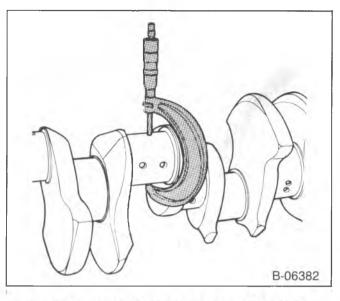
Figure 37—Measuring the Crankshaft Journals
