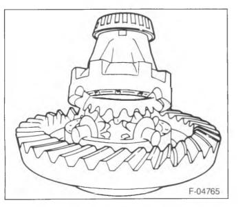
Figure 22—Installing the Case Halves
