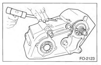
Figure 14—Installing the Shift Fork Roll Pin
