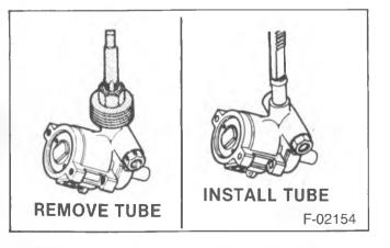
Figure 39—Remove and Install Return Tube
