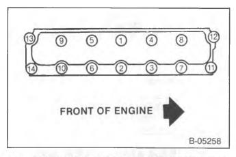
Figure 58—Cylinder Head Bolt Tightening Sequence
