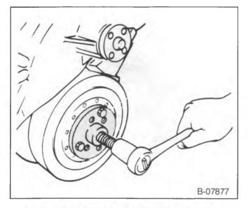
Figure 5—Removing the Torsional Damper
