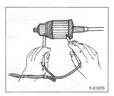
Figure 8—Testing the Armature for Grounds
