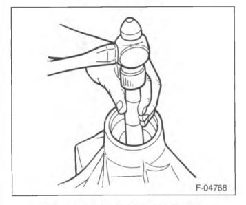
Figure 15—Removing the Bearing Cups
