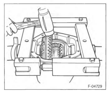
Figure 39—Installing the Differential Case
