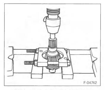
Figure 8—Removing the Pinion Inner Bearing
