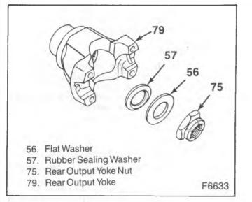
Figure 26-Installing the Rear Output Yoke
