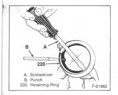
Figure 3—Removing the Retaining Ring
