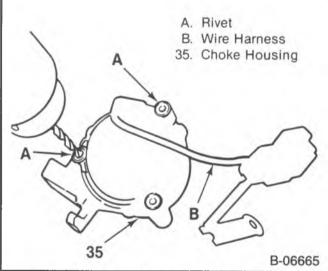
Figure 31 - Removing Choke Cover Attaching Rivets
