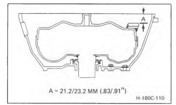
Figure 70 Proper Converter Installation
