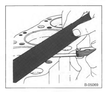
Figure 22—Checking the Block Gasket Surface
