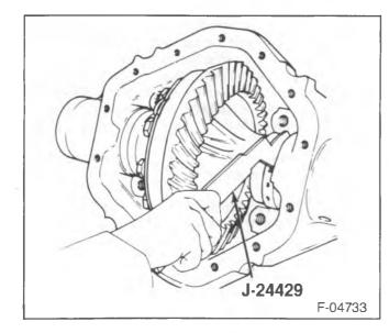
Figure 21—Adjusting the Nut
