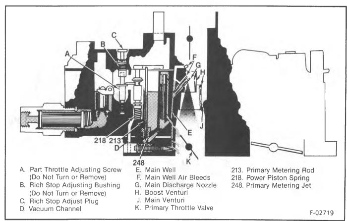
Figure 4 – Main Metering System
