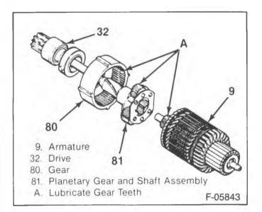
Figure 13—Armature, Gears and Drive
