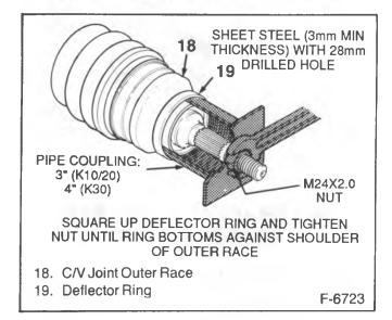
Figure 43—Installing Outer Deflector Ring
