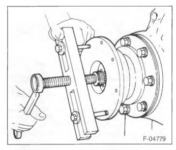
Figure 12—Removing the Pinion Flange
