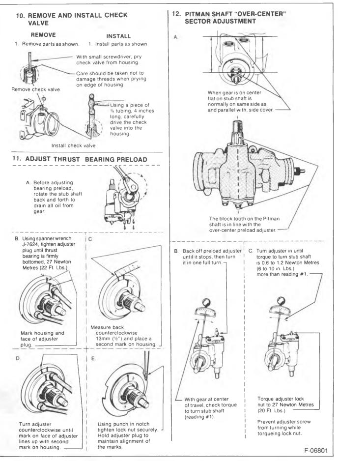
Figure 27—Removing and Installing the Check Valve and Adjusting the Thrust Bearing Preload and Pitman Shaft "Over-Center" Sector
