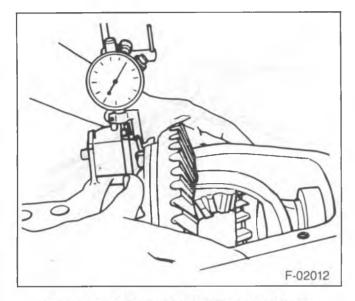
Figure 36—Measuring Differential Movement
