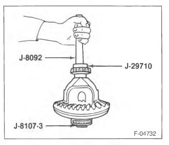
Figure 20—Installing the Side Bearing
