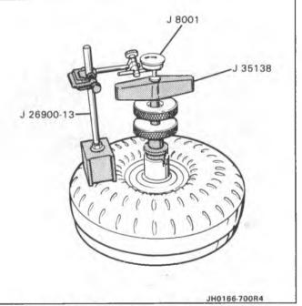
Figure 138 Checking Torque Converter End Play
