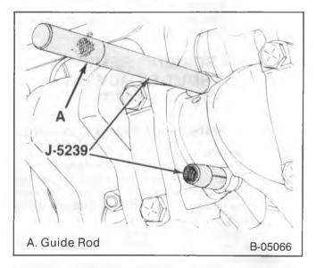
Figure 17—Removing the Piston and Connecting Rod
