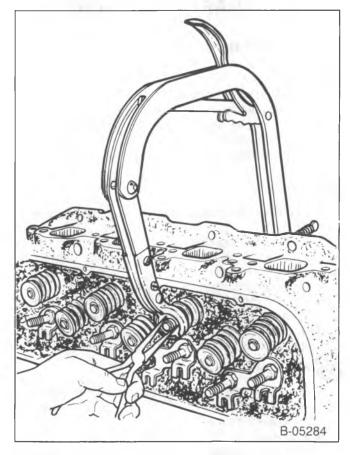
Figure 24—Compressing the Valve Springs
