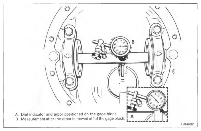
Figure 13—Checking Pinion Depth
