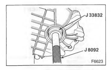
Figure 21—Removing the Front Output Bearing
