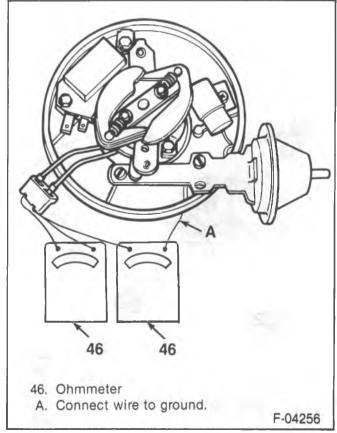
Figure 18—Checking the Pickup Coil
