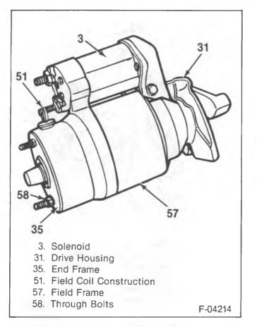
Figure 6—Light Duty Starting Motor
