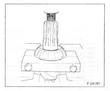
Figure 14—Removing the Pinion Inner Bearing
