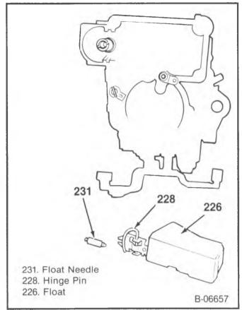
Figure 17 – Float and Float Needle
