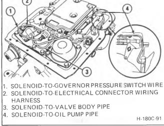
Figure 2 Hookup of Solenoid Pipes and Electrical Wires
