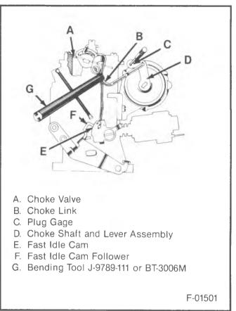
Figure 39 – Choke Stat Lever Adjustment
