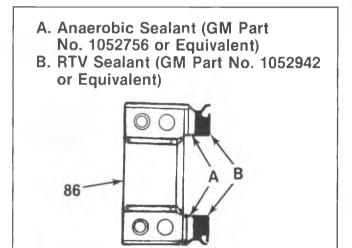
Figure 29—Applying Sealer to Rear Main Bearing Cap
