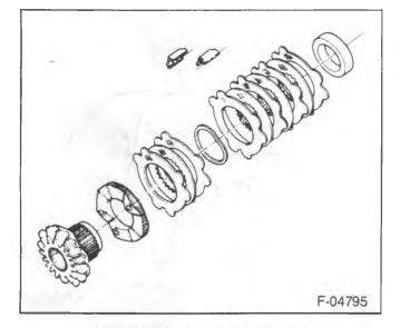
Figure 12—Cam Unit Components
