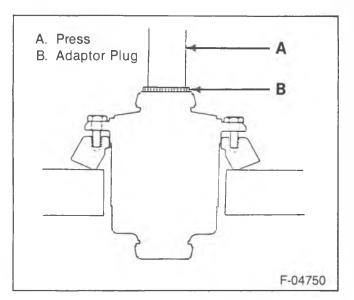
Figure 16—Installing the Ring Gear to Case
