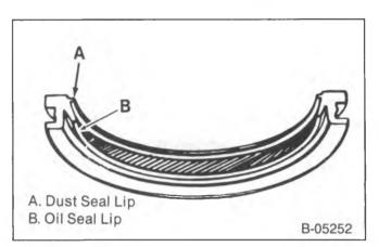
Figure 48—Crankshaft Rear Oil Seal Half
