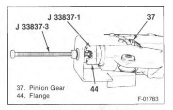
Figure 11—Remove the Pinion Flange
