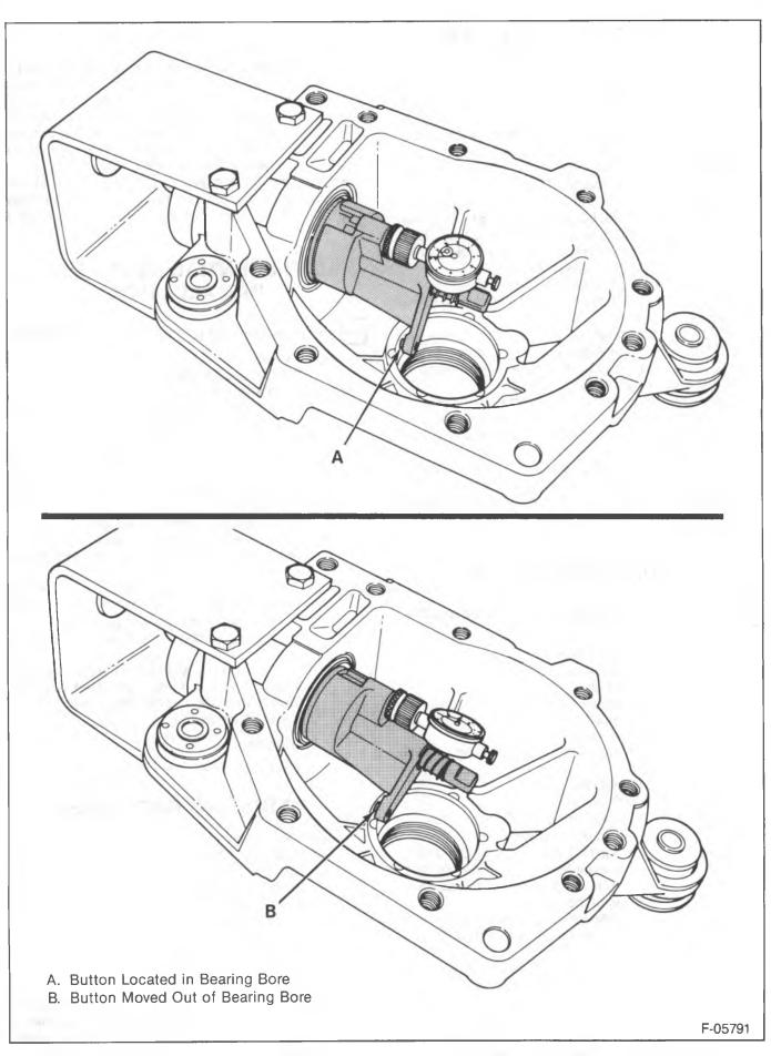
Figure 19—Measuring Pinion Depth
