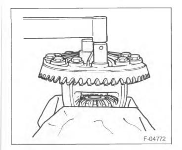
Figure 60—Installing the Ring Gear Bolts
