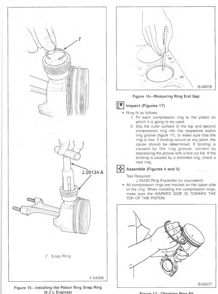
Figure 17—Checking Ring Fit
