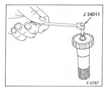
Figure 7—Removing the Pilot Bearing
