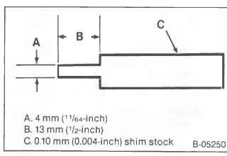
Figure 46—Oil Seal Installation Tool
