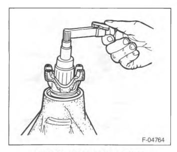
Figure 36—Checking Pinion Preload
