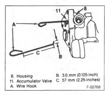
Figure 4—Removing the Accumulator Valve
