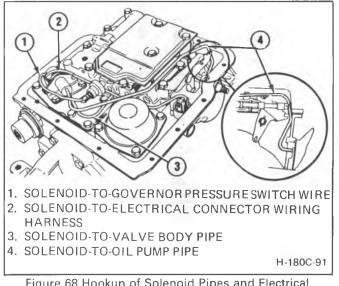
Figure 68 Hookup of Solenoid Pipes and Electrical Wires
