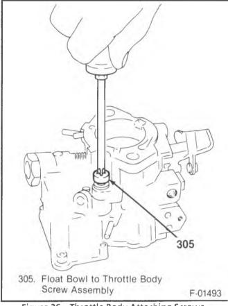
Figure 26 – Throttle Body Attaching Screws
