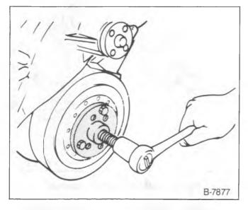
Figure 14—Removing the Torsional Damper
