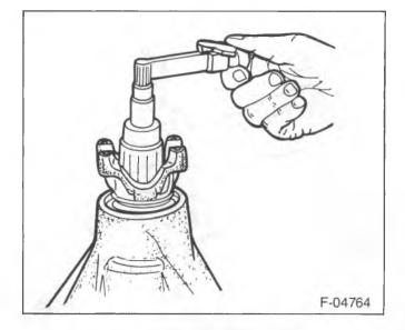
Figure 35—Checking Pinion Preload
