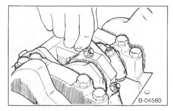
Figure 37—Checking Connecting Rod Side Clearance
