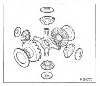
Figure 9-Differential Components
