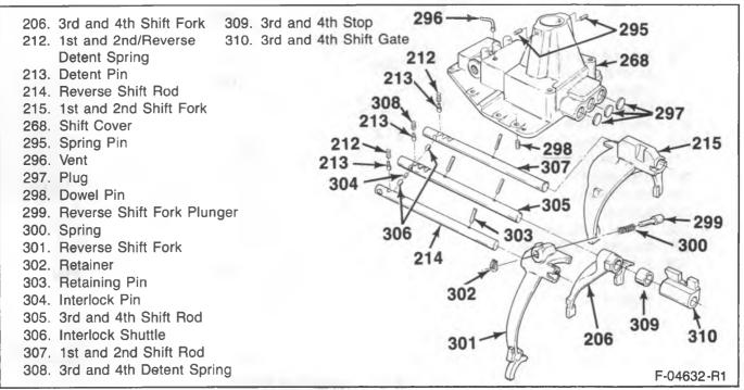
Figure 30B—C/K Shift Cover and Components
