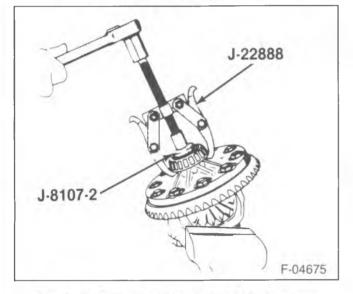
Figure 3—Removing Differential Side Bearings
