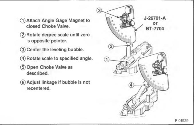
Figure 44 - Choke Valve Angle Gage
