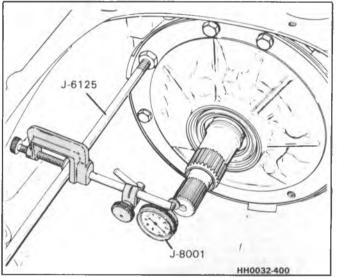
Figure 13 - Front Unit End Play Check
