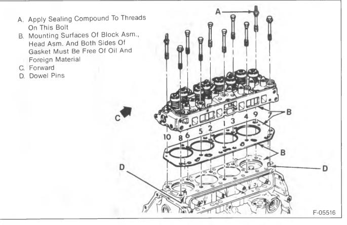
Figure 53—Cylinder Head Installation
