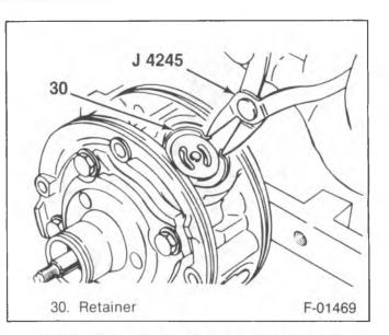
Figure 22—Replacing the Valve Plate Retainer
