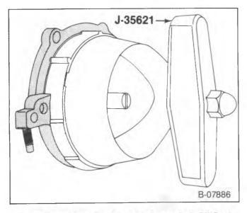
Figure 28—Installing the Rear Crankshaft Oil Seal
