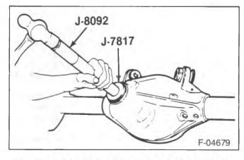
Figure 7—Installing the Front Pinion Bearing Cup
