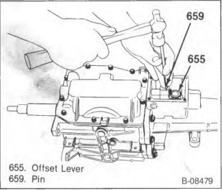
Figure 4-Removing the Offset Lever Pin
