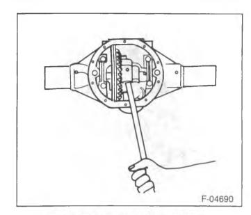
Figure 2—Prying the Differential Case
