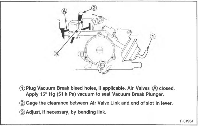
Figure 48 - Air Valve Link Adjustment
