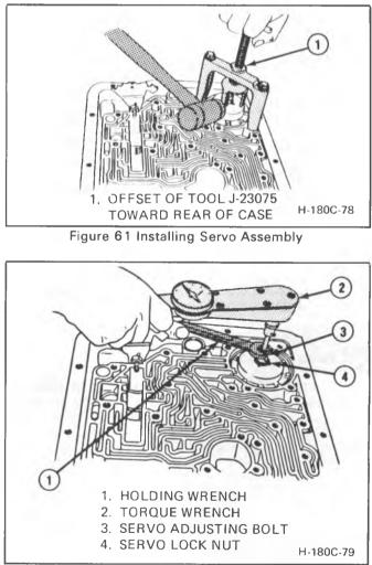
Figure 62 Adjusting Servo Apply Rod
