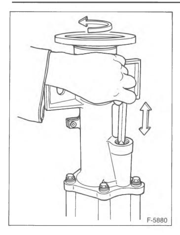
Figure 40—Checking the Shift Mechanism
