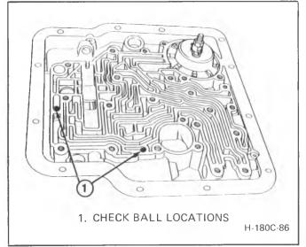
Figure 66 Installing Check Balls in Oil Passages
