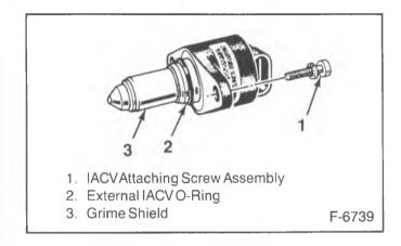
Figure 4—Flange Mounted Type IAC Valve
