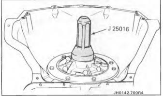
Figure 96 Oil Pump Seal
