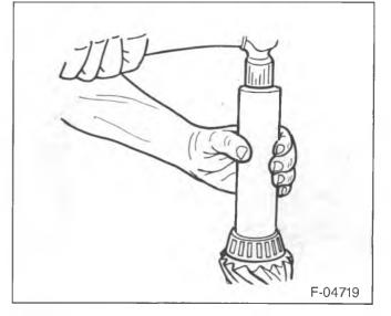
Figure 31—Installing the Inner Bearing
