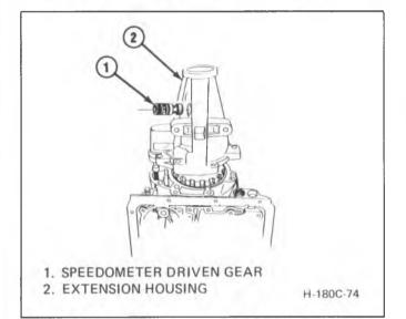
Figure 57 Extension Housing and Speedometer Driven Gear
