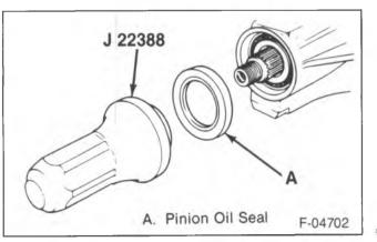
Figure 14—Installing the Pinion Oil Seal
