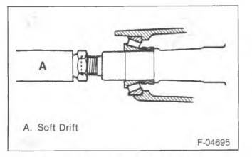
Figure 7—Removing the Drive Pinion
