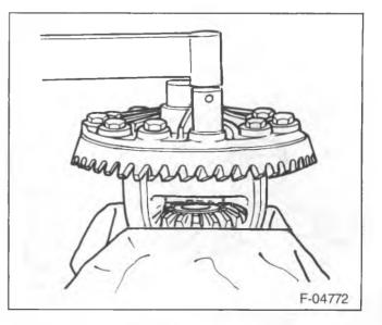
Figure 19—Installing the Ring Gear Bolts
