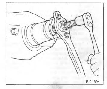
Figure 15—Installing the Pinion Flange
