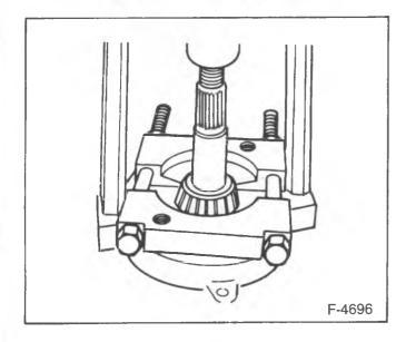
Figure 14—Removing the Pinion Bearing
