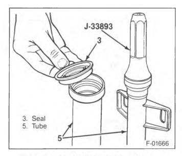
Figure 31—Installing the Shaft Seal
