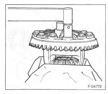
Figure 20—Installing the Ring Gear Bolts
