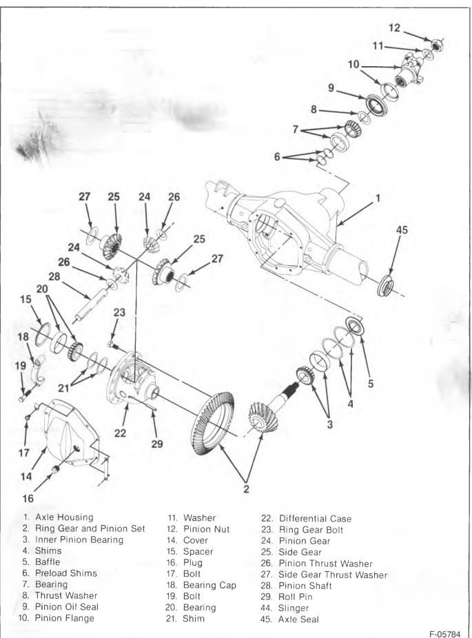
Figure 1—Front Axle Components
