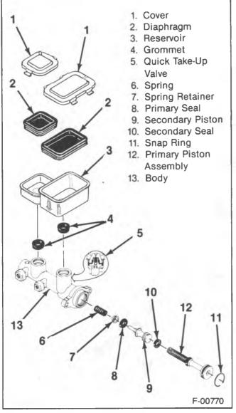
Figure 10—Composite Master Cylinder Components
