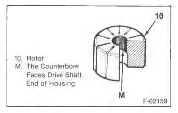
Figure 43-Installing the Rotor
