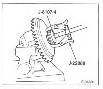
Figure 3—Removing Differential Side Bearing
