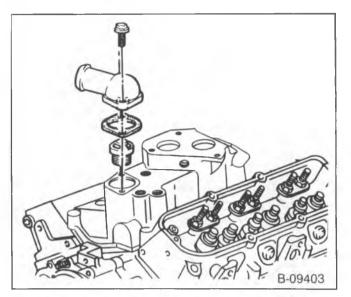
Figure 27—Thermostat and Water Outlet
