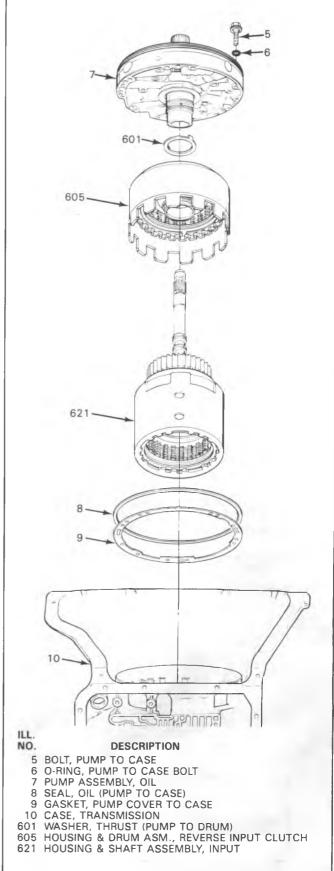
JH0075-700R4-R1 Figure 23 Input Clutch Removal
