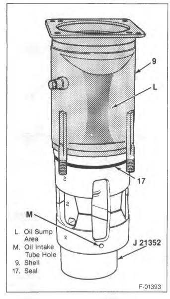
Figure 48—Installing the Compressor Shell
