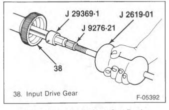
Figure 8—Removing the Input Gear Bearing
