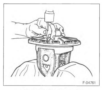
Figure 8—Removing the Lock Pin
