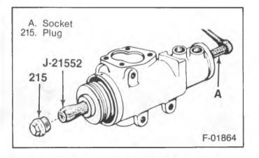
Figure 4—Removing the Plug and Piston Rack
