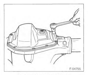
Figure 2-Removing the Axle Cover
