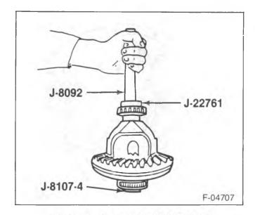
Figure 19—Installing the Side Bearing
