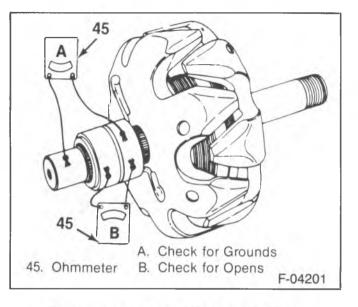
Figure 10—Checking Rotor Field Windings
