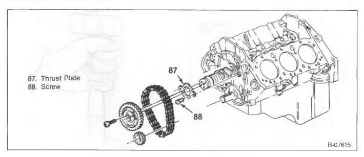
Figure 29—Camshaft and Components
