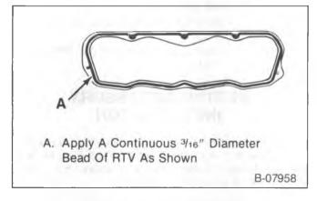
Figure 55—Applying Sealant to the Rocker Arm Cover
