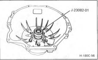
Figure 49 Aligning Converter Housing to Oil Pump
