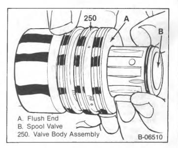
Figure 11—Remove or Install Valve Spool
