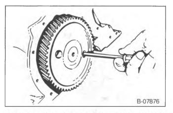
Figure 44—Installing the Camshaft Thrust Plate Bolts
