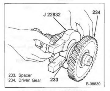
Figure 23—Installing Tool J 22832
