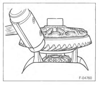
Figure 7—Removing the Ring Gear
