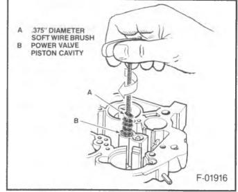
Figure 28 - Cleaning Power Piston Bore
