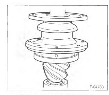
Figure 16—Installing the Pinion Flange
