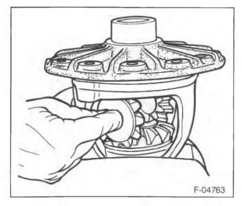
Figure 17—Installing the Pinion Gears
