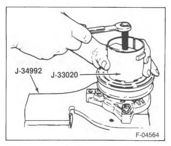
Figure 10—Removing the Pulley Rotor and Bearing Assembly
