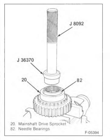
Figure 10—Installing the Needle Bearings to the Front Drive Sprocket
