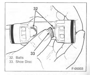
Figure 29—Installing the Front Shoe Disc
