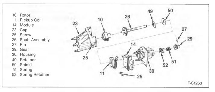
Figure 23—Distributor Components (Separate Coil and Sealed Connector)
