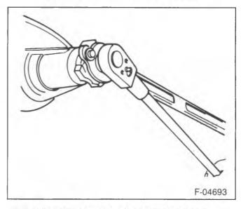
Figure 5—Removing the Drive Pinion Nut
