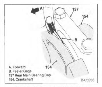
Figure 50—Measuring Crankshaft End Play
