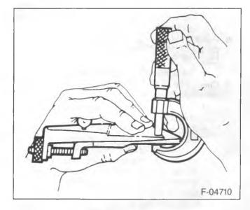
Figure 22—Measuring the Gage Plate Thickness
