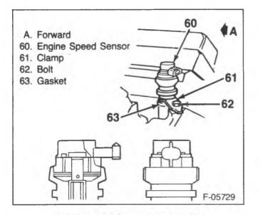
Figure 56—Oil Pump Drive Installed
