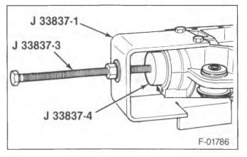
Figure 17—Installing the Outer Pinion Bearing Cup
