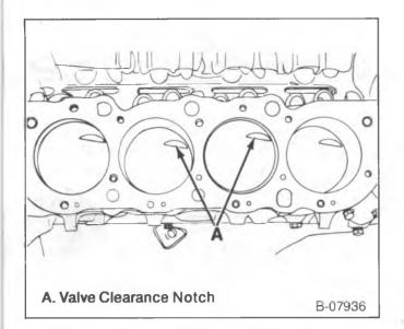
Figure 65—Piston Installed (7.4L Engines)
