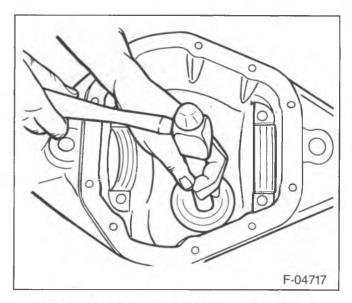
Figure 29—Installing the Pinion Inner Cup
