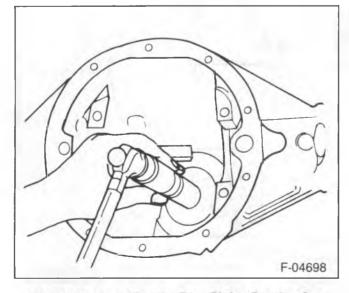
Figure 10—Installing the Rear Pinion Bearing Cup
