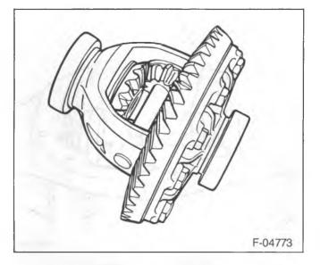
Figure 21—Differential with Master Bearings
