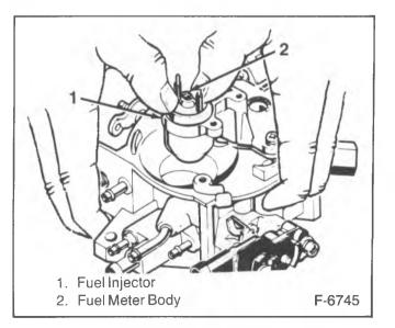
Figure 10—Installing Fuel Injector — TBI 220
