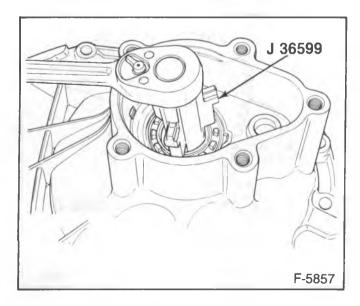
Figure 9—Turning the Adjuster Sleeve
