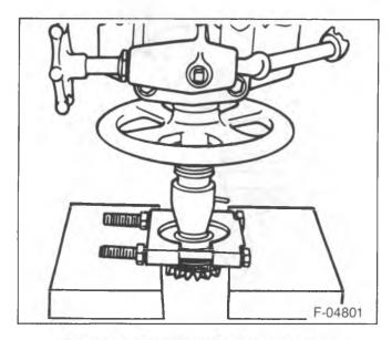
Figure 11—Removing the Thrust Sleeve
