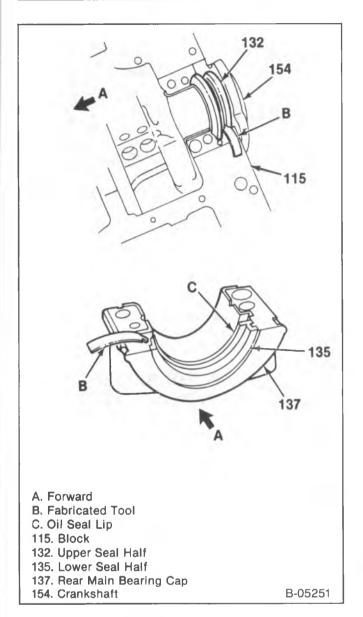
Figure 47-Crankshaft Rear Oil Seal Installation
