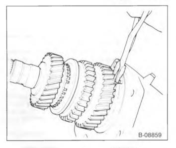
Figure 4—Removing the Mainshaft
