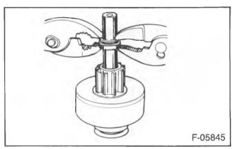
Figure 15—Forcing the Collars over the Stop Ring
