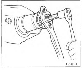
Figure 6—Pinion Flange Removal
