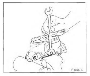
Figure 18—Installing Tube Seats
