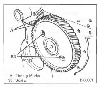
Figure 51—Timing Marks and Thrust Plate Screws
