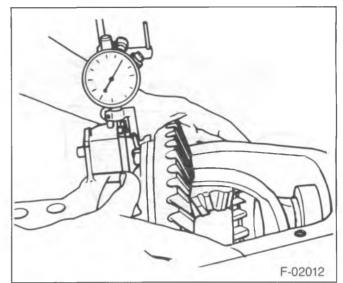
Figure 62—Determining Differential Shim Pack
