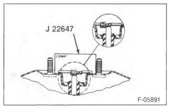
Figure 24—Gaging the Piston Rod
