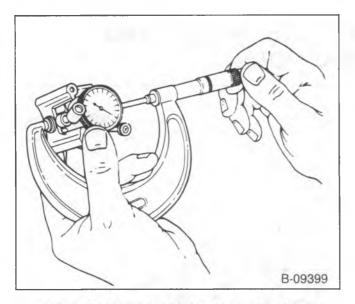
Figure 3—Measuring the Cylinder Bore Gage
