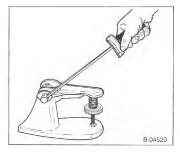
Figure 33—Measuring Valve Spring Tension
