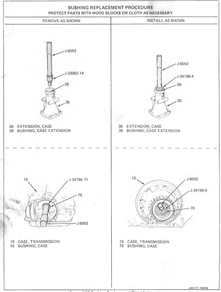
Figure 143 Bushing Replacement Procedure
