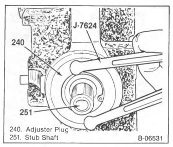
Figure 15—Bottoming the Adjuster Plug
