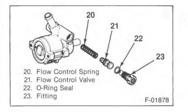
Figure 31—Removing the Fitting, Control Valve, Spring and Seal
