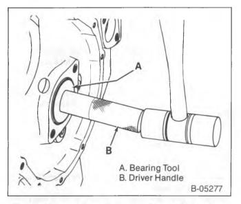
Figure 18—Replacing the Outer Camshaft Bearings
