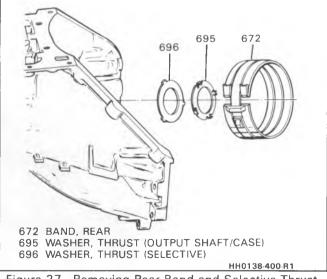
Figure 27 - Removing Rear Band and Selective Thrust Washer
