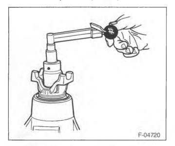
Figure 72—Checking the Pinion Preload
