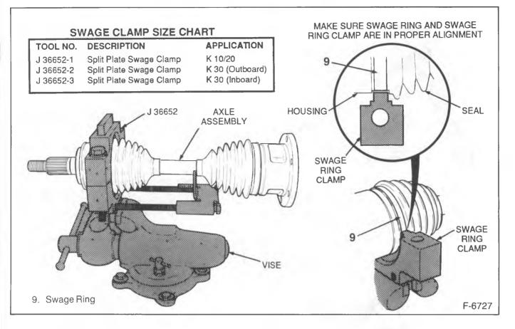
Figure 47—Installing Swage Ring
