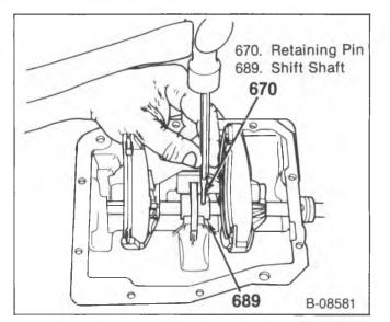
Figure 32—Removing the Shift Shaft Retaining Pin
