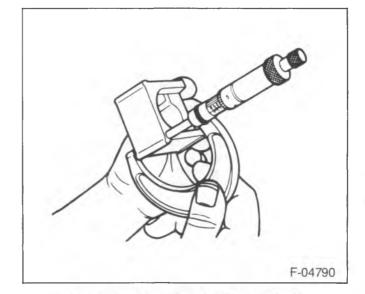
Figure 7—Measuring the Thrust Block
