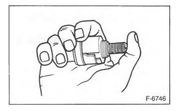
Figure 11—Adjusting Valve Pintle — Thread Type
