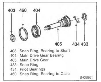
Figure 6—Main Drive Gear Components
