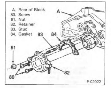
Figure 12—Rear Crankshaft Oil Seal Retainer Installation
