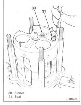
Figure 43—Installing the Discharge Crossover Tube
