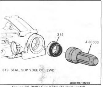
Figure 62 2WD Slip Yoke Oil Seal Install
