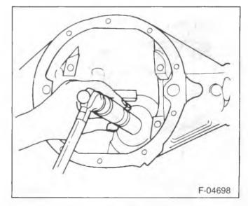
Figure 10—Installing the Rear Pinion Bearing Cup
