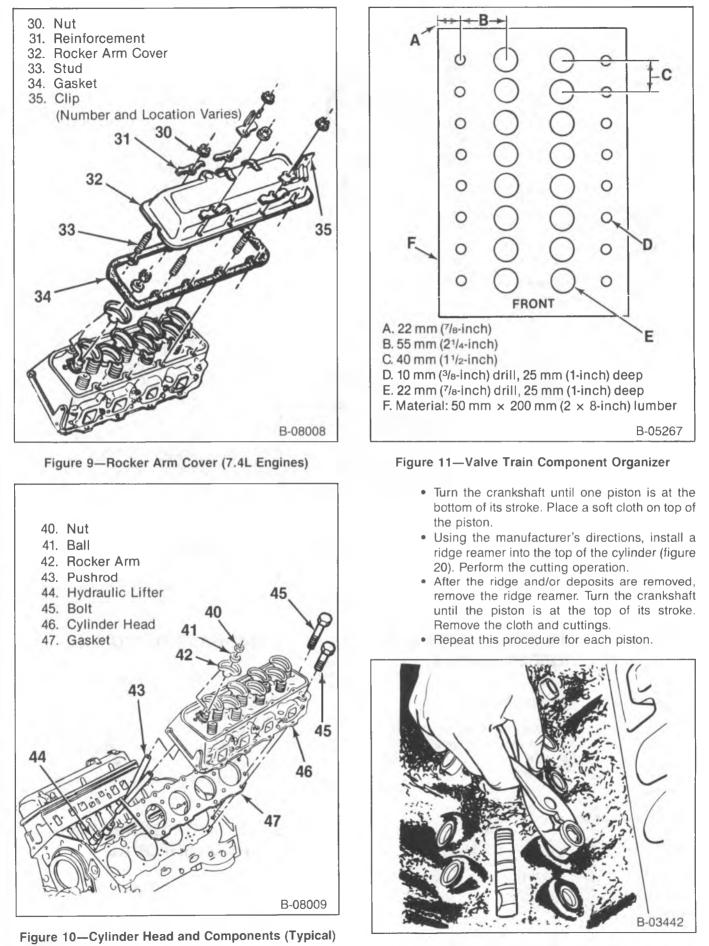
Figure 12—Removing the Hydraulic Lifter
