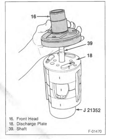
Figure 46—Installing the Front Head
