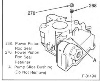
Figure 27 – Power Piston Rod Seal
