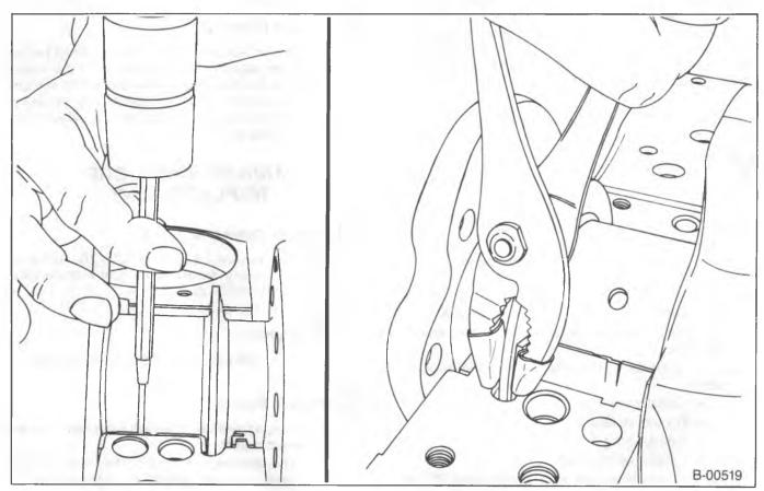
Figure 21—Removing the Upper Rear Main Bearing Insert
