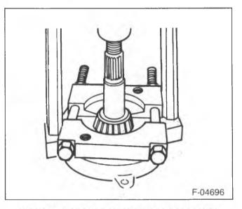
Figure 8—Removing Drive Pinion Rear Bearing
