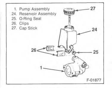
Figure 30—Removing the Reservoir
