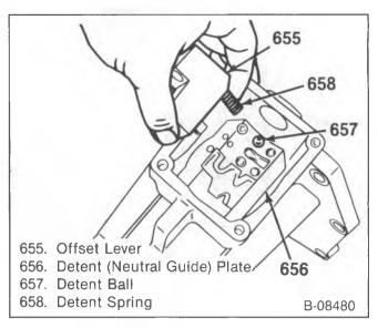
Figure 5-Detent Ball and the Spring
