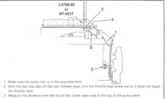
4. Adjust, if necessary, by supporting the pump lever at **S** and bending at the notch.
