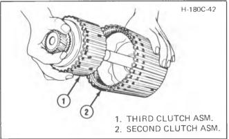
Figure 36 Installing Third Clutch Assembly Into Second Clutch Assembly
