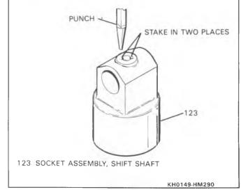
Figure 84 Staking Shift Shaft Socket Assembly
