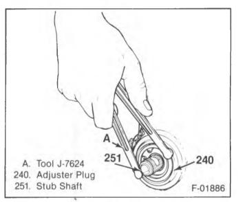
Figure 6—Removing the Adjuster Plug
