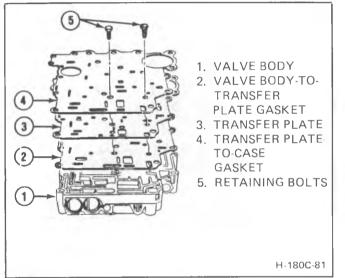
Figure 64 Removing Transfer Plate
