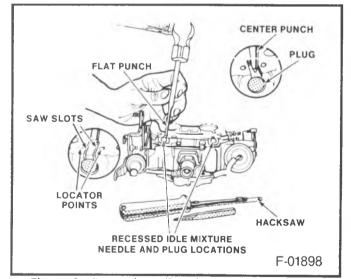
Figure 8 – Removing Idle Mixture Needle Plugs
