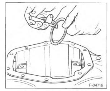
Figure 27—Measuring the Shims
