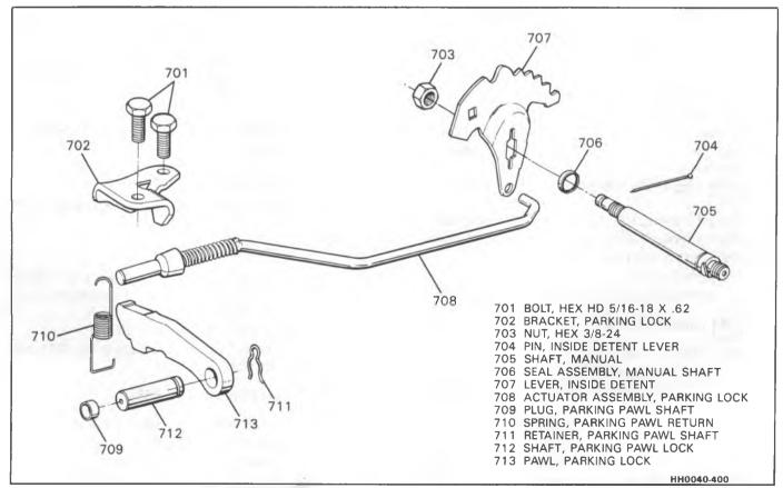
Figure 31 - Park Lock Pawl and Actuator Assembly
