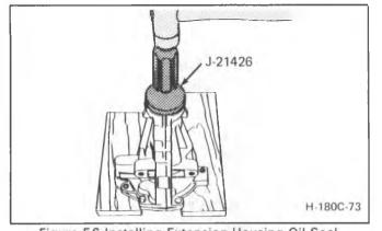
Figure 56 Installing Extension Housing Oil Seal
