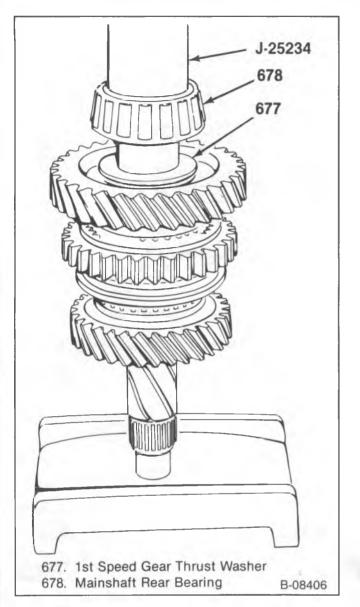
Figure 24—Installing the Mainshaft Rear Bearing
