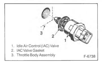
Figure 3—Thread Mounted Type IAC Valve
