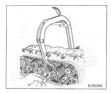
Figure 35—Compressing the Valve Springs
