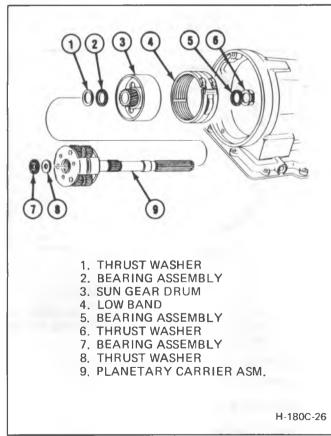
Figure 20 Installing Planetary Carrier
