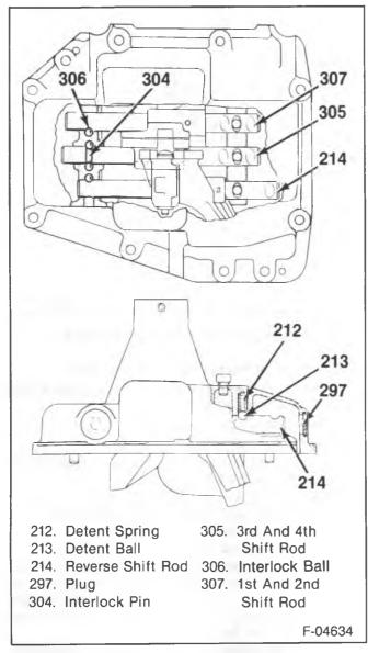
Figure 34A—R/V/P Interlock Shuttles and Pin
