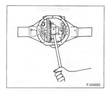
Figure 2—Removing the Differential Case
