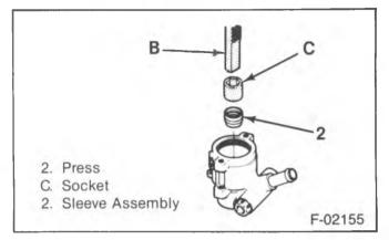
Figure 40—Install Sleeve Assembly
