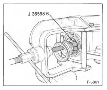
Figure 15—Removing the Outer Pinion Bearing and Seal
