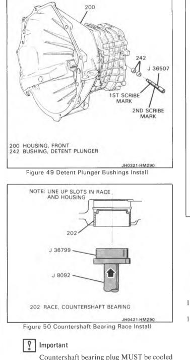
at O° C (32° F) for a MINIMUM of 20 minutes before installation.
