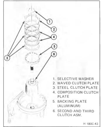
Figure 37 Installing Second/Third Clutch Assemblies Into Case
