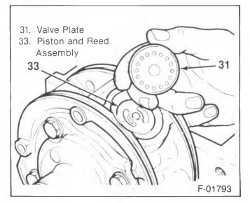
Figure 23—Replacing the Discharge Plate
