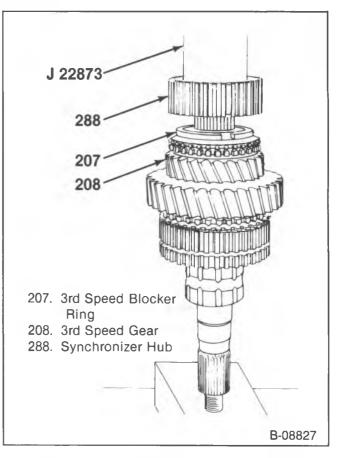
Figure 20 –Installing the 3rd and 4th Speed Synchronizer Hub
