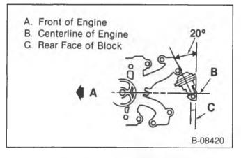
Figure 58—Vacuum Pump Installed
