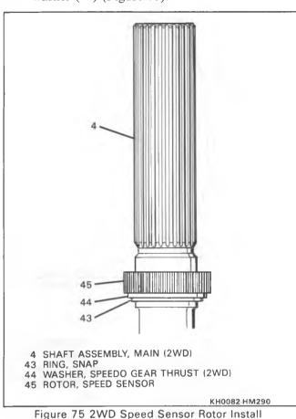
13. 2WD Speed sensor rotor (45) HEATED.
