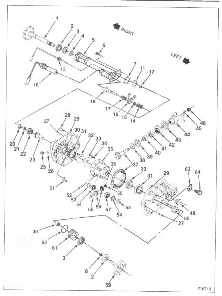
Figure 3—Front Axle Components (K35 Models)
