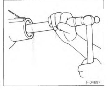
Figure 9—Installing Front Pinion Bearing Cup
