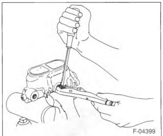
Figure 17—Removing Tube Seats
