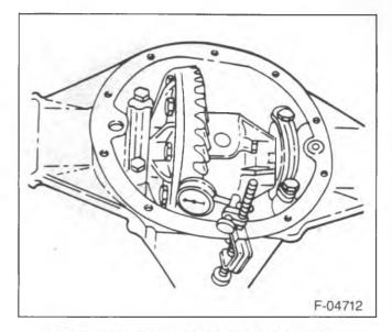
Figure 22—Checking Ring Gear Backlash
