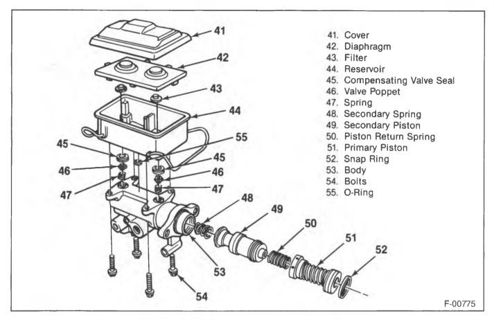
Figure 19—Bendix Master Cylinder Components
