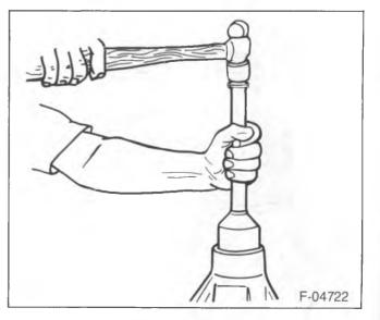
Figure 74—Installing the Pinion Seal
