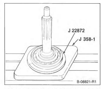
Figure 9—Removing the Main Drive Gear Bearing
