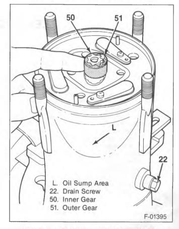
Figure 50—Positioning the Oil Pump Gears
