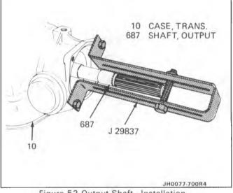
Figure 52 Output Shaft - Installation
