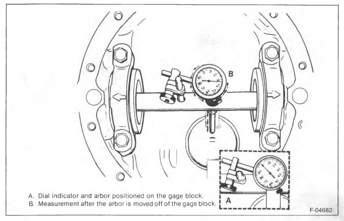
Figure 13—Checking Pinion Depth
