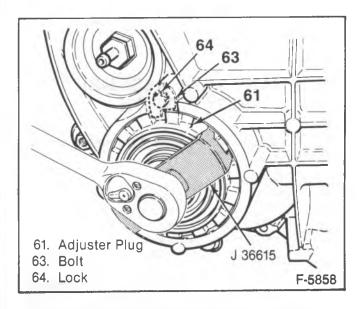
Figure 29—Turning the Adjuster Plug (K35 Models)
