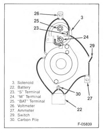
Figure 9—Hold-In Winding Test Connections
