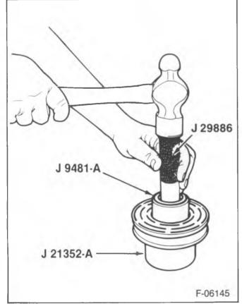
Figure 32—Pulley Rotor and Bearing Installation
