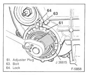
Figure 10—Turning the Adjuster Plug (K35 Models)
