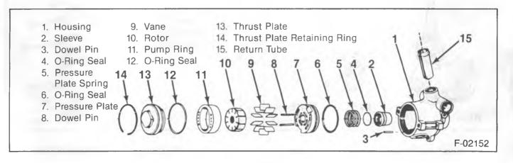
Figure 37—Pump Housing Components
