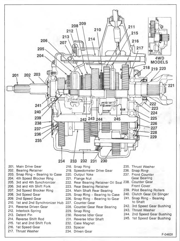
Figure 1B—C/K Four Speed Transmission
