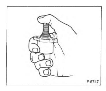
Figure 12—Adjusting Valve Pintle — Flange Type
