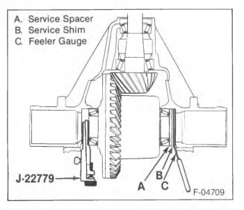
Figure 21—Measuring Side Bearing Shim Requirements
