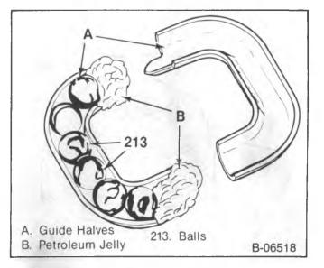
Figure 13—Retaining the Balls in the Ball Guide
