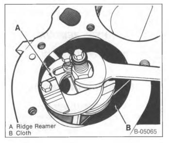
Figure 13—Removing the Cylinder Ridge
