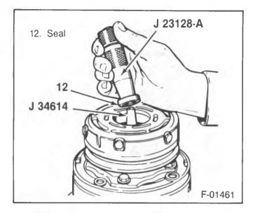
Figure 15—Removing the Shaft Seal with J 23128-A
