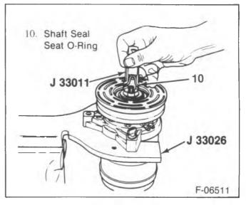
Figure 25 — Installing the Seal Seat O-Ring
