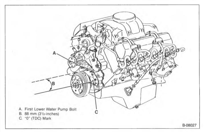
Figure 49—Aligning the Timing Mark
