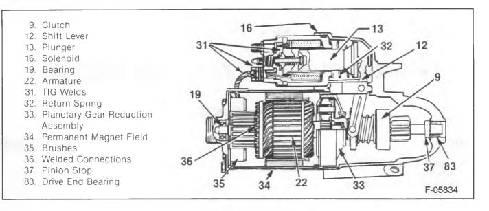
Figure 1—PG-200 (PMGR) Starting Motor
