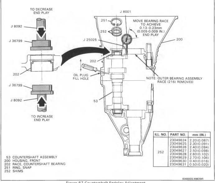
Figure 67 Countershaft Endplay Adjustment
