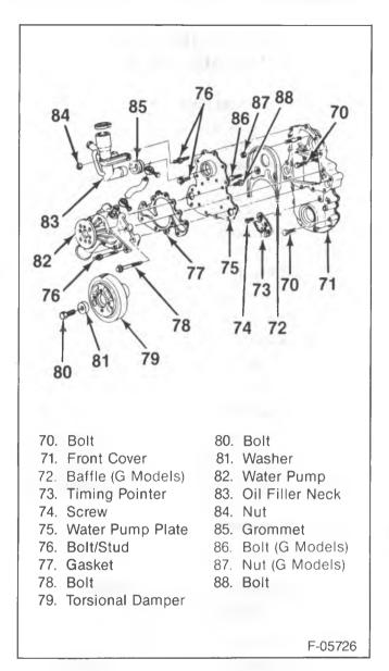
Figure 39—Front Cover and Components
