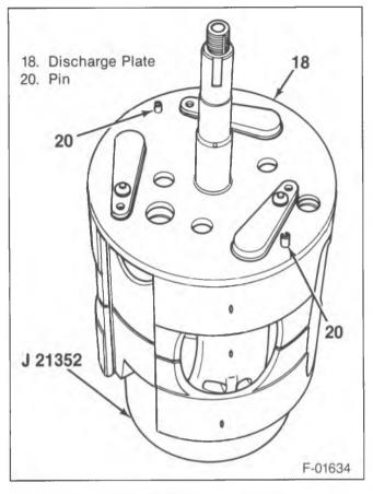
Figure 45—Installing the Front Discharge Valve Plate
