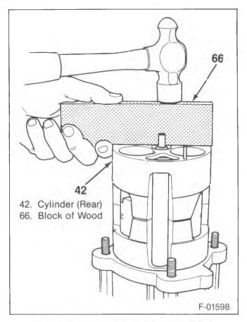
Figure 31—Assembling the Cylinder Halves
