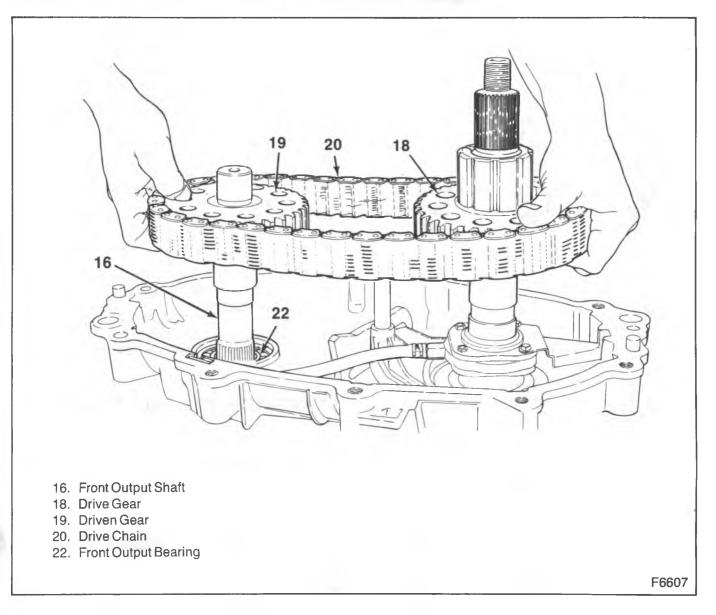
Figure 10—Removing the Drive Chain
