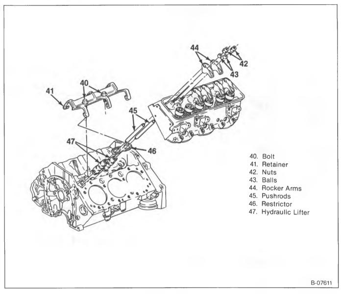
Figure 4—Valve Train Components
