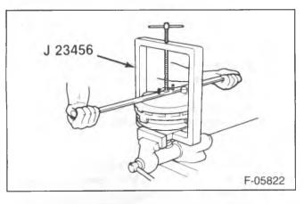
Figure 21—Unlocking and Locking Booster
