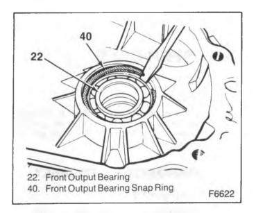
Figure 20—Removing the Front Output Bearing Snap Ring
