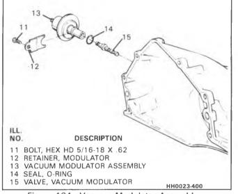
Figure 101 - Vacuum Modulator Assembly
