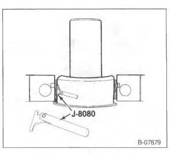
Figure 13—Removing the Main Bearing Insert
