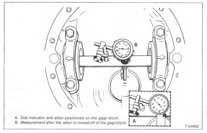
Figure 10—Checking Pinion Depth
