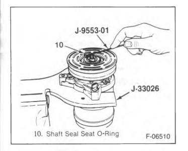
Figure 24 — Removing the Shaft Seal Seat O-Ring
