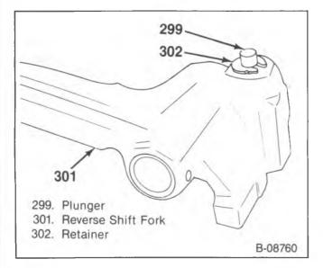
Figure 32—Plunger Retainer
