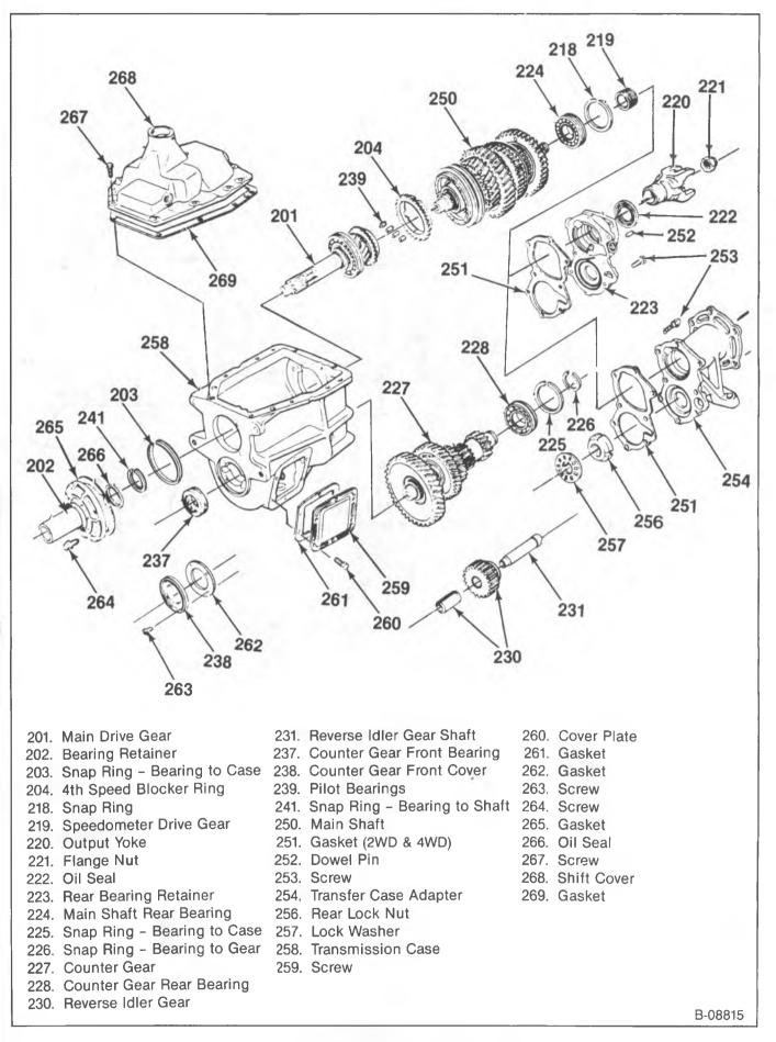
Figure 2—Transmission Components
