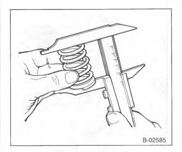
Figure 34—Measuring Valve Spring Length
