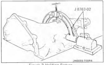
Figure 3 Holding Fixture
