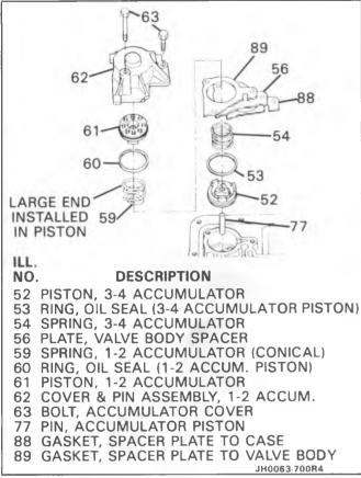
Figure 11 Accumulator Assembly
