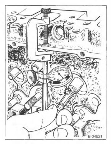
Figure 32—Measuring Stem to Bore Clearance (Typical)
