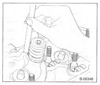
Figure 41—Measuring Valve Spring Installed Height
