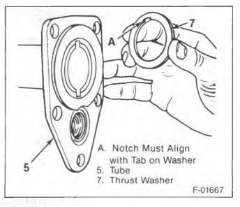
Figure 34—Installing the Thrust Washer
