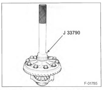
Figure 16—Installing the Differential Side Bearings
