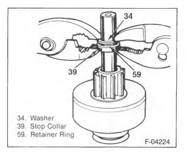
Figure 17—Forcing the Collar over the Retainer Ring
