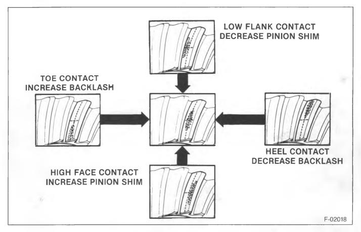
Figure 26—Gear Tooth Pattern
