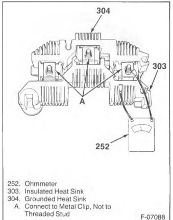
Figure 12—Rectifier Bridge Check
