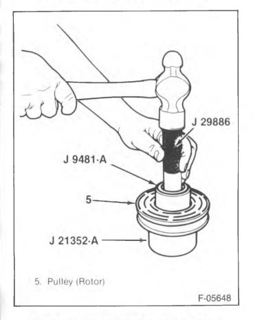
Figure 13 — Installing the Pulley Rotor Bearing
