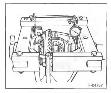
Figure 45—Spreading the Differential Case
