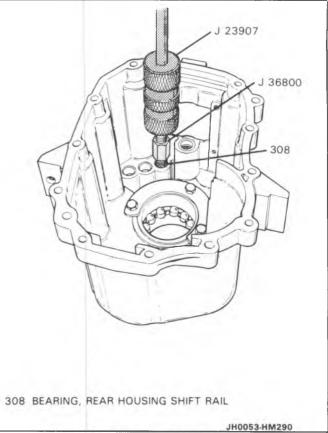
Figure 57 Removing Shift Rail Bearing
