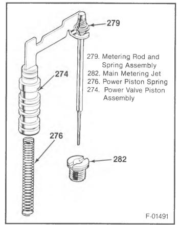
Figure 34 – Power Piston, Metering Rod and Jet
