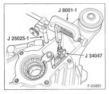
Figure 27—Measuring Backlash at the Ring Gear
