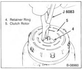
Figure 8—Removing the Rotor and Bearing Assembly Retainer Ring
