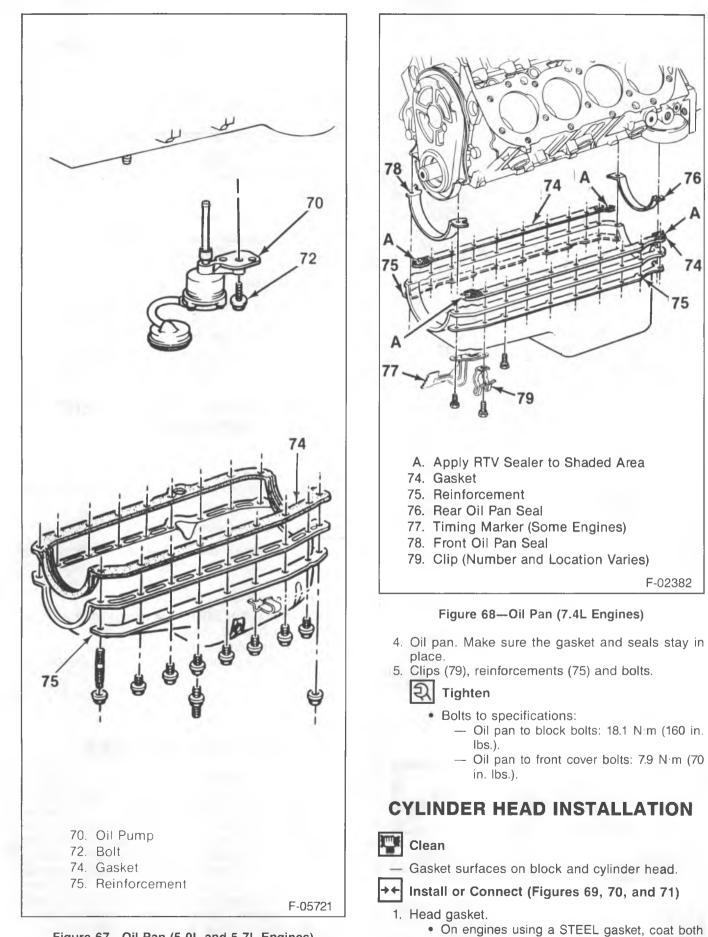
Figure 67—Oil Pan (5.0L and 5.7L Engines)
