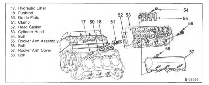
Figure 7—Cylinder Head and Components
