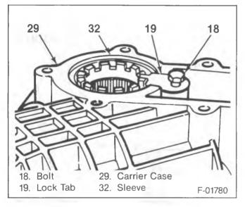
Figure 7—Removing the Lock Tabs
