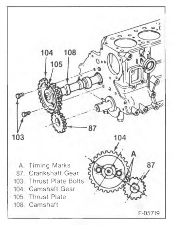
Figure 43—Camshaft and Timing Gears
