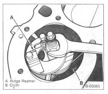
Figure 14—Removing the Cylinder Ridge
