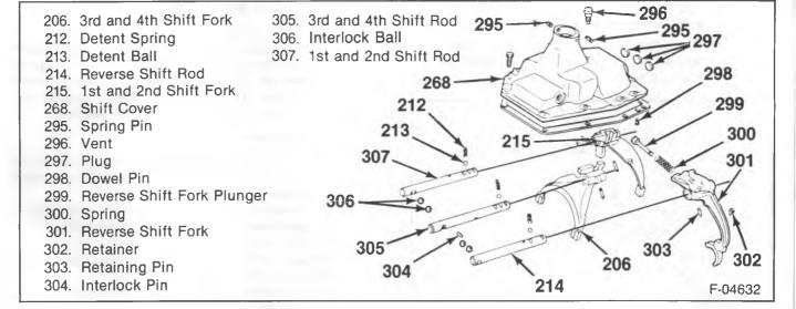
Figure 30A—R/V/P Shift Cover and Components
