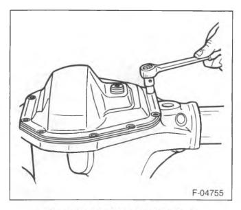
Figure 43—Removing the Axle Cover
