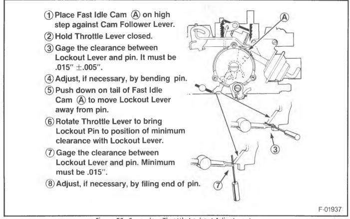
Figure 50 - Secondary Throttle Lockout Adjustment
