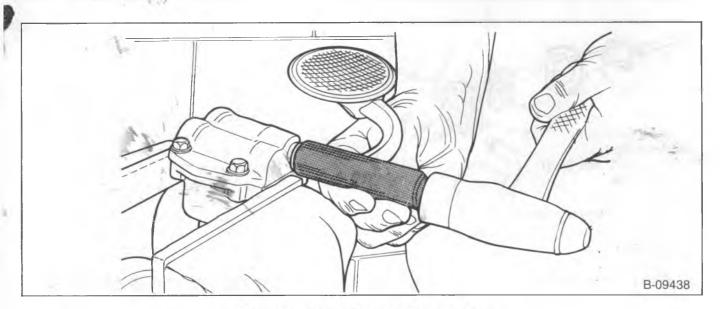
Figure 18—Installing the Oil Pump Screen
