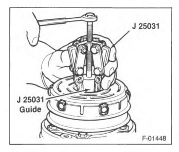
Figure 10—Removing the Clutch Rotor Assembly
