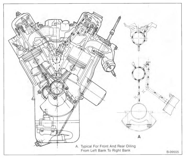
Figure 2—Engine Lubrication Diagram
