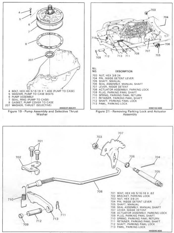
Figure 20 - Park Lock Pawl and Actuator Assembly
