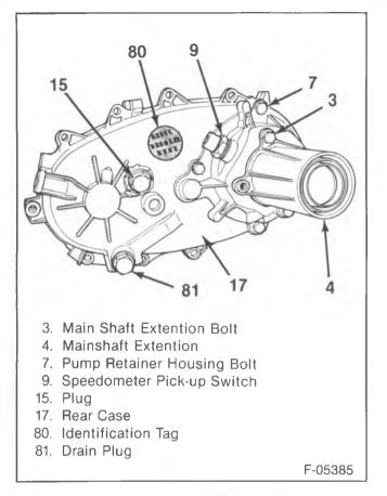
Figure 3—Rear View — 241 Transfer Case
