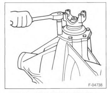
Figure 4—Removing the Pinion Cage
