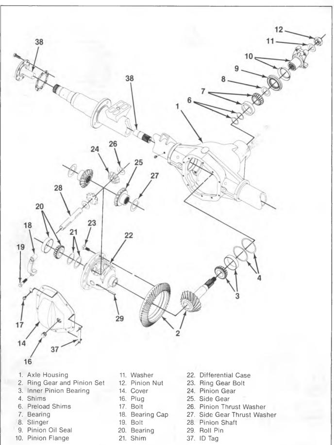
Figure 1—Rear Axle Components
