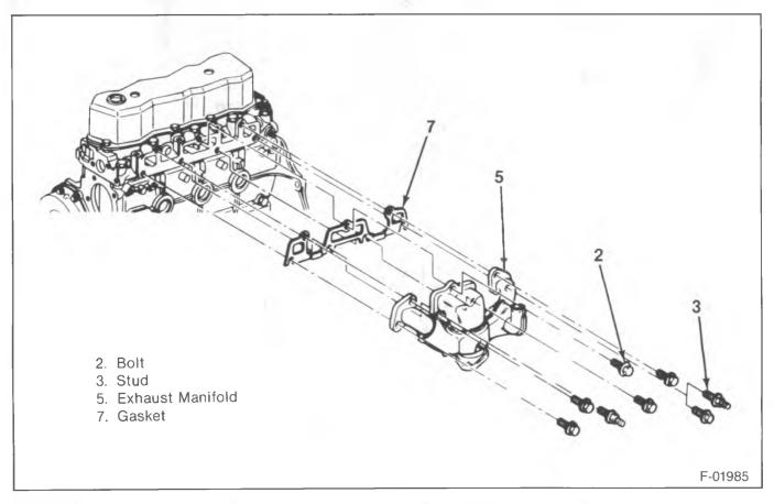
Figure 7—Exhaust Manifold Components
