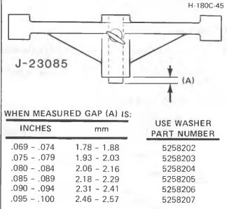
FOLLOWING THE PROCEDURE SHOULD RESULT IN FINAL END-PLAY FROM 0.36 mm TO 0.79 mm (.014 in. TO .031 in.)
