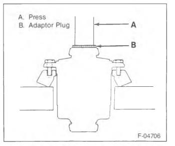
Figure 18—Installing the Ring Gear to the Case
