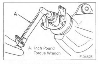
Figure 4—Checking Pinion Preload
