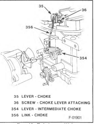
Figure 14 – Choke Lever and Link
