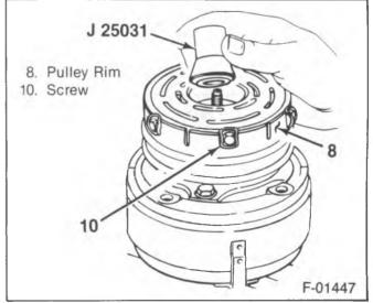
Figure 9—Installing the Rotor and Bearing Guide
