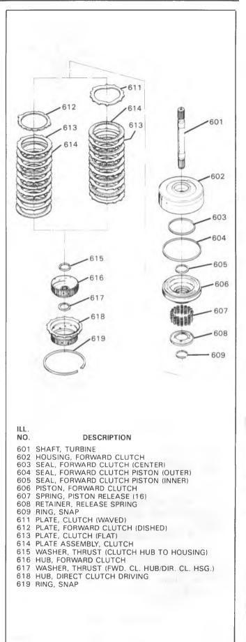
Figure 65 - Forward Clutch Assembly
