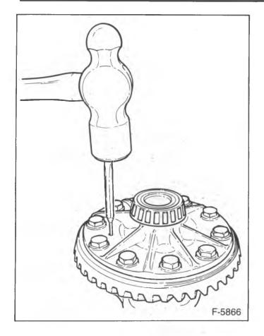
Figure 18—Removing the Pin (K15-25 Models)
