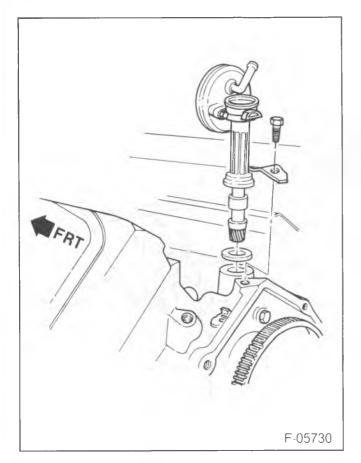
Figure 2—Vacuum Pump (R-V Models)
