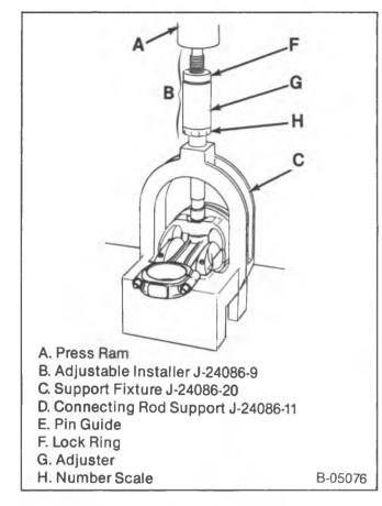
Figure 13-Installing the Piston Pin
