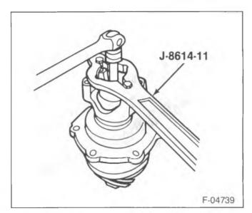
Figure 5—Removing the Drive Pinion Nut
