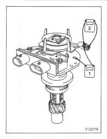
Figure 27—Testing the Pickup Coil
