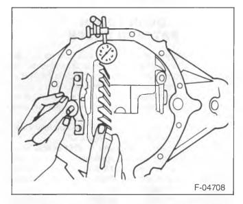
Figure 20—Installing Side Bearing Gaging Tool
