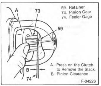
Figure 19—Measuring Pinion Clearance
