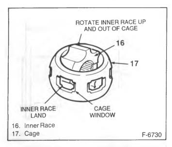
Figure 50—Separating Inner Race and Cage
