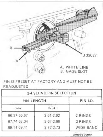
Figure 8 Servo Pin Length
