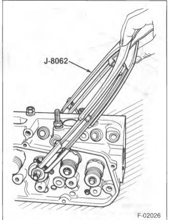
Figure 35—Compressing the Valve Springs
