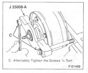
Figure 24—Installing the Shell
