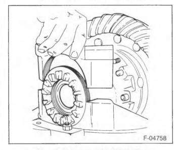
Figure 6—Removing the Bearing Cap
