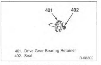
Figure 14—Bearing Retainer and the Seal
