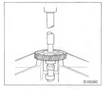
Figure 28—Removing the Camshaft Gear
