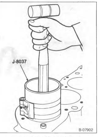
Figure 34—Installing the Piston
