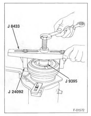
Figure 7—Removing the Pulley and Bearing
