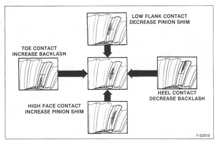
Figure 21—Gear Tooth Pattern
