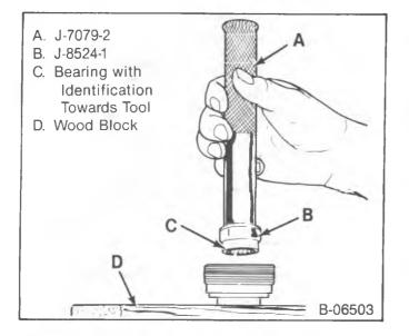
Figure 14—Installing the Needle Bearing
