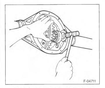
Figure 23—Installing the Final Preload Shim
