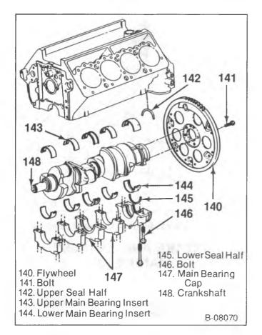
Figure 15—Crankshaft and Components
