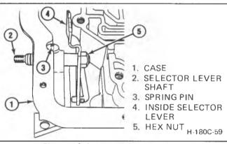
Figure 18 Selector Lever Installed
