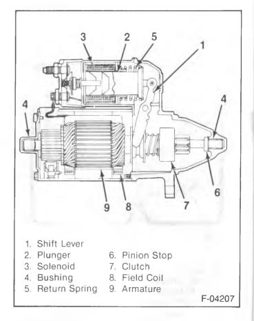
Figure 1—SD-200 (5MT) Starting Motor
