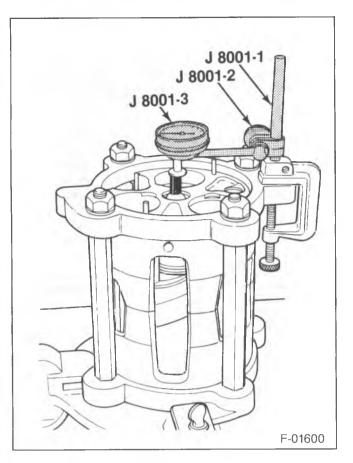
Figure 34—Gaging the Rear Thrust Plate
