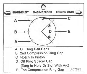
Figure 48—Piston Ring Gap Location
