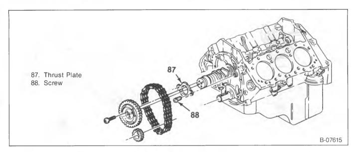
Figure 7—Camshaft and Components
