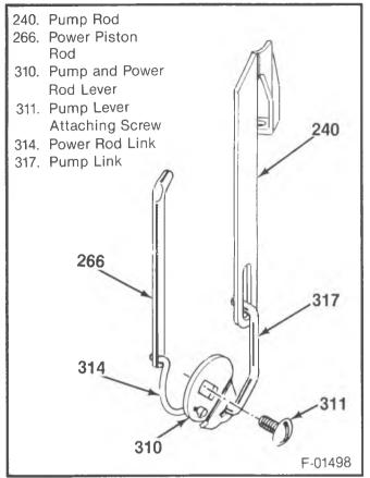
Figure 35 – Pump and Power Piston Linkage
