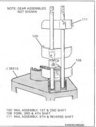
Figure 72 Proper Positions of Shift Forks and Rails
