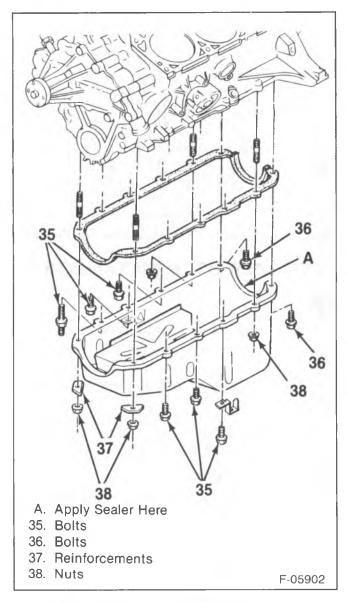
Figure 38—Oil Pan Installation
