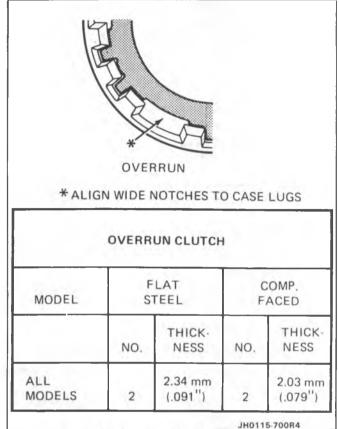
Figure 67 Overrun Clutch Plate Chart
