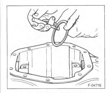
Figure 68—Measuring the Shims
