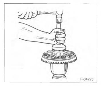
Figure 38—Installing the Differential Bearings
