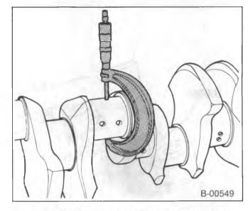
Figure 25—Measuring the Crankshaft Journals
