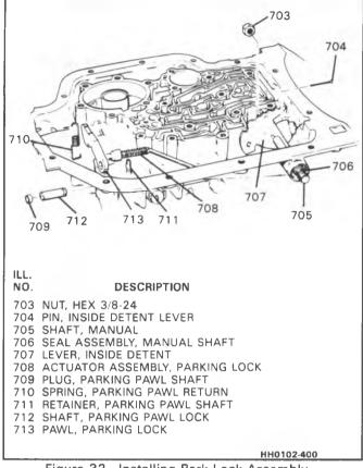
Figure 32 - Installing Park Lock Assembly
