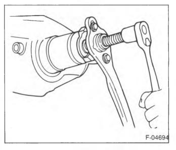
Figure 15—Installing the Pinion Flange
