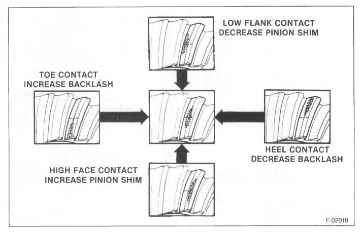
Figure 30—Gear Tooth Contact Pattern
