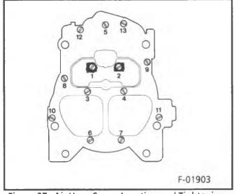
Figure 37 - Air Horn Screw Location and Tightening Sequence
