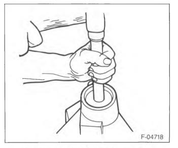
Figure 70—Installing the Pinion Front Cup
