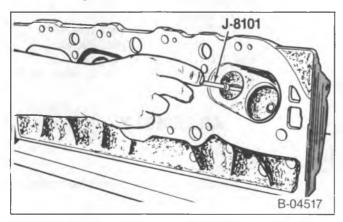
Figure 31—Cleaning the Valve Guides (Typical)
