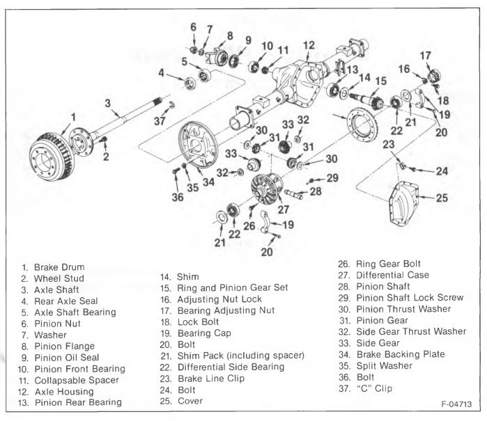
Figure 1—Rear Axle Components
