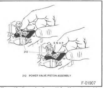
Figure 19 – Removing Power Valve Piston Assembly
