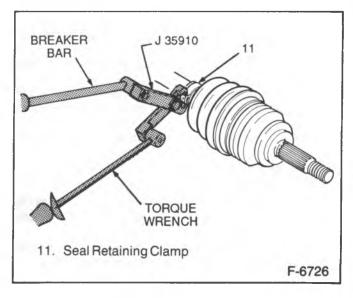
Figure 46—Installing Seal Retaining Clamp
