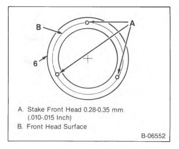
Figure 19—Clutch Coil Staking Locations
