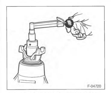
Figure 32—Checking the Pinion Preload
