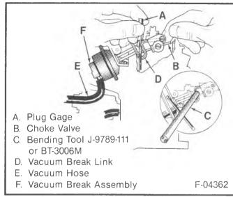
Figure 42 – Vacuum Break Adjustment
