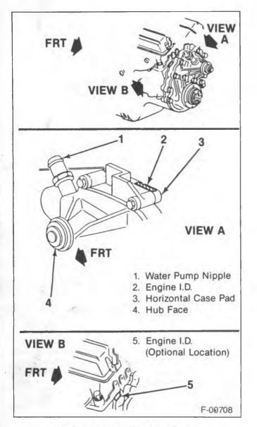
Figure 7-2.8L Engine I.D. Location
