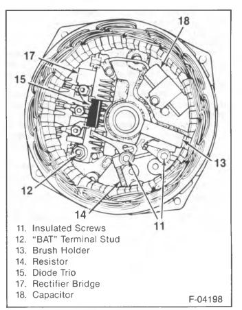
Figure 7—Slip Ring End Frame: 17-SI 100
