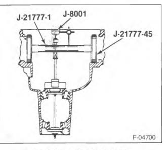
Figure 12—Pinion Depth Tools
