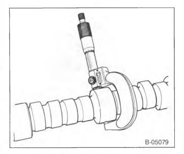
Figure 19—Checking the Camshaft Journals
