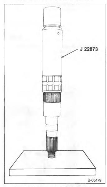
Figure 16 -Installing the 2nd Speed Bushing
