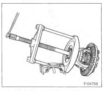
Figure 6—Removing the Differential Side Bearings
