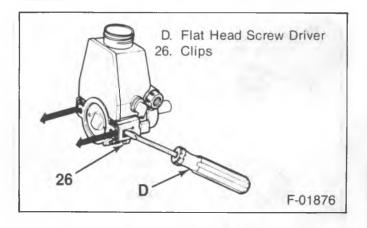
Figure 29—Removing the Reservoir Clips
