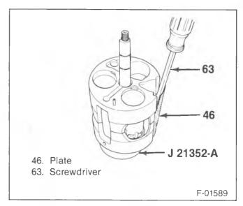
Figure 22—Removing the Rear Suction Reed Plate
