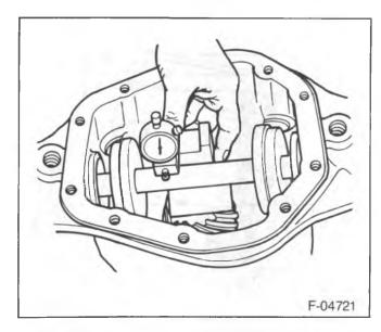
Figure 32—Checking the Pinion Depth Setting
