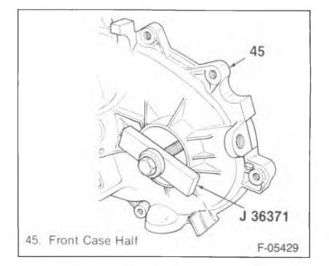
Figure 12—Installing the Front Output Bearing with J 3637
