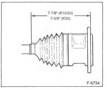
Figure 53—Installing Tri-pot to Housing
