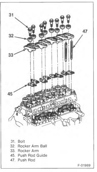
Figure 11—Valve Train Components
