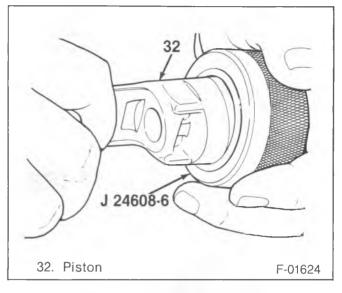
Figure 38—Sizing the Piston Ring
