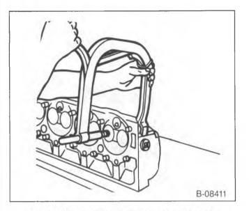
Figure 21—Compressing the Valve Springs
