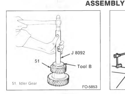
Figure 9—Installing the Bearing Cup
