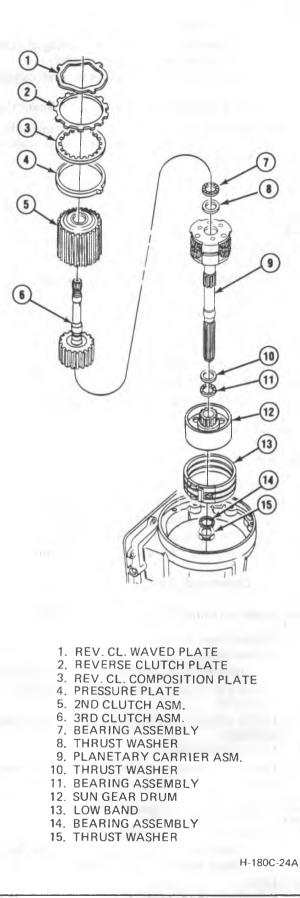
Figure 15 Internal Parts
