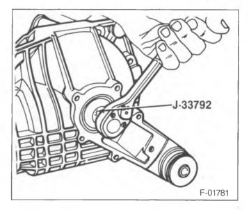
Figure 24—Adjusting the Sleeve
