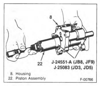
Figure 7—Installing the Piston Assembly
