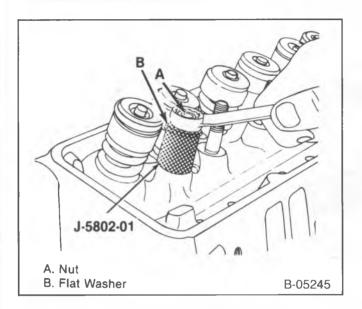
Figure 36—Removing the Rocker Arm Stud
