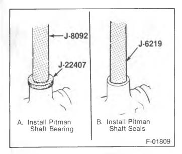
Figure 20—Installing the Pitman Shaft Bearing and Seals
