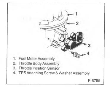
Figure 8—Throttle Position Sensor (TPS) TBI 700
