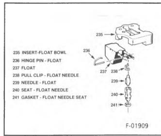
Figure 22 - Float, Needle and Seat
