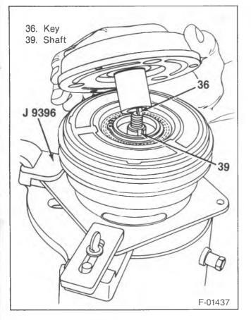
Figure 4—Aligning the Drive Plate Key
