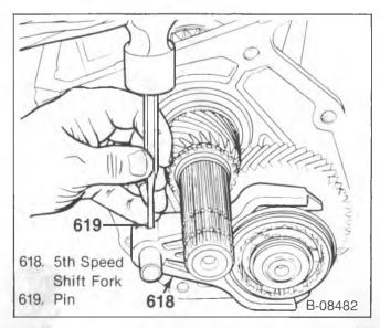
Figure 7—Removing the 5th Speed Shift Fork Pin
