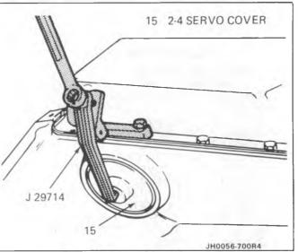
Figure 4 Servo Cover Removal
