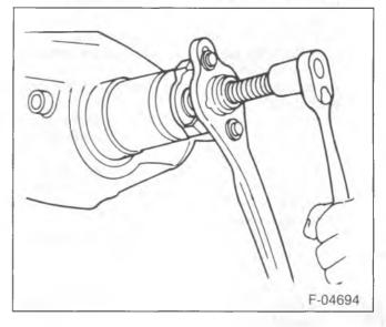
Figure 16—Installing the Pinion Flange
