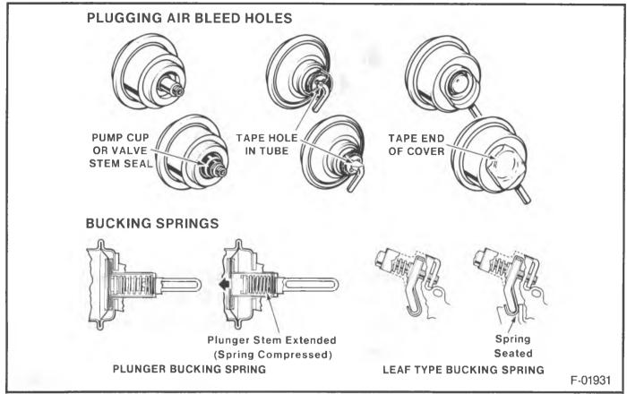
Figure 46 - Vacuum Break Adjustment Information
