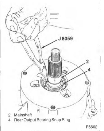
Figure 5—Removing the Output Bearing Snap Ring
