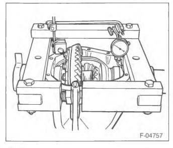
Figure 4—Spreading the Differential Case
