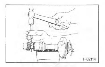
Figure 25—Removing the Roll Pin
