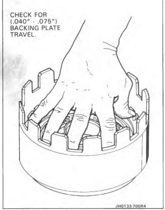
Figure 85 Reverse Input Backing Plate Selection
