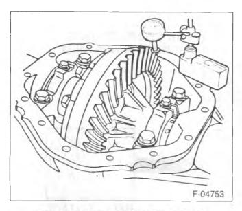
Figure 19—Measuring Gear Set Backlash
