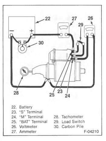
Figure 3—No Load Test Hookup
