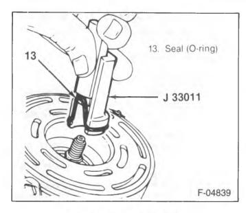
Figure 27—Installing the Seal
