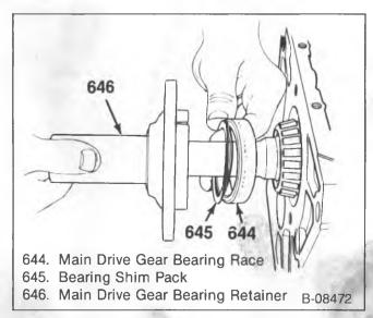
Figure 10-Main Drive Gear Shim Pack
