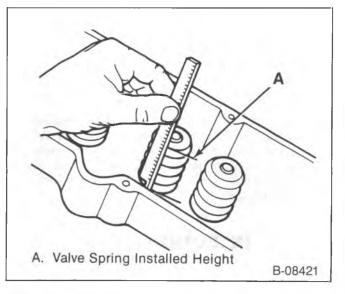
Figure 26—Measuring Valve Spring Installed Height (Typical)
