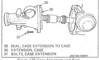
Figure 135 Case Extension and Seal
