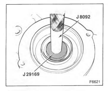
Figure 19—Removing the Front Input Bearing
