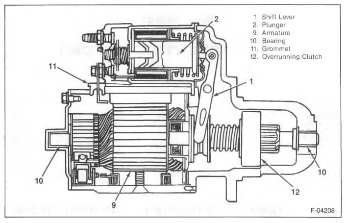
Figure 2—SD-300 (10MT) Starting Motor
