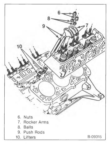
Figure 9—Valve Train Components
