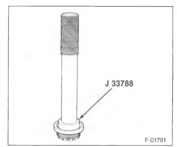
Figure 23—Installing the Sleeve Bearing
