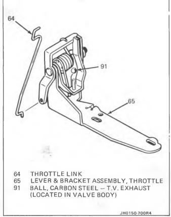
Figure 109 Throttle Lever and Bracket Assembly
