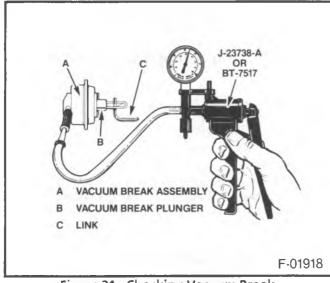
Figure 31 - Checking Vacuum Break
