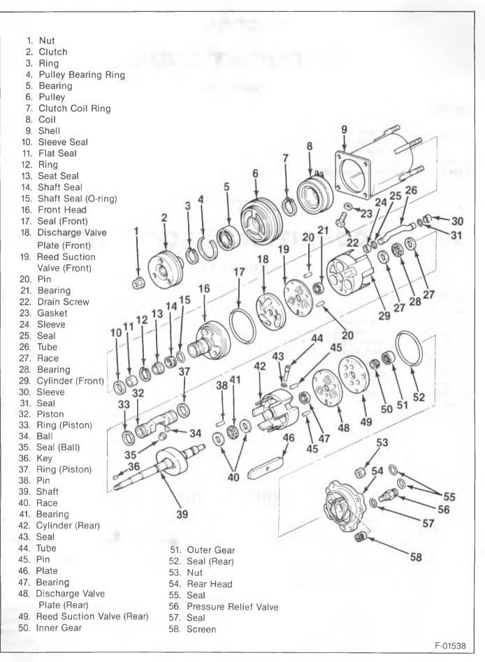
Figure 1—Compressor Component View
