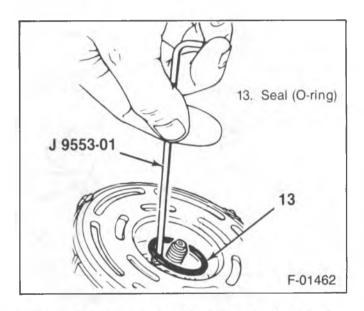
Figure 16—Removing and Installing the Shaft Seal
