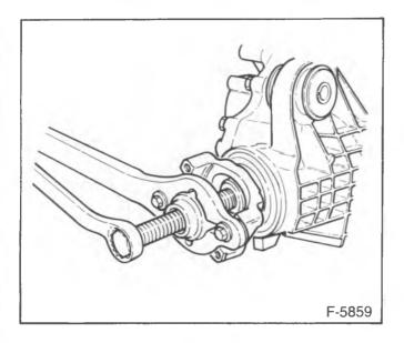
Figure 12—Removing the Pinion Flange
