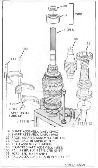
Figure 71 Countershaft and Reverse Idler Assembly Install
