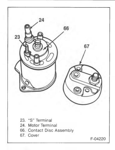
Figure 12—Solenoid Disassembled
