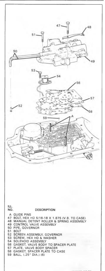
HH0098-400-R2 Figure 96 - Installing Control Valve Assembly
