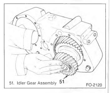
Figure 11—Installing the Idler Gear Assembly
