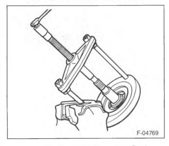
Figure 16—Removing the Pinion Inner Bearing
