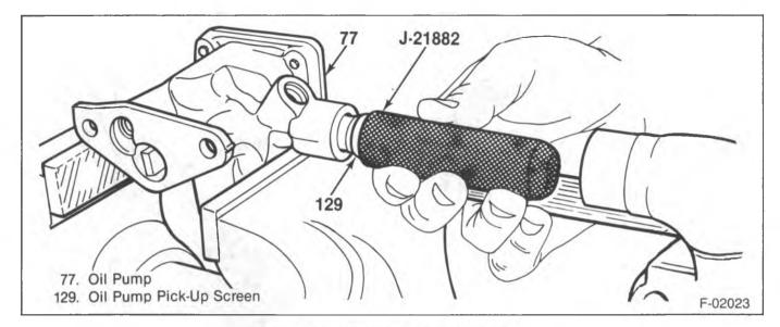
Figure 33—Installing the Oil Suction Pipe
