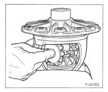
Figure 58—Installing the Pinion Gears
