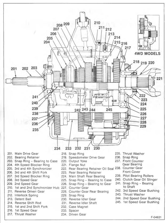
Figure 1A—R/V/P Four Speed Transmission
