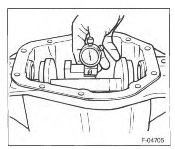
Figure 26—Scooter Gage on the Height Block
