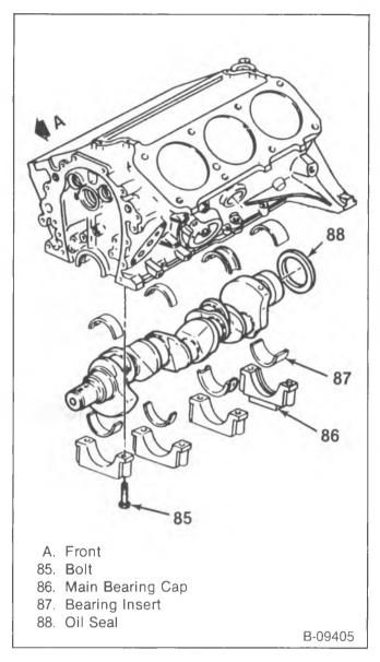
Figure 16—Crankshaft Installation
