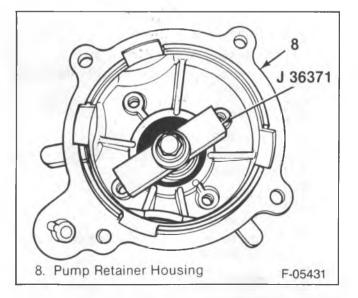
Figure 14—Installing the Pump Housing Bearing with J 36371
