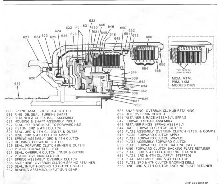
Figure 81 Input Clutch Assembly
