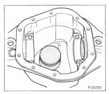
Figure 22—Master Pinion Block
