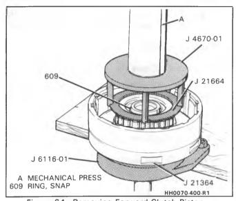
Figure 64 - Removing Forward Clutch Piston
