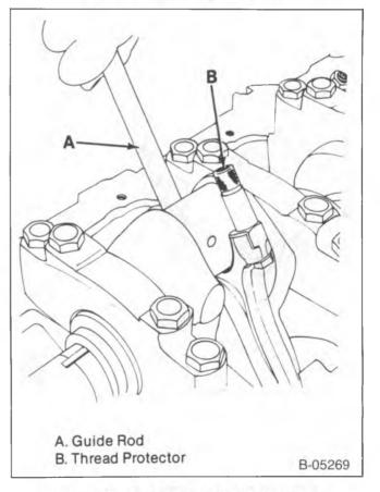
Figure 35—Guiding the Connecting Rod
