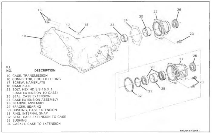
Figure 28 - Transmission Case And Extension Assembly
