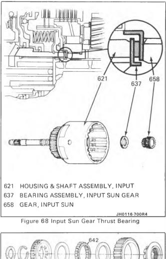
637 638 639 643 644 641 THE NOTCHES ABOVE EACH SPRAG MUST POINT UP AS SHOWN WHEN ASSEMBLED INTO THE OUTER RACE 637 BEARING ASSEMBLY, INPUT SUN GEAR 638 SNAP RING, OVERRUN CLUTCH HUB RET. 639 HUB, OVERRUN CLUTCH HUB RET. 639 HUB, OVERRUN CLUTCH HUB RET. 639 HUB, OVERRUN CLUTCH HUB RET. 634 644 641 644 RACE, FORWARD SPRAG ASSEMBLY 644 RACE, FORWARD CLUTCH OUTER JH0117.700R4.81
