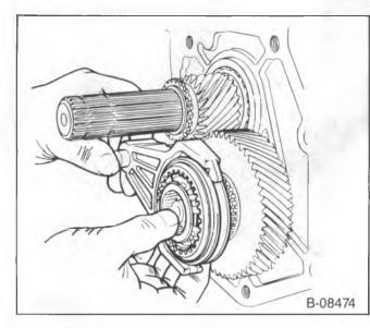
Figure 8—Removing the 5th Speed Shift Fork and the Synchronizer
