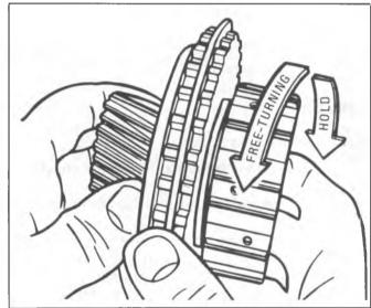
Figure 30 Testing Sprag Assembly
