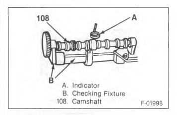
Figure 25—Measuring Camshaft Journal Runout
