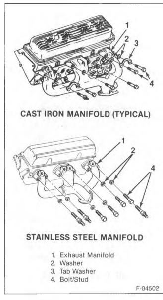
Figure 4—Exhaust Manifold (5.0L and 5.7L Engines)
