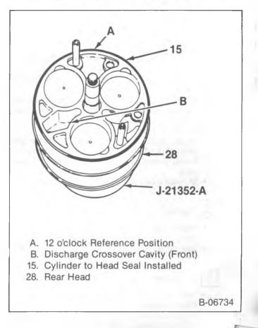
Figure 35 — Installing the Front Head
