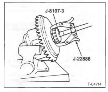
Figure 3—Removing Differential Side Bearings
