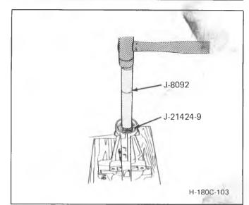
Figure 81 Removing or Installing Extension Housing Bushing
