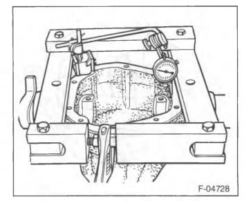
Figure 38—Mounting the Carrier Spreader
