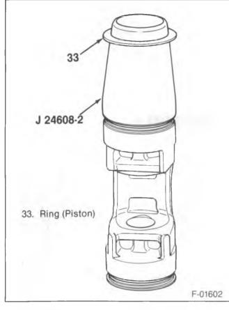
Figure 36—Piston Ring Position and Installer Guide
