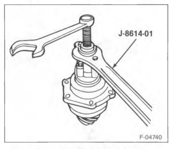
Figure 6—Removing the Pinion Flange
