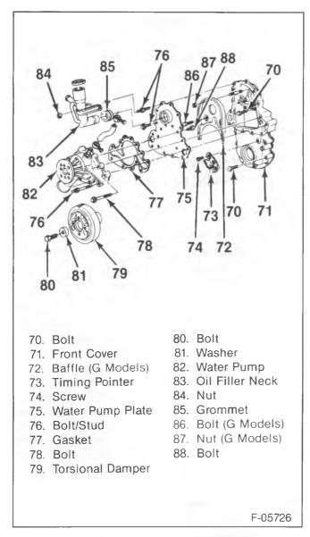
Figure 8—Front Cover and Components
