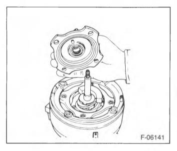
Figure 18—Removing the Front Head Assembly
