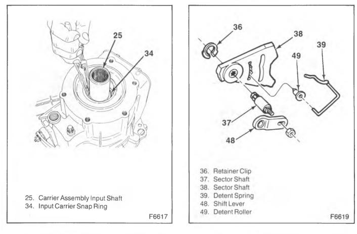
Figure 15—Removing the Carrier Assembly Snap Ring
