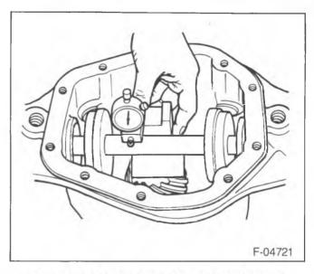
Figure 73—Checking the Pinion Depth Setting
