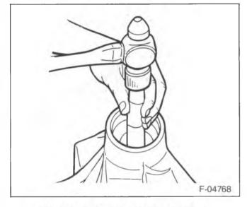
Figure 15—Removing the Bearing Cups
