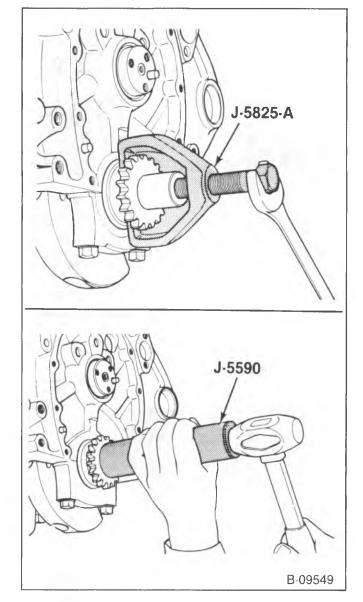
Figure 31—Crankshaft Sprocket Replacement (5.0L and 5.7L Engines)
