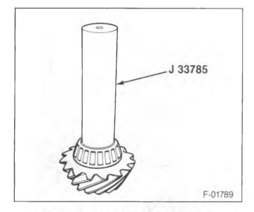
Figure 20-Installing the Pinion Bearing
