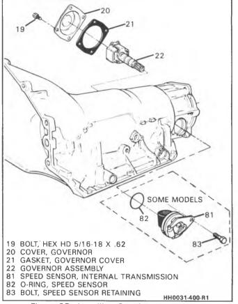
Figure 85 - Installing Governor Assembly
