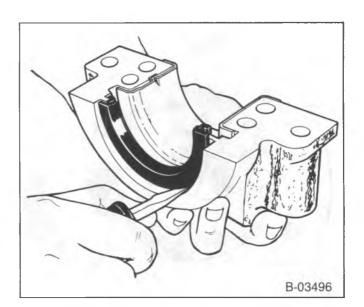
Figure 25—Removing the Rear Crankshaft Seal (7.4L Engines)
