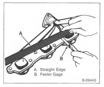
Figure 18—Checking Manifold Flange Alignment
