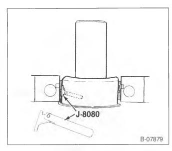
Figure 17—Removing or Installing the Main Bearing Insert
