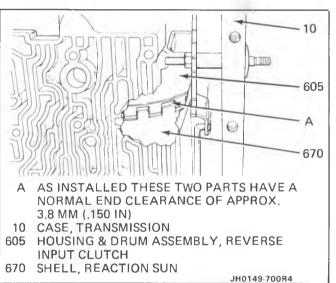
Figure 108 Clearance Between Reverse Input Clutch and the Sun Gear Shell
