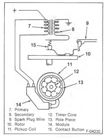
Figure 4—Basic Wiring Schematic
