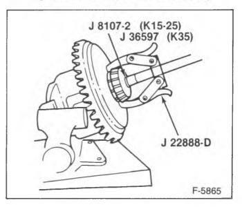
Figure 17—Removing the Side Bearings
