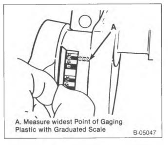
Figure 38—Measuring the Gaging Plastic
