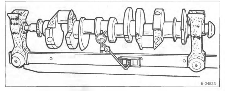
Figure 48—Checking Crankshaft Run-Out
