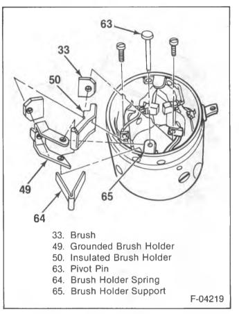
Figure 11—Replacing Brushes on the SD-300 (10MT)
