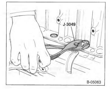
Figure 13—Removing the Valve Lifters
