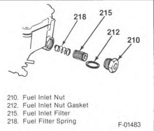
Figure 12 - Fuel Inlet Nut and Filter
