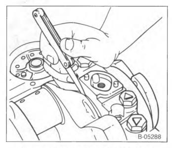
Figure 26—Measuring Crankshaft End Play
