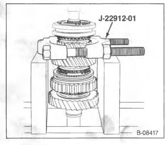
Figure 19—Removing the 3rd and 4th Synchronizer
