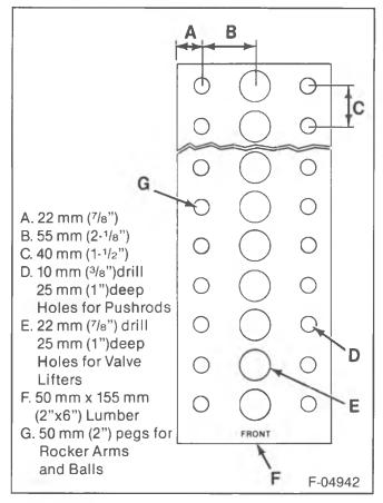
Figure 12—Valve Train Component Rack
