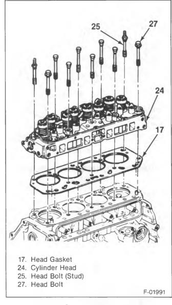
Figure 13—Cylinder Head Components
