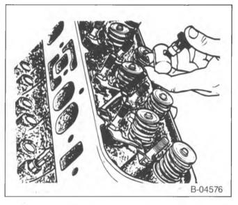
Figure 11—Removing the Hydraulic Lifter (Typical)
