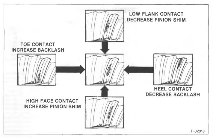
Figure 24—Gear Tooth Pattern
