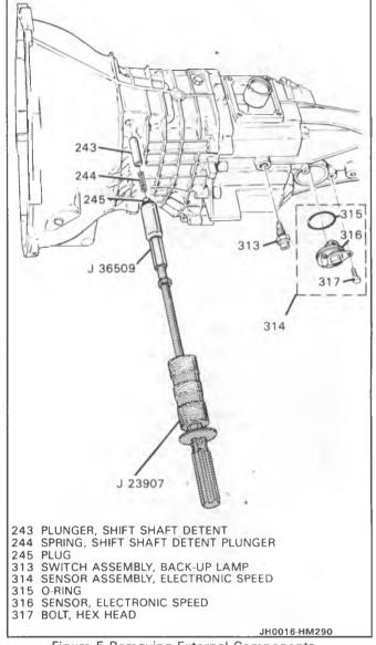
Figure 5 Removing External Components
