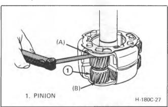
Figure 19 Planetary Carrier and Pinion Clearance
