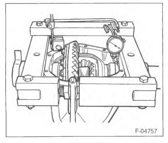
Figure 4—Spreading the Differential Case
