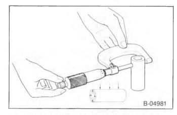
Figure 8—Measuring Piston Pin Diameter
