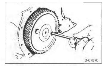
Figure 20-Removing the Camshaft Thrust Plate Bolts
