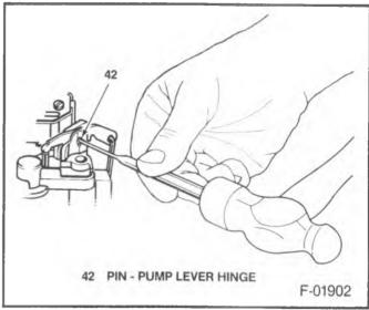
Figure 15 – Removing Pump Lever
