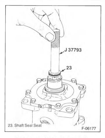
Figure 11—Removing the Shaft Seal Seat
