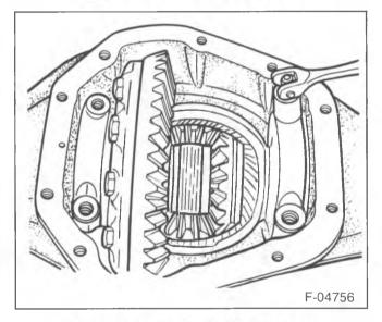
Figure 3—Removing the Bearing Cap
