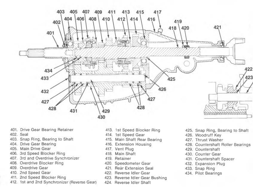
Figure 1—4 Speed 89 mm Transmission
