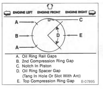
Figure 33—Piston Ring End Gap Locations
