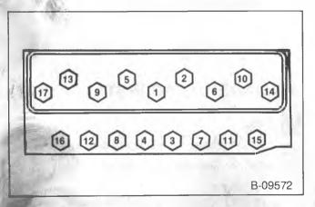
Figure 70—Cylinder Head Bolt Tightening Sequence (5.0L and 5.7L Engines)
