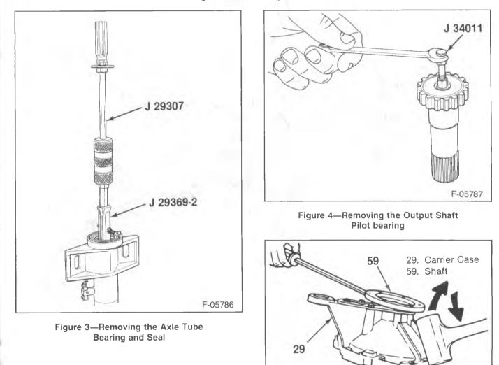
Figure 5—Removing the Axle Shaft
