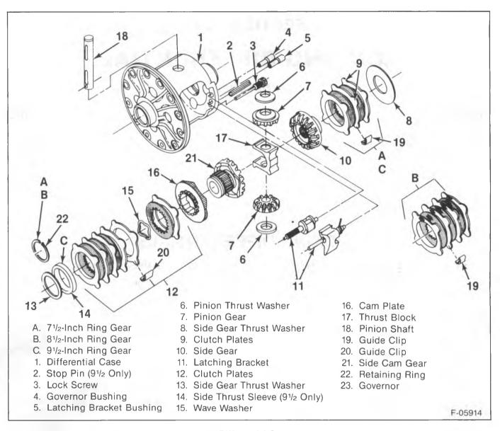
Figure 1—Differential Components
