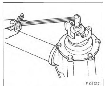
Figure 12—Checking Pinion Preload
