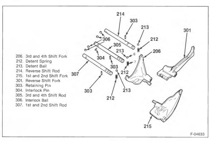
Figure 33A—R/V/P Shift Rod and Fork Positions
