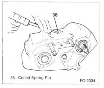
Figure 6—Removing the Shift Fork Roll Pin
