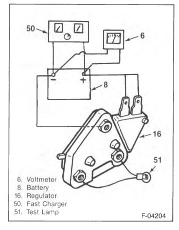
Figure 14—Testing the Voltage Regulator
