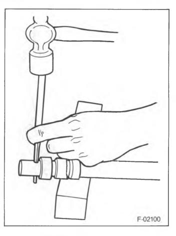
Figure 10—Removing the Roll Pin
