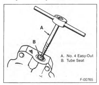
Figure 5—Removing the Tube Seat
