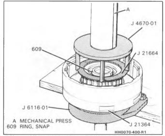
Figure 67 - Installing Forward Clutch Piston Release Springs
