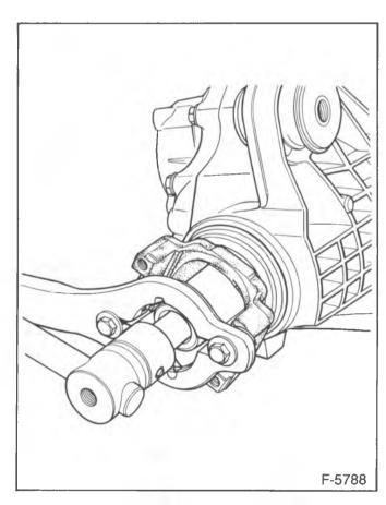
Figure 11—Removing the Pinion Nut
