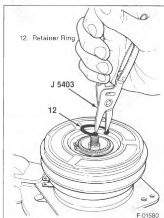
Figure 13—Removing/Installing the Shaft Seal Retaining Ring
