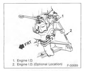
Figure 6-2.5L Engine I.D. Location
