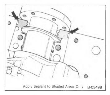
Figure 49—Applying Sealant to the Block
