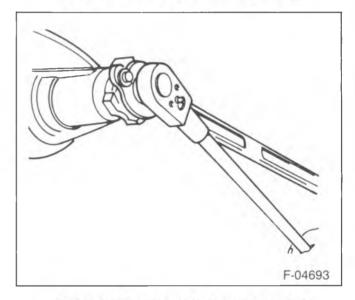
Figure 12—Removing the Drive Pinion Nut
