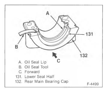
Figure 52—Crankshaft Rear Oil Seal Installation (7.4L Engines)
