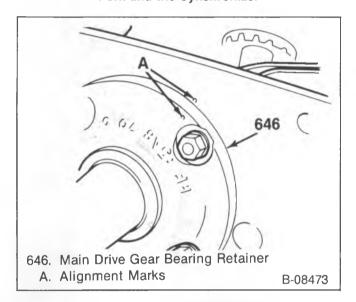
Figure 9—Bearing Cap Alignment Marks
