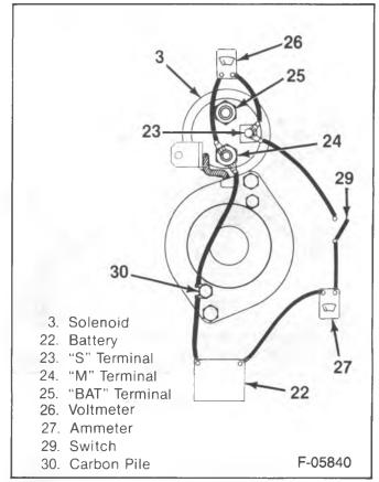
Figure 10—Pull-In Winding Test Connections
