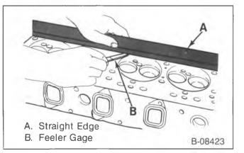
Figure 24—Checking the Cylinder Head for Warpage
