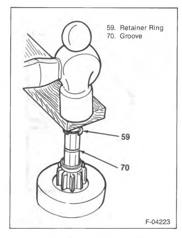
Figure 16—Forcing the Retainer Ring on the Shaft
