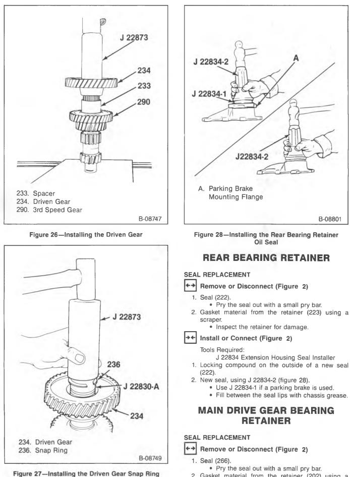
Gasket material from the retainer (202) using a scraper.
