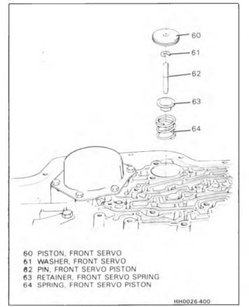
Figure 90 - Front Servo Assembly
