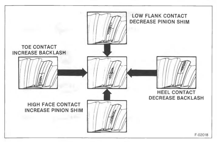
Figure 19—Gear Tooth Pattern
