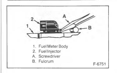
Figure 4—Removing TBI 700 Fuel Injector
