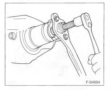
Figure 13—Removing the Pinion Flange
