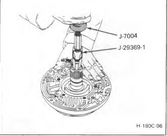
Figure 74 Removing Oil Pump Bushing - Front
