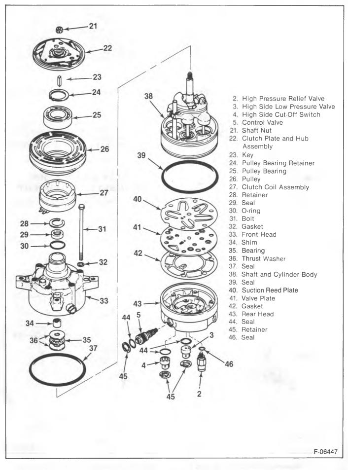
Figure 3—Compressor Components
