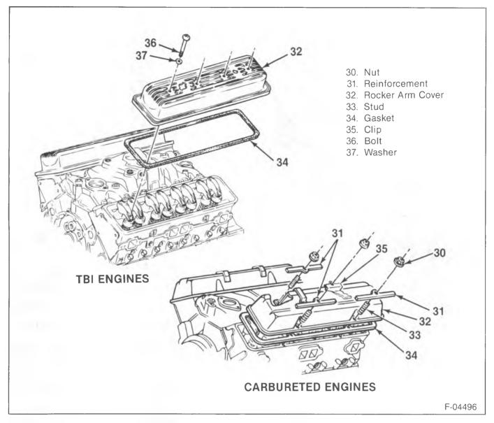
Figure 8—Rocker Arm Cover (5.0L and 5.7L Engines)
