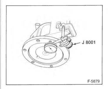
Figure 39—Measuring Axle Shaft End Play
