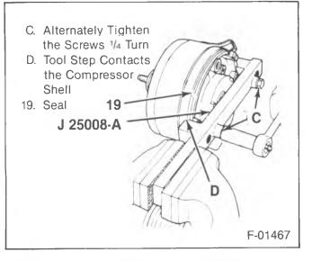
Figure 21—Removing the Shell
