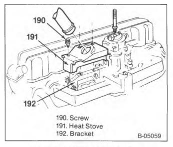
Figure 9—Manifold Heat Stove
