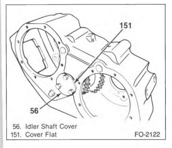
Figure 13—Idler Shaft Cover Alignment
