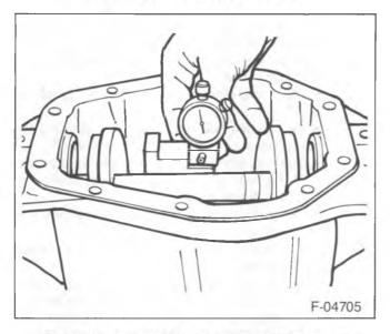
Figure 25—Scooter Gage on the Height Block
