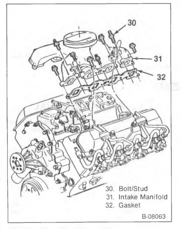
Figure 3—Intake Manifold
