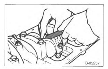
Figure 50—Measuring Connecting Rod Side Clearance
