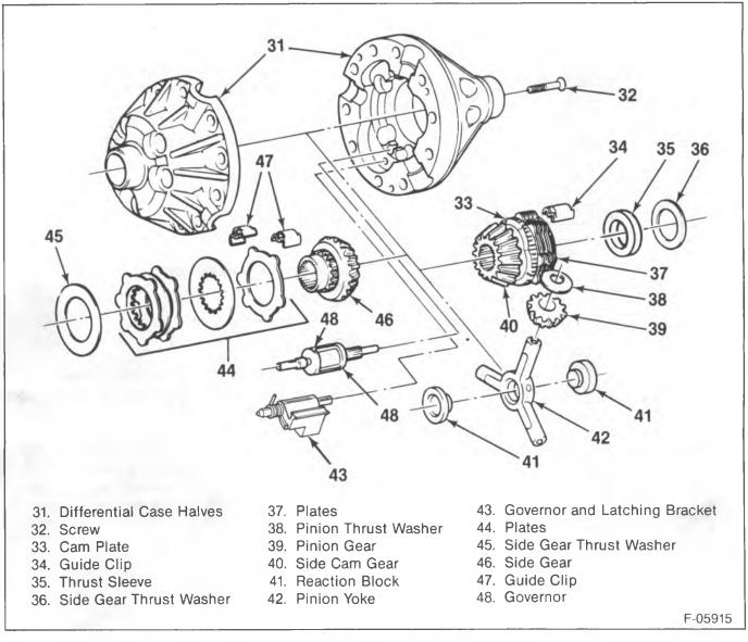
Figure 9—Differential Components
