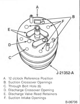
Figure 37 — Installing the Front Valve Plate
