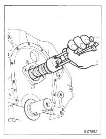
Figure 32—Replacing the Camshaft
