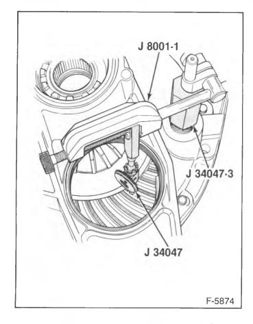
Figure 31—Measuring Backlash at the Ring Gear
