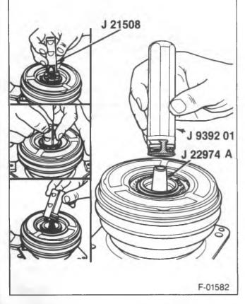
Figure 15—Removing/Installing the Shaft Seal and Seal
