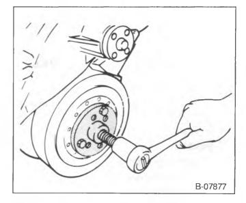
Figure 9-Removing the Torsional Damper (Typical)
