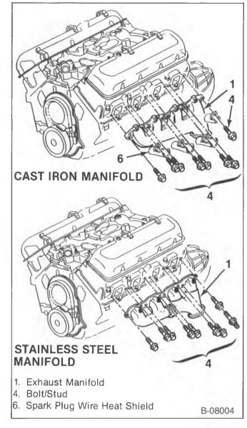
Figure 5—Exhaust Manifold (7.4L Engines)
