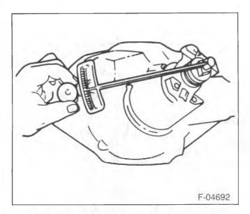
Figure 16—Checking Pinion Bearing Preload
