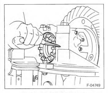
Figure 5—Punching the Carrier Leg
