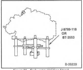
Figure 11 - Carburetor Holding Stand
