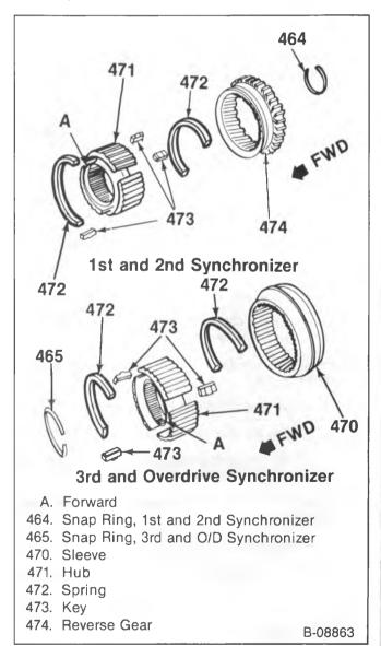
Figure 9—Synchronizer Components
