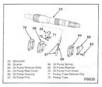
Figure 23—Mainshaft and Oil Pump Assembly
