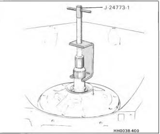
Figure 18 - Removing Pump Assembly
