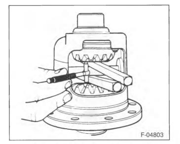
Figure 6—Measuring Side Gear Spread
