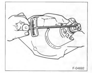
Figure 4—Checking Pinion Preload
