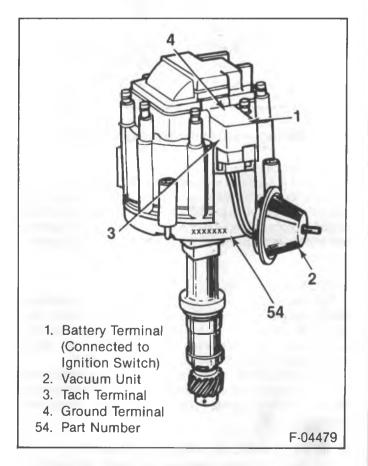
Figure 1—Distributor with Integral Coil
