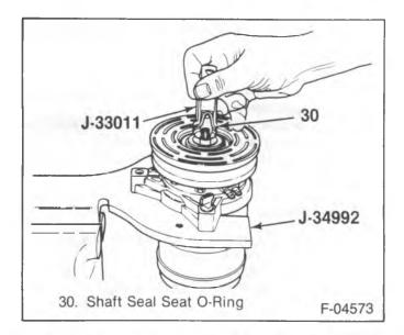
Figure 24—Installing the Shaft Seal Seat O-Ring
