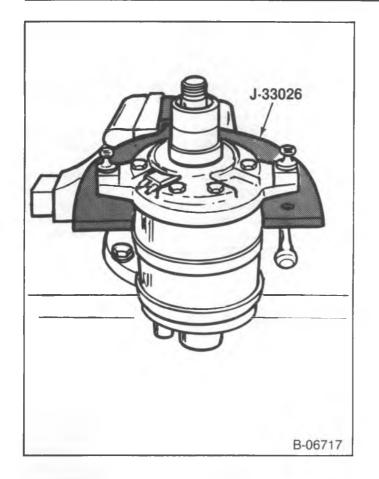
Figure 39 — installing the Compressor to J 33026
