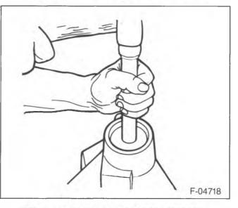
Figure 30—Installing the Pinion Front Cup
