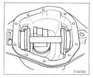
Figure 65—Pinion Height Block
