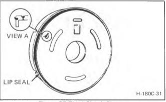
Figure 25 Third Clutch Piston
