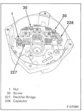
Figure 8—Rectifier Bridge in End Frame
