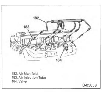
Figure 8—AIR Manifold Installation
