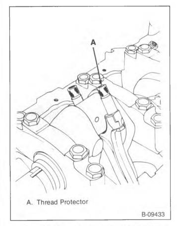
Figure 17—Connecting Rod Thread Protectors
