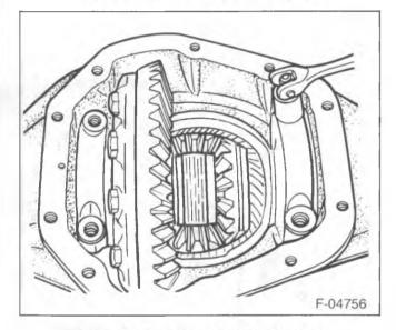
Figure 3—Removing the Bearing Cap
