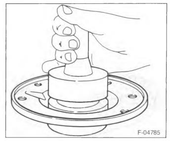
Figure 19—Installing the Seal
