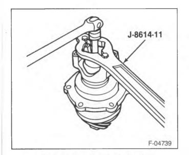
Figure 11—Installing the Pinion Nut
