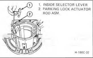
Figure 17 Installing Selector Lever
