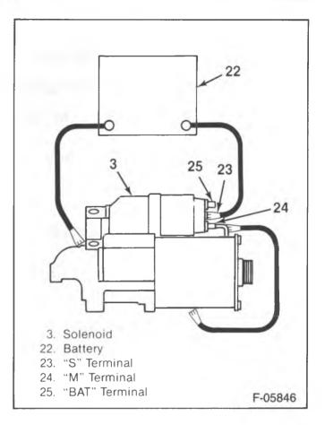
Figure 16—Pinion Clearance Check Circuit
