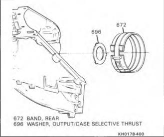
Figure 33 - Installing Rear Band and Selective Thrust Washer
