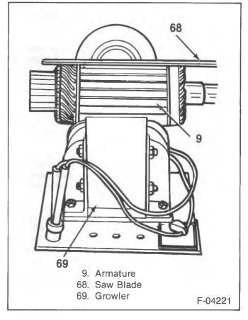
Figure 13—Testing the Armature for Short Circuits
