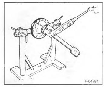
Figure 17—Installing the Pinion Nut
