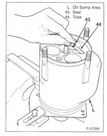
Figure 49-Installing the Oil Pick-Up Tube
