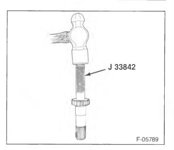
Figure 33—Installing the Differential Pilot Bearing
