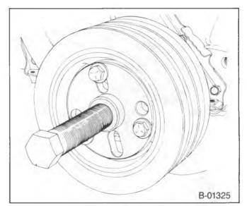
Figure 15—Removing the Torsional Damper
