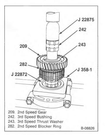
Figure 19 –Installing the 3rd Speed Gear Bushing
