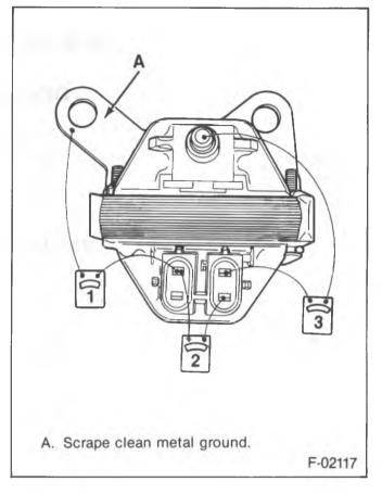
Figure 28—Testing the Ignition Coil
