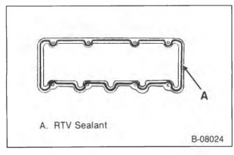
Figure 50—Applying Sealant to the Rocker Arm Cover
