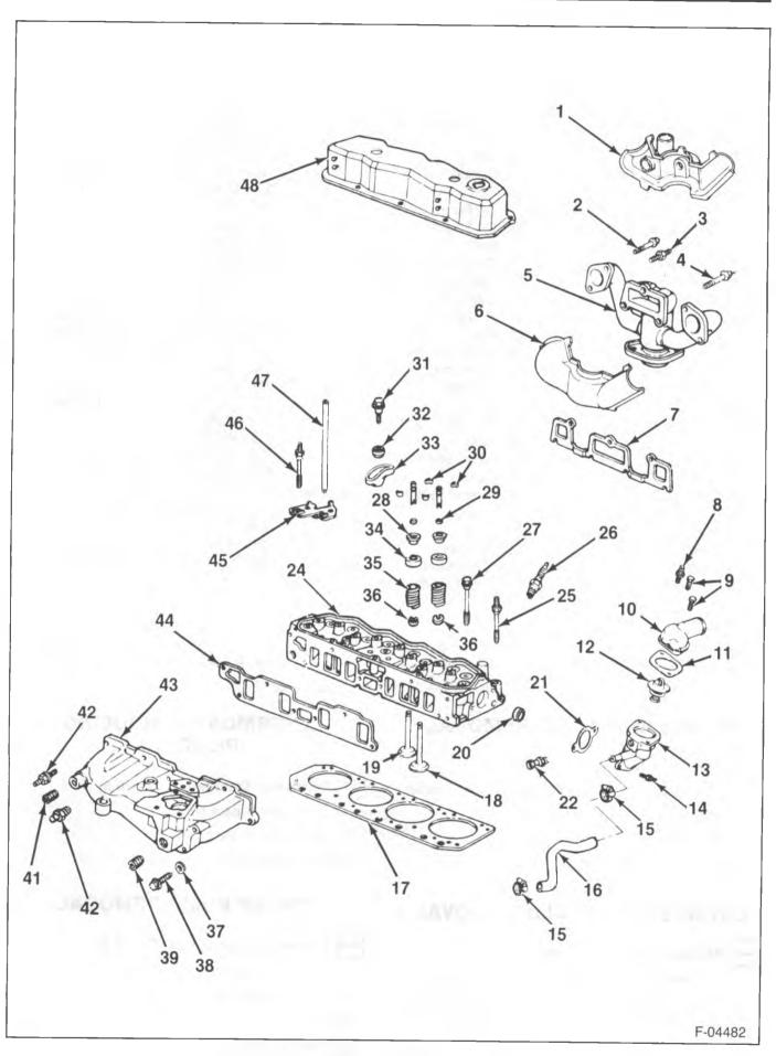
Figure 3-Cylinder Head, Manifolds, and Components
