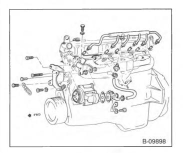
Figure 7—AIR System Components
