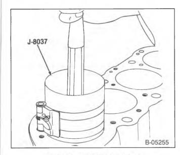
Figure 55—Installing the Piston
