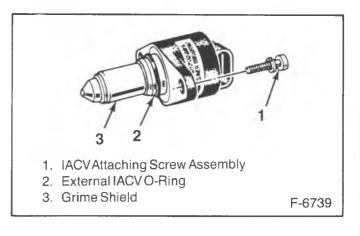
Figure 9—Flange Mounted IAC Valve — TBI 700
