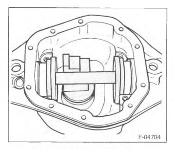
Figure 24—Pinion Height Block
