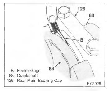
Figure 40—Measuring Crankshaft End Play
