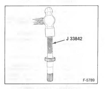
Figure 35—Installing the Pilot Bearing
