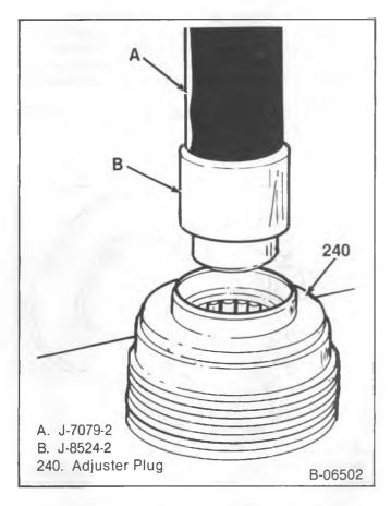
Figure 8—Removing the Needle Bearing
