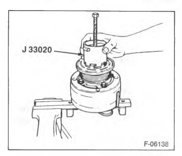
Figure 12—Pulley Rotor and Bearing Puller Installation
