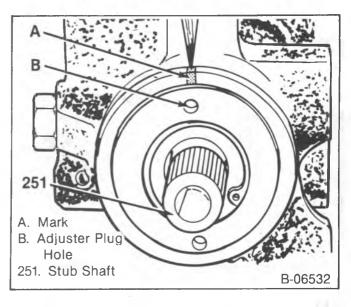
Figure 16—Marking the Housing
