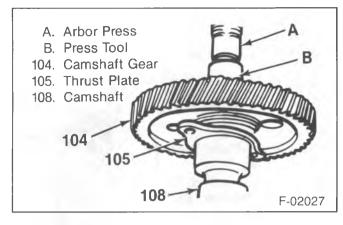
Figure 29—Installing the Camshaft Gear
