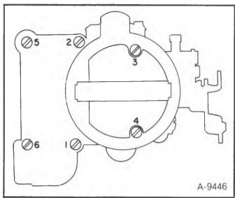
Figure 38 – Air Horn Screw Location and Tightening Sequence
