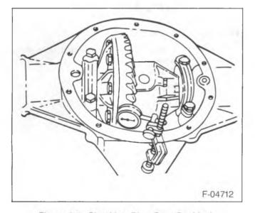
Figure 24—Checking Ring Gear Backlash
