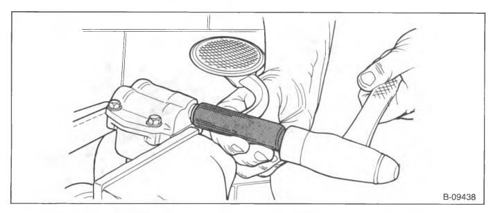
Figure 33-Installing the Oil Pump Screen and Pipe
