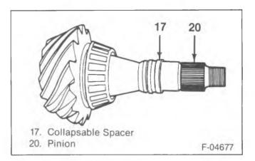
Figure 5—Pinion Collapsable Spacer
