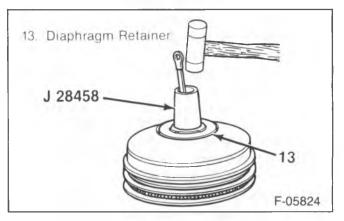
Figure 22—Installing the Diaphragm Retainer
