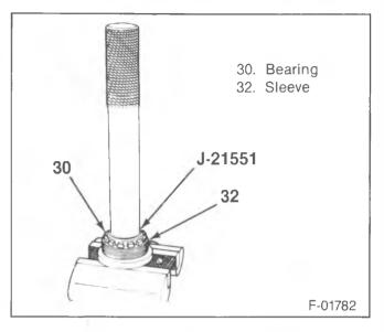
Figure 9—Remove the Sleeve Bearing
