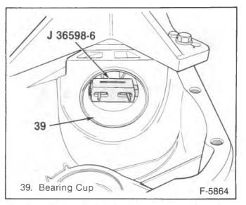
Figure 16—Removing the Inner Bearing Cup
