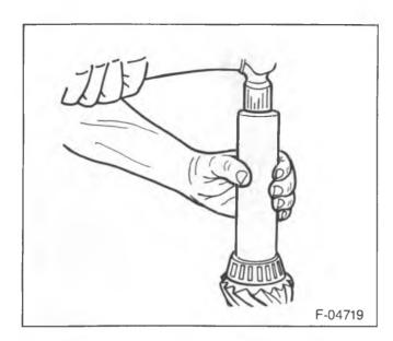
Figure 71—Installing the Inner Bearing
