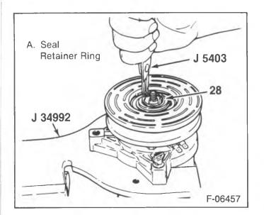
Figure 21—Removing or Installing the Shaft Seal Retainer
