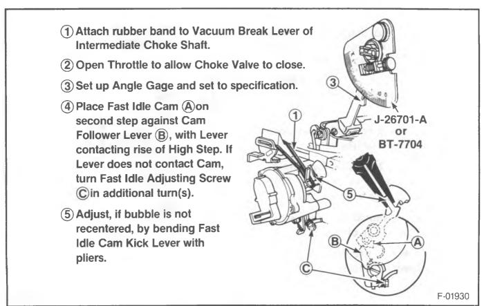
Figure 45 - Choke Link - Fast Idle Cam Adjustment
