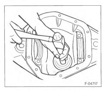
Figure 69—Installing the Pinion Inner Cup
