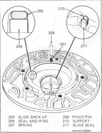
Figure 97 Slide Back Up and Slide Seal
