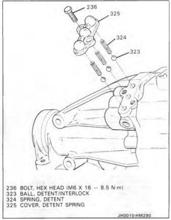
Figure 86 Detent Components Install
