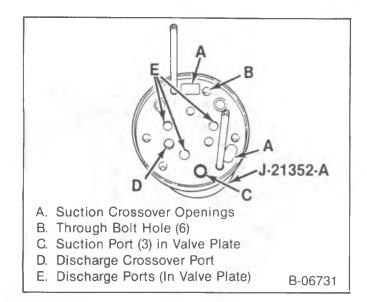
Figure 33 — Installing the Rear Valve Plate
