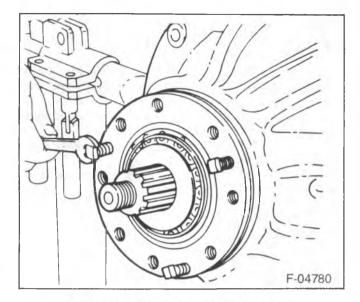
Figure 13—Removing the Pinion Cage
