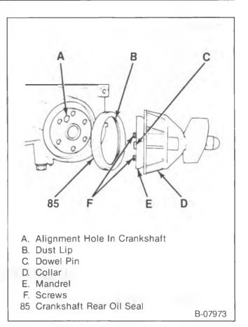
Figure 31—Installing the Crankshaft Oil Seal
