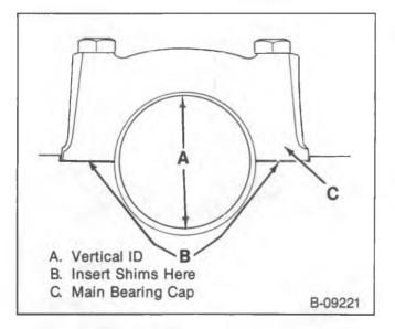
Figure 25—Main Bearing Cap Shim Location
