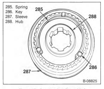
Figure 15 – Synchronizer Assembled
