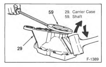
Figure 8—Removing the Left Shaft
