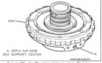
Figure 49 - Air Checking Intermediate Clutch
