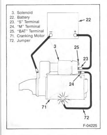
Figure 18—Pinion Clearance Circuit
