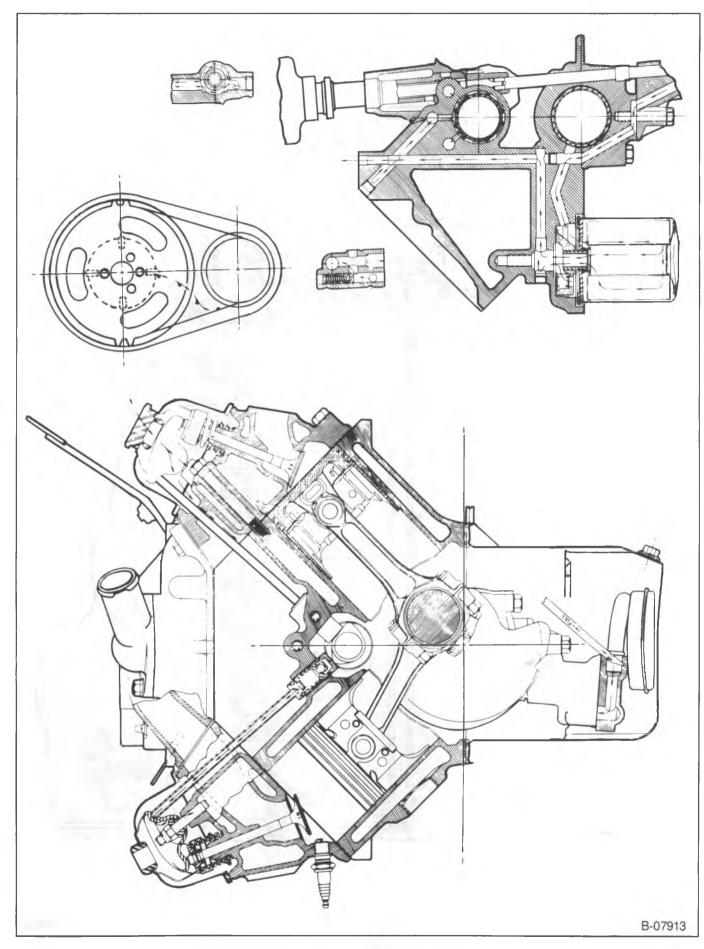
Figure 1—Lubrication Diagram (5.0L and 5.7L Engines)
