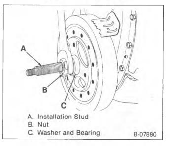
Figure 32—Installing the Torsional Damper
