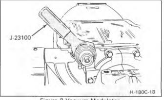
Figure 8 Vacuum Modulator
