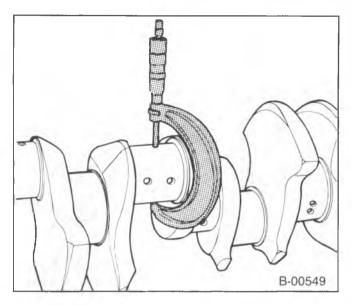
Figure 28—Measuring the Crankshaft Journals
