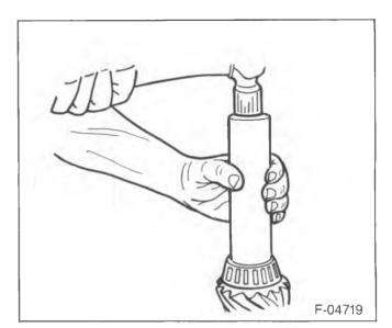
Figure 30—Installing the Inner Bearing
