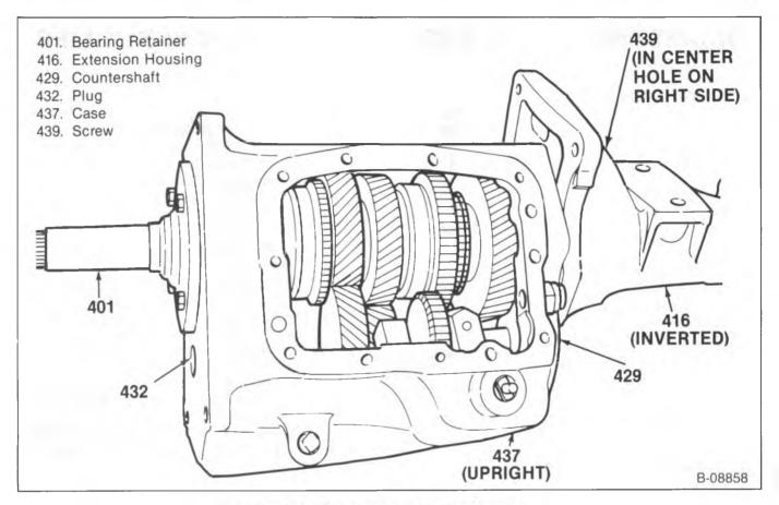
Figure 3—Turning the Extension Housing
