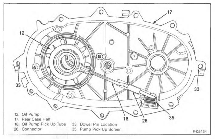
Figure 17—Oil Pump, Pickup, Screen, Doweled Case Holes
