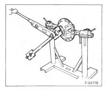
Figure 11-Removing the Pinion Nut
