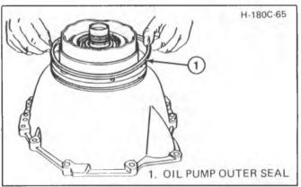
Figure 50 Installing Oil Pump Outer Seal
