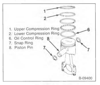
Figure 7—Piston and Components — 6.2 L
