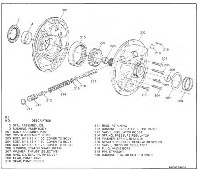
Figure 71 - Oil Pump Assembly
