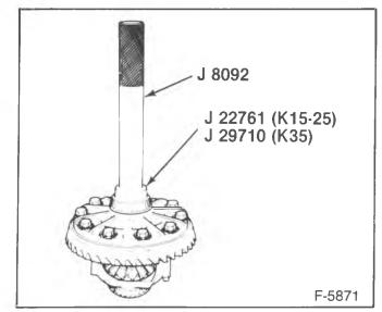
Figure 26—Installing the Differential Side Bearing
