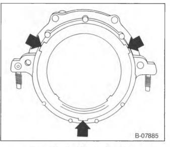
Figure 11-Seal Removal Notches
