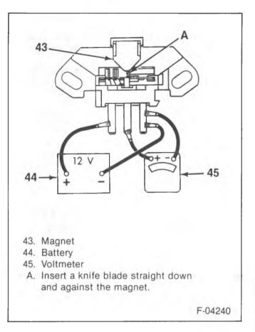
Figure 17—Testing the Hall Effect Switch
