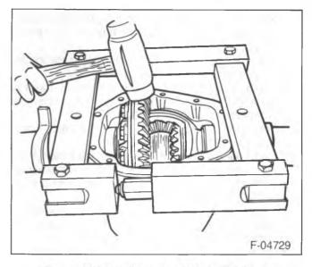
Figure 80—Installing the Differential Case
