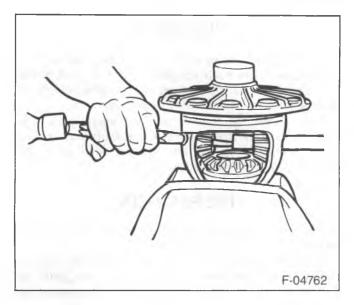
Figure 50—Removing the Pinion Shaft
