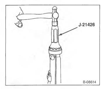
Figure 27—Installing the Extension Housing Oil Seal
