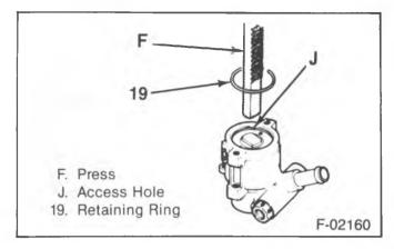
Figure 45—Installing the Retaining Ring
