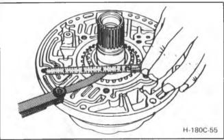
Figure 47 Checking Oil Pump Gear Clearance
