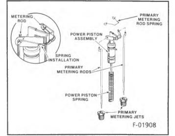
Figure 34 - Power Piston, Metering Rods and Jets
