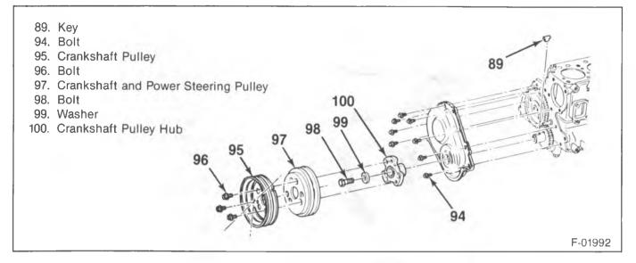
Figure 14—Timing Gear Cover and Components
