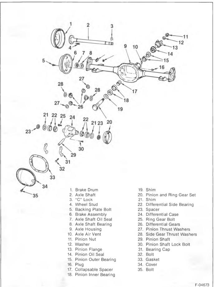
Figure 1—Rear Axle Components
