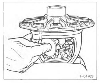
Figure 10-Removing the Pinion Gears
