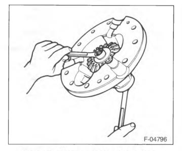
Figure 13—Clamping the Cam Unit In Place
