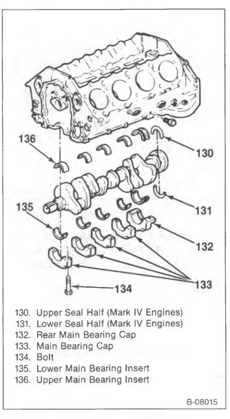
Figure 24—Crankshaft and Components (Typical)
