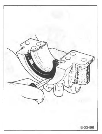
Figure 19—Removing the Lower Seal Half
