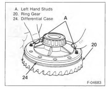
Figure 11—Aligning the Ring Gear Studs
