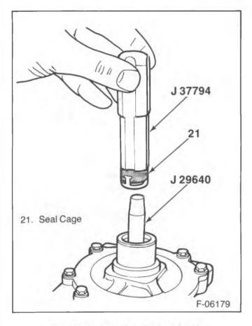
Figure 13—Installing the Seal Cage
