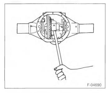
Figure 2—Prying the Differential Case from the Axle Housing
