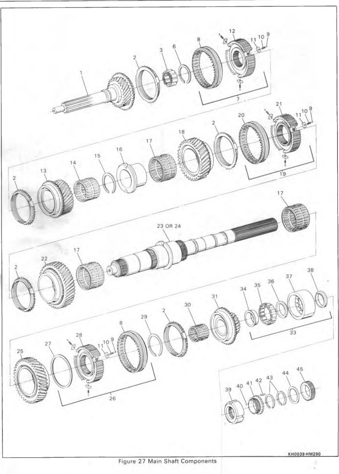
1 SHAFT, INPUT RING, SYNCHRONIZER 2 3 BEARING, PILOT BERAING, FILOT
