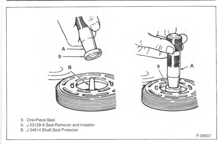
Figure 23 — Removing or Installing the Shaft Tip Seal
