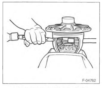
Figure 9-Removing the Pinion Shaft
