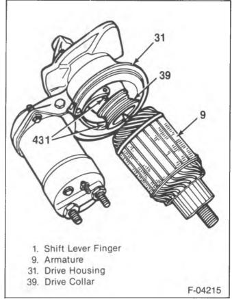
Figure 7—Disengaging the Drive Collar from the Shift Lever Fingers
