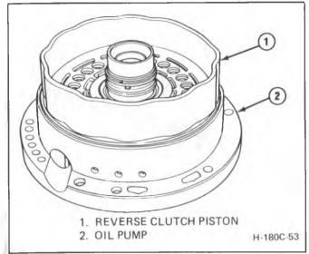
Figure 46 Installing Reverse Clutch Piston Into Oil Pump
