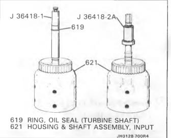
Figure 80 Turbine Shaft Oil Seal Rings
