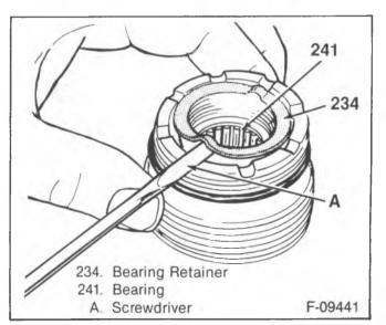
Figure 7—Removing the Bearing Retainer
