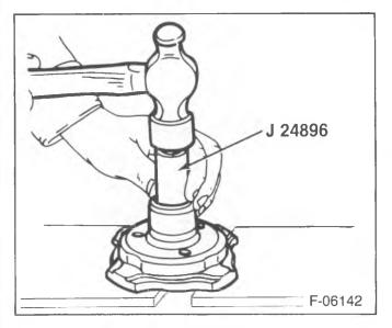
Figure 19—Removing the Bearing from the Front Head
