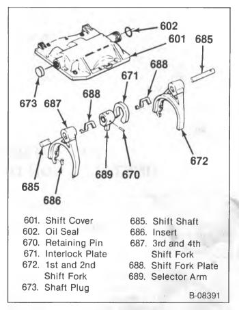
Figure 30—Shift Cover and Components
