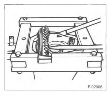
Figure 5—Removing the Differential
