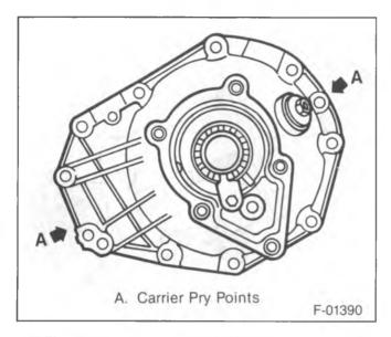
Figure 6—Separating the Carrier Case Halves
