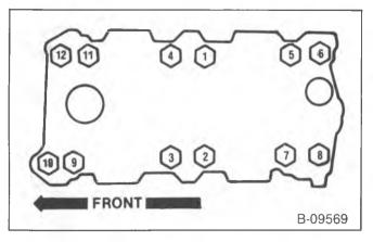
Figure 75—Intake Manifold Bolt Tightening Sequence (5.0L and 5.7L Engines)
