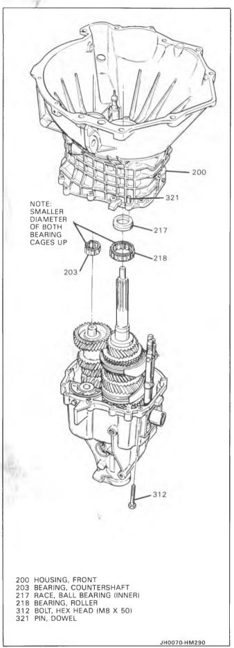
Figure 88 Front Housing Install
