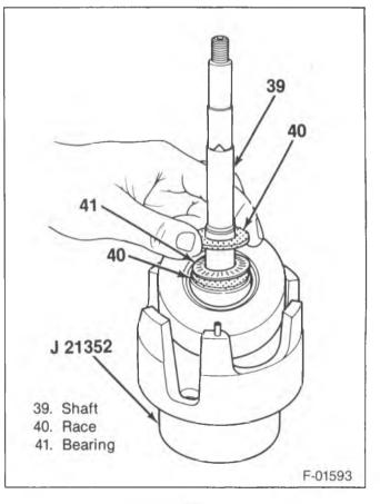
Figure 26—Removing the Front Thrust Races and Bearing
