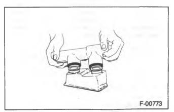
Figure 13—Installing the Reservoir
