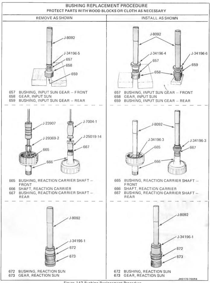
Figure 142 Bushing Replacement Procedure
