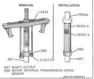
Fig. 51 Internal Transmission Speed Sensor Rotor
