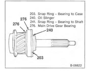
Figure 10—Main Drive Gear Assembly
