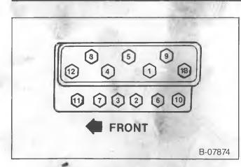
Figure 38—Cylinder Head Bolt Tightening Sequence
