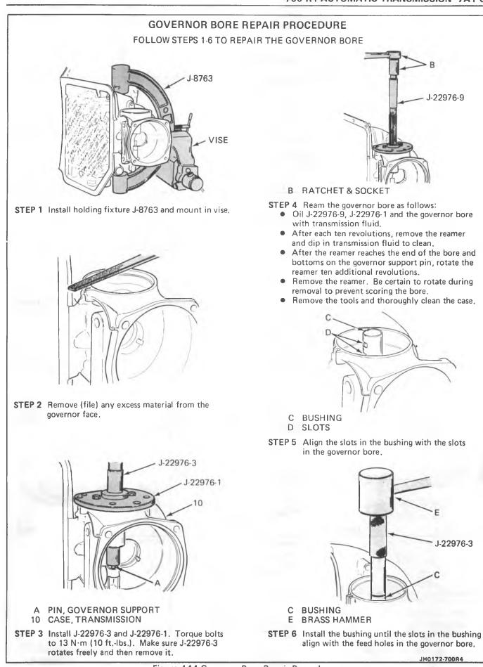
Figure 144 Governor Bore Repair Procedure
