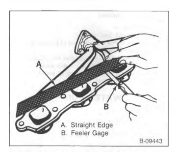
Figure 14—Checking Alignment of Manifold Flanges
