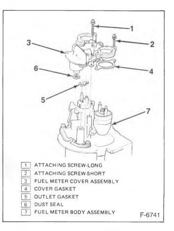
Figure 6—Replacing Model 220 Fuel Meter Cover
