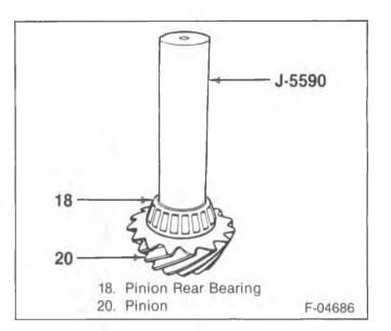
Figure 14—Installing the Pinion Inner Bearing
