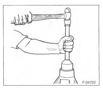
Figure 34—Installing the Pinion Seal
