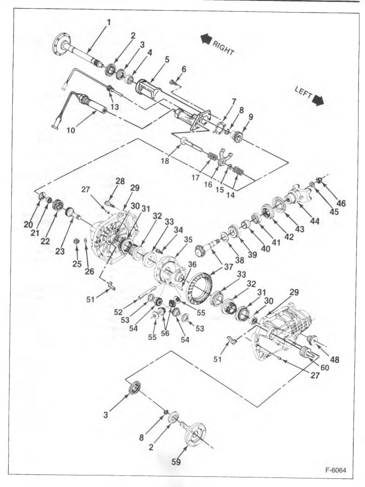
Figure 1—Front Axle Components (K-15-25 Models)
