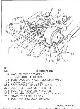
Figure 15 Removing Auxiliary Valve Body Assembly
