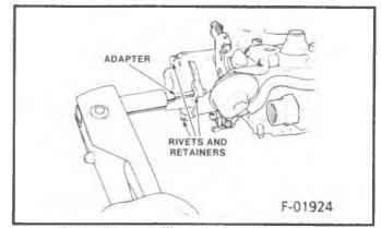
Figure 39 - Installing Choke Cover Rivets
