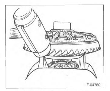
Figure 48-Removing the Ring Gear
