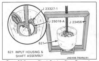
Figure 58 Overrun Clutch Retainer Ring - Removal
