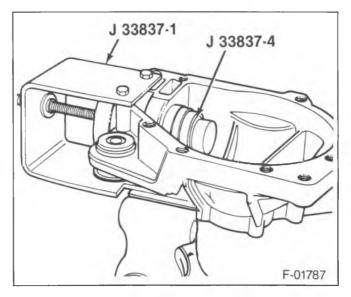
Figure 18—Installing the Inner Pinion Bearing Cup
