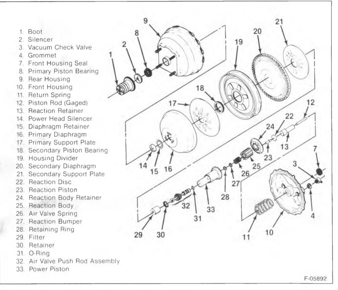
Figure 25—Tandem Vacuum Booster Components
