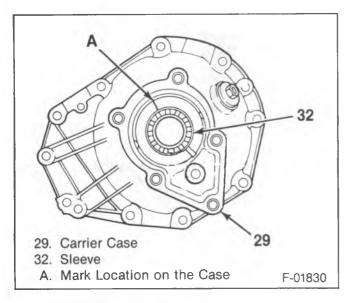
Figure 26—Marking Sleeve Location
