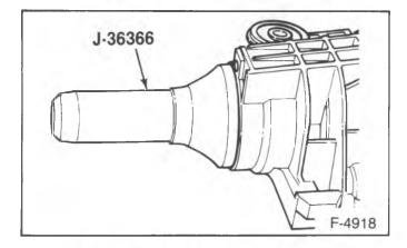
Figure 24—Installing the Pinion Seal
