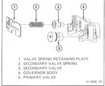
Figure 53 Governor Assembly - Exploded View
