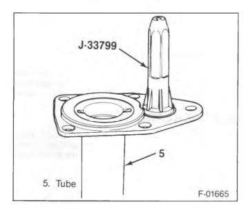
Figure 32—Installing the Shift Housing Seal
