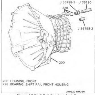
Figure 47 Shift Rail Bearings Install
