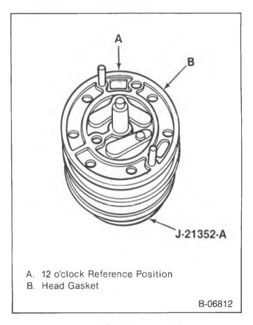
Figure 38 — Installing the Seal to the Front Head
