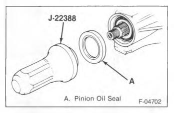
Figure 14-Installing the Pinion Oil Seal
