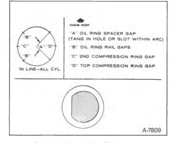
Figure 54—Piston Ring Gap Location
