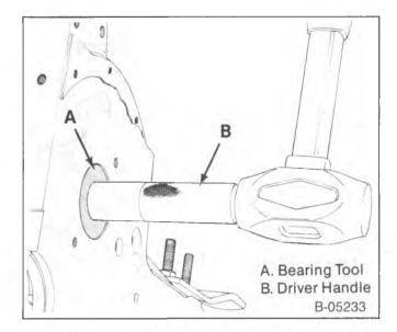
Figure 30—Removing or Installing Camshaft Bearings
