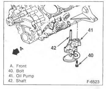
Figure 37—Oil Pump Installation
