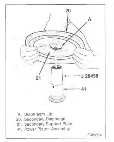
Figure 28—Assembling the Secondary Diaphragm and Support
