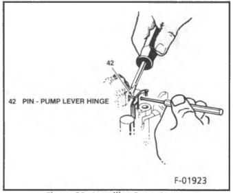
Figure 38 - Installing Pump Lever
