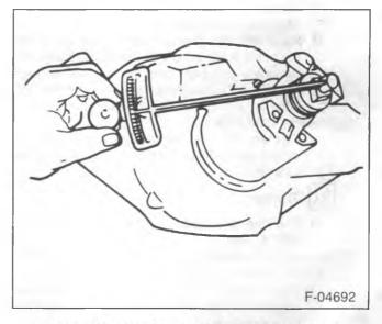
Figure 17—Checking Pinion Bearing Preload
