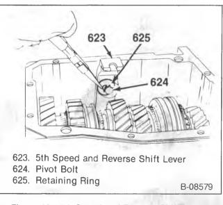
Figure 12—5th Speed and Reverse Shift Lever Retaining Ring
