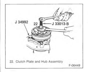
Figure 5—Removing the Clutch Plate and Hub Assembly check that the shaft key (23) is properly in place in the keyway, then install the clutch plate and hub assembly (22) to its final position.
