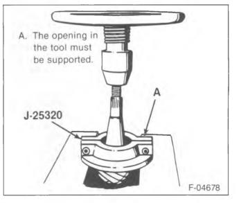
Figure 6—Removing the Pinion Rear Bearing
