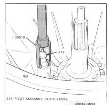
Figure 48 Clutch Fork Pivot Assembly Install
