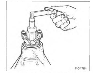
Figure 11-Checking the Pinion Preload
