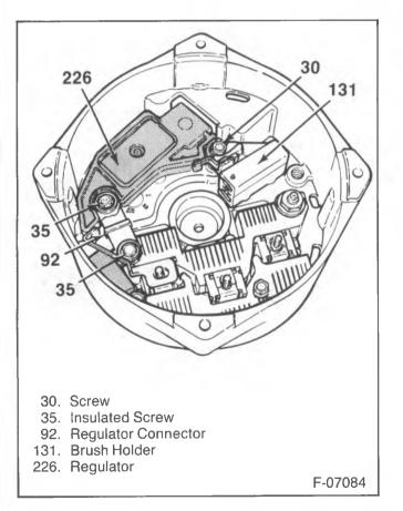
Figure 7-Slip Ring End Frame with Stator Removed
