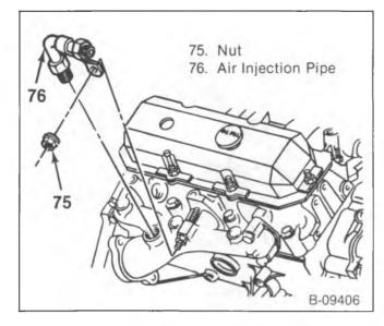
Figure 5—Air Injection Tube
