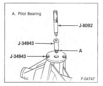
Figure 13-Installing the Pilot Bearing
