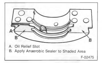
Figure 32—Applying Sealant to the Main Bearing Cap
