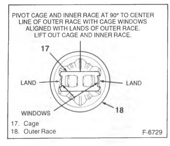
Figure 49—Separating Outer Race and Cage
