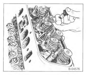
Figure 13—Removing the Hydraulic Lifter
