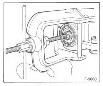
Figure 13—Removing the Pinion
