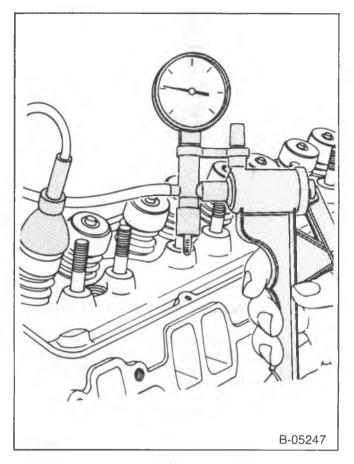
Figure 39—Checking the Valve Seals
