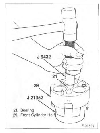
Figure 27—Installing the Needle Bearing
