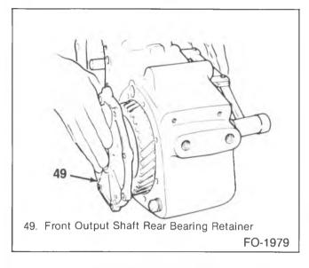
Figure 5—Removing the Front Output Shaft Bearing
