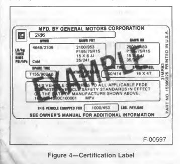
vehicle Certification Label shows the originally equipped tire size and recommended inflation pressures.
