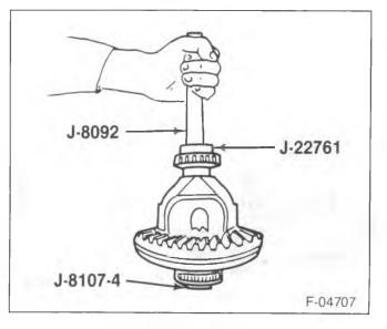
Figure 19—Differential Bearing Installation
