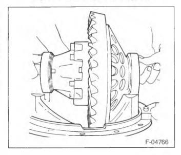
Figure 7—Removing the Differential
