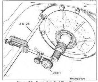
Figure 79 - Front Unit End Play Check
