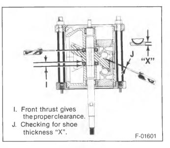
Figure 35—Checking the Piston and Shaft End Play
