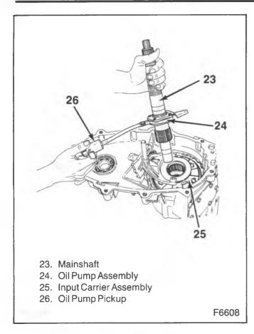
Figure 11—Removing the Mainshaft and Oil Pump
