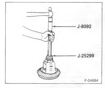
Figure 12—Installing the Side Bearing
