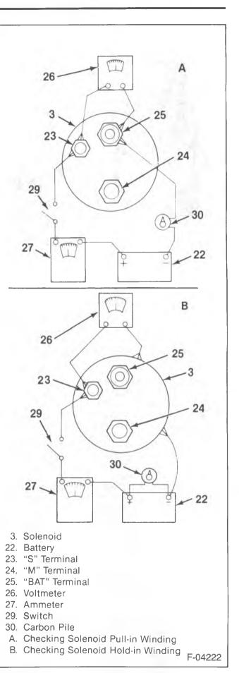
Figure 15—Solenoid Test Connections
