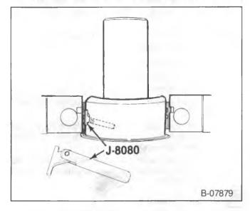
Figure 19-Removing the Upper Main Bearing Insert
