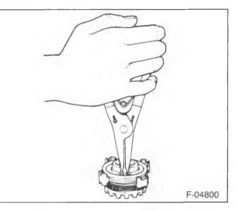
Figure 3—Removing the Retaining Ring
