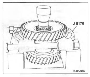
Figure 24—Removing the Driven Gear
