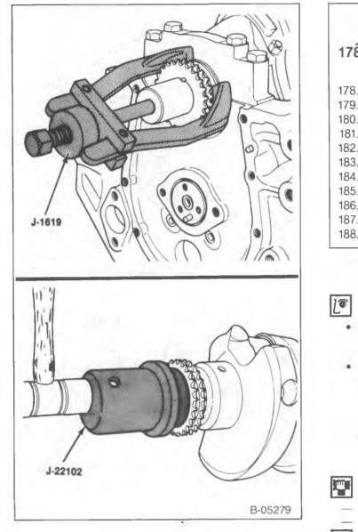
Figure 32—Crankshaft Sprocket Replacement (7.4L Engines)
