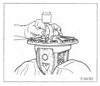
Figure 8-Removing the Lock Pin
