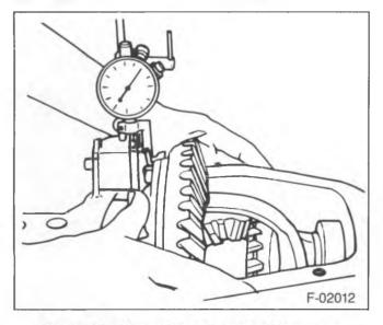
Figure 37—Measuring Differential Movement
