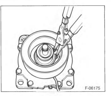
Figure 9—Removing the Coil Snap Ring
