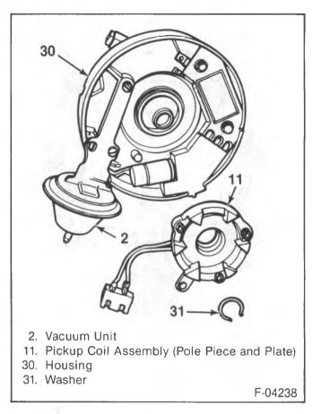
Figure 14—Pickup Coil Removed
