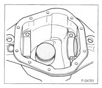
Figure 63—Master Pinion Block
