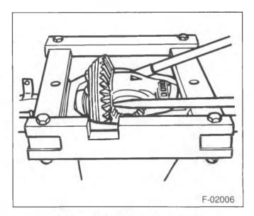
Figure 5—Removing the Differential
