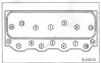
Figure 71—Cylinder Head Bolt Tightening Sequence (7.4L Engines)
