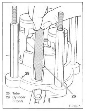
Figure 41—Installing the Discharge Crossover Tube
