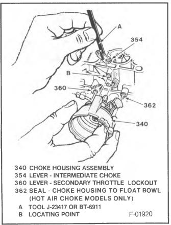
Figure 33 - Installing Choke Housing Assembly
