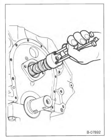
Figure 8—Replacing the Camshaft
