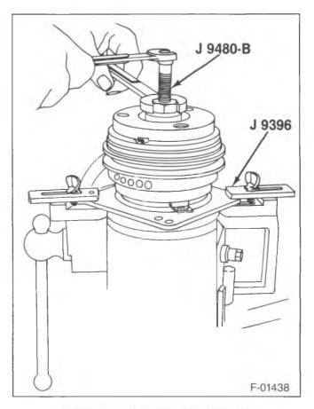
Figure 5—Installing the Drive Plate
