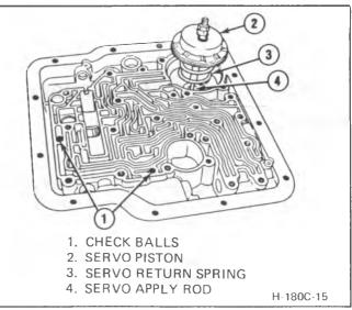
Figure 4 Check Balls and Servo Piston
