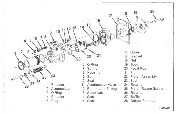
Figure 1—Hydro-Boost Components
