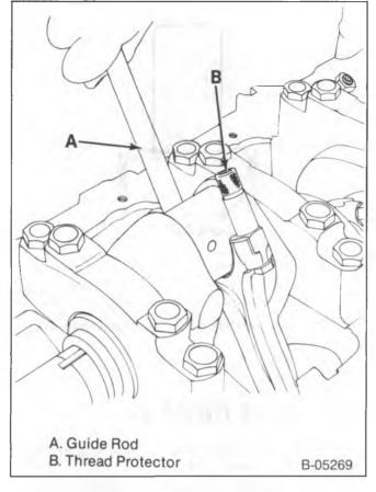
Figure 10—Replacing the Piston and Connecting Rod (Typical)
