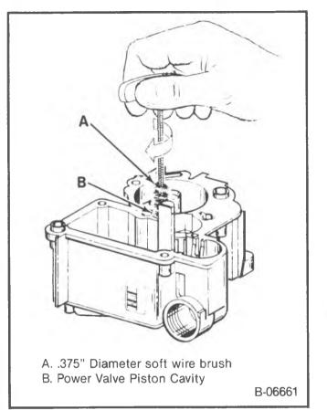
Figure 28 – Cleaning Power Piston Bore
