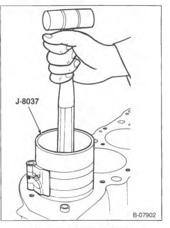
Figure 35—Installing the Piston
