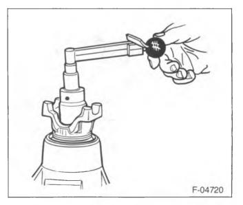
Figure 31—Checking the Pinion Preload
