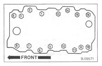
Figure 77—Intake Manifold Bolt Tightening Sequence (7.4L Engines)
