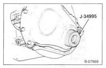
Figure 46—Installing the Timing Gear Cover
