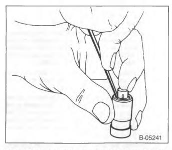
Figure 27—Installing the Check Ball Retainer (Typical)
