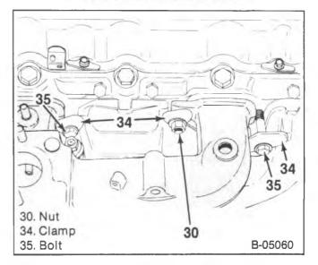
Figure 10—Manifolds Installed
