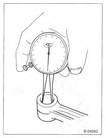
Figure 10—Measuring Piston Pin Bushing Inside Diameter
