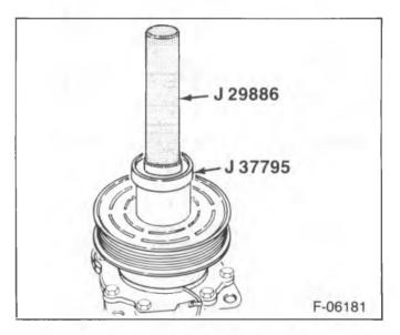
Figure 15—Installing the Rotor Pulley
