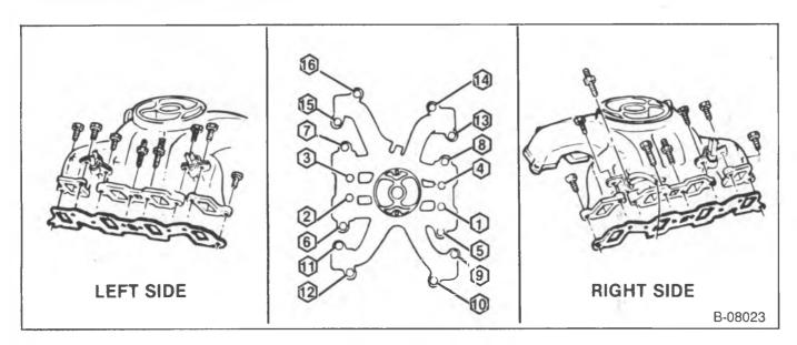
Figure 55—Intake Manifold Installation
