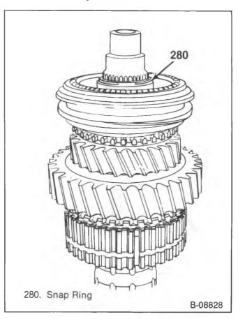
Figure 21 – 3rd and 4th Synchronizer Hub Snap Ring
