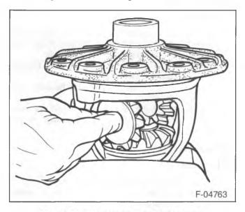
Figure 51—Removing the Pinion Gears
