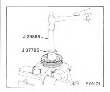
Figure 8—Removing the Bearing
