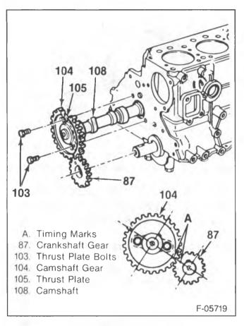
Figure 21—Camshaft and Timing Gears
