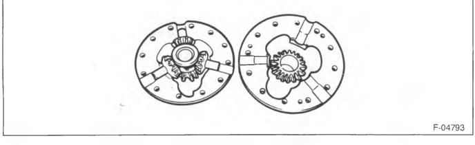
Figure 10—Differential Case Halves
