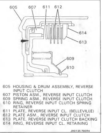
Figure 88 Reverse Input Clutch
