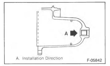
Figure 12—Drive End Bearing Installation
