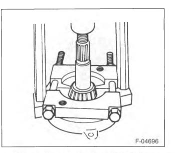
Figure 8—Removing the Pinion Rear Bearing
