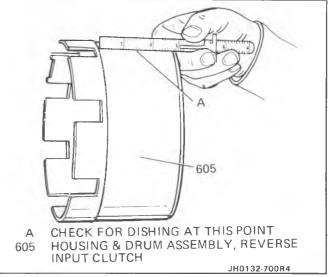
Figure 84 Check Reverse Input Housing For Dishing
