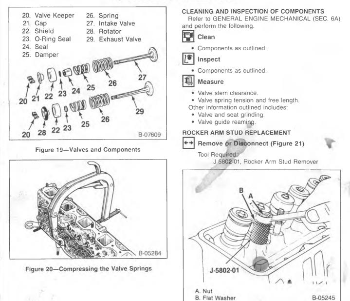
Figure 21—Removing the Rocker Arm Stud
