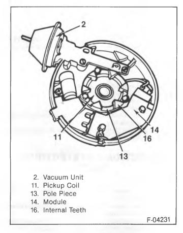
Figure 5—Top View of Distributor
