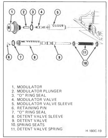
Figure 7 Detent Valve and Modulator Valve
