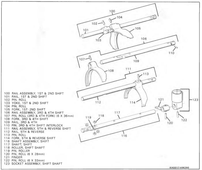
Figure 63 Shift Shaft/Rails Assembly Components
