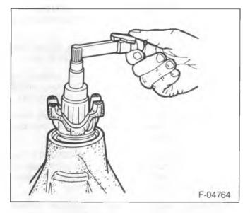
Figure 22—Measuring Pinion Bearing Preload
