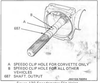
Figure 130 Speedometer Clip Holes
