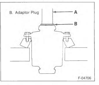
Figure 19—Installing the Ring Gear to the Case
