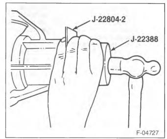
Figure 15—Installing the Pinion Oil Seal
