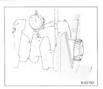
Figure 38—Checking Crankshaft Runout
