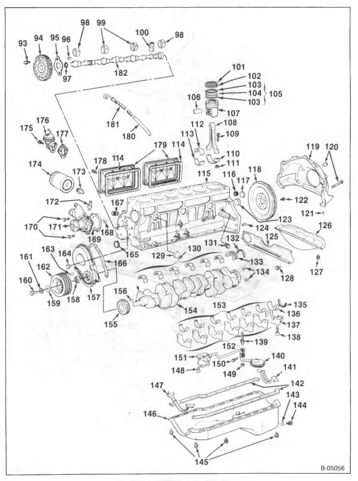
Figure 5—Block and Components
