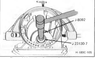
Figure 84 Installing Reaction Sun Gear Drum Bushing Sleeve
