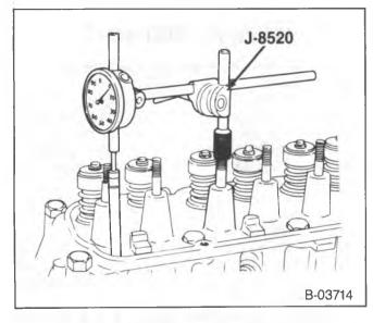
Figure 61—Measuring Camshaft Lobe Lift
