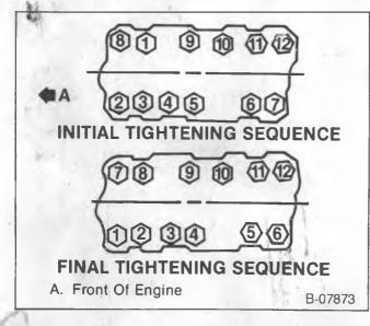
Figure 41—Intake Manifold Bolt Tightening Sequence
