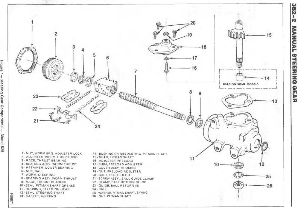
Figure 1—Steering Gear Components
