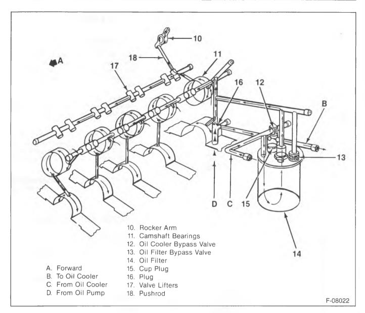
Figure 1—Lubrication Diagram
