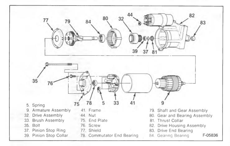
Figure 3—PG-200 Starting Motor Components
