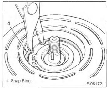
Figure 6—Removing the Internal Snap Ring
