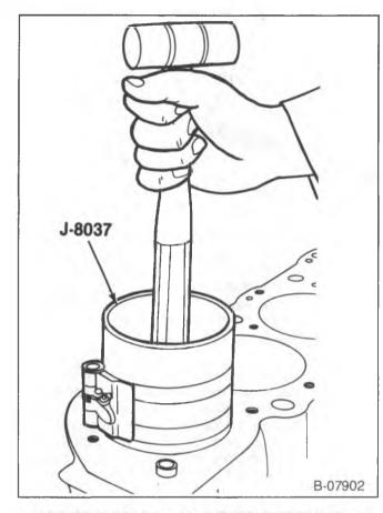
Figure 35—Installing the Piston and Connecting Rod
