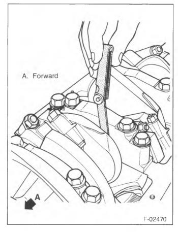
Figure 33—Measuring Crankshaft End Play
