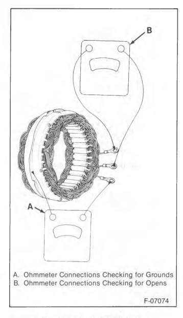
Figure 13—Checking the Stator
