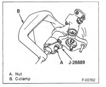
Figure 2—Removing the Accumulator
