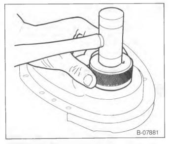
Figure 33—Installing the Front Crankshaft Seal (Typical)
