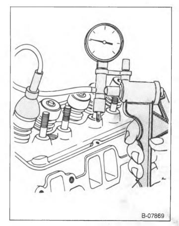
Figure 24—Checking the Valve Seals
