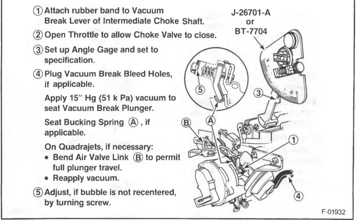
Figure 47 - Primary Side (Front) Vacuum Break Adjustment
