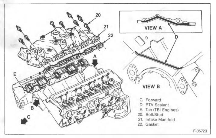
Figure 74—Intake Manifold (5.0L and 5.7L Engines)
