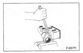
Figure 11-Removing the Reservoir
