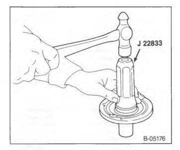
Figure 29 – Installing the Drive Gear Bearing Retainer Oil Seal
