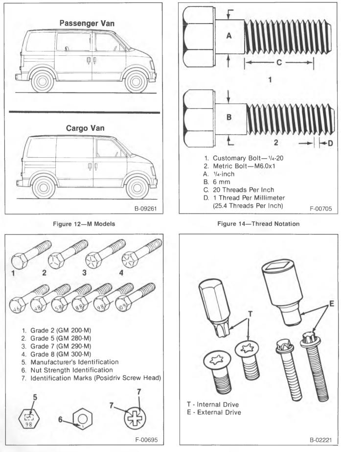
Figure 13—Bolt and Nut Identification
