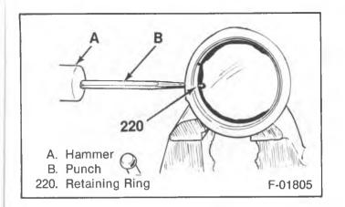
Figure 2—Unseating the Retaining Ring
