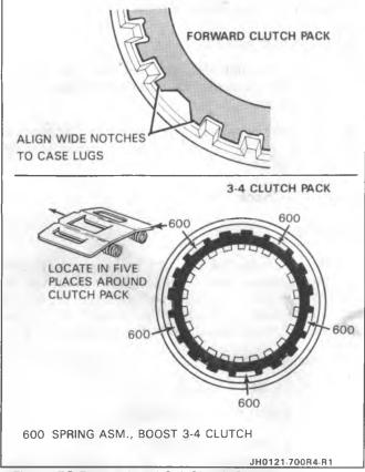
Figure 73 Forward and 3-4 Clutch Plates - Installed
