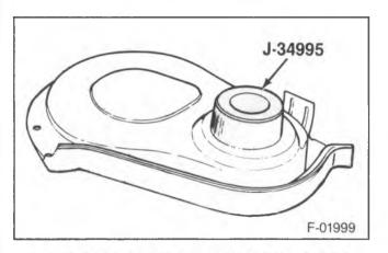
Figure 31-Installing the Front Crankshaft Seal
