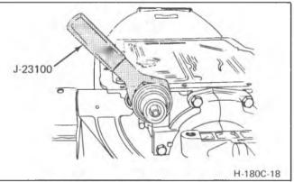
Figure 59 Installing Vacuum Modulator
