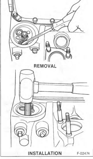
Figure 29—Oil Filter Bypass Valve Replacement
