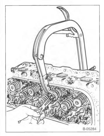
Figure 39—Compressing the Valve Springs
