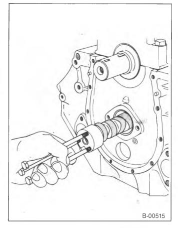
Figure 58—Installing the Camshaft
