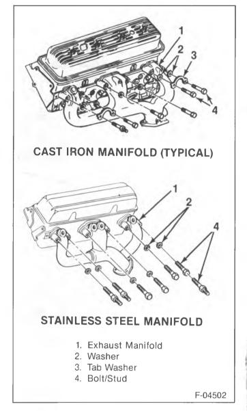
Figure 80—Exhaust Manifold (5.0L and 5.7L Engines)
