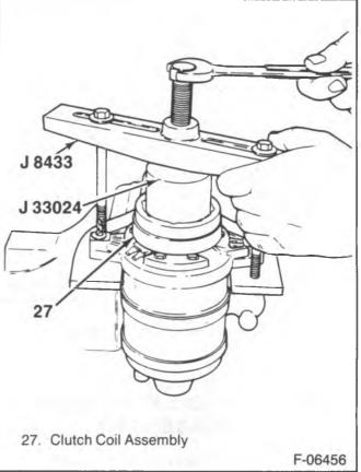
Figure 16—Removing the Clutch Coil Assembly
