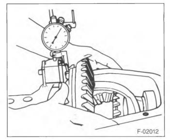
Figure 77—Measuring Differential Movement
