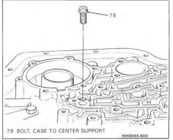
Figure 25 - Removing Center Support Bolt
