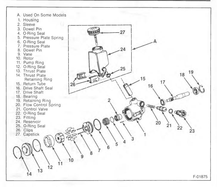
Figure 28—Power Steering Pump Components — Model TC
