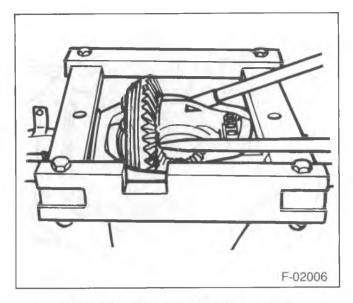
Figure 46—Removing the Differential
