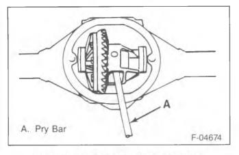
Figure 2—Removing the Differential Case
