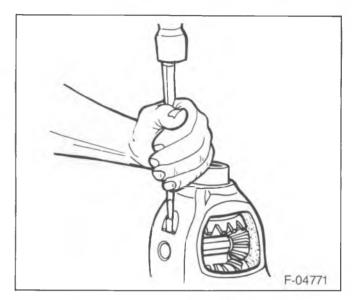
Figure 59—Installing the Lock Pin
