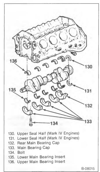
Figure 53—Crankshaft and Components (Typical)
