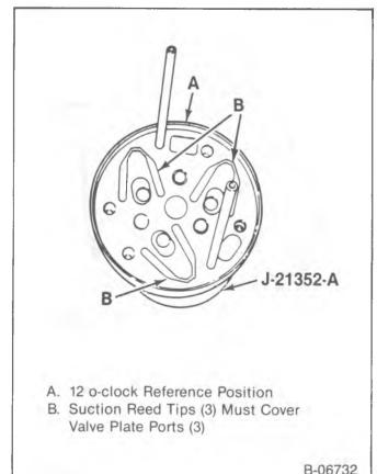
Figure 34 — Installing the Reed Plate
