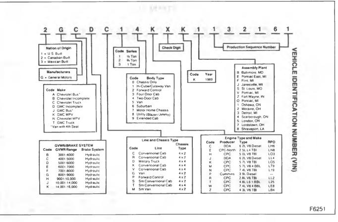
Figure 3—Vehicle Identification Number
