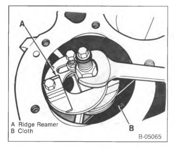
Figure 20—Removing the Cylinder Ridge
