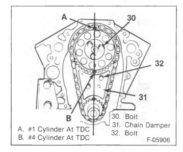
Figure 33—Camshaft Timing Marks
