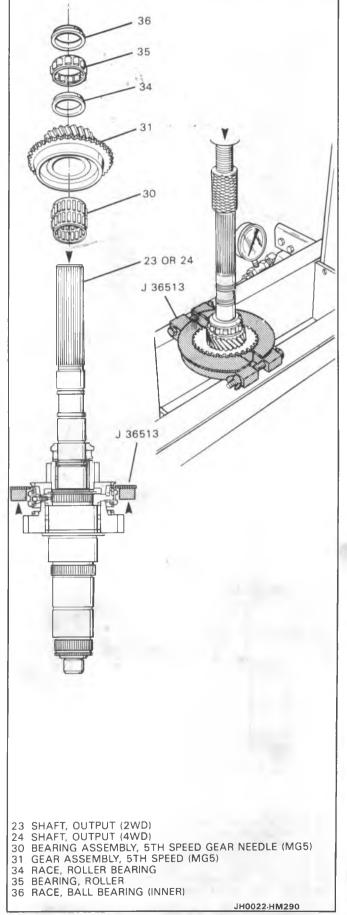
Figure 24 Removing 5th Gear Components
