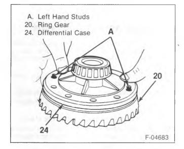
Figure 17—Ring Gear Studs
