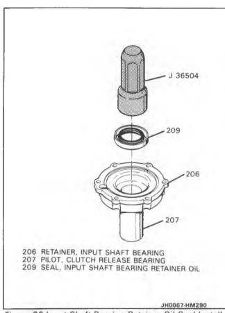
Figure 66 Input Shaft Bearing Retainer Oil Seal Install
