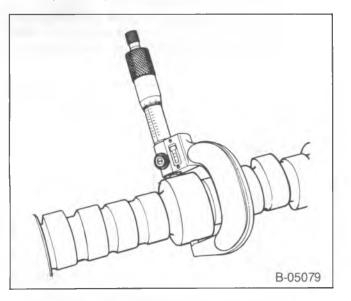
Figure 26—Checking the Camshaft Journals
