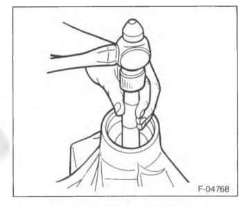
Figure 56—Removing the Bearing Cups
