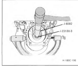
Figure 82 Removing or Installing Case Bushing
