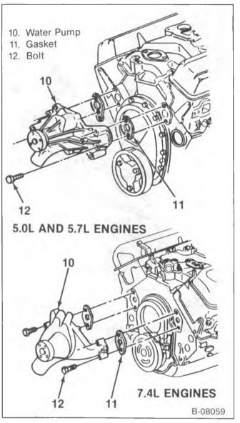
Figure 82—Water Pumps and Components
