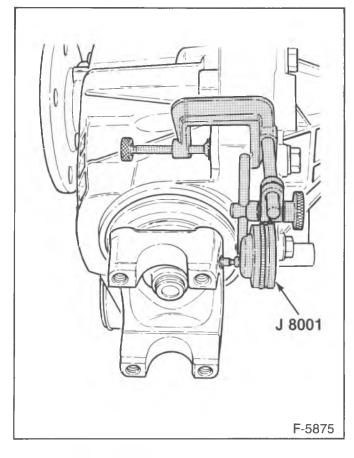
Figure 32—Measuring Backlash at the Pinion Flange
