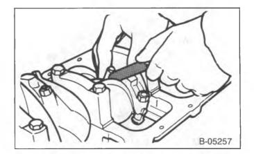
Figure 57—Measuring Connecting Rod Side Clearance
