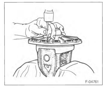
Figure 49—Removing the Lock Pin
