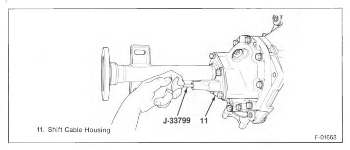
Figure 35—Checking the Shift Mechanism
