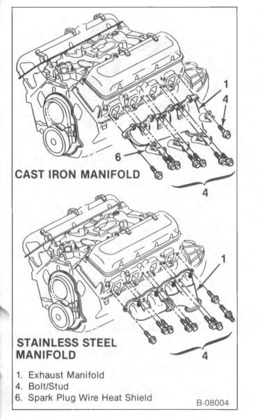
Figure 81—Exhaust Manifold (7.4L Engines)
