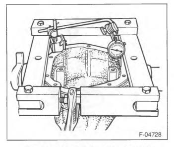
Figure 39—Mounting the Carrier Spreader
