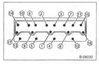
Figure 48—Head Bolt Tightening Sequence
