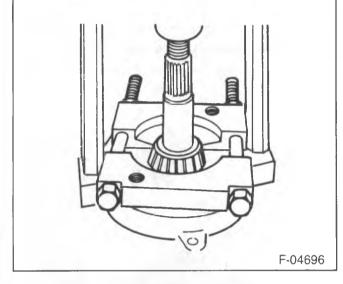
Figure 12—Removing the Pinion Bearing
