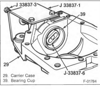
Figure 13—Removing the Inner Pinion Bearing Cup
