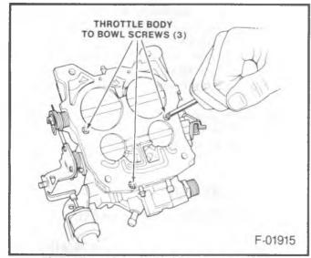
Figure 27 - Throttle Body Screw Location
