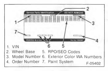
Figure 1—Service Parts Identification Label
