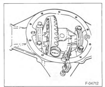
Figure 24—Checking Ring Gear Backlash
