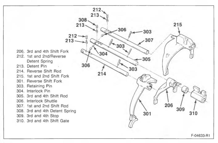
Figure 33B—C/K Shift Rod and Fork Positions
