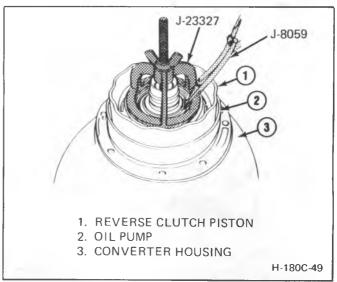
Figure 45 Compressing Reverse Clutch Piston Retainer
