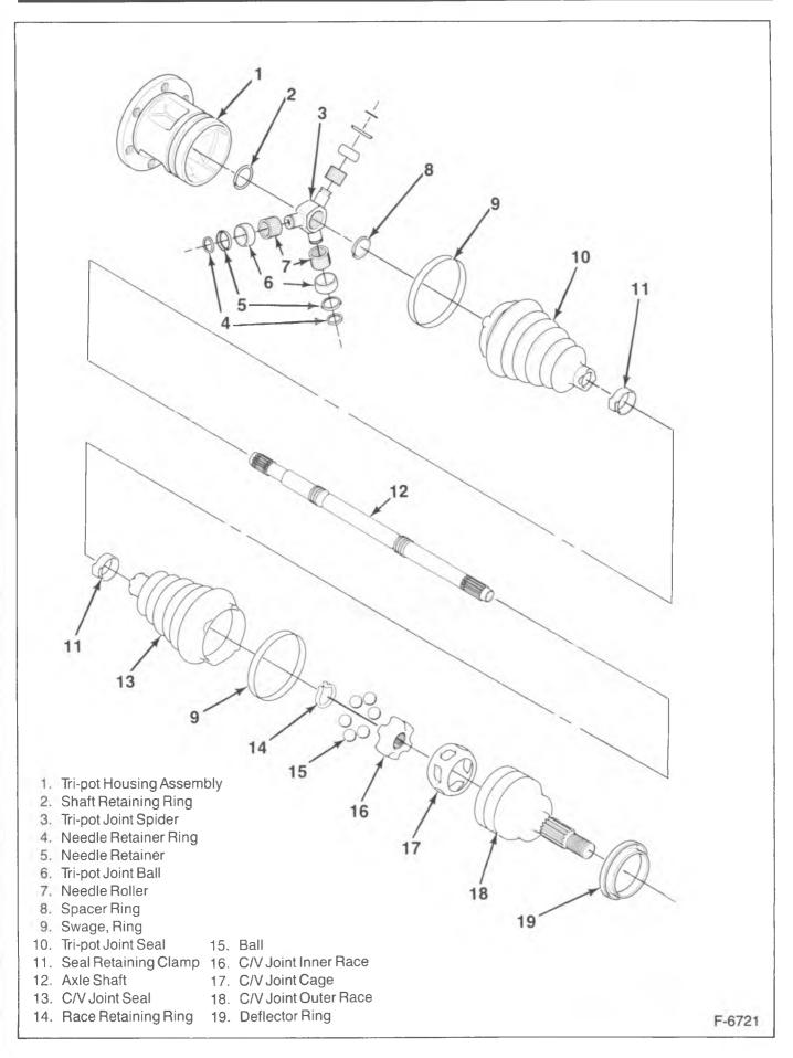
Figure 41—Front Drive Axle Components
