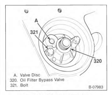
Figure 49-Oil Filter Bypass Valve
