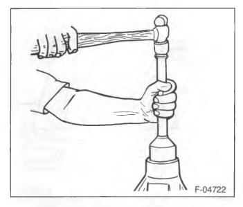
Figure 33—Installing the Pinion Seal
