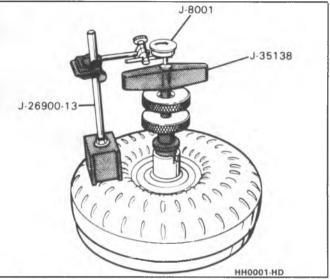
Figure 102 - Checking Torque Converter End Play
