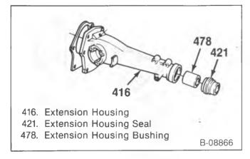
Figure 12—Extension Housing and Components
