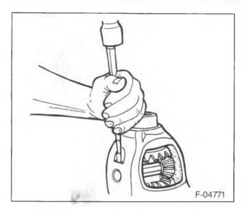
Figure 18—Installing the Lock Pin
