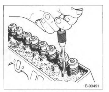
Figure 37—Reaming the Rocker Arm Stud Bore
