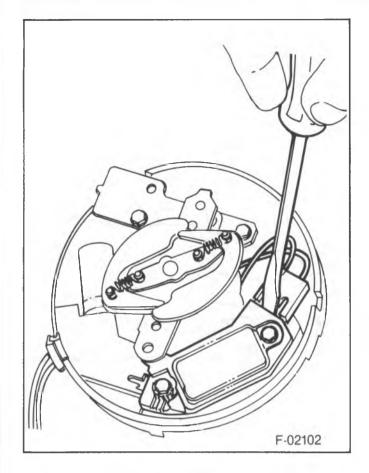
Figure 12—Removing the Pickup Coil Connector
