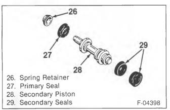
Figure 16—Secondary Piston Assembly
