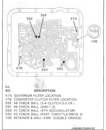
Figure 17 Case Checkballs and Filters
