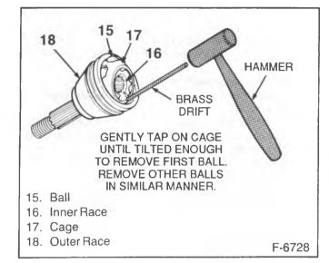
Figure 48—Removing C/V Joint Balls
