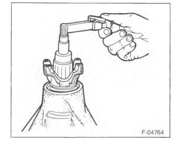
Figure 11-Checking the Pinion Preload
