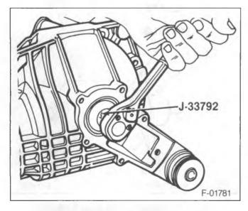
Figure 8—Removing the Side Bearing Cup
