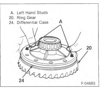
Figure 18—Aligning the Ring Gear Studs
