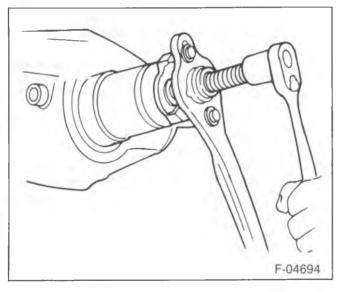
Figure 6—Removing the Pinion Flange
