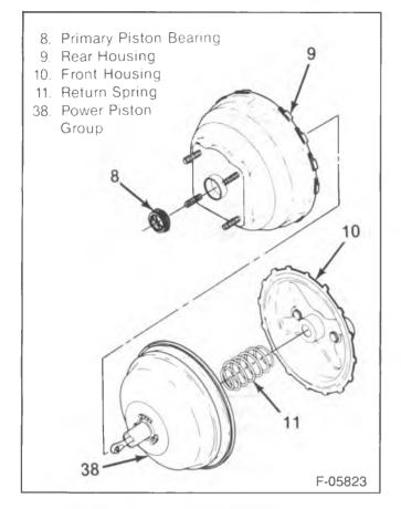
Figure 26—Booster Inner Components
