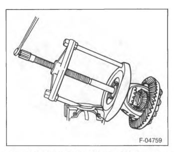
Figure 14—Removing the Differential Side Bearings
