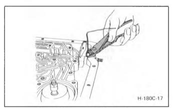
Figure 6 Removing Spring Pin
