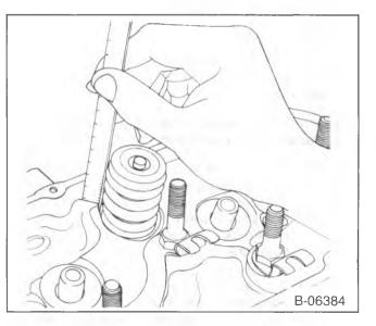
Figure 36—Measuring Valve Spring Installed Height
