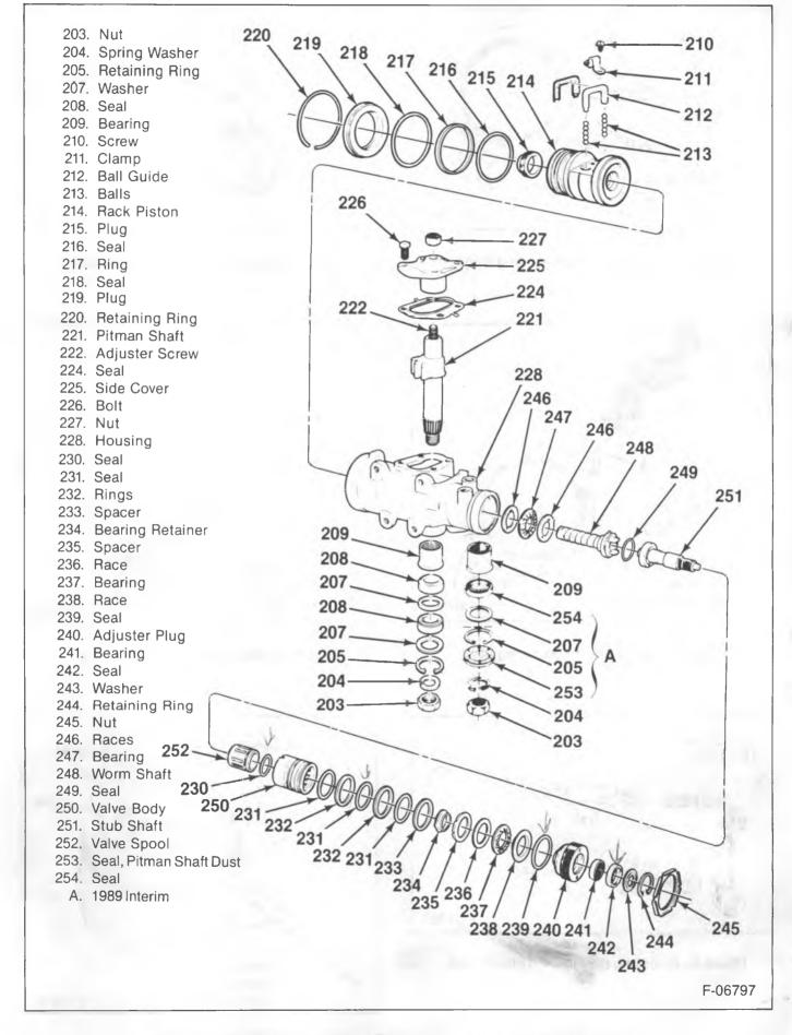
Figure 1—Integral Steering Gear Components — RV, G, P, ST and M Vehicles
