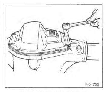
Figure 2-Removing the Axle Cover
