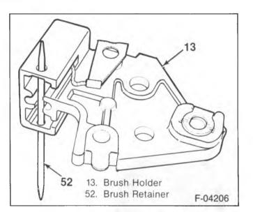
Figure 16-Brush Retainer Installed
