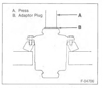
Figure 18-Installing the Ring Gear
