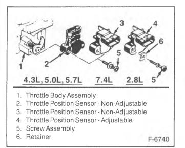
Figure 5—TBI Model 220 TPS Configuration
