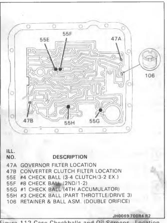
Figure 112 Case Checkballs and Oil Screens - Location
