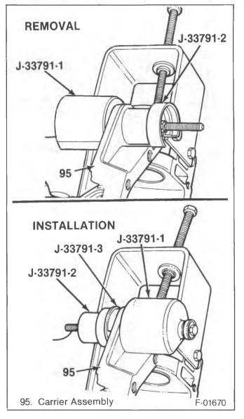
Figure 15—Replacing the Case Bushings
