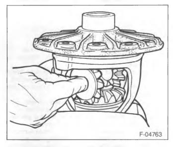
Figure 10—Removing the Pinion Gears
