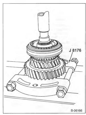
Figure 12 – Removing the Mainshaft from the 2nd and 3rd Speed Gears
