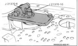
Figure 86 - Installing Servo Pin Gage
