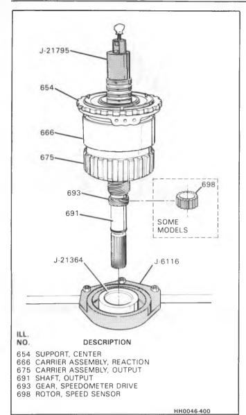
Figure 26 - Removing Center Support and Gear Unit Assembly
