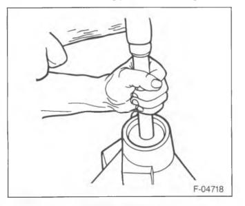
Figure 29—Installing the Pinion Front Cup
