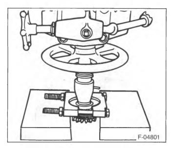
Figure 4—Removing the Thrust Ring
