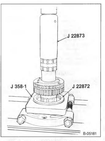
Figure 18 –Installing the 1st Speed Gear Bushing
