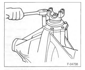
Figure 15—Installing the Pinion Cage
