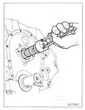
Figure 30—Installing the Camshaft
