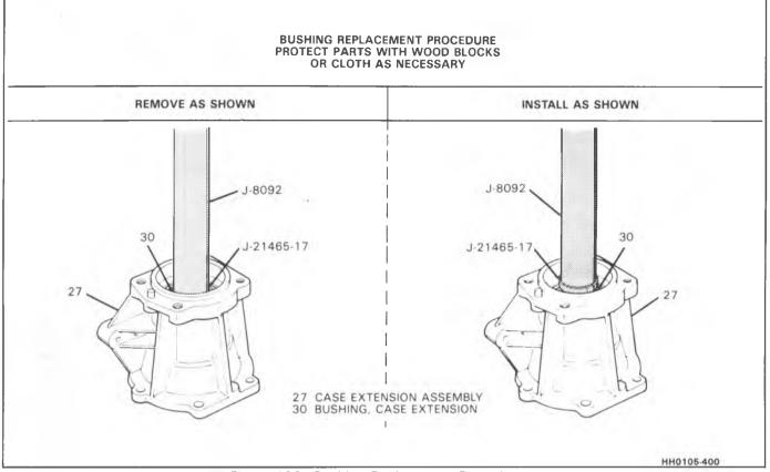
Figure 106 - Bushing Replacement Procedure
