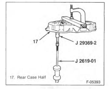
Figure 9—Removing the Front Output Shaft Rear Bearing
