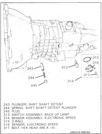
Figure 90 External Components Install
