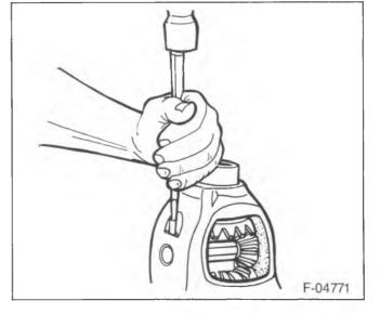
Figure 19—Installing the Lock Pin
