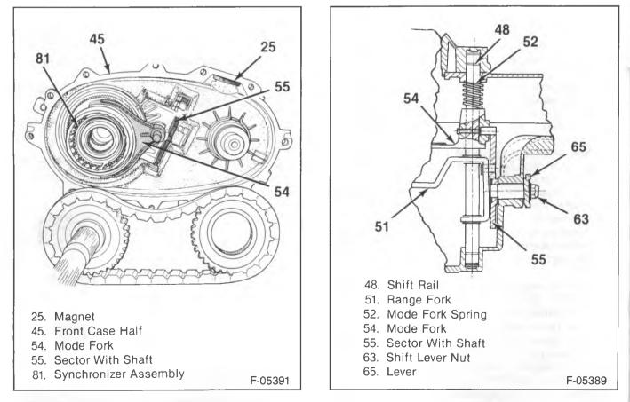
Figure 5—Mode Fork and Shaft Assembly
