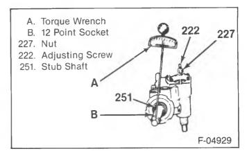
Figure 21—Aligning the Over-Center Preload
