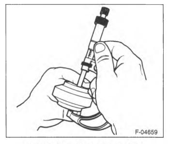
Figure 17—Measuring the Reaction Block
