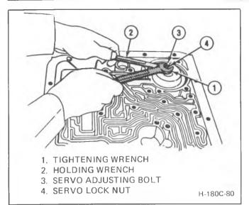
Figure 63 Tighten Servo Nut
