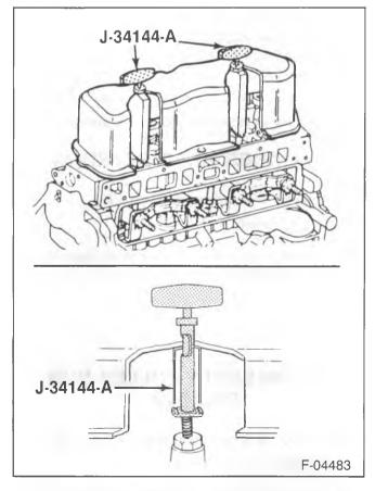
Figure 9—Removing the Rocker Arm Cover
