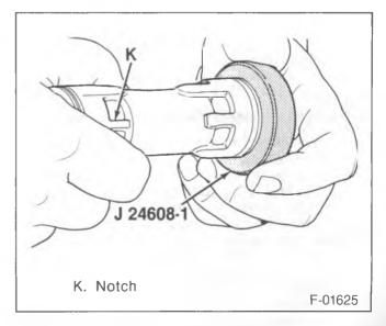
Figure 39—Gaging the Piston Ring Size
