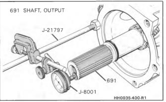
Figure 16 - Checking Rear Unit End Play
