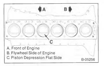
Figure 56—Pistons Installed
