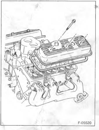
Figure 42—Rocker Arm Cover Installation
