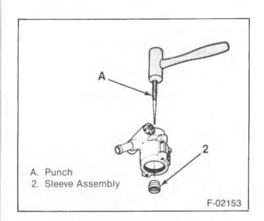
Figure 38—Removing the Sleeve Assembly
