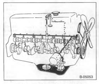
Figure 1—Lubrication Diagram (Side View)
