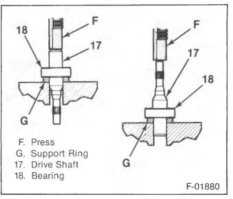
Figure 33—Remove and Install Driveshaft Bearing
