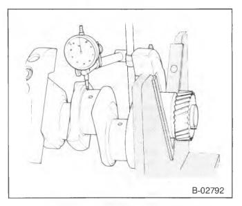
Figure 43—Checking Crankshaft Runout
