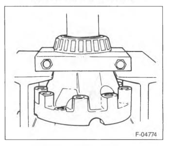
Figure 10-Removing the Differential Side Bearing
