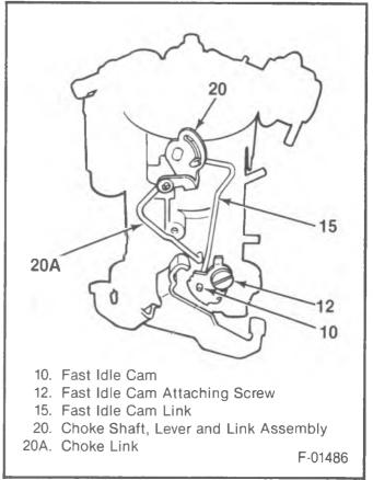
Figure 15 – Fast Idle Cam and Cam Link
