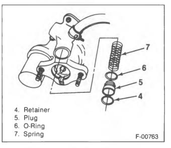
Figure 3—Removing the Plug and Spring
