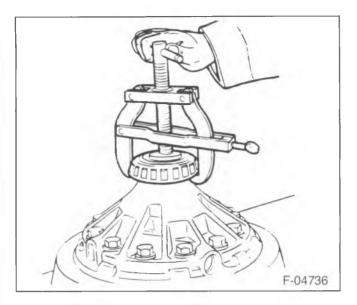
Figure 2-Removing the Differential Side Bearings
