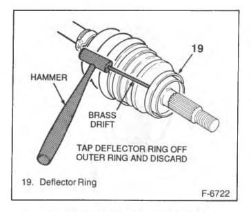
Figure 42—Removing Outer Deflector Ring
