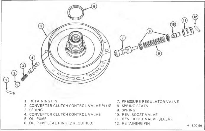
Figure 43 Exploded View - Valves in Oil Pump
