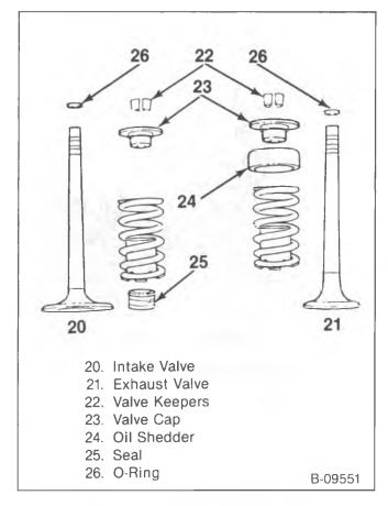
Figure 23—Valves and Components
