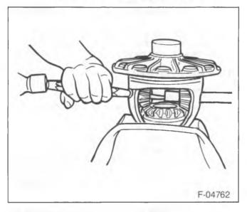
Figure 9—Removing the Pinion Shaft
