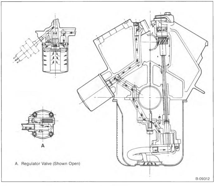
Figure 4—Engine Lubrication Diagram
