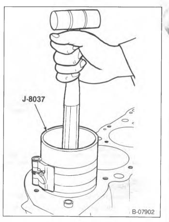
Figure 64—Installing the Piston
