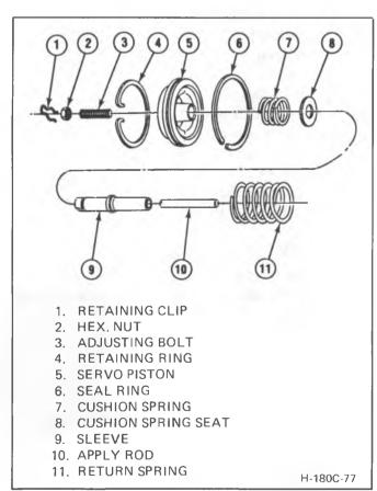
Figure 60 Servo Piston - Exploded View
