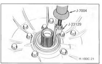
Figure 12 Removing Converter Housing Oil Seal
