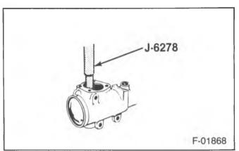
Figure 5—Removing the Pitman Shaft Bearing
