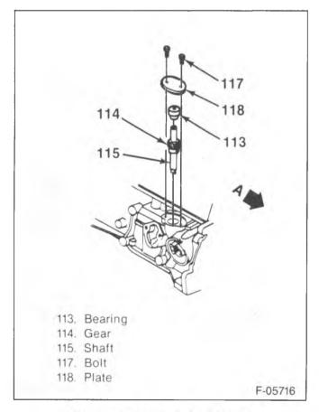
Figure 15-Oil Pump Drive Shaft
