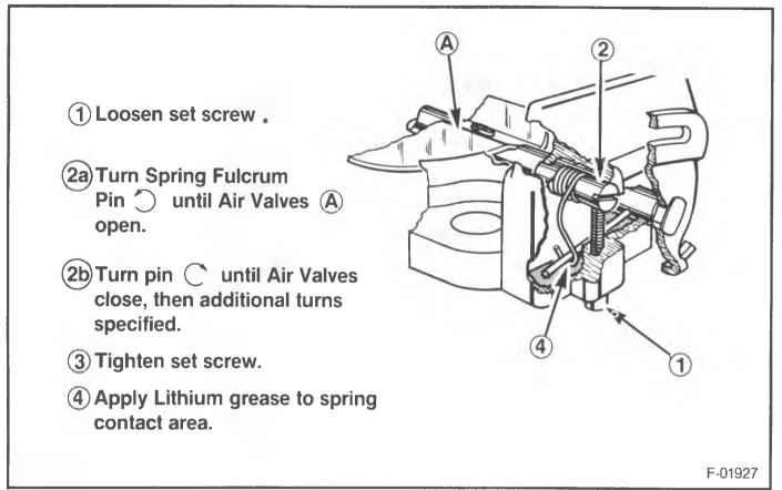
Figure 42 - Air Valve Return Spring Adjustment
