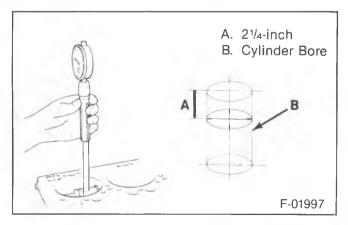
Figure 24—Measuring Cylinder Bore Diameter
