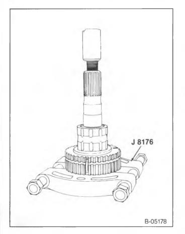
Figure 13 – Removing the Mainshaft from the 1st and 2nd Speed Synchronizer Hub
