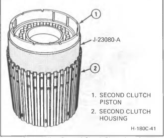
Figure 35 Installing Second Clutch Piston Into Second Clutch Drum
