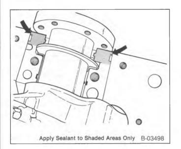
Figure 54—Applying Sealant to the Block (7.4L Engines)
