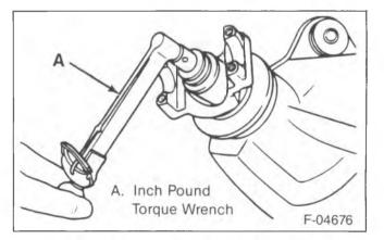
Figure 15—Checking Pinion Preload
