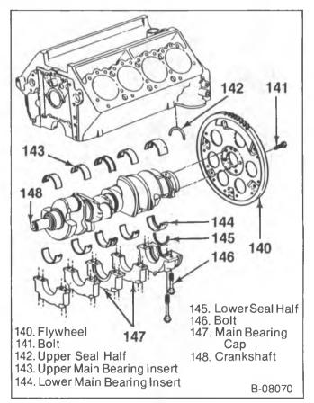
Figure 30—Crankshaft and Components
