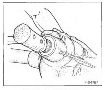
Figure 14-Removing the Pinion
