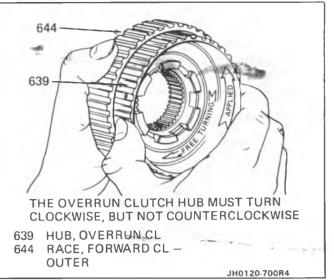
Figure 72 Check Sprag for Proper Operation
