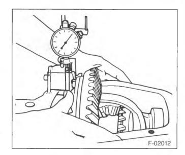
Figure 22—Determining Differential Shim Pack
