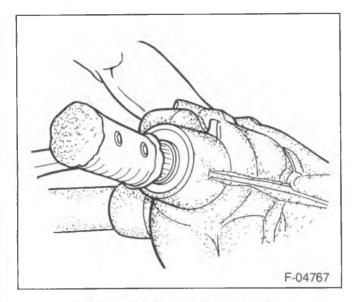
Figure 14—Removing the Pinion
