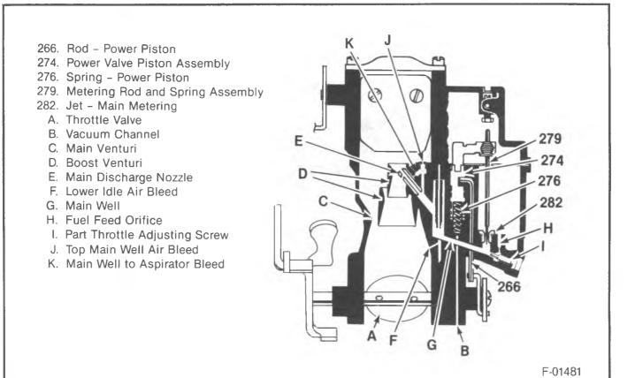
Figure 5 – Main Metering System
