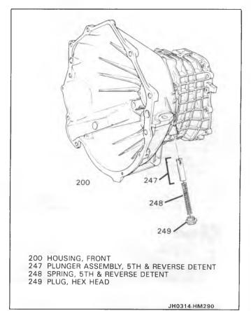
Figure 41 Removing 5th-Reverse Detent Plunger
