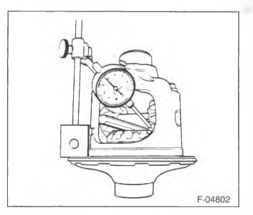
Figure 5—Checking Cam Gear Backlash
