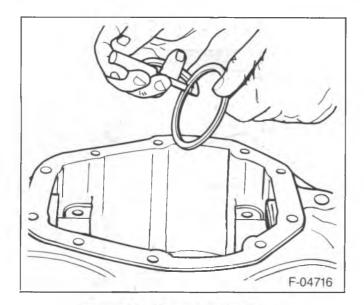
Figure 28—Measuring the Shims
