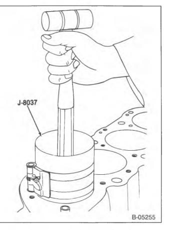
Figure 49—Installing the Piston
