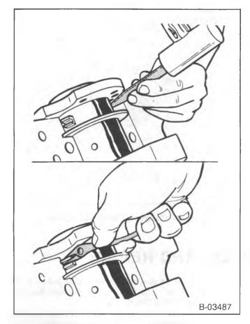
Figure 20—Removing the Upper Seal Half
