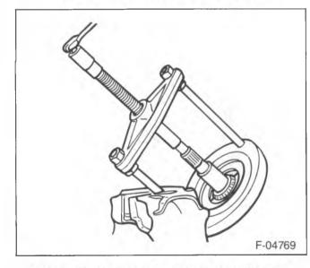
Figure 57—Removing the Pinion Inner Bearing
