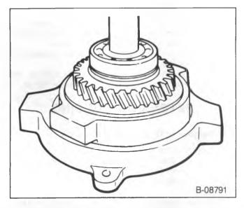
Figure 8—Pressing the Mainshaft through the Bearing
