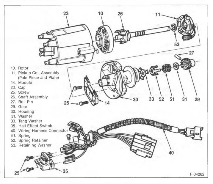
Figure 26—Distributor Components (Separate Coil)
