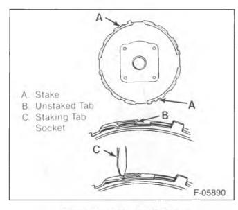
Figure 23—Staking the Tabs
