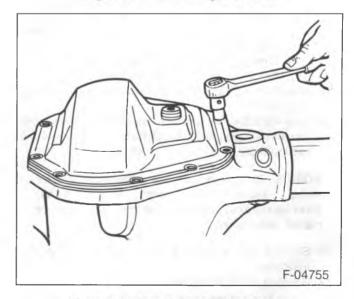
Figure 82—Installing the Axle Cover
