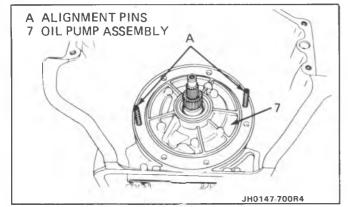
Figure 102 Oil Pump and Case
