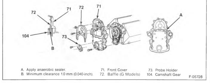
Figure 40—Front Cover Installation
