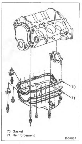
Figure 6—Oil Pan Installation
