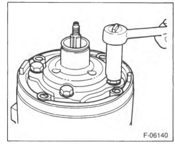
Figure 17—Removing the Front Head Mounting Screws
