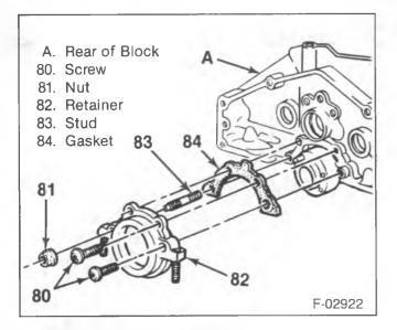
Figure 27—Rear Crankshaft Oil Seal Retainer Installation
