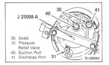
Figure 5—Compressor in Holding Fixture
