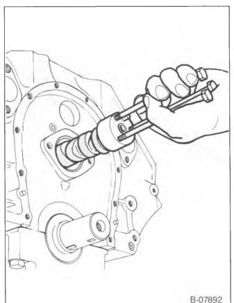
Figure 13—Replacing the Camshaft (Typical)
