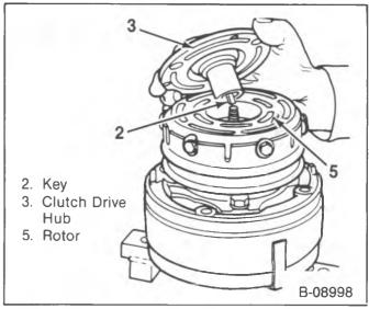
Figure 34—Installing the Shaft Key
