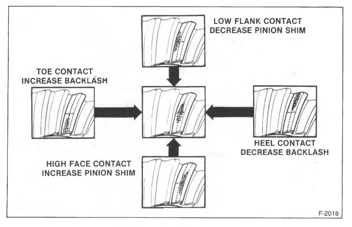
Figure 34—Gear Tooth Contact Pattern
