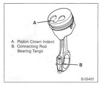
Figure 14—Aligning the Piston and Connecting Rod
