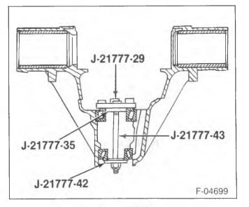
Figure 11—Gage Plate Components
