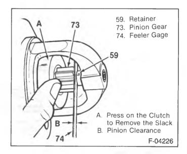
Figure 17—Measuring Pinion Clearance
