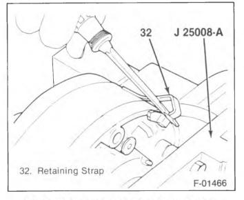
Figure 20—Releasing the Shell Retaining Strap
