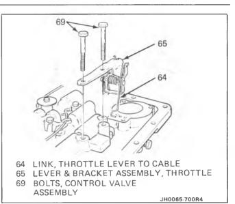
Figure 13 T.V. Lever and Bracket
