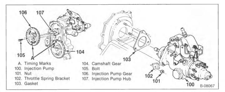
Figure 10—Injection Pump
