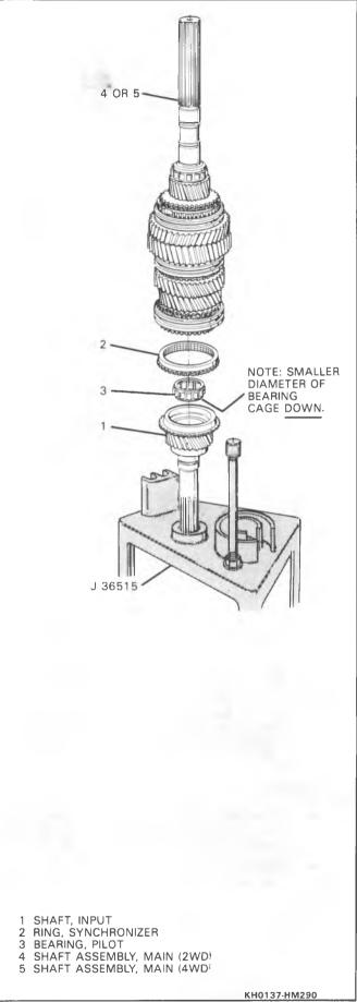
Figure 70 Mainshaft Components Install
