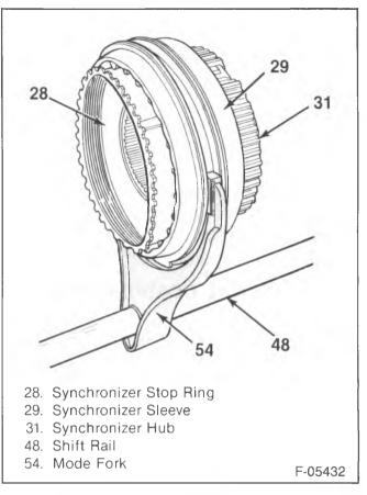
Figure 16—Synchronizer Hub Assembly and Mode Fork
