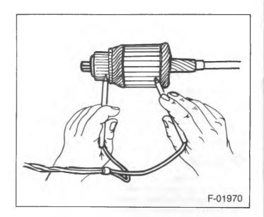
Figure 14—Testing the Armature for Grounds
