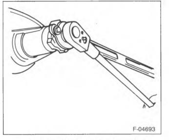
Figure 5—Pinion Flange Nut Removal
