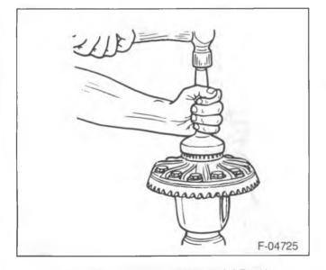
Figure 37—Installing the Differential Bearings
