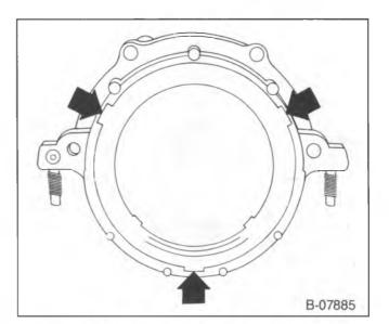
Figure 50—Seal Removal Notches
