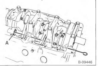
Figure 21—Checking Camshaft Bearing Oil Hole Alignment (Typical)
