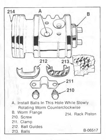
Figure 12—Installing the Balls into the Rack Piston
