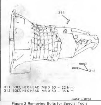
Figure 3 Removing Boits for Special Too
