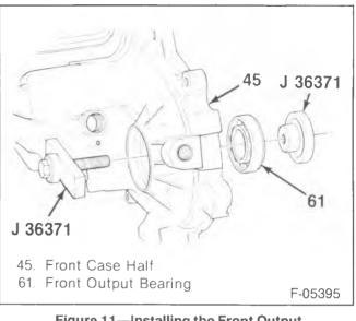
Figure 11—Installing the Front Output Bearing
