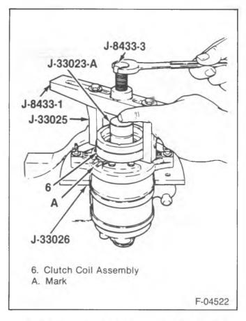
Figure 17 — Removing the Clutch Coil Assembly
