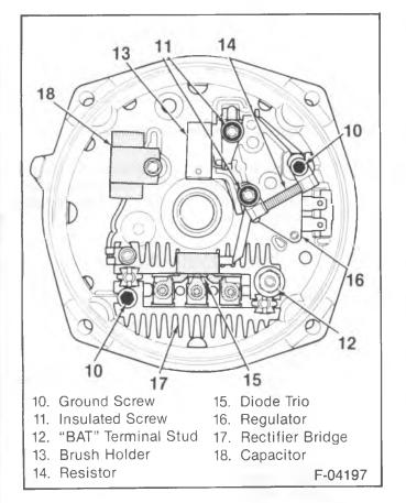
Figure 6—Slip Ring End Frame: 12-SI 100
