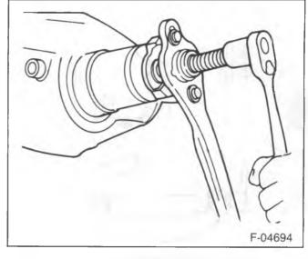
Figure 6—Removing the Pinion Flange
