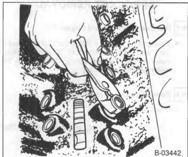
Figure 12—Removing the Hydraulic Lifter
