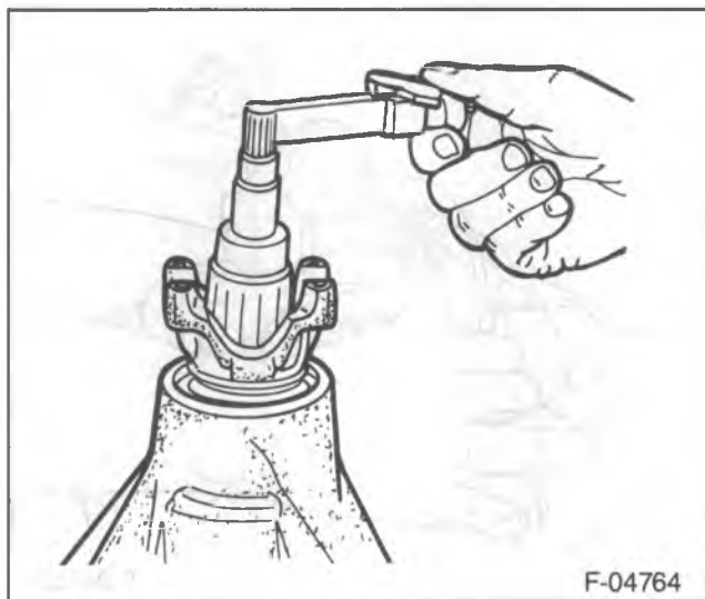
Figure 36—Checking Pinion Preload
