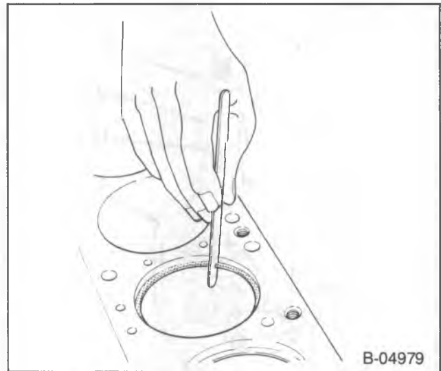
Figure 16—Measuring Ring End Gap
