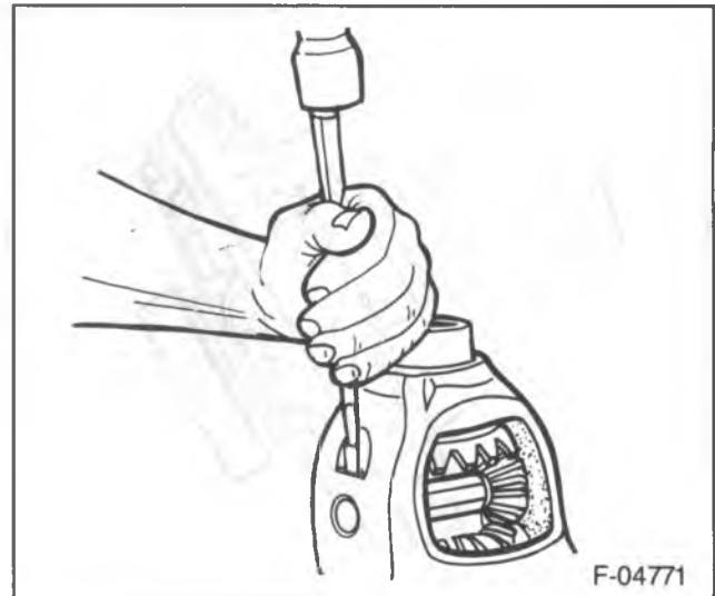
Figure 18—Installing the Lock Pin
