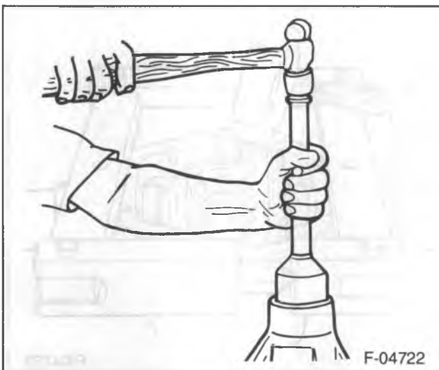
Figure 33—Installing the Pinion Seal
