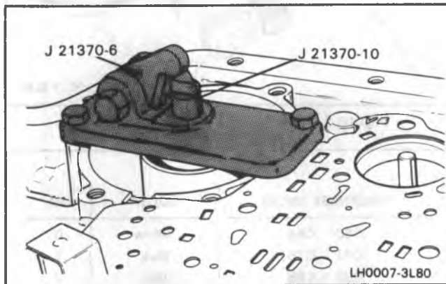
Figure 7 — Installing Servo Pin Gage
