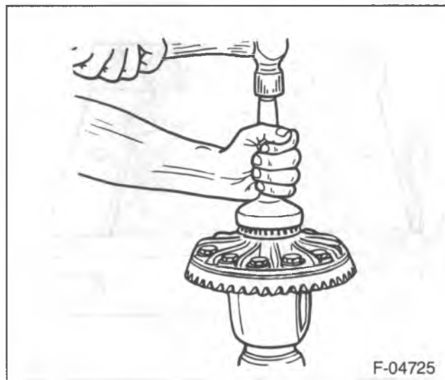
Figure 38—Installing the Differential Bearings
