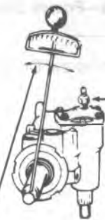
With gear at center of travel, check torque to turn stub shaft (reading #1).
