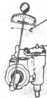
Torque adjuster lock nut to 27 Newton Metres (20 Ft. Lbs.)
