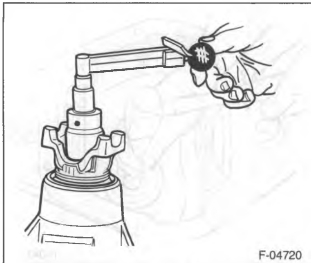
Figure 32—Checking the Pinion Preload
