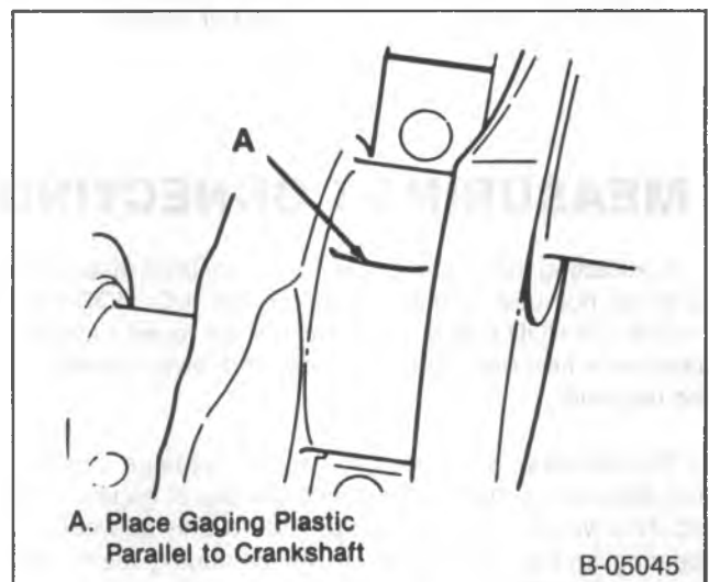
Figure 37—Placing the Gaging Plastic on the Bearing Journal
