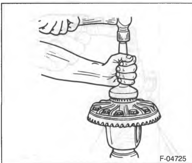
Figure 37—Installing the Differential Bearings
