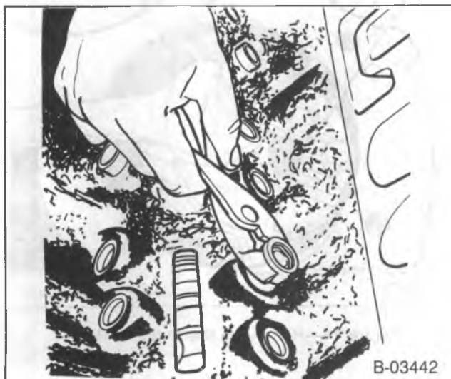
Figure 10—Removing the Hydraulic Lifter with J 3049
