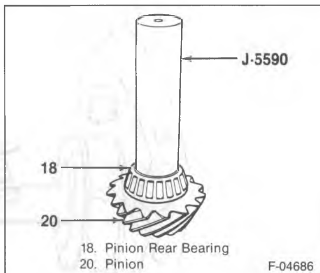
Figure 14—Installing the Pinion Inner Bearing
