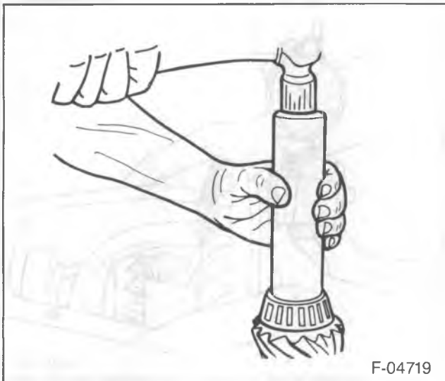
Figure 71—Installing the Inner Bearing
