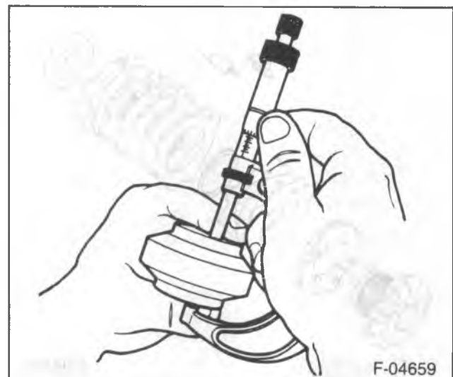
Figure 17—Measuring the Reaction Block
