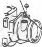
Remove check valve.
