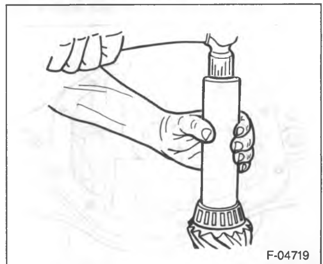
Figure 31—Installing the Inner Bearing
