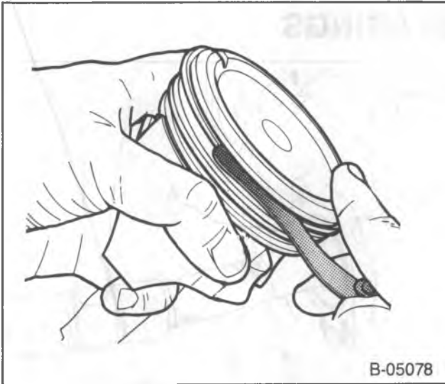
Figure 18—Measuring Ring Clearance
