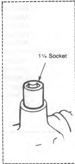
Install Pitman shaft seals.
