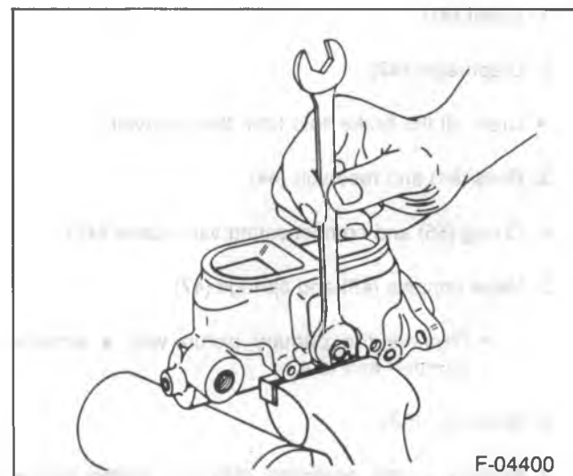
Figure 18—Installing Tube Seats
