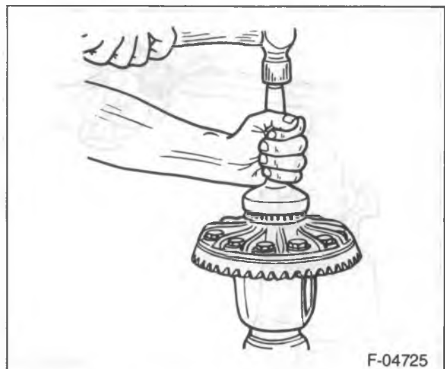
Figure 78—Installing the Differential Bearings
