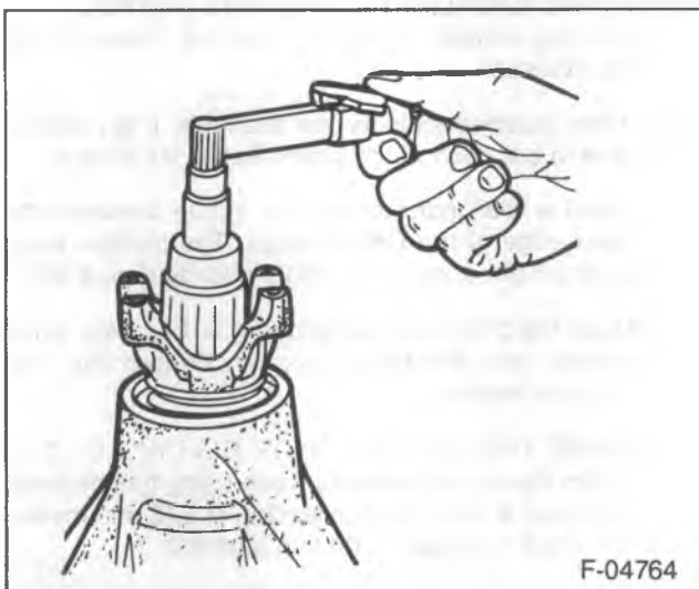
Figure 22—Measuring Pinion Bearing Preload
