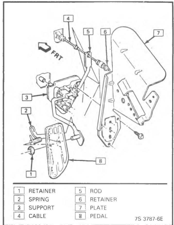
Figure 4-85 - Control Cable - 2.5L
