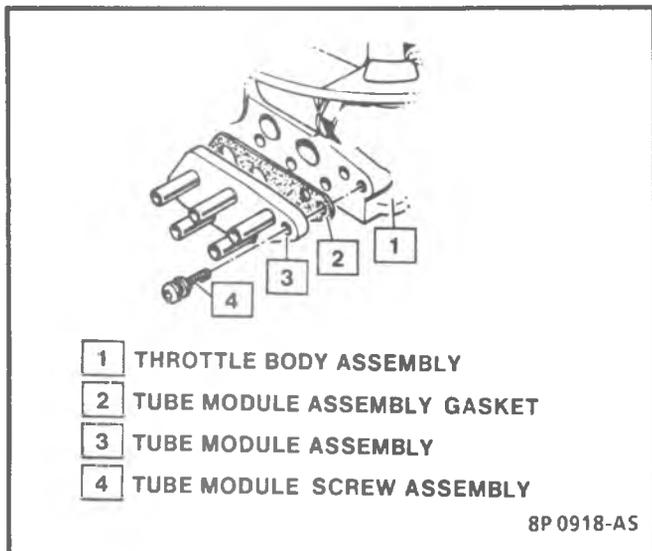
Figure 4-42 - Tube Module Assembly - TBI 700
