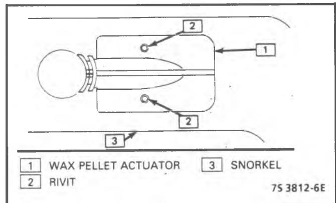
Figure 12-6 - Replacing Wax Pellet Actuator
