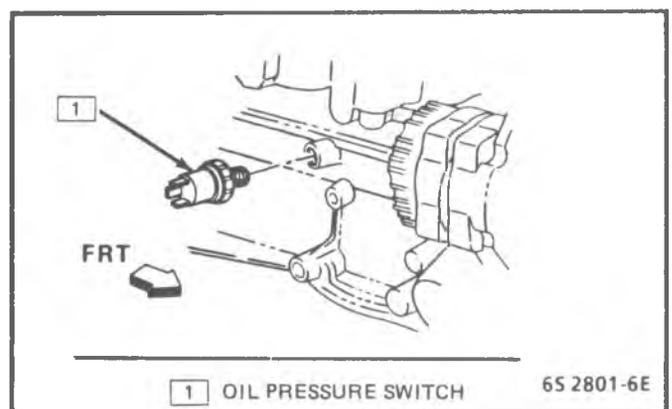
Figure 4-54 - Oil Pressure Switch (2.5L)
