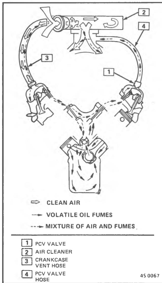
Figure 11-2 - PCV Flow (V6 and V8)
