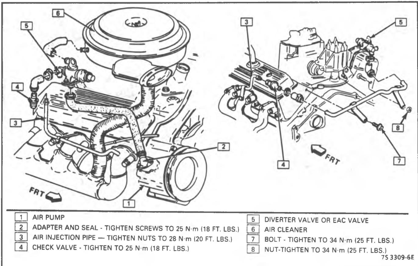
Figure 8-8 - Air System - 4.3L - G & M Series
