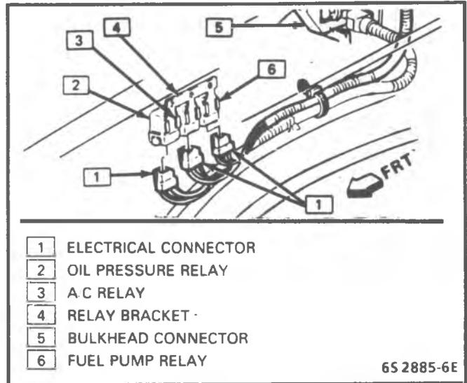
Figure 3-67 - A/C Clutch Control Relay - (S/T)
