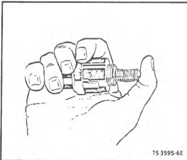
Figure 4-32 - Adjusting Valve Pintle - Thread Type
