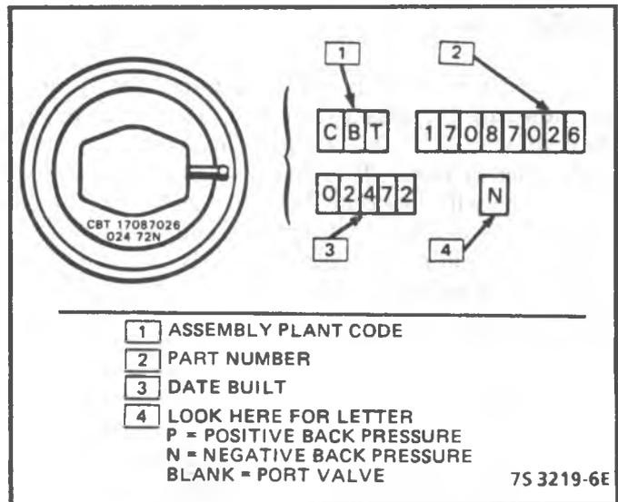
Figure 9-4 - EGR Valve Identification
