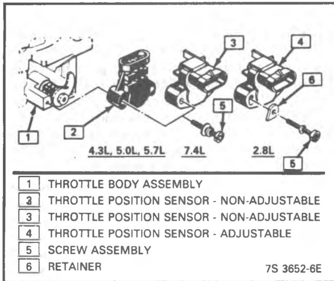
Figure 3-9 Throttle Position Sensor - V6/V8
