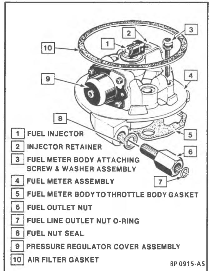
Figure 4-38 - Fuel Meter Assembly - TBI 700
