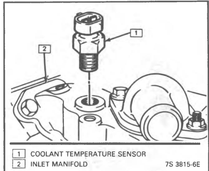
Figure 3-46 - Coolant Sensor
