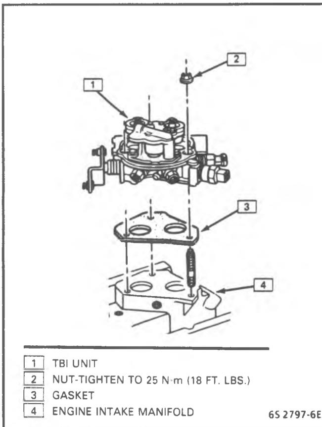
Figure 4-17 - Replacing TBI 220 Unit - 2.8L Engine
