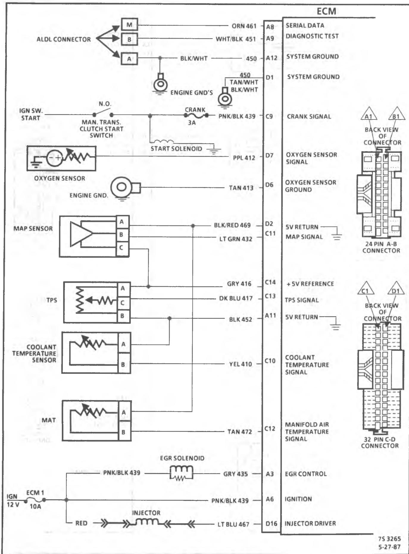
Figure 3-23 - ECM Wiring Diagram - 2.5L (1 of 3)
