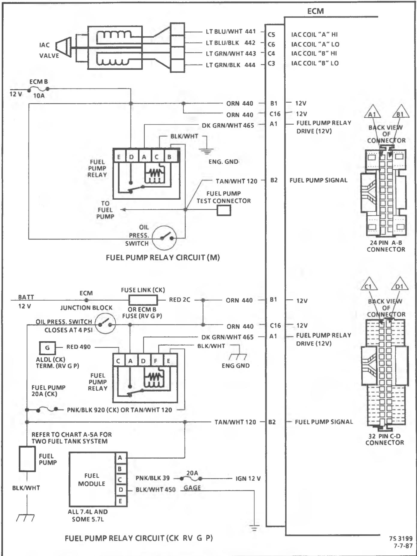
Figure 30 - ECM Wiring Diagram - 4.3L & V8 (2 of 4)
