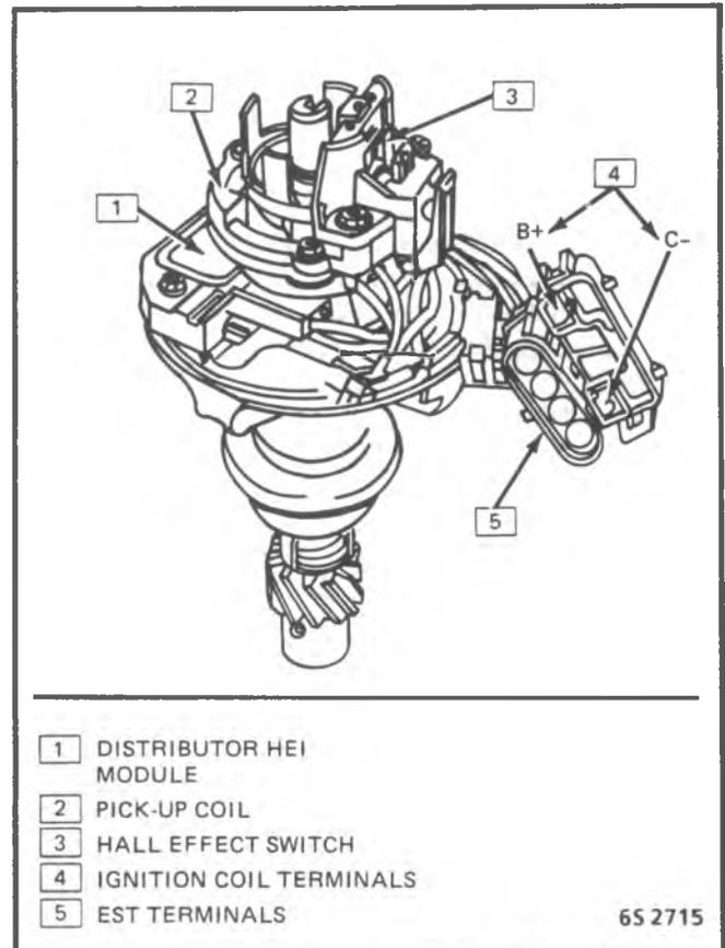
Figure 6-3 - Distributor (2.5L S/T Truck)
