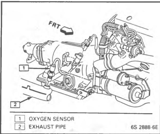
Figure 3-56 - Oxygen Sensor - 2.8L (ST)
