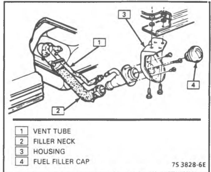
Figure 4-72 - Filler Neck - RV Chassis Cab
