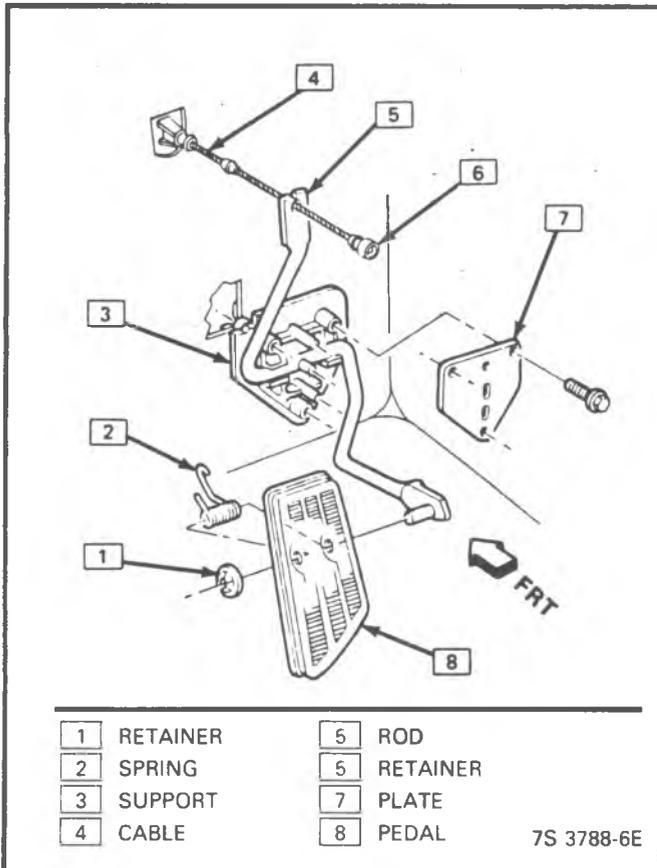
Figure 4-89 - Accelerator Pedal - CK
