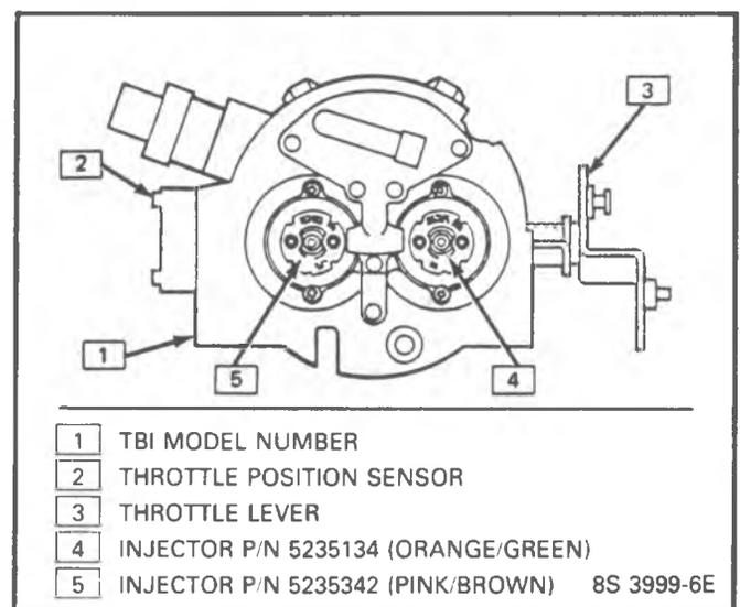
Figure 4-25 - Fuel Injector Color Code Locations
