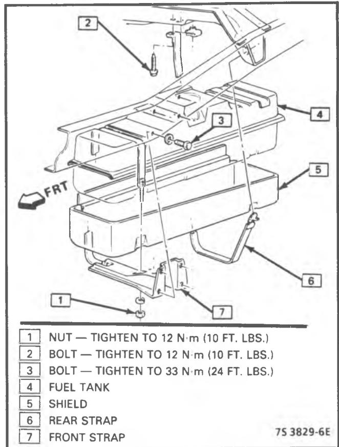
Figure 4-76 - Fuel Tank - CK Chassis Cab
