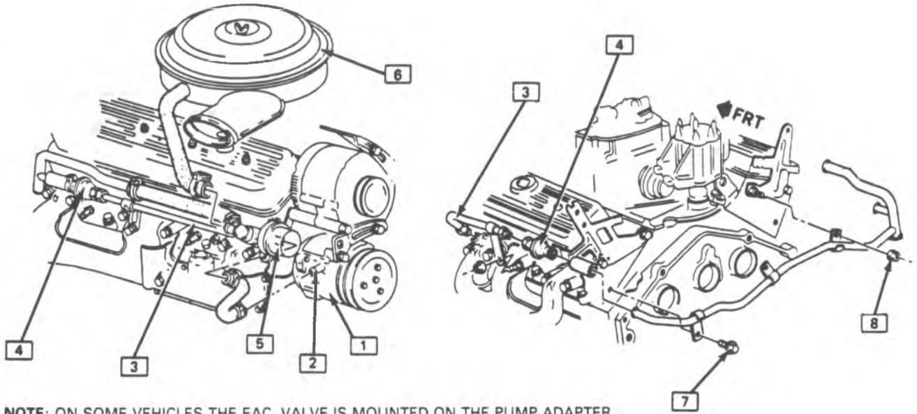
NOTE: ON SOME VEHICLES THE EAC VALVE IS MOUNTED ON THE PUMP ADAPTER
