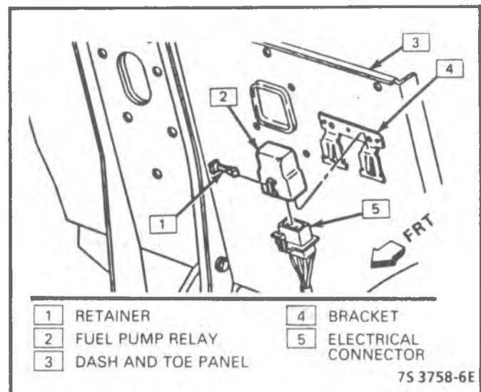
Figure 4-50 - Fuel Pump Relay (P)
