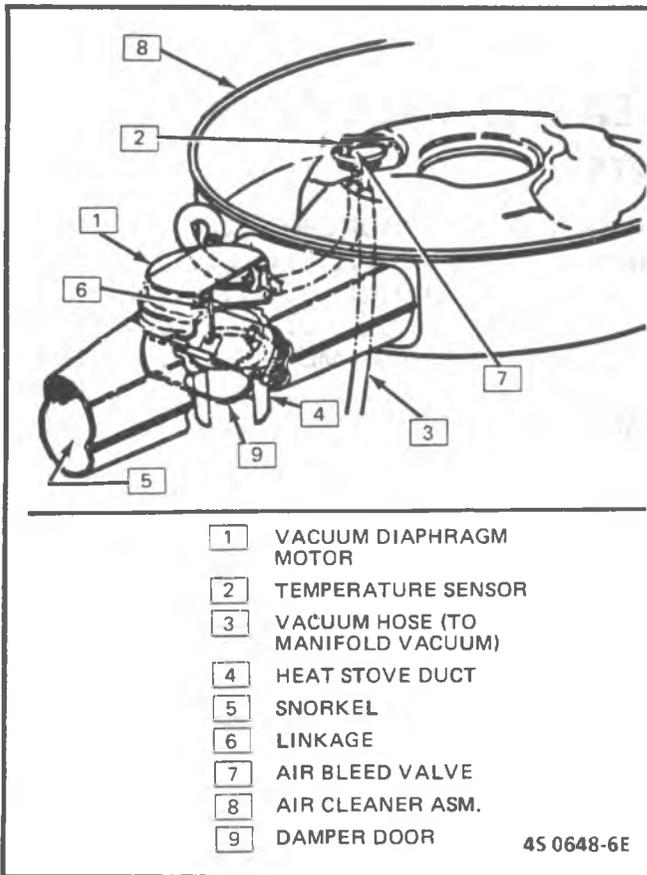
Figure 12-2 - THERMAC Air Cleaner - S/T Series
