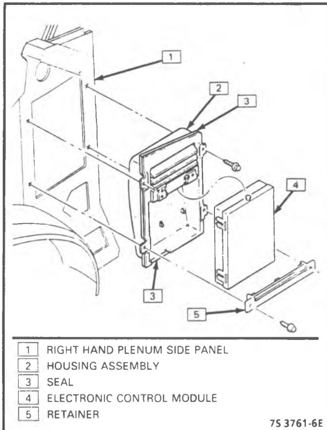
Figure 3-37 - Electronic Control Module (M)
