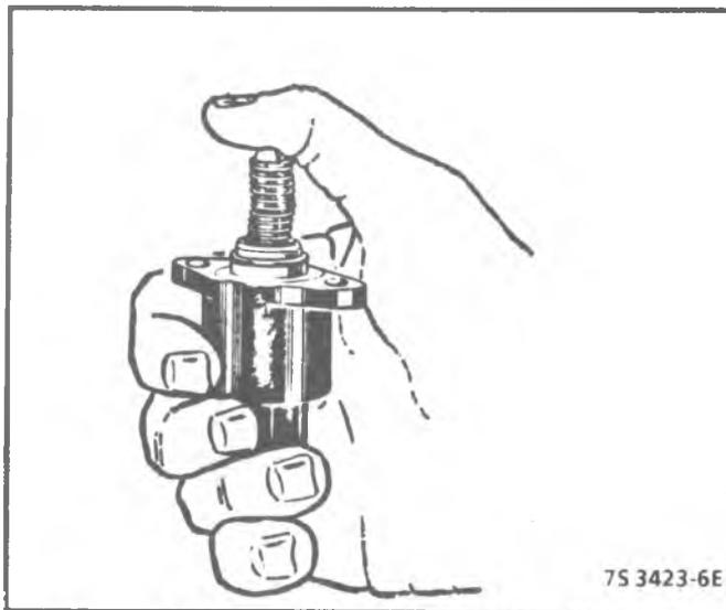
Figure 4-41 - Adjusting Valve Pintle - TBI 700
