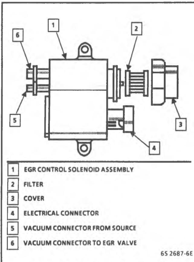
Figure 9-16 EGR Control Solenoid
