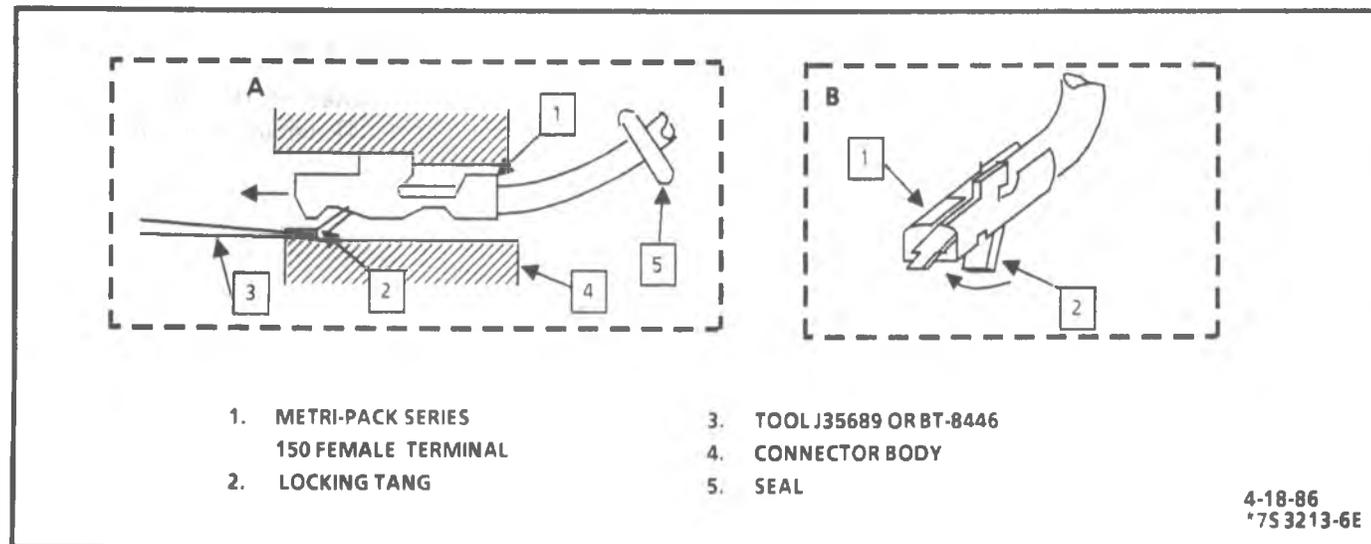
Figure 3-21 - Metri-Pack Series 150 Terminal Removal
