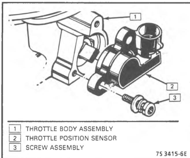
Figure 3-62 - Throttle Position Sensor - TBI 700
