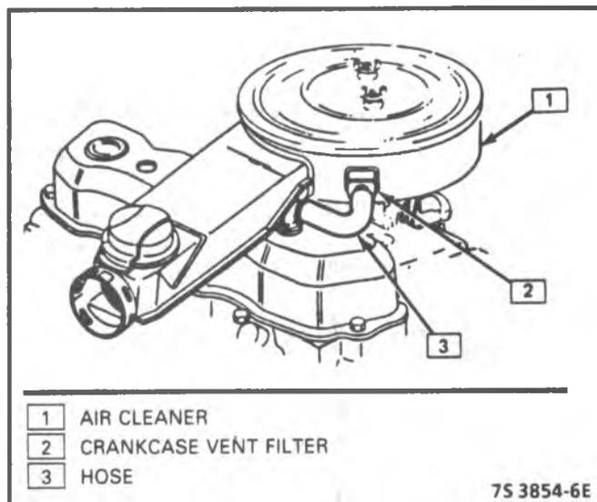
Figure 11-4 - Crankcase Vent Filter
