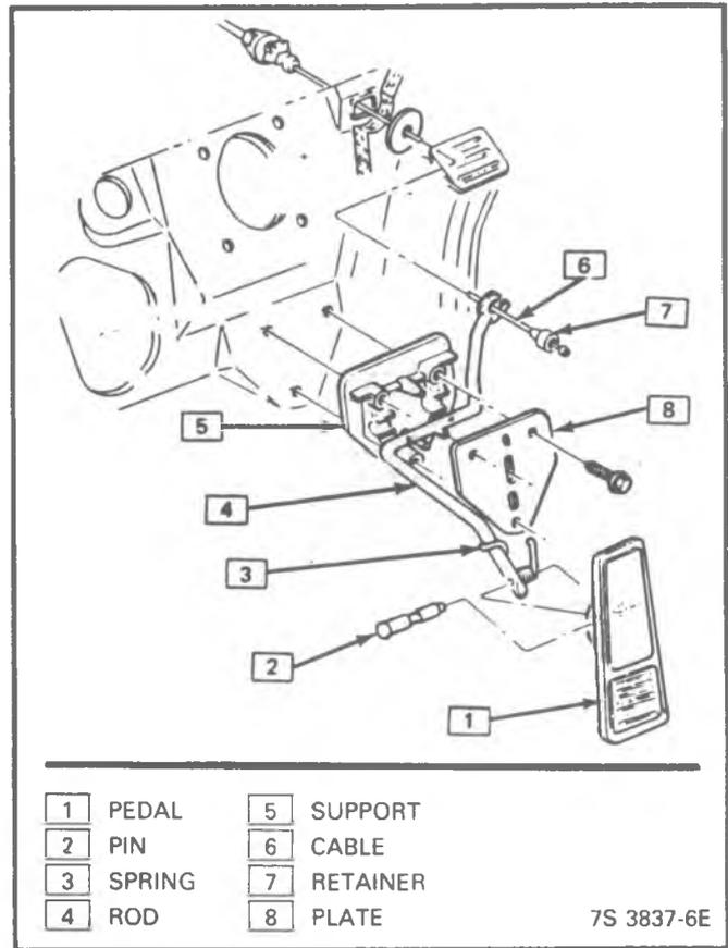
Figure 4-87 - Accelerator Pedal - M
