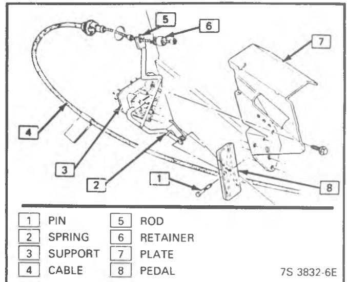
Figure 4-91 - Accelerator Pedal - P (42)
