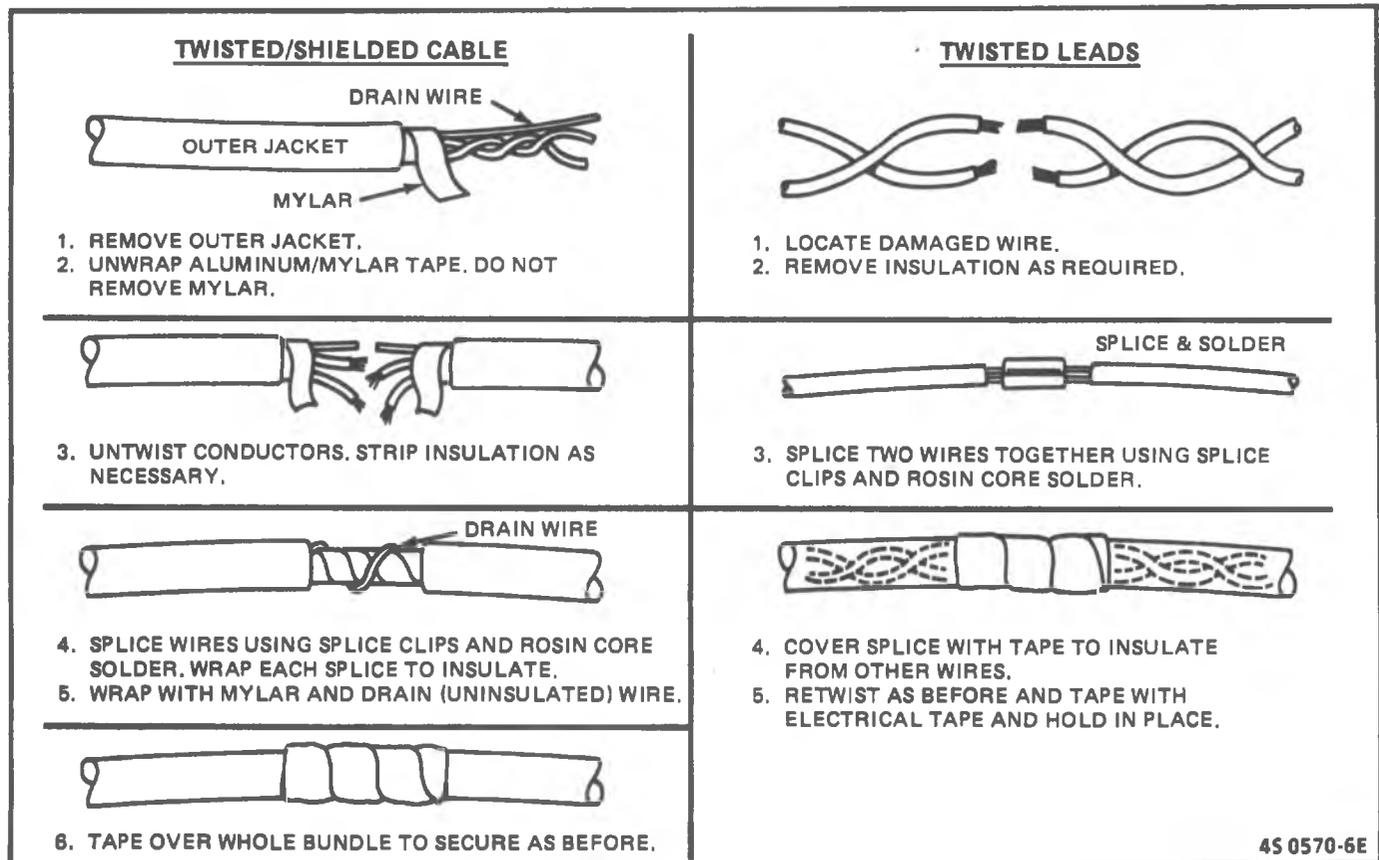
Figure 3-19 - Wire Harness Repair
