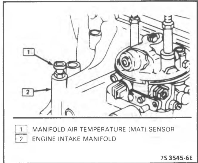
Figure 3-11 Manifold Air Temperature Sensor - L4
