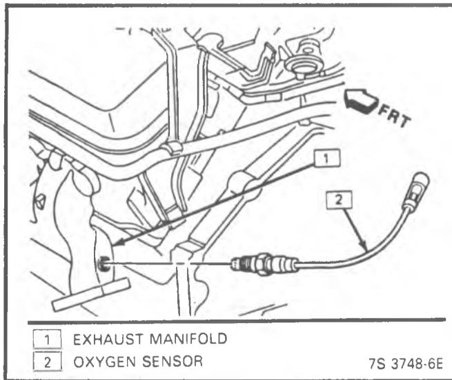
Figure 3-61 - Oxygen Sensor - 7.4L (RVG)
