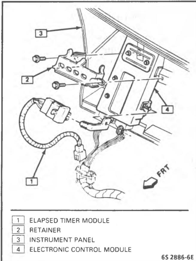
Figure 3-36 - Electronic Control Module (ST)
