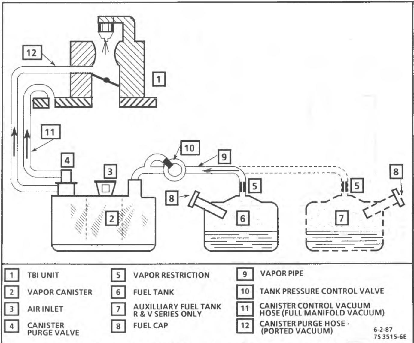
Figure 5-8 Evaporative Emissions Control System Schematic - 4.3L & V8 - Altitude
