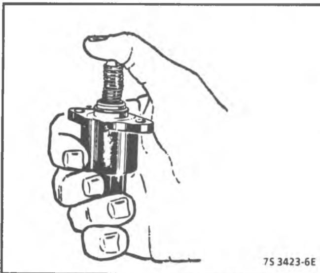
Figure 4-33 - Adjusting Valve Pintle - Flange Type
