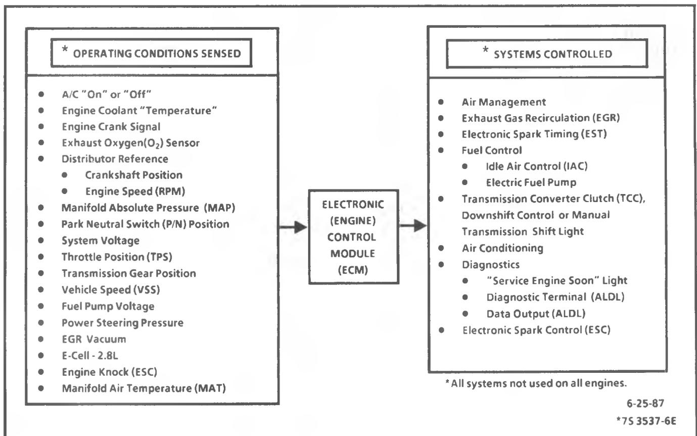
Figure 3-1 Computer Command Control System
