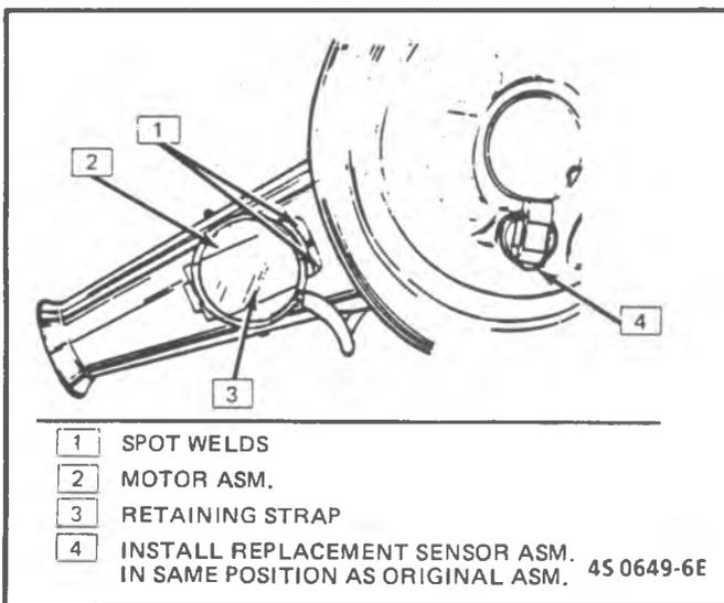
Figure 12-5 - Replacing THERMAC Vacuum Motor
