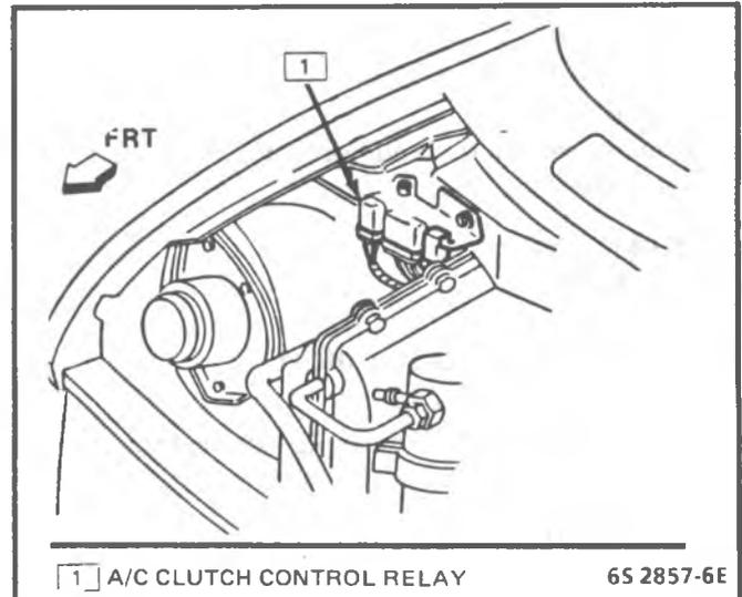
Figure 3-68 - A/C Clutch Control Relay - (M)
