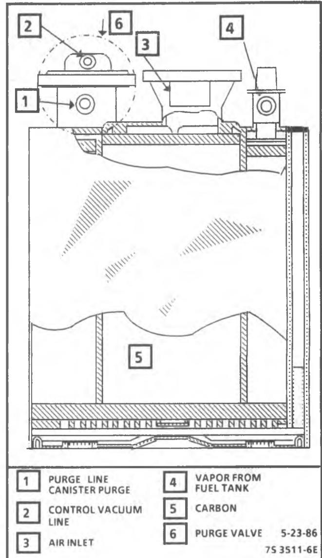
Figure 5-3 - Vapor Canister - 4.3L & V8 - Altitude
