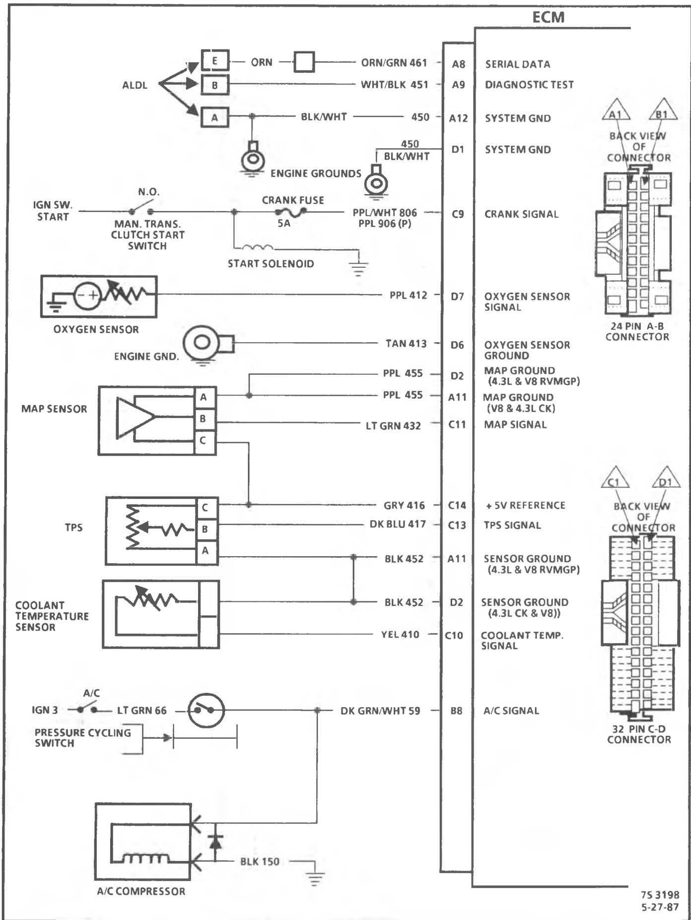
Figure 3-29 - ECM Wiring Diagram - 4.3L & V8 (1 of 4)
