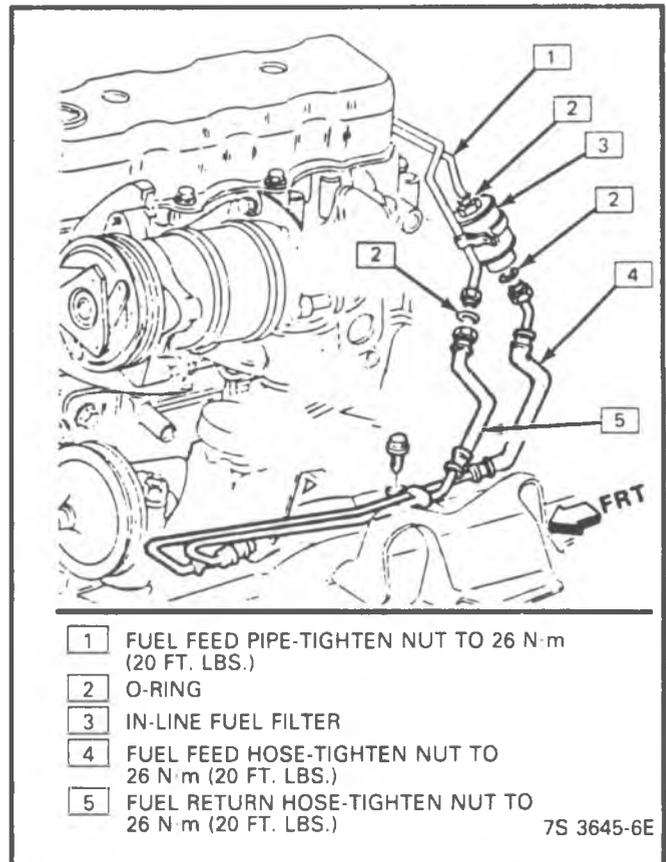
1 FUEL FEED PIPE-TIGHTEN NUT TO 26 N·m (20 FT. LBS.)
