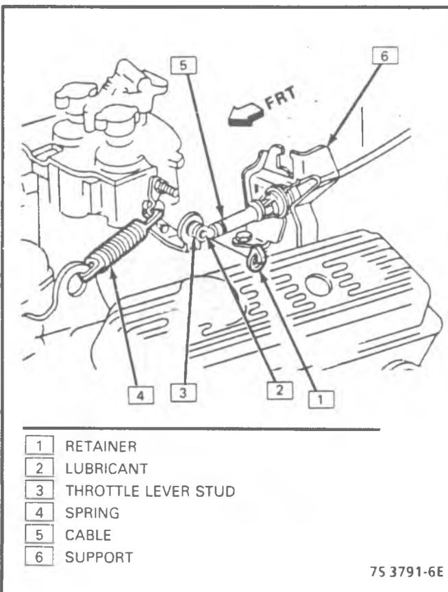
Figure 4-84 - Control Cable - 4.3L & V-8
