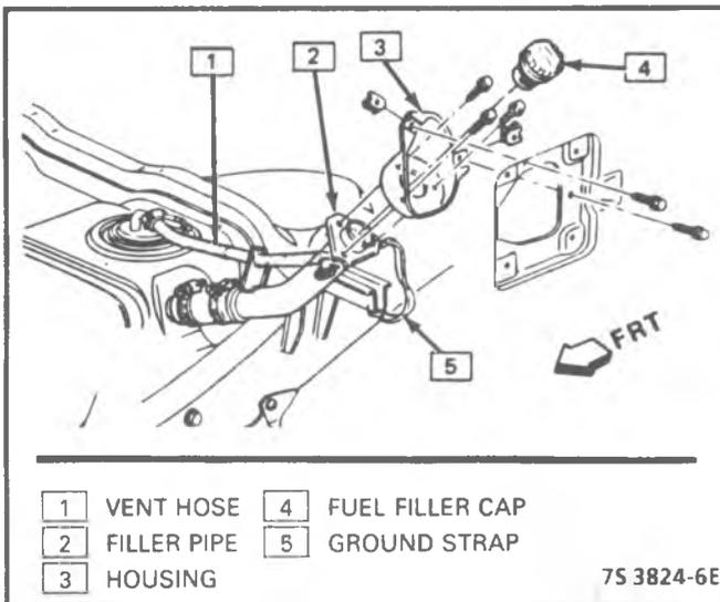
Figure 4-67 - Filler Neck - ST Pickup
