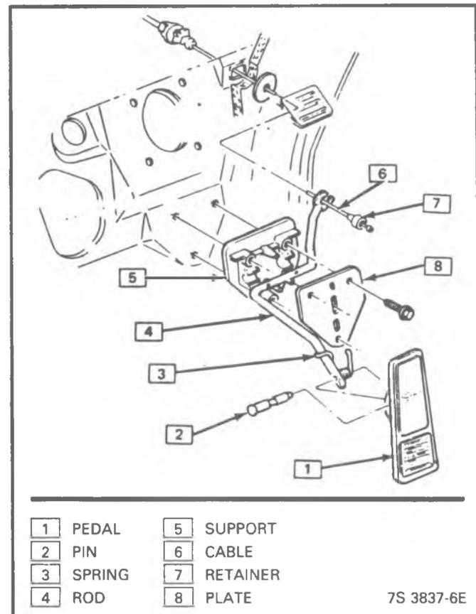
Figure 4-88 - Accelerator Pedal - RV
