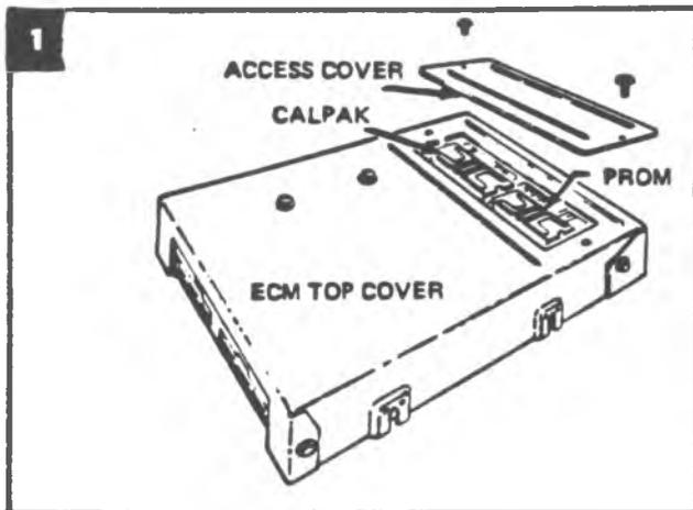
2. Remove PROM using the rocker-type PROM removal tool shown. Engage one end of the PROM carrier with the hook end of the tool. Press on the vertical bar end of the tool and rock the engaged end of the PROM carrier up as far as possible. Engage the opposite end of the PROM carrier in the same manner and rock this end up as far as possible. Repeat this process until the PROM carrier and PROM are free of the PROM socket. The PROM carrier with PROM in it should lift off of the PROM socket easily.
