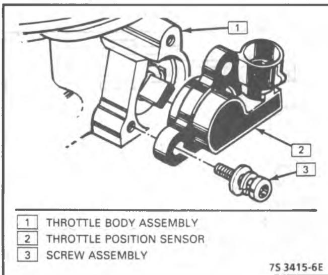
Figure 3-10 Throttle Position Sensor - L4
