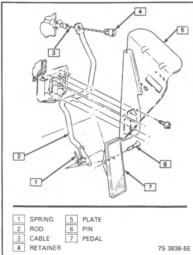
Figure 4-86 - Accelerator Pedal -ST
