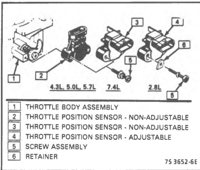
Figure 4-29 - TBI Model 220 TPS Configuration
