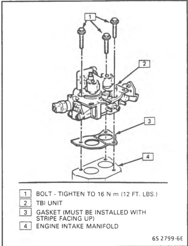
Figure 4-18 - Replacing TBI 220 Unit - 4.3L Engine
