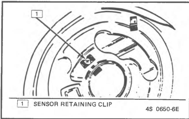
Figure 12-7 - Replacing THERMAC Sensor - S/T Series
