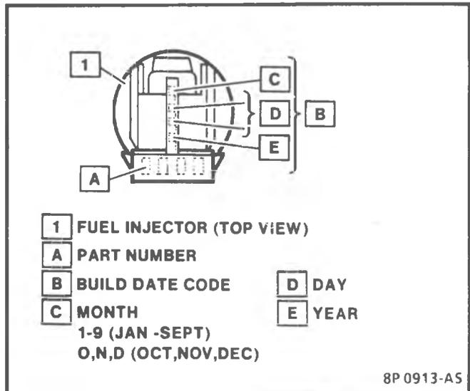
Figure 4-36 - Fuel Injector Part Number Location
