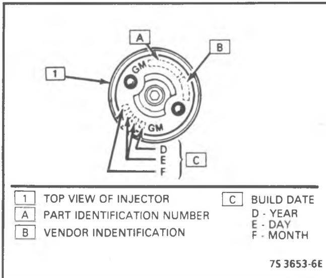
Figure 4-26 - Fuel Injector Port Number Location
