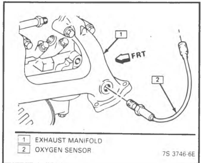
Figure 3-58 - Oxygen Sensor - 5.0L/5.7L (CK)
