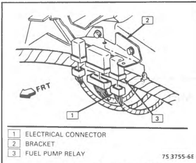
Figure 4-46 - Fuel Pump Relay (M)
