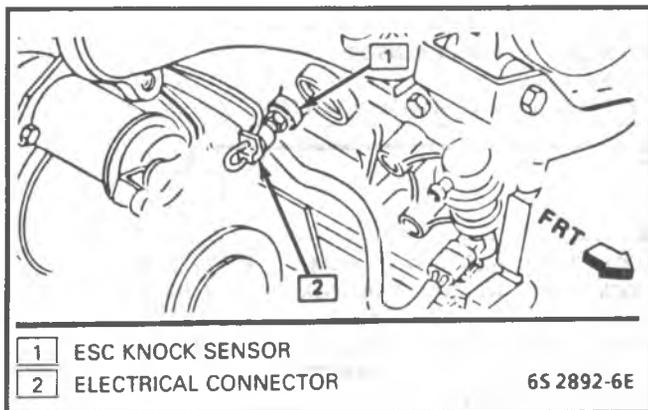
Figure 7-3 - ESC Knock Sensor - 2.8L, 5.0L, 5.7L
