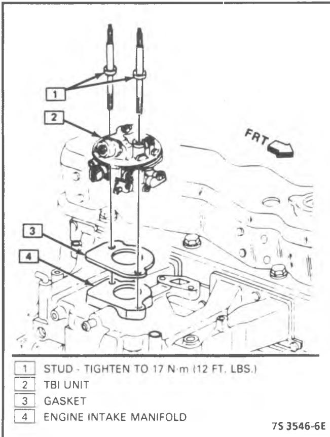
Figure 4-16 - Replacing TBI 700 Unit - 2.5L Engine
