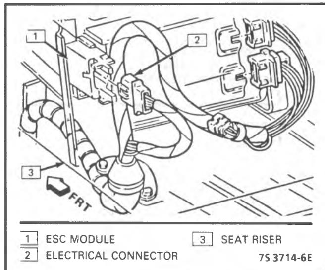
Figure 7-6 - ESC Module - G Series
