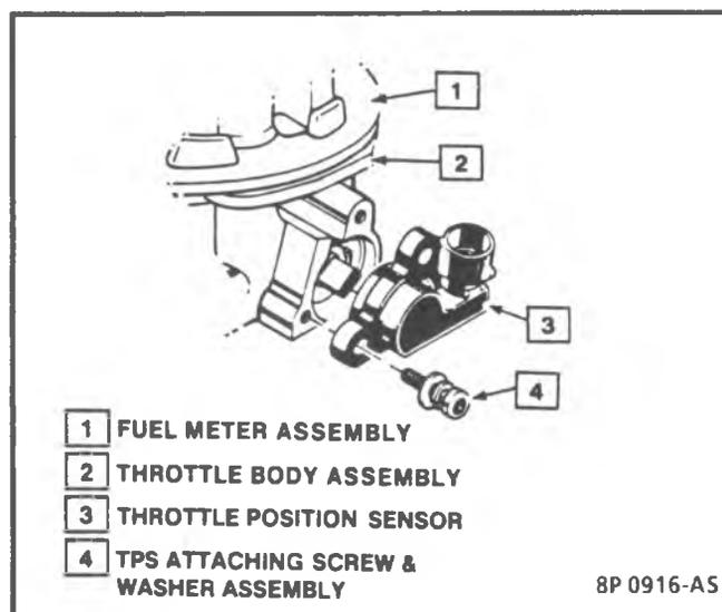
Figure 4-39 - Throttle Position Sensor (TPS) - TBI 700
