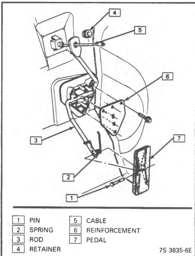
Figure 4-90 - Accelerator Pedal - G
