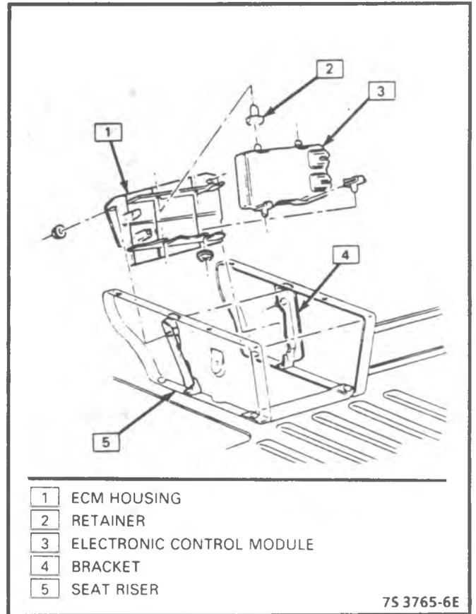
Figure 3-41 - Electronic Control Module (G)
