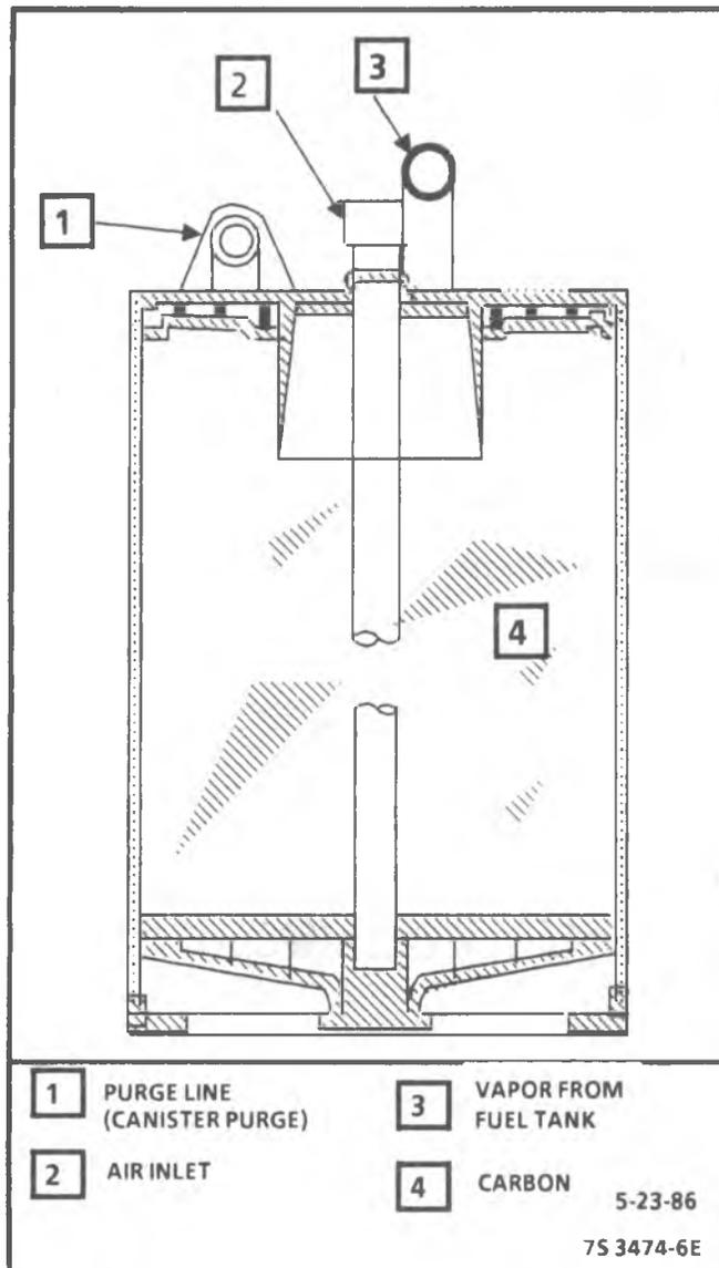
Figure 5-2 - Vapor Canister - 4.3L & V8 Except Altitude
