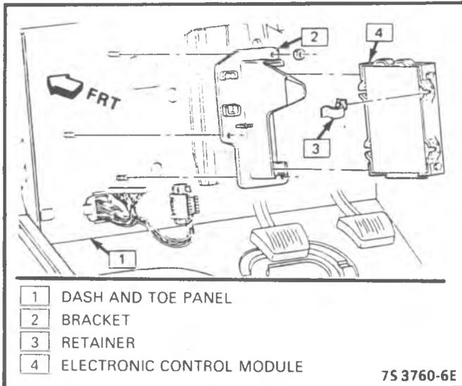
Figure 3-45 - Electronic Control Module (P)
