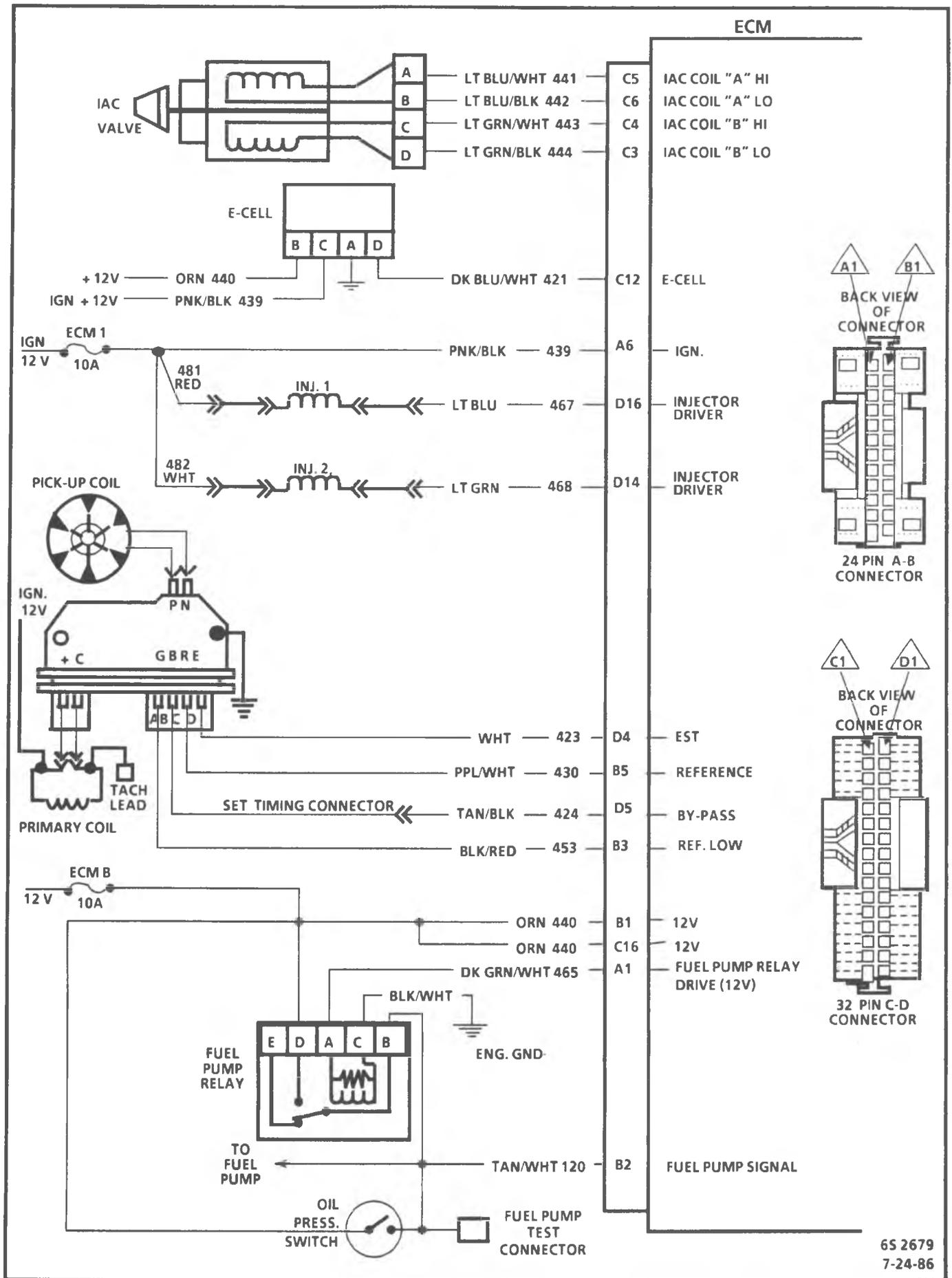
Figure 3-27 - ECM Wiring Diagram - 2.8L (2 of 3)
