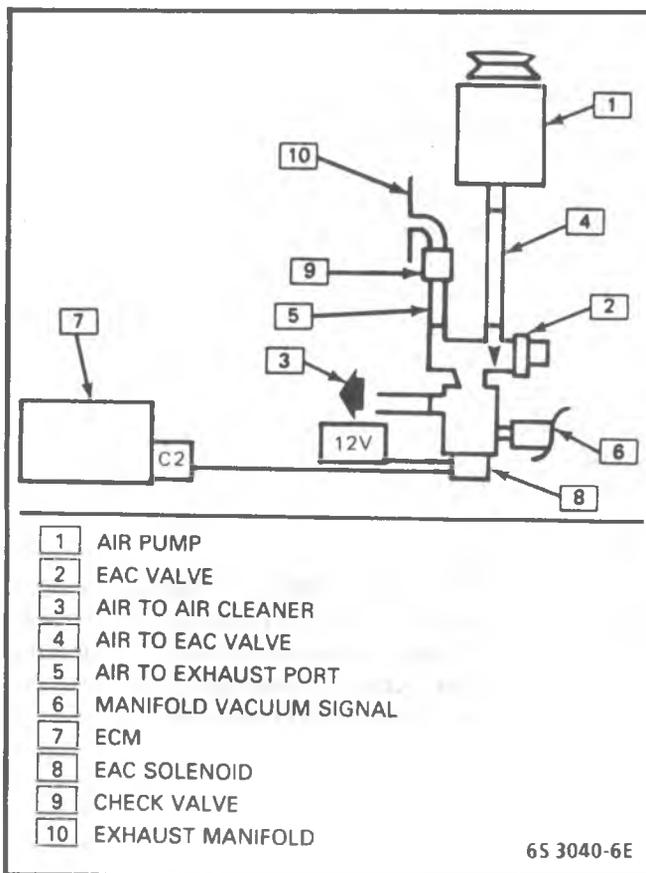
Figure 8-1 - AIR System - 2.8L
