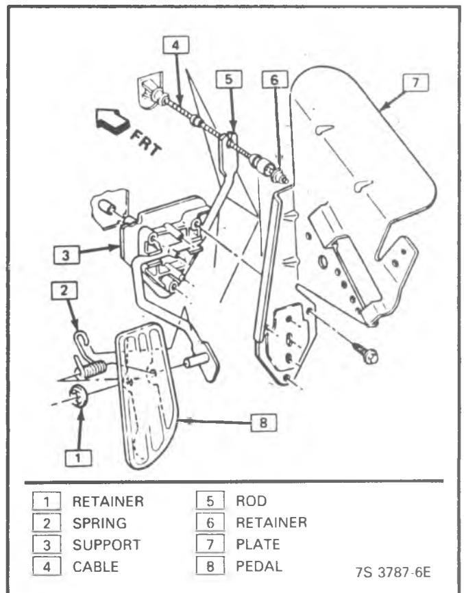
Figure 4-92 - Accelerator Pedal - P (32)
