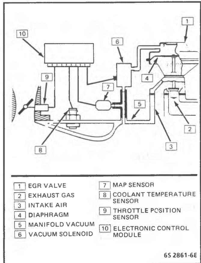
Figure 9-3 - EGR System - with Solenoid
