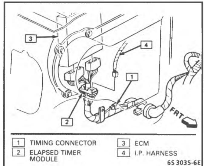
Figure 6-4 - Timing Connector (2.8L)
