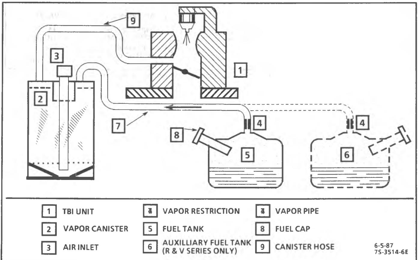
Figure 5-7 Evaporative Emissions Control System Schematic - 4.3L & V8 - Except Altitude
