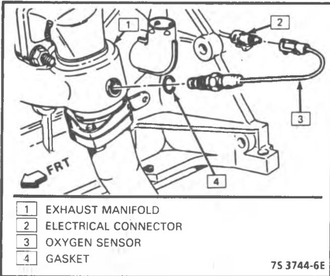
Figure 3-55 - Oxygen Sensor - 2.5L (M)
