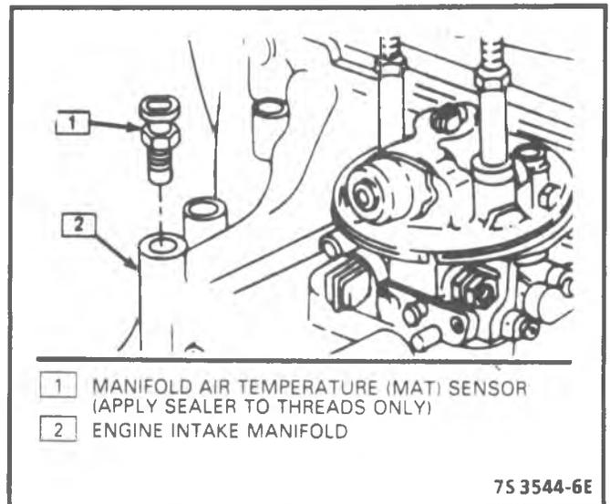
1 MANIFOLD AIR TEMPERATURE (MAT) SENSOR (APPLY SEALER TO THREADS ONLY)
