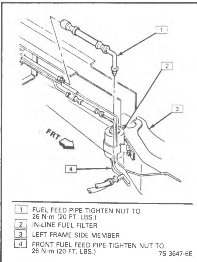
Figure 4-59 - Fuel Filter (M)
