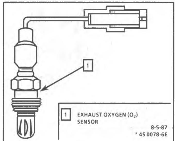
Figure 3-8 Oxygen Sensor
