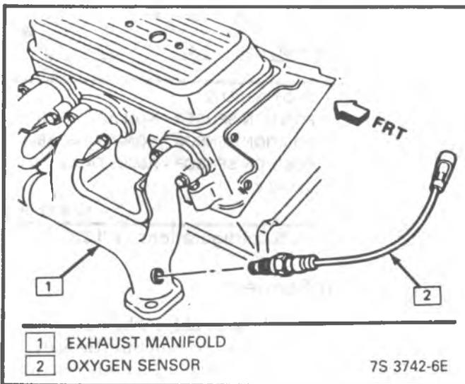
Figure 3-57 - Oxygen Sensor - 4.3L (STCKRVMG)
