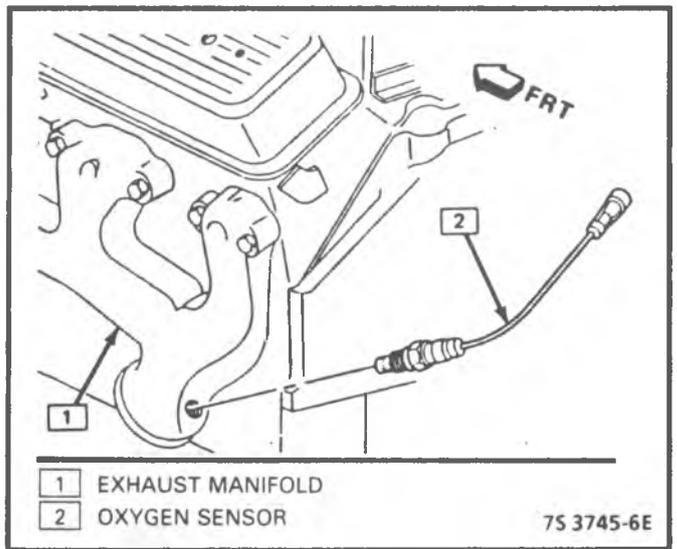
Figure 3-59 - Oxygen Sensor - 5.0L/5.7L (RVPG)
