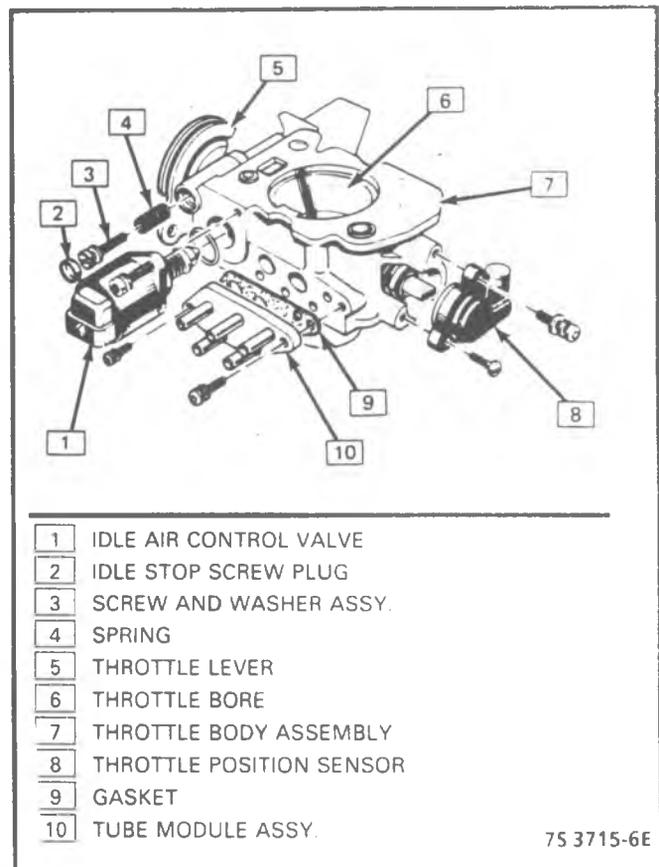
Figure 4-43 - Throttle Body Assembly
