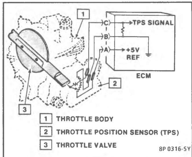
Figure 4-12 - Throttle Position Sensor (TBI 700)
