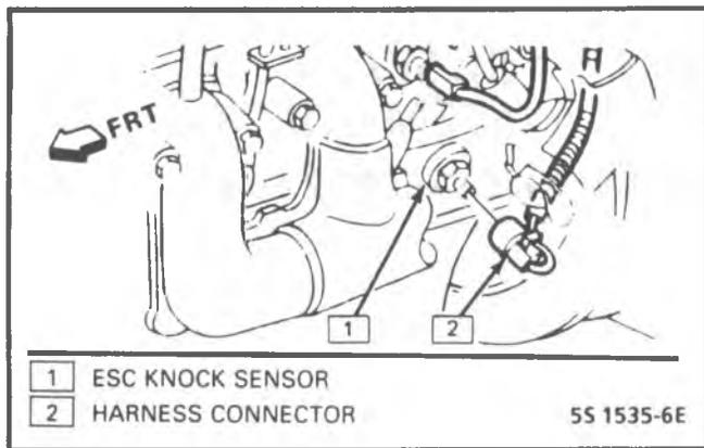
Figure 7-2 - ESC Knock Sensor - 4.3L
