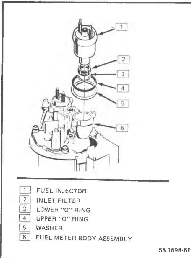
Figure 4-23 - Model TBI 220 Fuel Injector Parts
