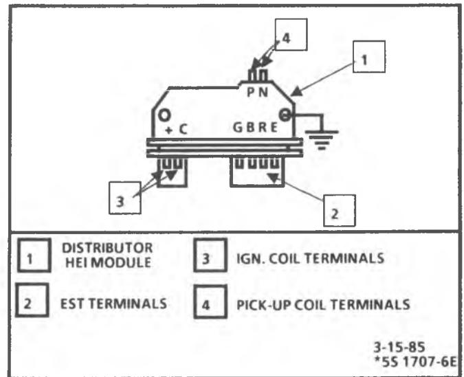
Figure 6-1 - Module (Except 2.5L S/T Truck)
