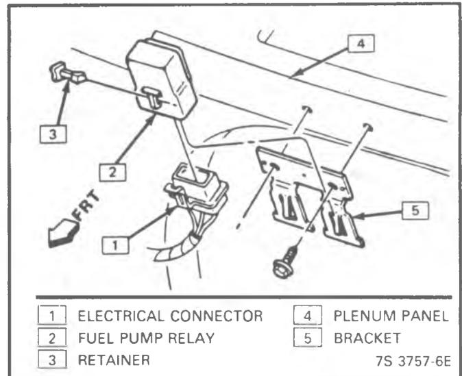
Figure 4-49 - Fuel Pump Relay (G)
