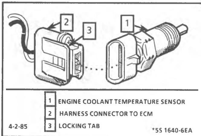
Figure 3-6 Coolant Temperature Sensor
