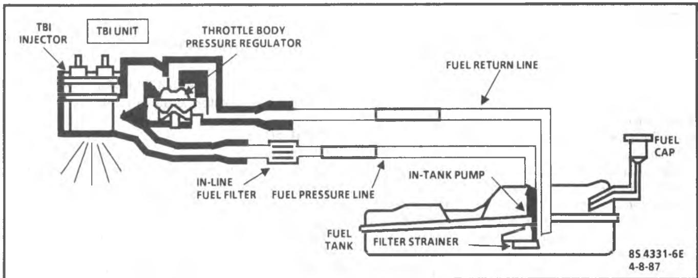
Figure 4-13 TBI Fuel Supply System (Typical)
