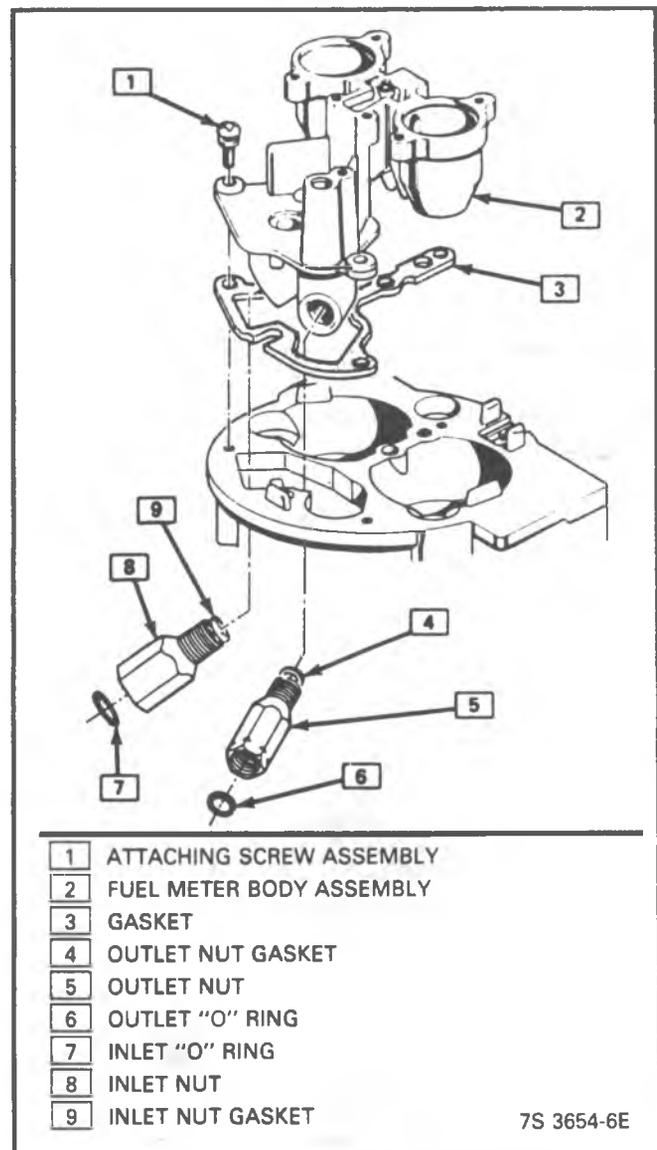
Figure 4-28 - Fuel Meter Body Assembly - TBI 220
