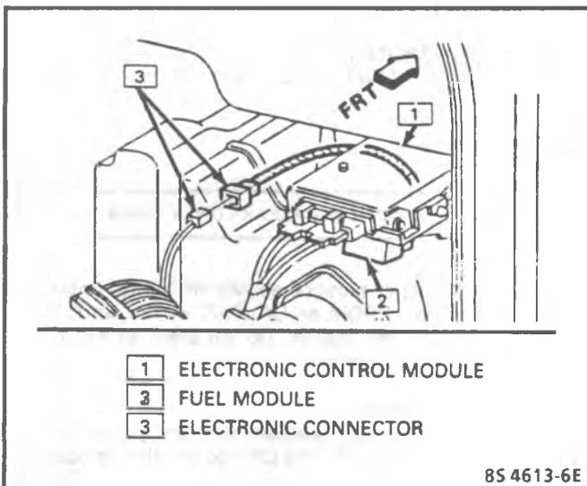
Figure 3-40 - Electronic Control Module (CK)
