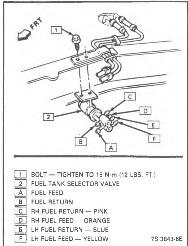
Figure 4-64 - Selector Valve - (RV)
