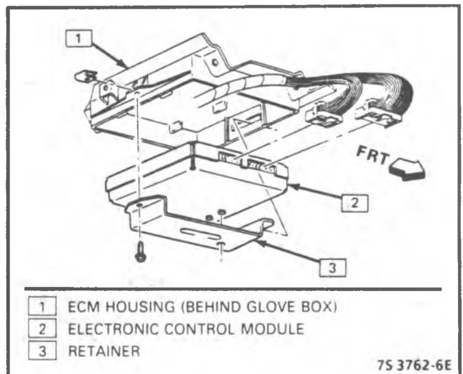
Figure 3-42 - Electronic Control Module (RV)
