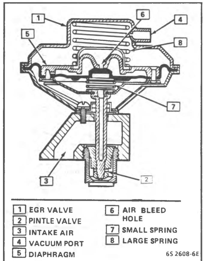
Figure 9-1 - Negative Backpressure EGR Valve 2.5L, 4.3L (except ST), 5.0L & 5.7L (under 8500 GVW) EVRV 2.8L, 4.3L (ST), 7.4L & 5.7L (over 8500 GVW)
