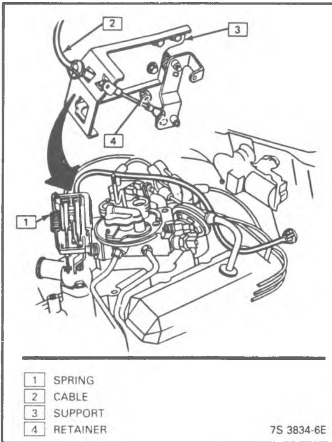
Figure 4-83 - Control Cable - 2.8L
