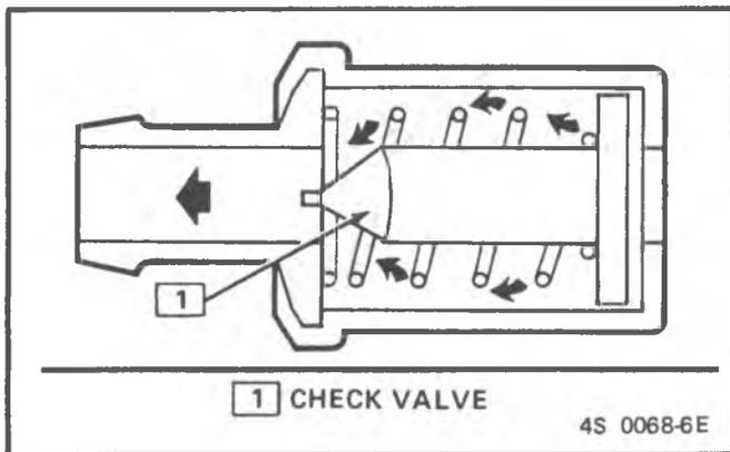
Figure 11-3 - PCV Valve Cross Section
