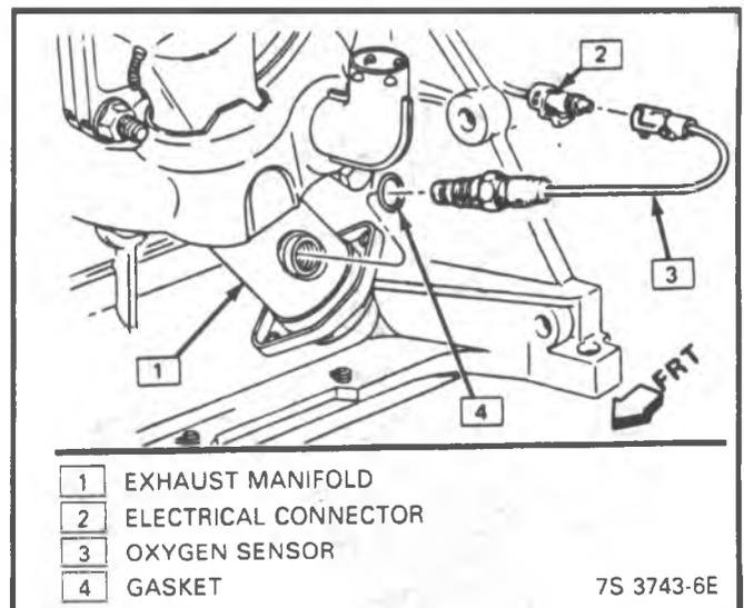
Figure 3-54 - Oxygen Sensor - 2.5L (ST)
