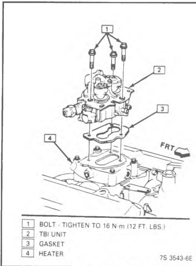
Figure 4-20 - Replacing TBI 220 Unit - 7.4L Engine
