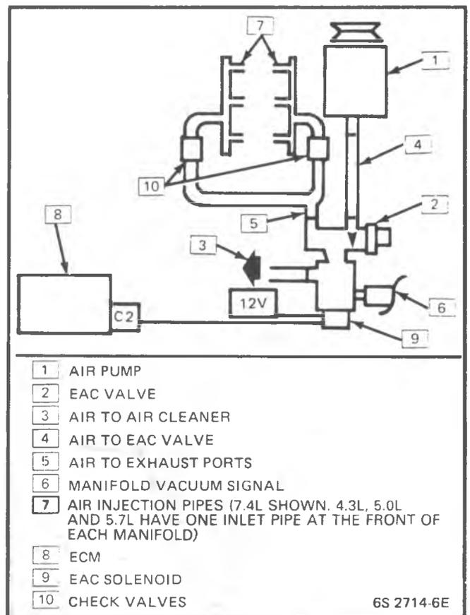
Figure 8-2 - AIR System - 4.3L & V8
