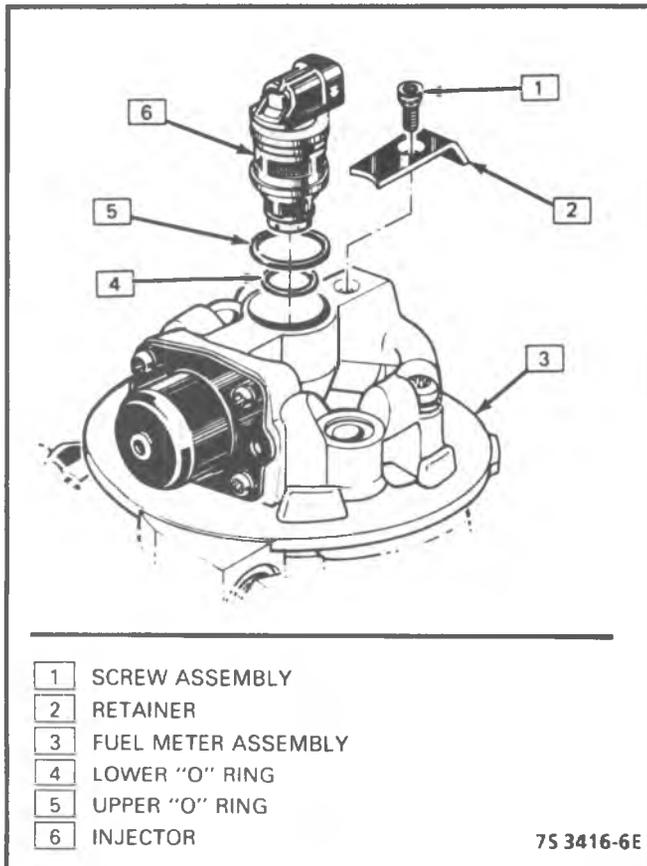
Figure 4-34 - Fuel Injection Parts (TBI 700)
