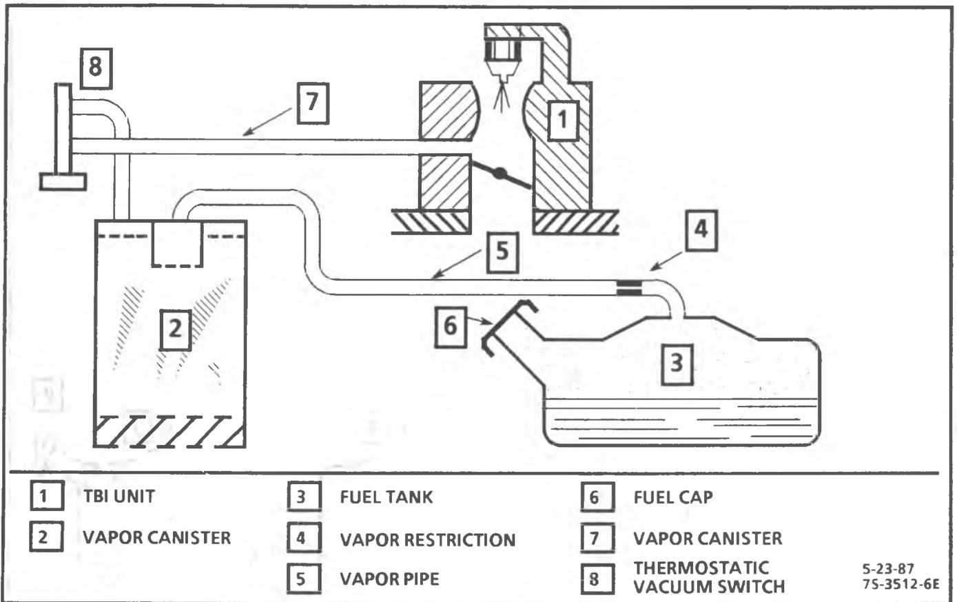
Figure 5-6 Evaporative Emissions Control System Schematic - 2.8L
