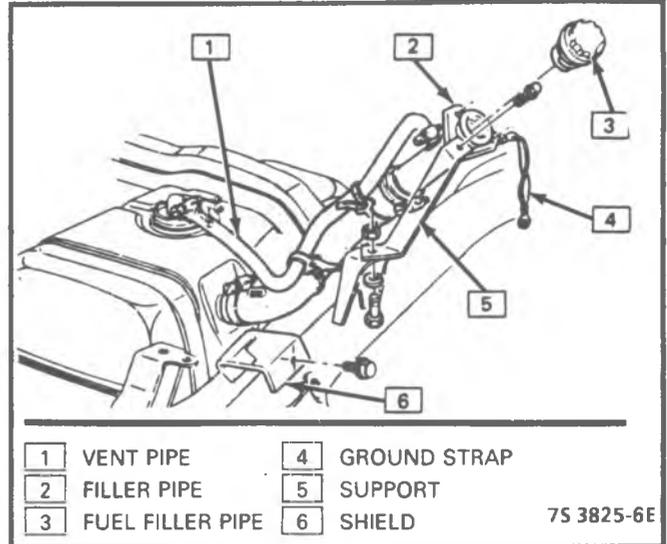
Figure 4-68 - Filler Neck - ST Chassis Cab
