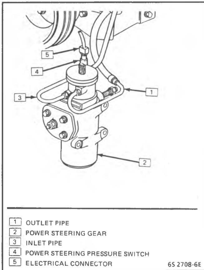
Figure 3-66 - Power Steering Pressure Switch
