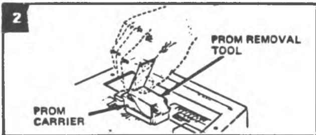
3. Inspect reference end of the PROM carrier and carefully set aside. Do not remove PROM from the carrier to confirm PROM correctness. Notch in PROM referenced to smaller notch in carrier and the ①.
