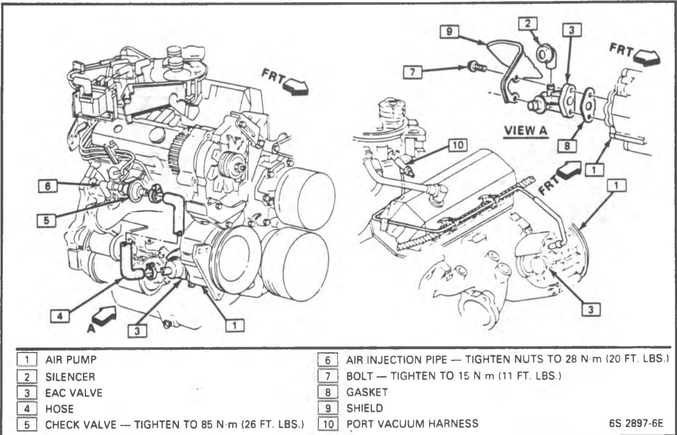
Figure 8-7 - Air System - 2.8L
