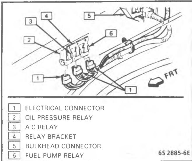
Figure 4-45 - Fuel Pump Relay (ST)
