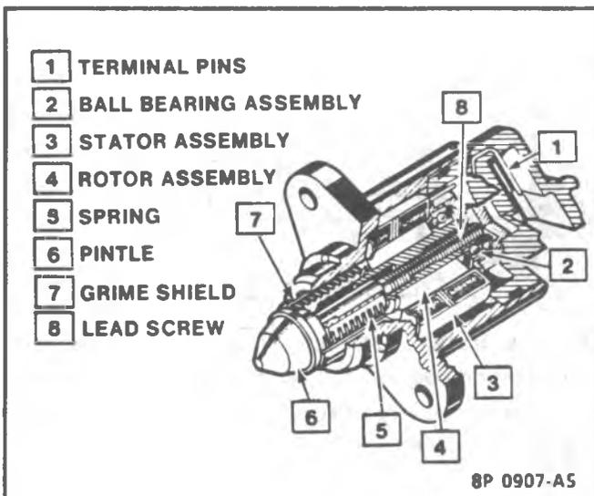
Figure 4-10 - Idle Air Control (IAC) Valve (TBI 700)
