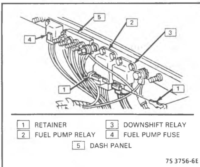
Figure 4-47 - Fuel Pump Relay (CK)
