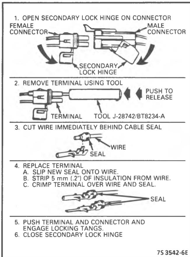
Figure 3-22 - Weather-Pack Terminal Repair
