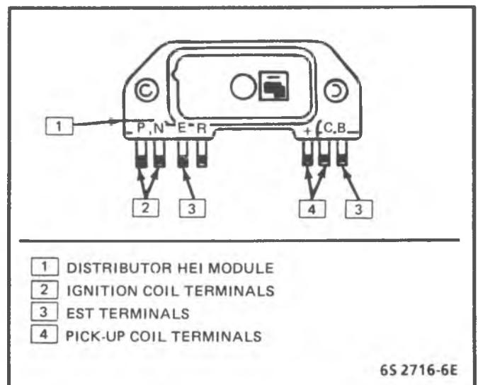
Figure 6-2 - Module (2.5L S/T Truck)
