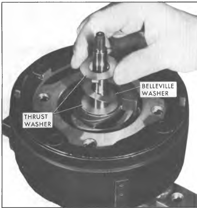
Fig. 88--Replacing Thrust and Belleville Washers
