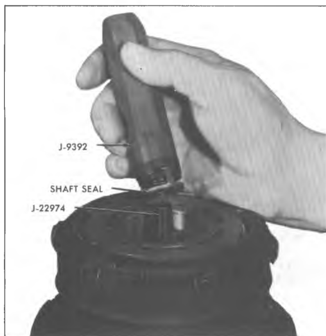
Fig. 75--Removing Shaft Seal
