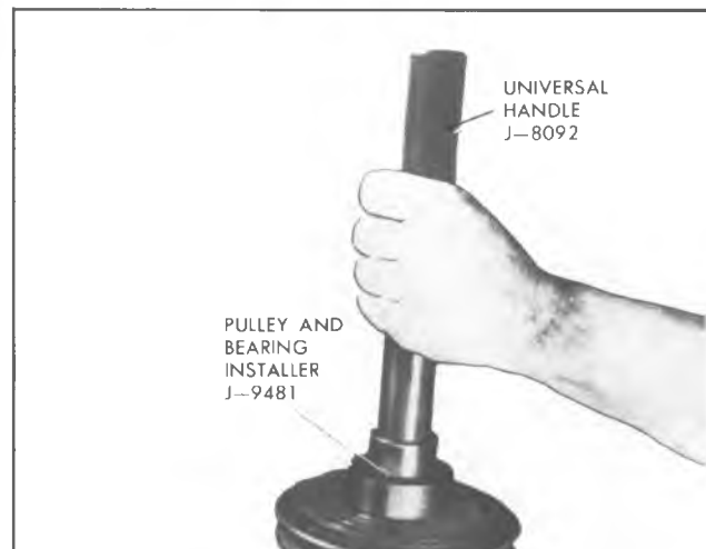
Fig. 12--Installing Pulley and Bearing Assembly
