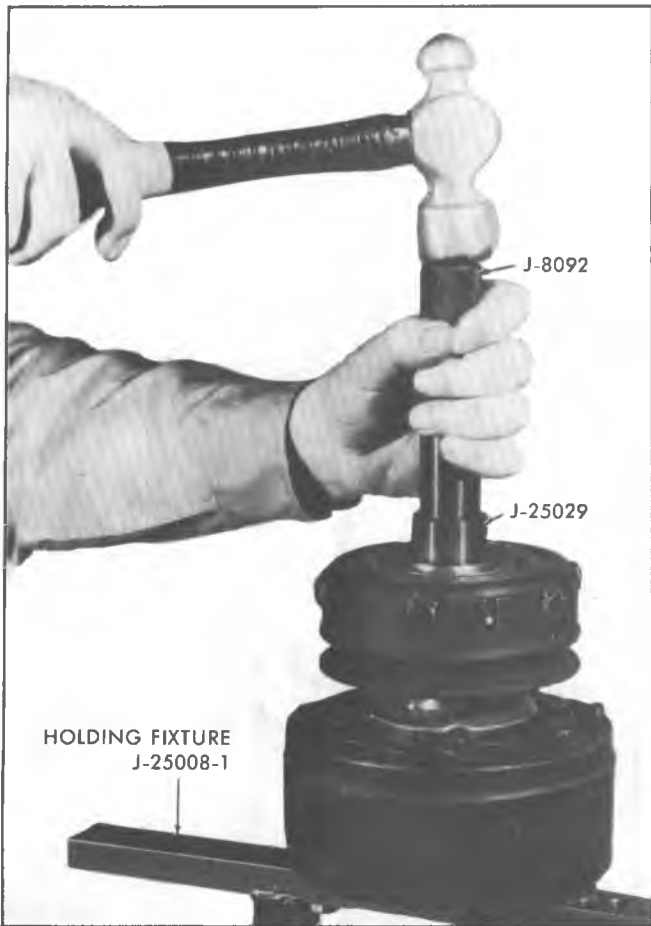
Fig. 85--Alternate Installation of R-4 Rotor and Bearing Assembly
