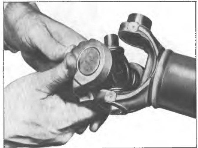
Fig. 8--Installing Trunnion into Yoke
