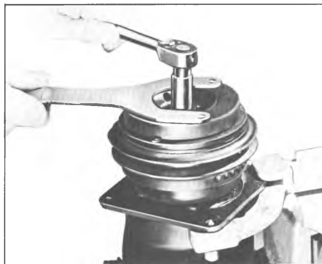
Fig. 3--Removing Shaft Lock Nut
