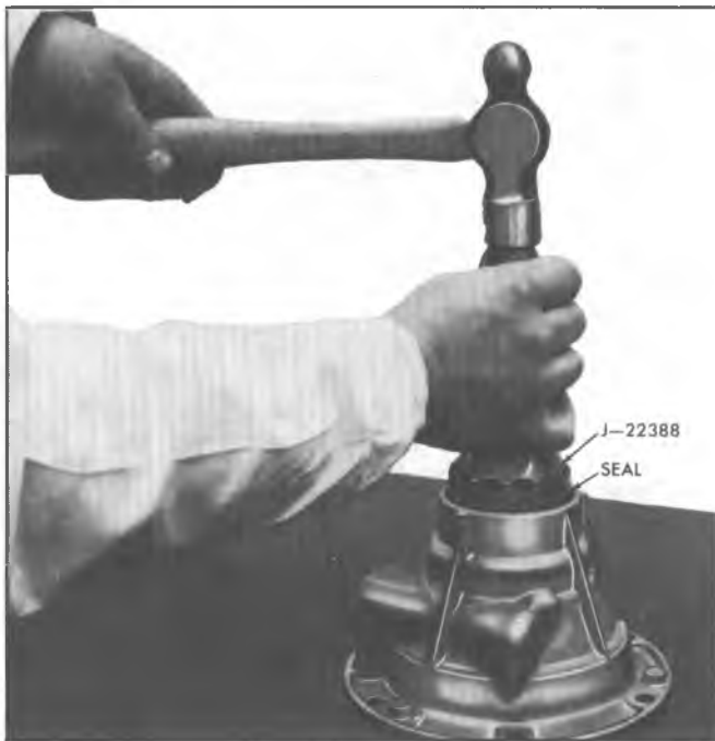
Fig. 7F—Installing Rear Output Housing Seal
