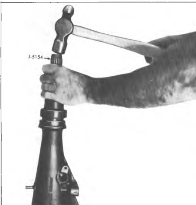
Fig. 16R--Installing Extension Housing Seal
