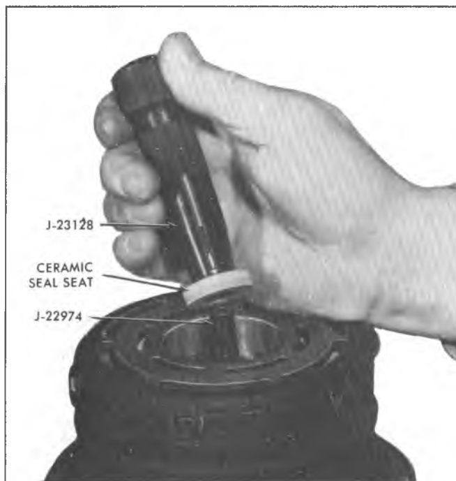
Fig. 74--Removing Seal Seat
