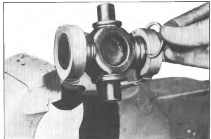
Fig. 9--Installing Snap Ring to Retain Trunnion
