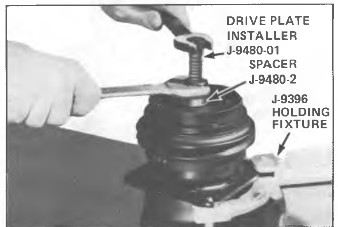
Fig. 8--Installing Drive Plate
