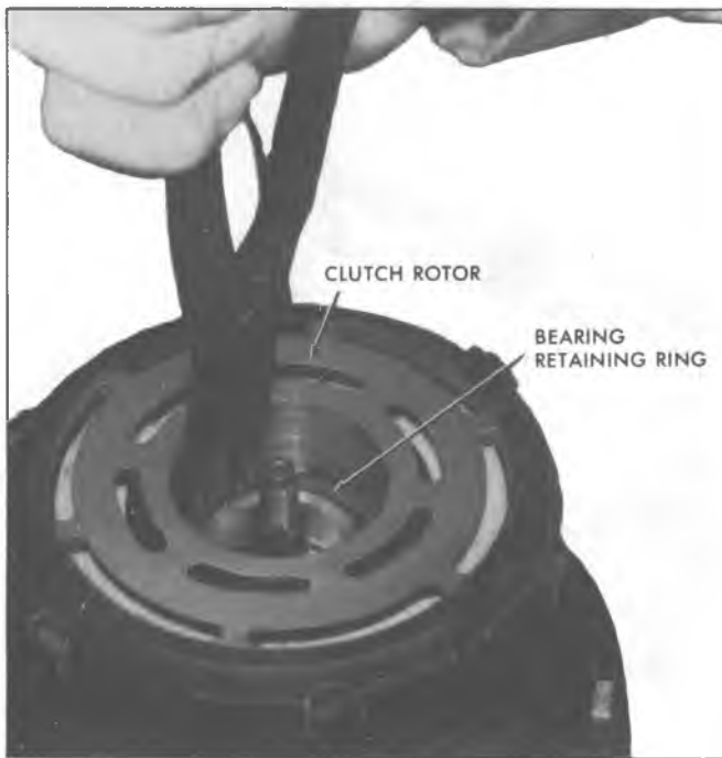
Fig. 77--Removing Bearing Retaining Ring
