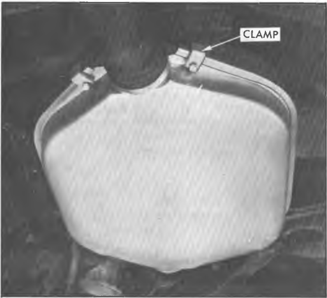
Fig. 16-Installing Bottom Cover Clamps
