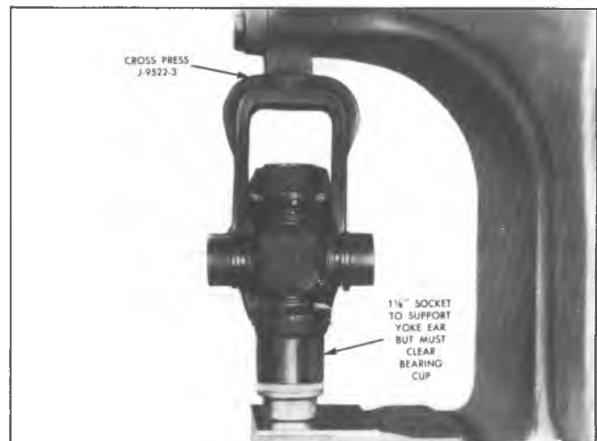
Fig. 5--Pressing Out Bearing Cup
