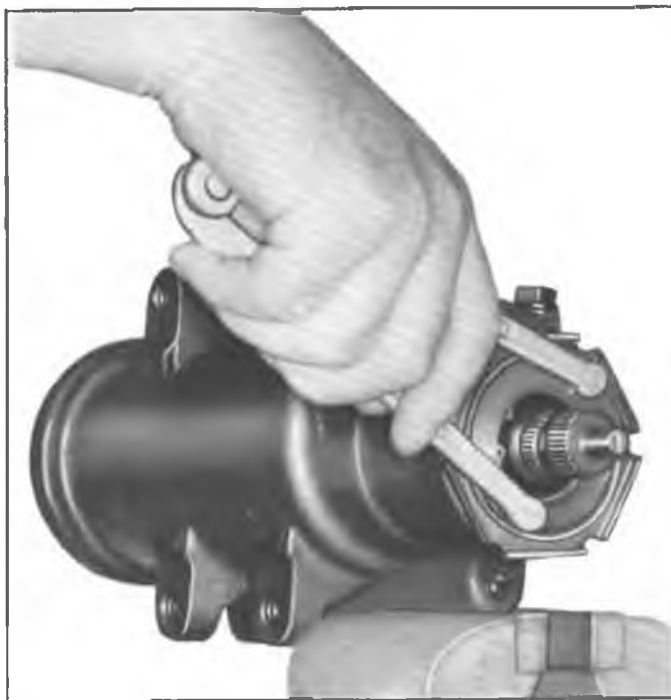
Fig. 36 - Removing Adjuster Plug
