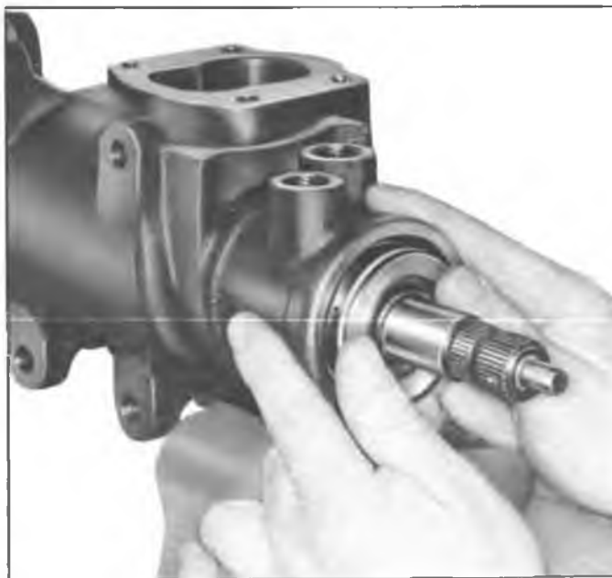
Fig. 55—Installing Valve Body
