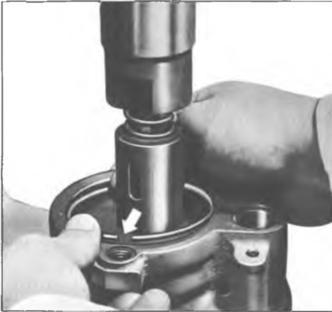
Fig. 29—Installing End Plate Retaining Ring
