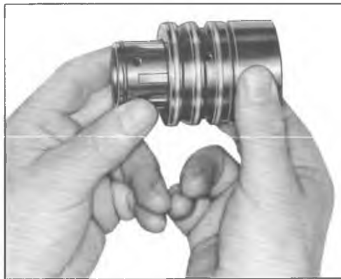
Fig. 44 - Removing Spool Valve
