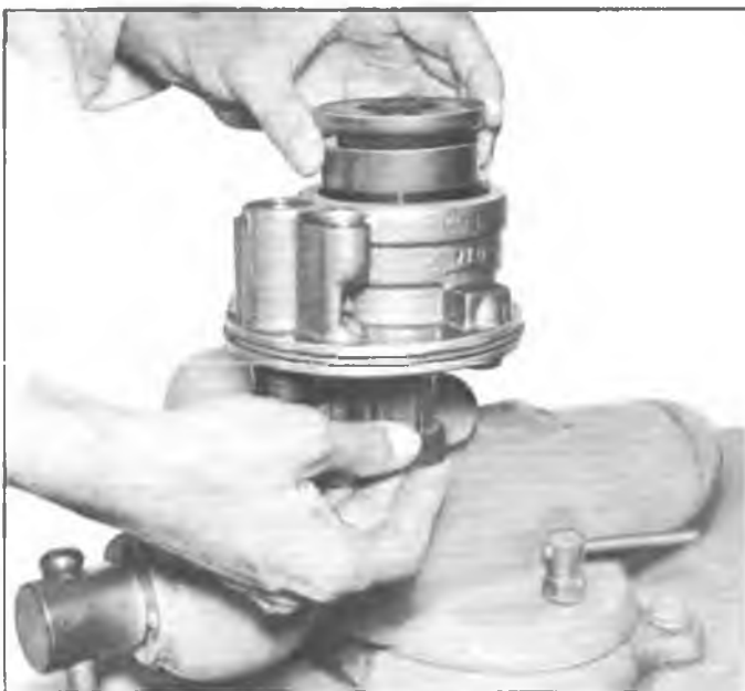
Fig. 19—Impeller Unit Removal
