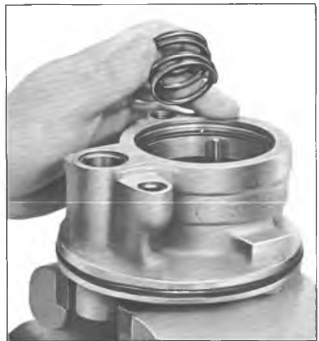
Fig. 28 - Installing Pressure Plate Spring
