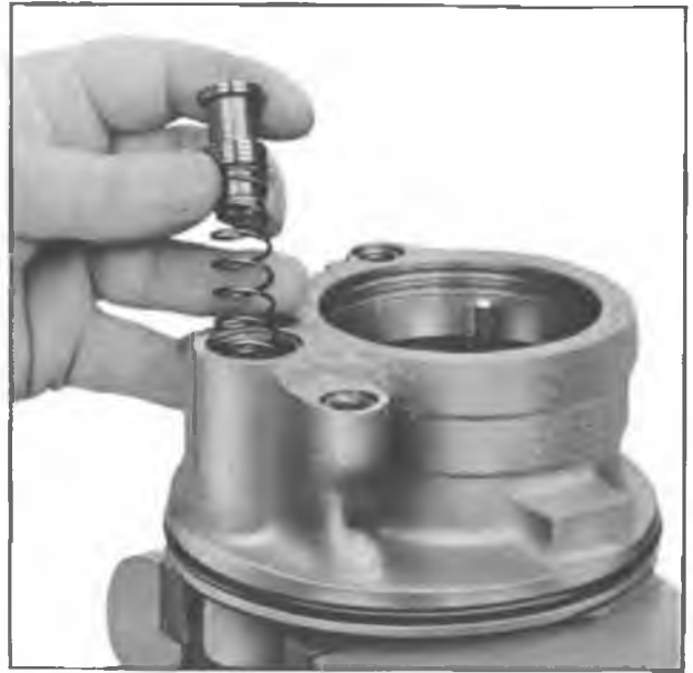
Fig. 30—Installing Flow Control Valve
