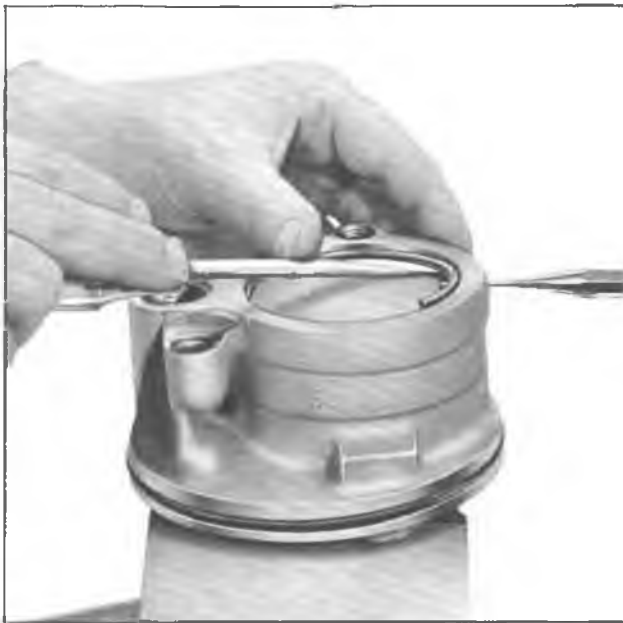
Fig. 18—Removing End Plate Ring
