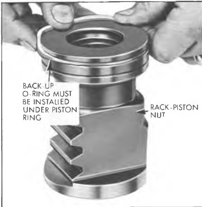
Fig. 58—Installing Ring on Rack-Piston
