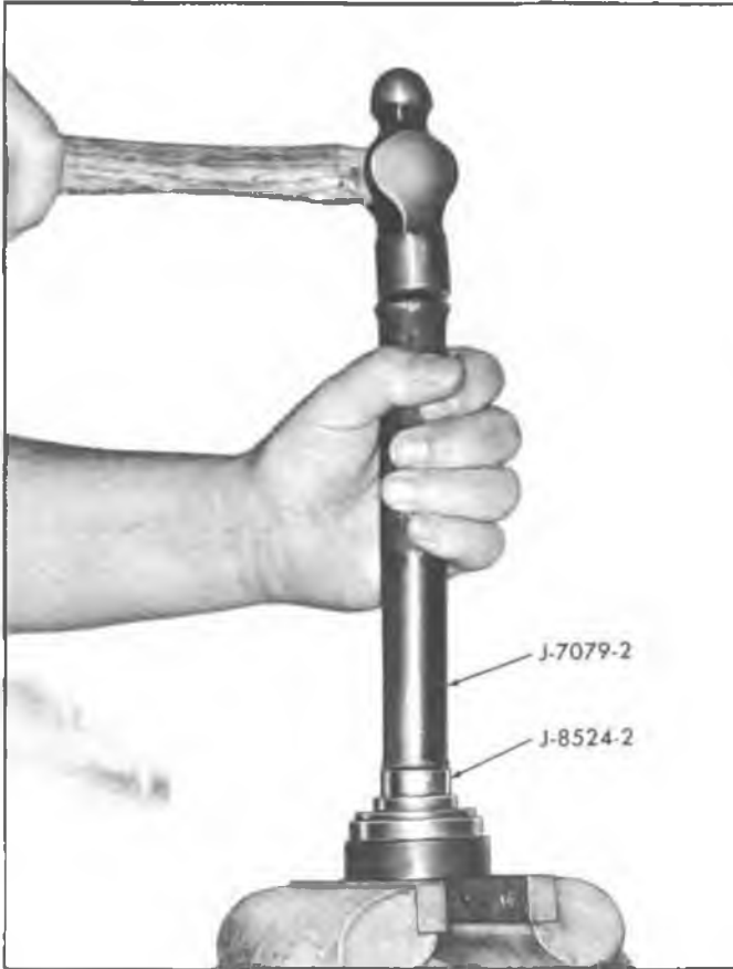
Fig. 39—Removing Bearing and Seal
