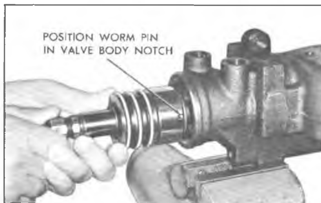
Fig. 53 – Valve to Worm Alignment
