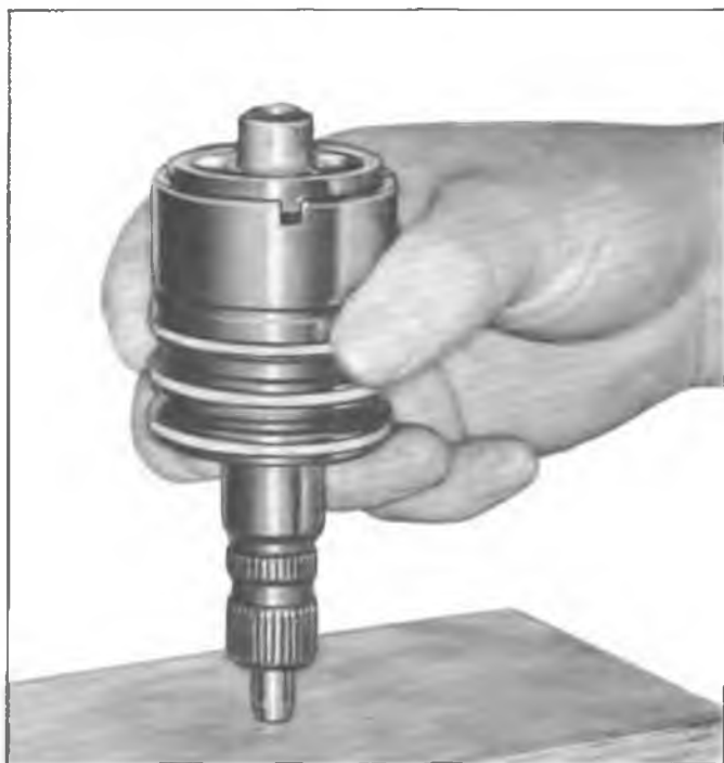
Fig. 43 - Removing Stub Shaft
