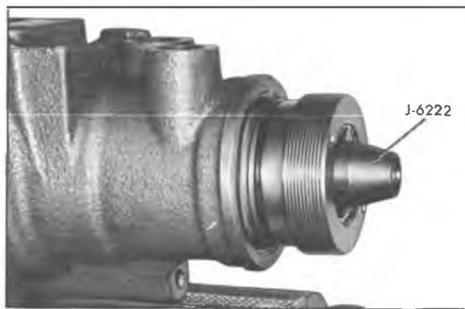
Fig. 57—Installing Adjuster Plug
