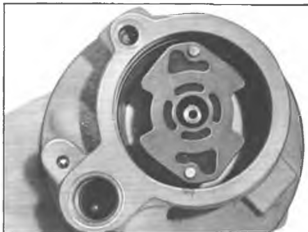
Fig. 23 – Installing Thrust Plate
