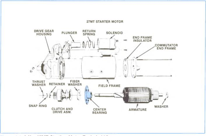
Figure 6-1, 6.2L - 27MT Starting Motor Exploded View.
