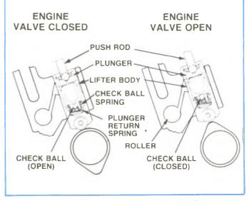
Figure 2-7, Roller Valve Lifter Operation.
