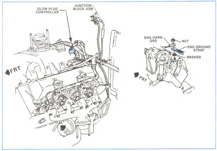
Figure 6-19, Glow Plug Controller Contamination.
