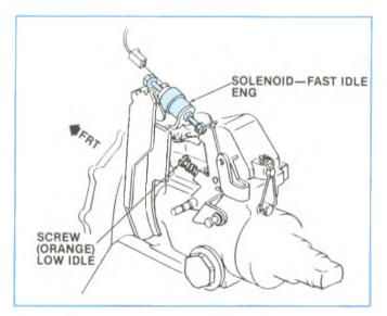
Figure 4-174, Idle Adjustment.
