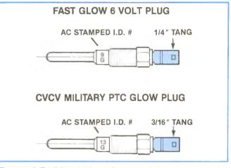
Figure 6-7, Glow Plug Comparison.
