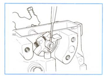
Figure 4-87, Removing Pin From Shaft.
