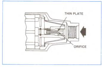
Figure 4-51, Viscosity Compensating Device.
