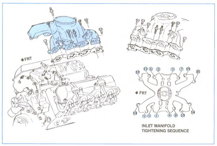
Figure 3-5, 6.2L Intake Manifold.
