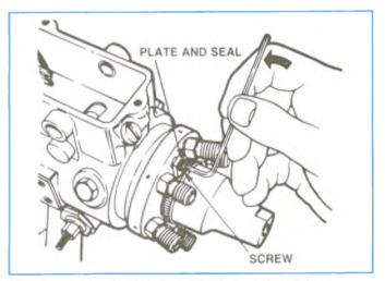
Figure 4-99, Removing End Cap Locking Screw.
