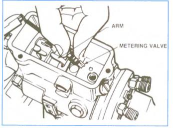
Figure 4-97, Removing Metering Valve.
