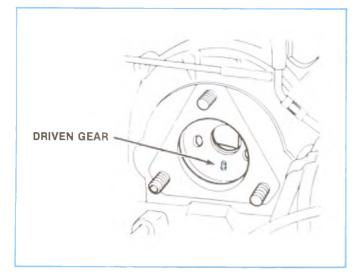
Figure 4-162, Slot of F.I. Pump Gear.
