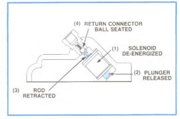
Figure 4-69, Solenoid De-Energized.
