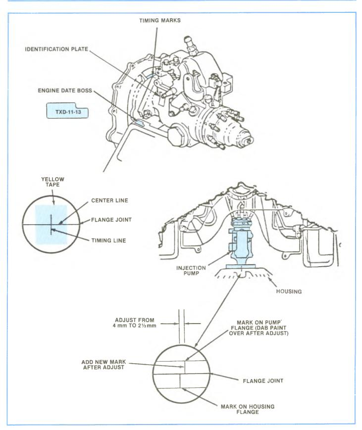
Figure 4-166, Timing Adjustment, Heavy Duty 6.2L Diesel Engine.
