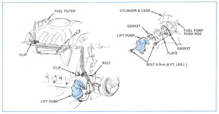
Figure 4-8, Mechanical Lift Pump Location.
