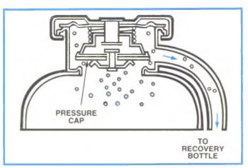
Figure 2-52, Radiator Cap With Pressure Valve Open.
