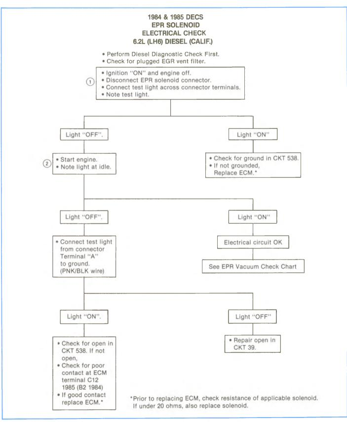
Figure 5-50, EPR Solenoid Electrical Check (1984 & 1985).
