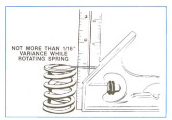
Figure 2-11, Checking Valve Spring.
