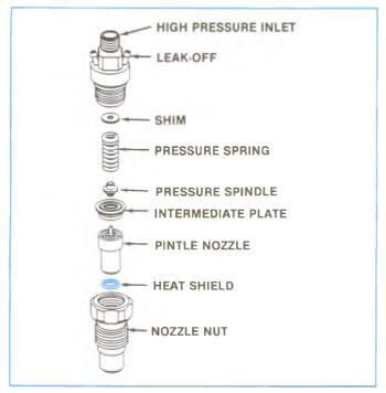
Figure 4-170, Nozzle Holder Assembly, Exploded View.
