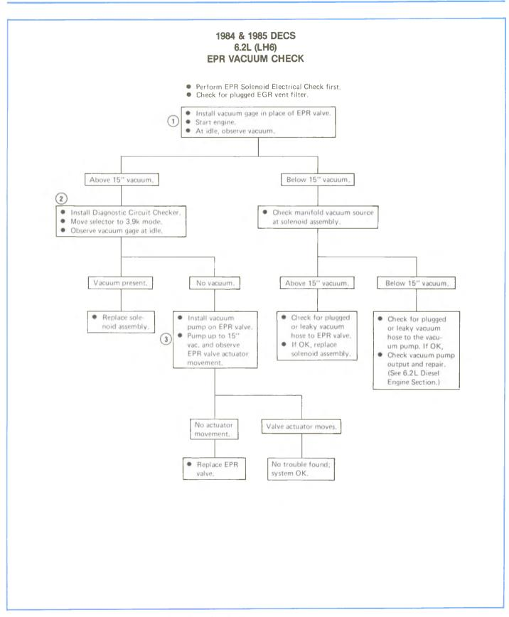
Figure 5-52, EPR Vacuum Check (1984 & 1985).
