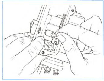
Figure 4-95, Disengaging Linkage Hook.
