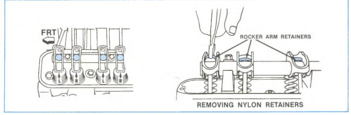
Figure 2-5, 1985 and Later Rocker Arm Assembly.
