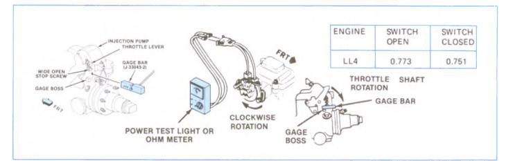
Figure 5-18, TPS Adjustment LL4-Model With 700-R4 (MD8) Transmission.
