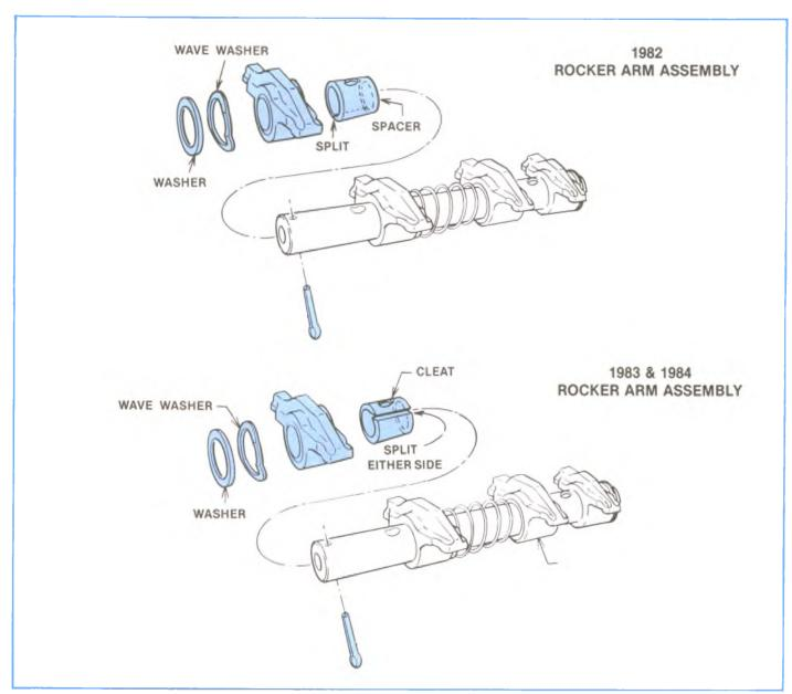
Figure 2-10, 1982-84 Rocker Shafts.
