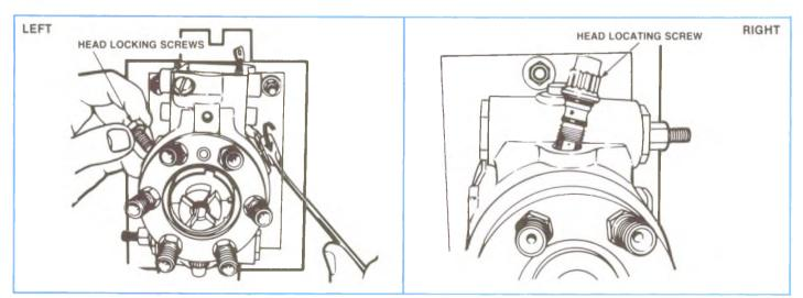
Figure 4-104, Removing Head Screws.
