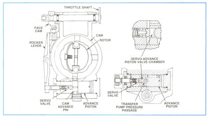
Figure 4-61, Mechanical Light Load Advance.
