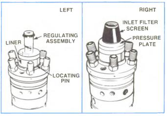
Figure 4-124, Installing Regulator and Pressure Plate/Screen.
