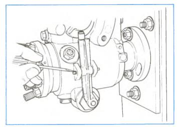
Figure 4-89, Removing Retaining Rings.
