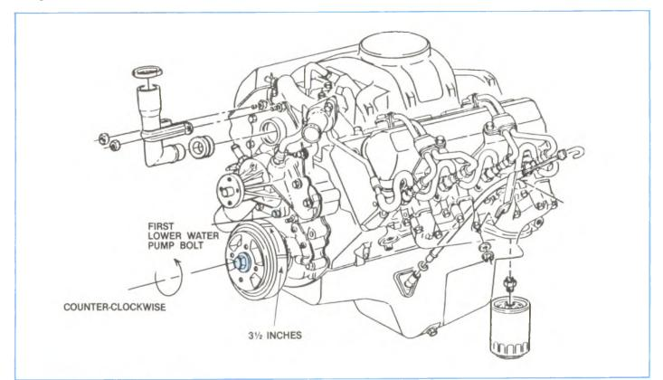
Figure 2-9, Balancer Position.
