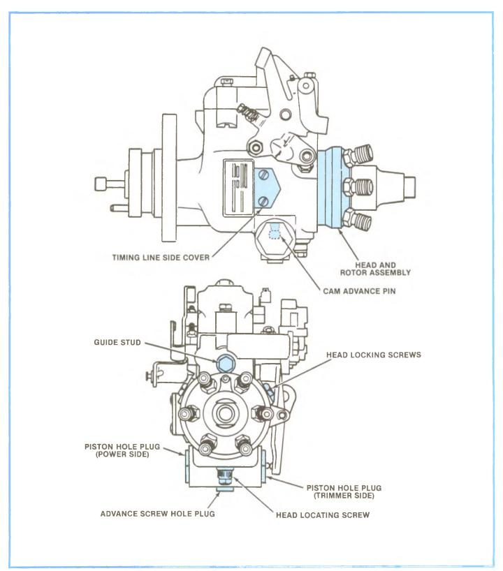
Figure 4-159, Injection Pump Components Location.
