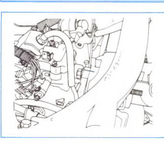
Figure 4-164, Aligned Timing Marks.
