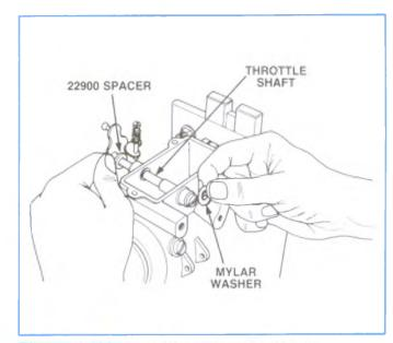
Figure 4-139, Installing Throttle Shaft and Clip.
