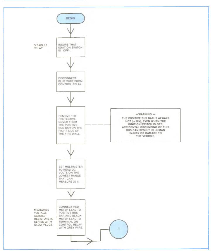
Figure 6-30, Troubleshoot Glow Plug Power Circuit, D-Truck.
