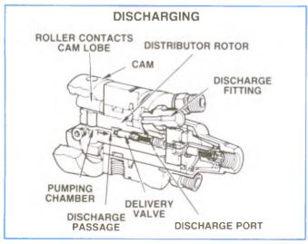
Figure 4-45, Delivery Valve Control.
