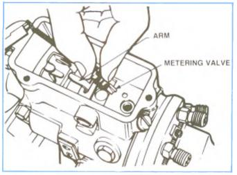
Figure 4-137, Lubricating Metering Valve.
