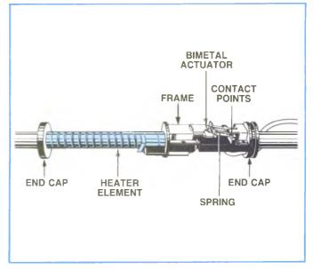
Figure 4-15, Diesel Fuel Heater Components.
