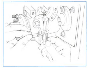
Figure 4-90, Removing Lever Assembly.
