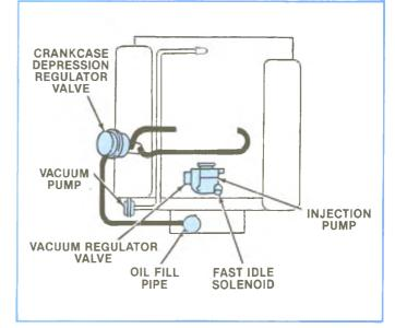
Figure 5-4, Emission System — LL4 Engine.
