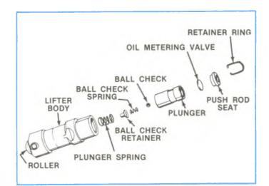
Figure 2-8, Valve Lifter Disassembled.
