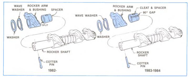
Figure 2-4, 1982-1984 Rocker Arm Assembly.
