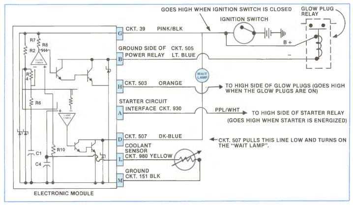
Figure 6-27, D-Truck Electronic Module Controller.
