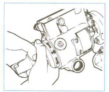
Figure 4-131, Installing Head.
