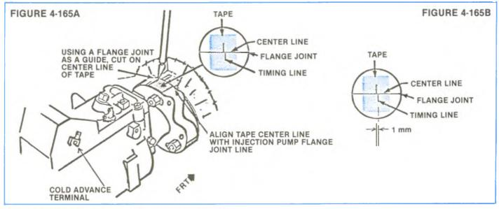
Figure 4-165A-B, Injection Pump Static Timing.
