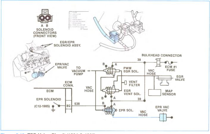
Figure 5-46, EPR Valve Circuit (1984 & 1985).
