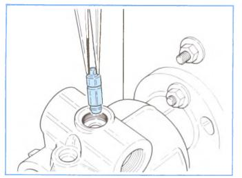
Then, insert the cam advance pin into its bore, making certain that it properly engages the cam ring. (Figure 4-145).
