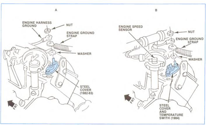
Figure 6-24 A and B, Installation of Temperature Inhibit Switch.
