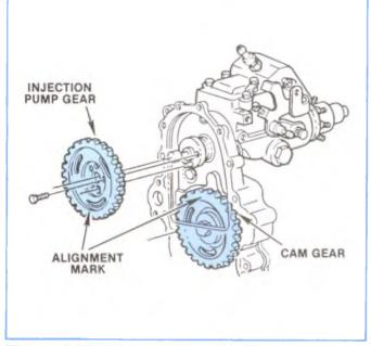
Figure 4-29, Pump Timing Gears.
