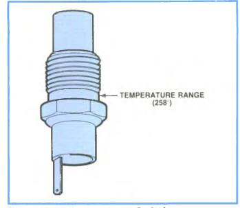
Figure 2-54, Temperature Switch.
