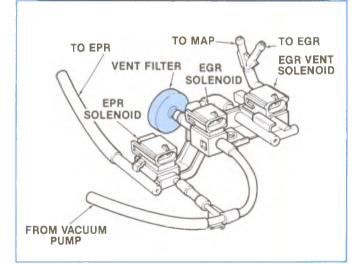
Figure 5-45, EGR, EPR, Vent Solenoid Assembly.
