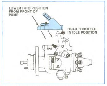
Figure 4-155, Installing Governor Cover.
