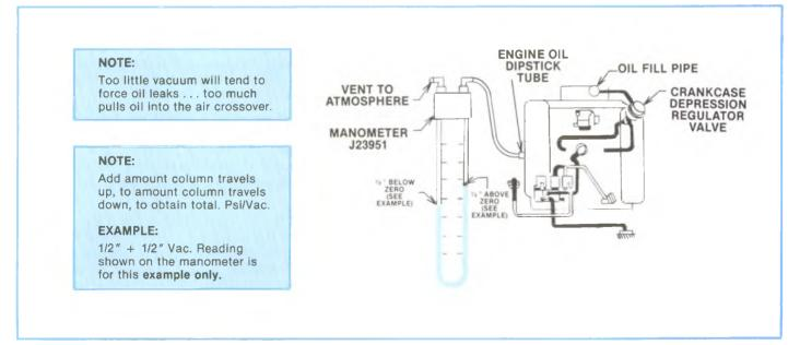
Figure 5-8, CDR Valve Test with Manometer.
