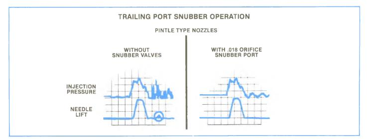
Figure 4-80, Trailing Port Snubber Graph.
