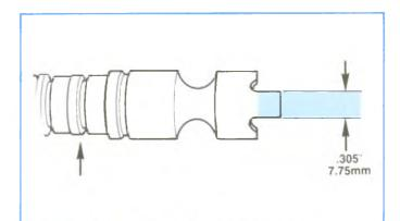
Figure 4-112, Drive Shaft Inspection.
