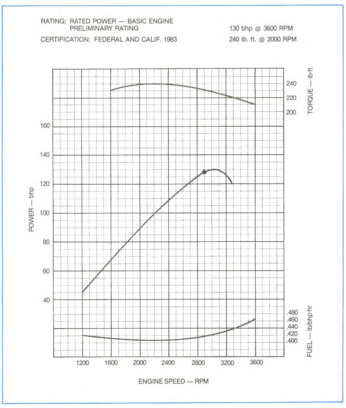
Figure 1-3, Engine Performance Curve, 6.2L — Light Duty (LH6).
