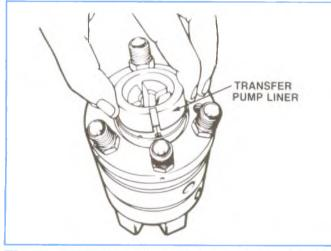
Figure 4-120, Installing Transfer Pump Liner.
