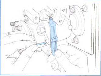
Figure 4-153, Installing Rocker Arm Pin.
