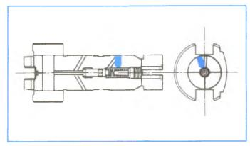
Figure 4-79, Trailing Port Snubber.
