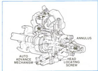
Figure 4-34, Fuel Flow To Hydraulic Head.
