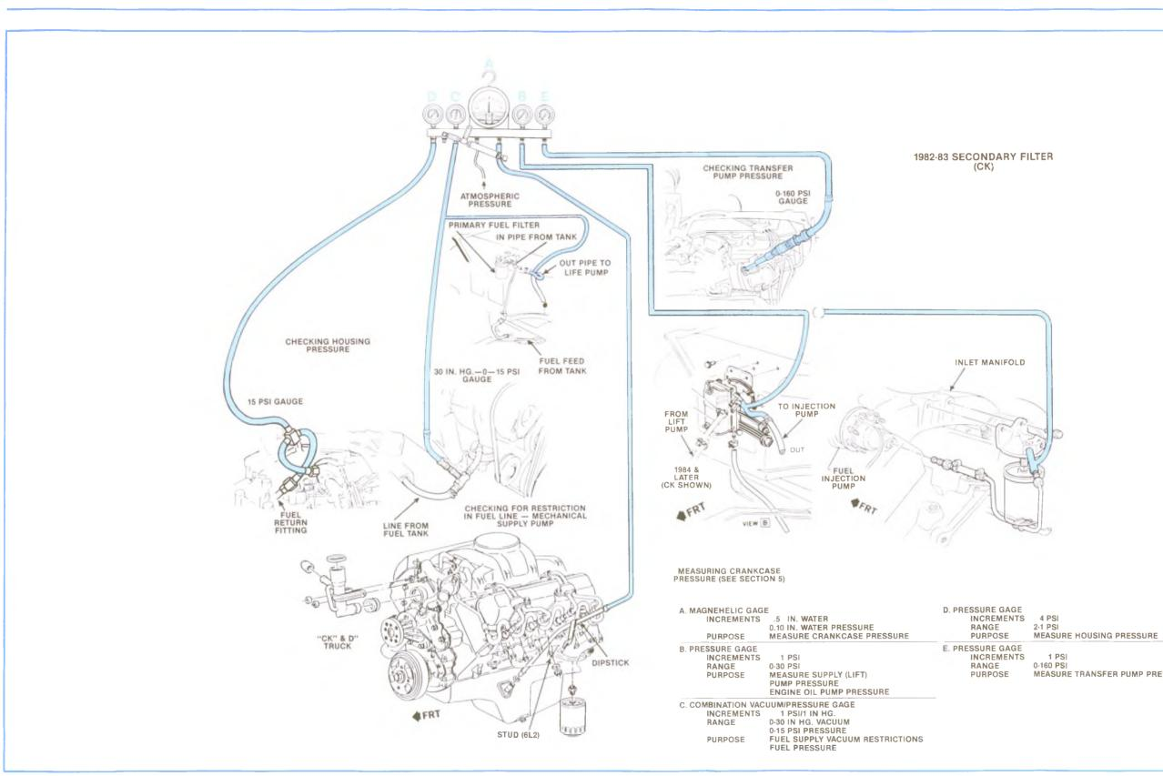
Figure 7-7, Gage Connections for Diagnosis Procedure.
