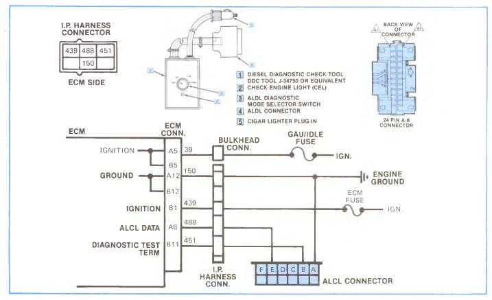
Figure 5-34, 1984 ECM Check Schematic.
