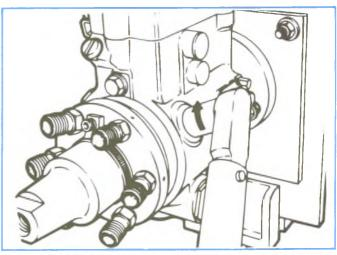
Figure 4-143, Torquing Head Locking Screws.
