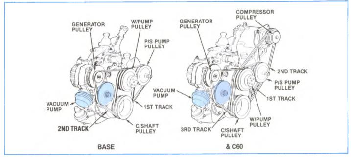
On applications with an engine mounted Model 80 fuel filter, a belt driven vacuum pump is used. This appears on 1984 and later units. See Figure 2-41.
