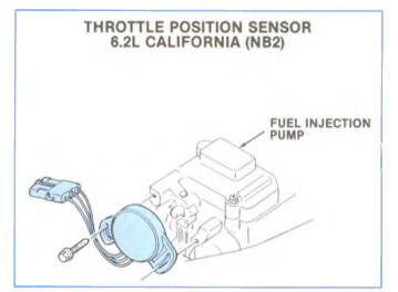
Figure 5-59, Throttle Position Sensor.
