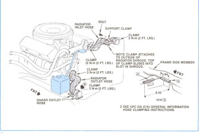
Figure 2-59, Pressure Coolant Recovery Tank (Bottle).
