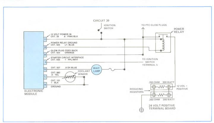
Figure 6-26, D-Truck Glow Plug System.
