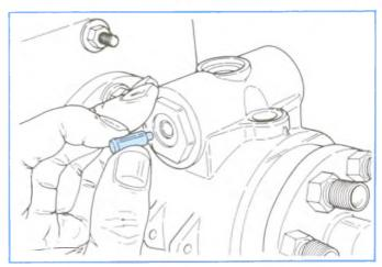
Figure 4-150, Installing Servo Advance Plunger.
