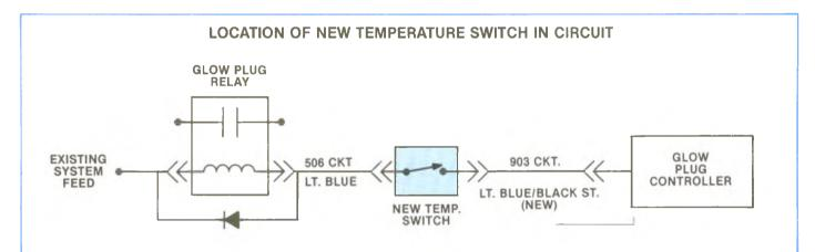
Figure 6-16, Temperature Inhibit Switch Circuit.
