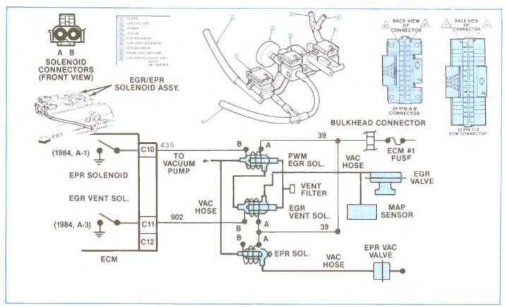
Figure 5-47, EGR/EGR Vent Schematic (1984 & 1985).
