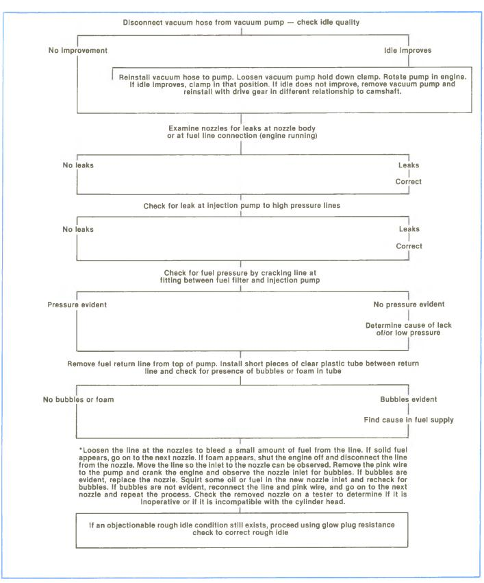
Figure 7-3, (Cont'd.) Diesel Engine Roughness Diagnosis Procedure.
