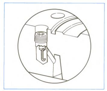
Fuel under transfer pump pressure is discharged from the transfer pressure annulus into a vent passage in the hydraulic head (Figure 4-56). Flow through the passage is restricted by a vent wire assembly to prevent excessive return oil and undue pressure loss.
