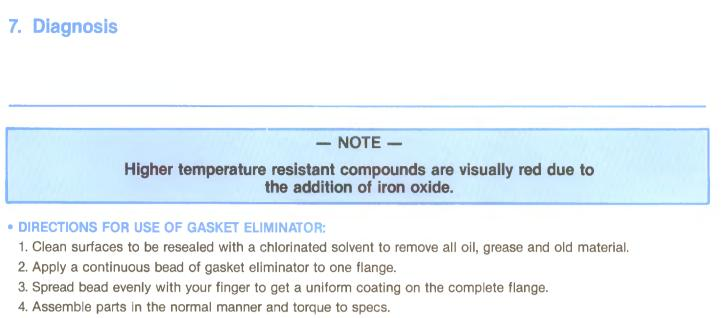
5. Vehicle can be operated after completion of assembly. No need to wait for gasket eliminator to cure.
