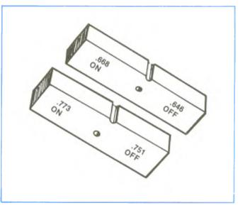
Figure 5-16B, Throttle Position Switch Gage Blocks
