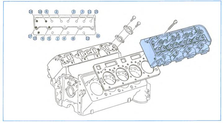
Figure 2-12, Cylinder Head.
