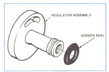
Figure 4-122, Installing Filter Screen Seal.
