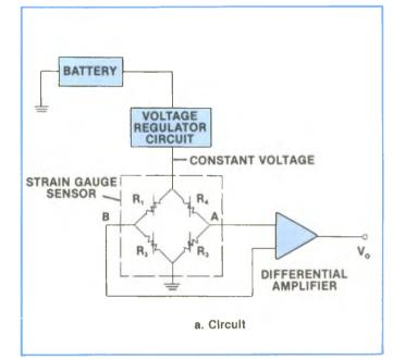
Figure 5-54A, Wheatstone Bridge Set-up.
