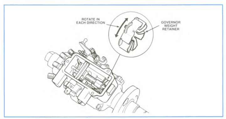
Figure 4-82, Failed Governor Weight Retainer Ring Checking Procedure.
