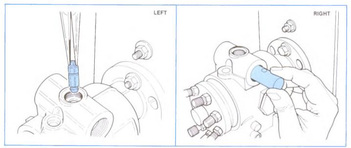
Figure 4-107, Removing Cam Advance Pin and Advance Piston.
