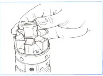
Figure 4-128, Installing Thrust Sleeve and Checking Weights.
