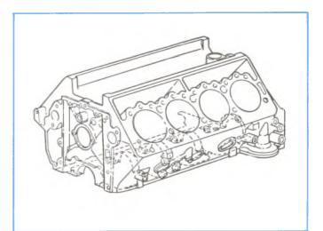
Figure 2-1, Cylinder Case.
