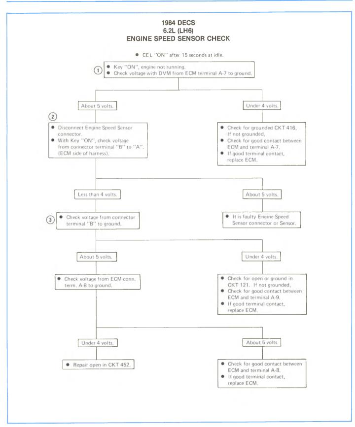
Figure 5-42, 1984 Engine Speed Sensor Chart.
