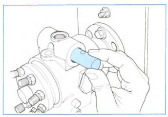
Figure 4-144, Installing the Advance Piston on Mechanical Light Load Pump.
