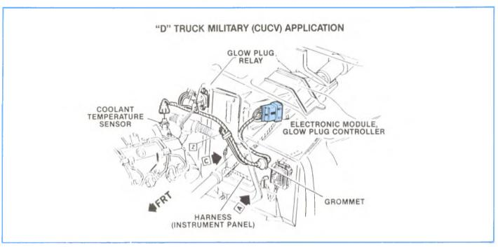
Figure 6-13, Electronic Module Glow Plug Controller (D-Truck).
