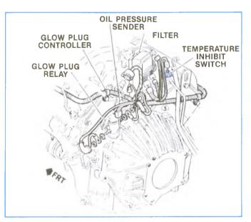
Figure 6-15, Temperature Inhibit Switch.
