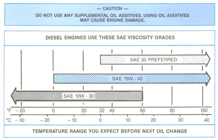
Figure 1-7, Ambient Temperature Range For Engine Oil.
