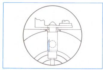
Figure 4-37, Metering Valve Light Load.
