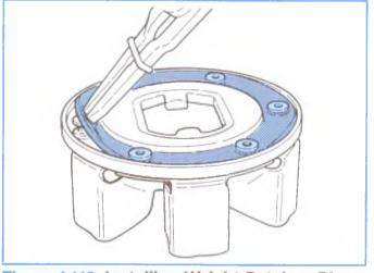
Figure 4-116, Installing Weight Retainer Ring With "Tru-Arcs".
