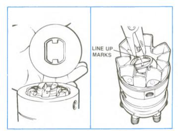
Figure 4-118, Installing Weight Retainer.
