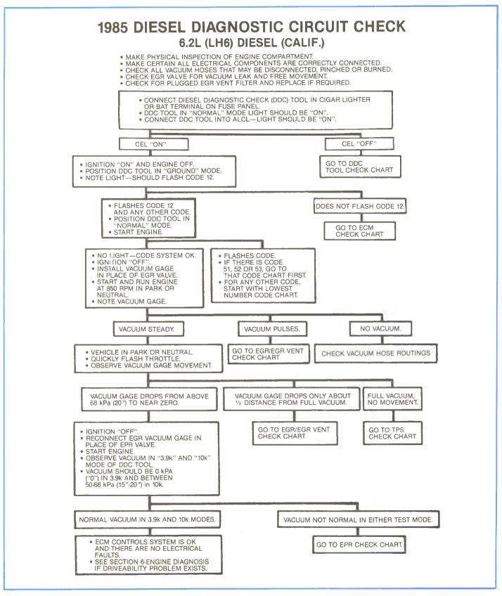
Figure 5-28, 1985 Diesel Diagnostic Circuit Check.
