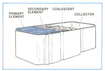
Figure 4-20, Model 80 Filter Cross-Section.
