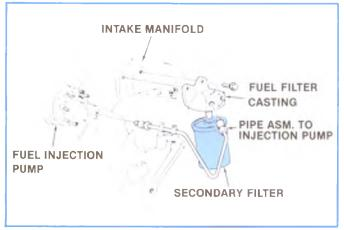
Figure 4-15a, Secondary Fuel Filter (C·K Series).
