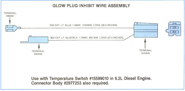
Figure 6-23, Glow Plug Inhibit Wire Assembly.
