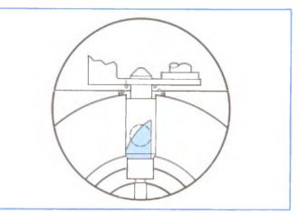
Figure 4-38, Metering Valve Full Load.
