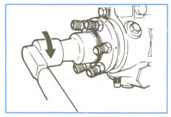
Figure 4-157, Installing the End Cap.
