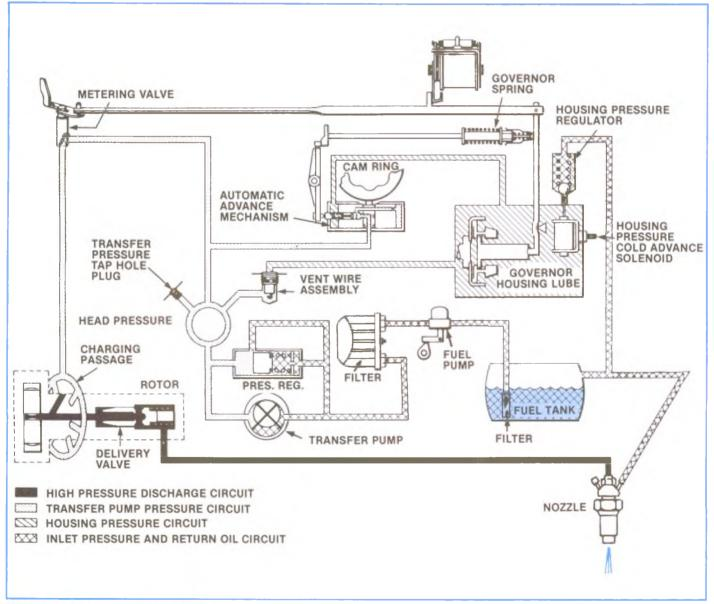
Figure 4-32, Pump Schematic.
