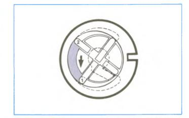
Figure 4-47, Transfer Pump In Mid Position.
