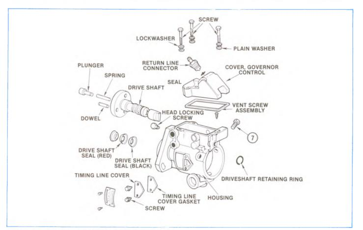
Figure 4-111A, Drive Shaft With Retaining Clip.
