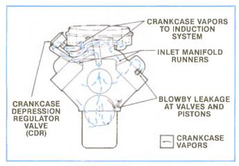
Figure 5-5, Crankcase Ventilation System.
