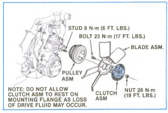
Figure 2-45, Viscous Fan Drive.
