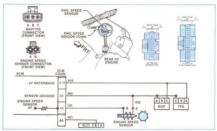
Figure 5-43, 1985 Engine Speed Sensor Schematic.
