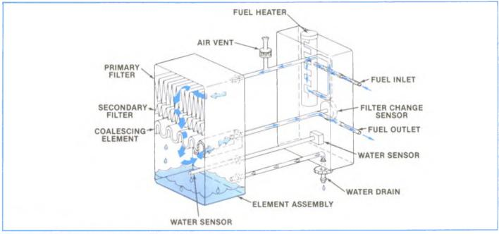
Figure 4-22, Filter and Base Flow Schematic.
