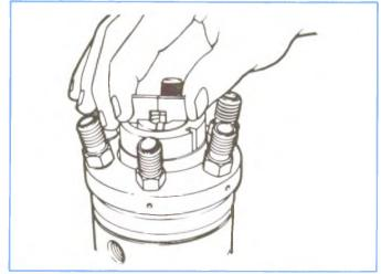
Figure 4-121, Installing Transfer Pump Blades.
