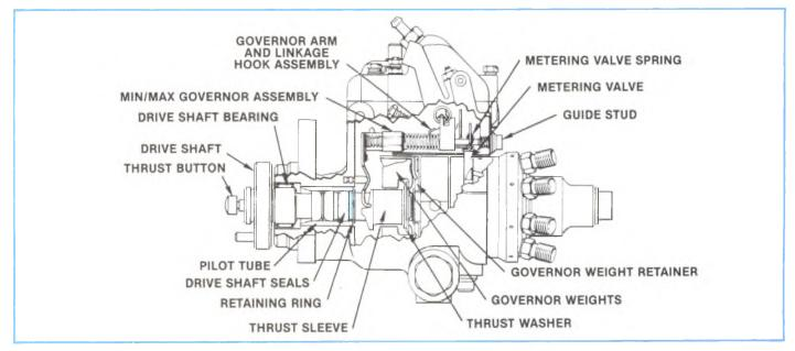
Figure 4-134, Installing Shaft in Pump.
