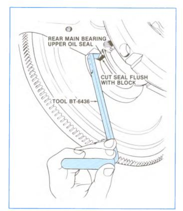
Figure 2-24, Cutting Seal In-Vehicle.
