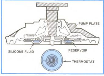
Figure 2-47, Fluid Reservoir and Thermostat.
