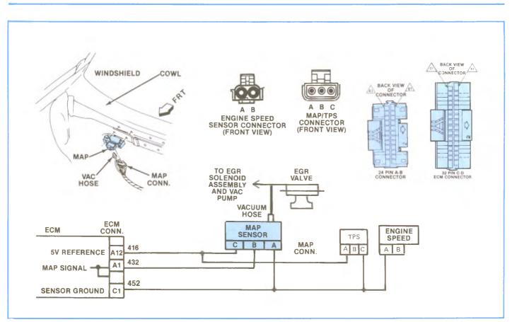
Figure 5-53, 1985 MAP Sensor Schematic.
