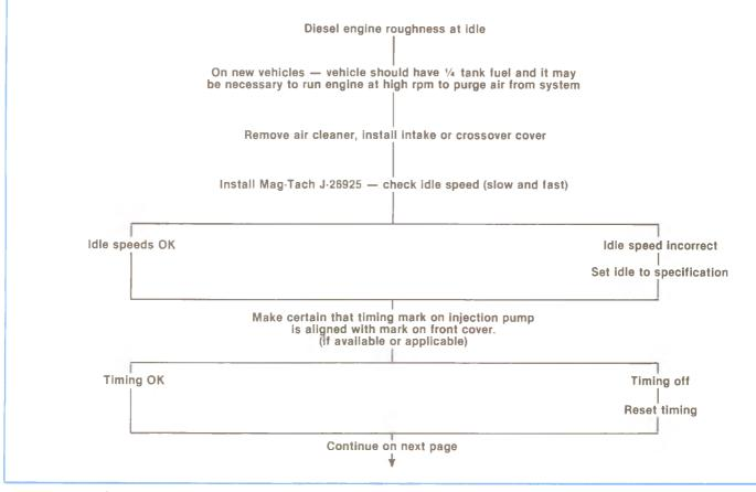
Figure 7-3, Diesel Engine Idle Roughness Diagnosis Procedure.
