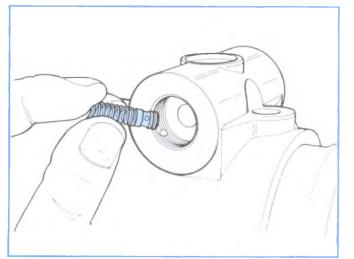
Figure 4-146, Installing Servo Valve.
