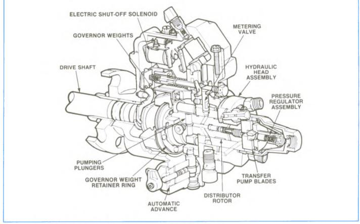
Figure 4-31, DB2 Distributor-Type Injection Pump Cutaway.
