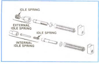
Figure 4-74, Internal Idle Spring Design.
