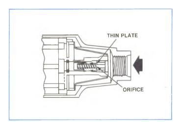
Figure 4-54, Orifice Control.
