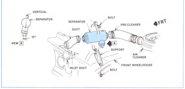
Figure 3-3. RPO K46 Air Pre-Cleaner Chamber.
