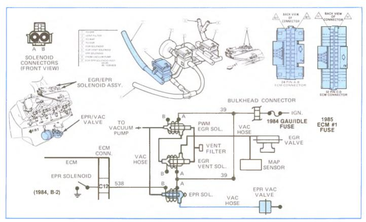
Figure 5-51, EPR Solenoid Schematic (1984 & 1985).
