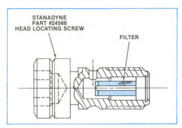
Figure 4-66, Head Locating Screw With Filter.
