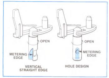
Figure 4-39, Metering Valve Designs.
