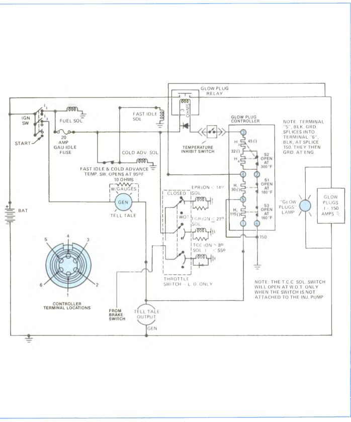
Figure 6-17, Glow Plug Schematic.
