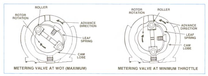
Figure 4-60, Cam Positioning.
