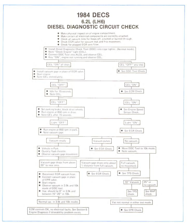
Figure 5-27, 1984 Diagnostic Circuit Check.
