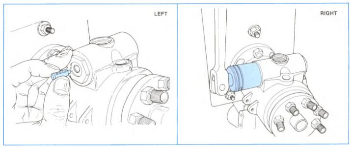
Figure 4-105, Removing Servo Advance Plunger and Piston Hole Plug.
