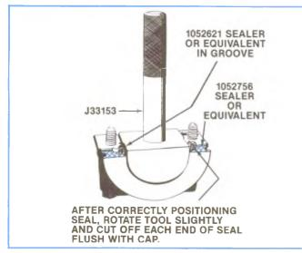
Figure 2-25, Installing Rear Main Lower Oil Seal.
