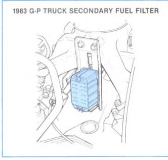
Figure 4-16, G-P Model 75 Secondary Fuel Filter.
