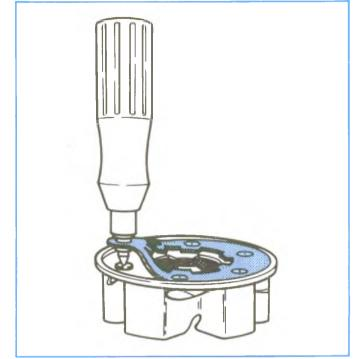
Figure 4-117, Installing Ring With Tool BT 8209-A.
