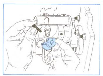
Figure 4-151, Installing Face Cam Screw.
