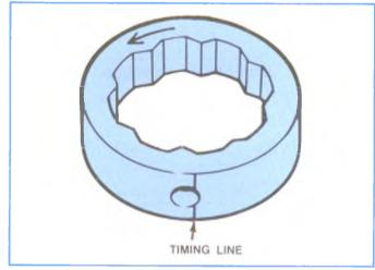
Figure 4-115, Cam Ring Timing Line.
