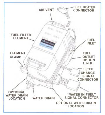
Figure 4-18, Model 80 Fuel Filter and Base Assembly.
