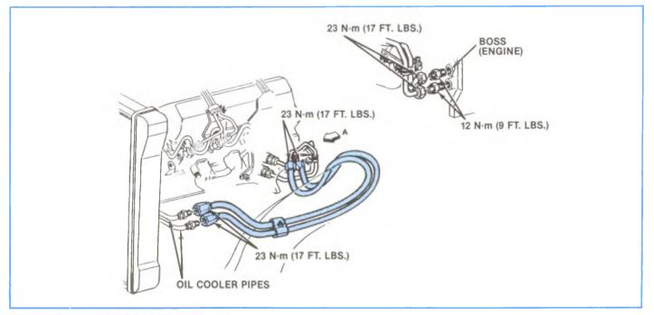
Figure 2-34, 6.2L Oil Cooler Lines.
