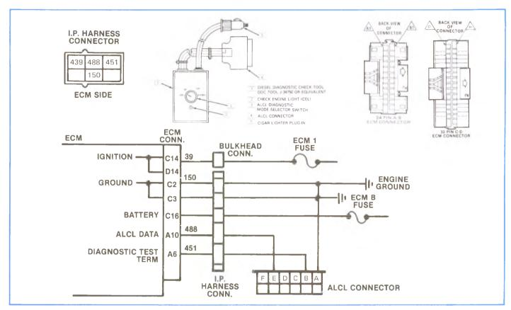
Figure 5-36, 1985 ECM Check Schematic.
