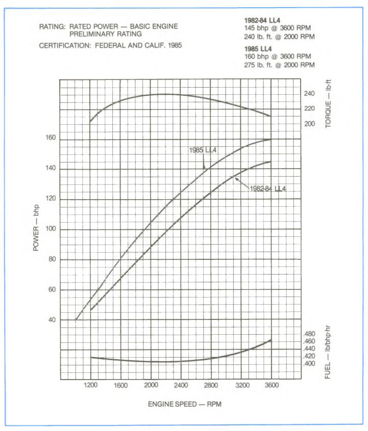
Figure 1-4, Engine Performance Curve, 6.2L — Heavy Duty (LL4)
