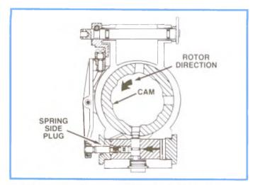
Figure 4-62, Cam and Rotor Movement.
