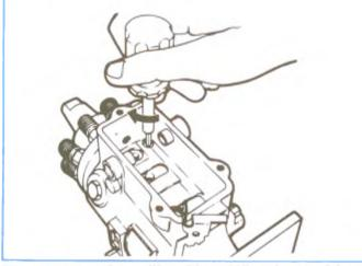
Figure 4-136, Installing Vent Wire Assembly.
