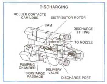
The fuel then flows through the discharge outlet and discharge port to the injection nozzle. (Figure 4-44).
