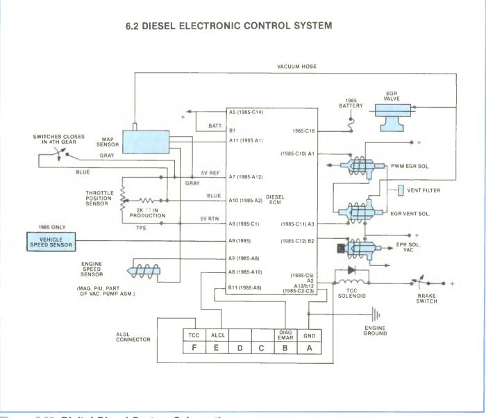
Figure 5-20, Digital Diesel System Schematic.
