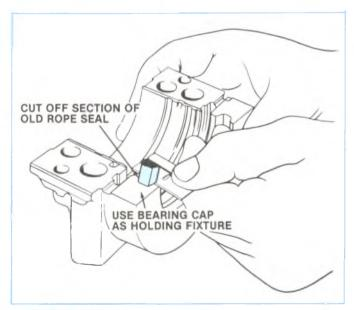
Figure 2-23, Cutting Section of Rope Seal.
