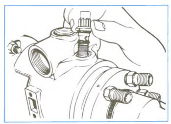
Figure 4-142, Installing Head Locating Screw.
