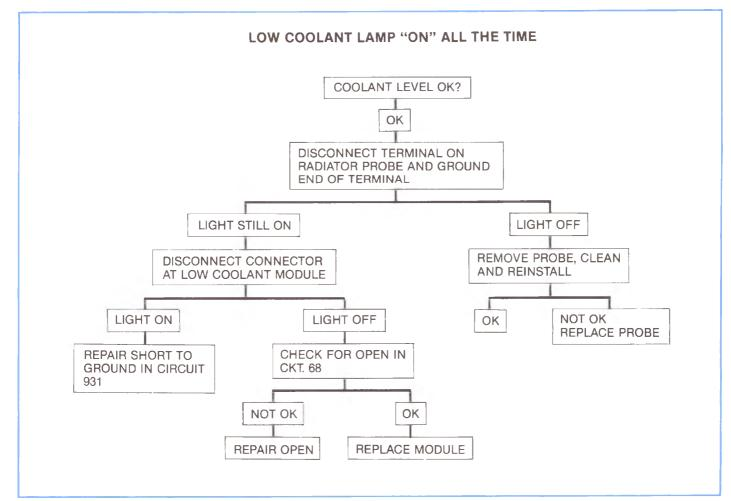
Figure 2-62, Low Coolant Lamp Remains "On".
