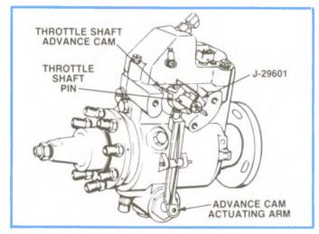
Figure 4-84, Face Cam Tool J-29601.
