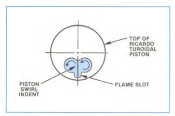
This piston has a half-clover shaped identation on the piston face, which at T.D.C. outlets to the pre-chamber, Figure 2-19. As the piston rises during the compression stroke, the air swirl begins in these two indentations. When the piston reaches the pre-chamber opening, the air swirl is increased in the spherical pre-chamber. This is a Ricardo Turoidal Piston design and is used with the Ricardo COMET V Pre-Chamber for more complete mixing of the air and fuel.
