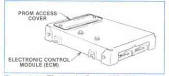
Figure 5-31, Electronic Control Module.
