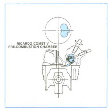
Figure 3-6, Pre-Combustion Chamber.
