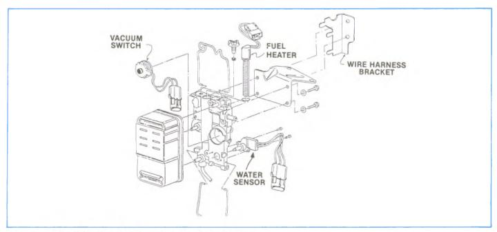
Figure 4-28, 1985 Model 80 Filter, Exploded View.
