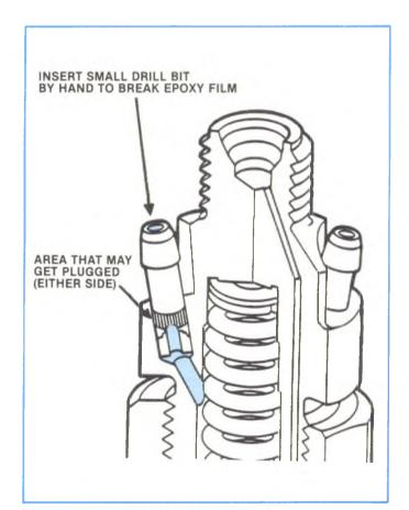
Figure 7-5, Fuel Injection Nozzle.
