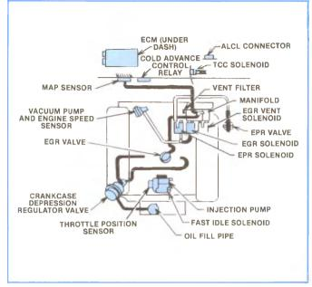
Figure 5-44, Emission Systems — California CK (LH6 Engine).
