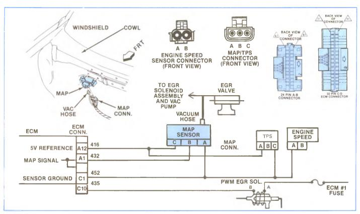
Figure 5-56, 1985 MAP Sensor Schematic (Code 31).
