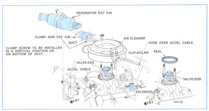
Figure 3-1, LH6 Air Intake System With EGR Valve
