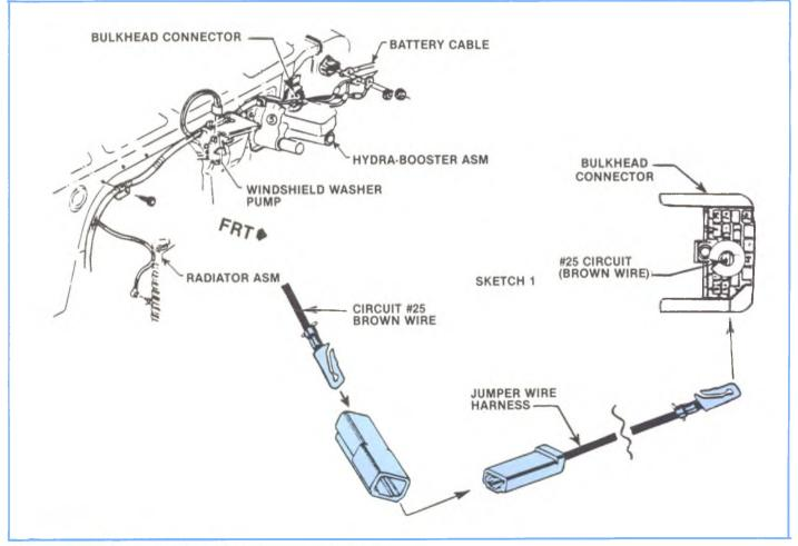
Figure 6-34, Jumper Wire Harness Installation.
