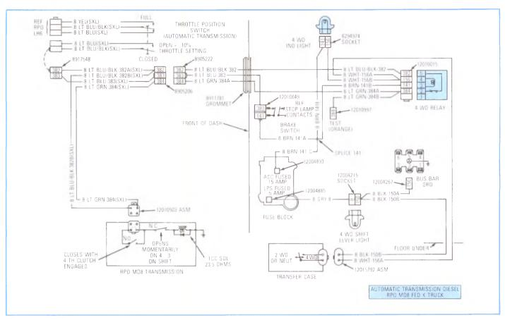
Figure 5-14, Wiring Diagram T.C.C. MD-8 K Truck.
