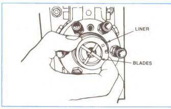
Figure 4-102, Removing Transfer Pump Blades and Liner.
