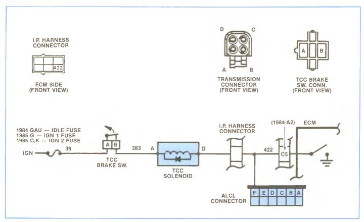
Figure 5-67, Torque Converter Clutch, TCC Circuit.
