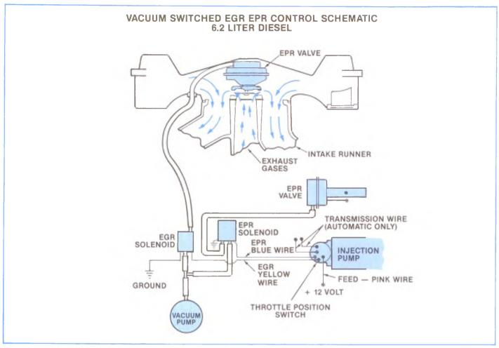
Figure 5-13, Federal EPR/EGR Schematic
