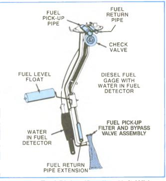
Figure 4-4, Fuel Pickup/Sending Unit With Water-in-Fuel Warning.
