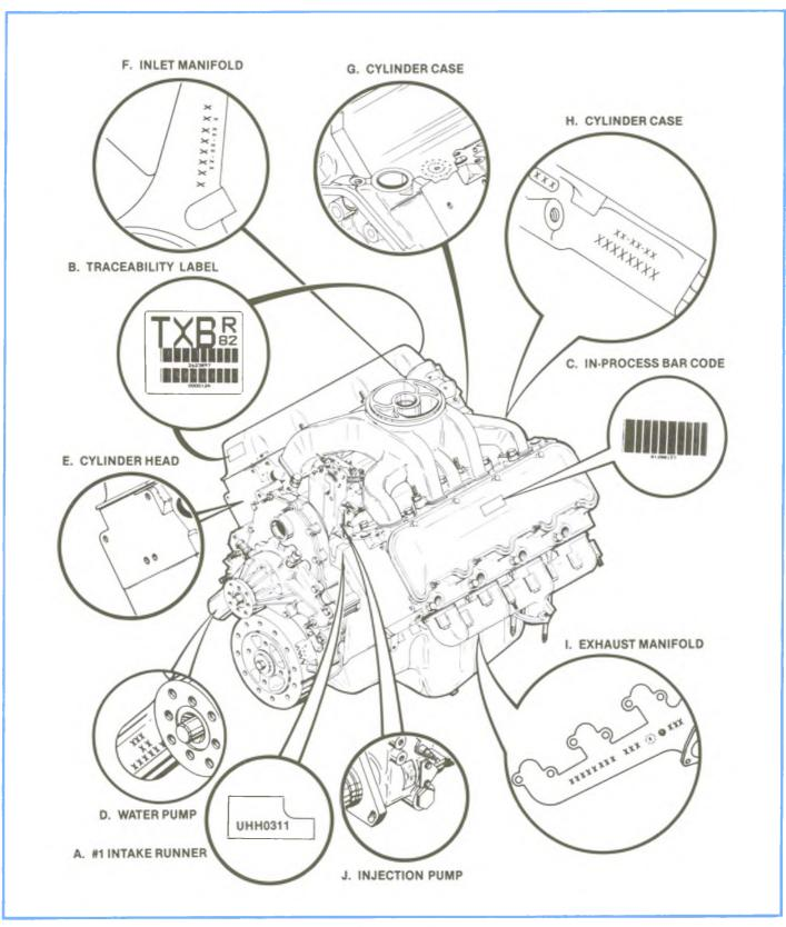
Figure 1-2, Engine Identification.
