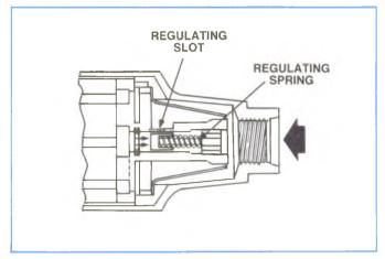
Figure 4-52, Thin Fuel Correction.
