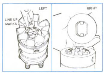
Figure 4-110, Removing Weight Retainer.
