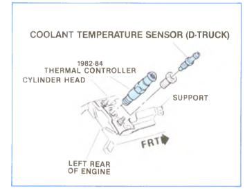
Figure 6-11, Thermal Controller.
