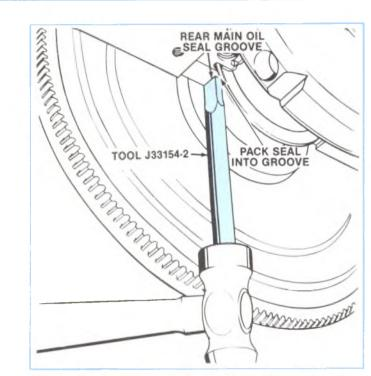
Figure 2-22, Packing Rear Main Upper Seal.
