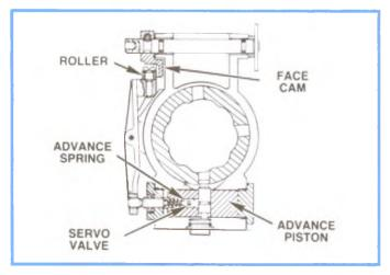
Figure 4-64, Face Cam To Rocker Lever Action.
