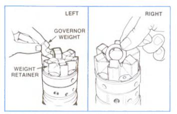
Figure 4-127, Installing Weights and Washer.
