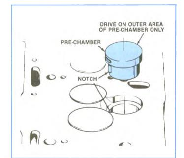
Figure 3-7, Pre-Chamber Installation in Cylinder Head.
