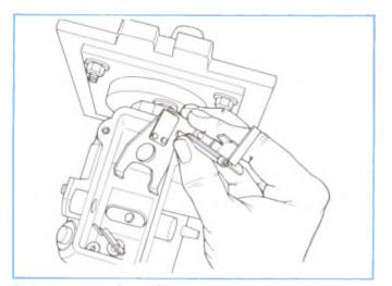
Figure 4-135, Installing Governor Arm.
