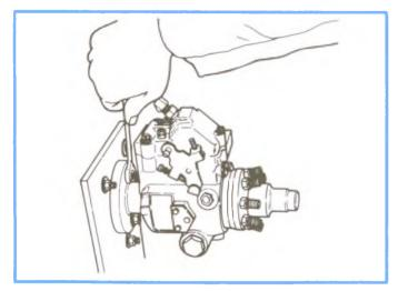
Figure 4-83, Mounting Pump in Fixture.
