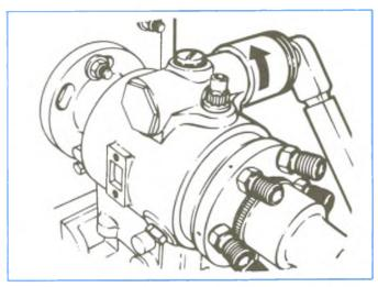
Figure 4-148, Tightening Piston Hole Plug.
