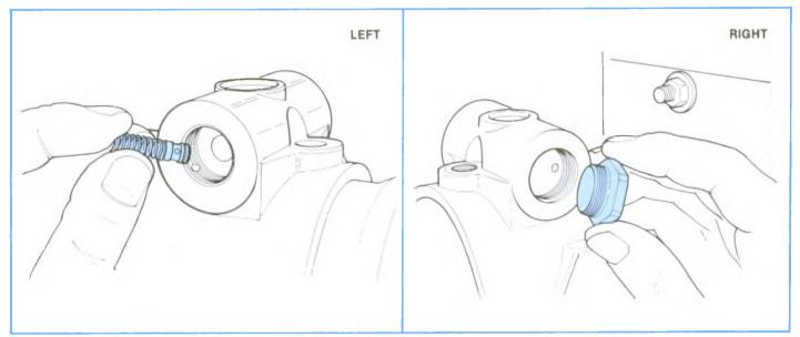
Figure 4-106, Removing Spring and Valve (Left) and Power Side Plug (Right).
