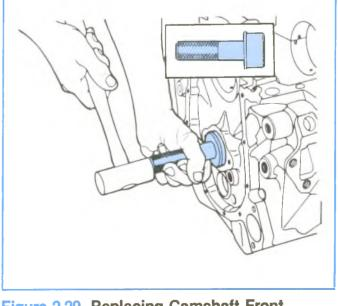
Figure 2-29, Replacing Camshaft Front Bearing
