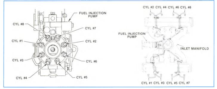
Figure 4-168, 6.2L High Pressure Fuel Lines.
