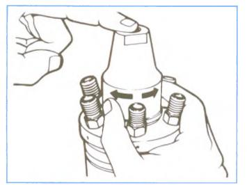
Figure 4-125, Installing Transfer Pump End Cap.
