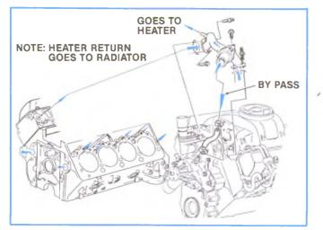
Figure 2-58, Cooling System Flow.
