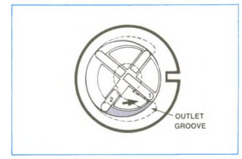
Figure 4-48, Transfer Pump In Lower Position.
