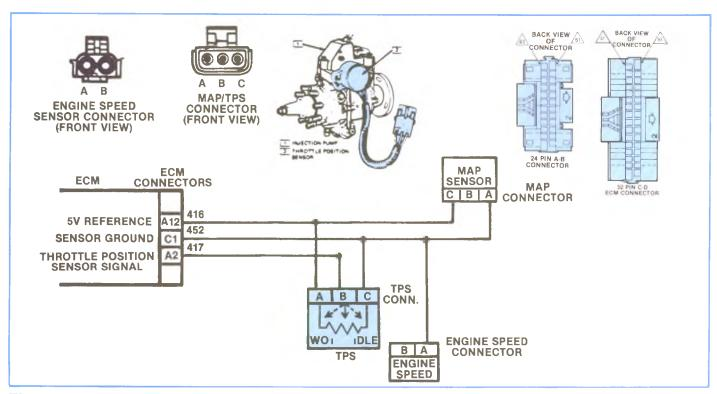
Figure 5-62, 1985 TPS Schematic.
