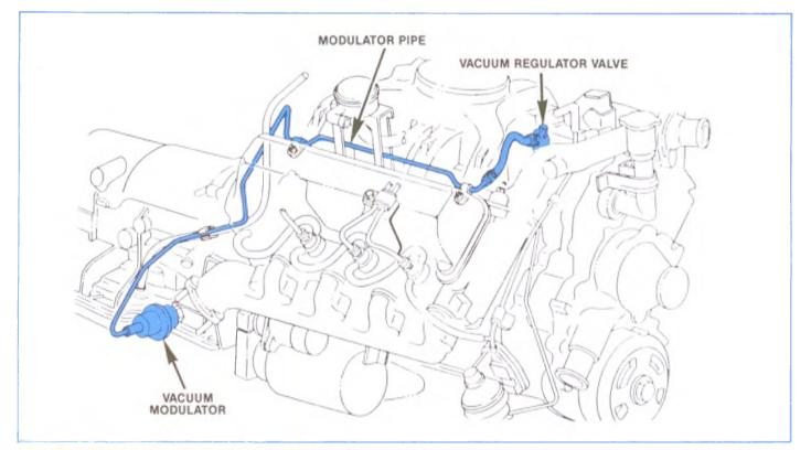
Figure 5-16, Vacuum Regulator Valve (VRV).
