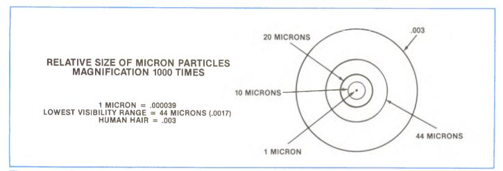
Figure 4-17, Relative Size of Micron Particles.
