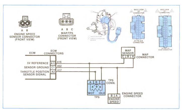
Figure 5-63, 1985 TPS Schematic.
