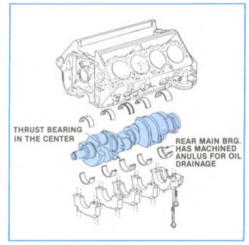
Figure 2-20, Crankshaft.
