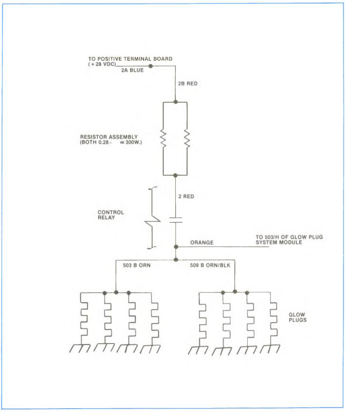
Figure 6-28, Glow Plug Power System, D-Truck.
