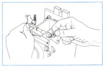
Figure 4-94, Removing Throttle Assembly.
