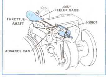
Figure 4-152, Feeler Gage to Position Cam.
