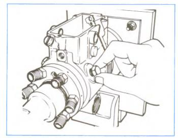
Figure 4-132, Hand Tightening Head Locking Screw.
