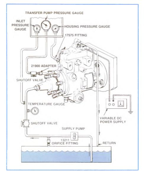
Figure 4-81, Typical Test Stand Installation.
