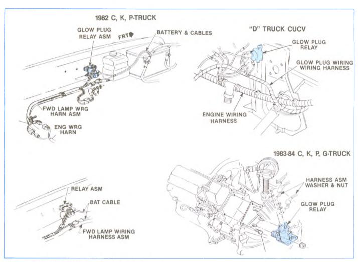
Figure 6-14, Glow Plug Relay Locations.
