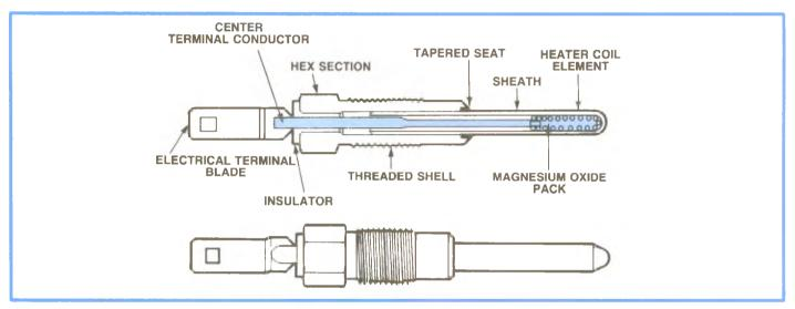
Figure 6-8, Typical AC Diesel Engine Glow Plug.
