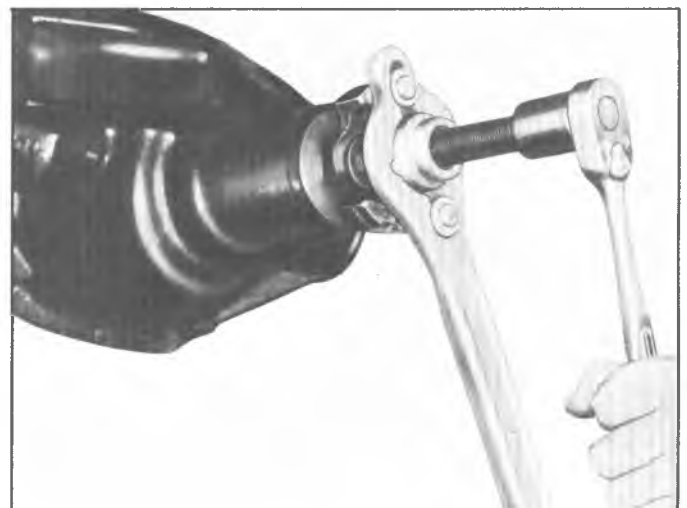
Fig. 13B—Drive Pinion Flange Removal
