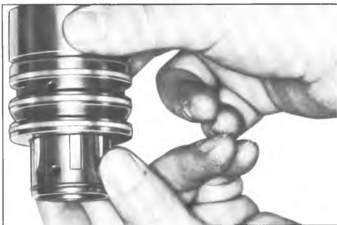
Fig. 44--Removing Spool Valve
