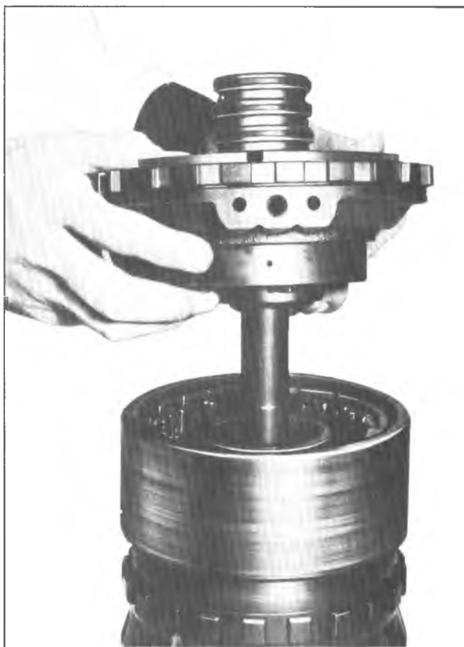
Fig. 39T--Removing Center Support Assembly
