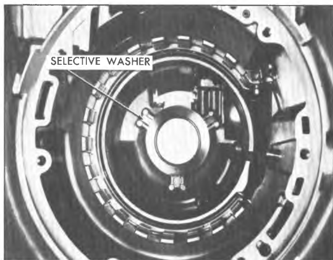
Fig. 37T--Removing Selective Washer
