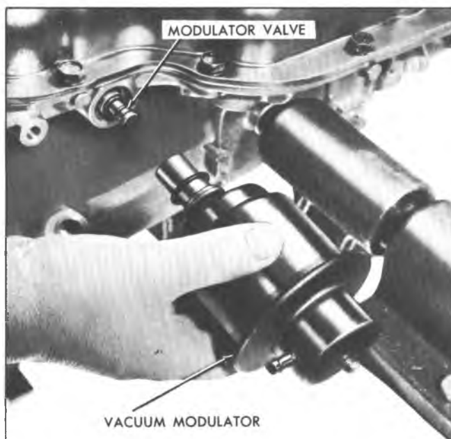
Fig. 153T--Installing Vacuum Modulator and Valve
