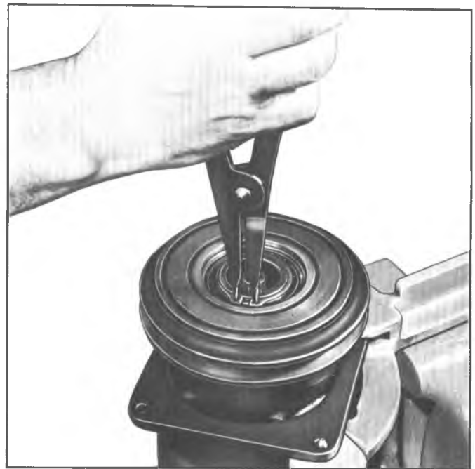
Fig. 6--Removing Pulley and Bearing Assembly Retainer Ring
