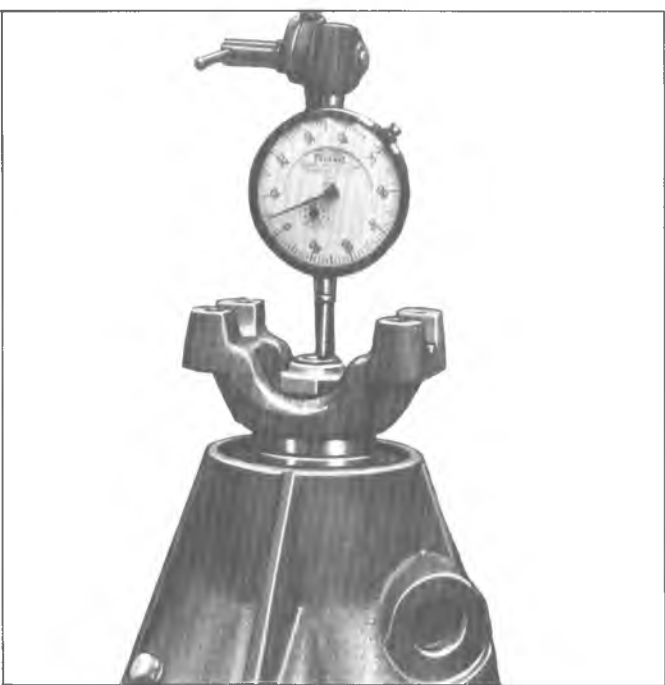
Fig. 24F—Checking Rear Output Shaft End Play
