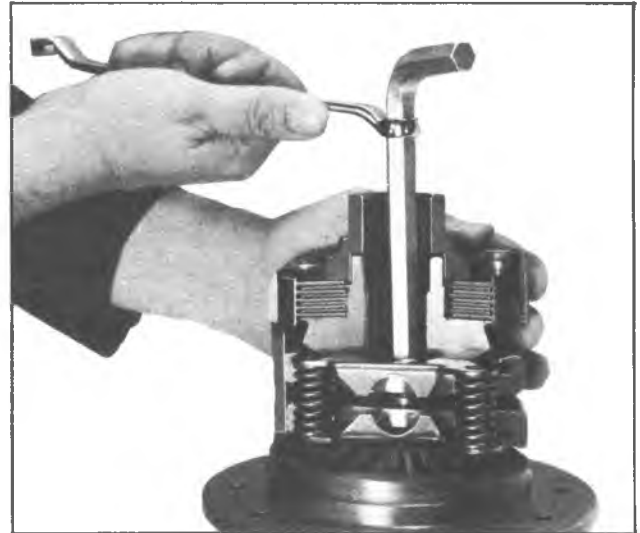
Fig. 5D—Removing Preload Spring Pack (Corvette)
