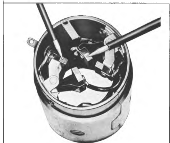
Fig. 7S--Field Coil Ground Test
