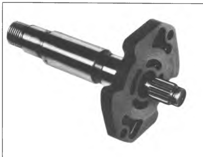
Fig. 22--Installing Thrust Plate
