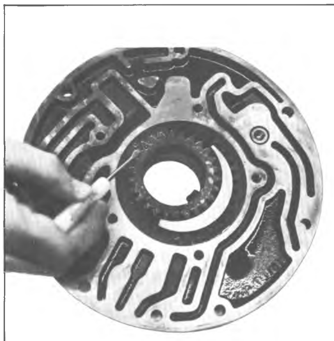
Fig. 63M--Installing Pump Drive and Driven Gears
