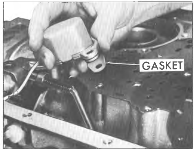
Fig. 14T-Removing Detent Solenoid and Gasket
