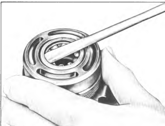
Fig. 7--Removing Lower Bearing Retainer--Except Corvette
