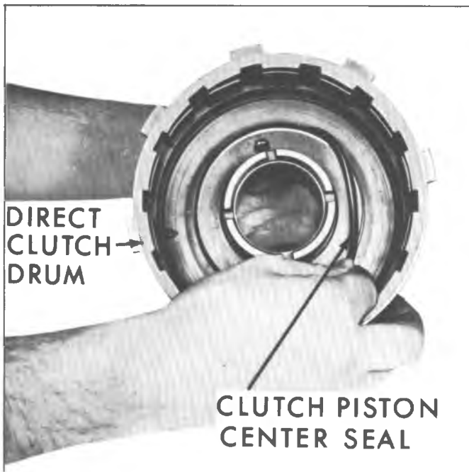
Fig. 74M--Removing Direct Clutch Piston Center Seal
