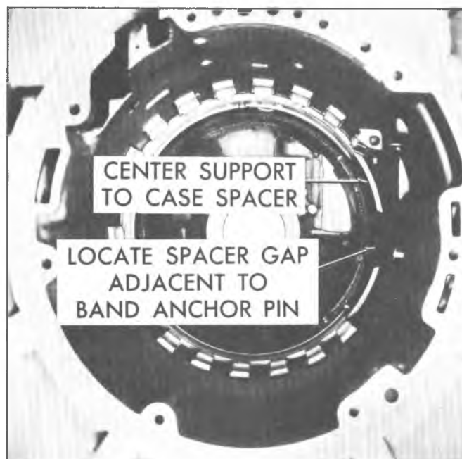
Fig. 129T-A--Installing Center Support to Case Spacer
