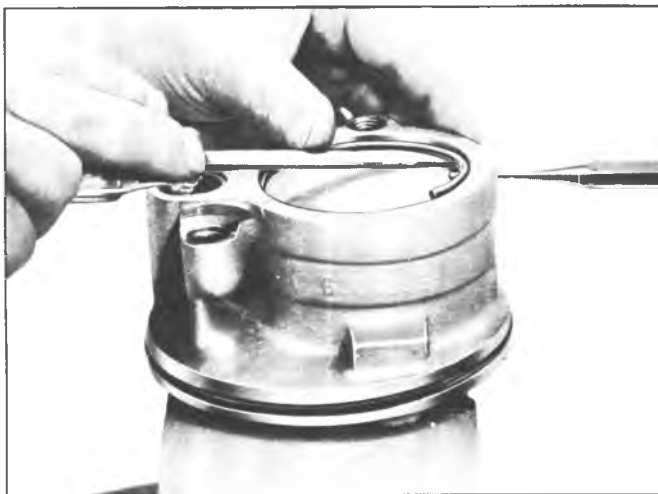
Fig. 18--Removing End Plate Ring
