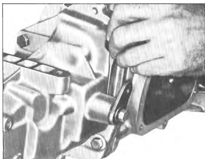
Fig. 4B--Removing Reverse Shifter Shaft Lock Pin
