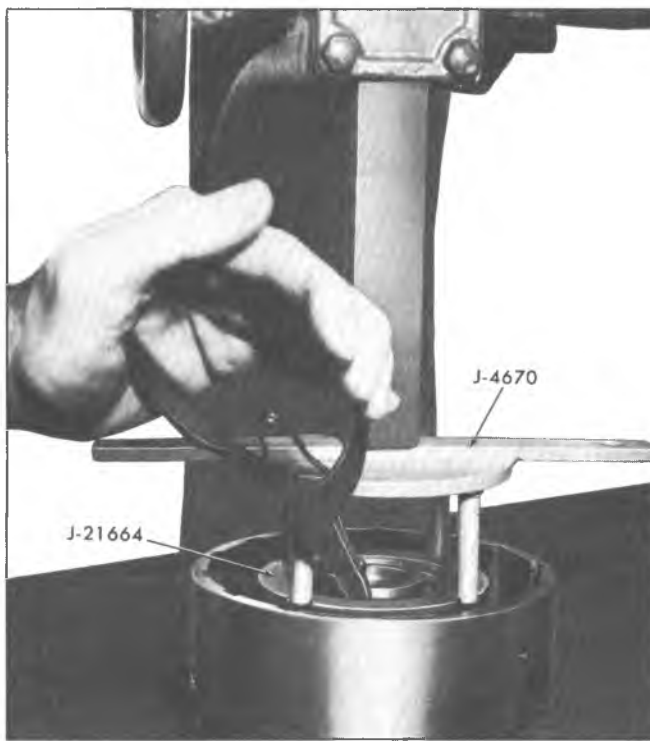
Fig. 70T--Removing Forward Clutch Spring Retaining Snap Ring
