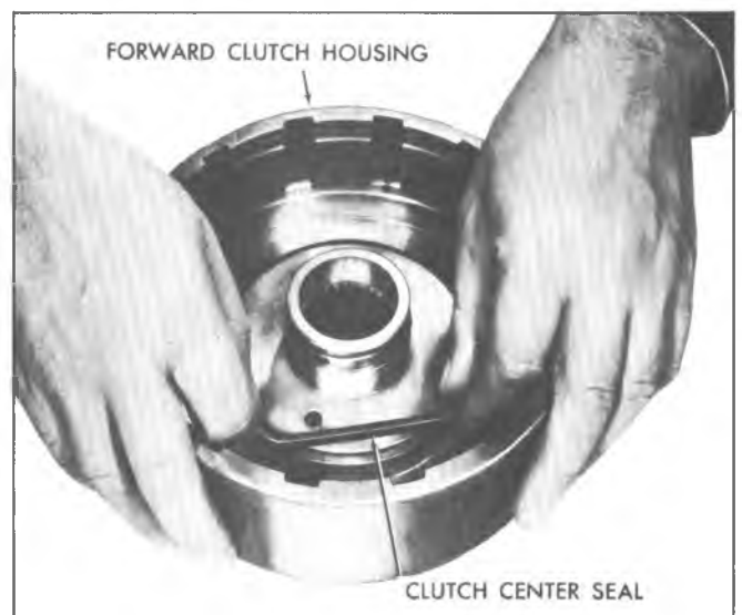
Fig. 72T--Removing Forward Clutch Center Seal
