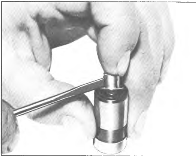
Fig. 31—Removing Ball Check Valve
