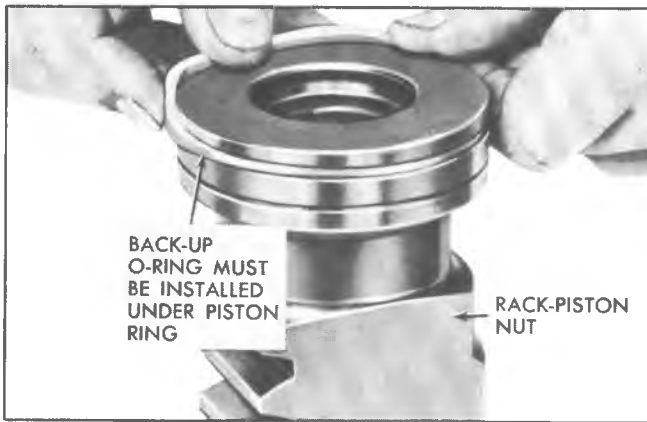
Fig. 47--Installing Ring on Rack-Piston
