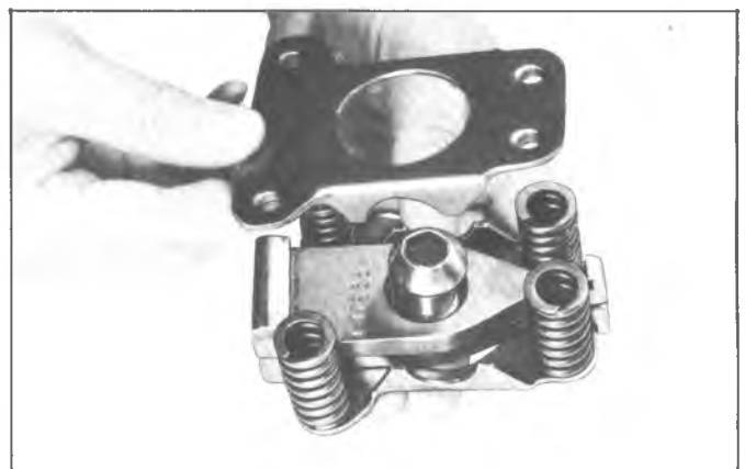
Fig. 13D—Installing Spring Pack Compression Tool (Corvette)
