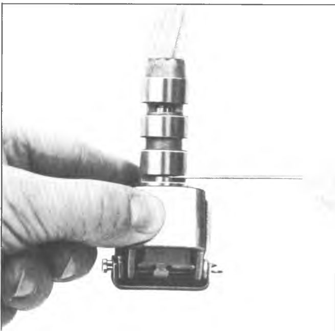
Fig. 48T-B--Checking Valve Opening With Weight Inward
