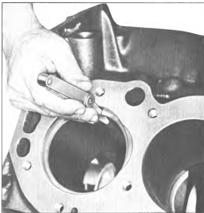
Fig. 55—Measuring Ring Gap
