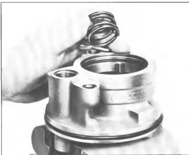
Fig. 28-Installing Pressure Plate Spring
