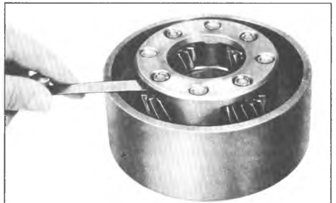
Fig. 105T--Checking Pinions End Play
