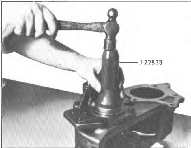
Fig. 15D--Installing Front Output Shaft Seal
