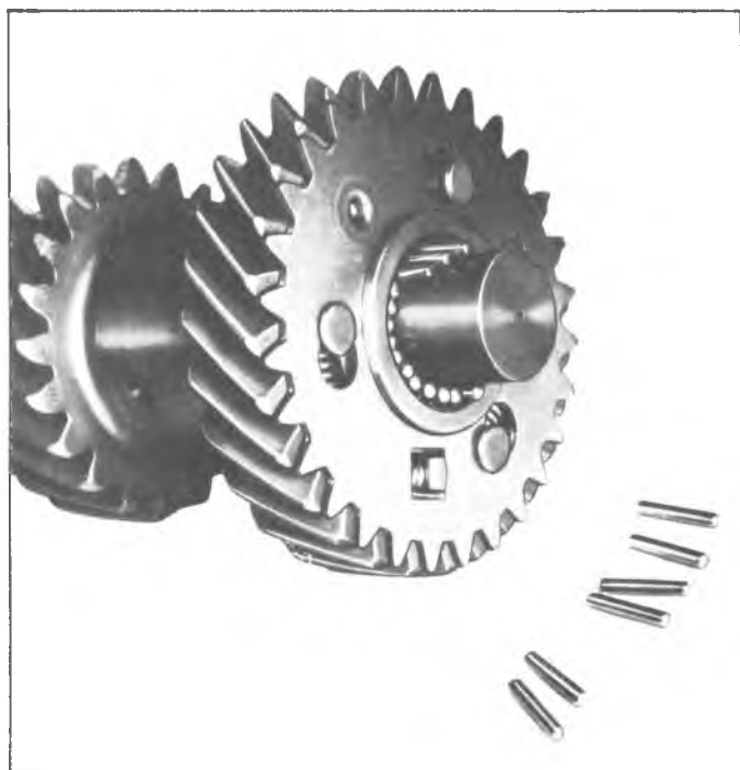
Fig. 19X--Loading Countergear Bearings
