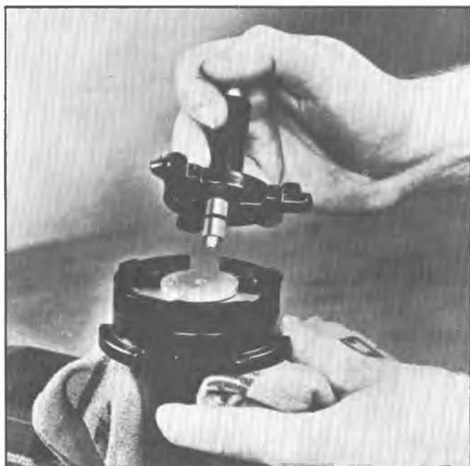
Fig. 12A--Installing Reaction Retainer on Power Piston
