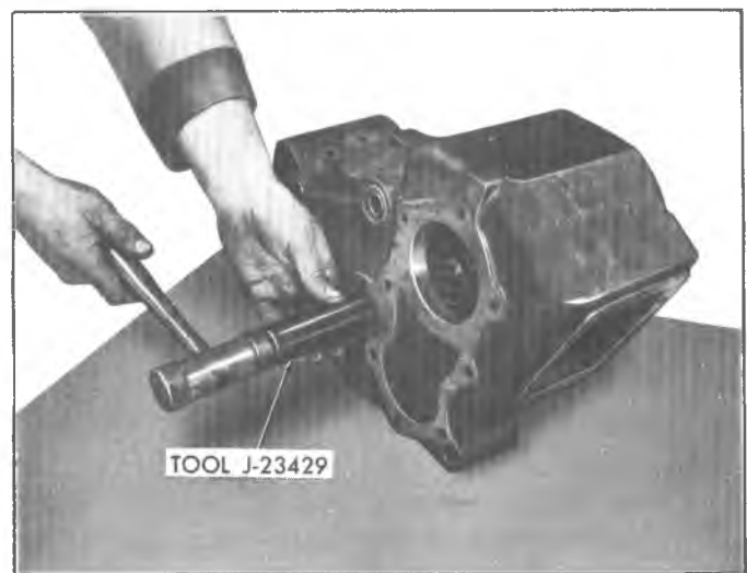
Fig. 8C--Removing Idler Gear Shaft
