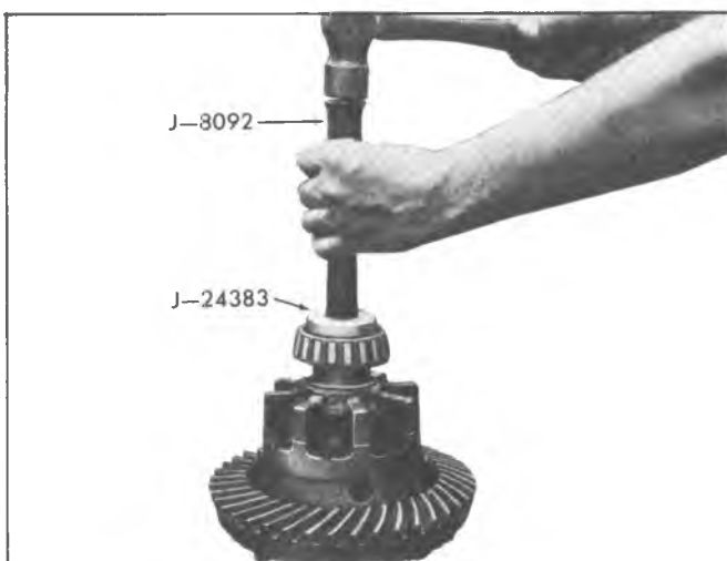
Fig. 7F—Installing Side Bearing
