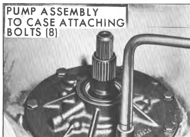
Fig. 26M--Removing Pump Attaching Bolts
