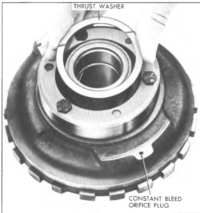
Fig. 40T--Removing Center Support Thrust Washer
