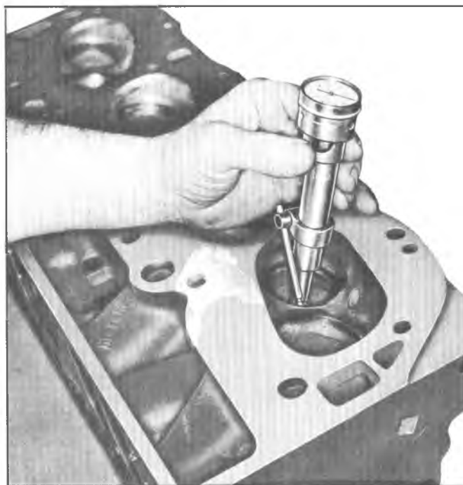
Fig. 24—Measuring Valve Seat Concentricity
