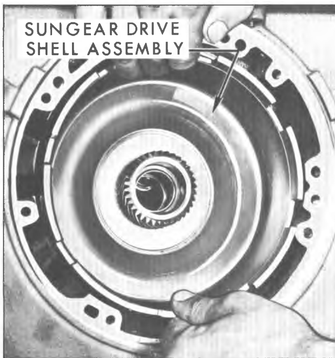
Fig. 38M--Removing Sun Gear Drive Shell
