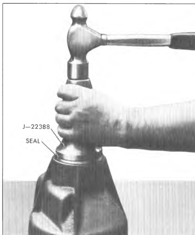
Fig. 19F—Installing Rear Output Housing Seal
