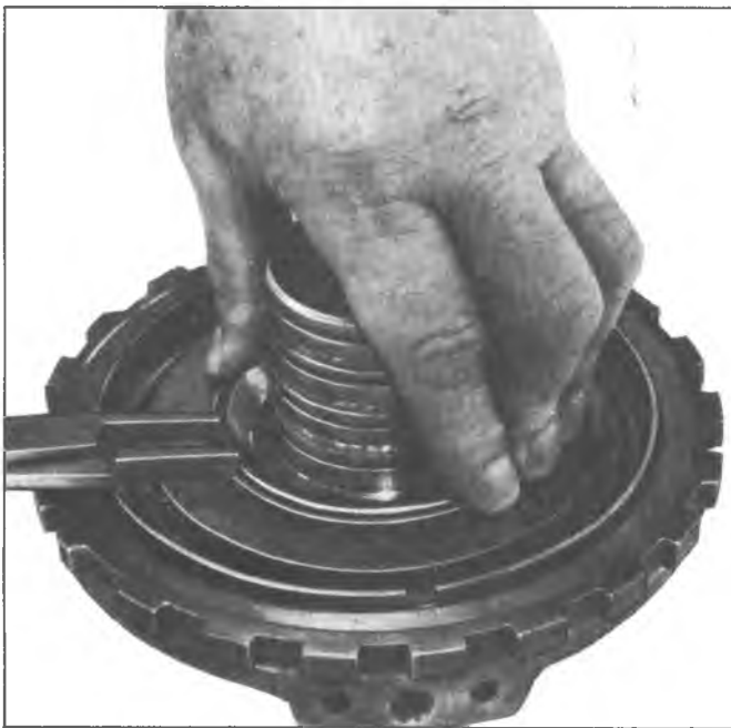
Fig. 103T--Installing Intermediate Clutch Piston Snap Ring
