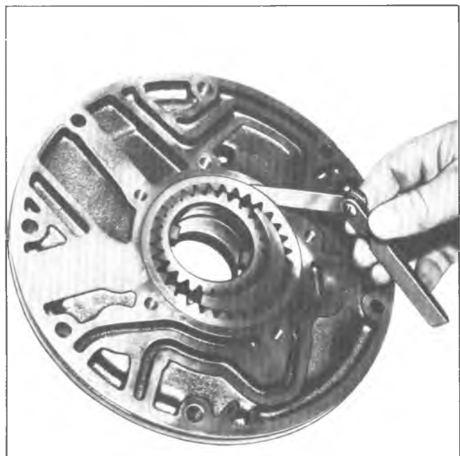
Fig. 17PG--Checking Driven Gear to Pump Body Clearance
