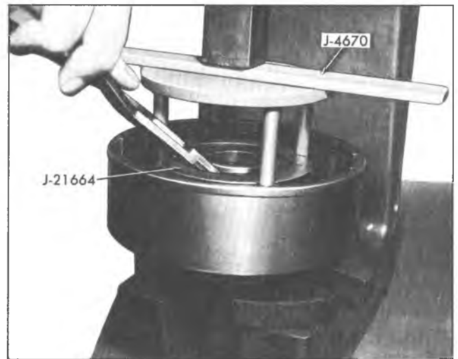
Fig. 81T--Removing or Installing Direct Clutch Snap Ring
