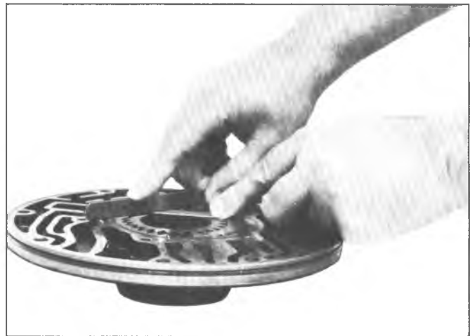
Fig. 60M--Checking Pump Body to Gear Face Clearance
