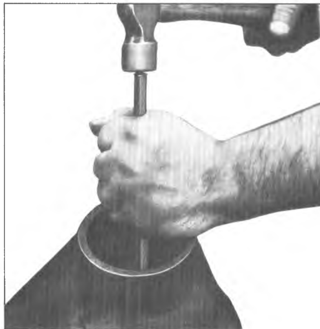
Fig. 18F—Removing Rear Output Shaft Front Bearing
