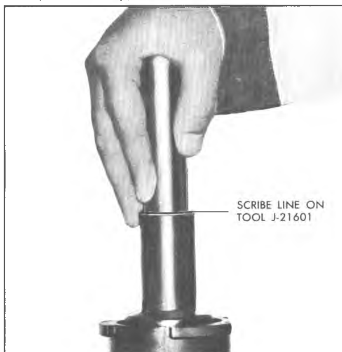
Fig. 10A--Installing Air Valve and Retainer
