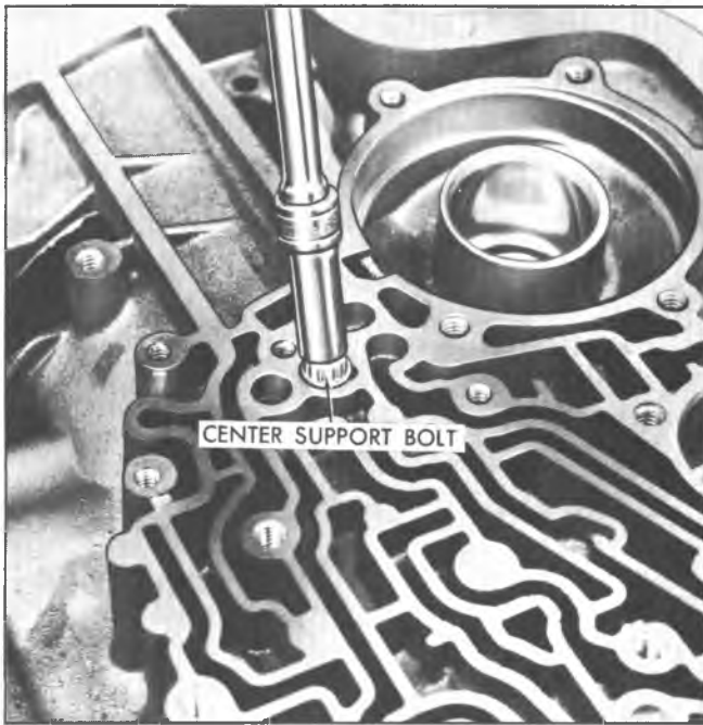
Fig. 33T--Removing Center Support Bolt
