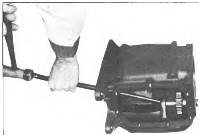
Fig. 6X--Removing Reverse Idler Gear Shaft
