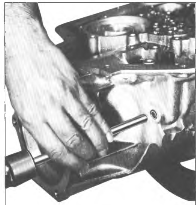
Fig. 127T--Installing Parking Pawl Shaft Cup Plug
