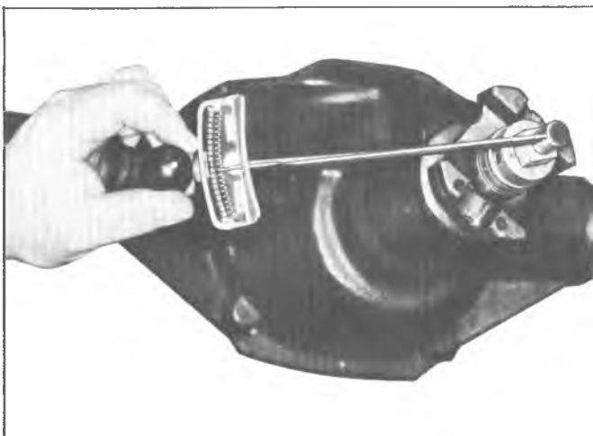
Fig. 24A—Measuring Rotating Torque
