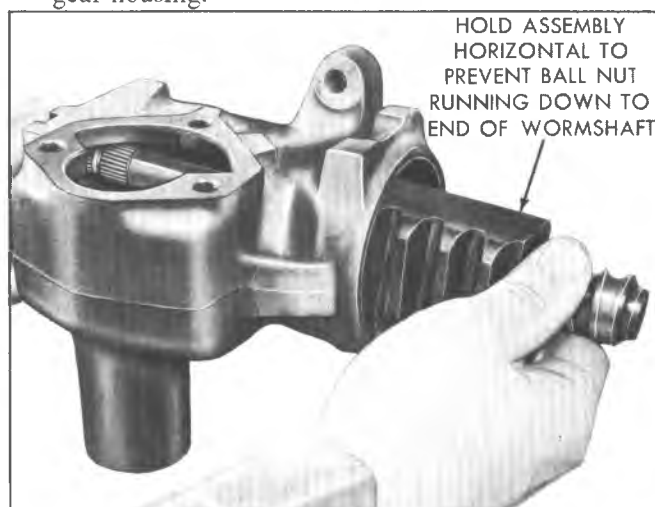
Fig. 6--Removing the Wormshaft and Ball Nut--Typical
