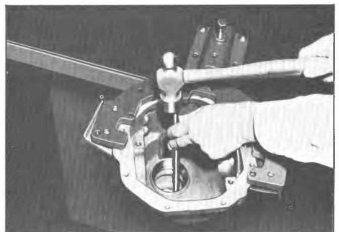
Fig. 16C—Removing Pinion Bearing Cup
