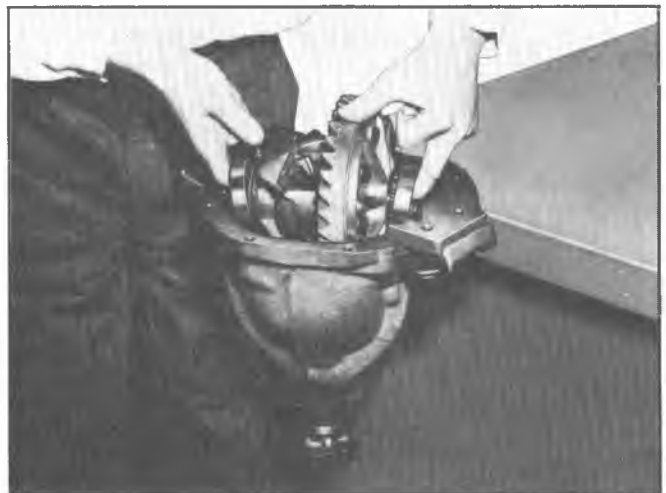
Fig. 8C—Installing Differential Assembly
