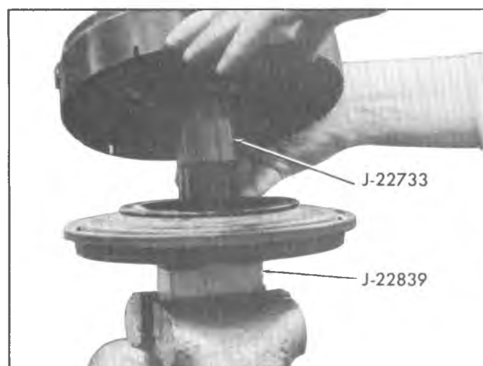
Fig. 8D--Seal Protector J-22733 Installed
