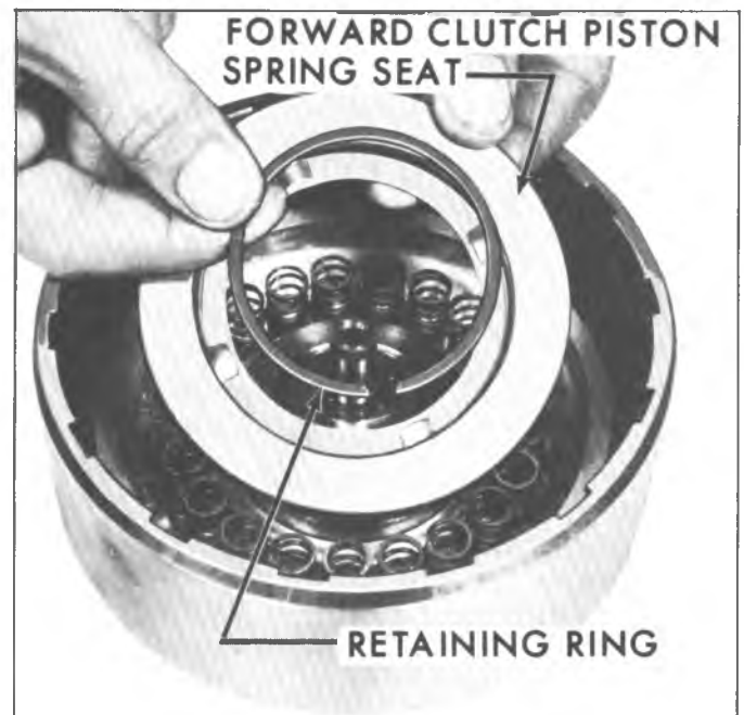
Fig. 76M--Installing Direct Clutch Springs, Spring Seat and Retaining Ring
