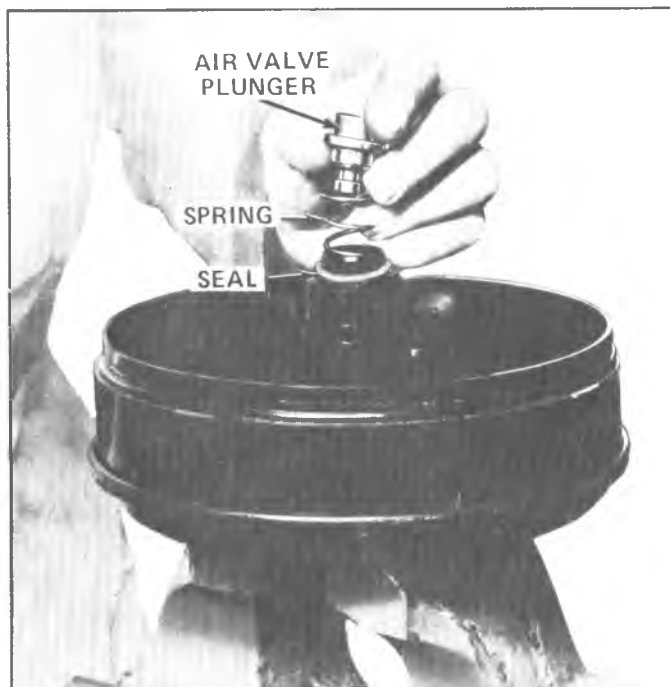
Fig. 9D--Installing Air Valve Assembly
