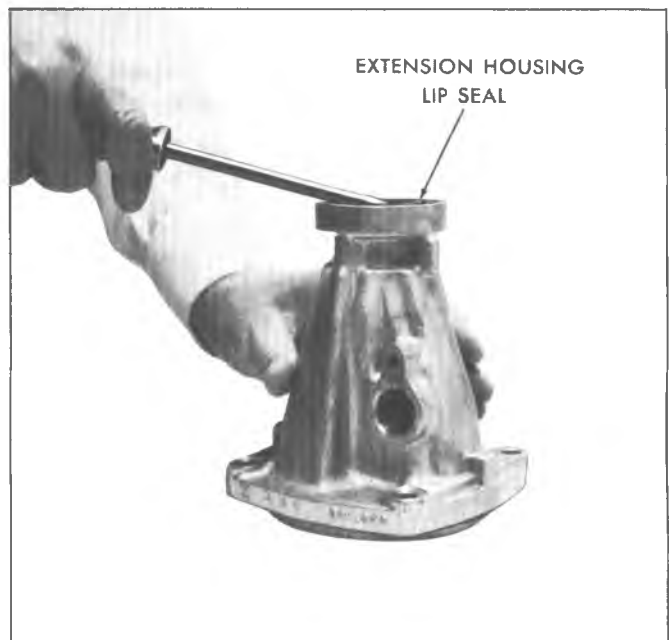
Fig. 4M--Removing Extension Housing Lip Seal
