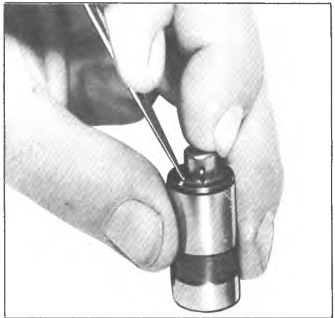
Fig. 32—Installing Ball Check Valve
