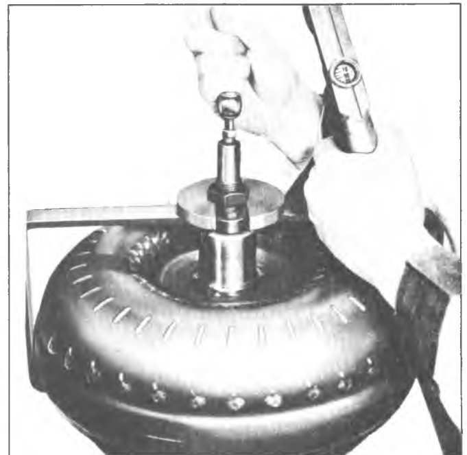
Fig. 114T--Air Checking Converter
