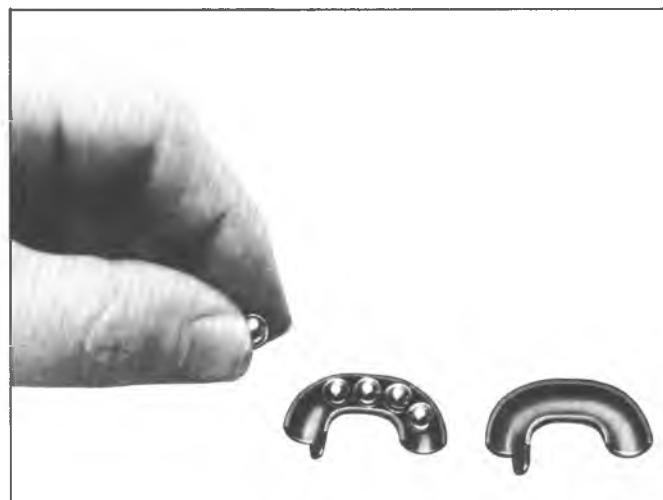
Fig. 13--Filling Ball Guides--Corvette
