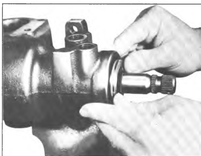
Fig. 56--Installing Valve Body
