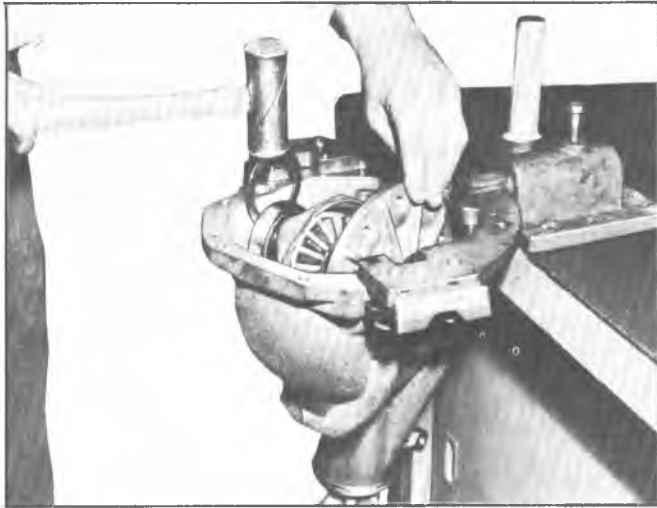
Fig. 11C—Installing Differential Shim
