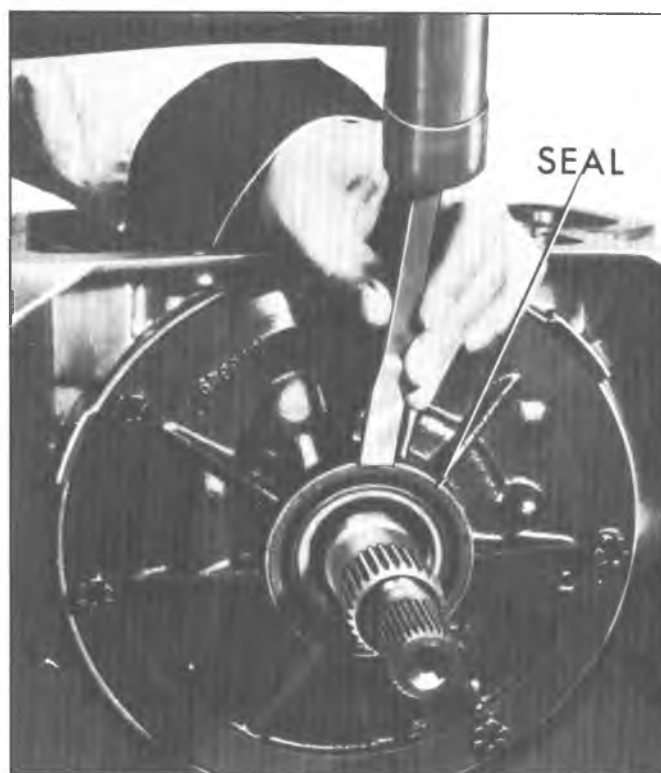
Fig. 26T--Removing Front Seal
