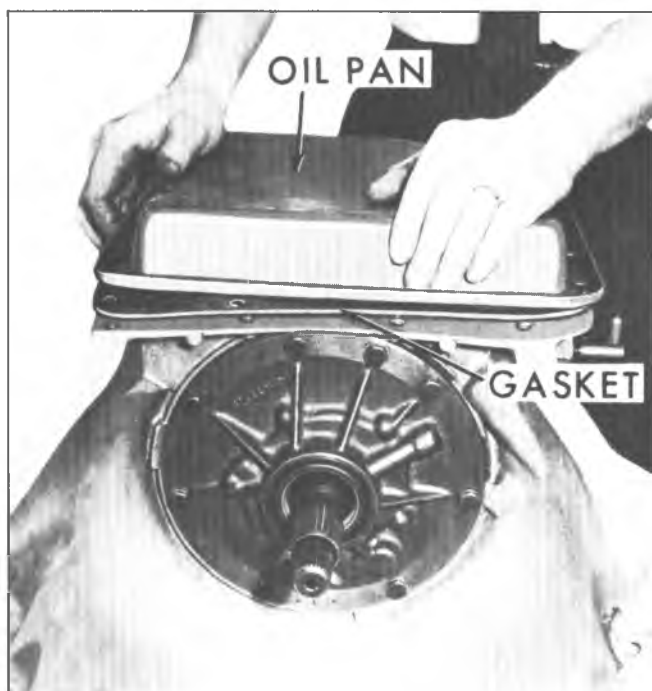
Fig. 9M--Removing Transmission Oil Pan
