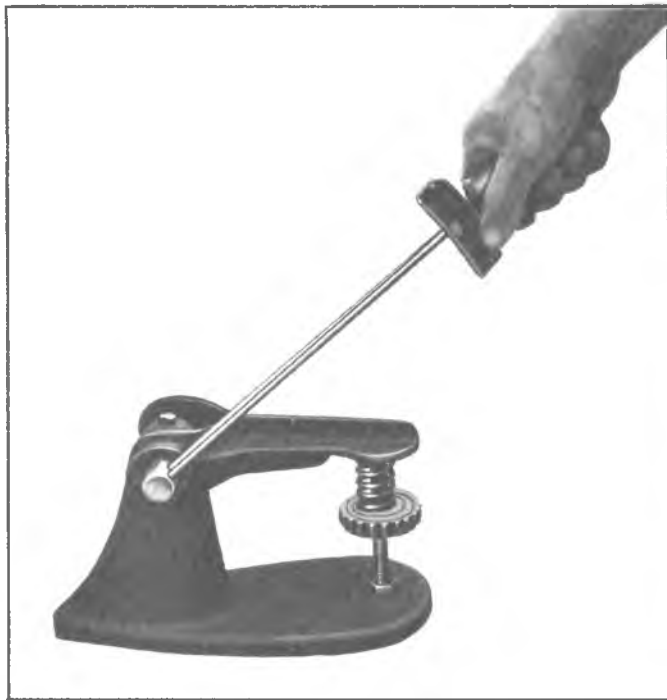
Fig. 17—Checking Valve Spring Tension
