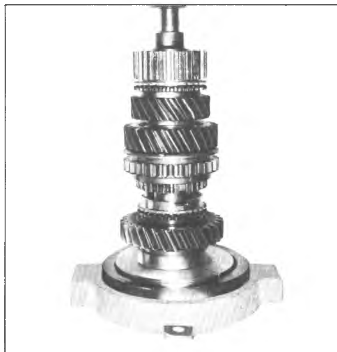
Fig. 17X--Installing Rear Bearing
