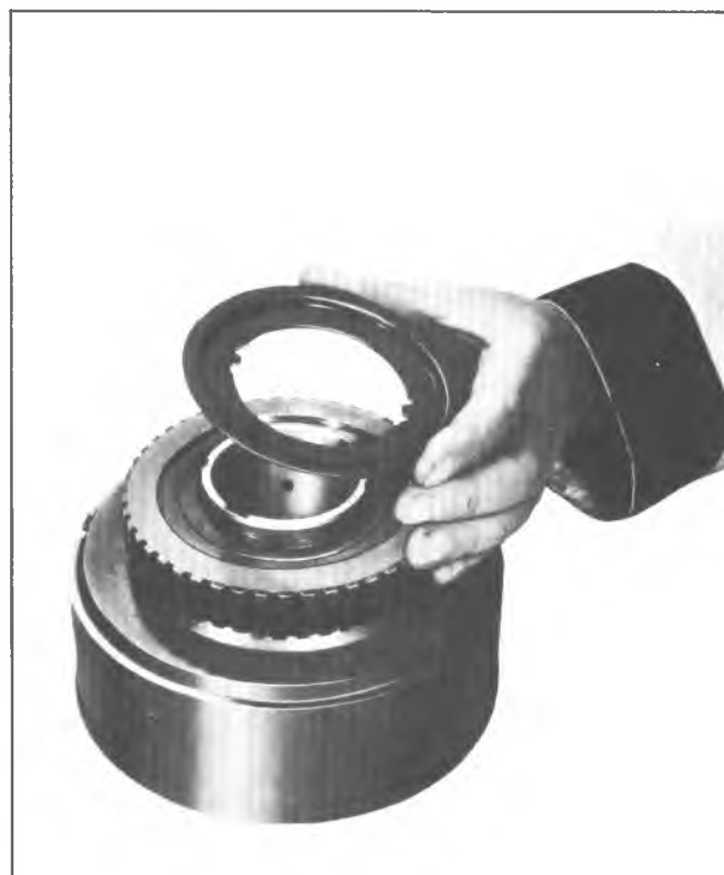
Fig. 94T--Installing Intermediate Clutch Retainer
