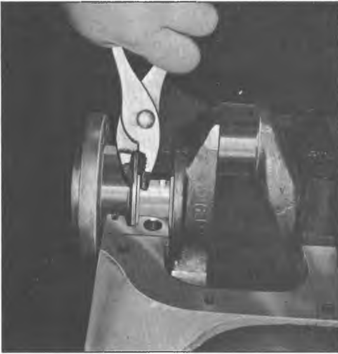
Fig. 42—Replacing Upper Main Bearing (In-Line)
