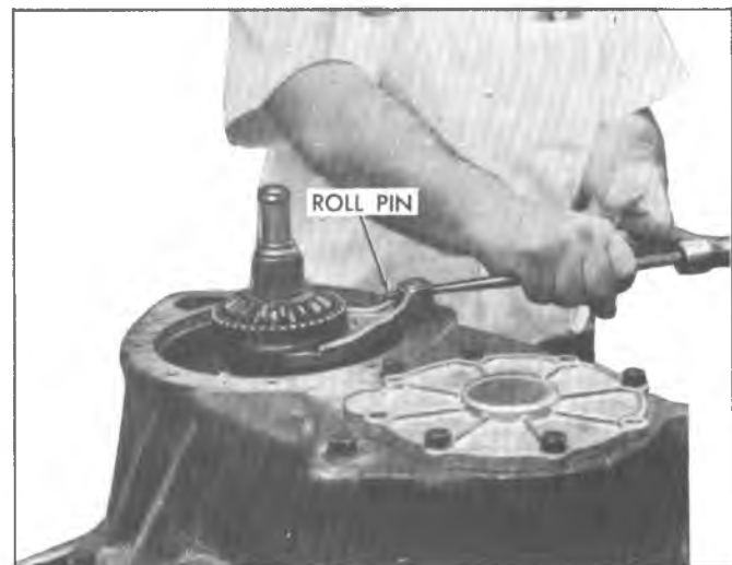
Fig. 9F—Removing Shift Fork Retaining Pin
