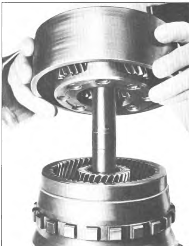
Fig. 121T--Installing Reaction Carrier
