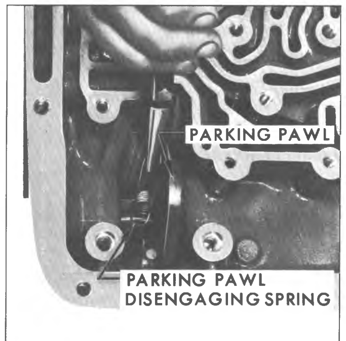
Fig. 23M--Removing Parking Pawl Disengaging Spring
