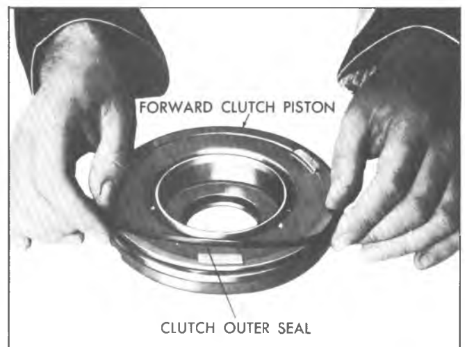
Fig. 71T--Removing Forward Clutch Piston Outer Seal
