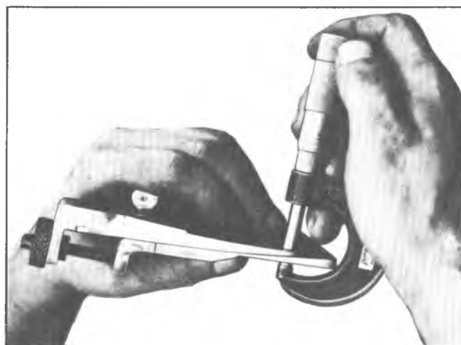
Fig. 10C—Measuring Gauge Plate Thickness
