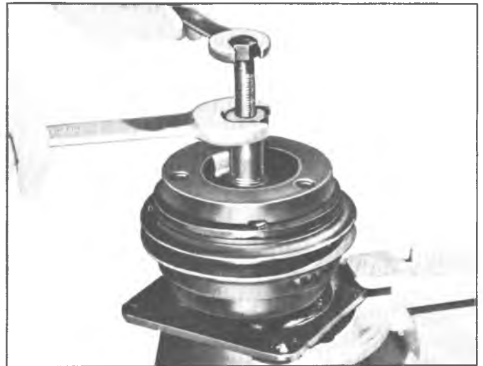
Fig. 3--Removing Hub and Drive Plate Assembly
