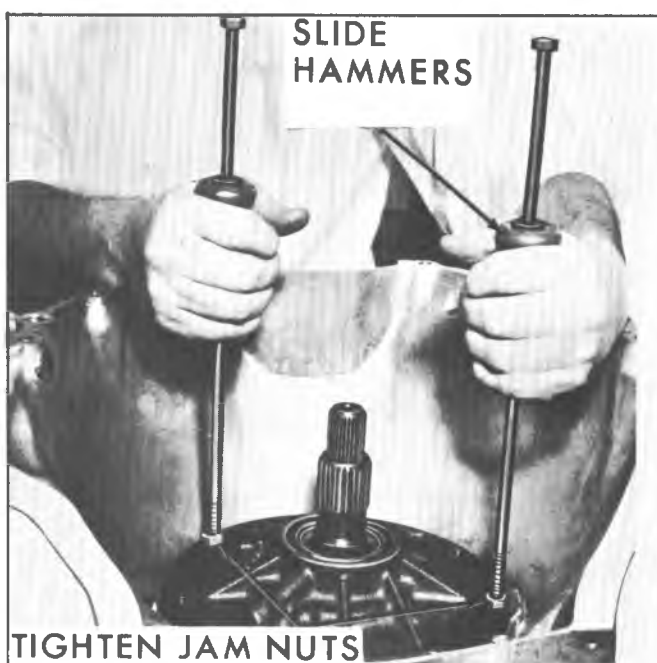
Fig. 27M--Removing Pump from Case
