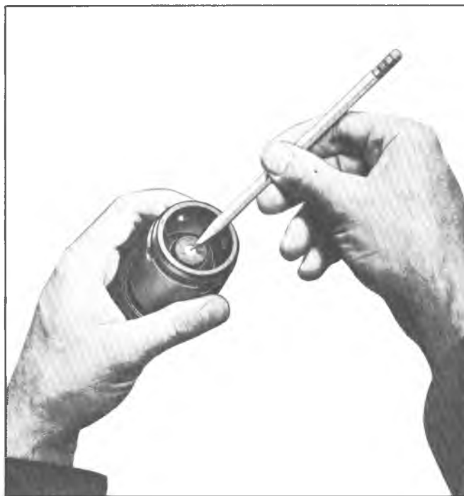
Fig. 7B--Removing Reaction Piston and Reaction Disc From Secondary Power Piston
