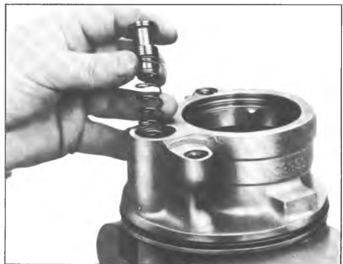
Fig. 30-Installing Flow Control Valve
