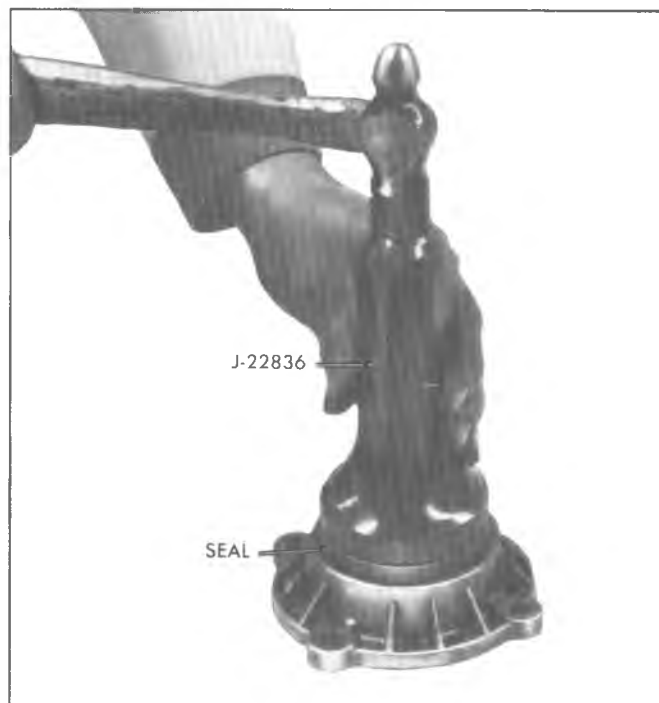
Fig. 16C--Installing Front Output Bearing Retainer Seal
