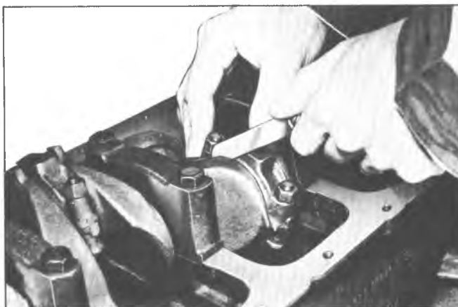
Fig. 45—Measuring Connecting Rod Side Clearance (In-Line)
