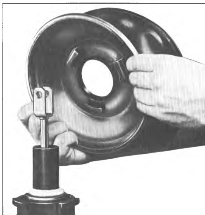
Fig. 11A--Installing Power Piston to Support Plate
