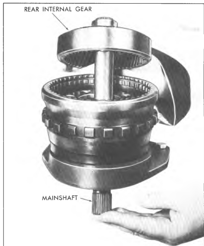
Fig. 44T--Removing Rear Internal Gear and Mainshaft
