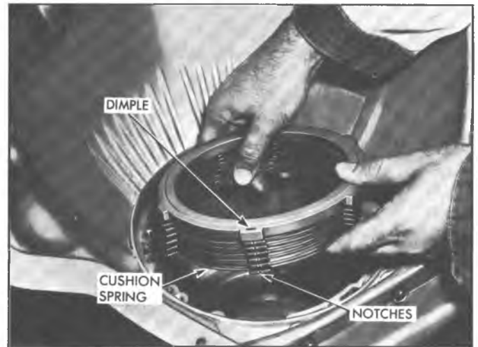
Fig. 30PG--Installing Clutch Plates (Typical)
