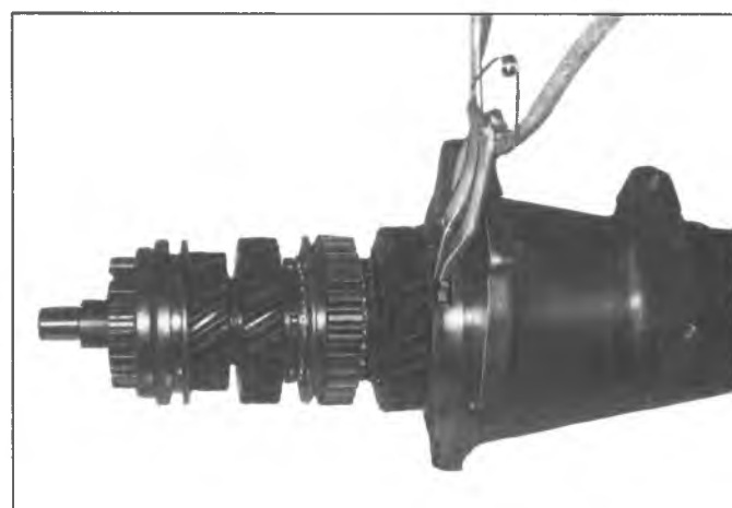
Fig. 4X--Extension to Rear Bearing Snap Ring
