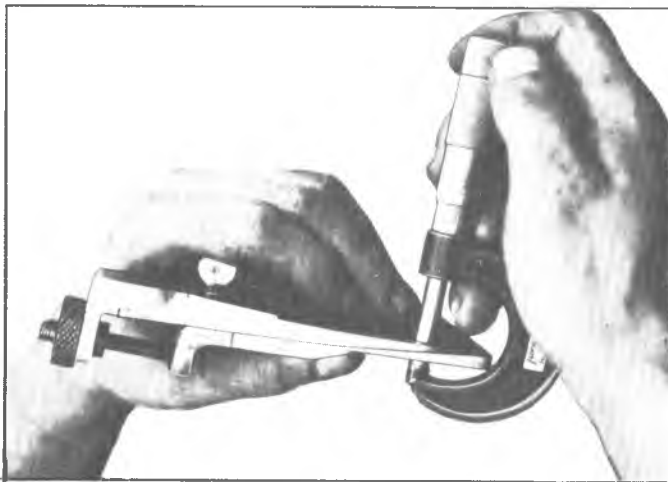
Fig. 8B—Measuring Gauge Plate Thickness
