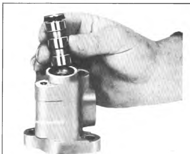
Fig. 65--Removing Spool from Housing
