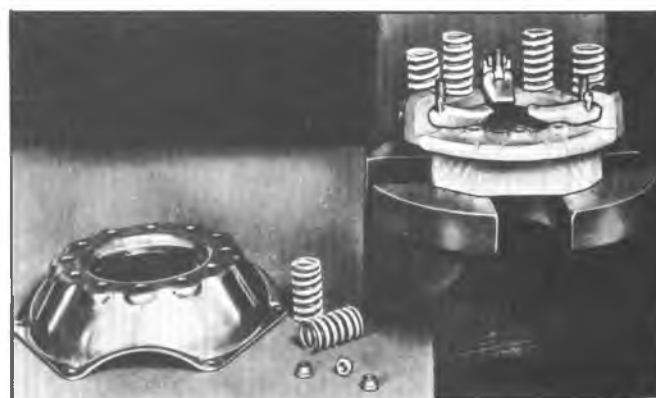
Fig. 3E--Disassembly of Clutch
