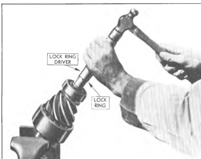
Fig. 5G—Pinion Rear Bearing Lock Ring Installation
