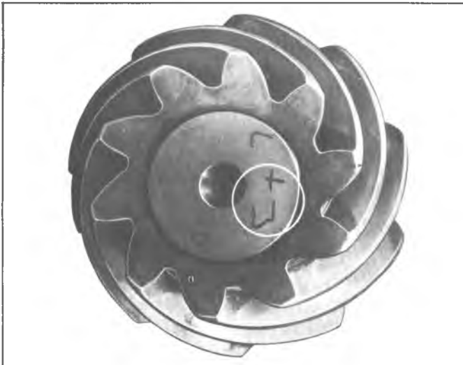
Fig. 10F—Pinion Code Location
