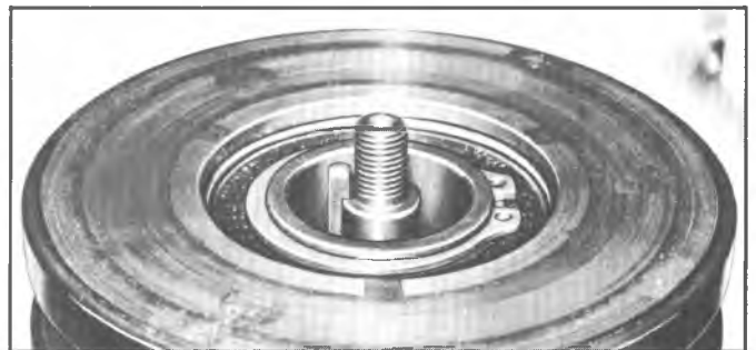
Fig. 4--Drive Plate Key Installed in Keyway
