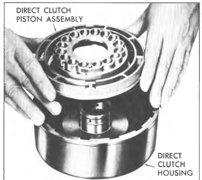
Fig. 82T--Removing Direct Clutch Piston Assembly
