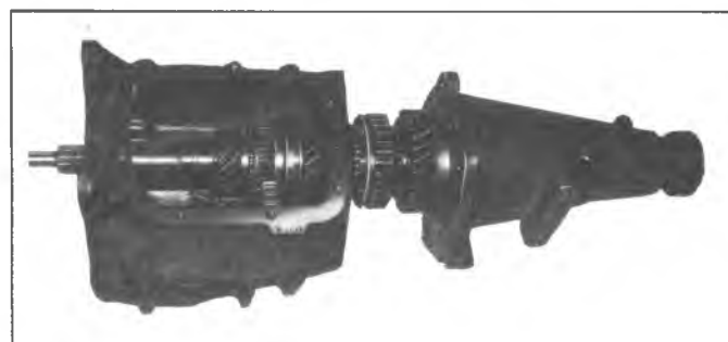
Fig. 3X--Removing Clutch Gear and Mainshaft
