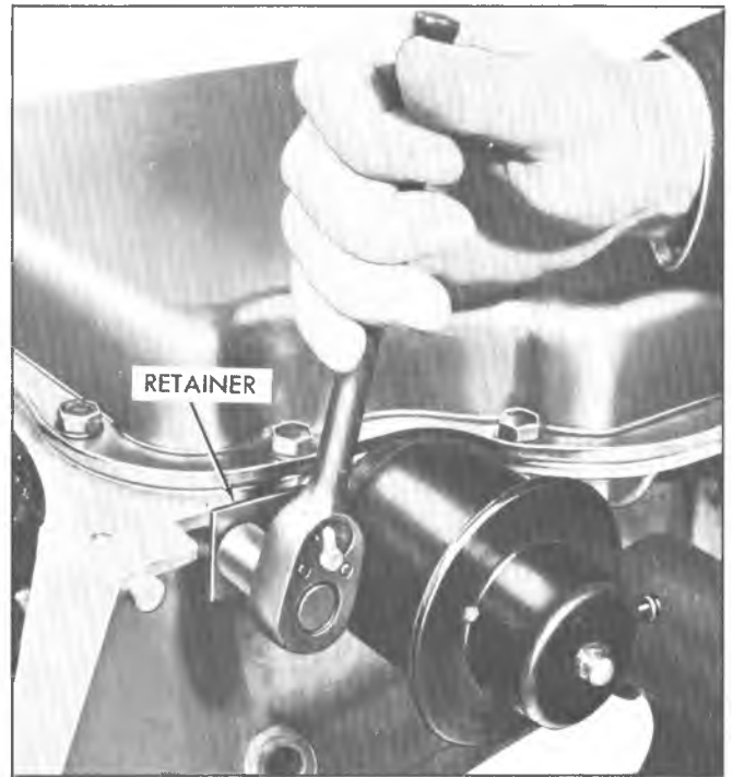
Fig. 3T--Removing Modulator Retainer
