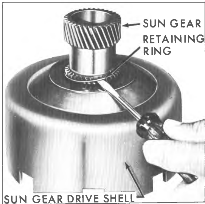
Fig. 86M--Removing Sun Gear Drive Shell Rear Retaining Ring
