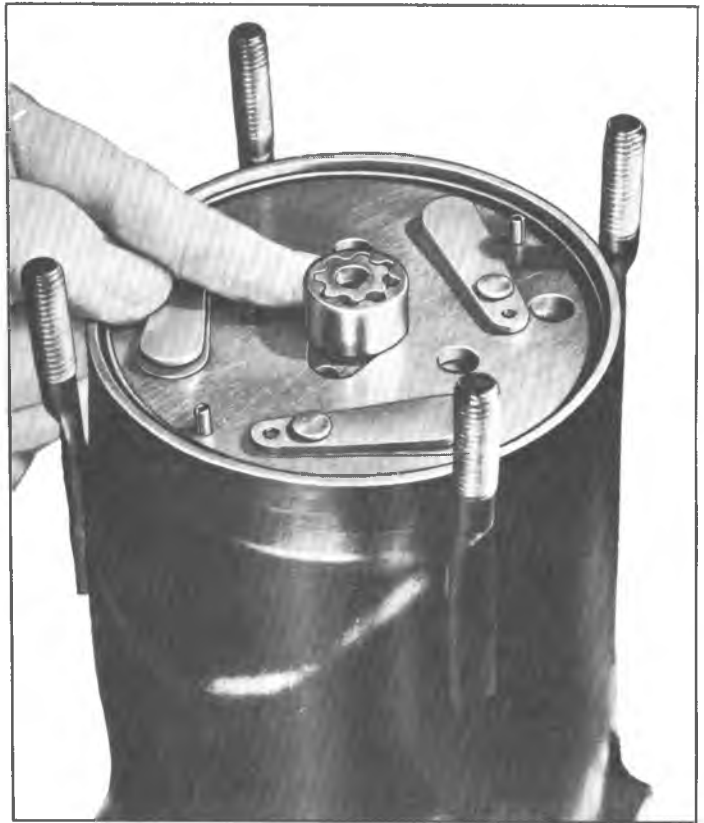
Fig. 15--Proper Oil Pump Gear Positioning
