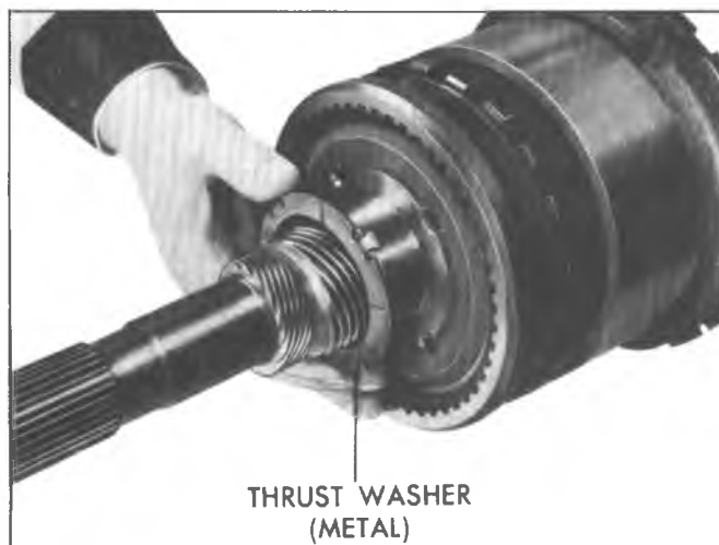
Fig. 126T--Installing Case to Output Shaft Thrust Washer
