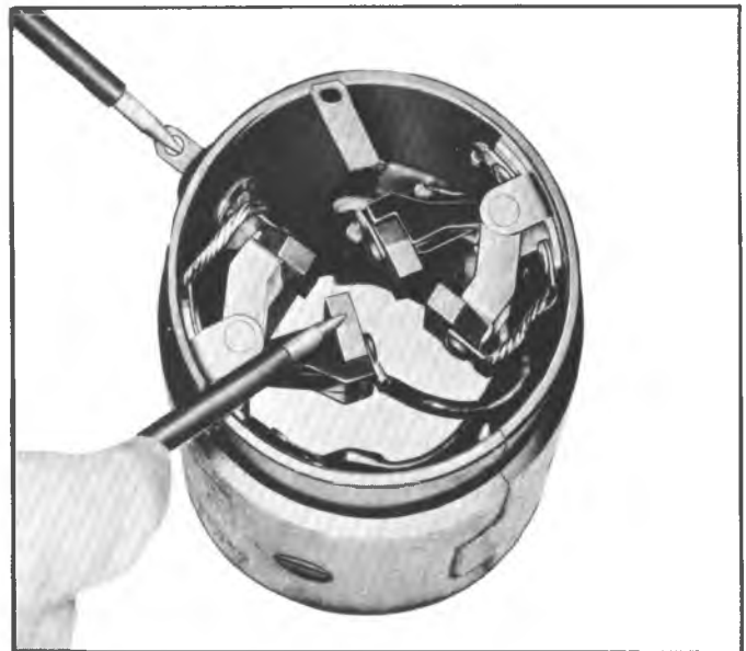
Fig. 6S--Field Coil Open Circuit Test
