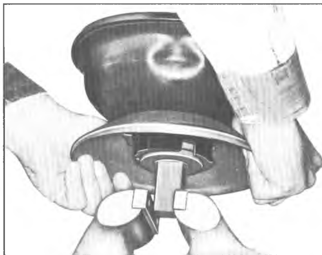
Fig. 7A--Separating Power Piston from Support Plate
