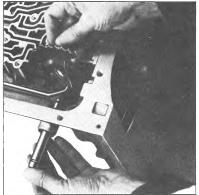
Fig. 134T--Installing Manual Shaft to Case
