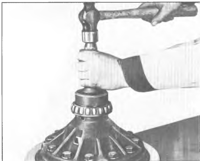
Fig. 8G—Differential Bearing Installation
