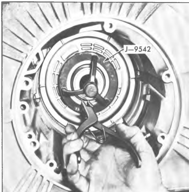
Fig. 8PG--Removing Rear Piston Spring Retainer Snap Ring
