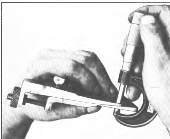
Fig. 8A—Measuring Gauge Thickness
