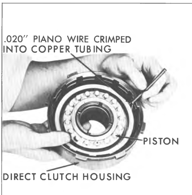
Fig. 75M--Installing Direct Clutch Piston
