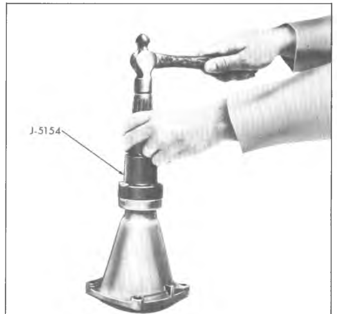
Fig. 106M--Installing Extension Housing Seal
