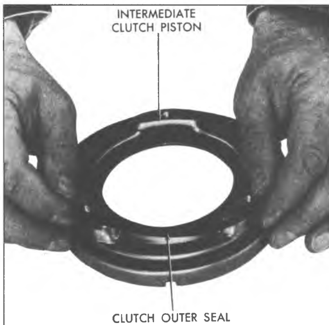
Fig. 101T--Installing Intermediate Clutch Outer Seal
