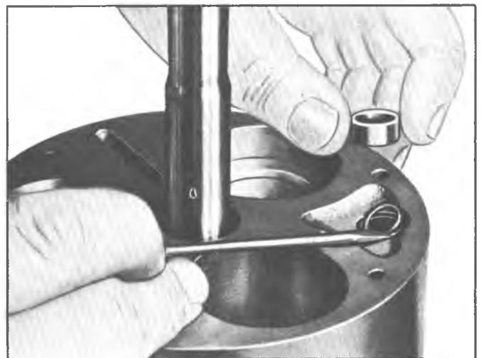
Fig. 26--Installing Discharge Crossover Tube Front "O" Ring and Spacer
