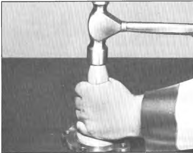
Fig. 4G—Pinion Oil Seal Installation
