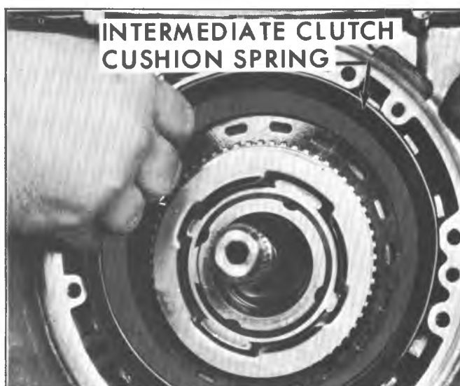
Fig. 28M--Removing Intermediate Clutch Cushion Spring
