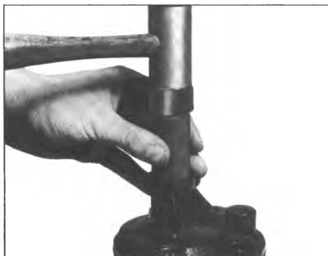
Fig. 21--Installing Seal Using Tool J-22670
