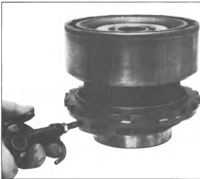
Fig. 96T--Air Checking Direct Clutch Assembly
