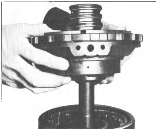
Fig. 125T--Installing Center Support to Reaction Carrier
