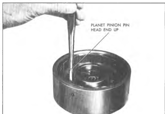
Fig. 109T--Installing Planet Pinion Pin
