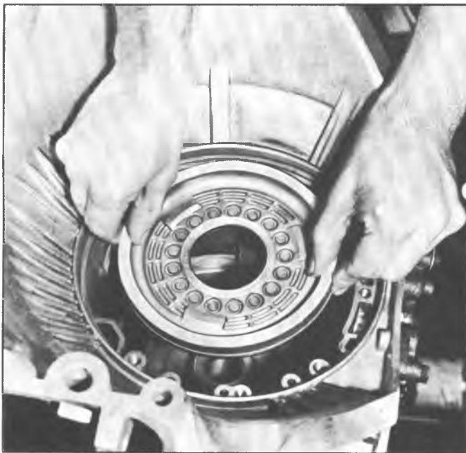
Fig. 29PG--Installing Reverse Piston
