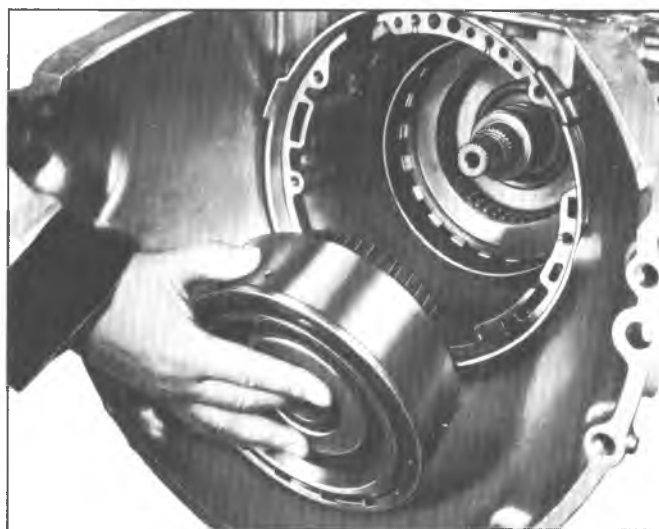
Fig. 29T--Removing Direct Clutch Assembly
