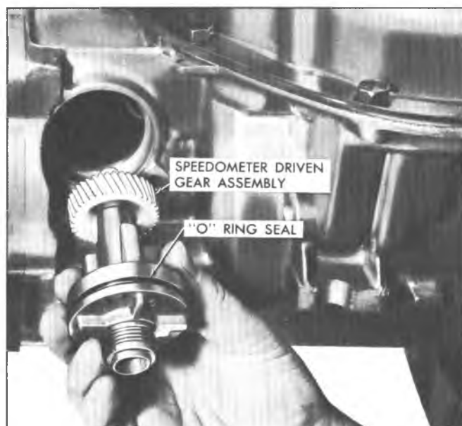
Fig. 155T--Installing Speedometer Driven Gear and Sleeve
