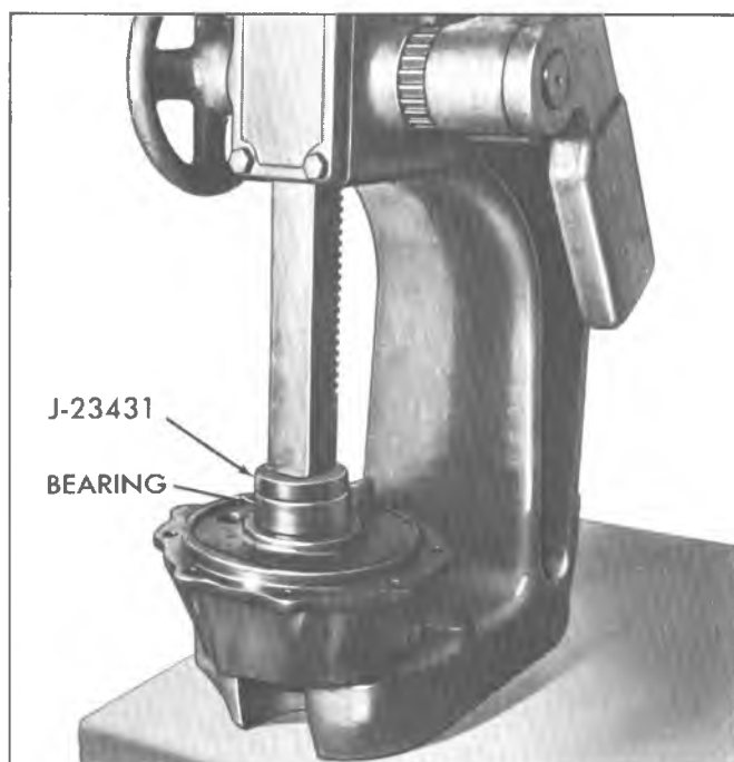
Fig. 17C--Installing Rear Output Shaft Housing Bearing
