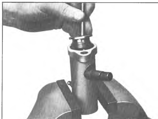
Fig. 72--Replacing Adjuster Plug and Shaft
