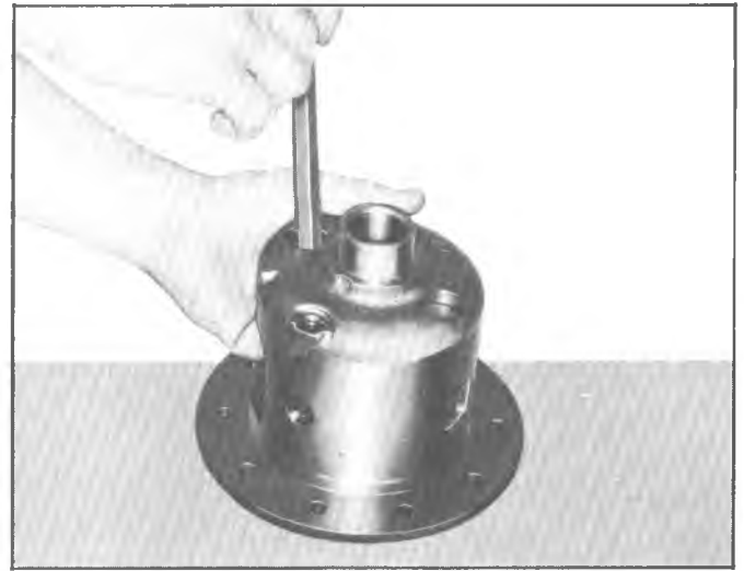
Fig. 9D—Removing Side Gear
