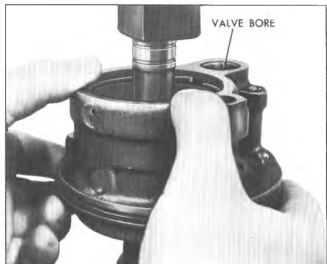
Fig. 29-Installing End Plate Retaining Ring
