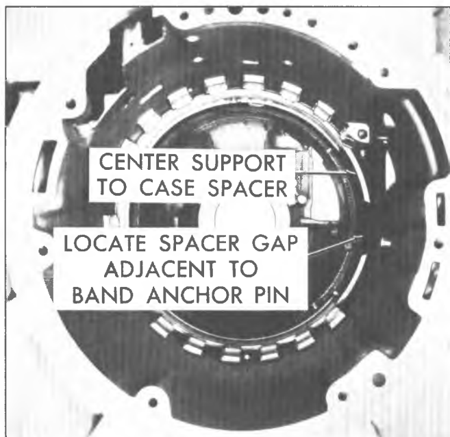
Fig. 37T-A--Removing Center Support to Case Spacer
