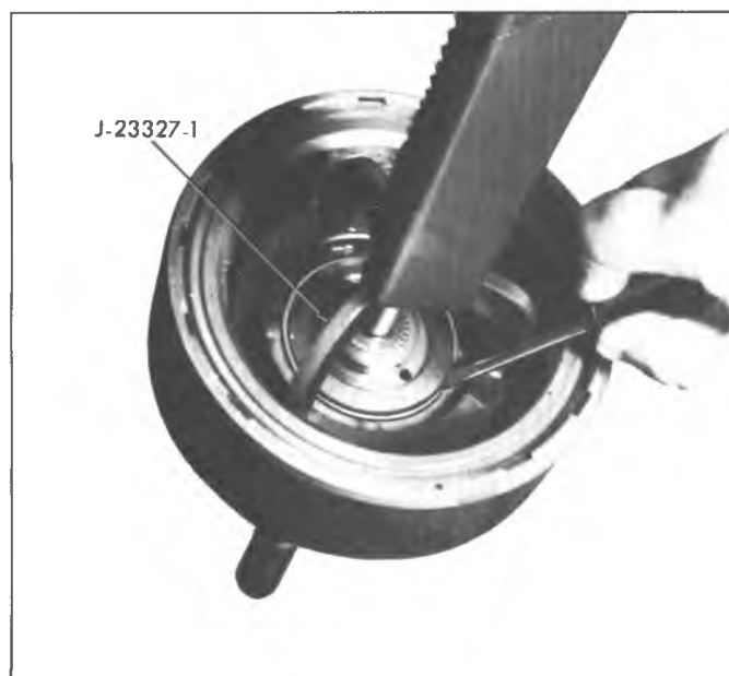
Fig. 80M--Compressing Forward Clutch Piston Return Seat
