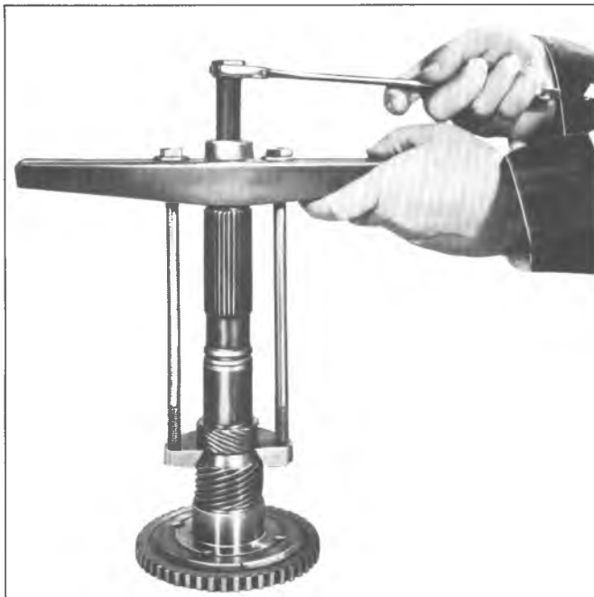
Fig. 47T-A--Removing Steel Speedometer Drive Gear
