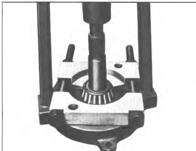
Fig. 15A—Removing Drive Pinion Rear Bearing.
