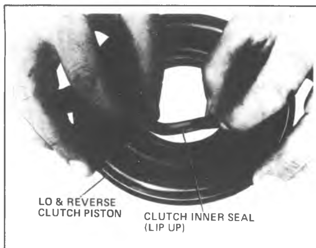
Fig. 7A-79A—Removing or Installing Low and Reverse Clutch Inner Seal
