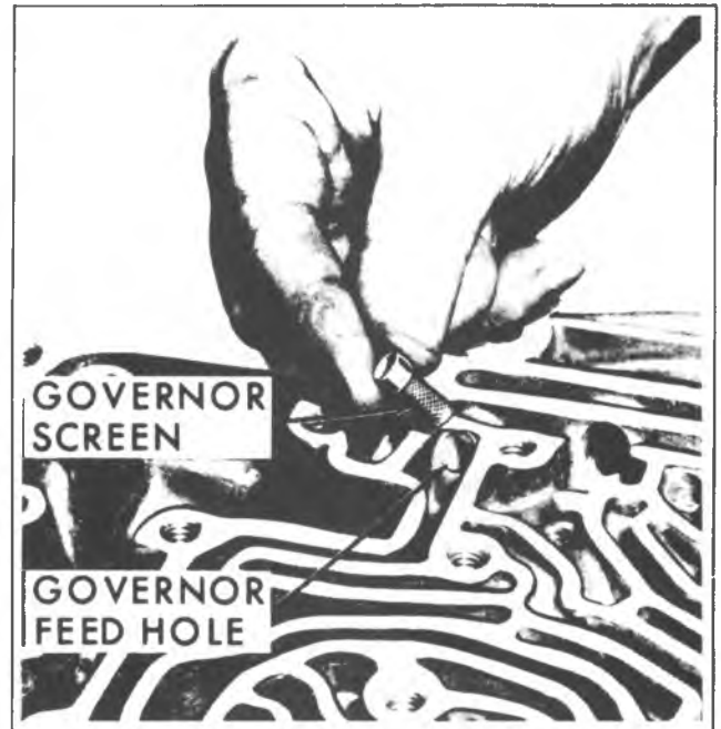
Fig. 7A-20B--Removing Governor Feed Screen
