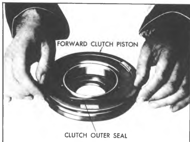
Fig. 7A-84C--Removing Forward Clutch Piston Outer Seal
