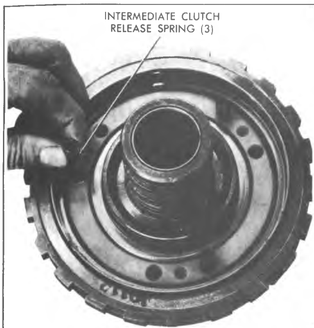
Fig. 7A-123C--Installing Intermediate Clutch Release Springs
