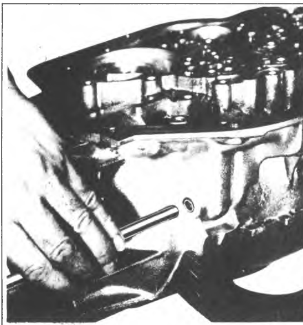
Fig. 7A-154C--Installing Parking Pawl Shaft Cup Plug
