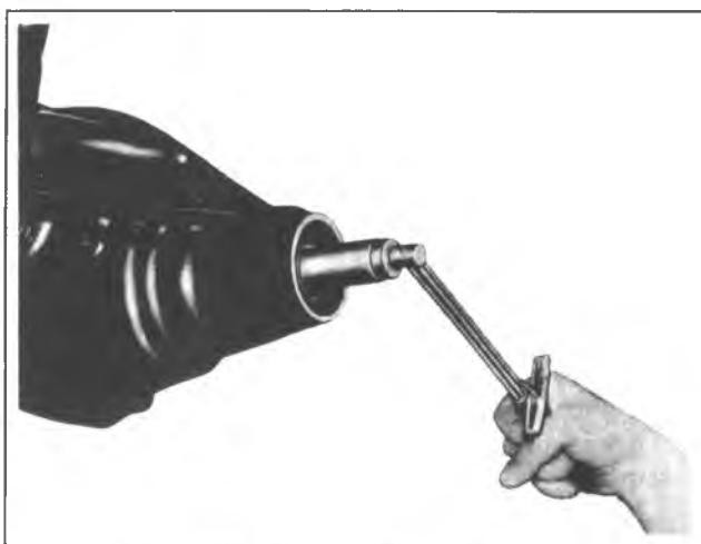
Fig. 19B—Measuring Rotating Torque
