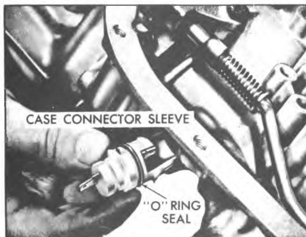
Fig. 7A-19C--Removing Electrical Connector and "O" Ring Seal
