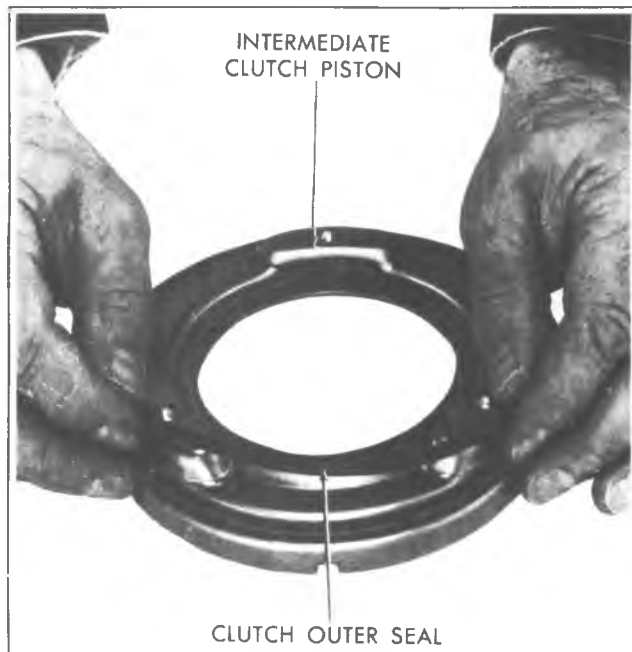
Fig. 7A-120C--Installing Intermediate Clutch Outer Seal
