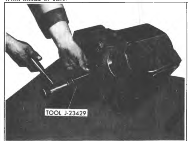
Fig. 7D-8R—Removing Idler Gear Shaft
