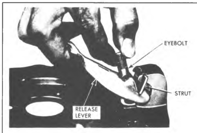
Fig. 7C-5E-Removing or Installing Lever
