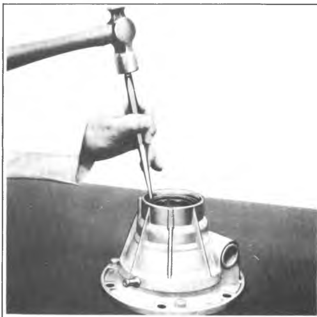
Fig. 7D-18S—Removing Rear Output Shaft Front Bearing
