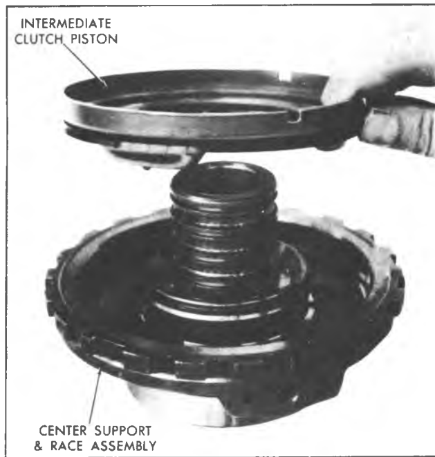
Fig. 7A-117C--Removing Intermediate Clutch Piston
