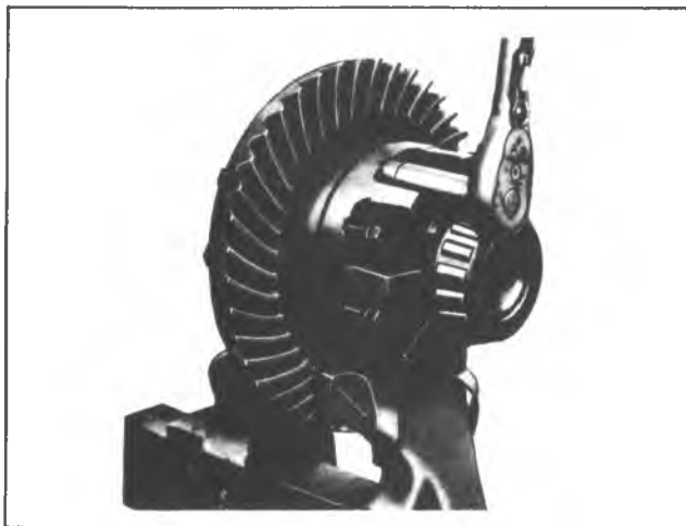
Fig. 3F—Separating Case Halves
