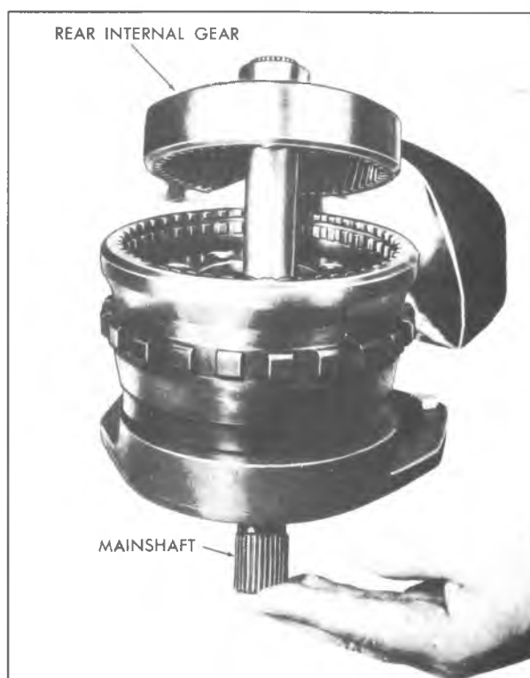
Fig. 7A-51C--Removing Rear Internal Gear and Mainshaft
