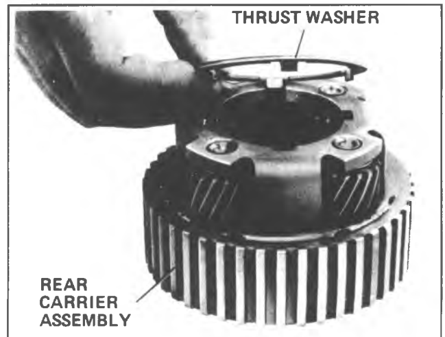
Fig. 7A-38A—Removing Thrust Washers
