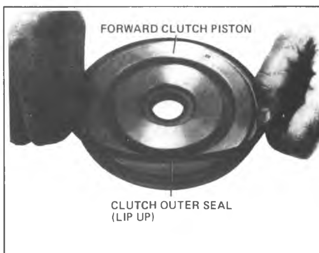
Fig. 7A-114A-Removing or Installing Outer Piston Seal
