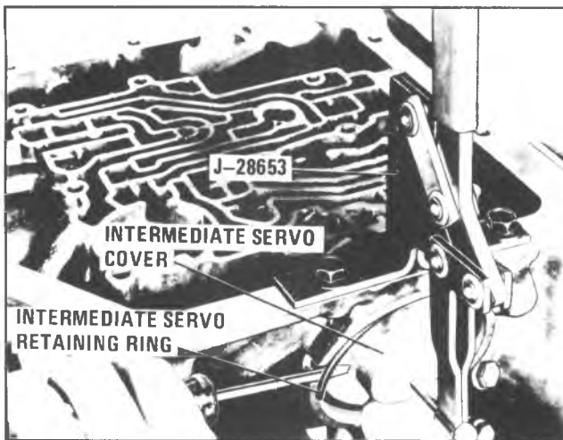
7A-150A--Installing Retaining Ring
