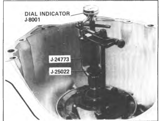
Fig. 7A-19A—Checking Front Unit End Play
