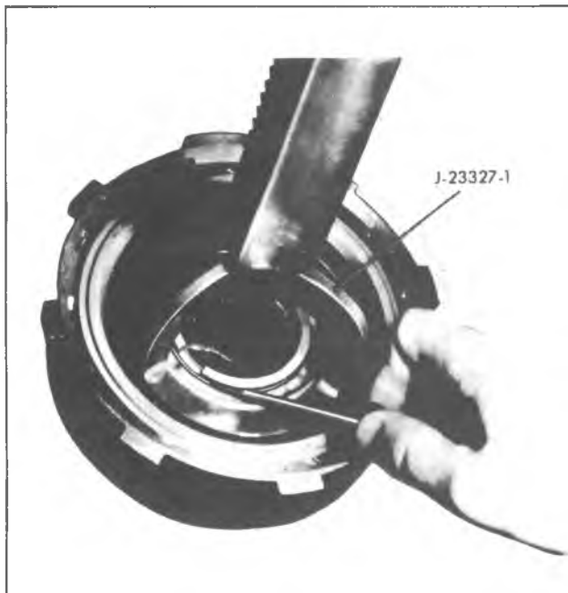
Fig. 7A-76B--Removing Direct Clutch Outer and Inner Seals
