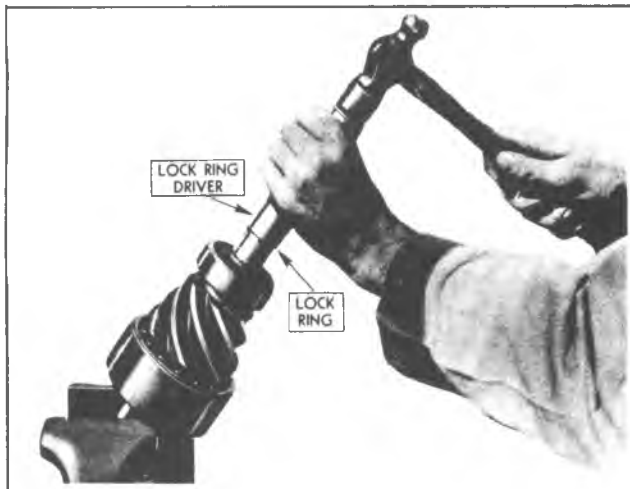
Fig. 5G-Pinion Rear Bearing Lock Ring Installation
