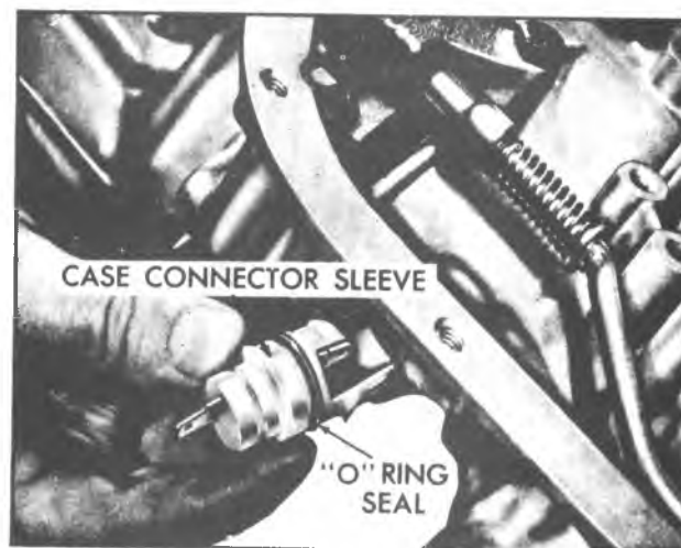
Fig. 7A-178C--Installing Electrical Connector and "O" Ring Seal
