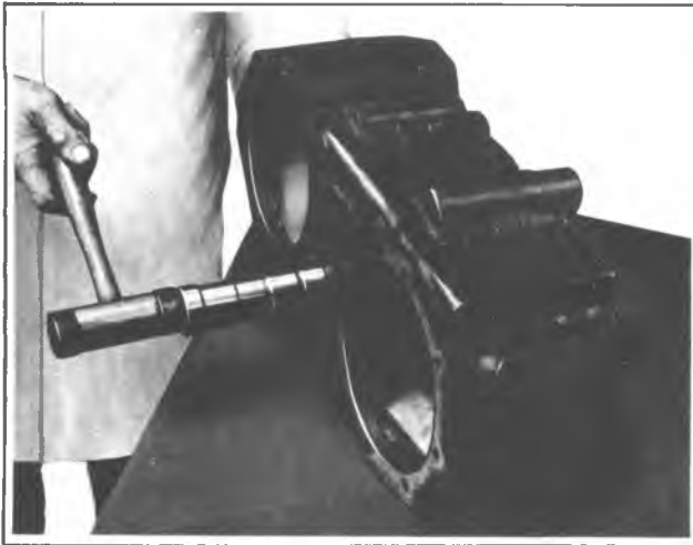
Fig. 7D-13R--Installing Idler Shaft
