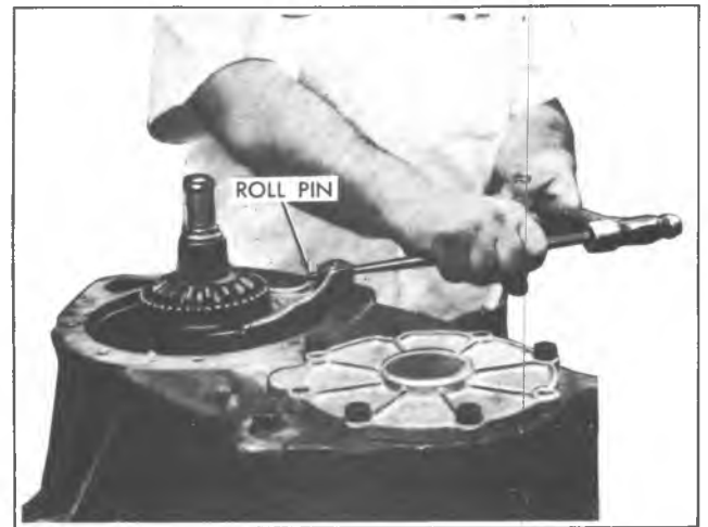
Fig. 7D-6S-Removing Shift Fork Retaining Pin
