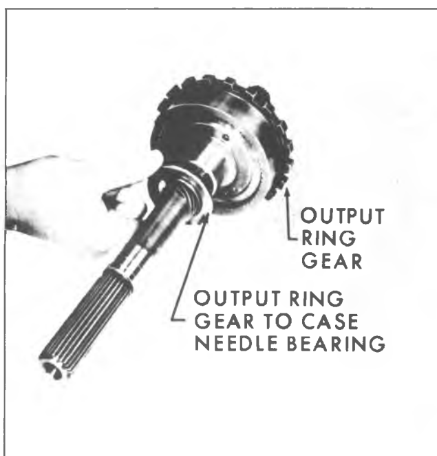
Fig. 7A-47B--Removing Output Ring Gear to Case Needle Bearing Assembly
