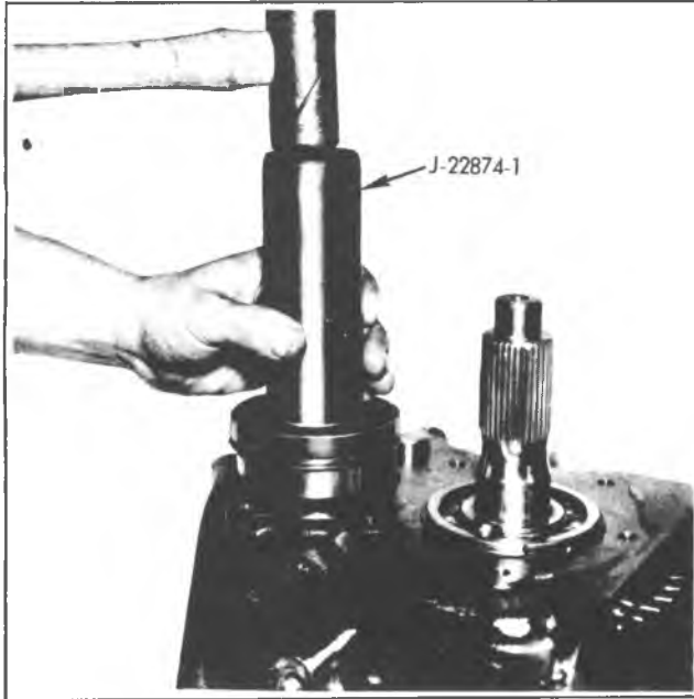
Fig. 7B-25L--Installing Countergear Rear Bearing
