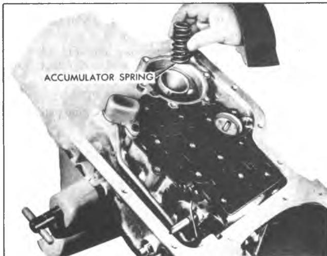
Fig. 7A-180C--Installing Rear Accumulator Spring
