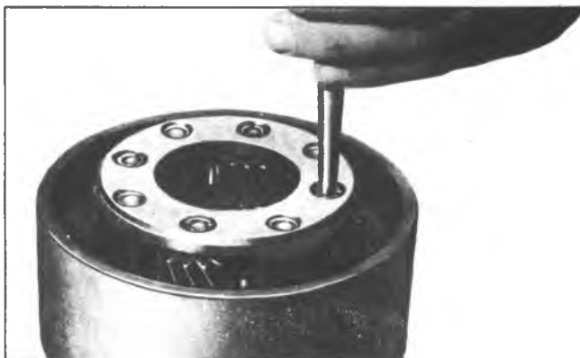
Fig. 7A-130C--Removing Planet Pinion Pin
