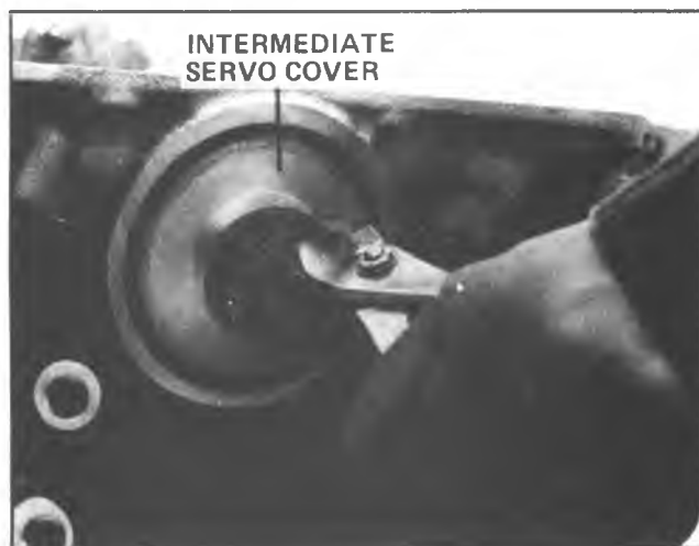
Fig. 7A-13A—Removing Intermediate Servo Cover
