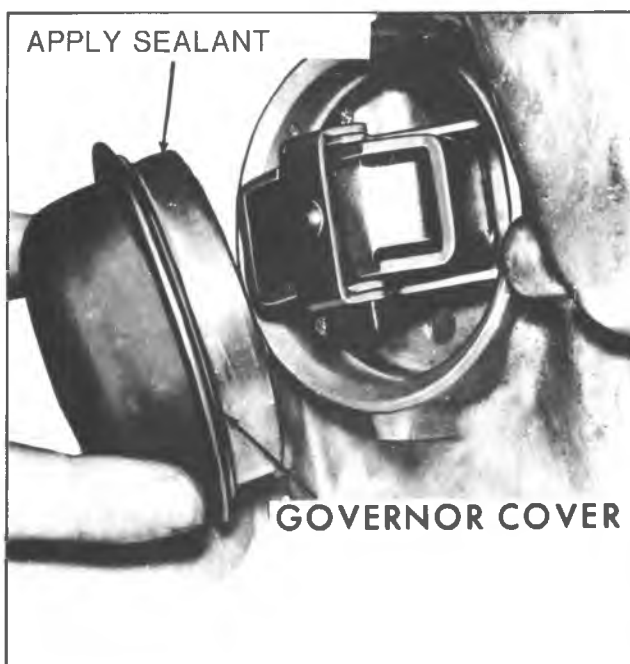
Fig. 7A-10B--Governor Cover and "O" Ring Seal
