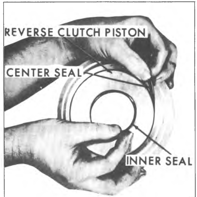
Fig. 7A-52B--Removing Low and Reverse Clutch Piston Center and Inner Seal
