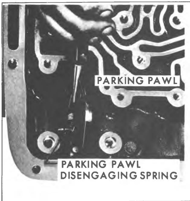
Fig. 7A-26B--Removing Parking Pawl Disengaging Spring
