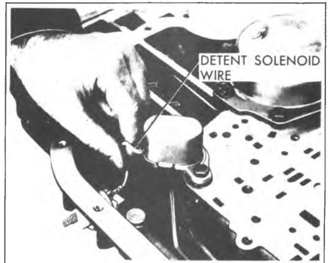
Fig. 7A-12C--Disconnecting Detent Solenoid Wire
