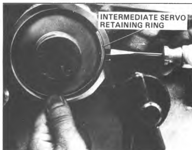
Fig. 7A-12A—Removing Retaining Ring
