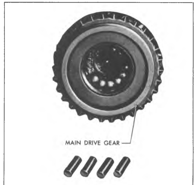
Fig. 7B-17A—Loading Pilot Bearings
