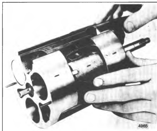
Figure 1D-61 Installing A-6 Suction Cross-over Cover
