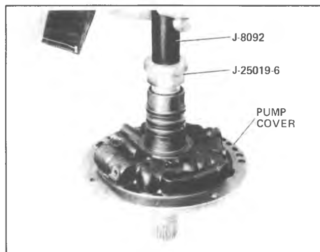
Fig. 7A-171A—Installing Pump Cover Bushing - Rear
