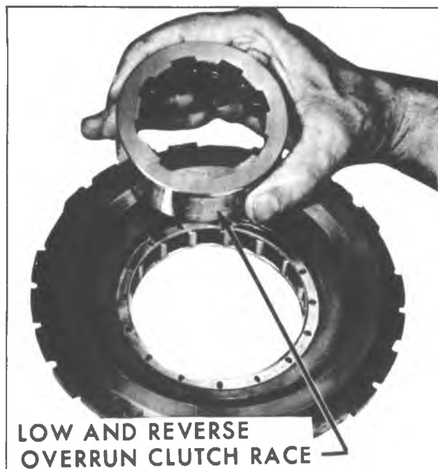
Fig. 7A-94B--Removing Overrun Clutch Inner Race
