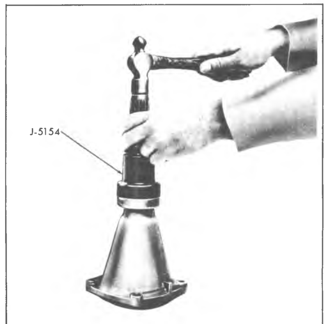
Fig. 7A-110B—Installing Extension Housing Seal
