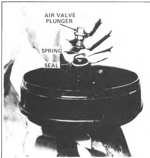
Fig. 5-10B—Installing Air Valve Plunger
