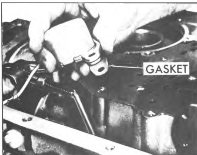
Fig. 7A-18C--Removing Detent Solenoid and Gasket
