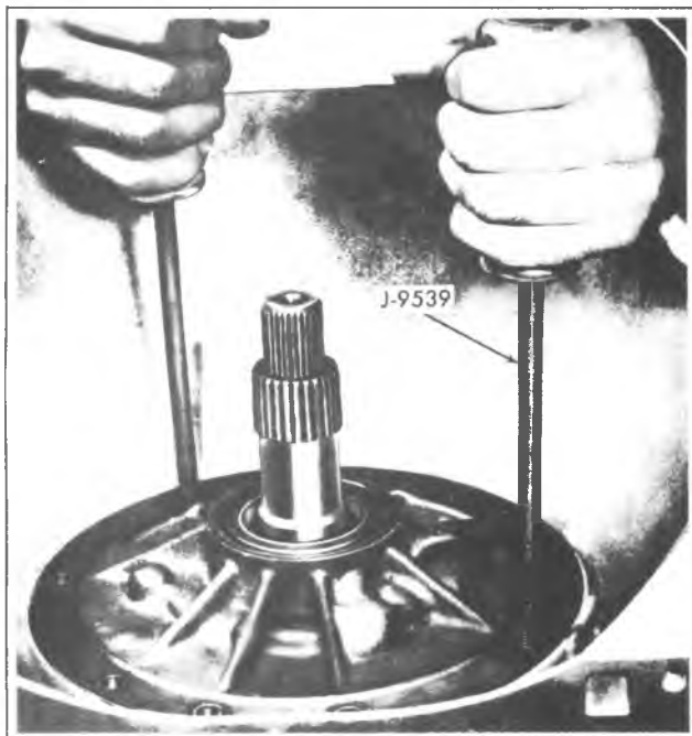
Fig. 7A-32C--Removing Pump Assembly
