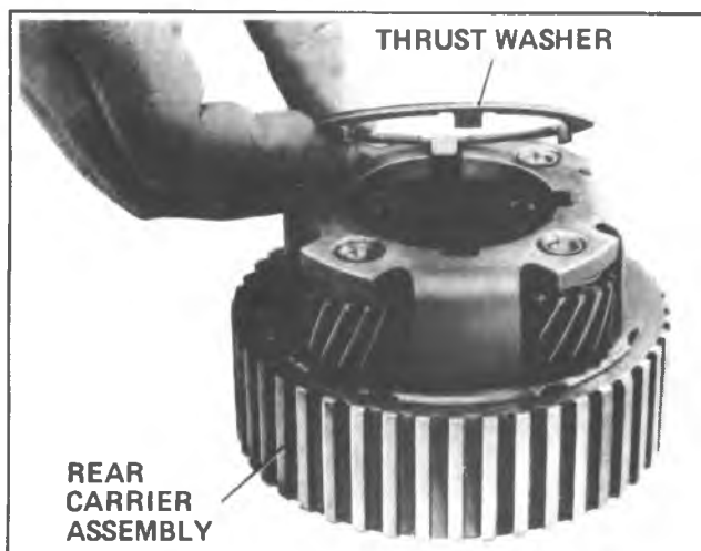
Fig. 7A-71A-Installing Thrust Washer
