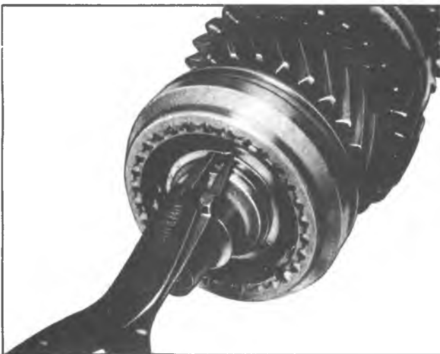
Fig. 7B-7A--Removing 2nd-3rd Clutch Hub Retaining Ring
