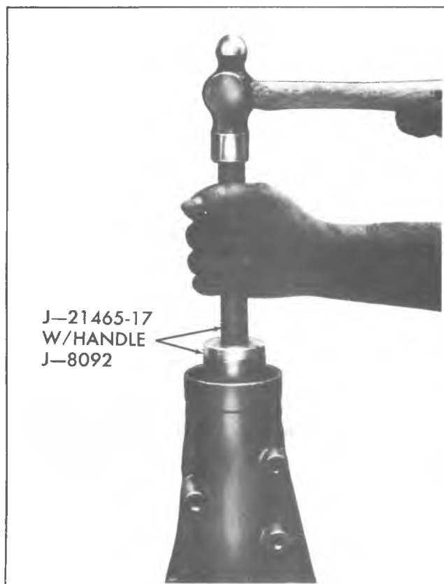
Fig. 7B-14K--Removing Rear Extension Bushing
