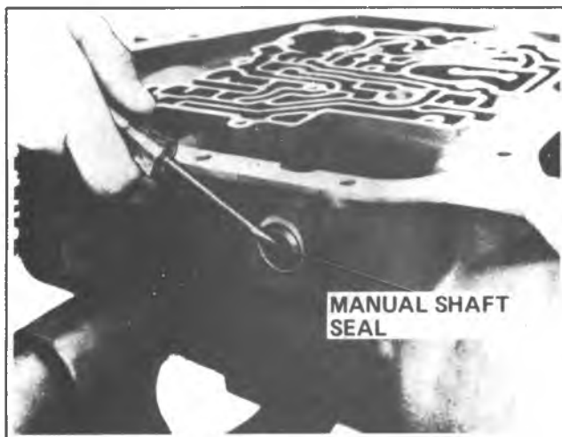
Fig. 7A-44A—Removing Manual Shaft Seal From Case
