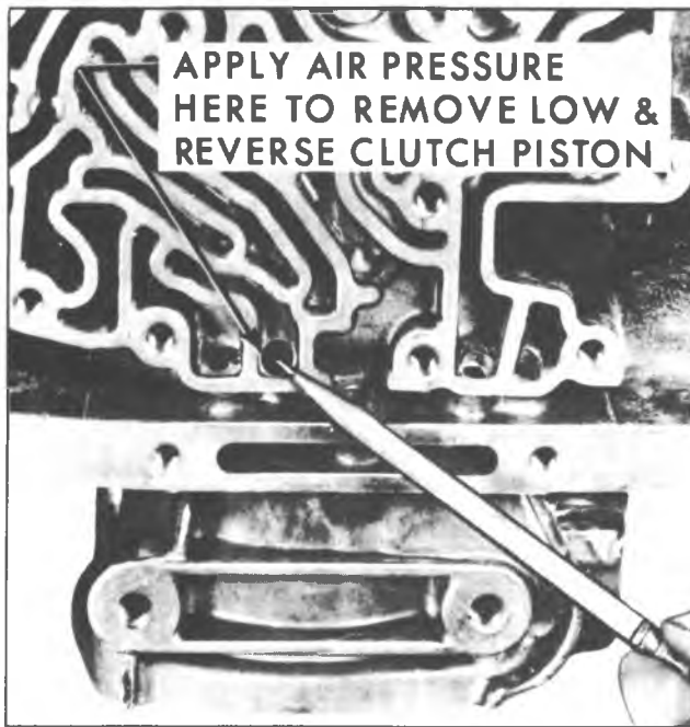
Fig. 7A-50B--Removing Low and Reverse Clutch Piston
