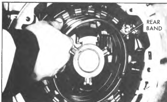
Fig. 7A-156C--Installing Rear Band
