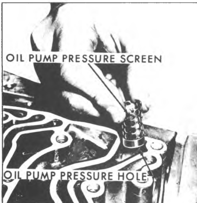
Fig. 7A-19B--Removing Oil Pump Pressure Screen
