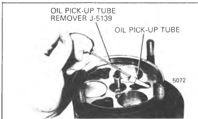
Figure 1D-33 Removing A-6 Oil Pick-Up Tube
