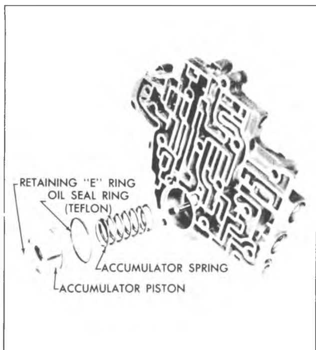
Fig. 7A-66C--Front Accumulator Assembly - Exploded View
