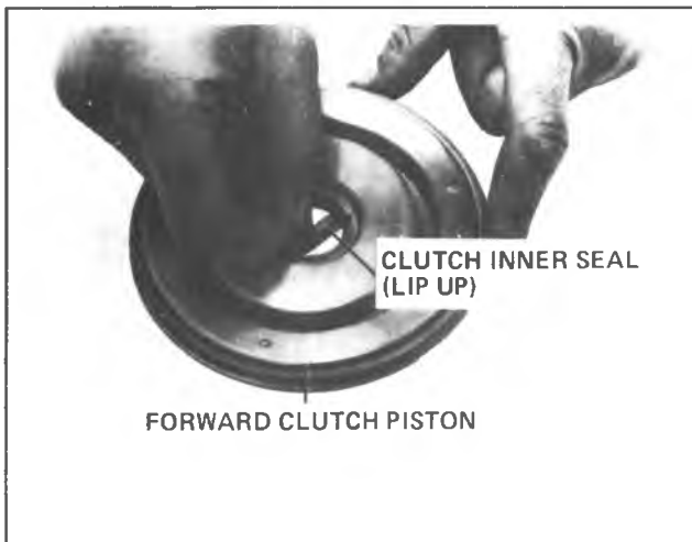
Fig. 7A-115A--Removing or Installing Inner Piston Seal
