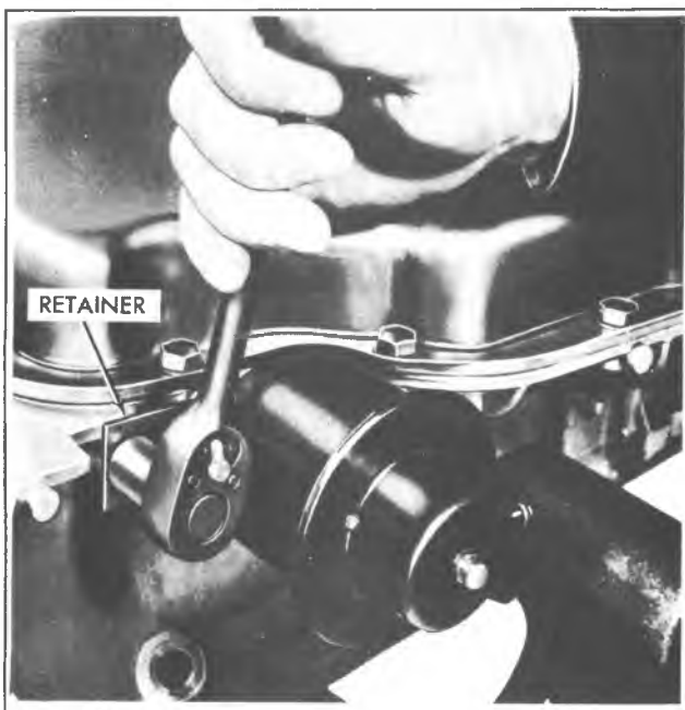
Fig. 7A-3C--Removing Modulator Retainer
