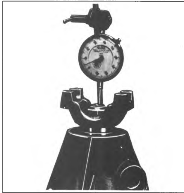
Fig. 7D-24S--Checking Rear Output Shaft End Play
