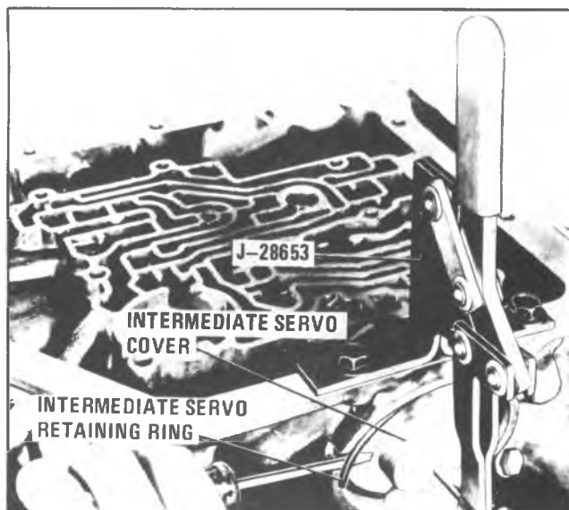
Fig. 7A-11A—Depressing Servo Cover
