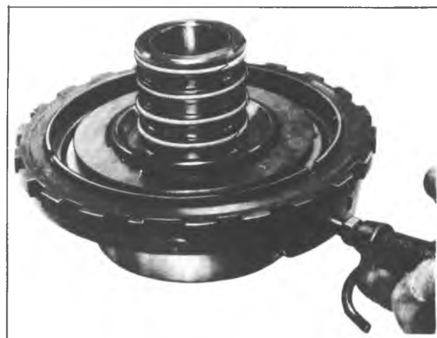
Fig. 7A-126C--Air Checking Intermediate Clutch Piston
