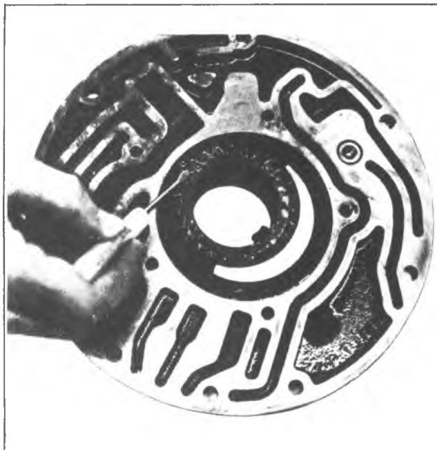
Fig. 7A-66B--Installing Pump Drive and Driven Gears
