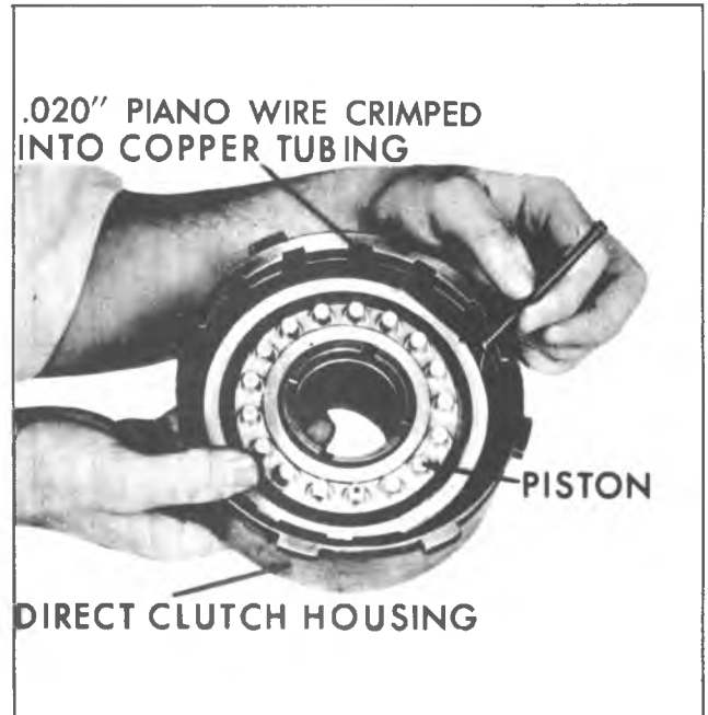
Fig. 7A-78B--Installing Direct Clutch Piston
