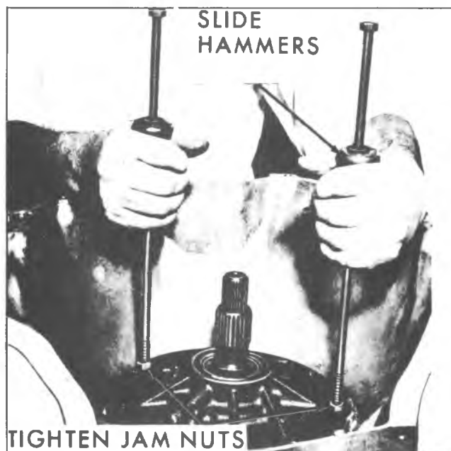
Fig. 7A-30B--Removing Pump from Case
