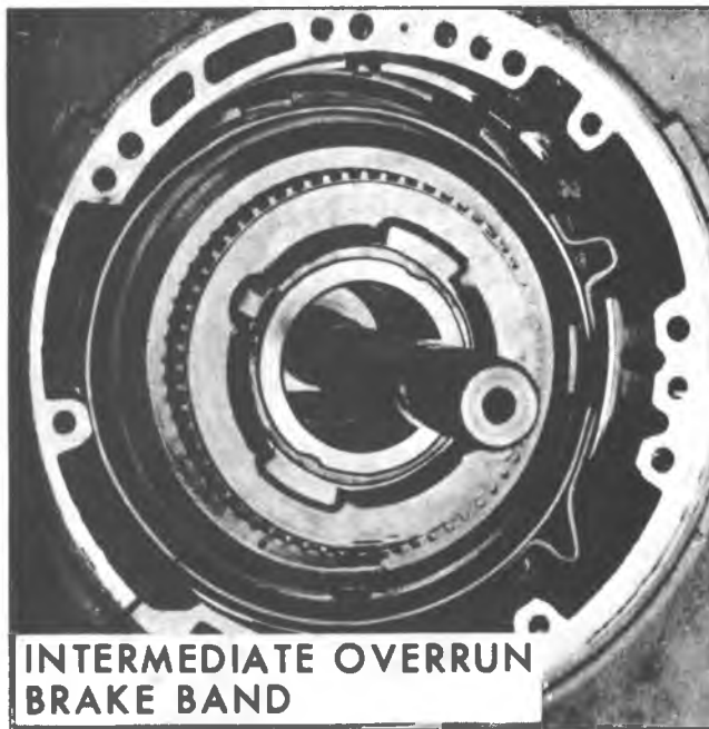
Fig. 7A-34B--Removing Intermediate Overrun Brake Band
