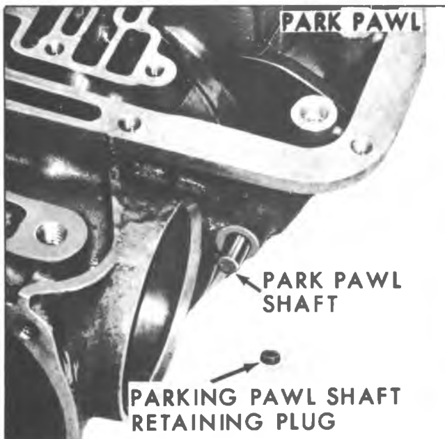
Fig. 7A-27B--Parking Pawl Shaft Retaining Plug, Parking Pawl Shaft and Parking Pawl
