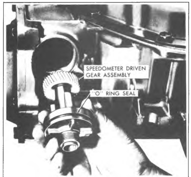
Fig. 7A-188C--Installing Speedometer Driven Gear and Sleeve
