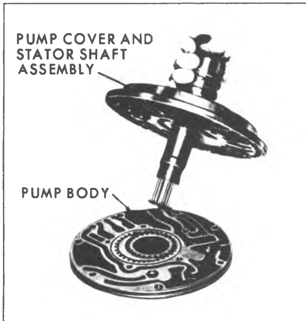
Fig. 7A-62B--Separating Pump Cover From Pump Body
