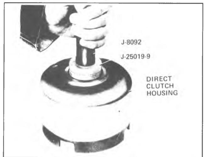
Fig. 7A-175A-Installing Direct Clutch Housing Bushing - Front
