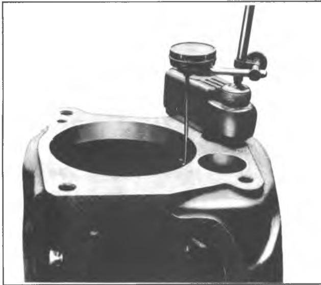
Fig. 7B-20K—Checking Countergear End Play
