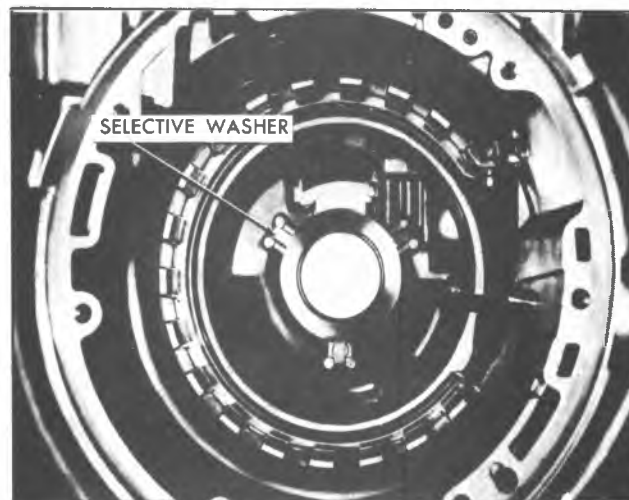
Fig. 7A-43C--Removing Selective Washer
