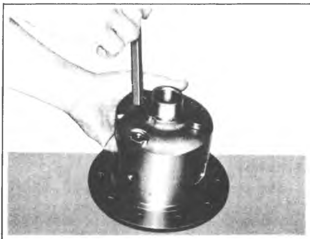
Fig. 8D-Removing Side Gear
