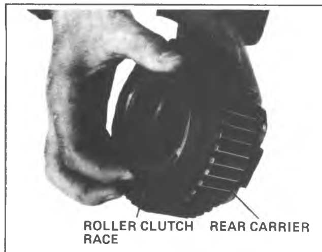
Fig. 7A-70A-Installing Roller Clutch Race
