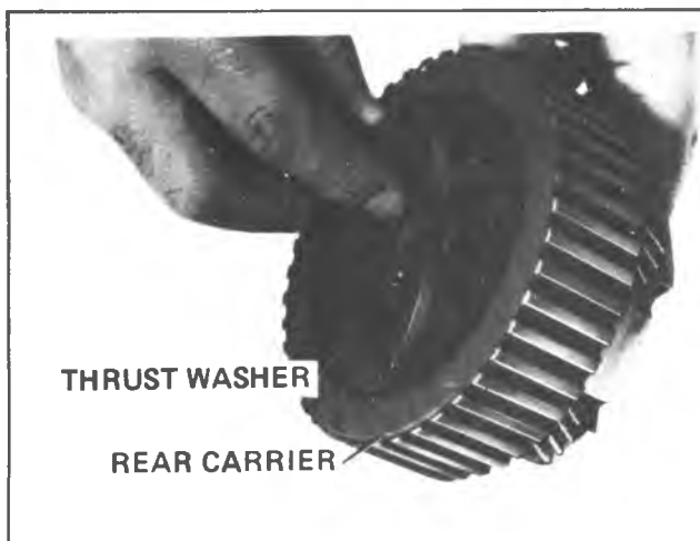
Fig. 7A-67A-Installing Thrust Washer Into Rear Carrier
