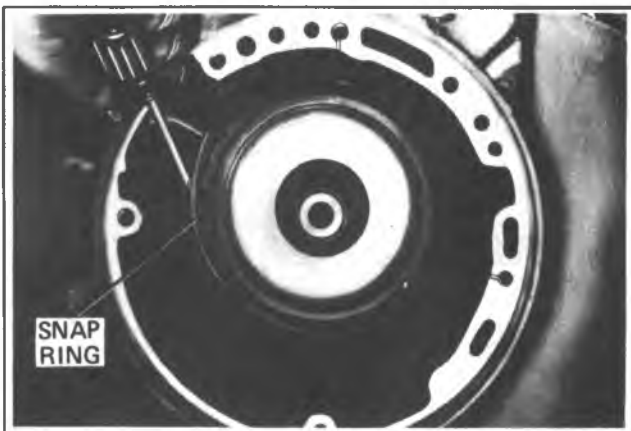
Fig. 7A-34A--Removing Low and Reverse Housing to Case Snap Ring
