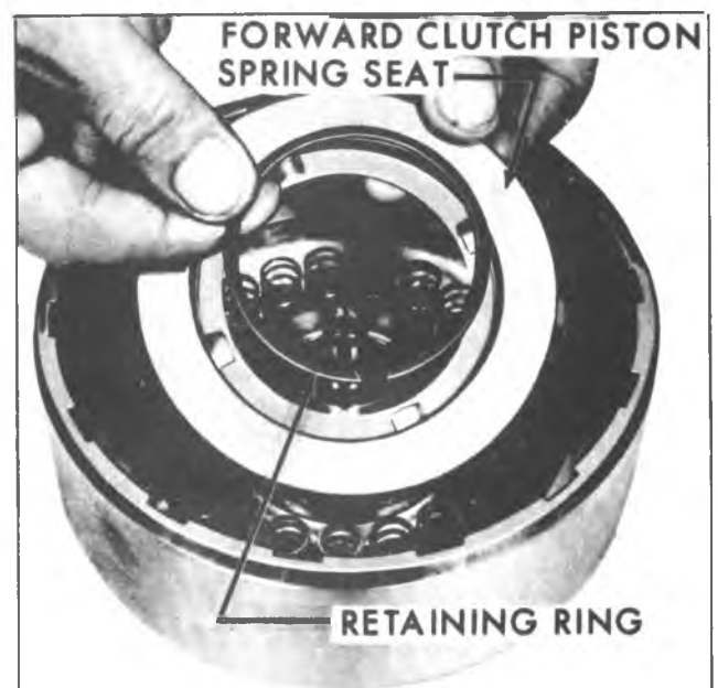
Fig. 7A-79B--Installing Direct Clutch Springs, Spring Seat and Retaining Ring
