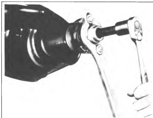
Fig. 13B-Drive Pinion Flange Removal
