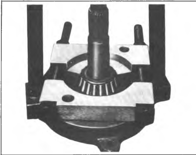
Fig. 18F--Removing Inner Pinion Bearing Cone and Roller
