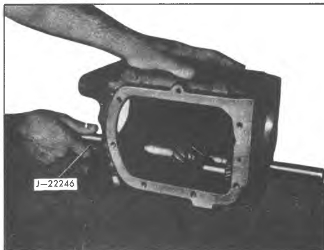
Fig. 7B-5A—Removing Counter Gear Shaft
