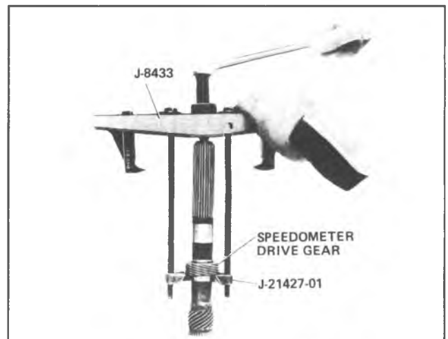
Fig. 7A-60A-Removing Steel Gear
