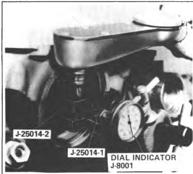
Fig. 7A-16A—Checking for Proper Intermediate Band Apply Pin
