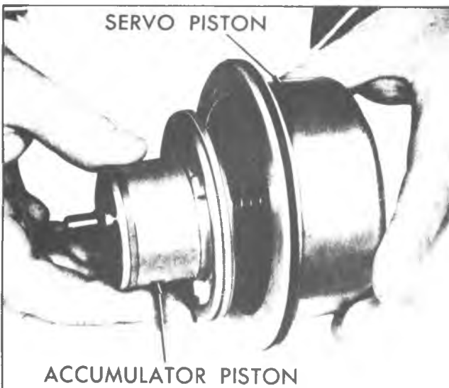
Fig. 7A-62C--Removing Rear Accumulator Piston from Rear Servo Piston
