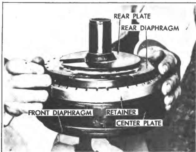
Fig. 5-11B—Installing Rear Diaphragm Retainer
