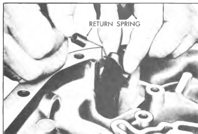
Fig. 7A-24C--Removing Parking Pawl Return Spring
