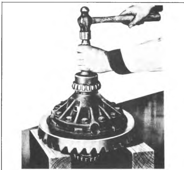
Fig. 5E--Differential Bearing Installation
