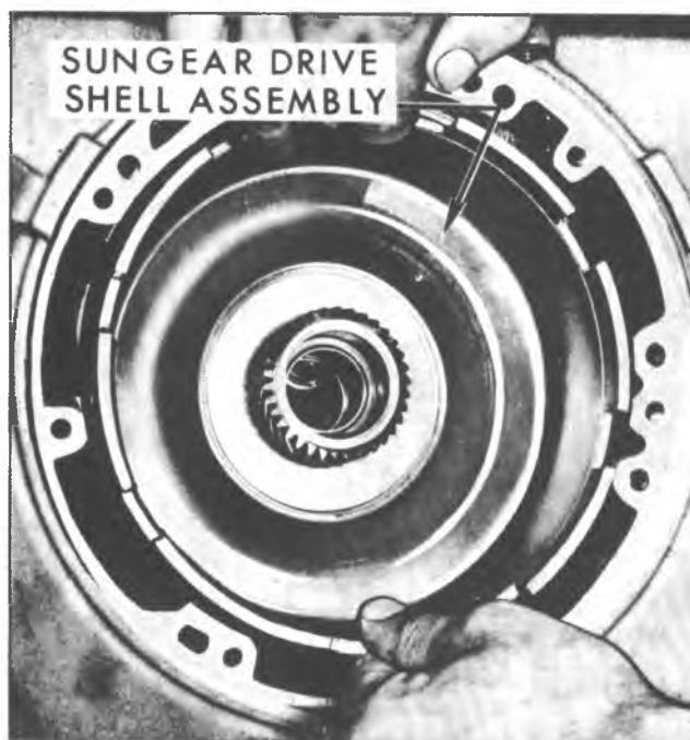
Fig. 7A-41B--Removing Sun Gear Drive Shell
