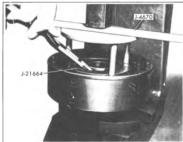
Fig. 7A-94C--Removing or Installing Direct Clutch Snap Ring
