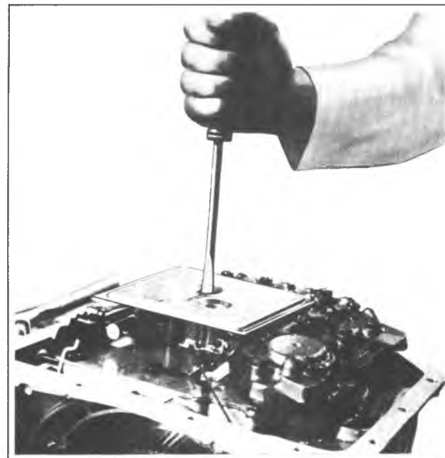
Fig. 7A-13B--Removing Oil Pump Suction Screen (Strainer) from Valve Body
