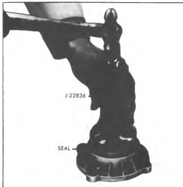
Fig. 7D-16R--Installing Front Output Bearing Retainer Seal
