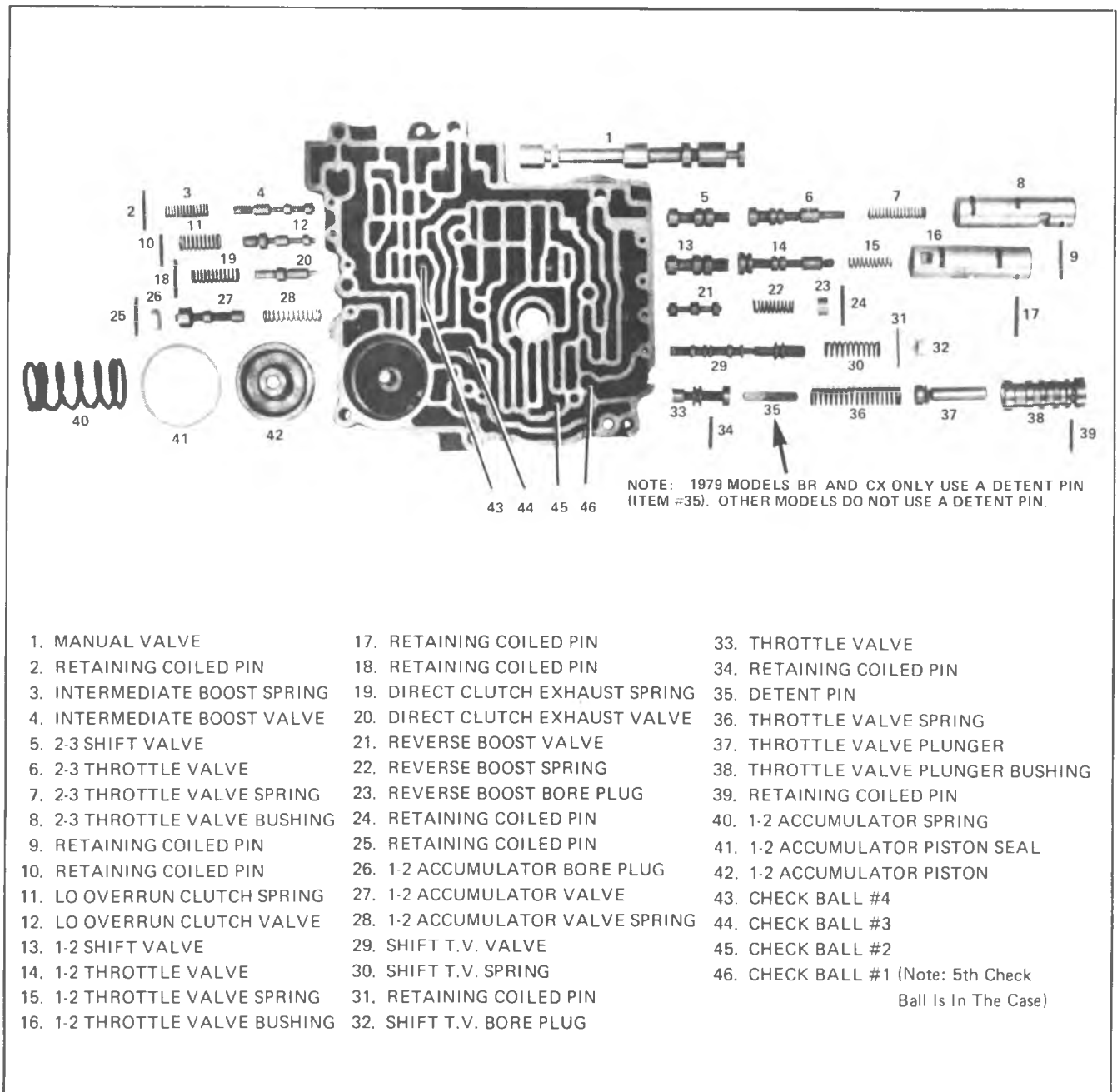
Fig. 7A-152A—Control Valve Assembly - Exploded View
