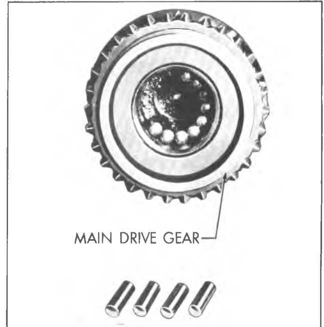
Fig. 7B-20J—Loading Mainshaft Bearings
