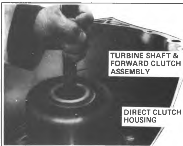
Fig. 7A-23A-Removing Forward and Direct Clutch Assemblies
