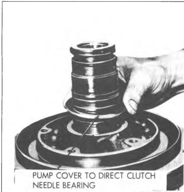
Fig. 7A-108B—Pump Cover to Direct Clutch Torrington Bearing
