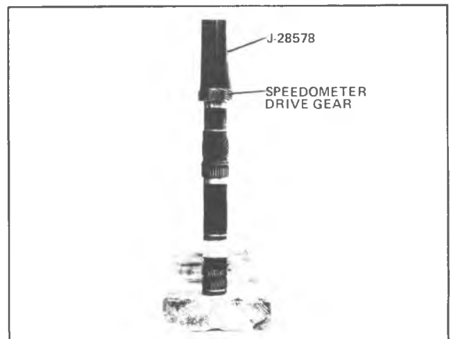
Fig. 7A-61A-Installing Steel Gear
