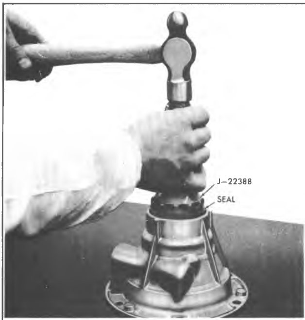
Fig. 7D-19S—Installing Rear Output Shaft Seal
