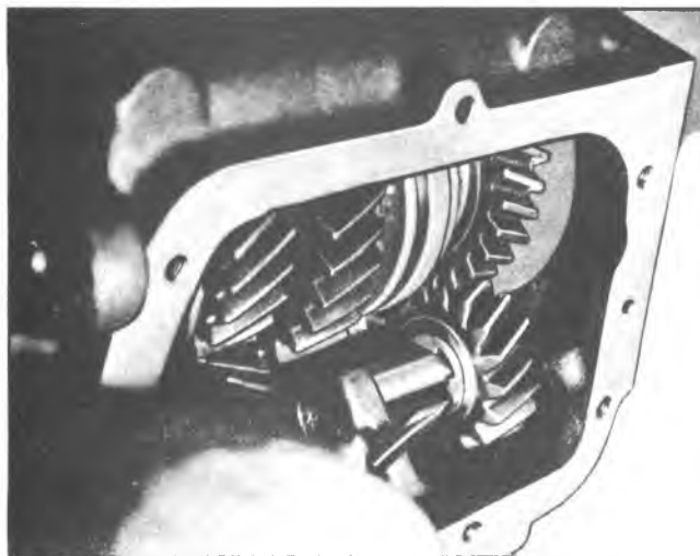
Fig. 7B-3A—Removing Reverse Idler Shaft "E" Ring
