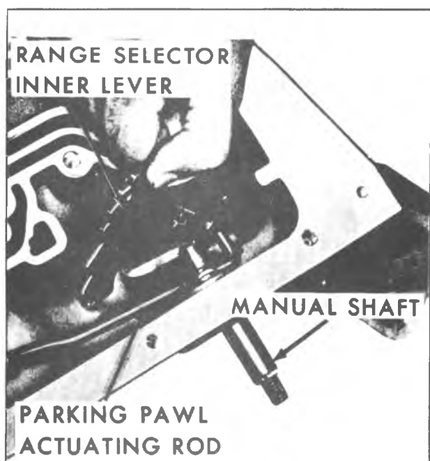
Fig. 7A-23B--Removing Manual Shaft and Inner Lever and Parking Pawl Actuator Rod from Case
