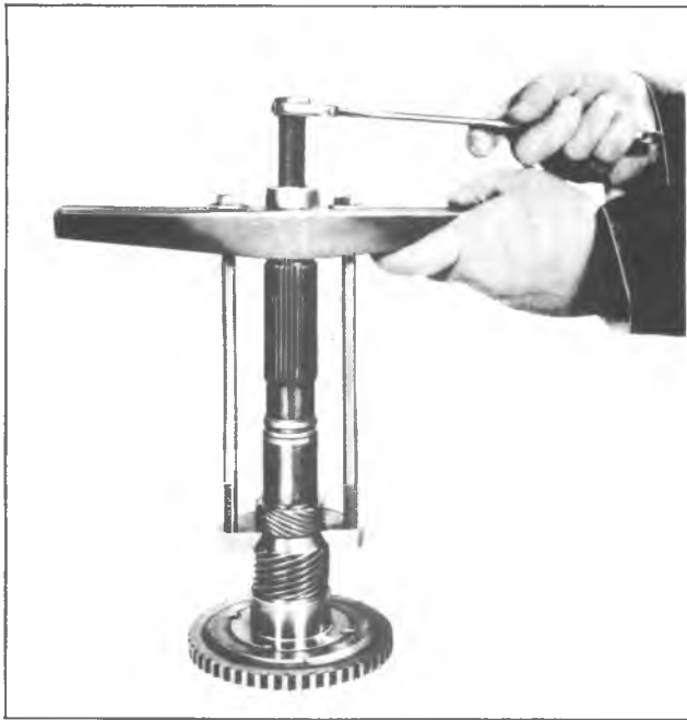
Fig. 7A-55C--Removing Steel Speedometer Drive Gear
