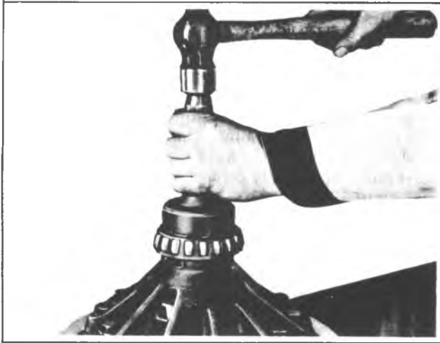
Fig. 8G--Differential Bearing Installation
