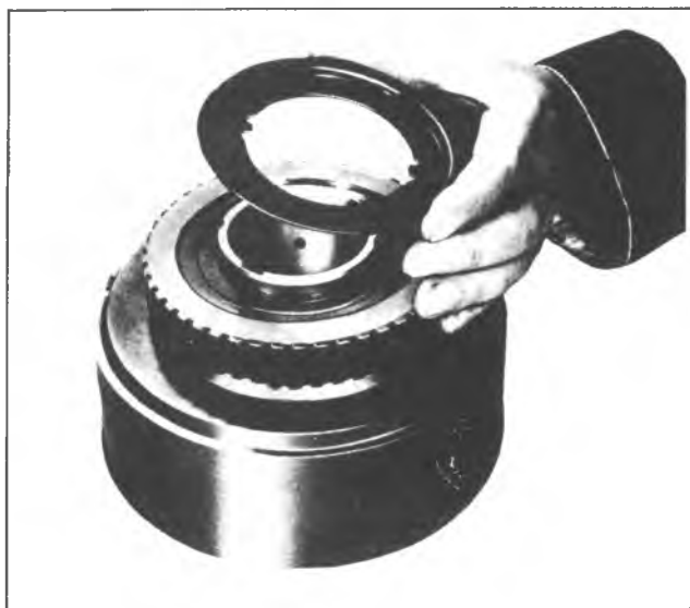
Fig. 7A-109C--Installing Intermediate Clutch Retainer
