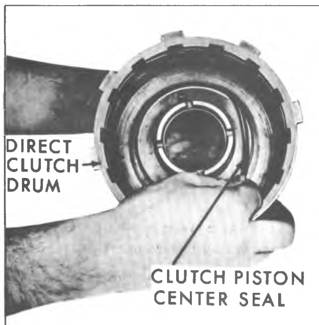
Fig. 7A-77B--Removing Direct Clutch Piston Center Seal
