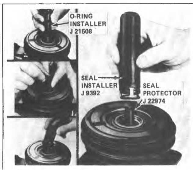
Figure 1D-23 Replacing A-6 Seal and O-Ring
