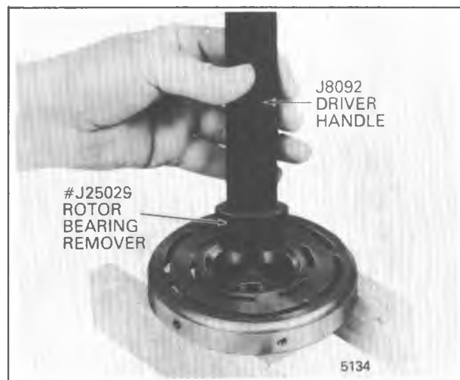
Figure 1D-84 R-4 Clutch Rotor Bearing Removal
