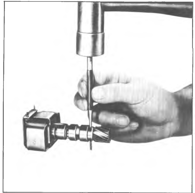
Fig. 7A-60C--Removing Governor Gear Retaining Pin
