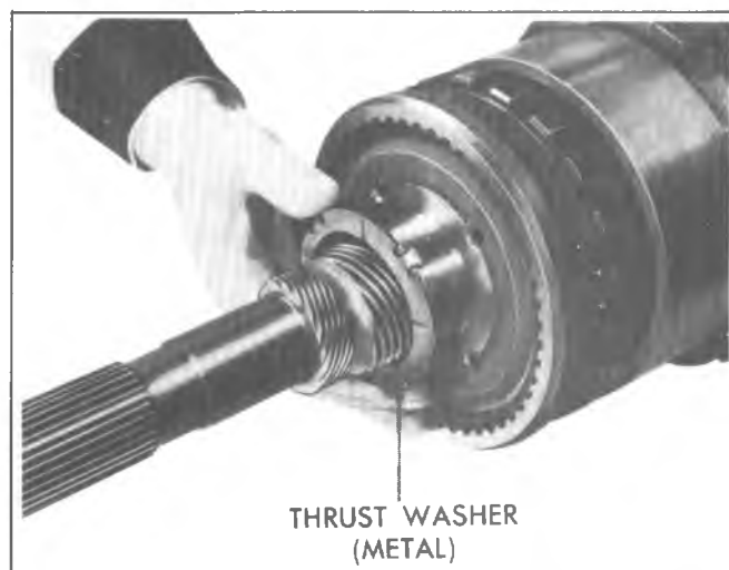
Fig. 7A-153C--Installing Case to Output Shaft Thrust Washer
