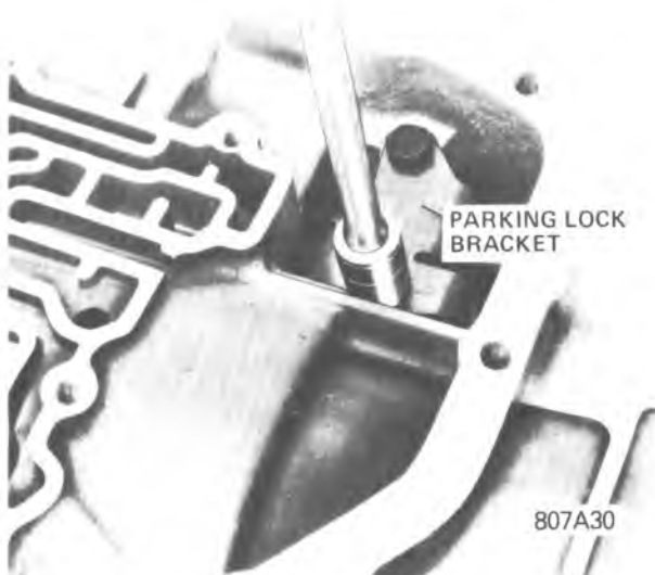
Figure 7A1-58 Removing Parking Pawl Bracket Bolt
