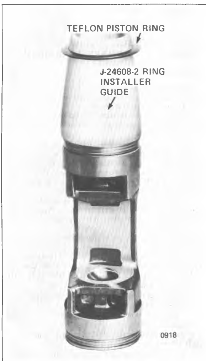
Figure 1D-51 A-6 Teflon Piston Ring Positioned on Ring Installer Guide
