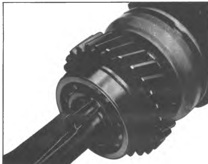
Fig. 7B-8A—Removing Rear Bearing Retaining Ring
