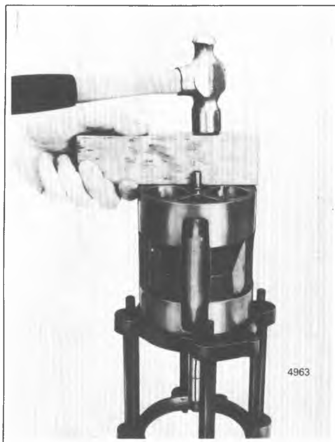
Figure 1D-44 Assembling A-6 Cylinder Halves
