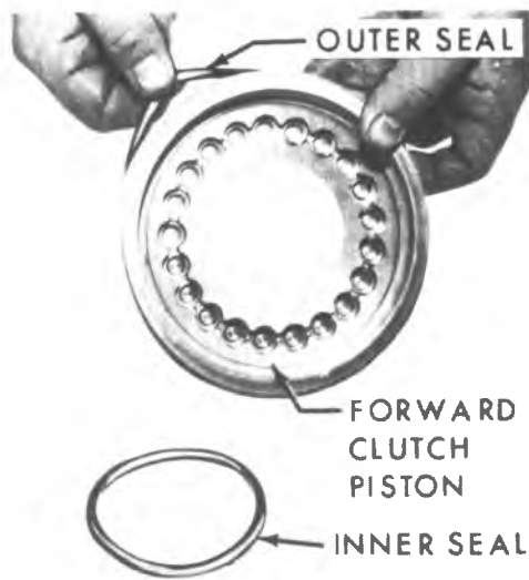
Figure 7A5-65 Removing Forward Clutch Piston Inner and Outer Seals
