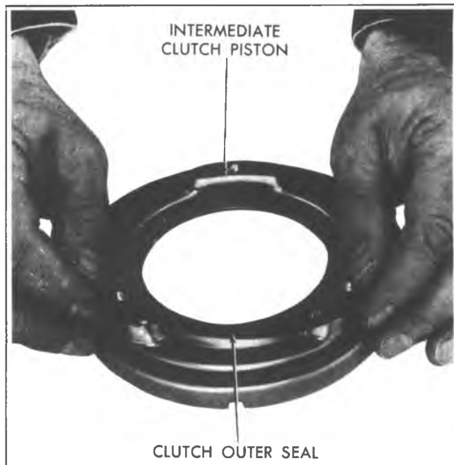
Fig. 7A-120C--Installing Intermediate Clutch Outer Seal
