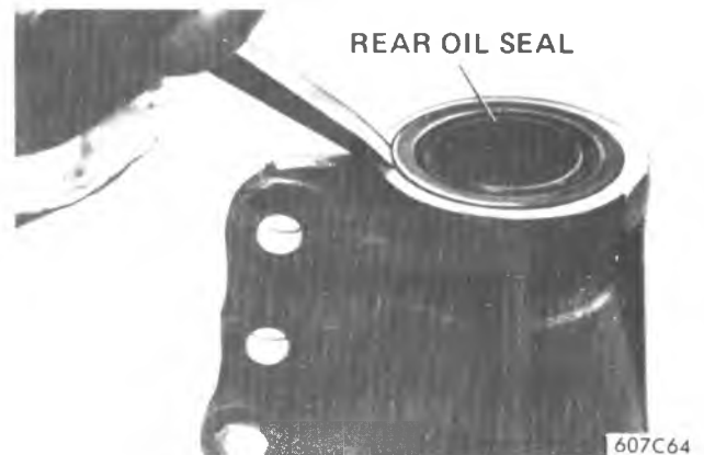
Figure 7A1-53 Removing Rear Oil Seal
