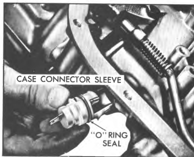
Fig. 7A-178C--Installing Electrical Connector and "O" Ring Seal
