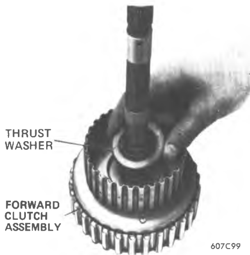
Figure 7A1-123 Removing Forward Clutch to Direct Clutch Thrust Washer
