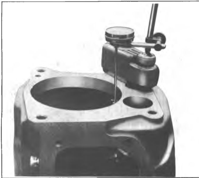
Fig. 7B-20K—Checking Countergear End Play
