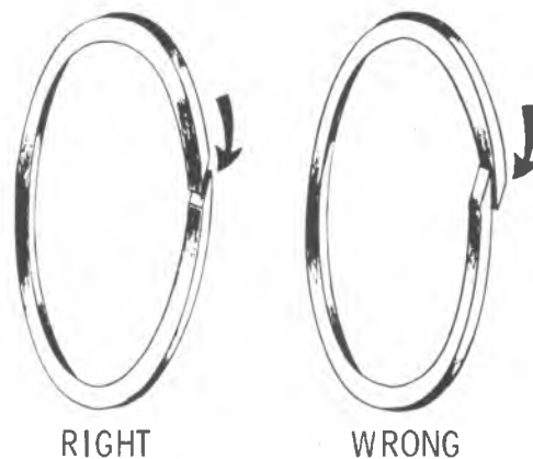
Figure 7A1-16 Teflon Oil Seal Rings
