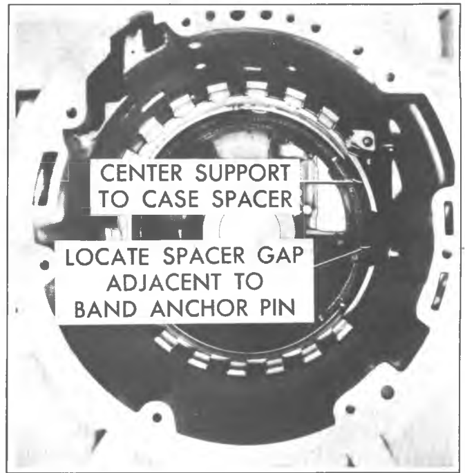
Fig. 7A-157C--Installing Center Support to Case Spacer
