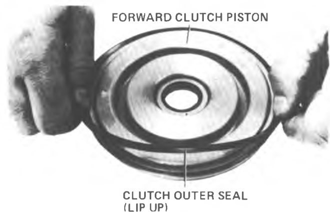
Figure 7A1-126 Removing or Installing Outer Piston Seal
