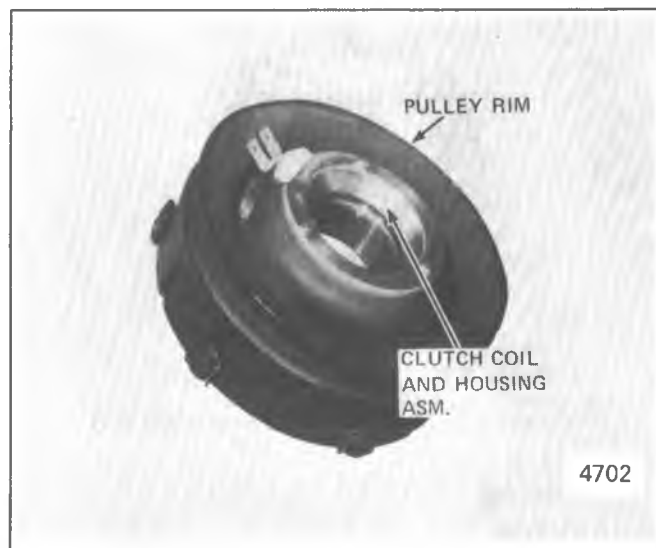
Figure 1D-90 Assembling R-4 Clutch Coil, Pulley Rim and Rotor and Bearing
