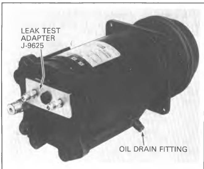
Figure 1D-25 Leak Testing A-6 Compressor
