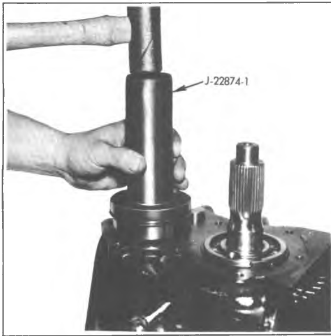
Fig. 7B-25L—Installing Countergear Rear Bearing
