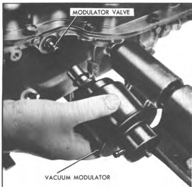
Fig. 7A-186C--Installing Vacuum Modulator and Valve
