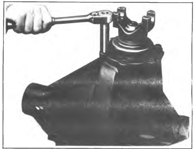
Fig. 7E—Removing Retainer Bolts
