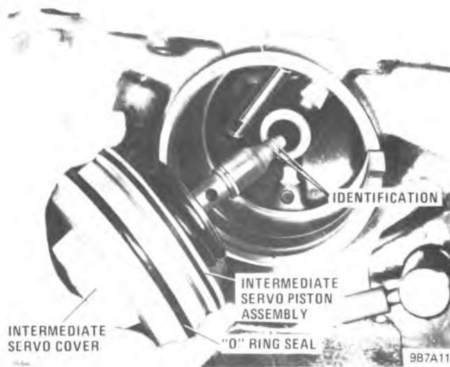
Figure 7A1-162 Installing Intermediate Servo Piston into Cover
