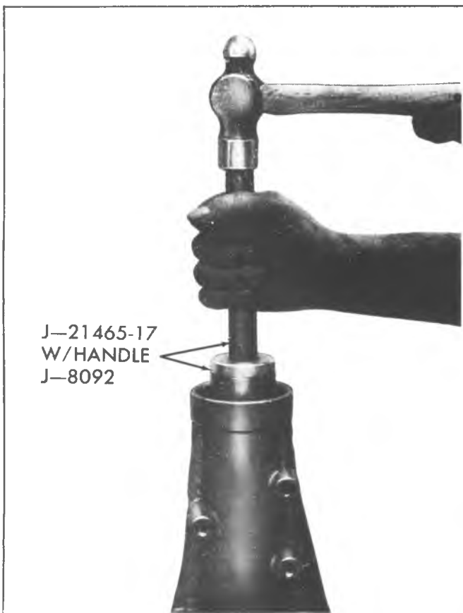
Fig. 7B-14K-Removing Rear Extension Bushing
