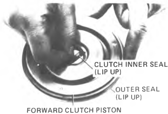
Figure 7A1-127 Removing or Installing Inner Piston Seal
