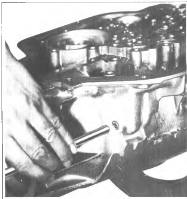
Fig. 7A-154C--Installing Parking Pawl Shaft Cup Plug
