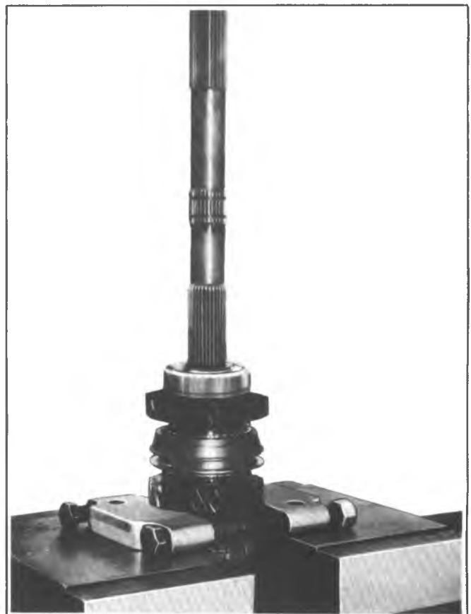
Fig. 7B-12K—Pressing Rear Bearing From Mainshaft
