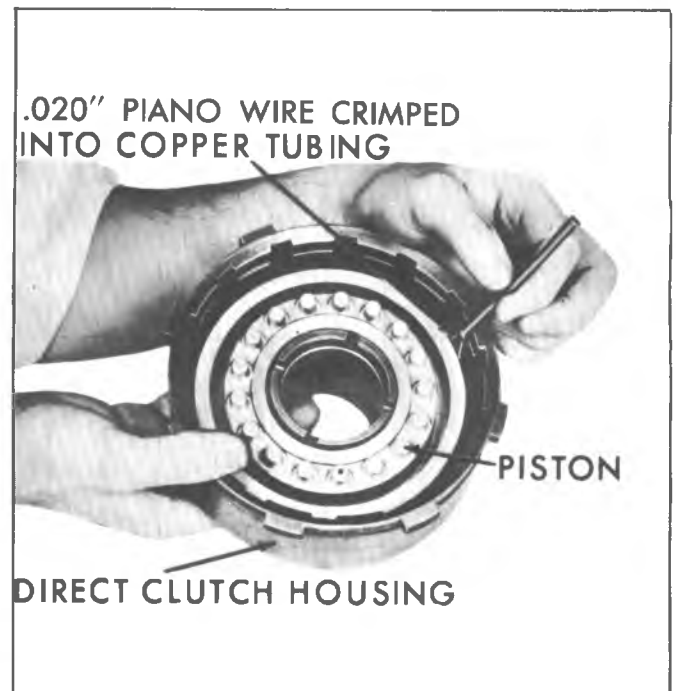
Fig. 7A-78B--Installing Direct Clutch Piston
