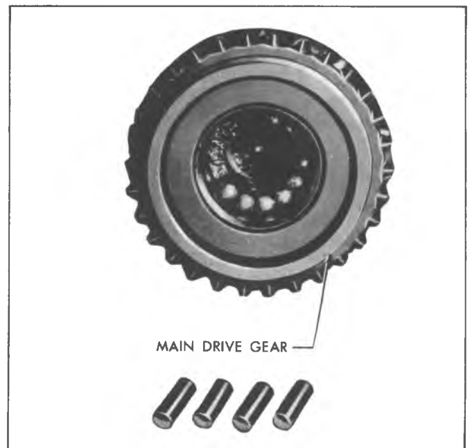
Fig. 7B-17A--Loading Pilot Bearings
