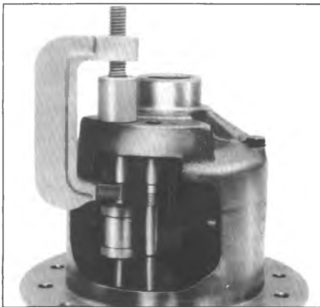
Fig. 4B-5H-Bearing Puller J-26252
