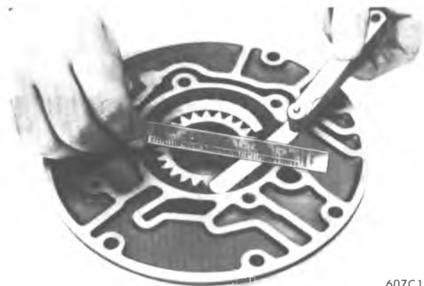
Figure 7A1-145 Checking Pump Body-to-Gear End Clearance
