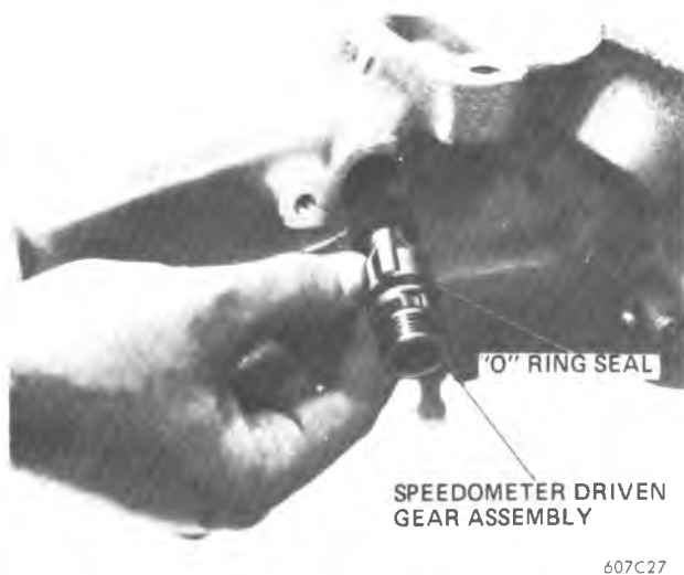
Figure 7A1-180 Removing and Installing Speedometer Driven Gear - Typical
