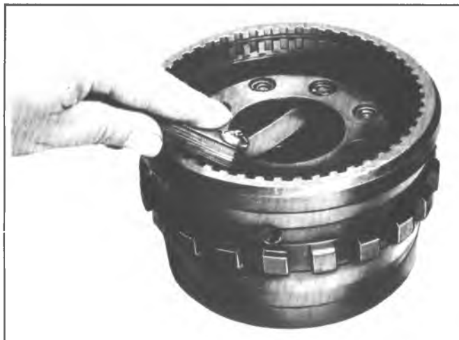
Fig. 7A-129C--Checking Output Carrier Pinion End Play
