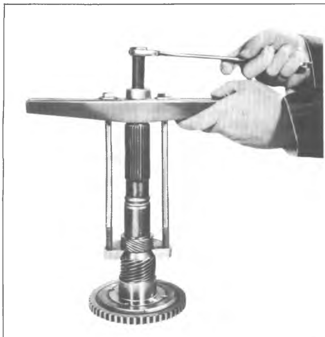
Fig. 7A-55C--Removing Steel Speedometer Drive Gear
