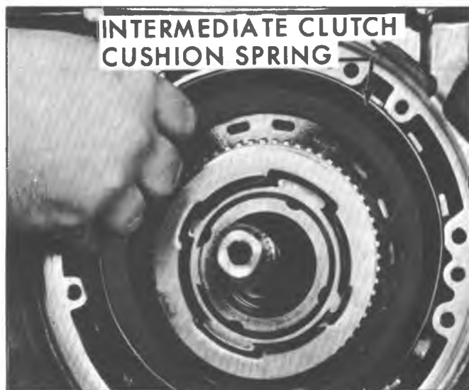
Fig. 7A-31B--Removing Intermediate Clutch Cushion Spring
