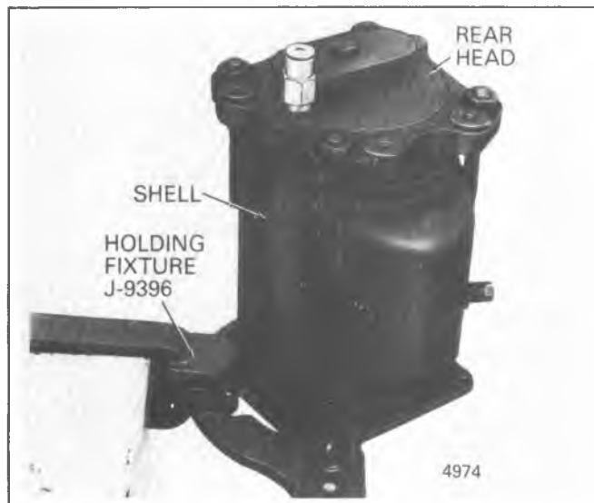
Figure 1D-29 A-6 Compressor Installed in Holding Fixture
