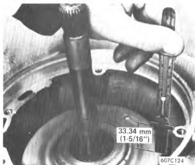
Figure 7A1-136 Direct and Forward Clutch Assemblies Properly Installed
