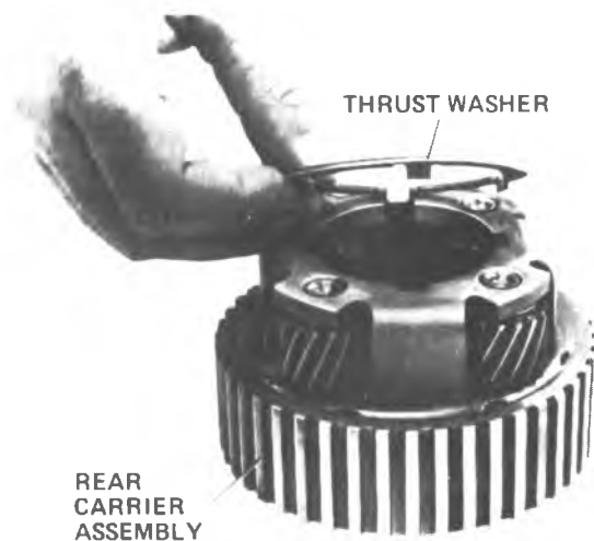
Figure 7A1-83 Installing Thrust Washer
