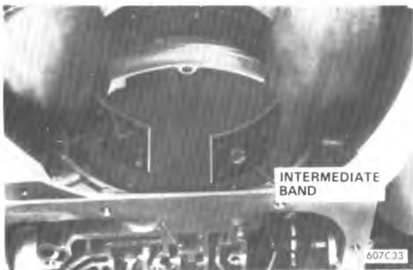
Figure 7A1-36 Removing Intermediate Band Assembly
