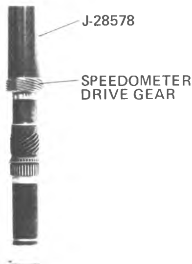
Figure 7A1-74 Installing Speedo Gear (Steel)
