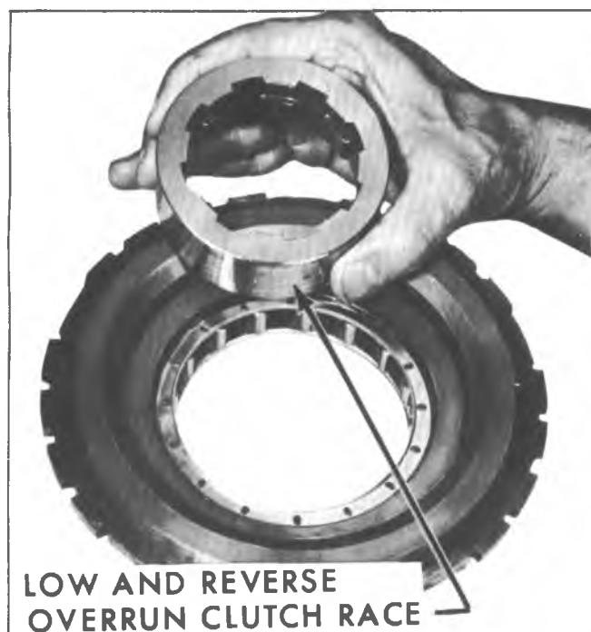
Fig. 7A-94B--Removing Overrun Clutch Inner Race
