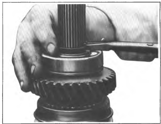
Fig. 7B-11K—Removing Rear Bearing Snap Ring
