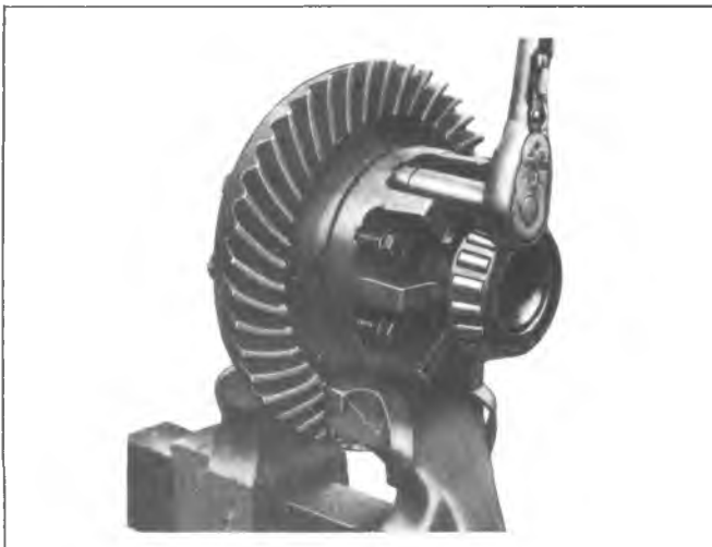
Fig. 3F—Separating Case Halves
