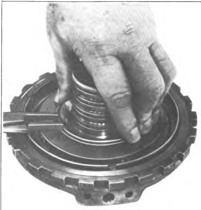
Fig. 7A-113C--Removing Intermediate Clutch Piston Snap Ring
