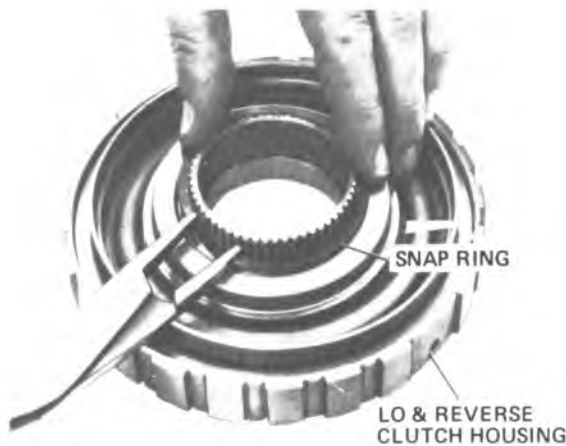
Figure 7A1-94 Installing Lo and Reverse Clutch Retaining Snap Ring
