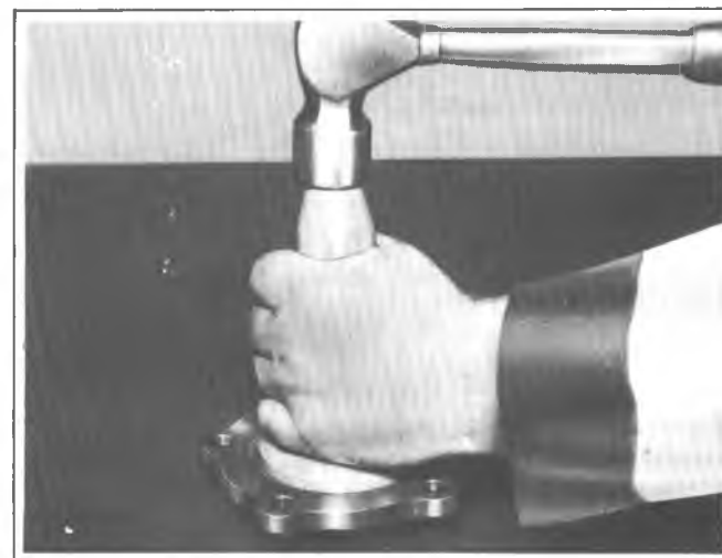
Fig. 4G--Pinion Oil Seal Installation
