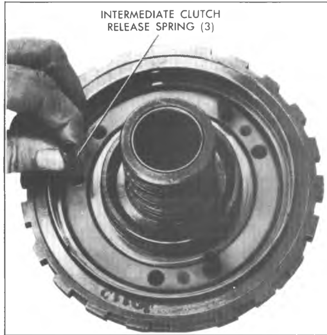
Fig. 7A-115C--Removing Clutch Release Springs
