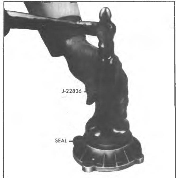
Fig. 7E-16R--Installing Front Output Bearing Retainer Seal
