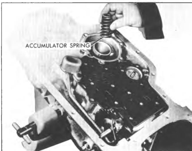
Fig. 7A-180C--Installing Rear Accumulator Spring
