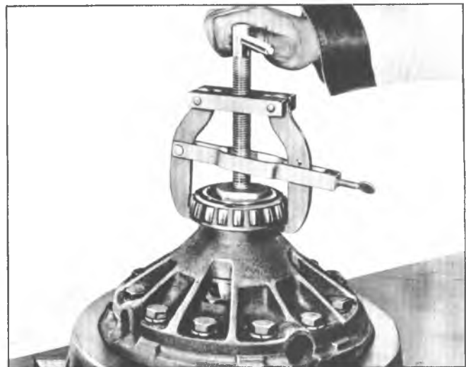
Fig. 4E-Differential Bearing Removal
