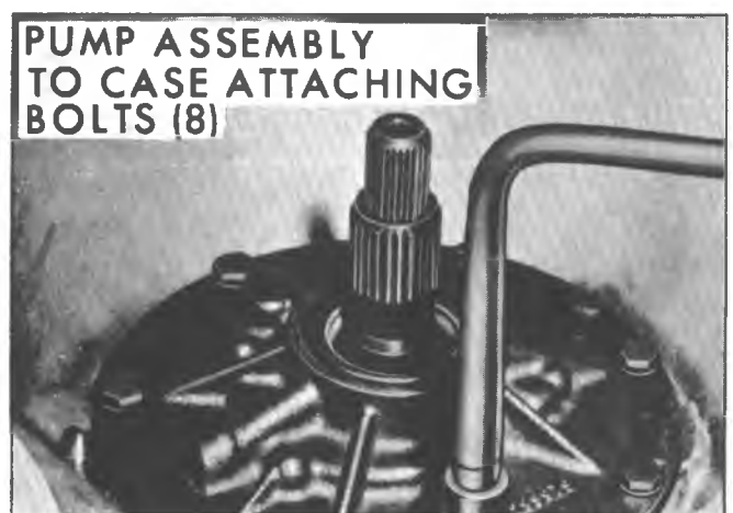
Fig. 7A-29B--Removing Pump Attaching Bolts
