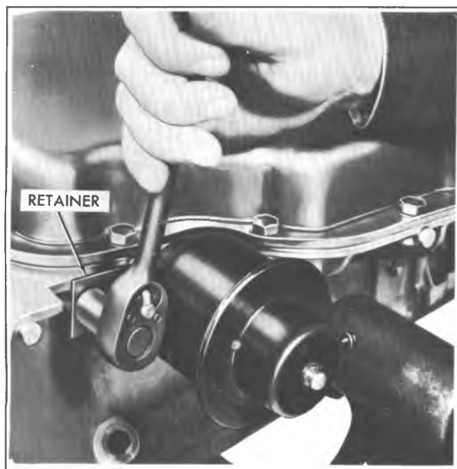
Fig. 7A-3C--Removing Modulator Retainer
