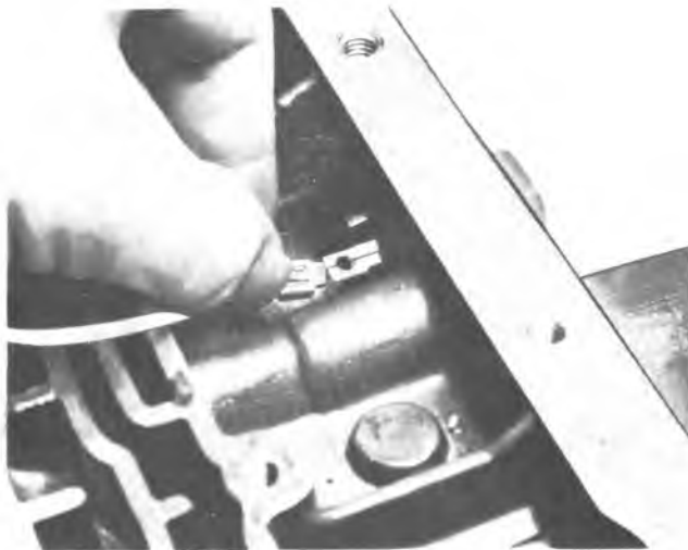
Figure 7A1-24A Removing Lead Wire
