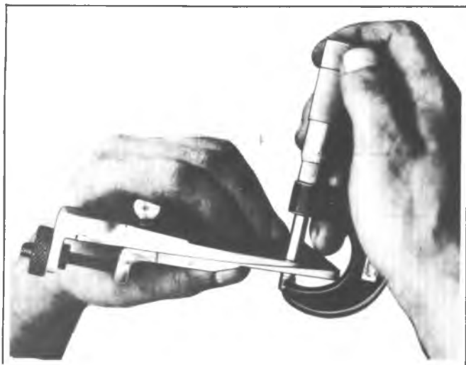
Fig. 8B--Measuring Gage Plate Thickness
