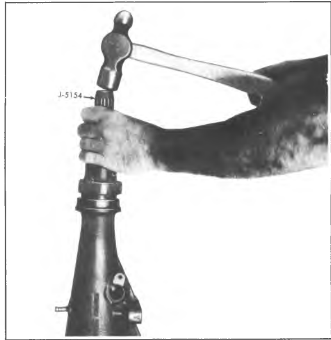
Fig. 7B-16B—Installing Extension Housing Seal
