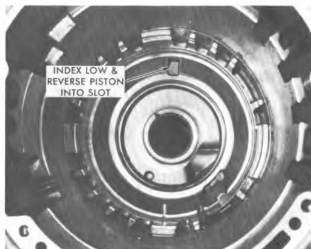
Figure 7A5-80 Low & Reverse Piston Indexing Slot
