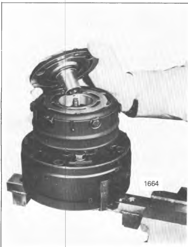
Figure 1D-79 Installing R-4 Shaft Key
