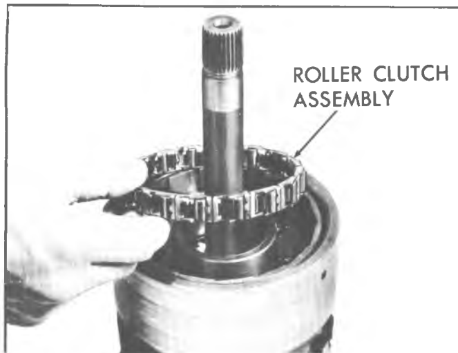
Fig. 7A-150C--Installing Roller Clutch to Reaction Carrier
