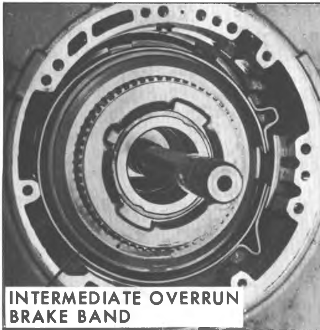
Fig. 7A-34B--Removing Intermediate Overrun Brake Band
