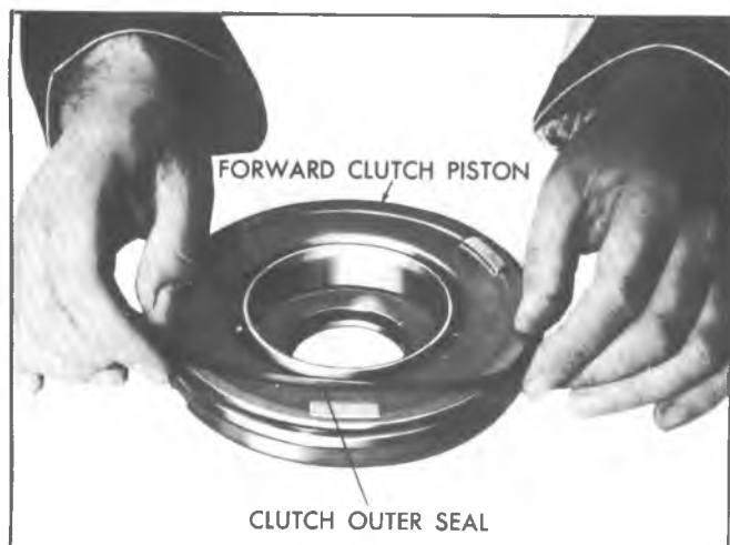
Fig. 7A-84C--Removing Forward Clutch Piston Outer Seal
