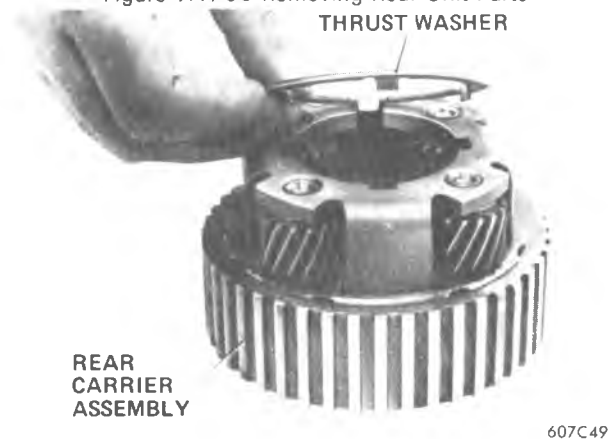
Figure 7A1-51 Removing Thrust Washer
