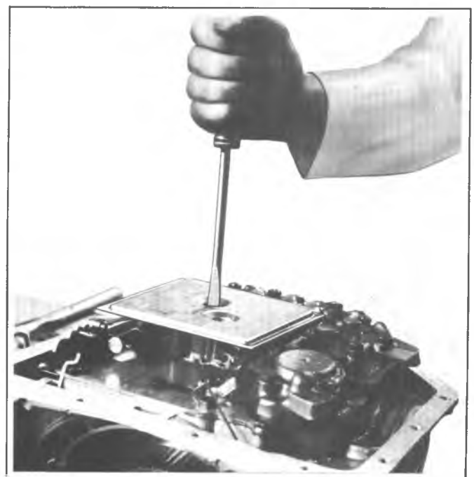
Fig. 7A-13B--Removing Oil Pump Suction Screen (Strainer) from Valve Body
