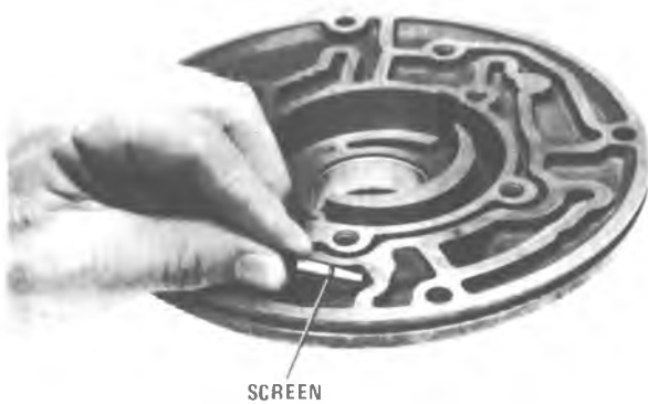
Figure 7A1-141B Removing Screen
