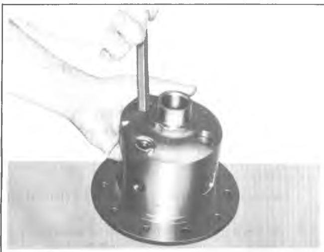
Fig. 8D-Removing Side Gear
