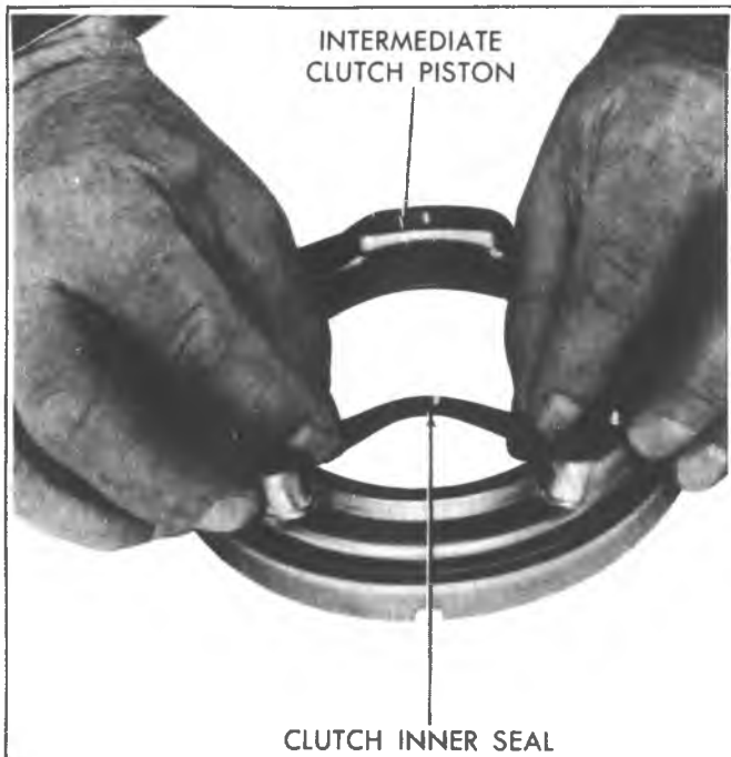
Fig. 7A-119C--Installing Intermediate Clutch Inner Seal
