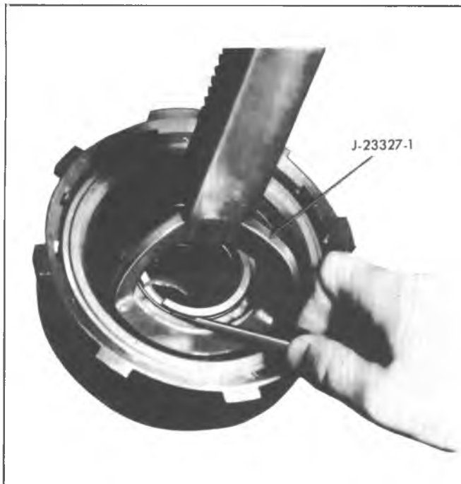
Fig. 7A-76B--Removing Direct Clutch Outer and Inner Seals
