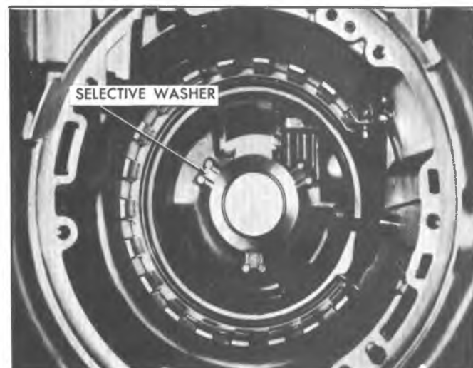
Fig. 7A-43C--Removing Selective Washer
