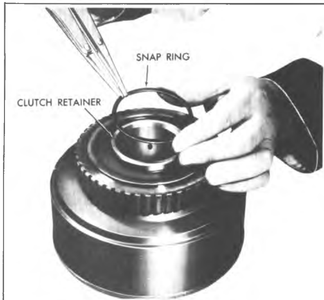
Fig. 7A-92C--Removing Intermediate Clutch Retainer Snap Ring
