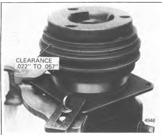
Figure 1D-11 Checking A-6 Air Gap
