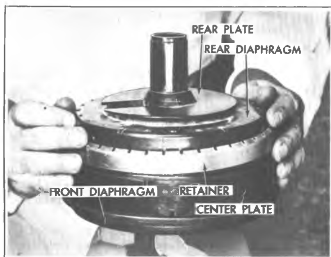
Fig. 5-11B—Installing Rear Diaphragm Retainer
