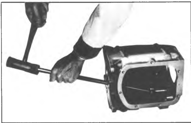
Fig. 7B-6A—Removing Reverse Idler Shaft
