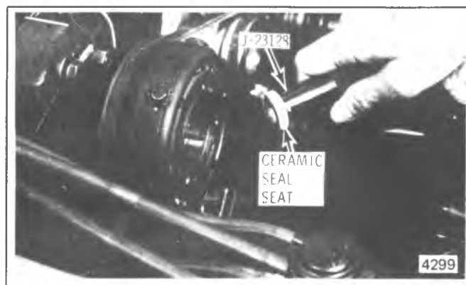
Figure 1D-93 Removing R-4 Ceramic Seal Seat (On Car)
