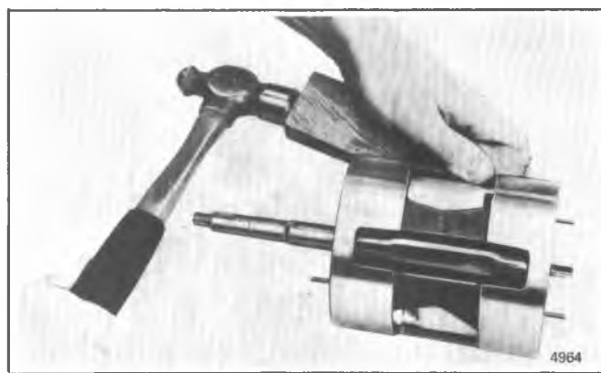
Figure 1D-36 Separating A-6 Cylinder Halves
