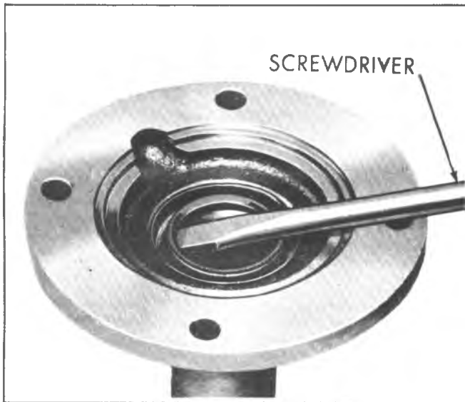
Fig. 7B-14J—Removing Bearing Retainer Oil Seal
