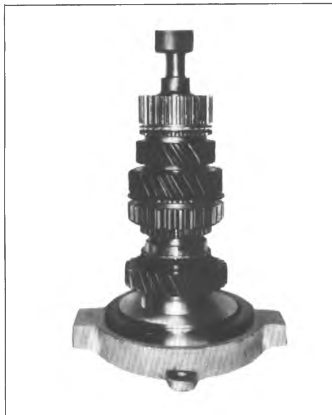
Fig. 7B-17J-Installing Rear Bearing
