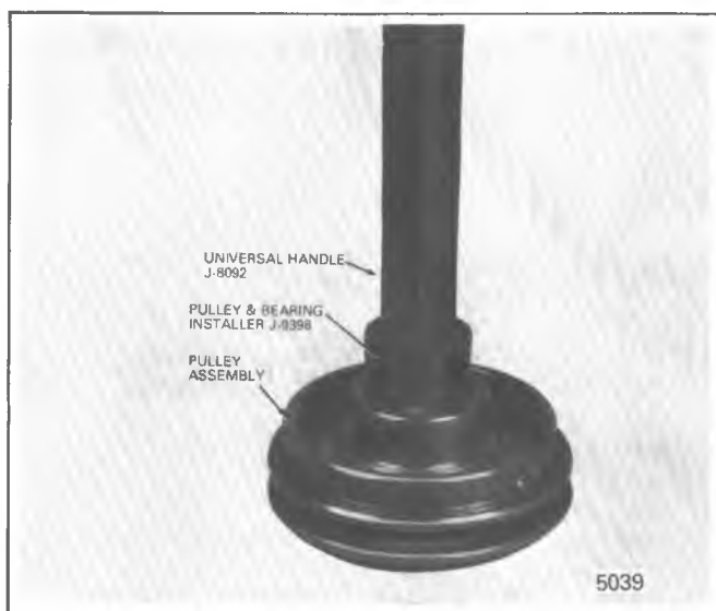
Figure 1D-16 Removing Bearing From A-6 Pulley Assembly
