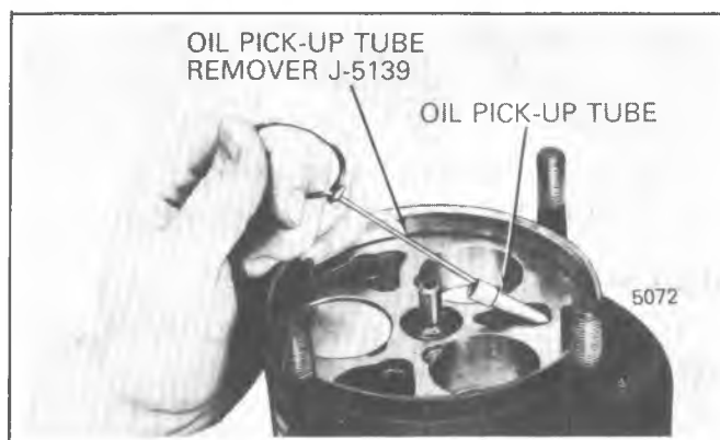
Figure 1D-33 Removing A-6 Oil Pick-Up Tube
