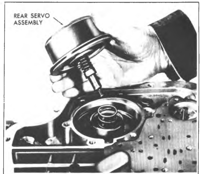
Fig. 7A-181C--Installing Rear Servo Assembly
