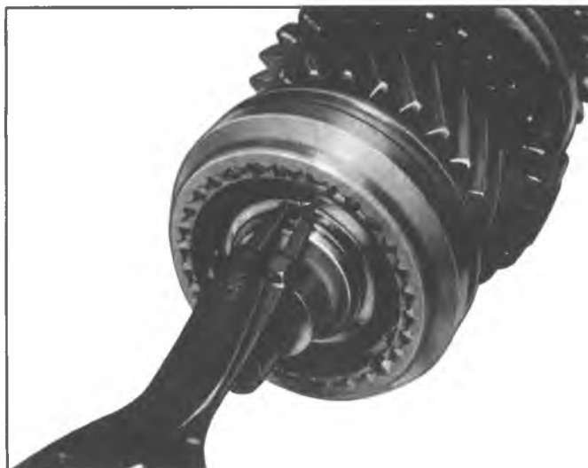
Fig. 7B-7A—Removing 2nd-3rd Clutch Hub Retaining Ring
