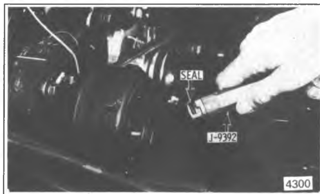
Figure 1D-94 Removing R-4 Seal (On Car)
