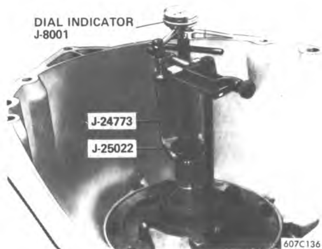
Figure 7A1-153 Checking Front Unit End Play
