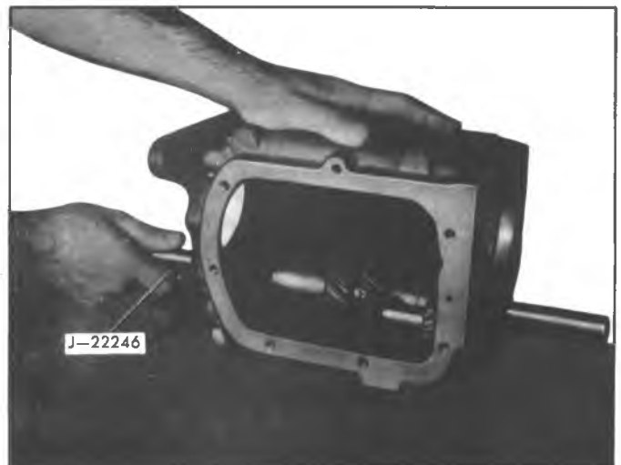
Fig. 7B-5A—Removing Counter Gear Shaft
