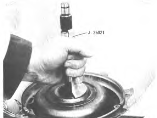
Figure 7A1-135 Installing Direct and Forward Clutch Assemblies
