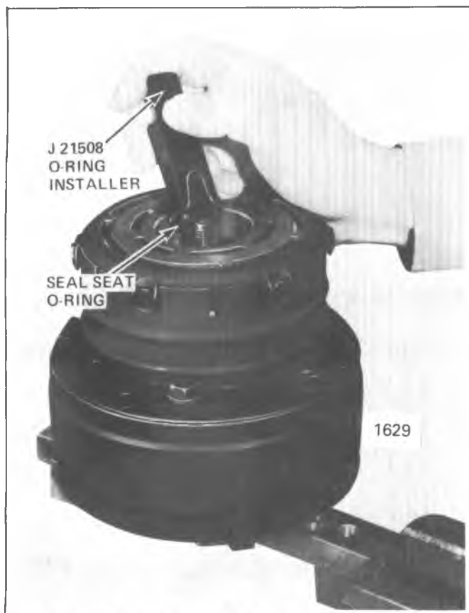
Figure 1D-101 - Installing R-4 Seal Seat O-Ring (Off Car)
