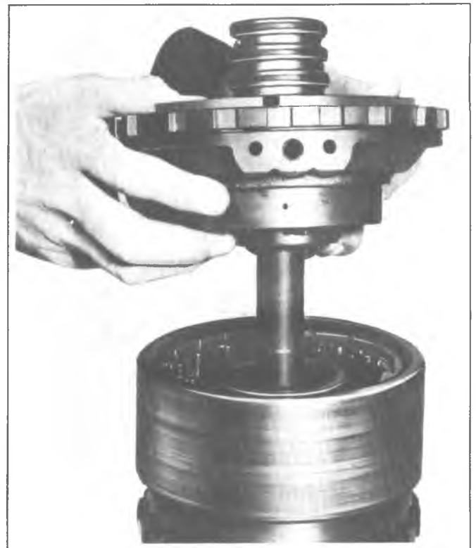
Fig. 7A-46C--Removing Center Support Assembly
