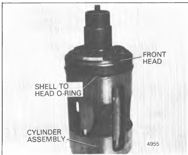
Figure 1D-71 A-6 Shell-To-Front Head O-Ring Installation
