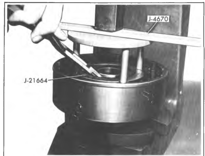
Fig. 7A-94C--Removing or Installing Direct Clutch Snap Ring
