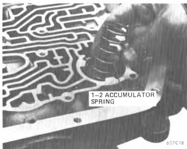
Figure 7A1-21 Removing 1-2 Accumulator Spring
