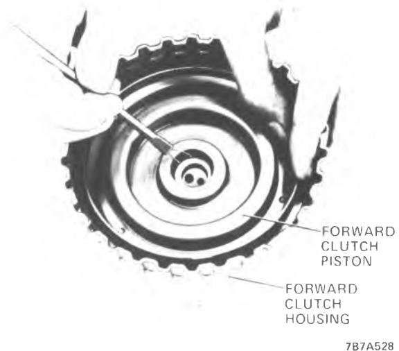
Figure 7A1-130 Installing Forward Clutch Piston
