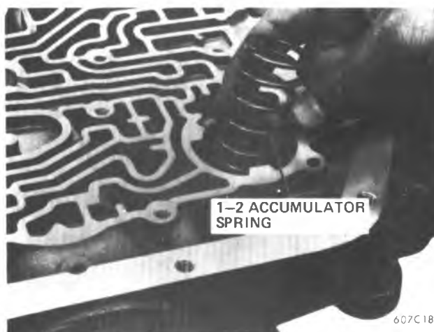
Figure 7A1-172 Installing 1-2 Accumulator Spring
