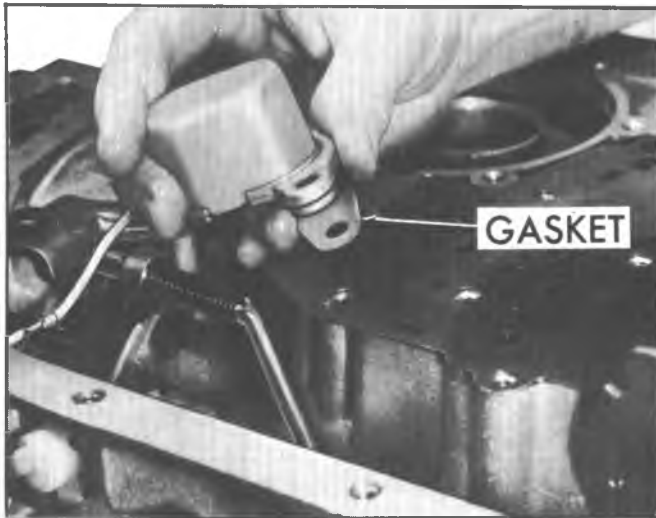
Fig. 7A-18C--Removing Detent Solenoid and Gasket
