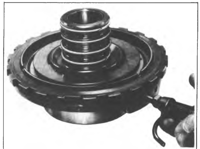
Fig. 7A-126C--Air Checking Intermediate Clutch Piston
