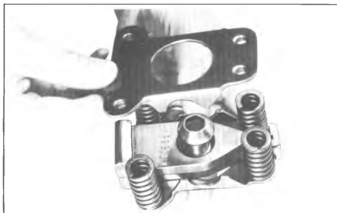
Fig. 12D--Installing Spring Pack Compression Tool (Corvette)
