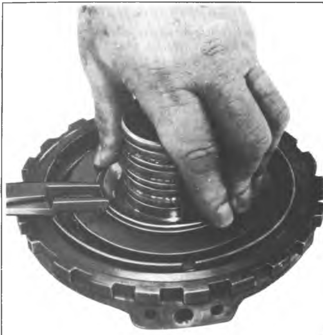
Fig. 7A-124C--Installing Intermediate Clutch Piston Snap Ring
