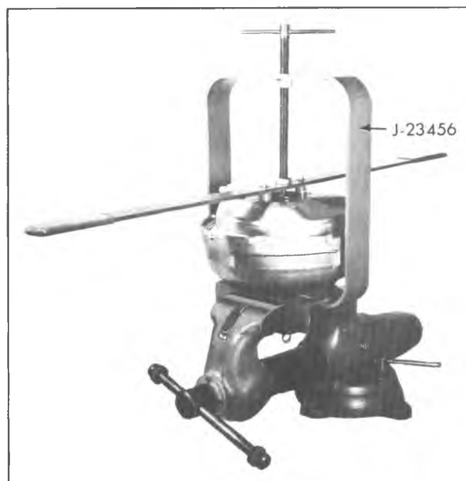
Fig. 5-1A—Unlocking Front and Rear Housings
