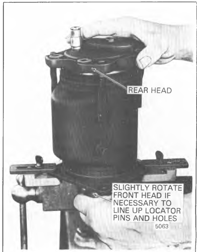
Figure 1D-72 Installing A-6 Rear Head
