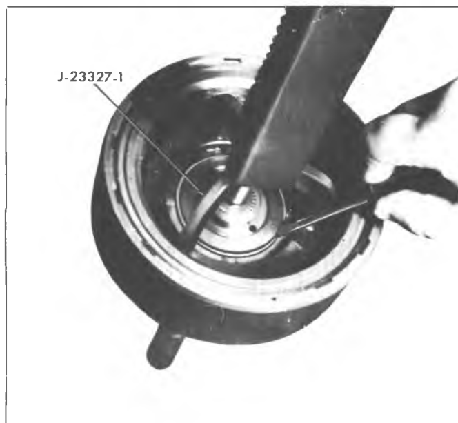
Fig. 7A-84B--Compressing Forward Clutch Piston Return Seat
