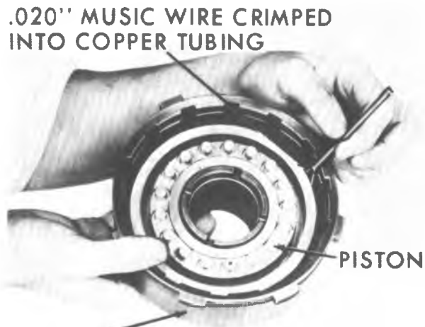
Figure 7A5-58 Installing Direct Clutch Piston
