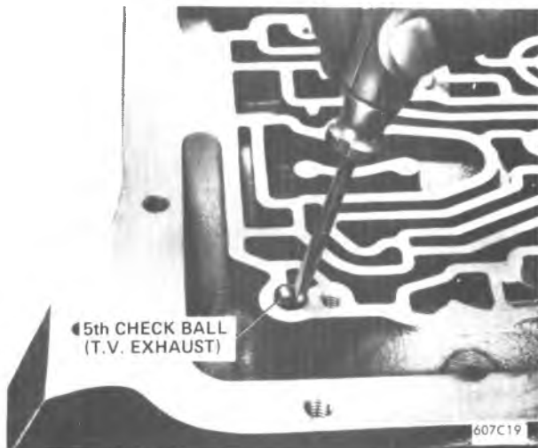
Figure 7A1-173 Installing 5th Check Ball
