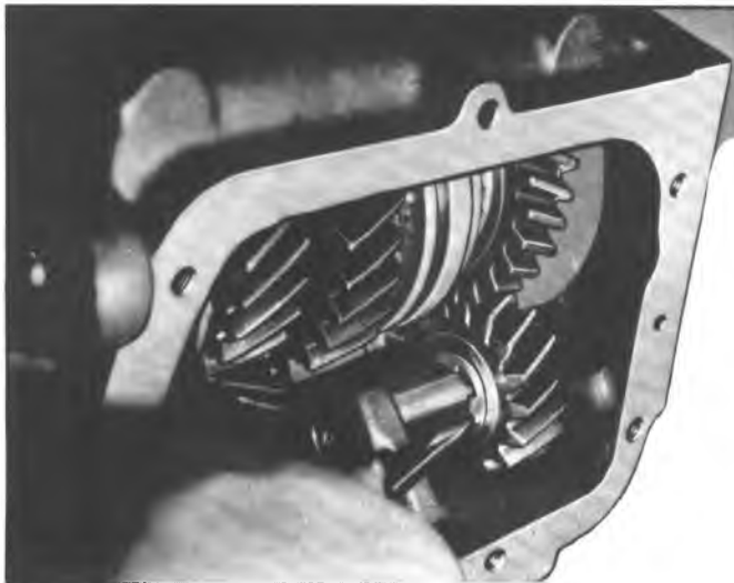
Fig. 7B-3A—Removing Reverse Idler Shaft "E" Ring
