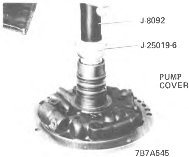
Figure 7A1-184 Installing Pump Cover Bushing - Rear
