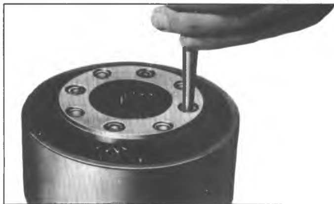
Fig. 7A-130C--Removing Planet Pinion Pin
