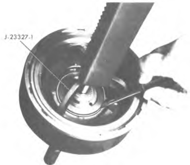
Figure 7A5-64 Compressing Forward Clutch Spring Retaining Seat
