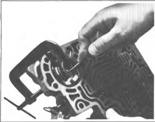
Fig. 7A-55B--Removing Direct Clutch Accumulator Piston Retaining "E" Ring
