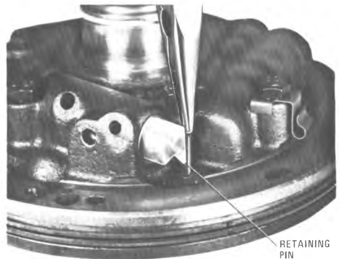
Figure 7A1-139C Removing Retaining Pin
