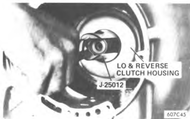
Figure 7A1-48 Removing Low and Reverse Clutch Housing
