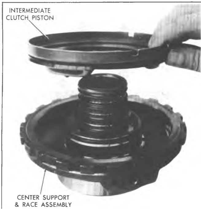
Fig. 7A-117C--Removing Intermediate Clutch Piston
