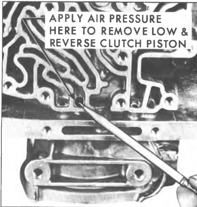
Fig. 7A-50B--Removing Low and Reverse Clutch Piston
