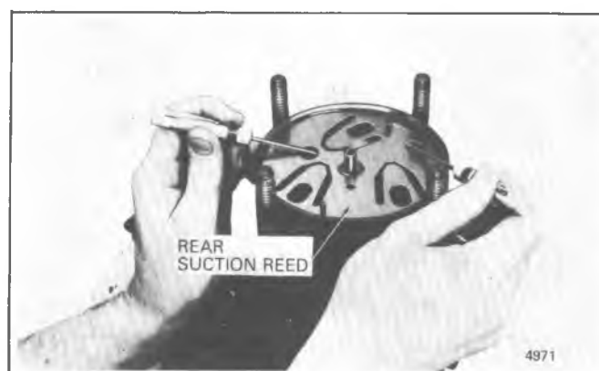
Figure 1D-32 Removing A-6 Rear Suction Reed
