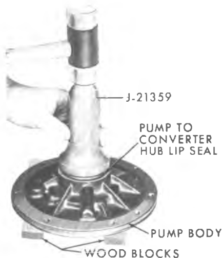
Figure 7A5-48 Installing Hub Lip Seal
