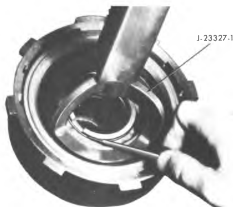
Figure 7A5-52 Removing Direct Clutch Retaining Ring
