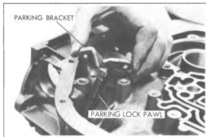
Fig. 7A-23C--Removing Parking Bracket
