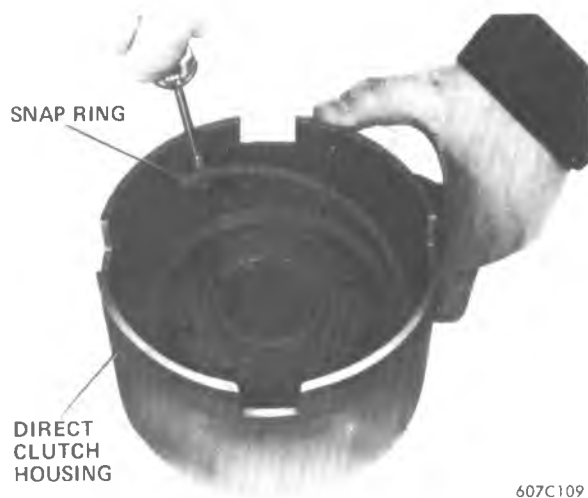
Figure 7A1-113 Removing Direct Clutch Snap Ring
