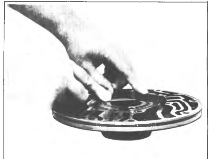
Fig. 7A-63B--Checking Pump Body to Gear Face Clearance
