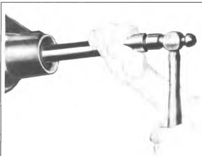
Fig. 17B—Installing Pinion Front Bearing Cup
