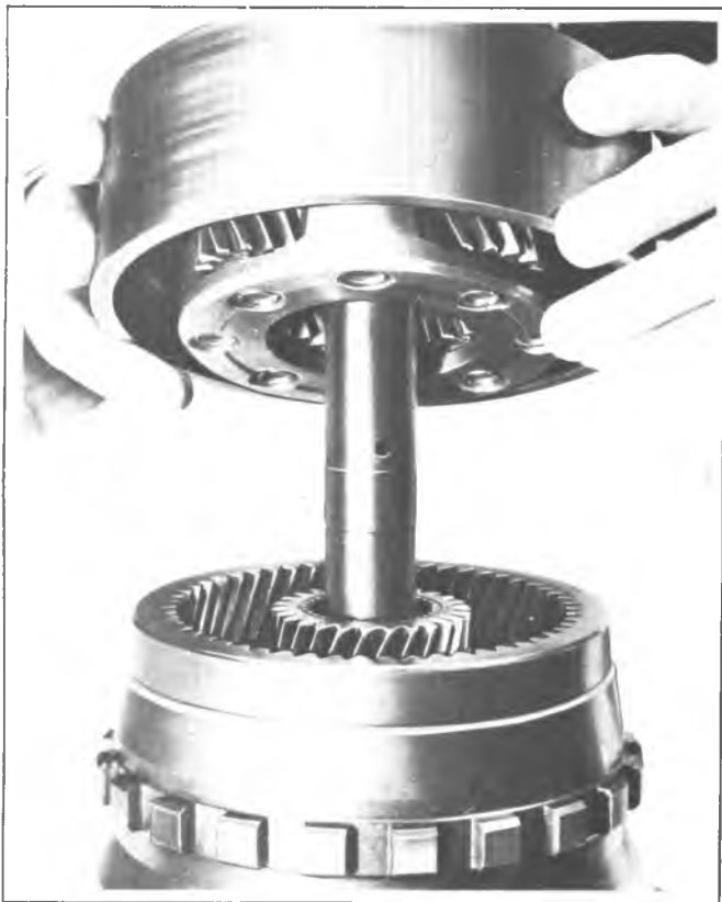
Fig. 7A-147C--Installing Reaction Carrier
