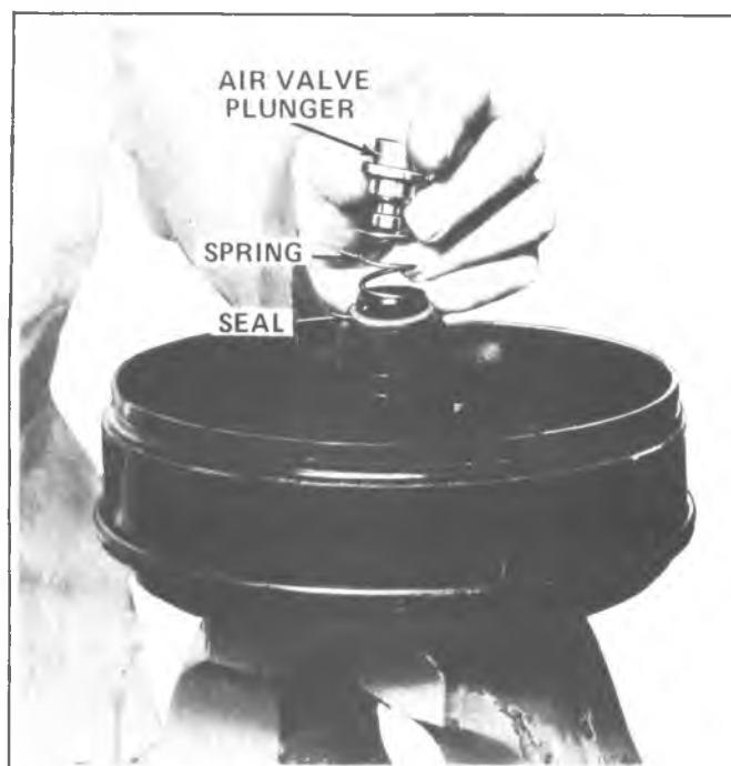
Fig. 5-10B—Installing Air Valve Plunger
