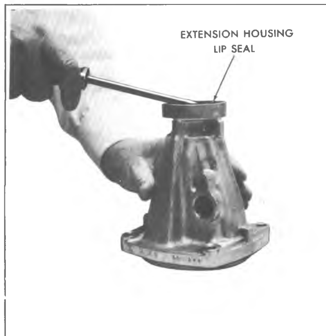
Fig. 7A-7B--Removing Extension Housing Lip Seal
