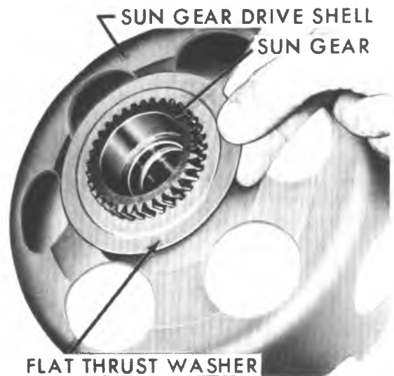
Figure 7A5-71 Removing Sun Gear to Drive Shell
