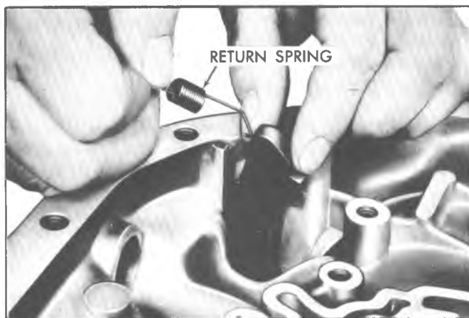
Fig. 7A-24C--Removing Parking Pawl Return Spring
