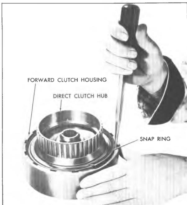
Fig. 7A-89C--Installing Forward Clutch Housing to Direct Clutch Hub Snap Ring
