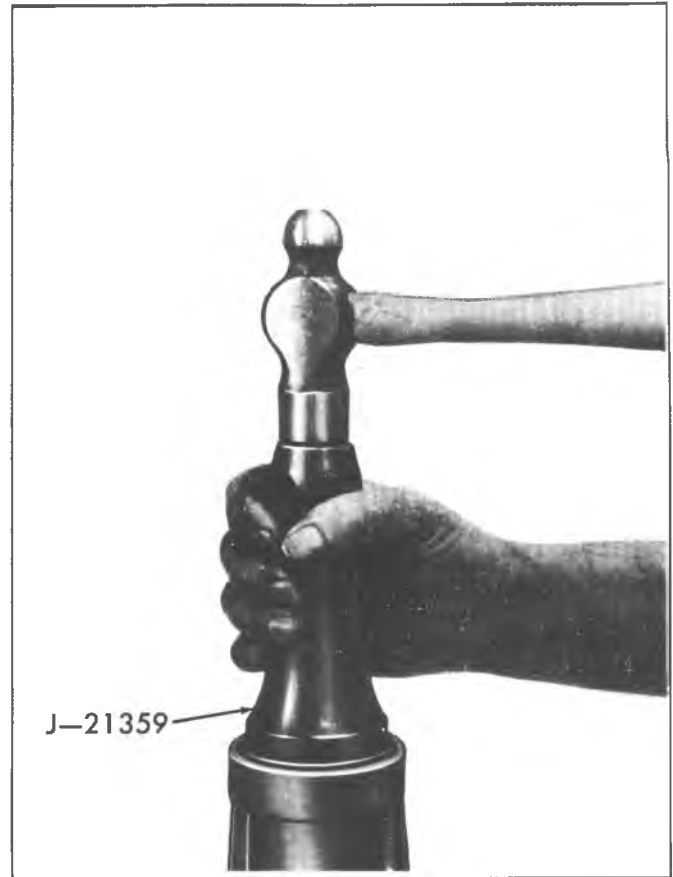
Fig. 7B-15K-Installing Rear Extension Seal
