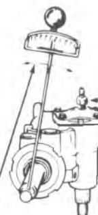
With gear at center of travel, check torque to turn stub shaft (reading #1).
