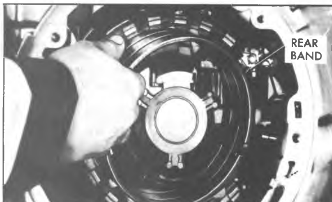
Fig. 7A-156C--Installing Rear Band
