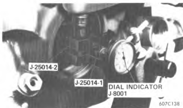
Figure 7A1-160 Intermediate Band Apply Gages
