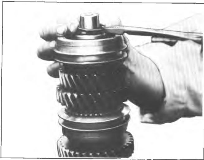
Fig. 7B-9K—Removing 3-4 Clutch Assembly Retainer
