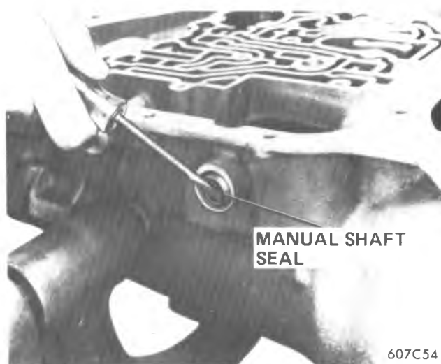
Figure 7A1-57 Removing Manual Shaft Seal From Case
