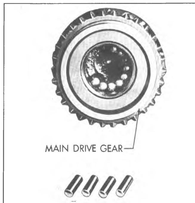
Fig. 7B-20J—Loading Mainshaft Bearings
