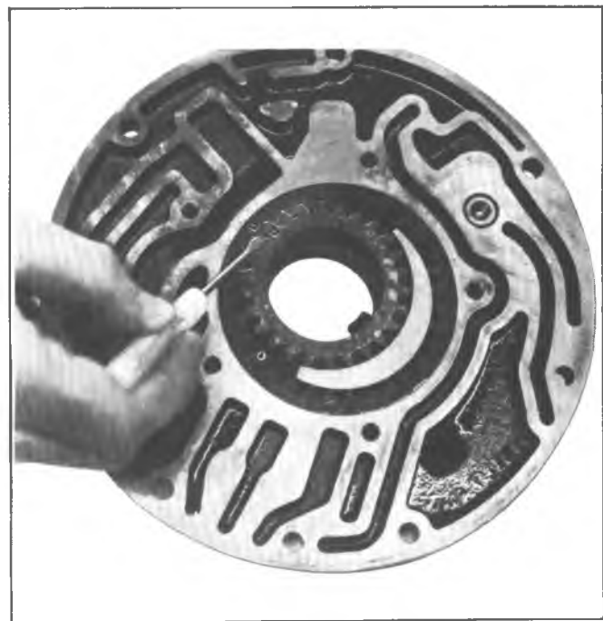
Fig. 7A-66B--Installing Pump Drive and Driven Gears
