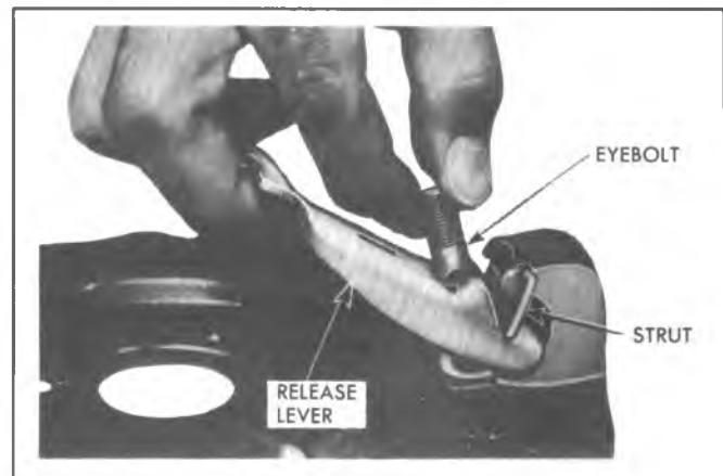
Fig. 7C-5E-Removing or Installing Lever
