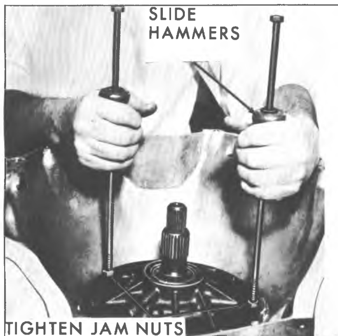
Fig. 7A-30B--Removing Pump from Case
