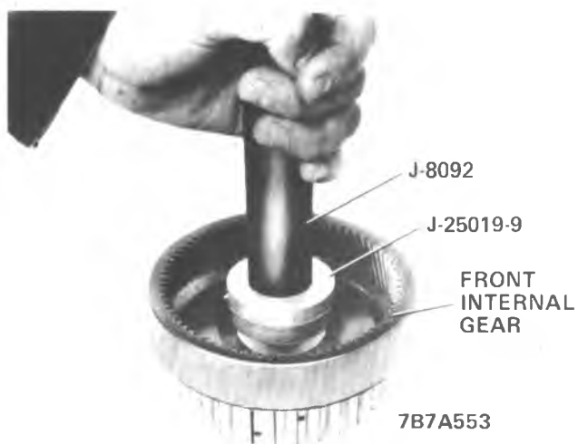
Figure 7A1-192 Installing Front Internal Gear Bushing
