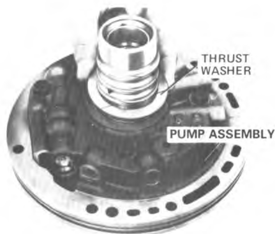
Figure 7A1-138 Removing Thrust Washer from Pump
