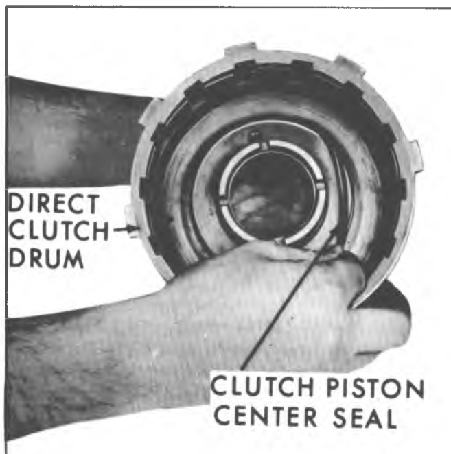
Fig. 7A-77B--Removing Direct Clutch Piston Center Seal
