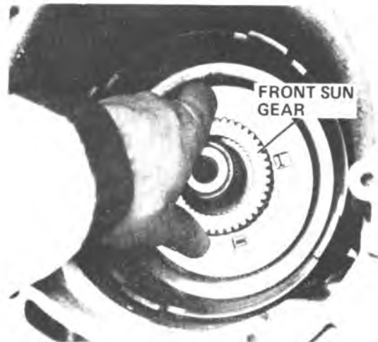
Figure 7A1-102 Installing Front Sun Gear
