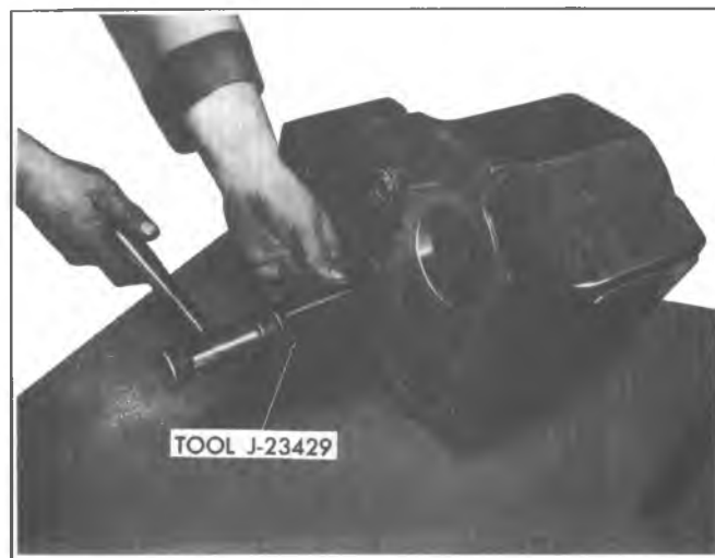
Fig. 7E-8R-Removing Idler Gear Shaft
