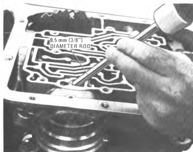
Figure 7A1-29C Installing 3rd Accumulator Check Valve Assy.
