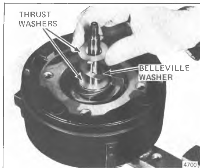
Figure 1D-105 Replacing R-4 Thrust and Belleville Washers
