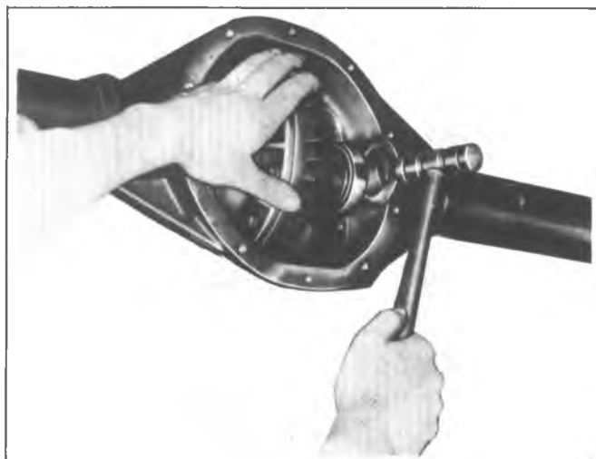
Fig. 9B--Installing Differential Shim
