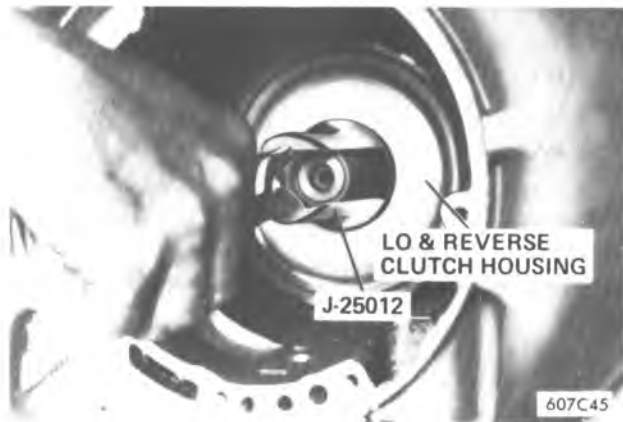
Figure 7A1-97 Installing Low and Reverse Clutch
