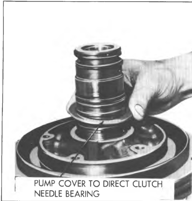
Fig. 7A-108B--Pump Cover to Direct Clutch Torrington Bearing
