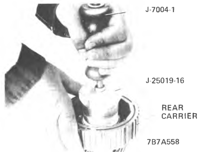
Figure 7A1-197 Removing Rear Carrier Bushing
