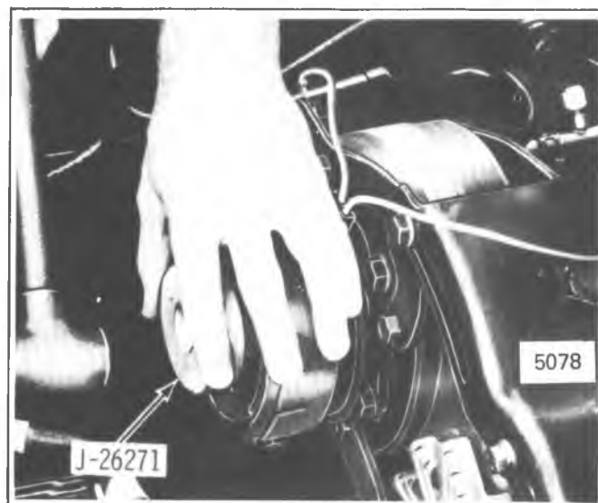
Figure 1D-87 Installing R-4 Rotor and Bearing Assembly (On Car)
