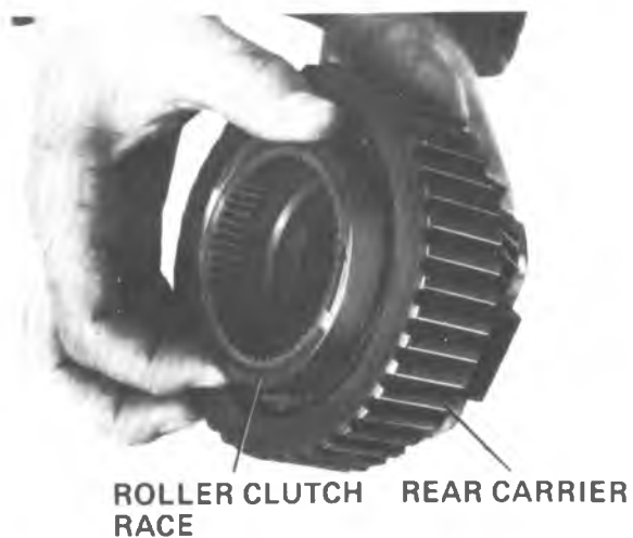
Figure 7A1-82 Installing Roller Clutch Race
