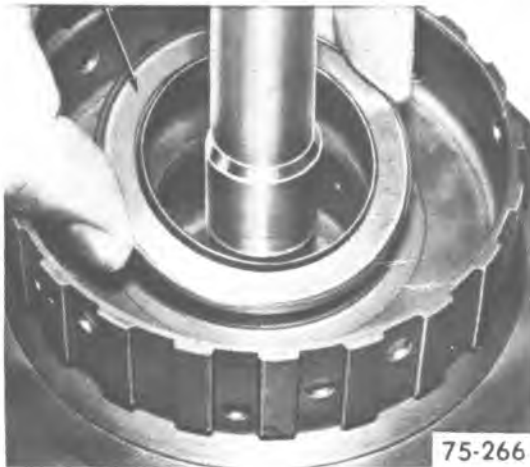
Figure 7A5-61 Direct Clutch Drum to Forward Clutch Housing Needle Bearings
