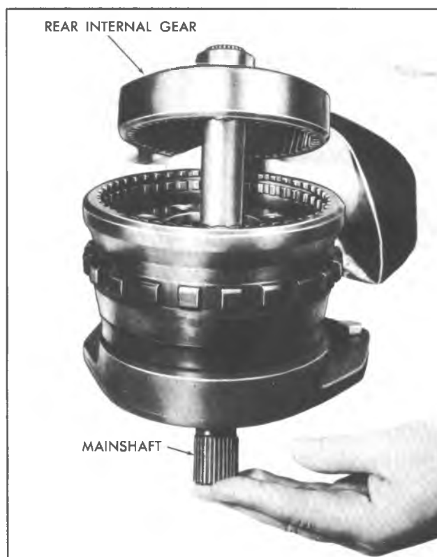
Fig. 7A-51C--Removing Rear Internal Gear and Mainshaft
