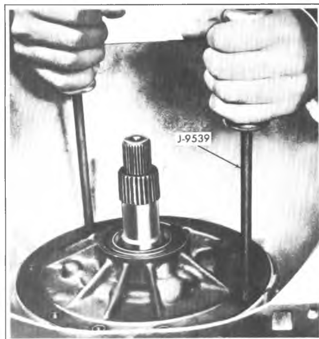
Fig. 7A-32C--Removing Pump Assembly
