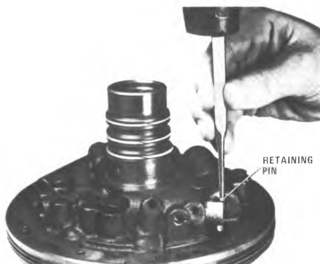
Figure 7A1-150B Install Retaining Pin
