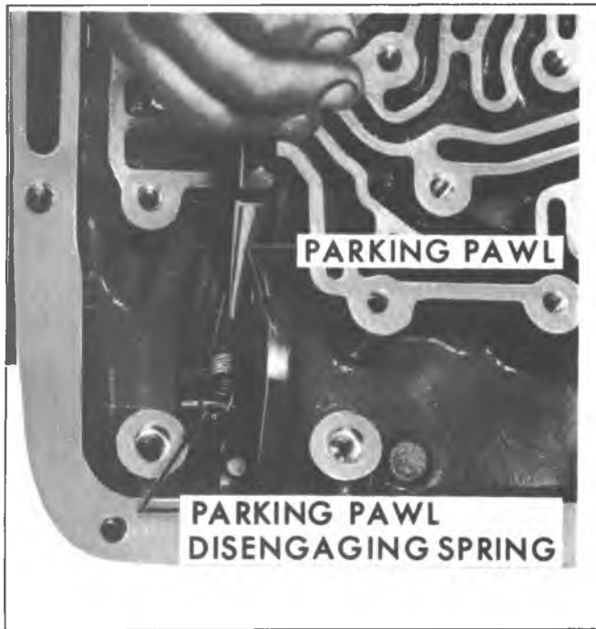
Fig. 7A-26B--Removing Parking Pawl Disengaging Spring
