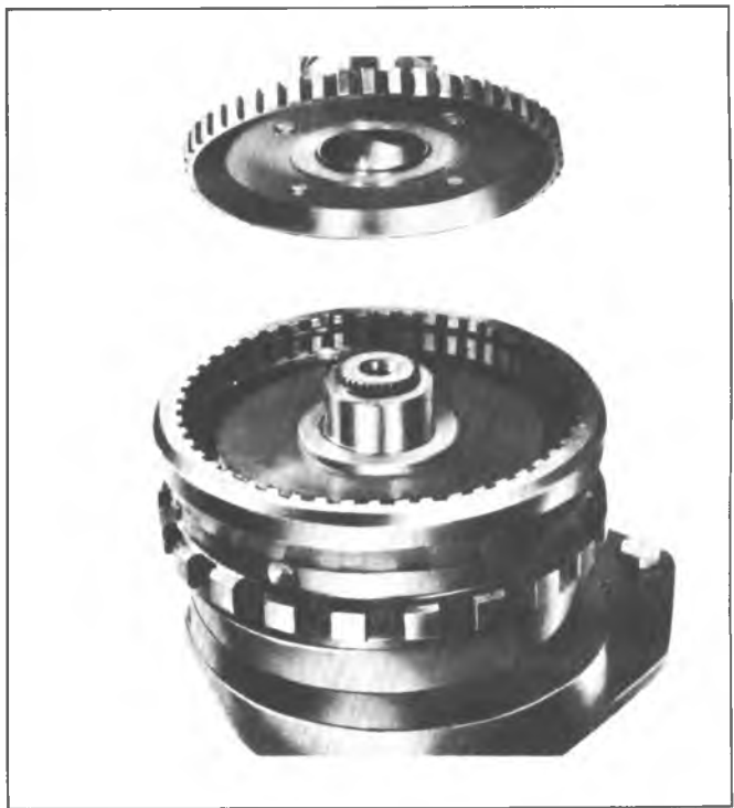
Fig. 7A-145C--Installing Output Shaft
