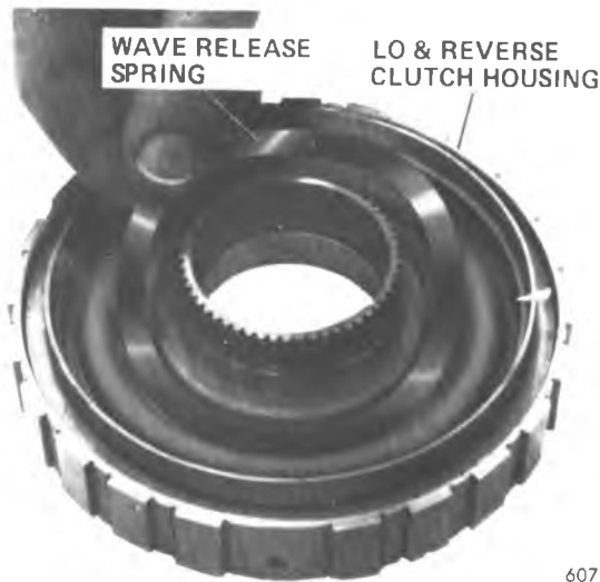
Figure 7A1-93 Installing Lo and Reverse Clutch Wave Release Spring
