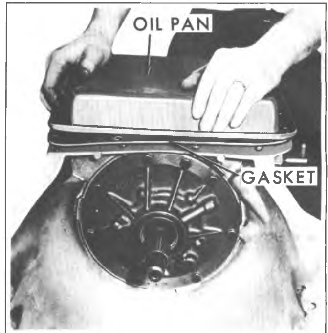
Fig. 7A-12B--Removing Transmission Oil Pan
