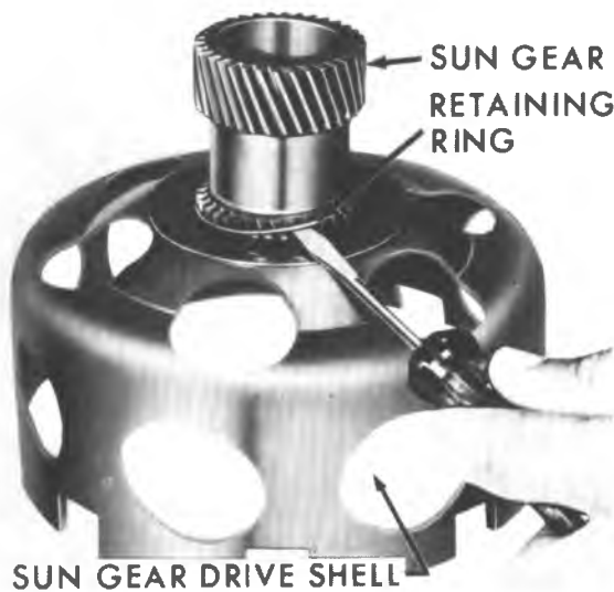
Figure 7A5-70 Removing Sun Gear Drive Shell Rear
