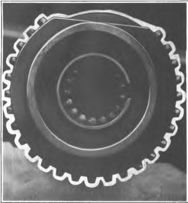
Fig. 7B-12L—Pilot Roller Bearing Installed
