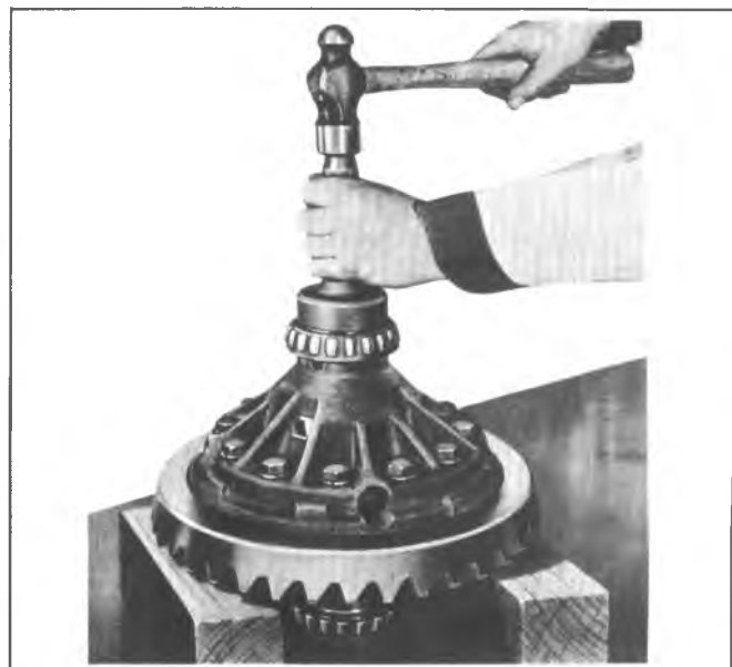
Fig. 5E-Differential Bearing Installation
