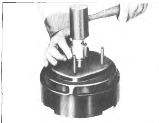
Fig. 5-6B--Removing Rear Seal
