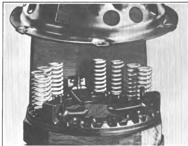
Fig. 7C-10E-Assembling Cover and Pressure Plate
