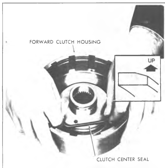
Fig. 7A-85C--Removing Forward Clutch Center Seal
