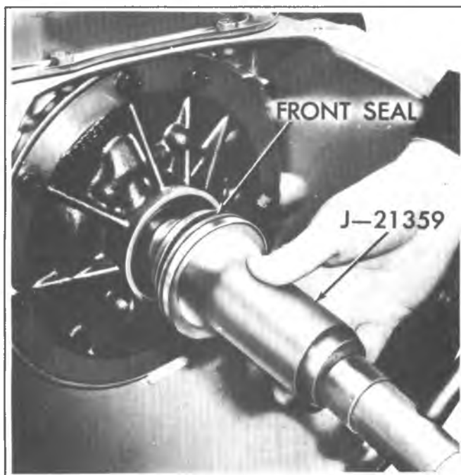
Fig. 7A-168C--Installing Pump Seal
