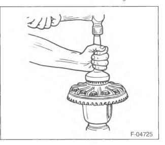
Figure 78—Installing the Differential Bearings
