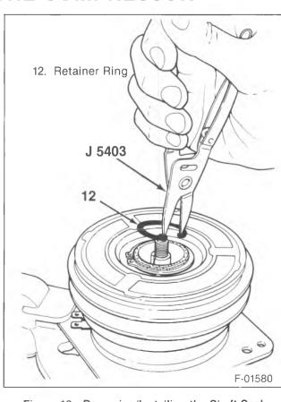
Figure 13—Removing/Installing the Shaft Seal Retaining Ring
