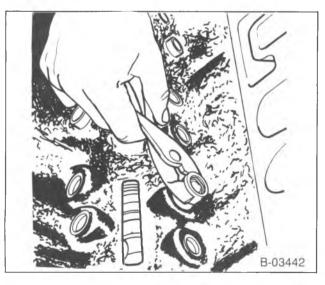
Figure 10—Removing the Hydraulic Lifter with J 3049
