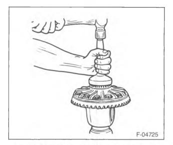
Figure 38-Installing the Differential Bearings
