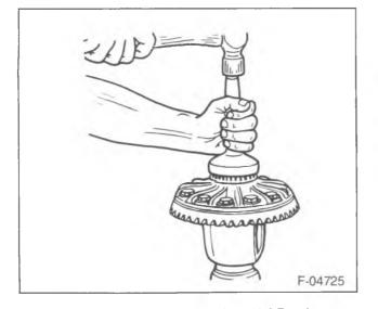
Figure 37—Installing the Differential Bearings
