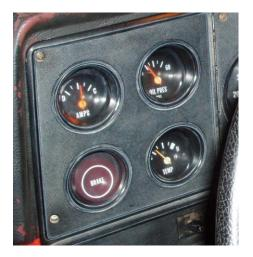
You will need to find a newer replacement voltage gauge that will physically fit inside of the older cluster in place of the ammeter. We were told that '76-'90 clusters have volt gauges, so we made a trip to the local Pick-N-Pull to look for GM clusters. We found that '90 clusters are very different and that the '90 volt gauge will not fit. Then we found a '77 cluster with a voltage gauge that will fit.
