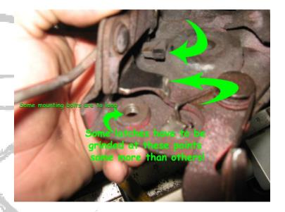
• Some Doors will require grinding the front inside hump so that the glass can clear: (see Below)
