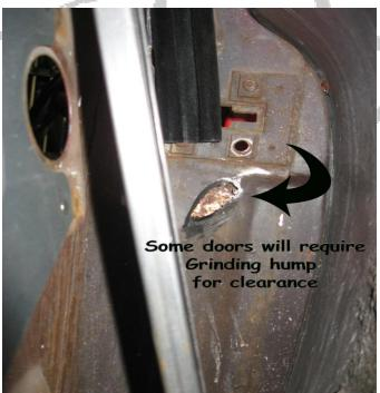
• Most doors will most likely need to <u>scrape</u> the rubber material sprayed on by the factory DIRECTLY under the area where the Roller Brackets that are glued to the glass meets the INSIDE door skin:
