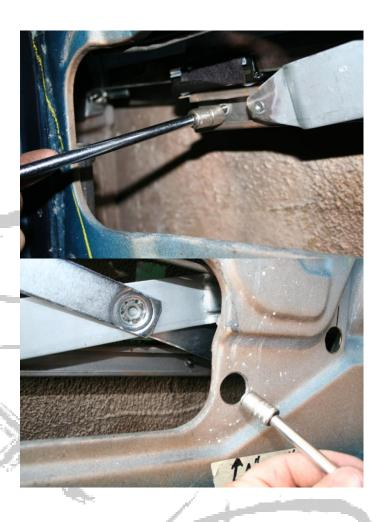
Roll the New Door Glass all the way to the top with some help because <u>REMEMBER</u> it does not have the Main Vertical Channel bolted on.
