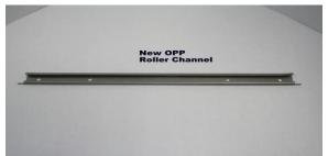
Roller Channel (Used to replace the old roller channel, has two holes one on each end including fold down tabs.) Mounts between door glass brackets and the rollers on the regulator.
