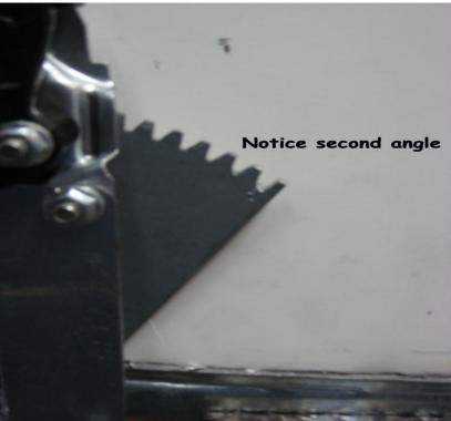
Simply BEND the last tooth away from the motor, that tooth will stop on the bracket oposite the motor:
