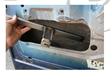
Slide in the side with the bigger mounting bracket first.
