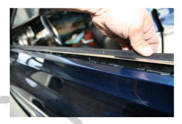
With the window in the down position, push the new scraper down to the edge of the door. The weatherstrip adhesive will dry in roughly 15-20 minutes.
