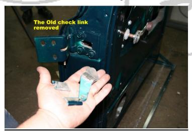
Here is the Old check link completely removed.
