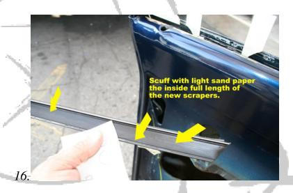
Before installing make sure to scuff the inside part of the scraper. **Scuff** the shiny part **NOT** the felted part.
