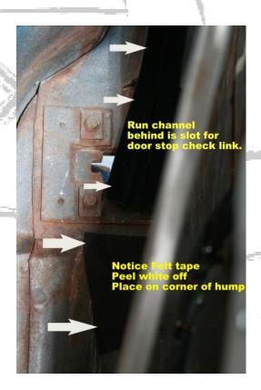
13. This is an inside view of the door looking at the inside upper hinge bolts, and the slot left from removing the
