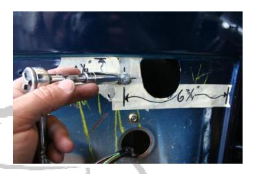
the glass slide into the New Vertical channel and push up so the nut on the new bracket meets with the New hole made on the door and bolt it ON. Take note that on getting the new rollers to slide into the new channel, you will need to wiggle the bracket a little bit so it may pass the shape of the door from the inside.
