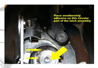
Use the weatherstrip adhesive provided and put a moderate amount on the circular part of the latch assembly, Give it about a minute to start becoming tacky and press the New Run channel firmly on the glued area until it has fully dried, Which should roughly take about 5 Minutes
