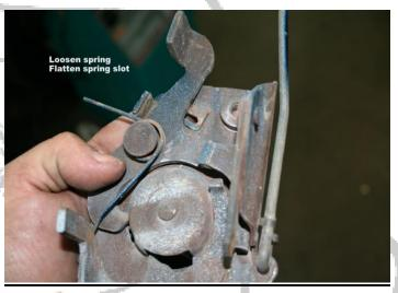
Locate the top of the latch assembly; you will need to bend flat the slot where the latch spring is. You will also need to give the old spring a 90 degree elbow for the new location of the same spring. Refer to pictures provided.
