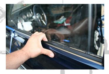
Make sure the new scraper sits flush to the inside edge of the door were the glue was applied. Slide you hand along the scraper to make sure the scraper make full contact to the lip of the door skin.
