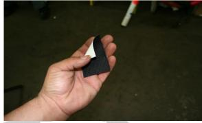
Felt tape. Used on preventing front edge of glass on scraping the inside of the skin of the sheet metal. Place on the corner of the inside hump. Quantity (2 pieces)
