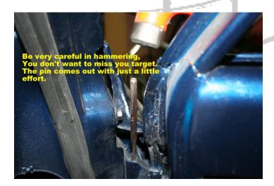
8. Take you thin center punch and hammer down the pin that holds your check link in place. Hit it down until the check link clears away from the pin. Slide the old Check Link inside the door and remove it. Be extremely careful at this point, The Door can swing open and damage your door on the outside of the skin. You kinda don't want that!!
