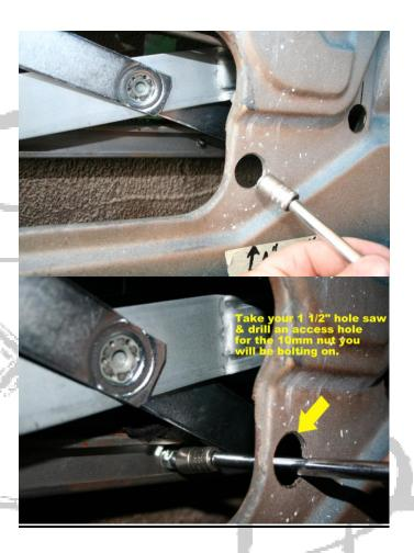
11. **Take your 1 ½" Hole Saw and Drill** yourself an access hole for the 10mm nut you will be bolting on.
