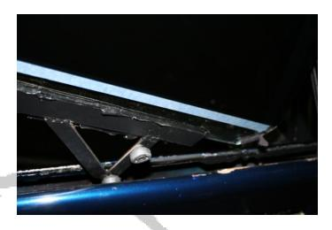
14. Tape the edge of the body with masking tape so you won't scratch the paint or the glass, but since I am a professional I just do it carefully. Bring it in on a angle to make the install easier. Once inside, attach the two 10mm nuts that are provided in the kit and tighten them up. You may have to push the glass towards the outside so it can pass the inside hump with the new felt.
