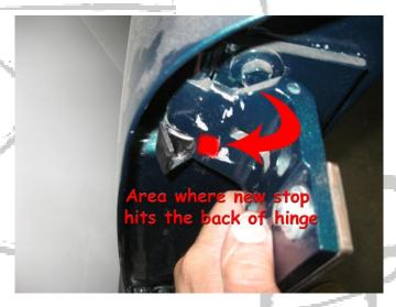
The red square is the contact area of the hinge where it hits the new bracket. (Felt this area or the bracket itself.)
