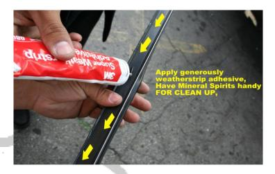
Apply the Glue and place it in between the glass and the inner or outer door skin, which ever one you are working on.
