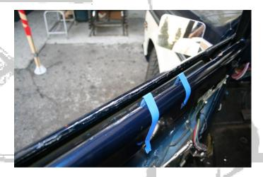
**Tape the glass** to the side you are not installing the new scraper on. This will give you a little more clearance.
