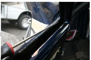
4. Use a long flat screw driver to wedge the new run channel all the way into its slot.
