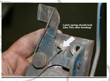
Take note of the 90 degree angle on the spring and how the slot is flush now. (This needs to be done because the glass will need to pass very close to this Latch assembly.)
