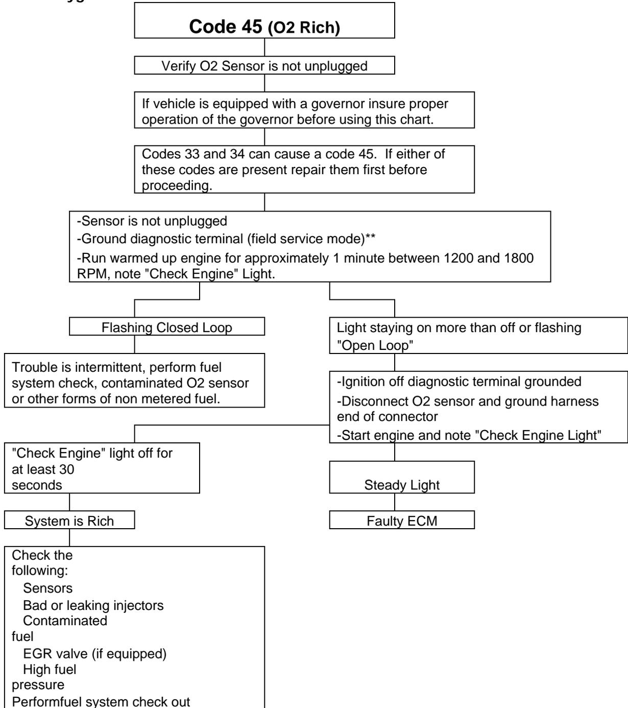
\*\* Service diagnostic mode is entered the same as Engine Off Self Test. Ground out Pin A and B on the ALDL connector with the engine running. Rapid flashing (approx 1/2 - 1 sec interval) is open loop. Flashing at a slower rate indicates closed loop.
