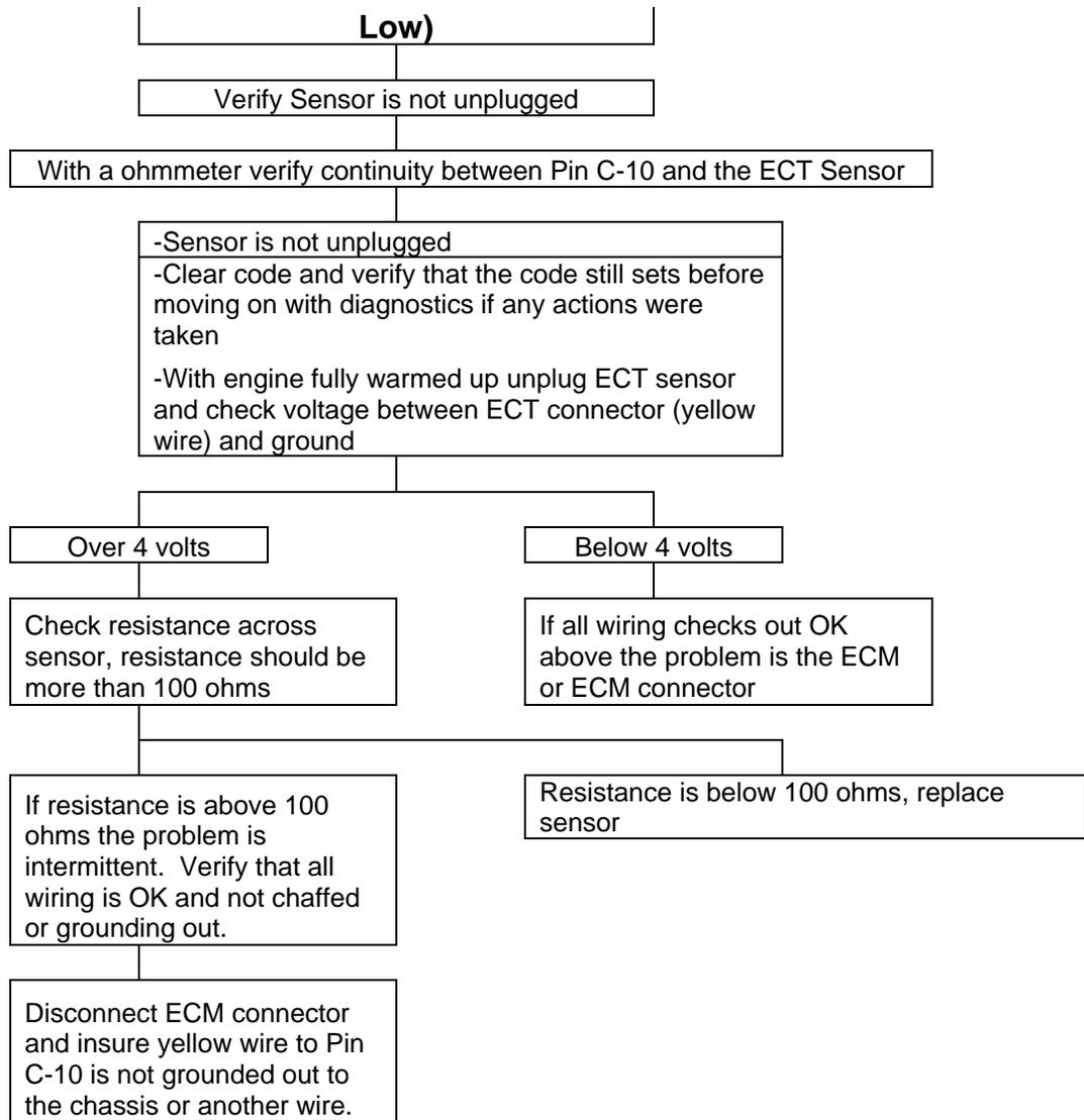
**15. Low temperature indicated at engine coolant temp. sensor**
