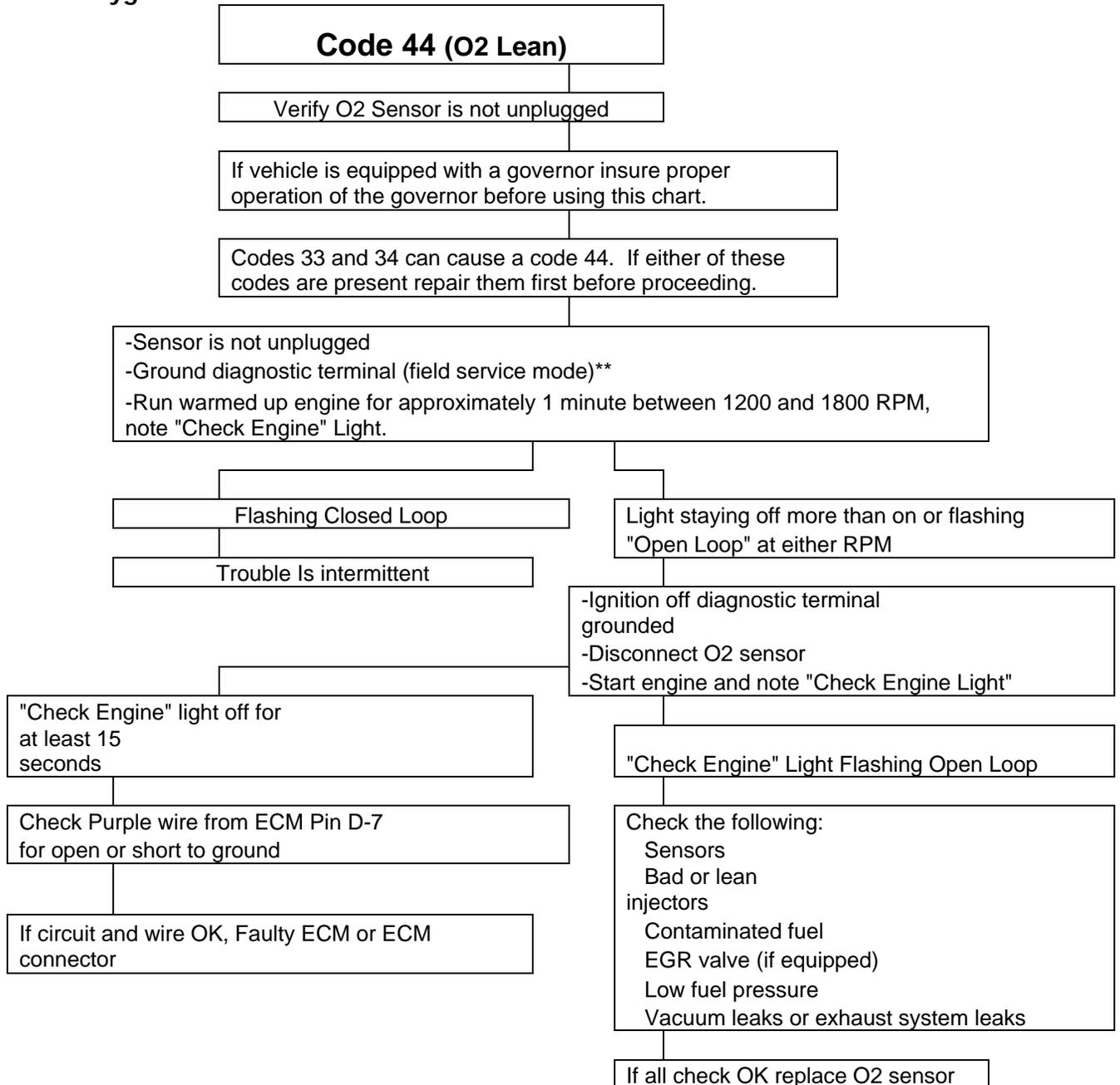
\*\* Service diagnostic mode is entered the same as Engine Off Self Test. Ground out Pin A and B
